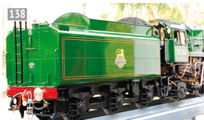
The tender tank is held onto the frames by just four central 2BA studs. The brackets where it meets the buffer beam are dummy.
