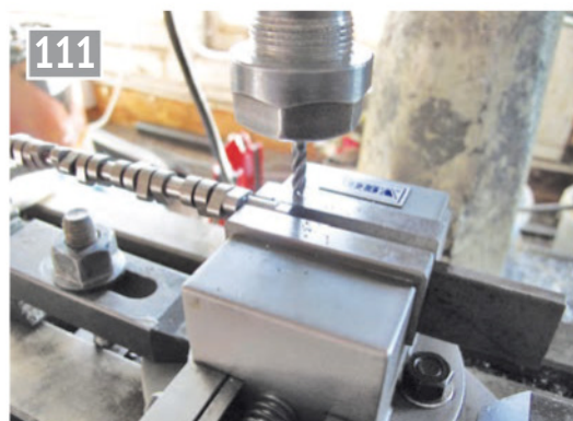
111 Machining the first grub screw locating flat.
