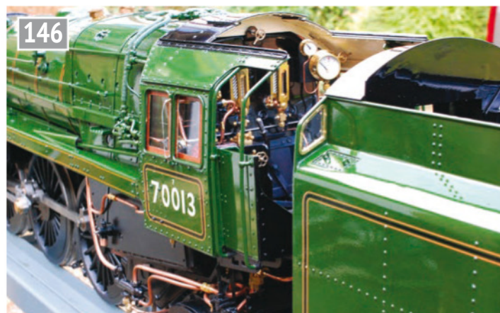
It looks nice, but there are some problems here with tender and cab alignment caused by the boiler height and an over-long drawbar.
