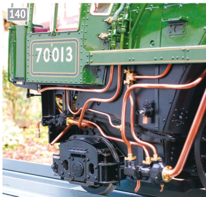
The tender tank is held onto the frames by just four central 2BA studs. The brackets where it meets the buffer beam are dummy.
