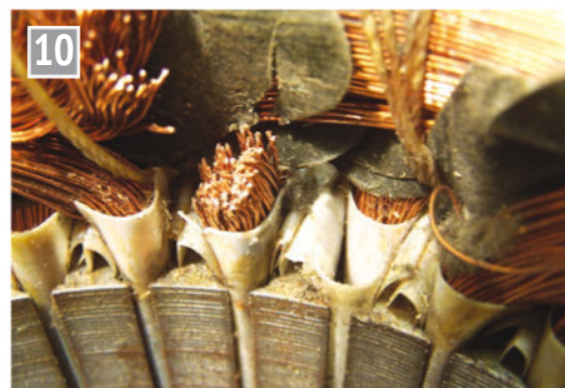
The wires cut off for ease of removal.
