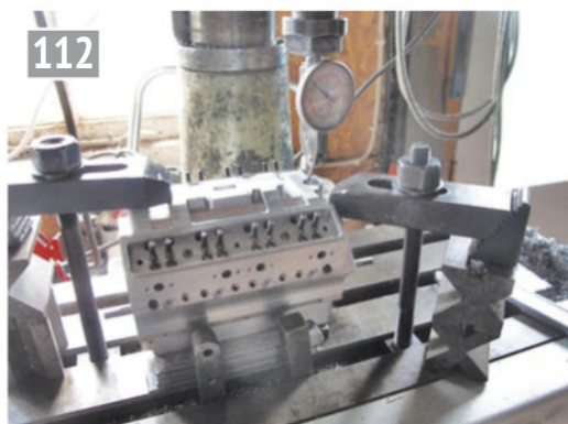
112 Setting the manifold bore true to the machine spindle.
