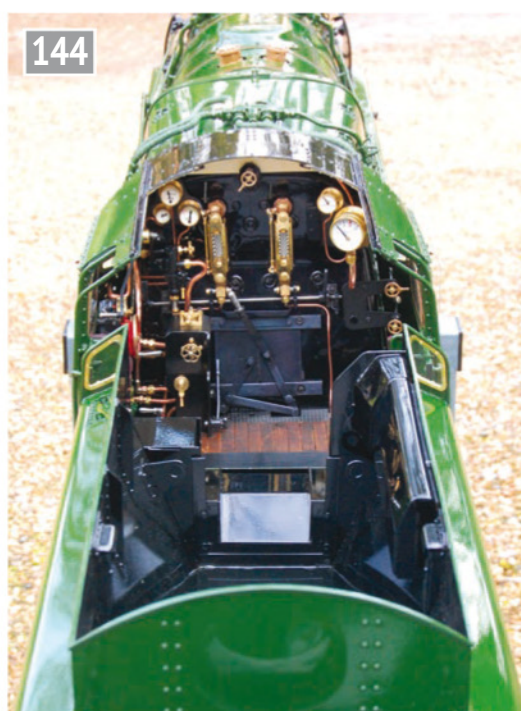
LEFT: This is a driver's eye view. There is easy cab access with the large tender bulkhead insert removed. The tool tunnel adds interest, without getting in the way. The footrests are on the tender which means that I can work all the controls by hand, but a small handle makes operating the reverser much easier.
