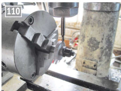
110 Centring the two M3 holes in the timing gear.
