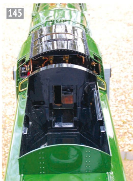
LEFT: This is a driver's eye view. There is easy cab access with the large tender bulkhead insert removed. The tool tunnel adds interest, without getting in the way. The footrests are on the tender which means that I can work all the controls by hand, but a small handle makes operating the reverser much easier.
