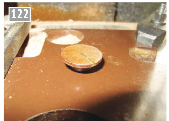
The finished rotor.
