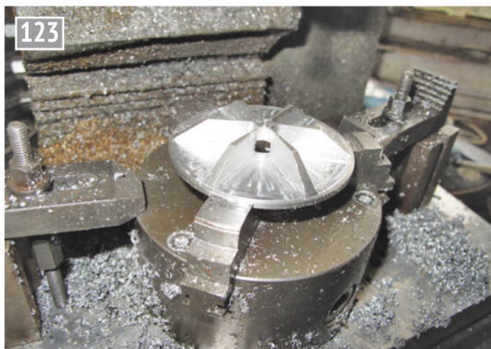
The air scrubber pockets.
