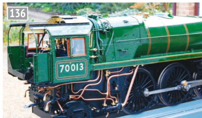
In their day, Britannias would have had all the pipework below the running plate painted black. I have taken a small 'builder's liberty' by leaving it in bare copper, just as the full size engine is today.
