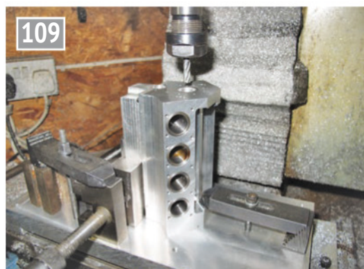
109 Crankcase assembly set to machine timing gear pockets.
