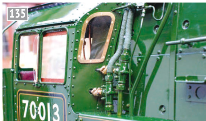
The window frames are made from two sections of brass held together with 14BA CSK screws. 1mm thick glass is sandwiched between the two frames. The sliding side windows are also glass and edged with mahogany laminate.
