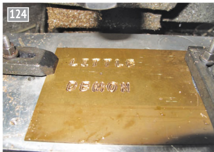
Engraving air scrubber cover plate.
