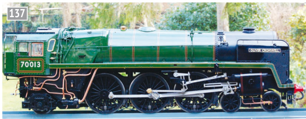
A characteristic of a BR Class 7 is the boiler line rising to join the firebox, then falling before meeting the cab.
