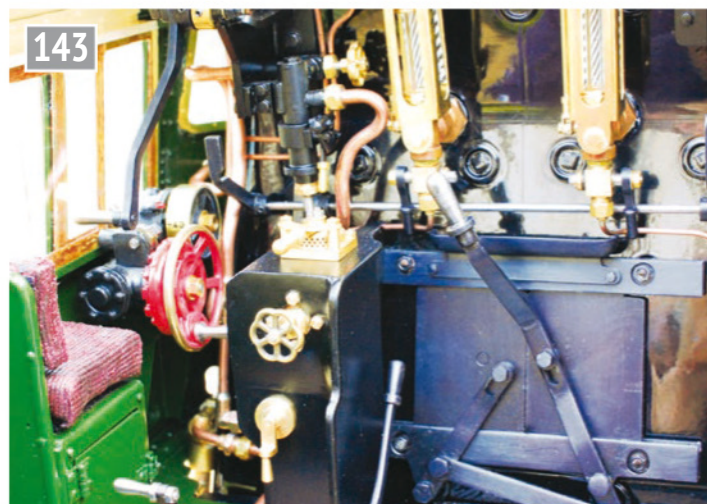
The firebox doors have been 'chemically black' treated. Britannias did not have red reverser handwheels, although some 9Fs did.
