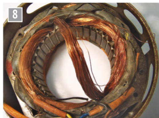
The windings from one slot separated from the rest.
