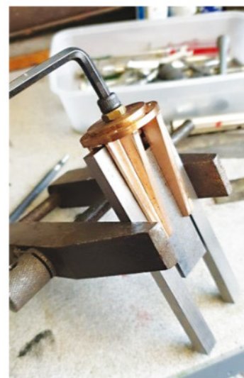
6. Here is the jig used for silver soldering the guides to the covers. A tool clamp is used along with some packing to hold the guides tightly against the steel block. The cap screw which is attached to the steel block and goes through the gland nut (just as the valve spindle would) is tightened to pull the two sides up close against the cover. Before this is fully tightened I brush on some flux around the mating surfaces to help with penetration and then tighten fully, being sure that the cover is aligned correctly to the guides.
