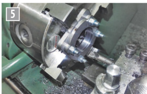
Machining the axle box plates.
