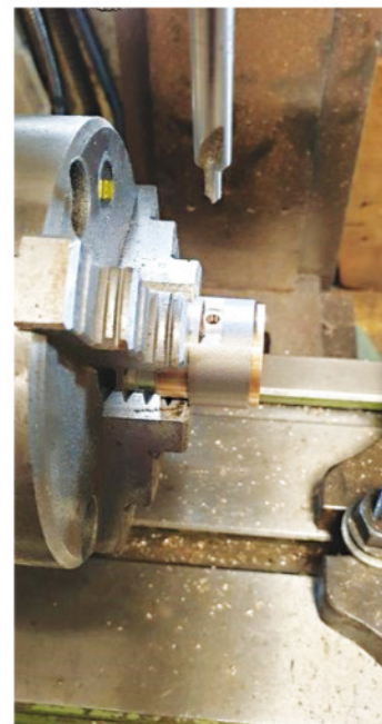
LEFT: 16. Setting up the first liner. I first needed to be able to find the centre for the port on the 'X' axis ('Y' was already set via the rotary table centre). As the port is very small and not so easy to clock I decided to turn up a peg that fits into the port. The peg is stepped to allow clearance from the chuck. I only needed to do this once, with the rotary table dial set at 0 and locked on the mill table and the DRO also set at 0 for both X and Y I don't need to use the peg again as the thimble seen in the picture sets each liner in its correct position for this operation. RIGHT: 17. Centre drilling the liner for the first port hole - here I used a long centre drill and the rotary table is set to 0 degrees.
