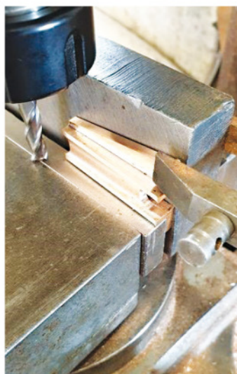
5. The last operation was the shallow angle along the side of the guide. I used some steel to give support behind.
