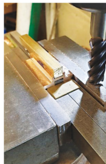
2. The top slot is similarly bridged to avoid distortion while the slot sides are cut.
