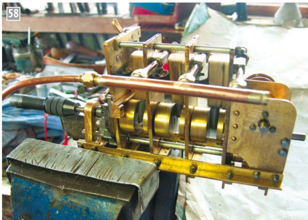
The author's engine running on compressed air with very little vibration. The whirring image on the left is the handle of the pin vice used for assembly.
