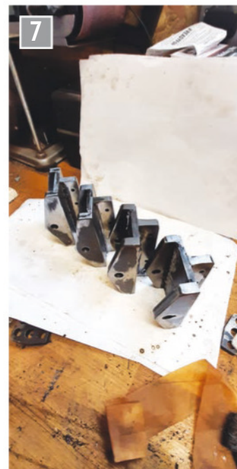
Completed fabricated brackets.
