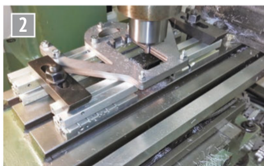
Cleaning up the sides of the 'W' frames.
