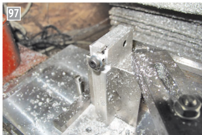
Holding arrangement to produce the roller slot.
