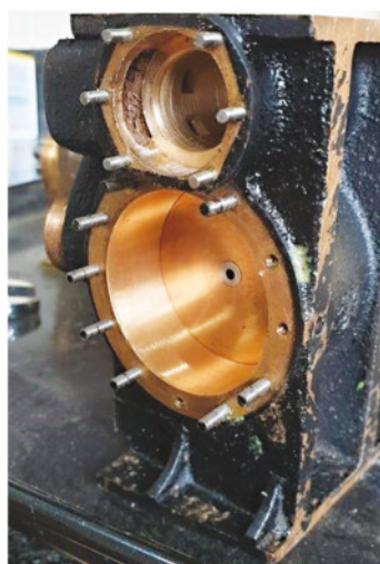
20. A trial fit with the middle cylinder front liner. I was happy that the liner stopped fully against its lip.
