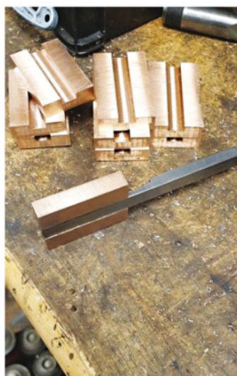
1. Bronze blank machined to size with a bridging piece fitted to avoid distortion while the slot sides are cut.
