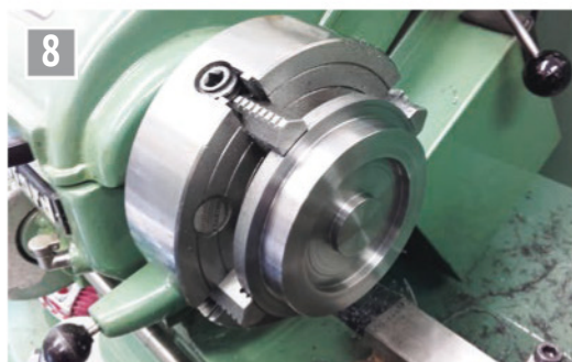
Wheel blank machining in progress.
