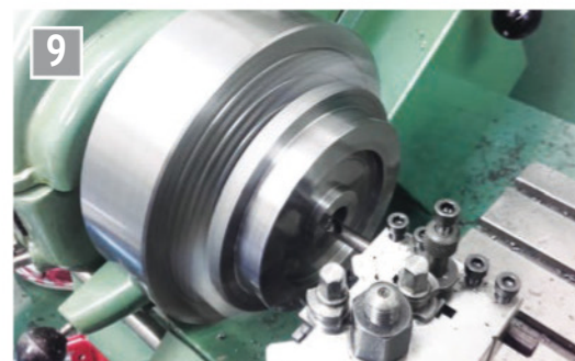
A light cut to finish the wheel bore to size.
