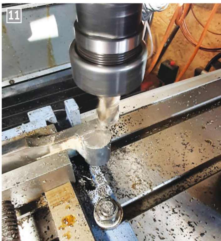
Milling the bar frame during fabrication.
