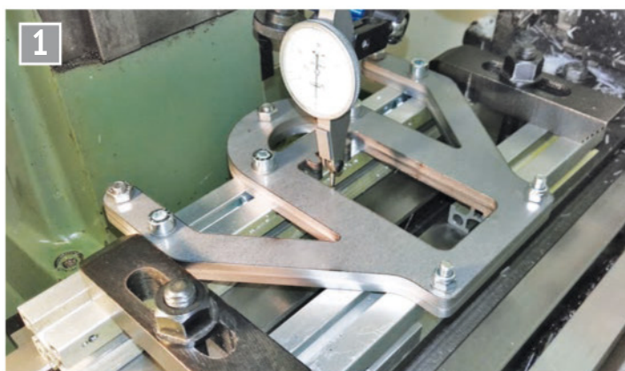
'W' frame mill setup clocked.
