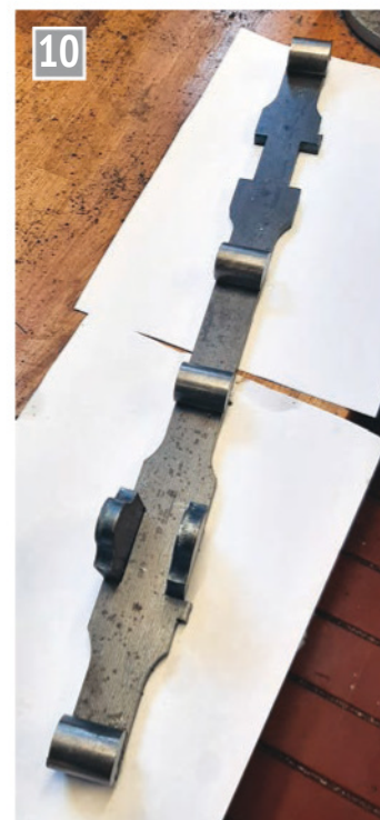
Bar-frame being fabricated.
