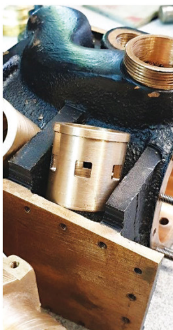
18. This is the first liner with its ports completed apart from a final polish and ream. I am not going to square off the corners, preferring to leave the radius as it guarantees that all six ports and liners will be identical.
