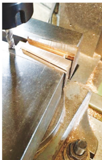
4. Machining the angles along the top and bottom of the guide using a swivelling machine vice.
