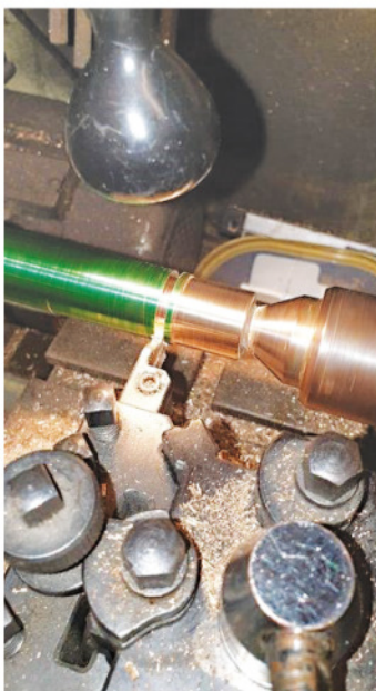
12. I then set about profiling each liner, drilling \frac{3}{8} through each and parting off. Before parting off each lip diameter was checked to be a 'rattling' fit into each cylinder recess.
