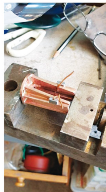
10. Oil pots secured in position, ready for soft soldering to the crosshead guides.
