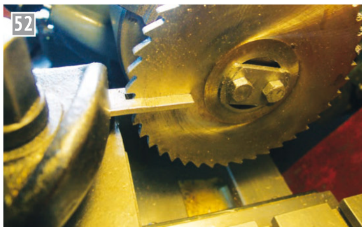
Here the piece of stainless strip is being cut to width; note the thinner section which will act as the spacer for the assembly.
