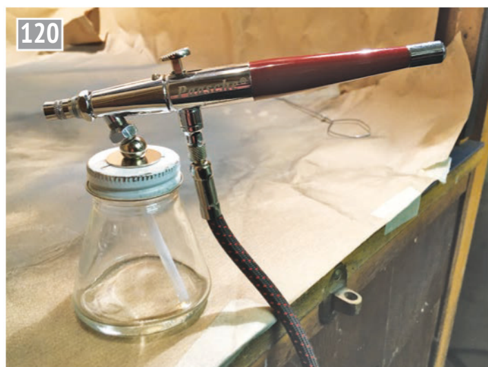
The 'upmarket' airbrush that did all the spraying. A Paasche VL Series with 'double-action' trigger, optional 90ml paint bottle and a range of nozzle+needle pairs.
