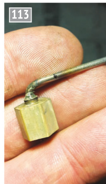
The handle soldered and bent.
