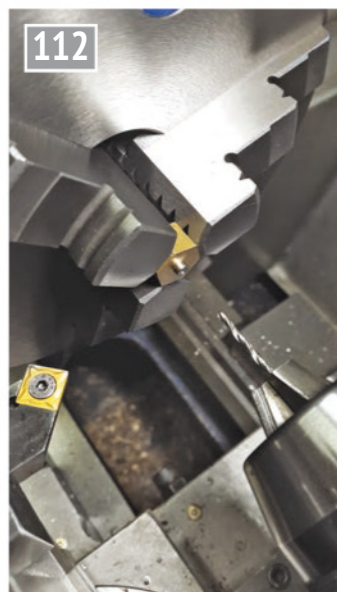
Drilling the hole for soldering the handle.
