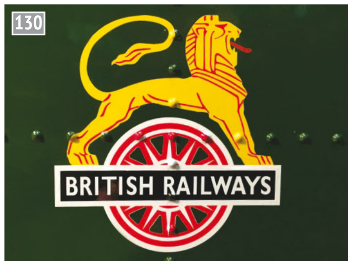
The tender emblem also had all its rivet holes cut with the 1.5mm punch. Then the artwork was touched up with enamel paints and very small brushes.
