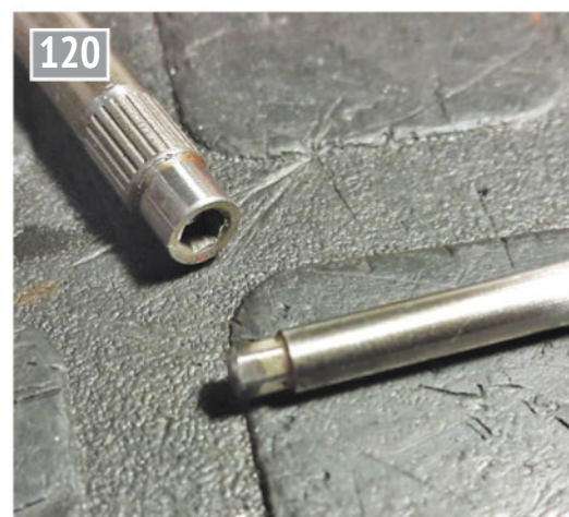
Blowdown valve spindle and box spanner.
