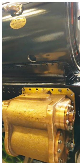
16. Holes in the smokebox for the steam pipes line up nicely with the cylinders.
