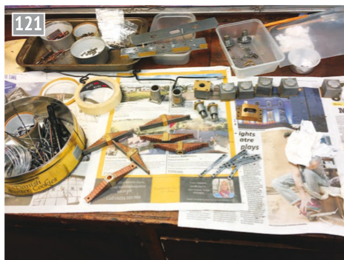
The reality of painting – lots of parts to be cleaned and then hung on wires or arranged on jigs for spraying.
