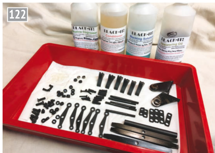
An alternative to painting small parts. 'Black-It' solutions give a smart appearance to steel, but it is not a corrosion protector.
