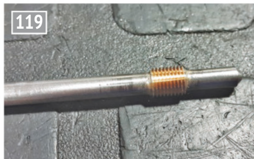
119 Blowdown valve spindle machined.
