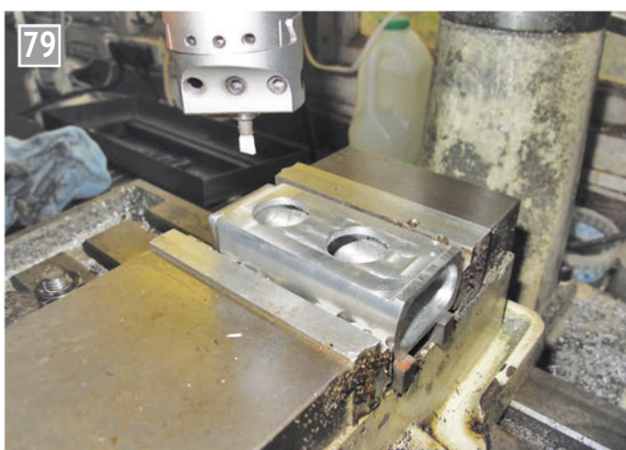
Milling out the carburettor location bores.
