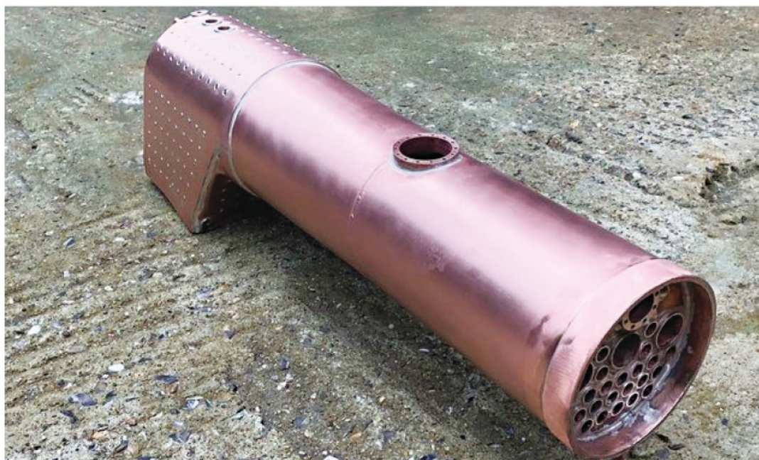
9. The completed boiler.
