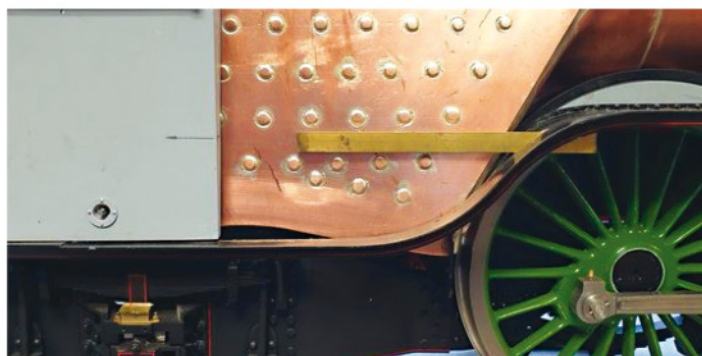
14. Lining up the slot in the running board for the reverser.
