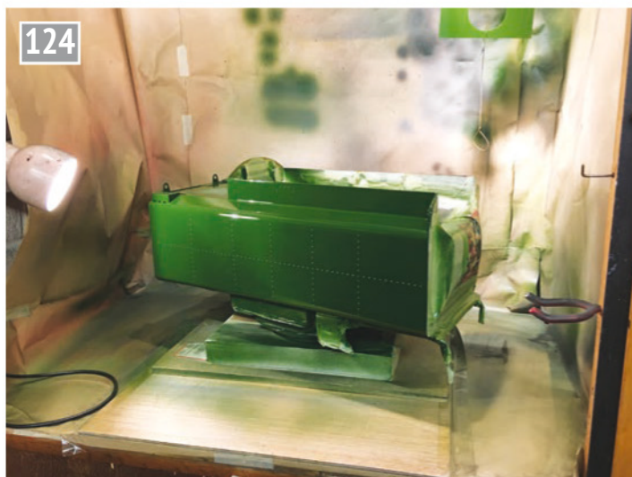
The tender is supported on a turntable to enable spraying of all sides while the fumes are carried up and out by the extraction fan. The close spotlight allows you to see a reflection while spraying so that just enough paint is applied to fully wet the surface.
