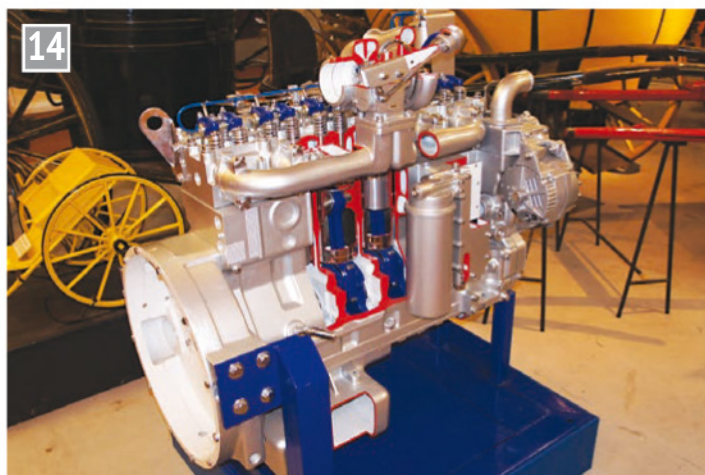
14 Cummins Turbo Technologies Ltd. (formerly Holset Engineering) made components for this Series C engine used in a Dennis fire engine. It was sectioned by John Bywater helped by his brother, Peter and David Charlesworth. A six cylinder engine of 8.3 litres capacity.
