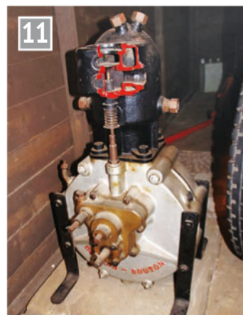
De Dion Bouton engine; one of many imported from France.
