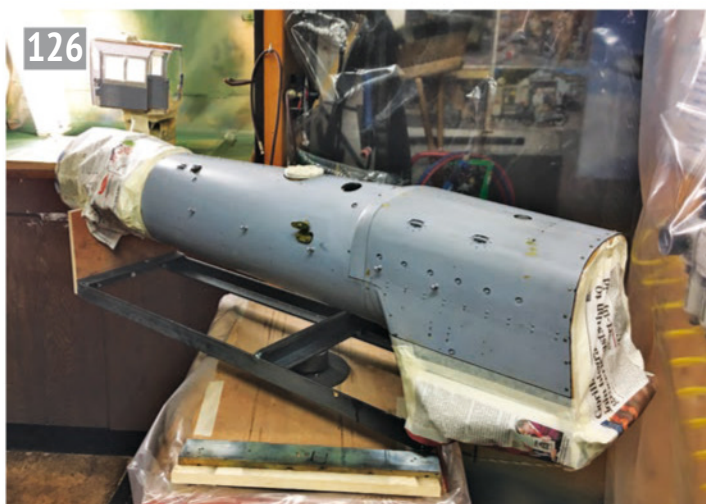
That is a big and heavy boiler. It was lifted by an engine crane onto a welded cradle that sits on a ball bearing, which is bolted to the red metal cabinet. The cabinet has castors underneath. The edges of the workshop have been covered with clear PVC sheet making, in effect, a bigger spray cabinet.
