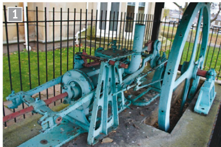
The Fieldhouse winding engine, an unusual design from around 1850, preserved thanks to the initiative of Model Engineer reader, Bill Stocks.
