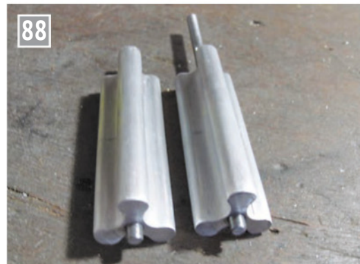
Rotors with high spots removed.
