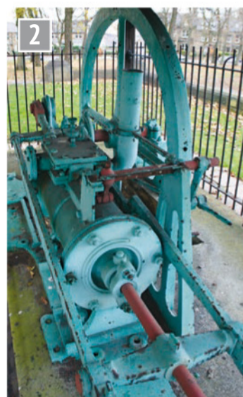
The unusual layout of the Fieldhouse engine resembles a table engine laid horizontal.
