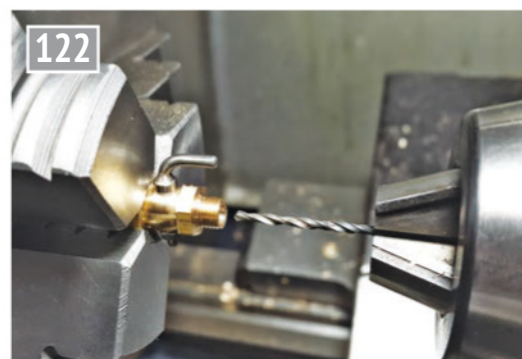
Drilling through the spindle.
