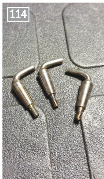
114 Some taper spindles ready for fitment and cross drilling.
