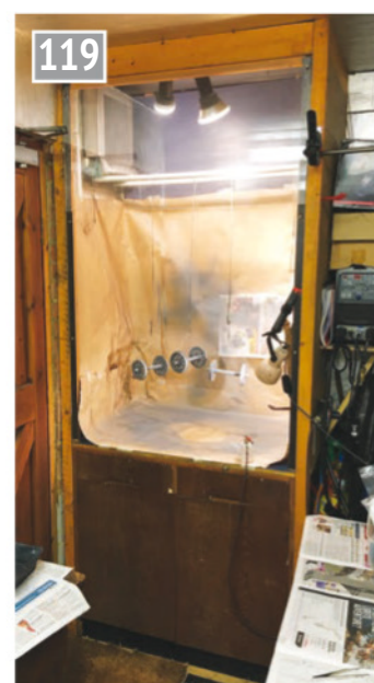
For paint spraying some fume extraction is essential. This is a fume cupboard that anyone can build in a reasonably sized workshop. Sited in a corner, wooden framing on top of a cupboard, perspex hung on screws to make the windows and a large 10 inch Ventaxia fan at the top. Items for painting hang by wires from bars above, with fishing line swivels added to enable rotation.
