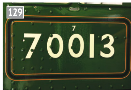
Each transfer has to be marked for the rivet position and then a hole cut with a small 1.5mm punch.
