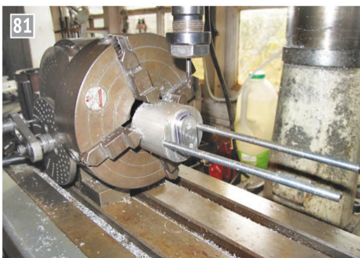
The work is transferred to the dividing head.
