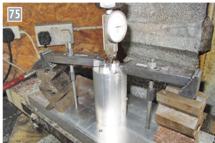
Setting the scoop square for machining the channel.
