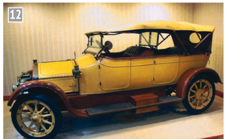
The Vulcan had a two stroke engine of 3888cc generating 25 hp. This car was brought back from South Africa to be restored by David Brown apprentices. It is on loan to the Tolson museum.
