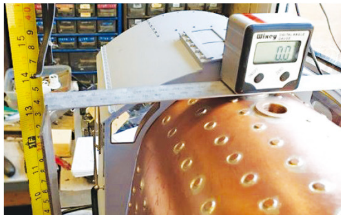
12. Checking the height of the boiler.
