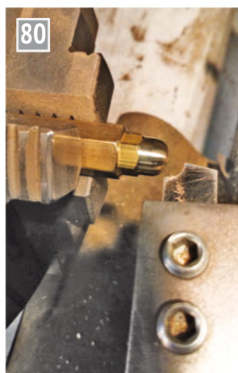
Shaping the ends of the acorn nuts.
