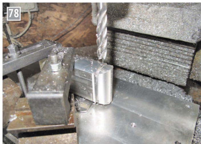
Milling a male spigot to match the channel.
