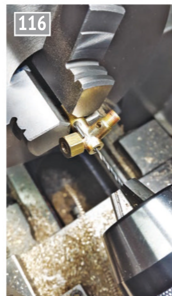
116 Cross drilling the spindle in the assembly.
