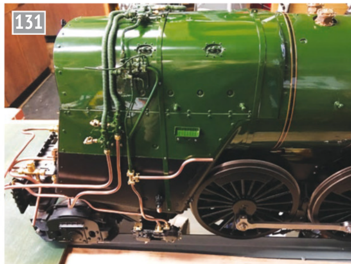
Once painted and lacquered the boiler could be craned back onto the frames. Then all the detail painted parts could be added.
