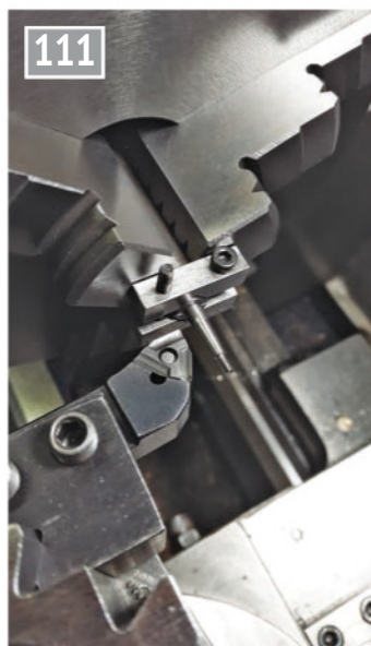
Machining the taper spindle.
