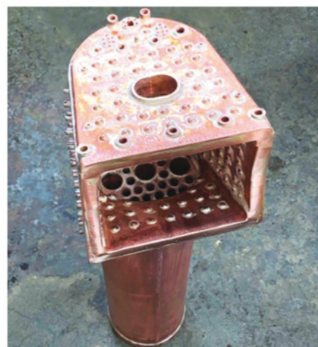
8. Not much left to do – the stay ends will be trimmed, the boiler will be given a good clean and then tested at twice its working pressure for two hours.
