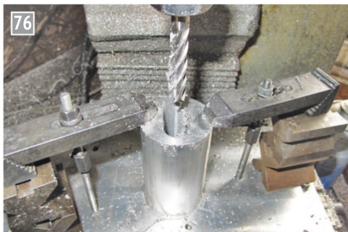
Machining out the sides of the channel.
