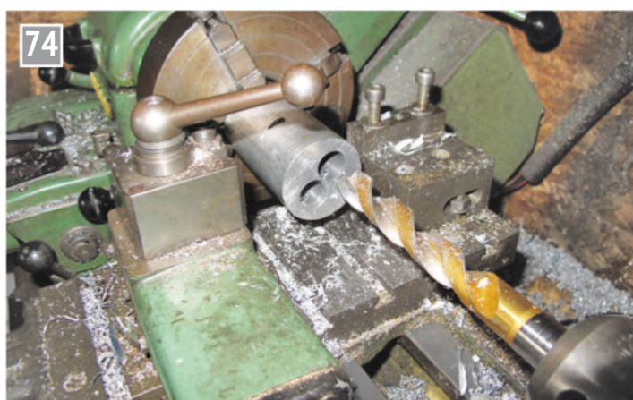
Drilling the channel end radii.
