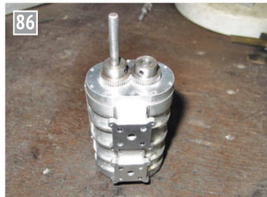
Rotor spindles are installed and gears fitted.
