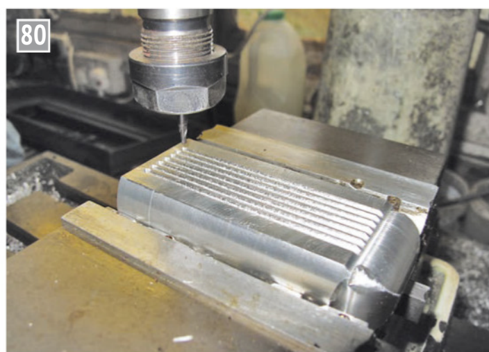
Machining the grooves onto the top face.
