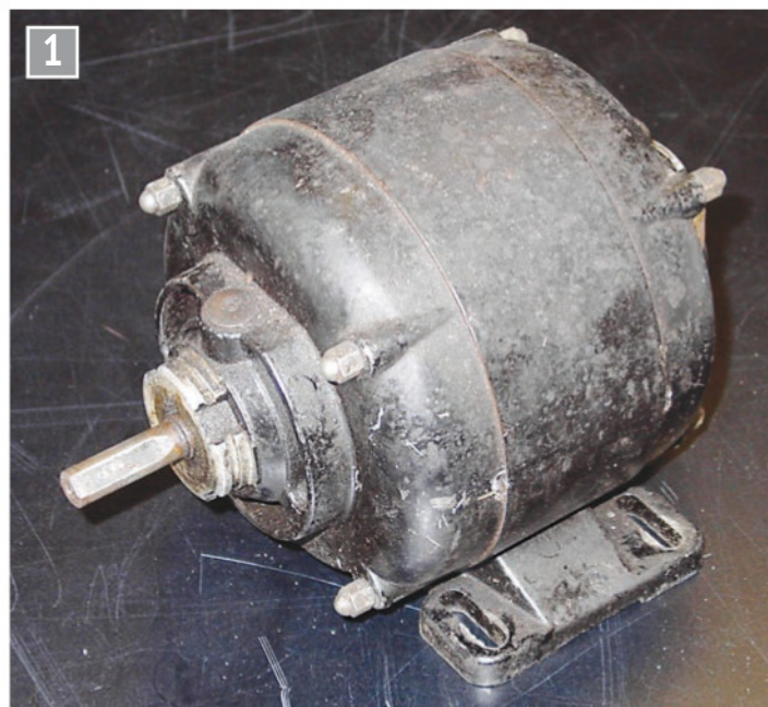
The Metropolitan-Vickers motor similar to the existing lathe motor.
