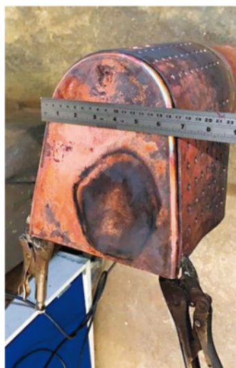
1. Here is the backhead being fitted to the outer wrapper.
