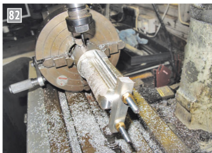
Generating the outside form of the scoop.
