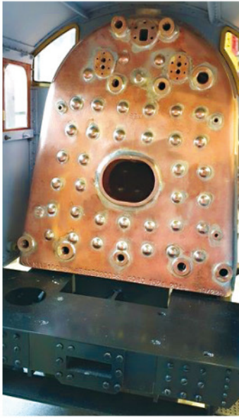
10. Close up of the backhead.
