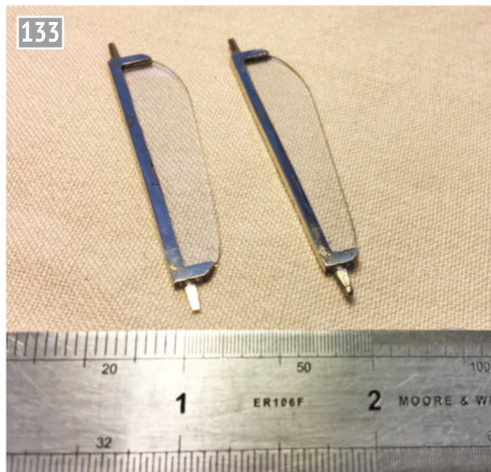
The small cab-side wind deflectors are fitted with 1mm thick glass. After cutting, the curved shape is smoothed under soapy water with 180 grit wet and dry paper.
