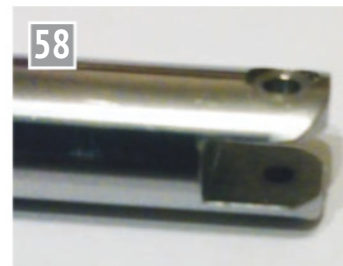
The finished slot.
