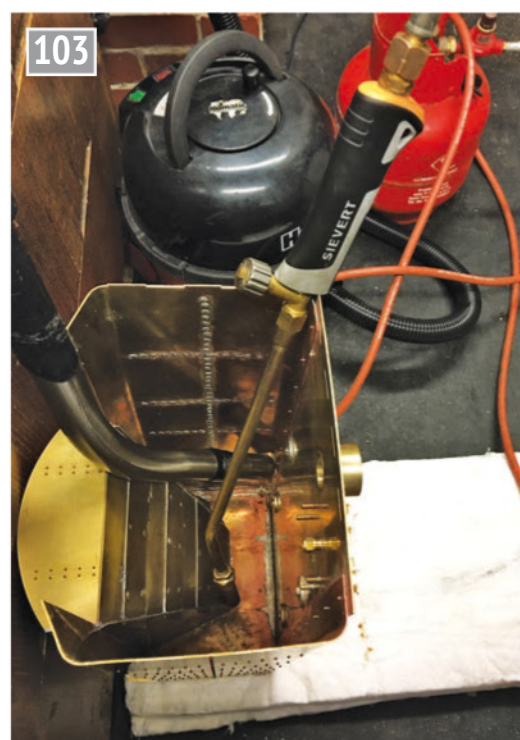
In front is the dummy water level indicator and behind, at the top of the tender side, is the dummy inspection hatch used by shed staff to maintain the water level indicating apparatus. These are not standard kit parts and present a mini-project of their own.
