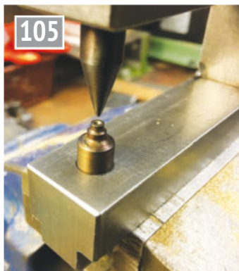
105 The jig frame holds a small round-nosed punch above a recessed die. The punch and die were turned from \frac{3}{8} inch silver steel, then hardened and tempered. When a brass plate is held between and the punch tapped with a hammer, a small dimple is produced.
