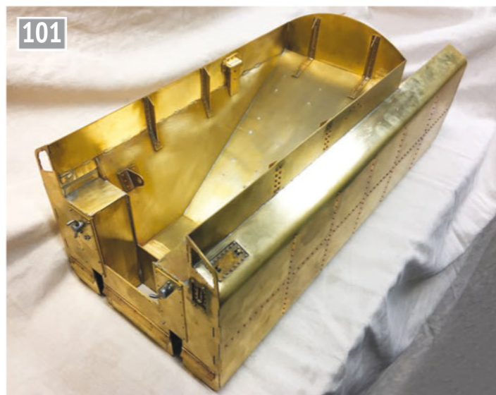
The double-skinned bulkhead was soldered first to the coal chute, then the two sides added and finally to the soleplate.
