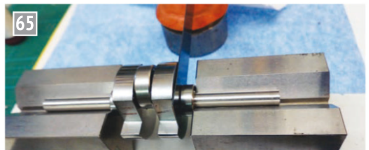
Checking the squareness of the crank.
