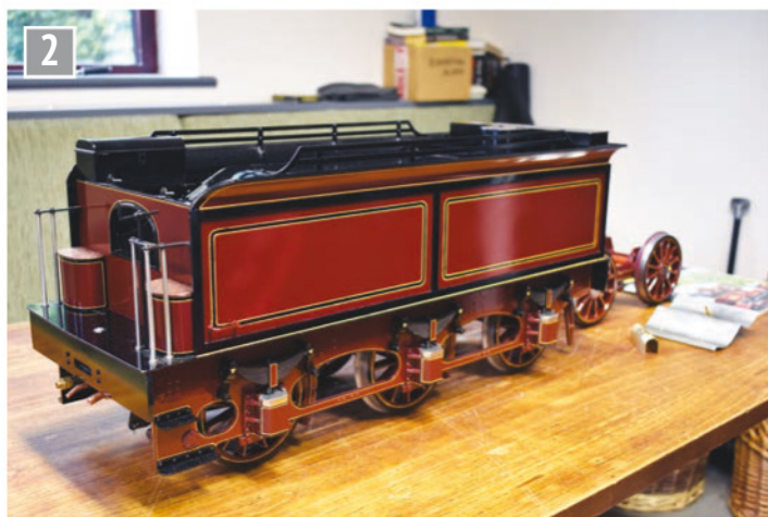
The tender from a Johnson Single in 5 inch gauge being built by Roger Locock.
