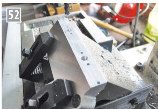
Drilled holes and counterbores.
