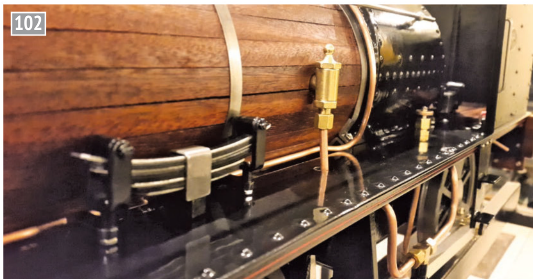
Running boards showing rivets and cut-outs for clack etc.
