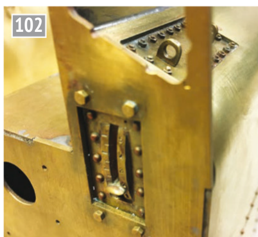
In front is the dummy water level indicator and behind, at the top of the tender side, is the dummy inspection hatch used by shed staff to maintain the water level indicating apparatus. These are not standard kit parts and present a mini-project of their own.
