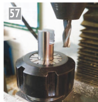
Cutting a slot into the piston.
