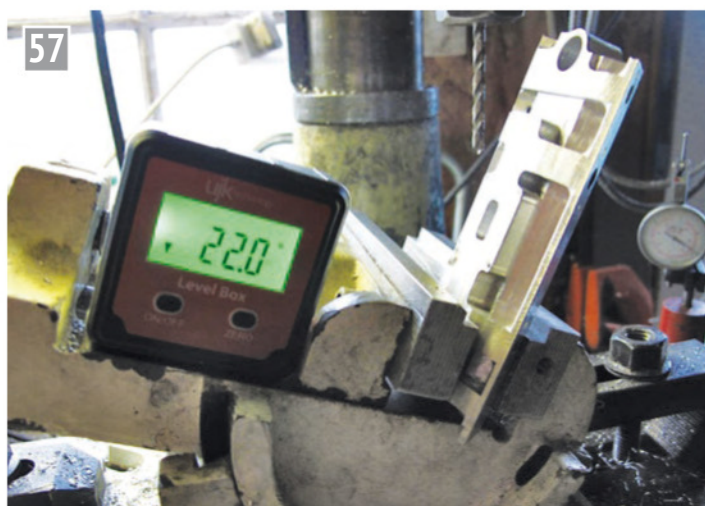
57 Connecting the cross-feed bores to the fuel/air intake pocket.
