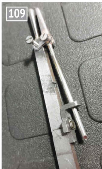
109 Checking for correct sizing on the reversing lever.
