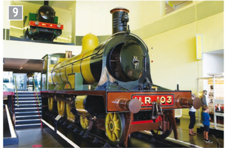
The Highland Railway Jones Goods of 1894 was the first 4-6-0 to run on a British railway and was the most powerful locomotive in Britain at the time. A Glasgow and South Western Railway 0-6-0 tank engine of 1917 is above.
