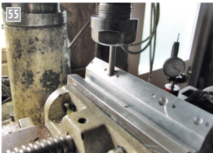
55 Picking up the counter bore using a \frac{3}{16} inch rod.
