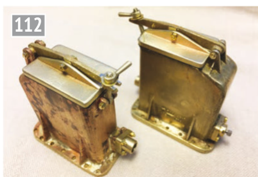
112 The filter boxes have lids that are pulled down onto thin neoprene gaskets. Inside are brass-framed, brass gauze filter panels that sit between the drilled water passage and the triangular outlet flange. The shut-off valves are dummies.
