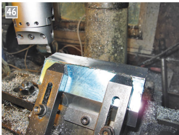
Fly cutting to final close fit to the engine block.
