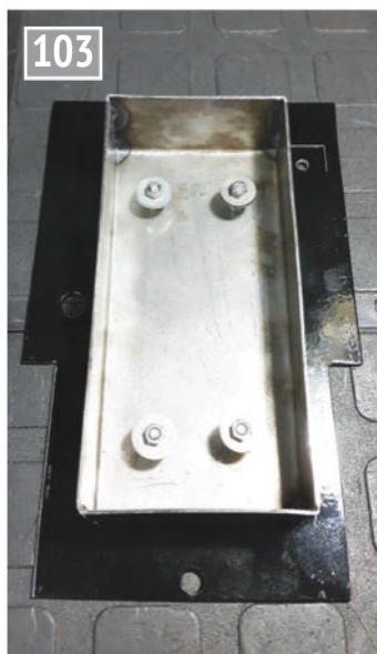
Bunker lead tank box with lead anchors.
