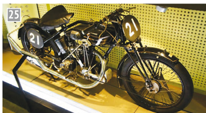
The 248cc Gerrard motorcycle was built around 1923 to a design by J. A. Porter.
