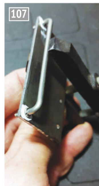
Setup for soldering the hand railing.
