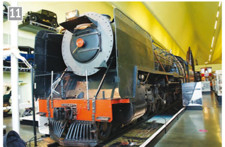
South African Railways 4-8-2 built in Glasgow by North British and now repatriated. Built with massive proportions for the Cape gauge of 3 foot 6 inches.
