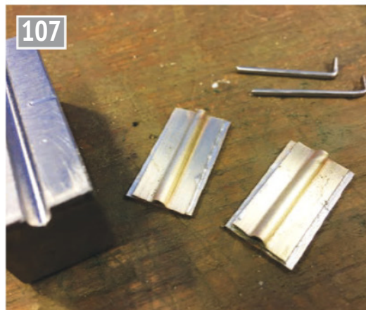
107 To make the sliding door bolts a press tool was made to form the circular channel. The formed plate was then soft soldered to a flat base and the assembly then cut to make the bolt catch and slider.
