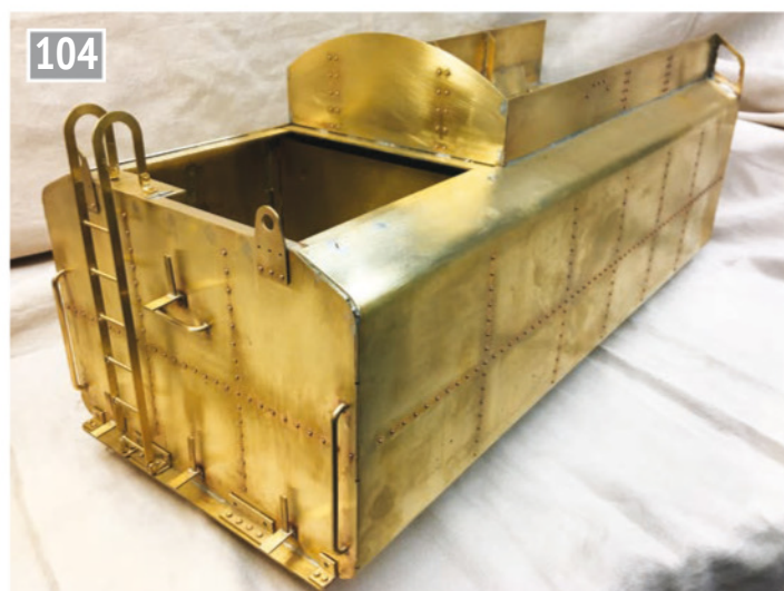
The tender rear plate is attached last and here all seams can be easily heated to achieve a seal.
