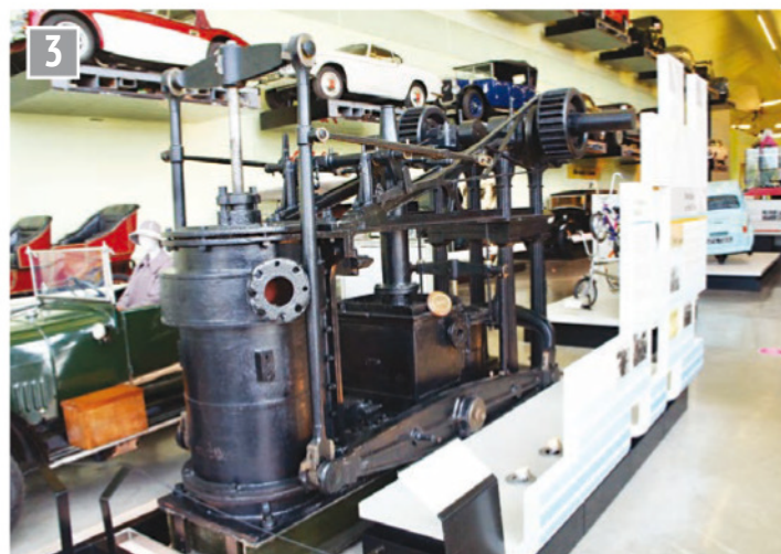
Built soon after Comet the Industry worked until a collision in 1862. This side lever engine was built by Caird and Co. of Greenock and installed in 1828. It was nicknamed the coffee grinder because of the noise it made
