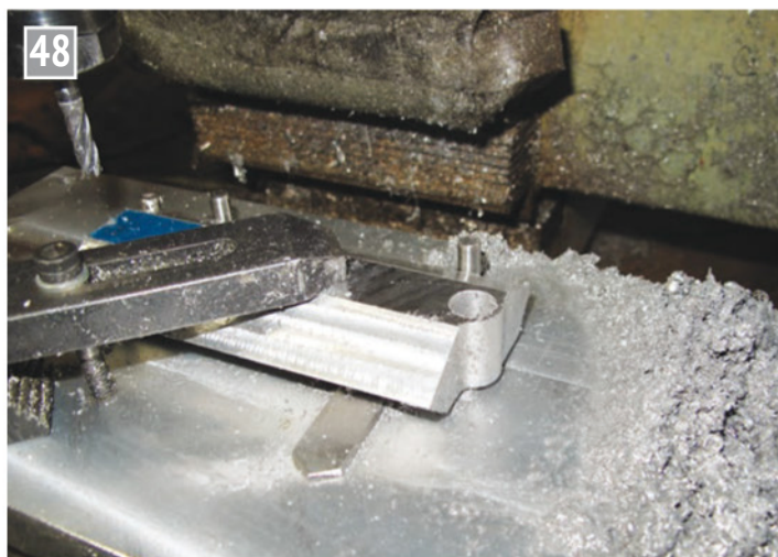
Generating the rear detail and distributor bore.
