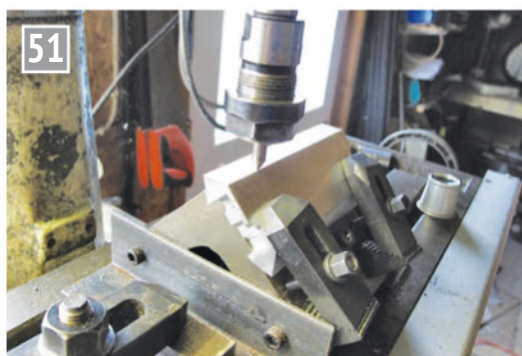
Establishing centre line of securing bolt holes.
