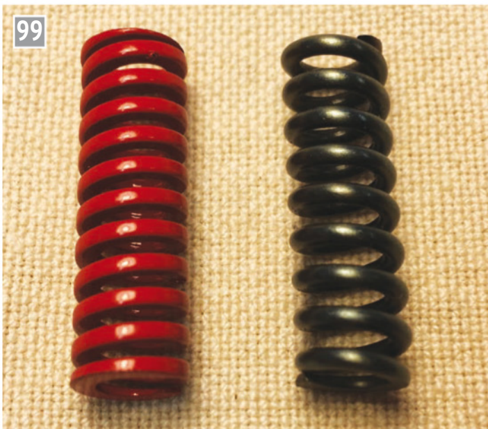
99 The red die spring on the left is wound from square section wire and offers a higher spring rate than the conventional black coil spring.
