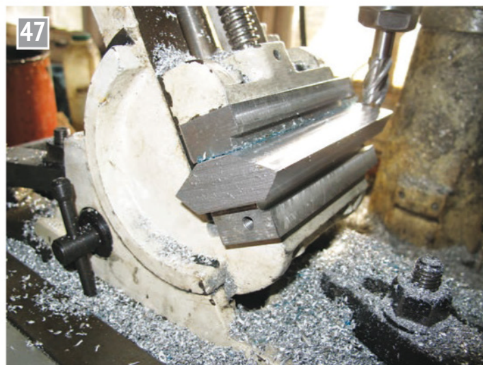
Machining the outside faces.
