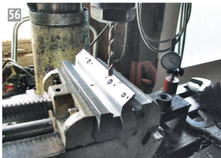
56 Drilling \frac{3}{16} inch diameter feed bore at 5 degrees.
