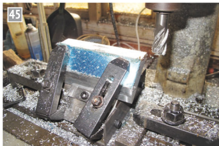
Milling side faces central to the block.
