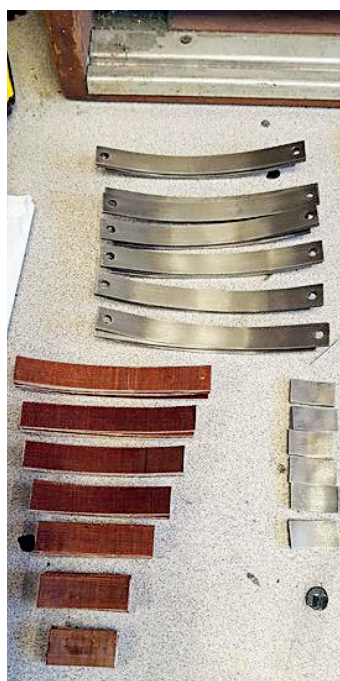
LEFT: 5. Here we have all of the steel springs cut/machined to size ready for forming. RIGHT: 6. I then scaled up the digital drawing and printed that to scale and cut out the top spring profile from it, which I then used as a template to cut out the shape from a suitable piece of wood as shown in this picture. I then shaped each spring steel leaf using the heavy round steel bar also seen in the picture. Forget the decorating roller shown - this wasn't heavy enough for the job in hand. The Tufnol leaves were simply boiled up in a saucepan.
