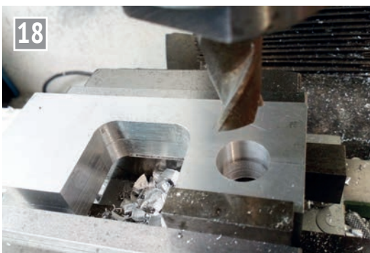
Opening out the bearing hole.
