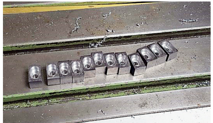
21. Each block was then returned to the vice and placed against the same stop to have the recess machined in the centre. I machined the recess to a length that leaves enough metal on each end after allowing for the tapered ends. The depth is enough to allow for the rubber insert that forms the 'shock' to fit inside.
