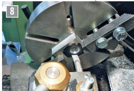
8 Boring the front plate.
