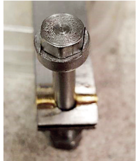
19. Here is the nut sitting comfortably in the slot.
