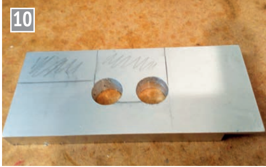
Marking out for shaping the sides.
