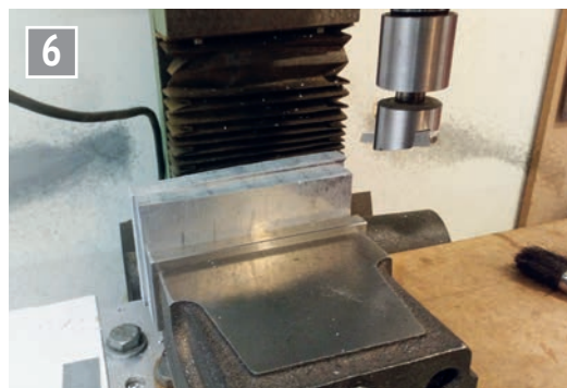
Making the base from flat plate – trimming the sides.
