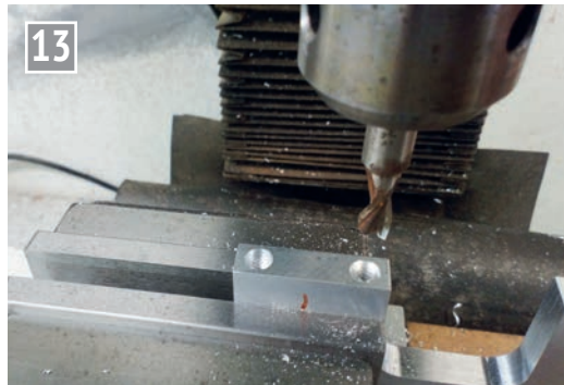
Counterboring the bolt holes.
