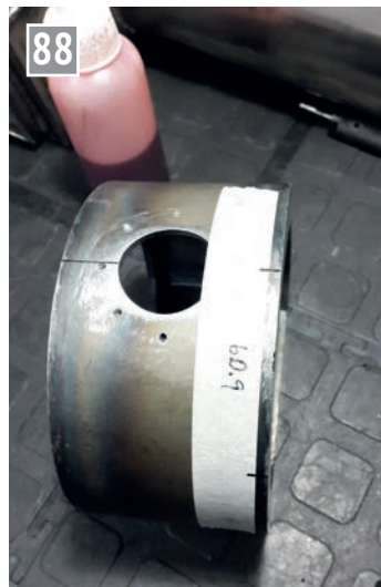
Marking out the handrailing holes.
