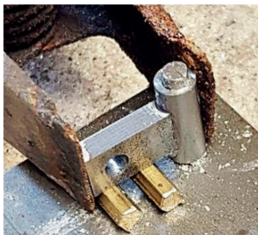
LEFT: 3. I then needed to braze the parts together. The white stuff seen is soap - I used a bar of soap over the jig parts to stop any parts becoming stuck due to unwanted silver solder and the parts are held with a rusty clip. RIGHT: 4. Here we have the finished parts.
