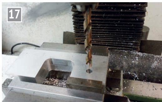
Initial drilling of the bearing hole.
