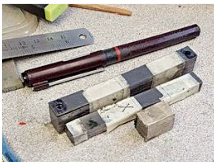
LEFT: 5. Here we have all of the steel springs cut/machined to size ready for forming. RIGHT: 6. I then scaled up the digital drawing and printed that to scale and cut out the top spring profile from it, which I then used as a template to cut out the shape from a suitable piece of wood as shown in this picture. I then shaped each spring steel leaf using the heavy round steel bar also seen in the picture. Forget the decorating roller shown - this wasn't heavy enough for the job in hand. The Tufnol leaves were simply boiled up in a saucepan.
