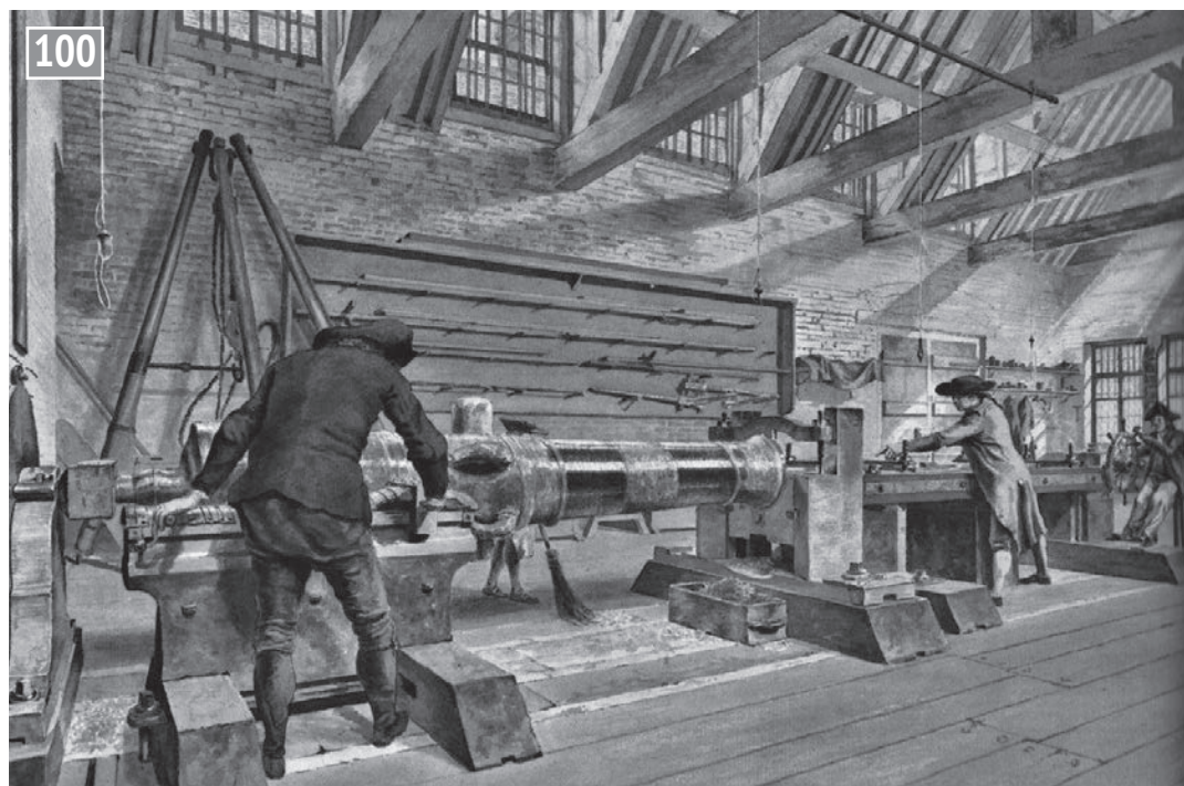
100 Cannon boring and turning machine at Woolwich Arsenal. Watercolour By Jan or Pieter Verbruggen. The original watercolours are part of the Semeijns de Vries van Doesburgh Foundation collection but the reproduction is taken from Prof. Ing. Carel de Beer's The Art of the Gunfounding.
