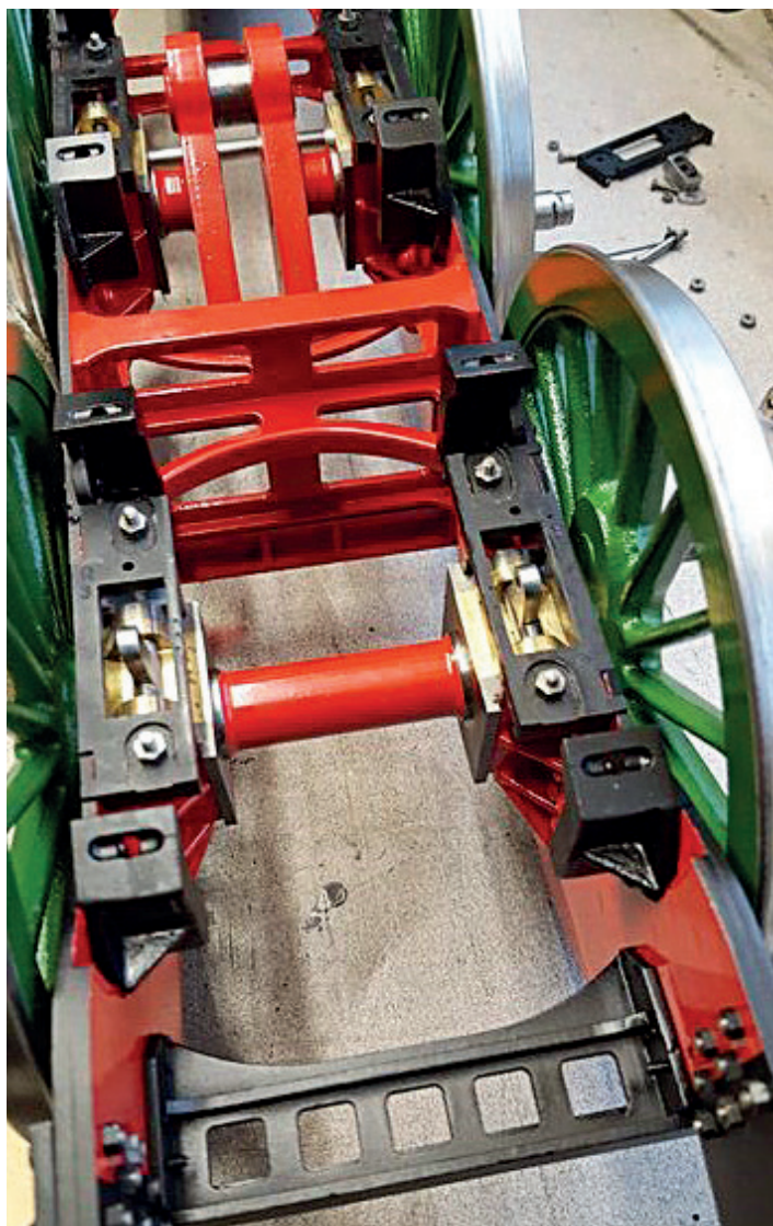
28. This picture shows the swivels fitted to the axleboxes on the rear driver, I had to remove the horn stays, lift the axle assembly partially out of the horns, drift out the pins in the axlebox, insert the swivel, replace the pin, lower the axle and then refit the horn stay.
