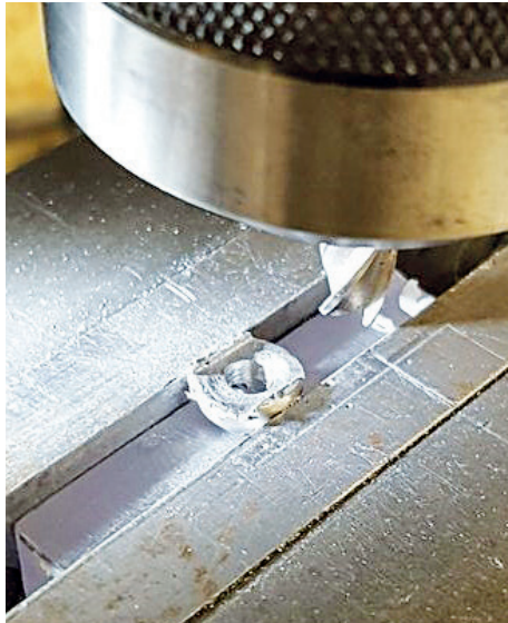
18. The washer was then turned over and the slot machined using a 1/4 inch endmill, to fit the nut.
