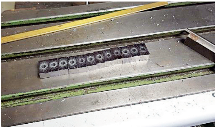
20. After machining to size, all twelve blocks were drilled, using the Perspex stop to ensure all holes were central to the block.
