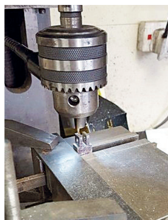
8. The fork is 4mm wide - simple enough but I had to be extra careful here as the only cutter that I had was a cheap, plain shank cutter and with no 4mm collet for my ER25 I was forced to use the drill chuck. This took more than a day but I got there in the end and most importantly with no mishaps.
