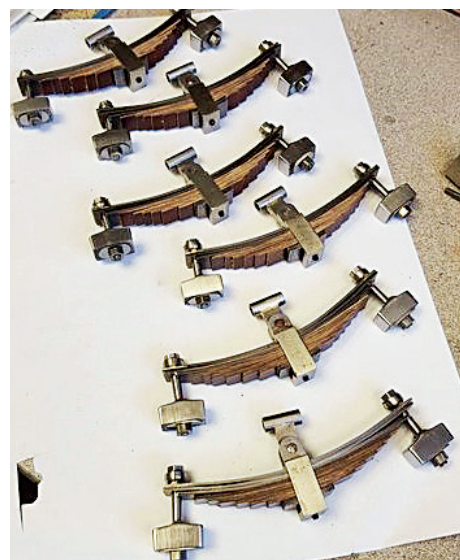
27. The main driver springs are now finished except for a little polishing to remove the last marks and then I'll need to give them a coat of semi-gloss black paint after first giving them an acid 8 coating.
