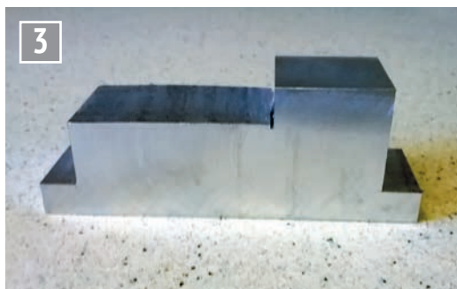
Cut to rough shape with a hacksaw.
