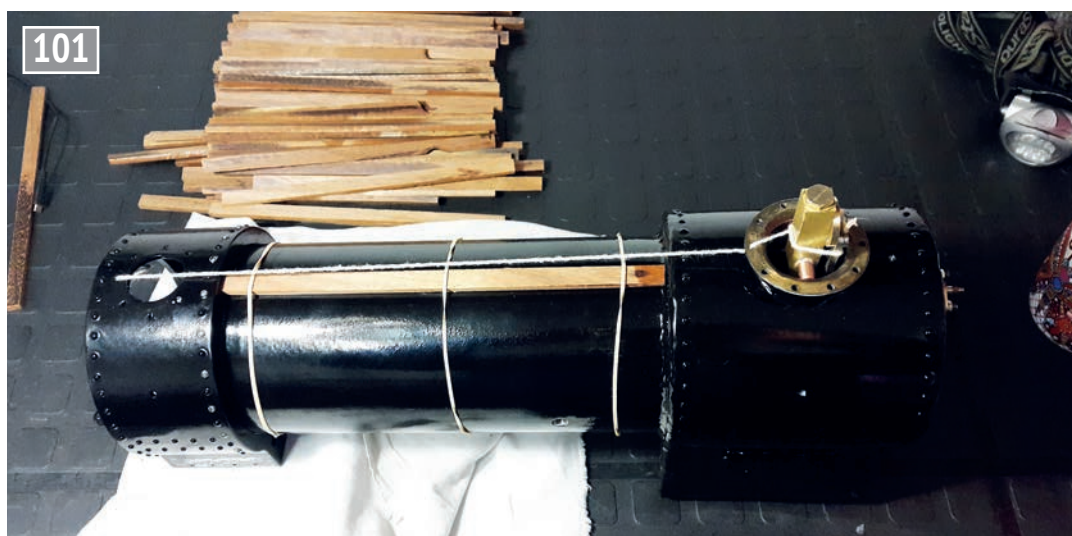
Fitting the boiler cladding.
