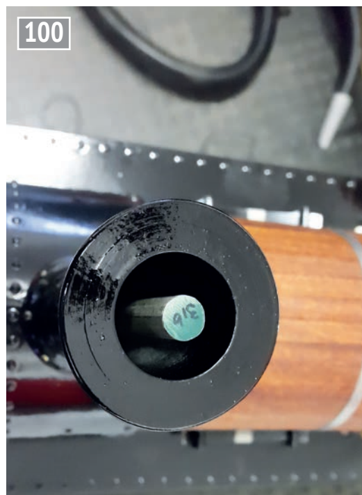
Checking alignment of exhaust.
