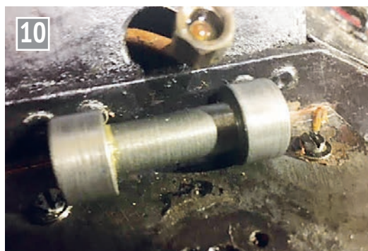
The burnished outer face of the pulled through piston valve.
