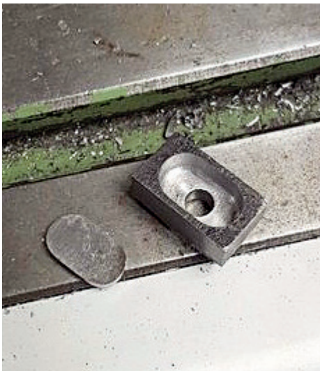
22. I then needed to make the twelve metal inserts which trap the rubber within. These were all done by hand and the picture shows one shock with its insert.
