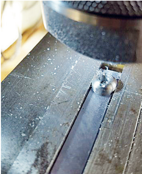
17. I now needed to machine the scallop to fit over the top leaf grip. I did this using a 3mm ball nose cutter.
