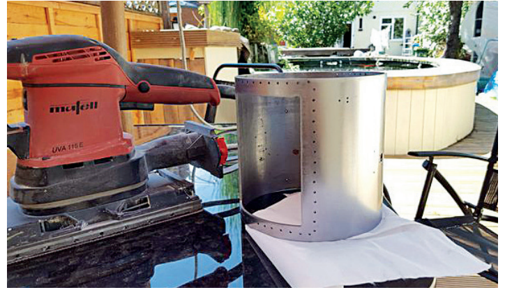
16. The smokebox benefitted from a little attention from an orbital sander.
