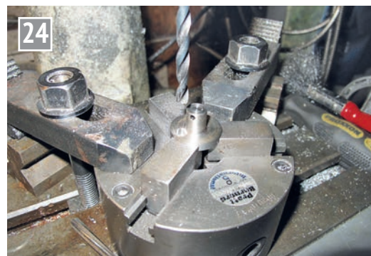
Drilling the second crankpin hole displaced 90 degrees to the first.
