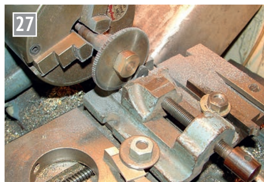
Sawing the slot in the brake block.
