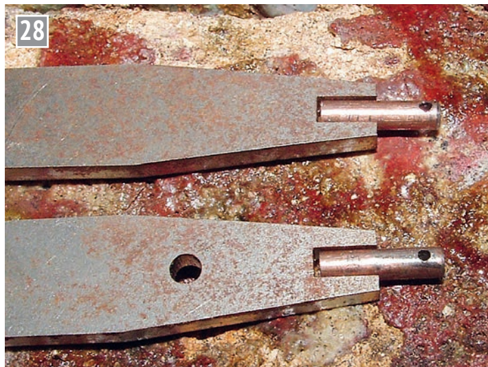
Forming the ends of the brake beams.
