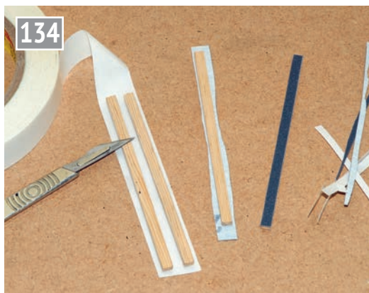
The stages in making polishing sticks.
