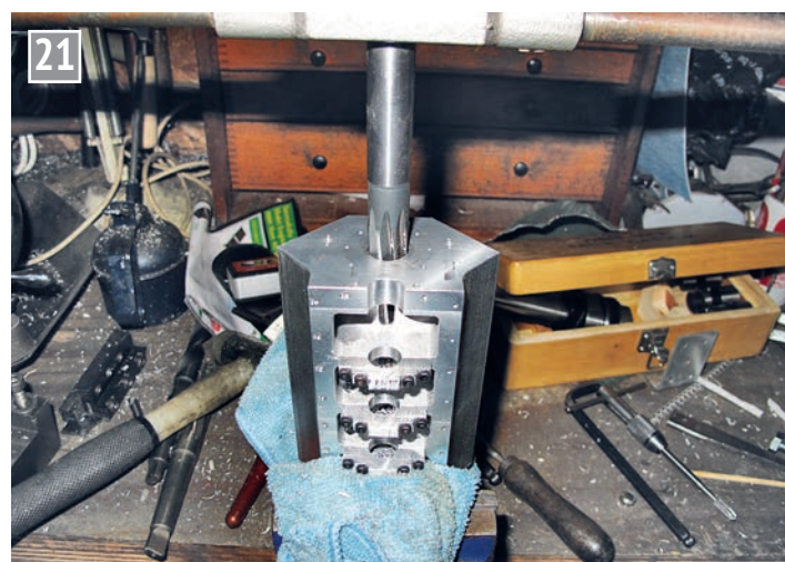
Final reaming of the main bearing clamps.
