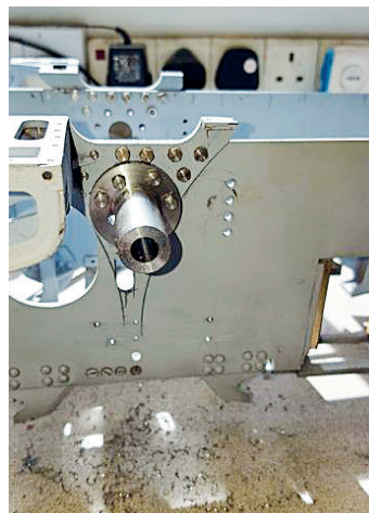
4. Back to the frames again to check that the holes line up.
