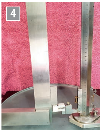
Accuracy check at the bottom of a large set square.
