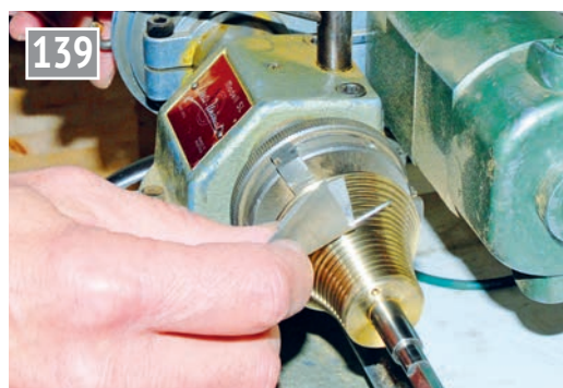
The Fusée is polished by hand turning the lathe whilst holding the abrasive paper around a thick needle against the groove.
