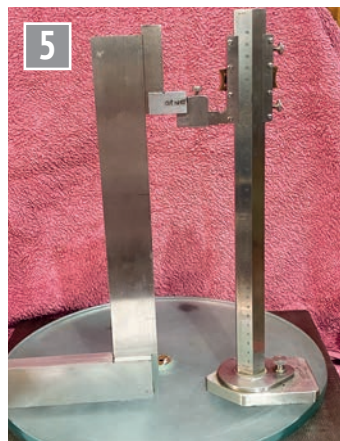
Accuracy check at the top of a large set square.
