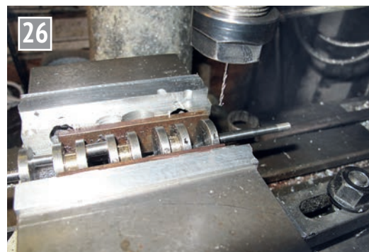
Cross drilling and pinning the journals.
