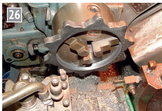
Turning the brake ring.
