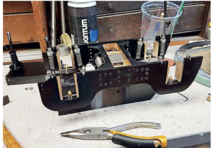
10. The bogie after painting and reassembly.
