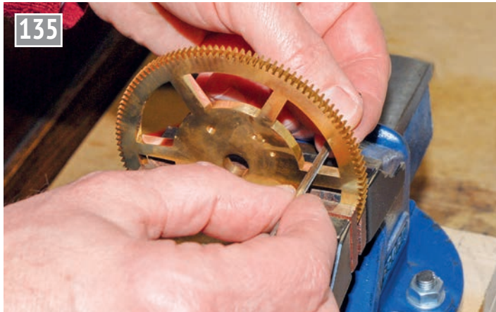
Polishing a wheel crossing with a home-made polishing stick.
