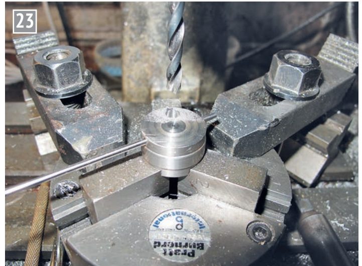
Drilling for the crankpin.
