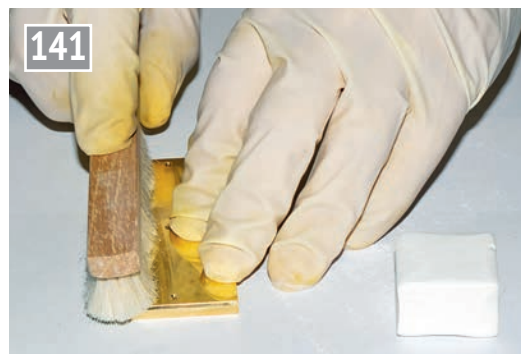
The final stage, polishing with a soft brush and French chalk. For an unknown reason I was wearing oversized gloves!
