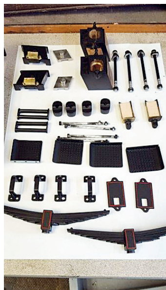
13. Here is a closeup of the various components for reassembly of the Cartazzi axle. As you can see the lining for the spring and axlebox covers has been applied.
