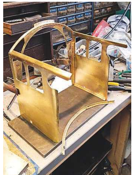
RIGHT: 7. The spectacle plate and side sheets are now joined using brass angle. The right angle along the bottom of the side sheets has been silver soldered in place with rivets along the side and four holes drilled through the bottom to take 8BA round head screws for holding the cab to the floor.
