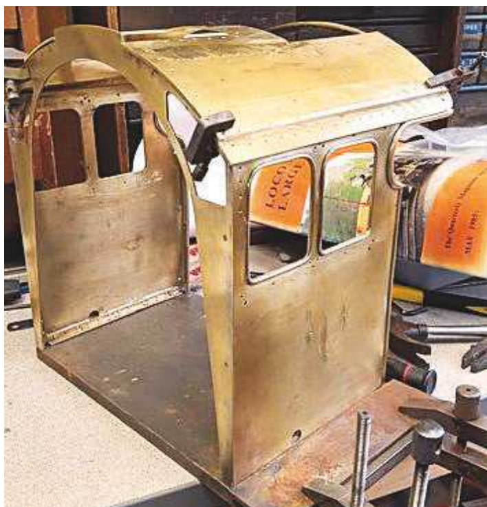
19. Here we see the roof in place ready for the fixing holes to be spotted through.
