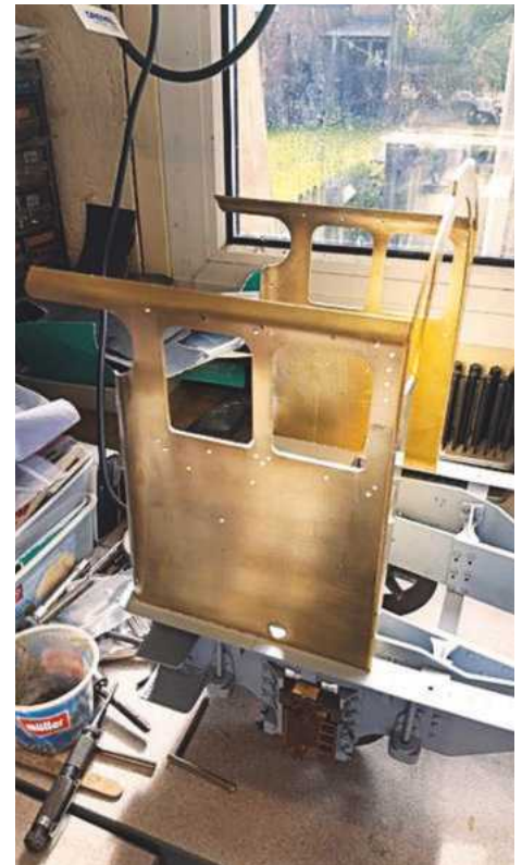
5. Here we see how the basic shape is coming together - it's just taped for now to check for which way I'm going to butt the edges together.
