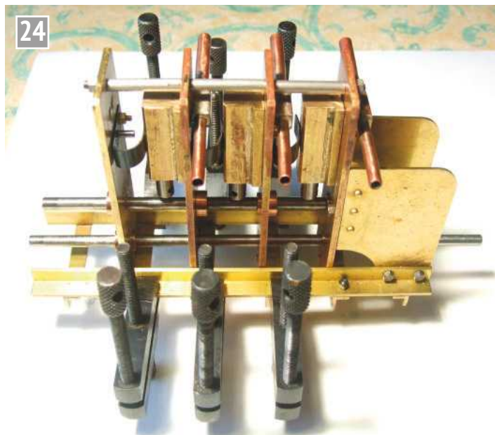
The front three mounting plates are still only held with small clamps and two \frac{3}{16} inch shafts are used to check the alignment of the bearings.
