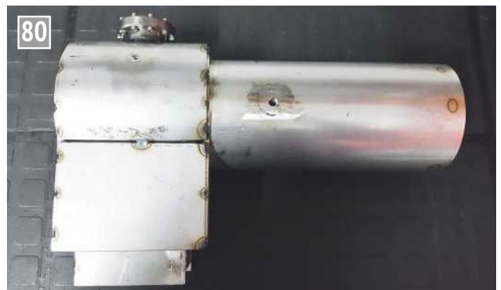
Outer shell tack welded.
