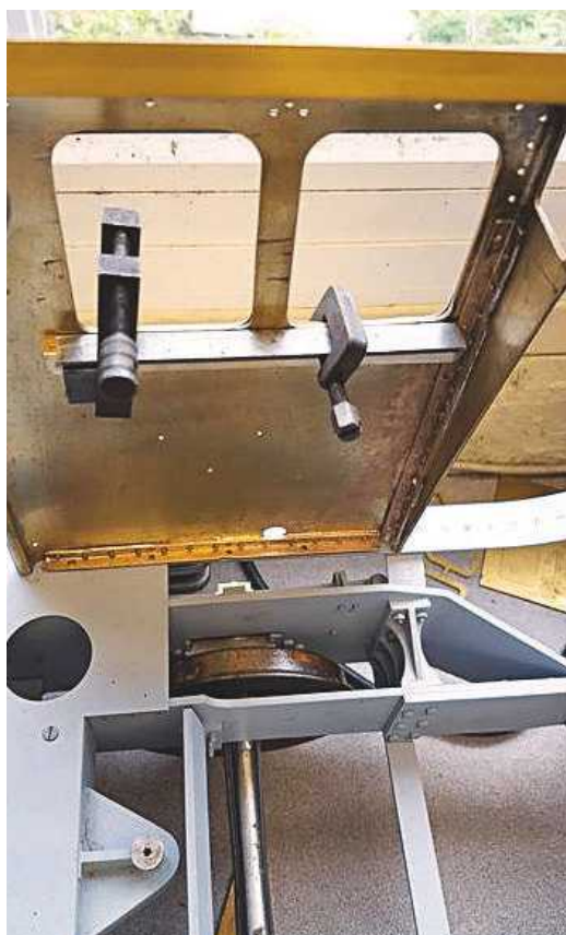
LEFT: 17. With the runners made, the mounting holes needed to be plotted and drilled. I used a thin strip of steel as a guide to keep the runner parallel with the window opening and also to give a small step up from runner to window. I clamped the bottom runner in place and using a fine marker pen marked the position for the holes through the mounting holes in the side sheet. Once happy that all was good I held both bottom runners together (back to back) in the machine vice and drilled through taking care of both sides in one hit.
