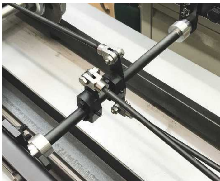
The central brake shaft. Note how the bosses are bolted to the levers and the bosses are fixed to the shaft with taper pins. The bosses could probably be fixed to the shaft with Loctite retainer. The pins provide a positive mechanical lock but one which can be dismantled if required.
