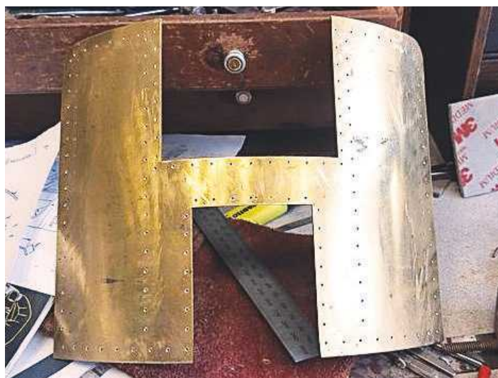
15. Here we have the roof with all of the holes drilled and countersunk. Most are countersunk on the top except for the rain gutter strip holes which are countersunk underneath.
