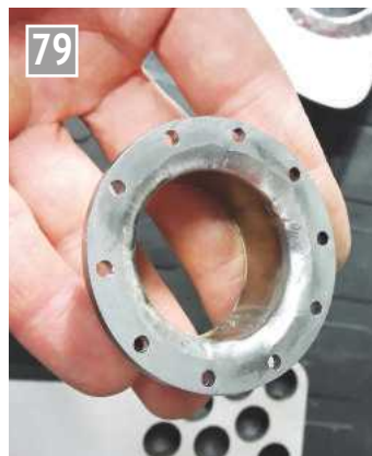
Steam dome flange and stub.
