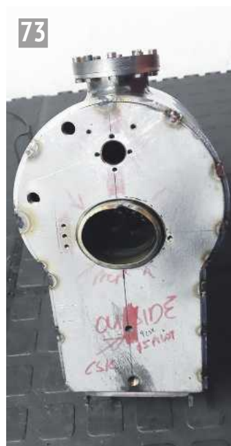
Backhead tacked with all holes predrilled.
