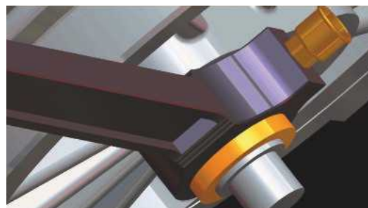
Big end assembly in 3D CAD.
