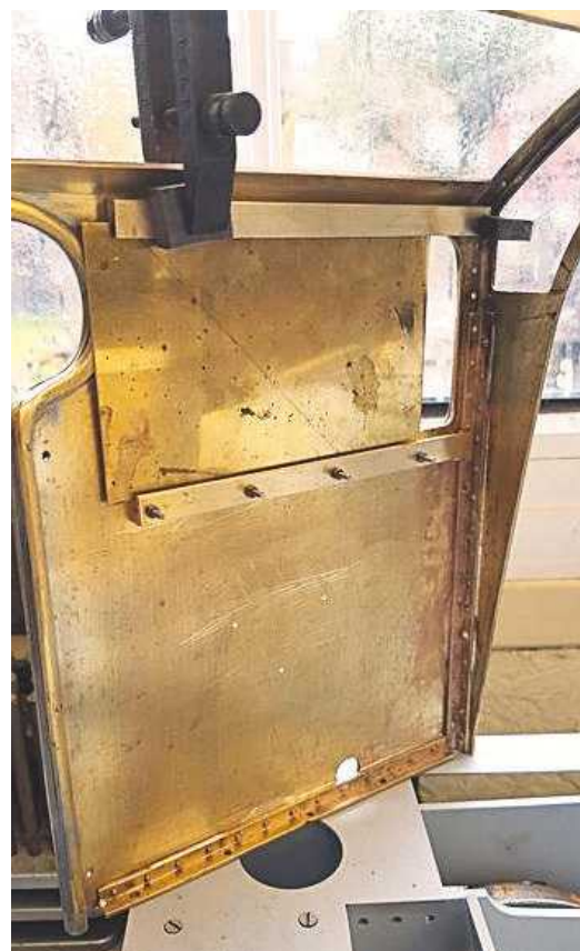
LEFT: 17. With the runners made, the mounting holes needed to be plotted and drilled. I used a thin strip of steel as a guide to keep the runner parallel with the window opening and also to give a small step up from runner to window. I clamped the bottom runner in place and using a fine marker pen marked the position for the holes through the mounting holes in the side sheet. Once happy that all was good I held both bottom runners together (back to back) in the machine vice and drilled through taking care of both sides in one hit.
