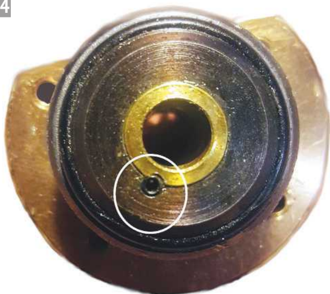
The input gear and clutch disk are pinned together as well as being press fitted.
