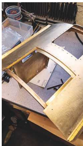
20. The service hatch supports have been fitted and rivetted in place.
