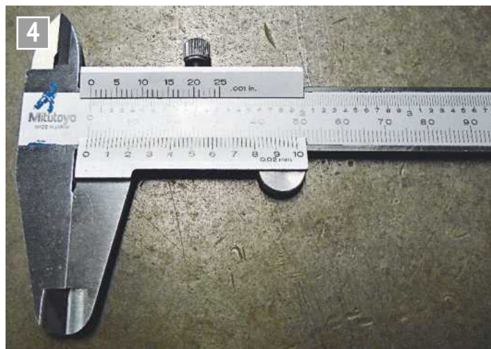
This Vernier caliper reads zero when fully shut.
