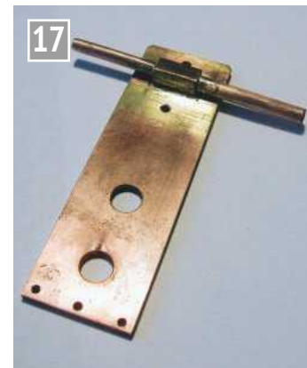
Adding the steam inlet and exhaust block and pipes by silver soldering may slightly distort the working face slightly but a rub on fine emery tape on a surface plate or drilling table will correct matters.
