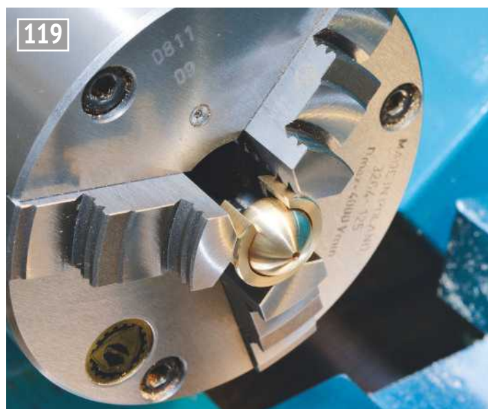
Drilling a hole through the sun using a ball collet.
