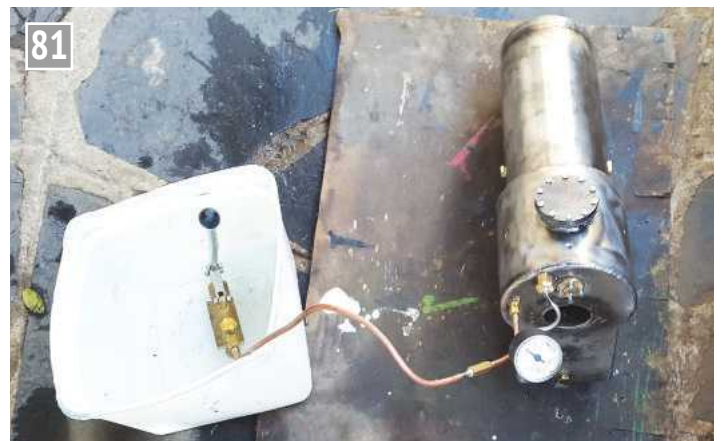
Hydraulic boiler test.
