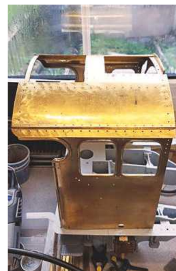
16. This picture shows the roof sitting on the cab with the gutter strips in place.
