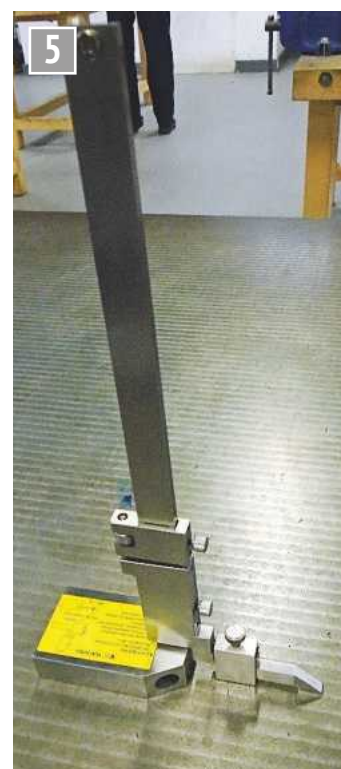
Vernier height gauge on a surface plate set so that zero reading can be verified.
