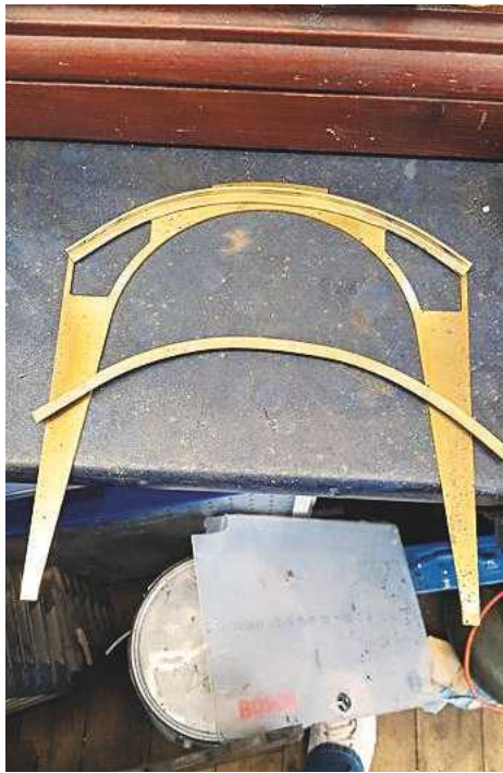
LEFT: 3. I then repeated this for the rear roof frame support. Here are both sections for the curved frames lying on top of the spectacle plate for size. These will be annealed one more time to reach the final shape.
