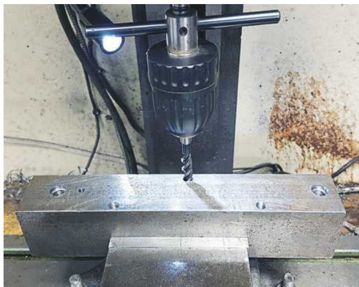
8. Here is the holding jig mounted in the machine vice. I drilled and tapped a few holes for holding down clamps - one in the middle on the far side and two others equally spaced between that and the two end 10 mm holes.
