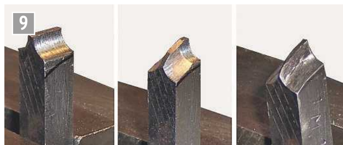
Grinding the back relief on a cutter.
