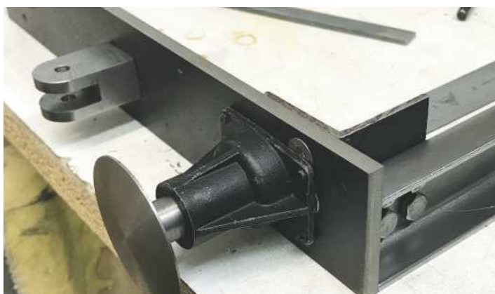
Here you can see the buffer beam bolted to the channel longeron with the 40 x 40 x 3 mm angle bracket. The countersunk screws can be seen on the face of the beam, partially covered by the buffer stock. One side of the bracket has a half-moon cut-out to clear the nut on the back of the buffer stock.
