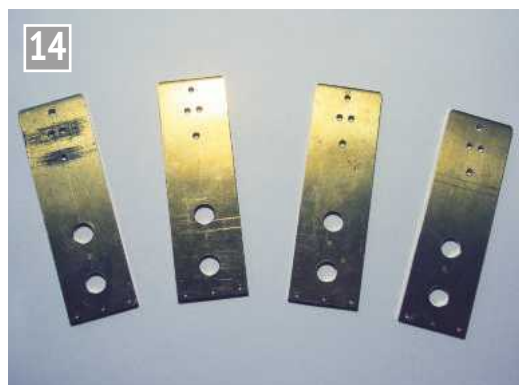
Here the four plates have been finished except for the 8BA holes and identified A-D on their faces sides.
