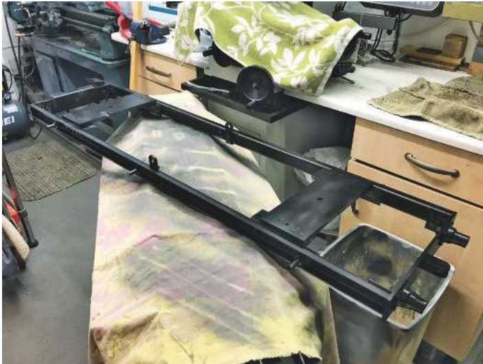
An underside view of the chassis during painting. Note the countersunk screws in the bogie stretcher, to provide the bogie rotation ball races with a flat bearing surface. Note also the small chamfer filed in the front bogie stretcher, needed to clear the front brake pull rod.
