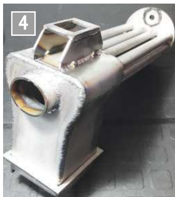
Inner boiler welded assembly.
