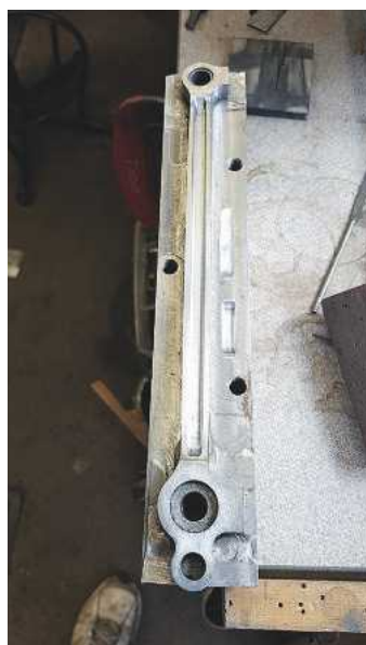
16. This picture shows the first half of the middle section having been machined to size.
