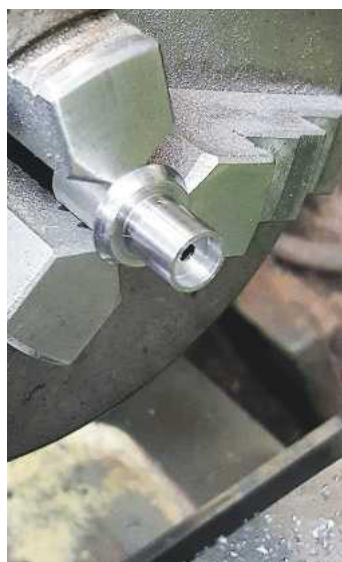
4. The leading pins are a little more involved - these have a no. 34 hole drilled right through with recesses either end. The journal is slightly shorter too.
