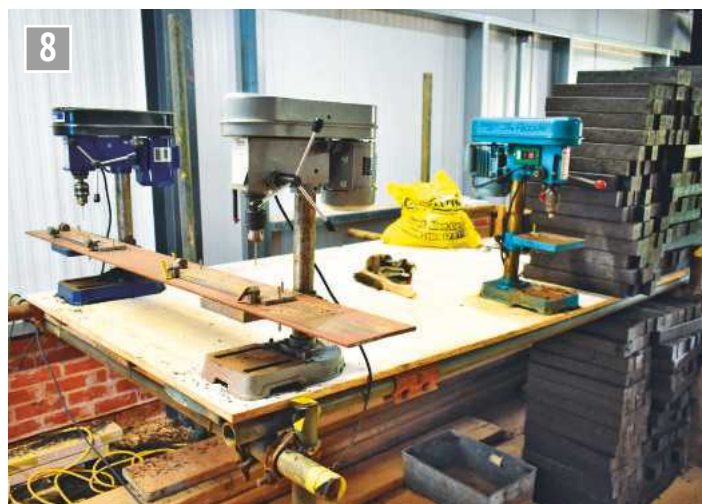
Part of the sleeper drilling operation.
