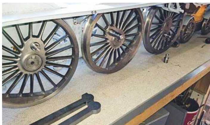
5. Here is a picture to show the various parts together. I won't fix the crankpins permanently (I still need to machine the square for the return crank) until I have machined up the bearings.
