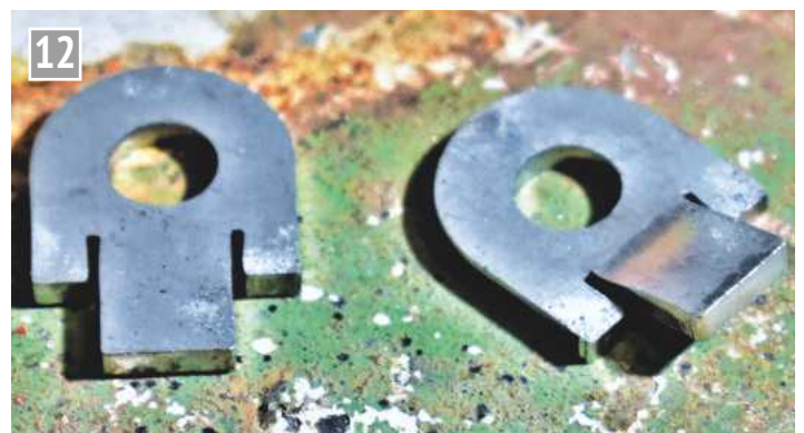
Rail clips before and after bending.
