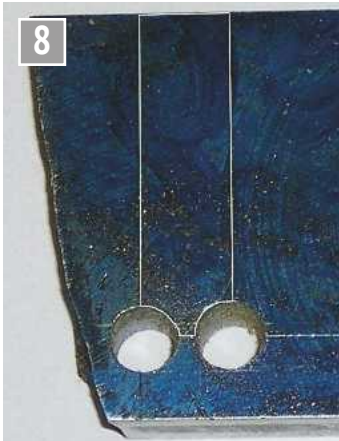
A cutter marked out on a piece of hardenable steel.
