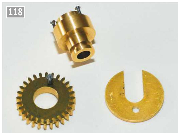
Slip washer to allow the tellurian to be adjusted.
