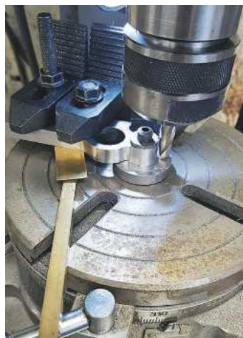
16. This picture shows the first half of the middle section having been machined to size.
