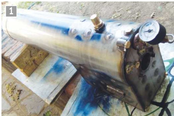
Pressure testing my first stainless boiler.
