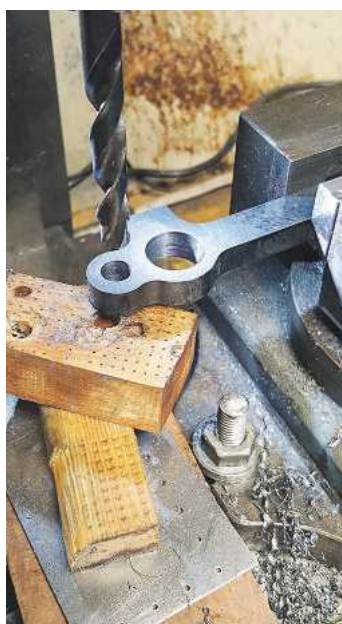
6. I decided to drill the centres of the leading coupling rods first. I need to be careful here as the knuckle hole is of two different sizes to allow for the pin.
