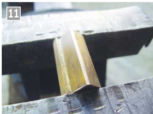
Putting a chamfer of the outer corners of the cylinder blocks for appearance's sake.
