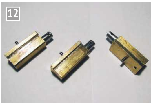
The cylinder assemblies ready for the next stage in the build.
