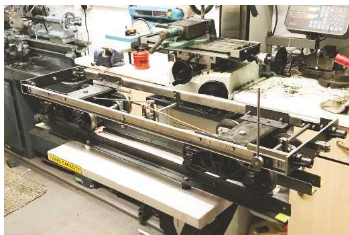
Here the chassis has been assembled, complete with the brake gear, showing the very simple all-bolted construction.
