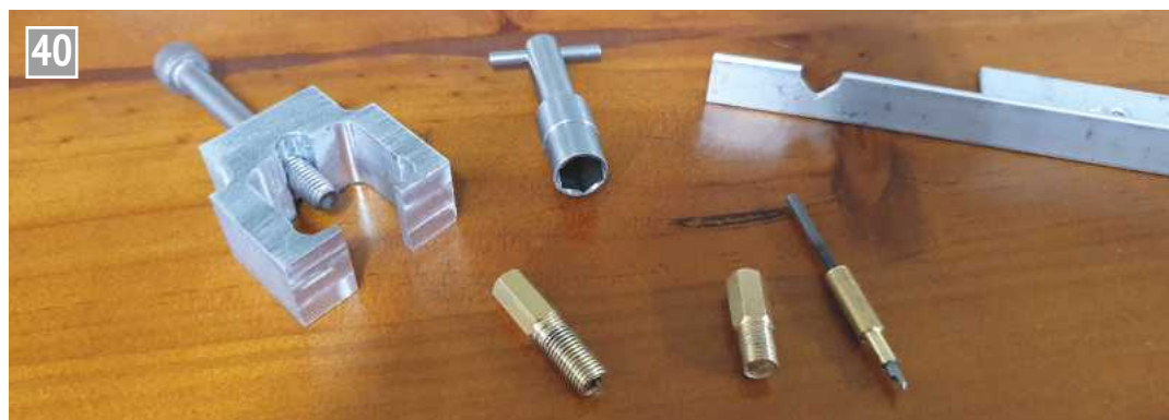
Plug for determining TDC and other gadgets.
