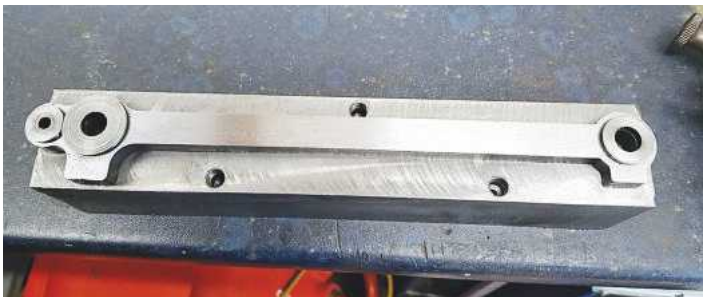
12. Here we have the leading rod again in its jig but this time it's joined by the three buttons, ready for profiling. The buttons have been hardened to protect them during the next stages, or should I say protect the job underneath. The buttons are stepped to be a good fit in the 3 bush holes and the two on the knuckle joint have been flat edged to fit.
