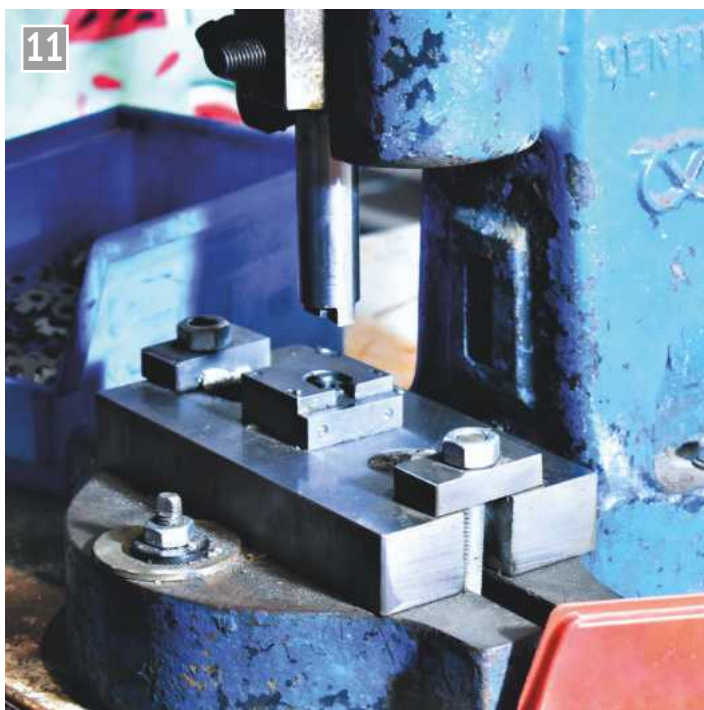
Close up of the rail clip bending jig.
