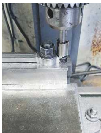
19. First job for the buckle is to counter bore the leading rod to create the tongue.
