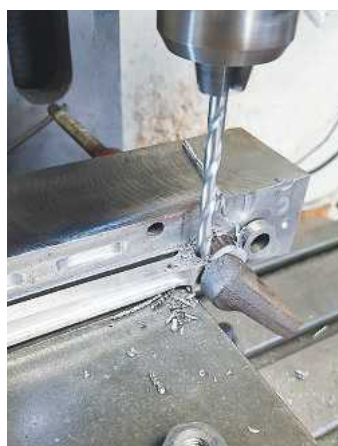
20. The next thing is the slot and the first job is to cross drill the trailing rod.
