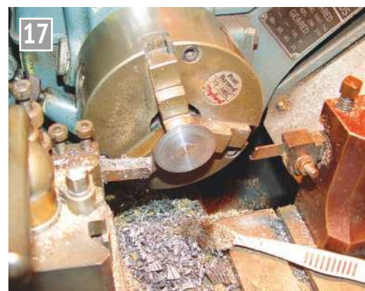
Machining a buffer head with Doug's special tool.
