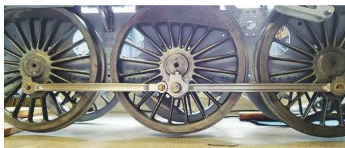
20. The next thing is the slot and the first job is to cross drill the trailing rod.
