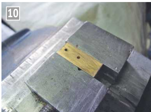
Marking out and drilling the hole for the pivot pin and the steam port.
