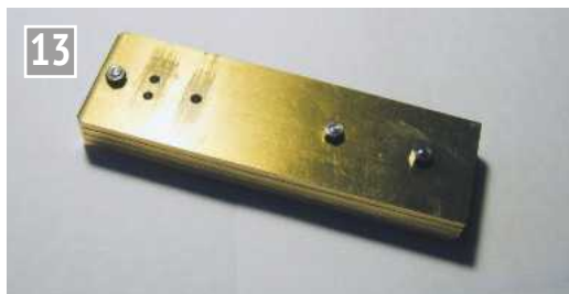
This view shows the four plates bolted together for the marking out and drilling of the steam ports and the cylinder pivots. Toolmaker's clamps were used to hold the pack for the drilling and reaming of the \frac{1}{16} inch holes afterwards.
