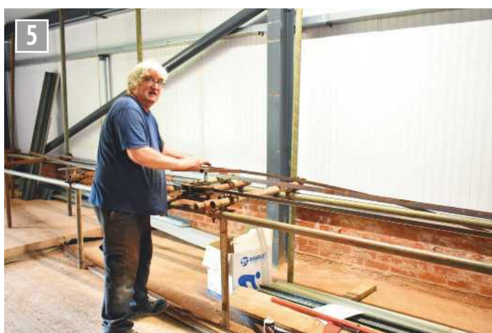
Gordon Roberts using the bending machine for the rail.
