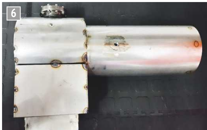
Outer boiler assembly tacked.
