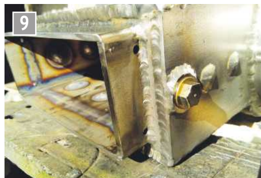
Foundation ring welding.
