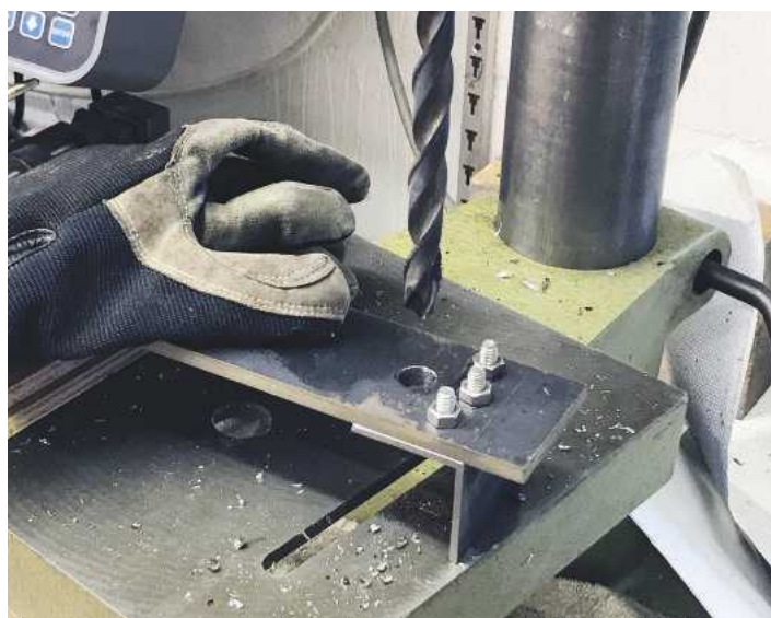
Drilling the buffer beam for the buffers. Gloves are a necessary precaution for a job like this. Note that the bracket has already been bolted to the beam. In this case the blank bracket was clamped to the beam which had accurately placed water cut holes, and the holes in the bracket were 'spotted through'. After this, the holes in the beam were countersunk for Allen screws, so that the buffer stocks could sit on a flat face.
