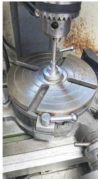
14. I drilled a \frac{3}{16} inch hole in the end of the stub to allow for a quick set-up of the rotary table. The hole was deep enough and the \frac{3}{16} steel rod true enough to allow for a quick and accurate alignment.
