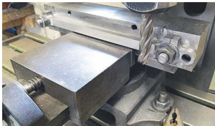
16. This picture shows the first half of the middle section having been machined to size.
