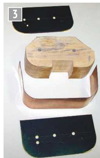
The pieces for forming the case in brass. Note the cutaway parts of the wood former where the initial spot brazing will be applied.
