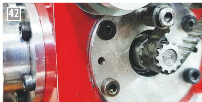
Holes for jacking timing base/rear bearing holder.
