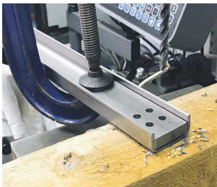
A simple jig was used to drill the four 6 mm holes (for M6 bolts) in the ends of the channel longerons. The other end of the 48 inch long channel was resting on the table of the nearby milling machine, and the drilling machine table adjusted to bring the job level.
