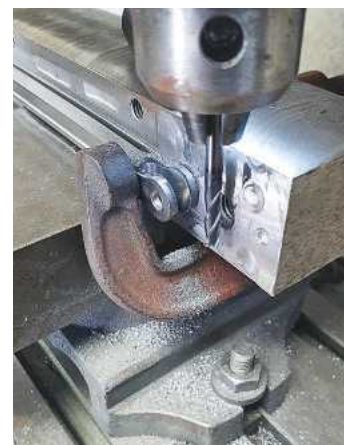
21. I then cut out the middle by hand with a hacksaw and milled the opening to size. This is a little larger than the tongue which is to allow a little sideways movement when subjected to an uneven track.
