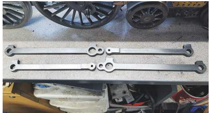
11. And so the four rods are ready for the profiling of their edges.
