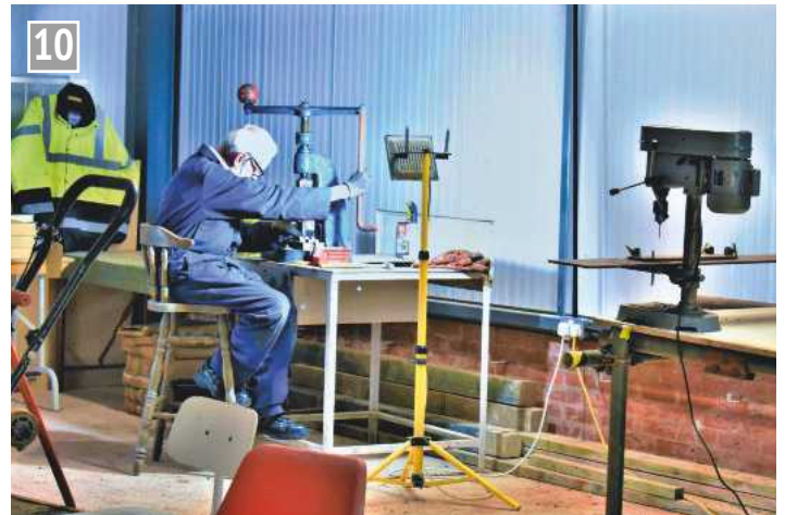
The fly press in operation bending the rail clips.
