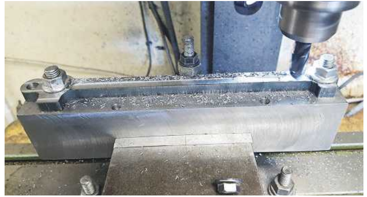
10. A view showing me working along the length. All I had to do was move the various clamp bolts as I reached them.
