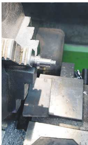
3. Here is one of the trailing pins finished, except for a little polishing of the journal. I'll machine up the caps to fit later. Seems that I forgot to blow down the thread for this picture!
