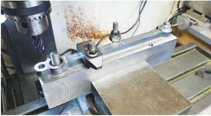
9. Picture shows a start being made on reducing the thickness from the left. (Before anyone takes me to task for using the chuck rather than a Clarkson's, I had no option as the new cutters are all plain shank and I had no collet chuck... I had no issues though.)
