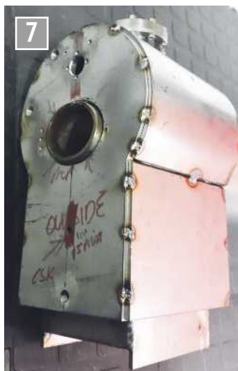
Weld preparations negating the need to back purge.
