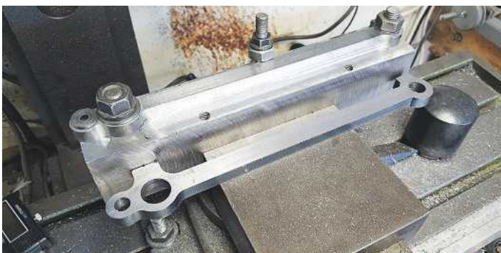
12. Here we have the leading rod again in its jig but this time it's joined by the three buttons, ready for profiling. The buttons have been hardened to protect them during the next stages, or should I say protect the job underneath. The buttons are stepped to be a good fit in the 3 bush holes and the two on the knuckle joint have been flat edged to fit.
