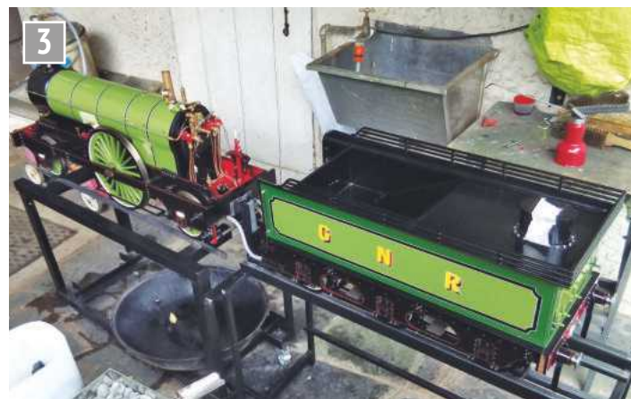
Checking blower and safety valve for limit pressure during first steaming.
