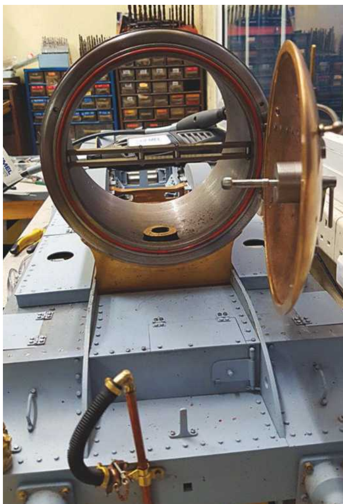
17. A view with the door open, showing the dart in position and also the door seal temporary fitted into its groove to check that all tightens up properly.
