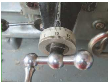
Laurie Leonard shows how to improve the cross-slide lead screw on Myford Lathes.
