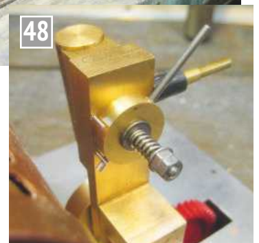
Stops for the reversing valve were fitted to the engine frame which completed the work on the engine.
