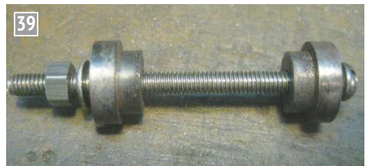
Some hardened filing buttons were made.
