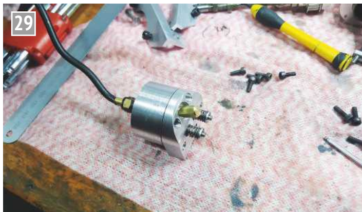
Lapping valves under pressure.
