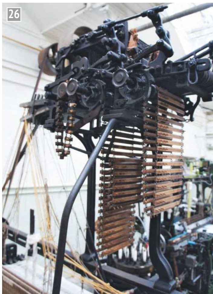
26 A dobby loom used a heald shaft to lift the warp threads. Instead of punched cards here wooden lags with pegs in holes control operation and it can be programmed to create simple patterns.
