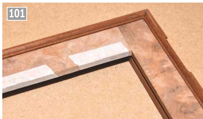
Securing the veneer while the glue dries.
