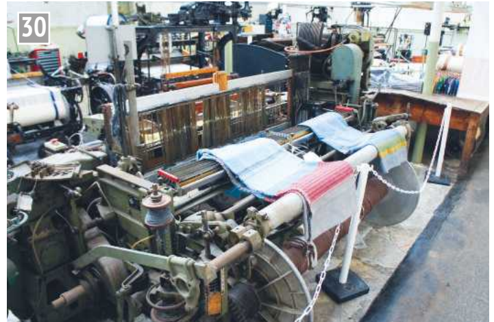
Telescopic Rapier loom made by Adolf Saurer in France around 1975. One end of a rapier (a rod or steel tape) carries weft yarn and moves across the fabric's width, carrying the weft yarn through the shed to the opposite side. The rapier is then retracted, leaving the new pick in place. Unfortunately, this loom was placed the wrong way round in the museum - the beam would normally be behind.
