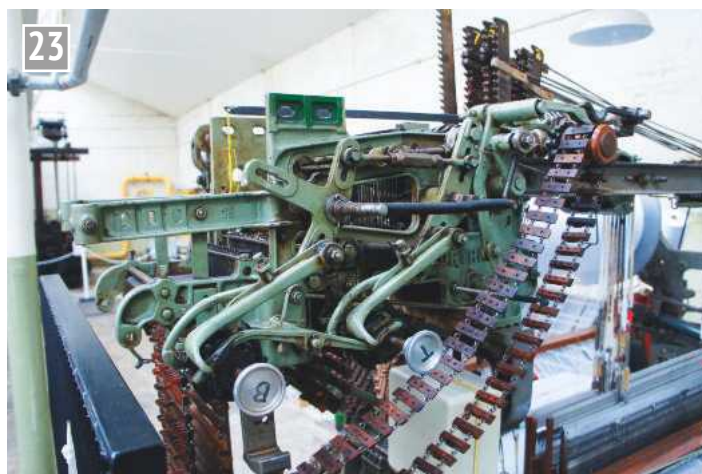
Detail of Terry towelling loom - this one made by Northrop features a dobby mechanism to programme weaving simple patterns.
