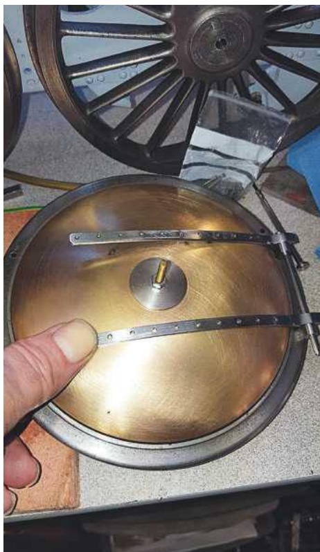
10. Next the hinge strap was shaped by hand to match the door. This takes a little time as it's a compound curve but it's only a gentle curve so no real problem and the rivets will hold them tightly in place.
