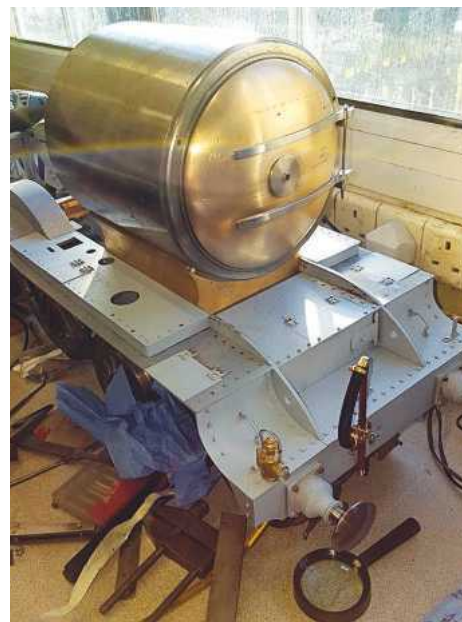
LEFT: 11. Once the hinges were shaped I re-locked the door ring on the milling table sitting on some parallel bars, taped under the hinges to stop any slip on the \frac{1}{16} drill bit, lined up with the centre of the hinge strap near the hinge block and then, once happy that all was square, I moved over to one of the centre holes in the hinge strap and drilled the first hole through the hinge into the door. I then placed a rivet to hold it in place and moved along a few holes and drilled another. Doing it like this helps keep the hinge straps running at 90 degrees to the hinge pin, or at least that's how I tackled this particular job. Also of note is that the door sealing ring has been put in its groove so that the hinge is in its correct position for sealing the door properly. Once the central hinge holes had been drilled (the outer holes have to be done by hand off the table due to the angle) I then moved to plot, using a centre drill, the door handle point, two stanchion points and the lower central rivet hole for the door lamp bracket. RIGHT: 12. Here is the door in place, with the door closed.
