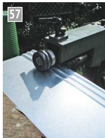
Rolling corrugated sheet.
