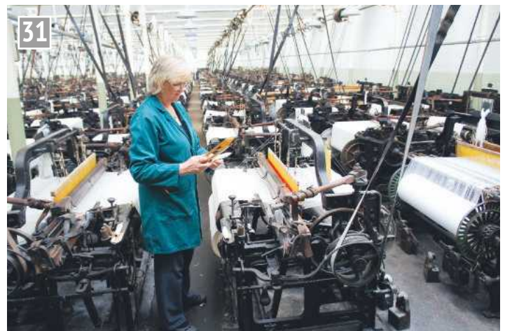
Former staff member, Renee Flynn inserts a pirn into a shuttle for use in one of the mill's Lancashire looms.
