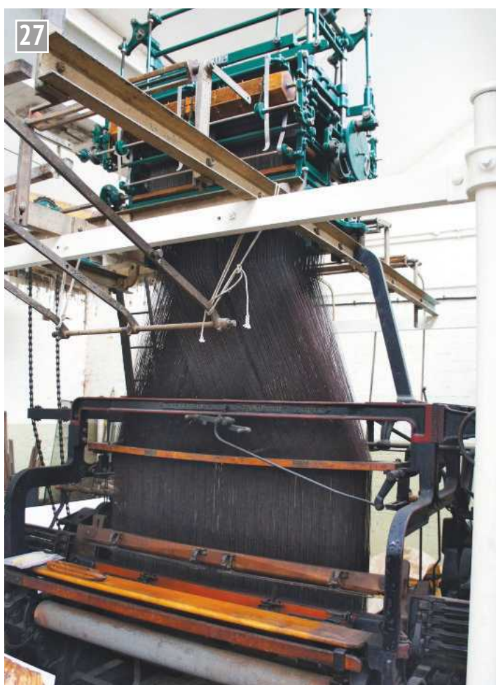
27 The most complex loom in the museum, this Jacquard loom uses punched cards to control lifts of numerous harnesses holding healds to make elaborate designs. The card principle was later used by Hollerith for early computers.
