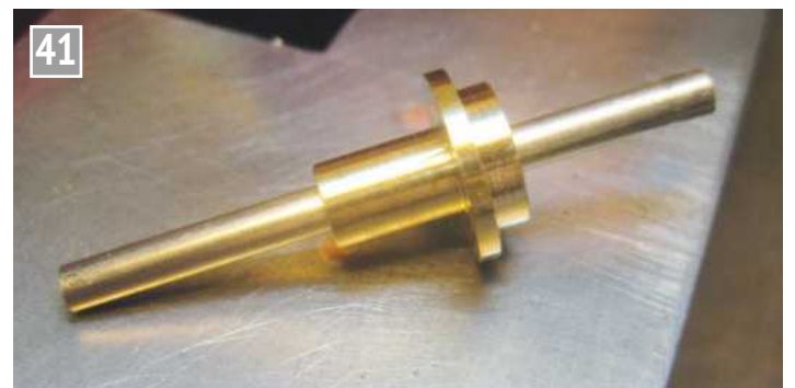
The cylinder end covers which would be glued in place were made. The piston rod end cover has no seal, just a long reamed hole.
