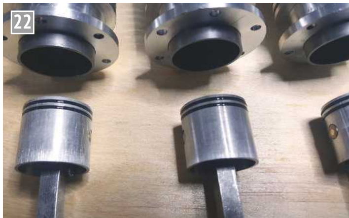
Pistons with Viton 'O' rings.
