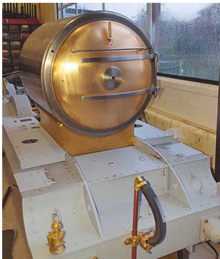
14. This picture shows the lamp iron riveted to the door and the door handrail fitted although not tightened up yet. I had to counterbore the rear of the door to get the 7BA nuts to reach the handrail knob threads. Once painted I will return to the handrail and solder the parts together and round off the ends so that they are enclosed as in the prototype.
