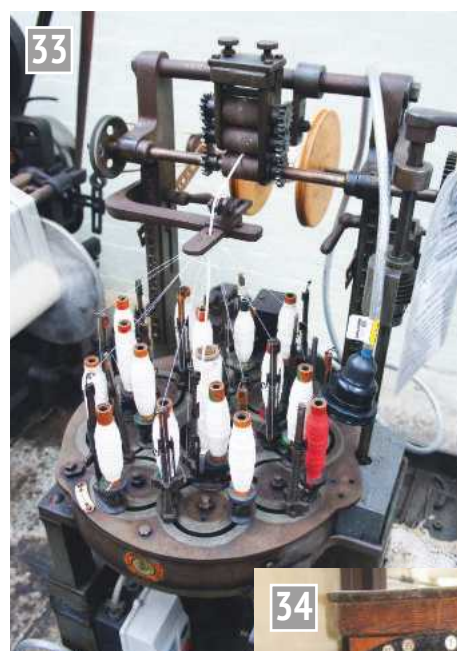
Braiding maker - weaving wasn't the only technique used. Knitting machines and this braiding maker were also important.
