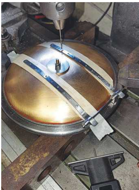
LEFT: 11. Once the hinges were shaped I re-locked the door ring on the milling table sitting on some parallel bars, taped under the hinges to stop any slip on the \frac{1}{16} drill bit, lined up with the centre of the hinge strap near the hinge block and then, once happy that all was square, I moved over to one of the centre holes in the hinge strap and drilled the first hole through the hinge into the door. I then placed a rivet to hold it in place and moved along a few holes and drilled another. Doing it like this helps keep the hinge straps running at 90 degrees to the hinge pin, or at least that's how I tackled this particular job. Also of note is that the door sealing ring has been put in its groove so that the hinge is in its correct position for sealing the door properly. Once the central hinge holes had been drilled (the outer holes have to be done by hand off the table due to the angle) I then moved to plot, using a centre drill, the door handle point, two stanchion points and the lower central rivet hole for the door lamp bracket. RIGHT: 12. Here is the door in place, with the door closed.
