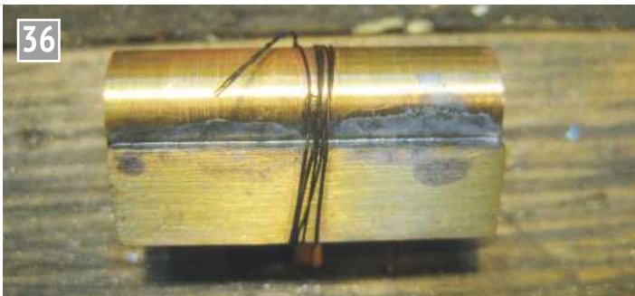
The cylinder was soldered to the port block and then holes were drilled for the steam passageways into the cylinders.
