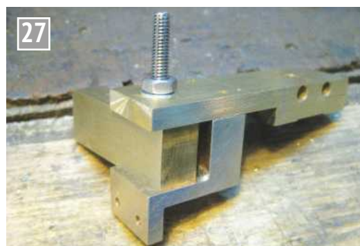
A block of brass was soldered to the angle so it could be attached by screws to the engine frame.
