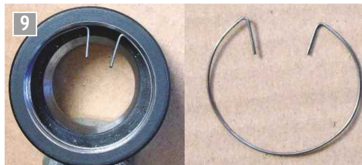
The 'two wire' method for measuring an internal thread.
