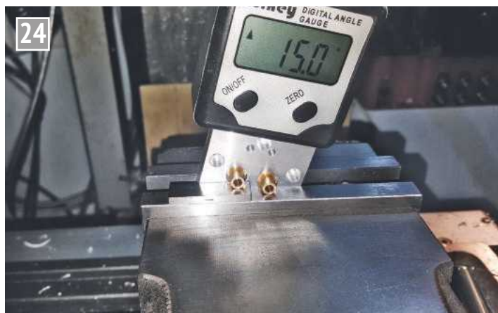
Using the valve guides as a sine bar.
