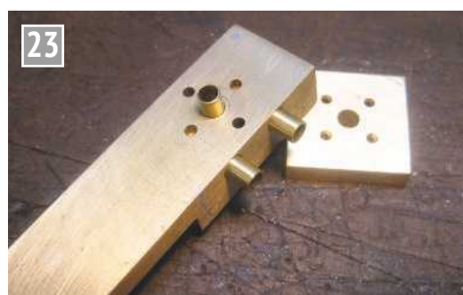
The ports are drilled a bit more than half way through the valve and then the passageways are drilled. This photograph shows the valve that has had the ends of its passageways plugged along with how the valve was stopped oscillating with the cylinder. Instead of being mounted on the cylinder trunnion it has its own brass tube bearing.
