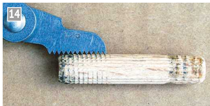
Measuring the pitch from the imprint on the dowel.
