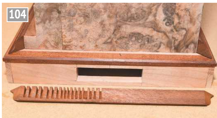
Relieving the back of a moulding for flexibility.
