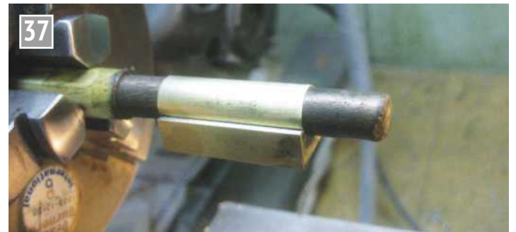
The cylinder bore was lapped using a wooden lap charged with Brasso metal polish.
