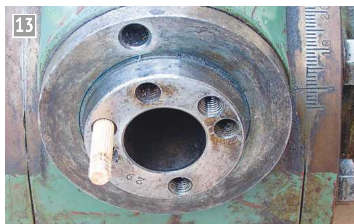
Using a dowel to get an imprint of a thread.
