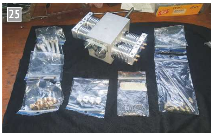
Bags of small components made as a break between the more complicated parts.
