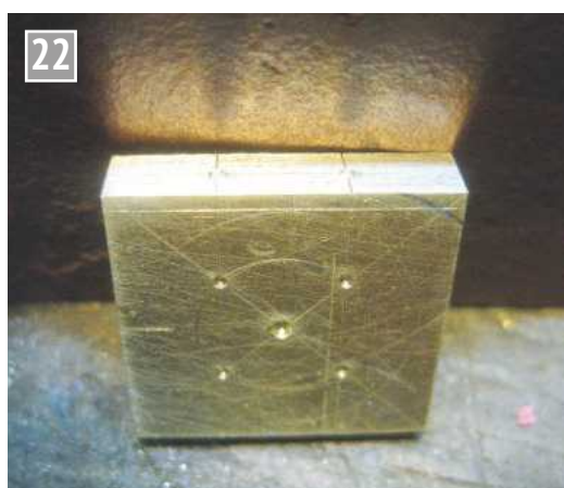
A square of 5mm was marked out to the same dimensions as used on the cylinder frame for the ports.
