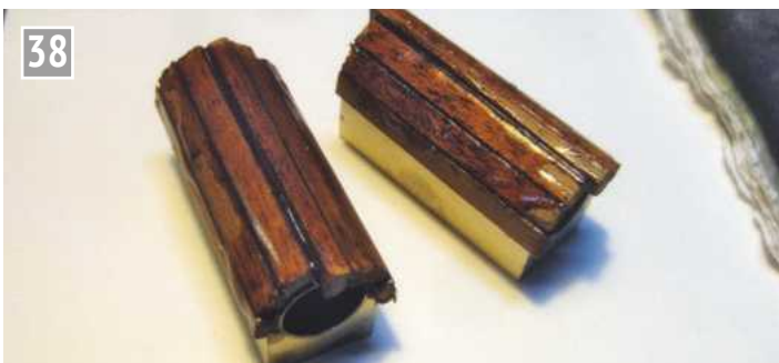
The wall thickness of the cylinder was made up by gluing strips of mahogany to it.
