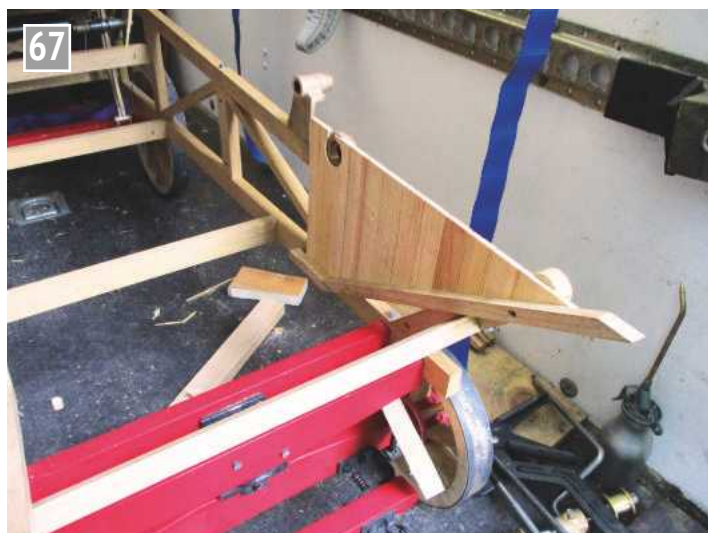
Hopper side fitted to the elevator frame.
