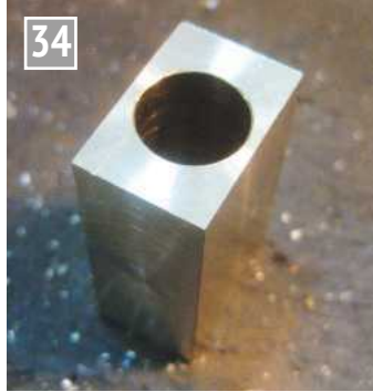
The lathe is used to make the hexagonal rod into a rectangle 32 x 13mm, which is then split to make two port blocks.
