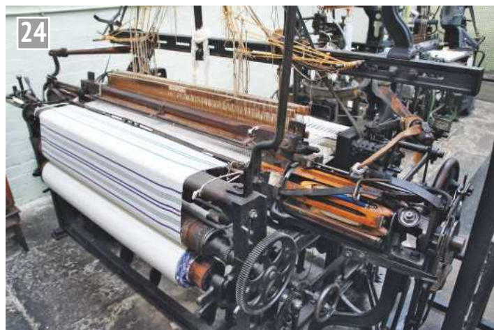
This loom has several shuttles, each for a different colour, to weave a striped fabric.
