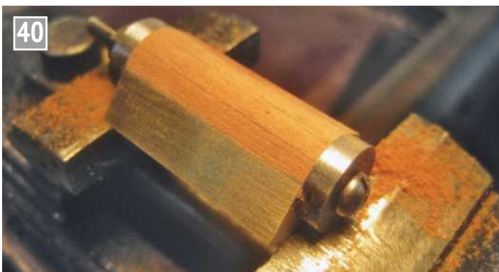
The wood was filed away to these buttons.
