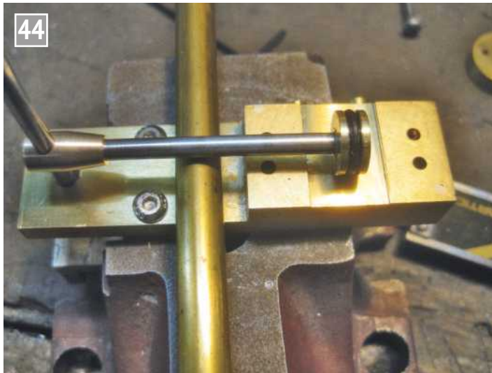
The length of the piston rod was checked using the engine frame as a jig.
