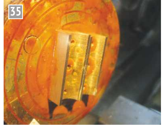
A shellac chuck was used to finish the port blocks.
