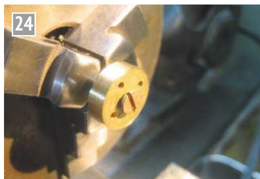
The valve was turned into a round shape and the position of one of its ports indicated with a pop mark.
