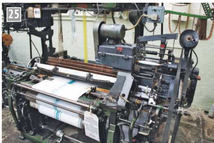
25 A Northrop dobby loom still used to weave glass cloths. Note the string of punched cards top right. Holes controlled operation to weave simple patterns or lettering. (Mill made glass cloths are highly recommended.)
