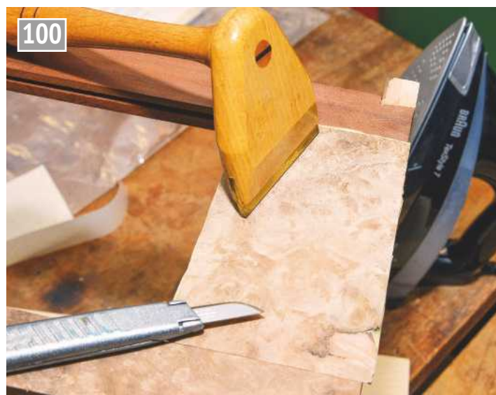
Smoothing the veneer with the veneer 'hammer'.
