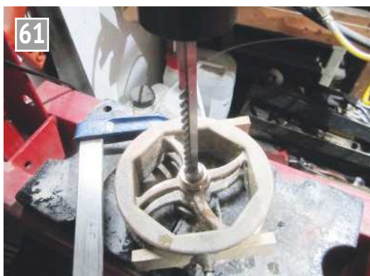
61 Broaching the keyways in the chain wheels.
