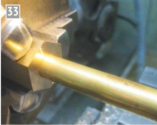
The hexagonal rod is turned to 32mm long and then drilled to accommodate the brass tube.
