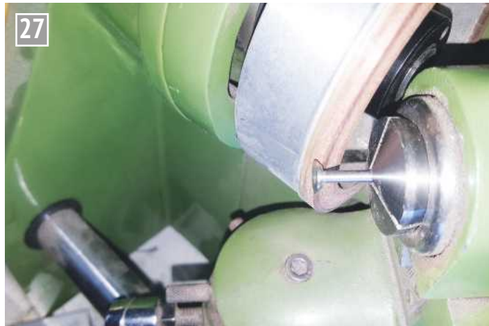
Grinding valve bevel on tool and cutter grinder.
