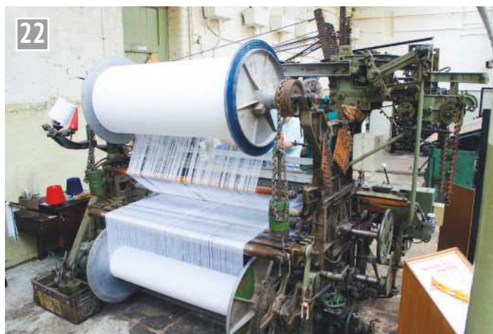
Terry towelling loom with two weaver's beams so that loops can be created.
