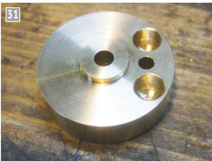
Flywheel with mounting hole for the crankpin and balancing holes.
