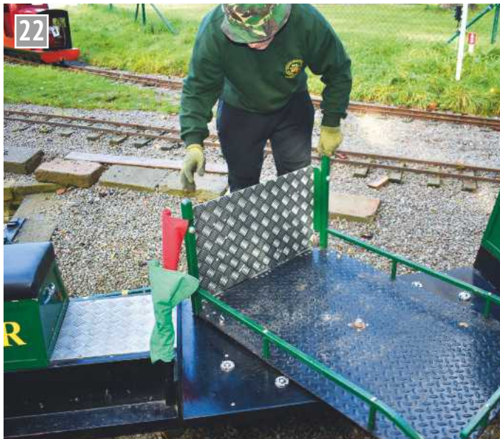
The club-built disability carriage demonstrating the swivel action of the platform.
