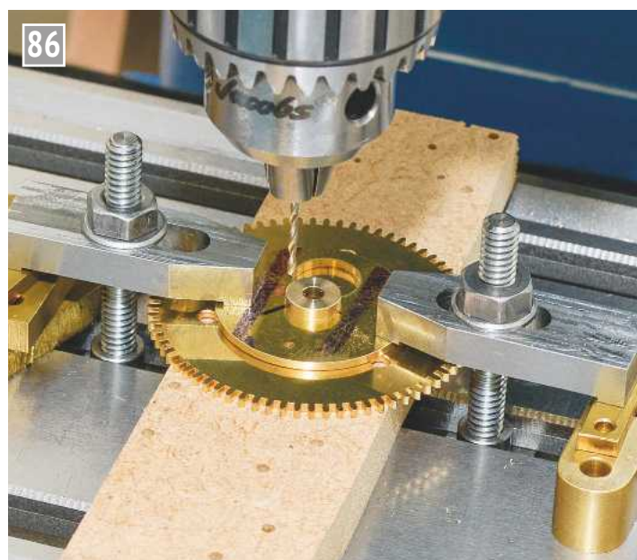
Drilling through the washer and hour wheel.
