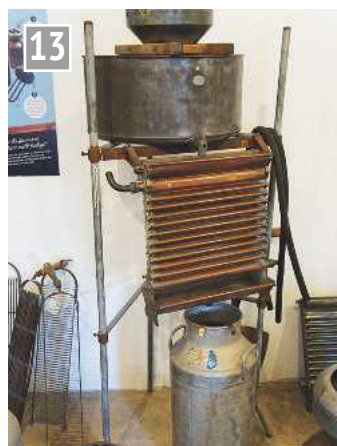
Milk coolers reduced risk of spoilage in transport to markets.
