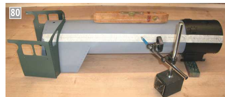
80 Marking out for the handrail stanchions.
