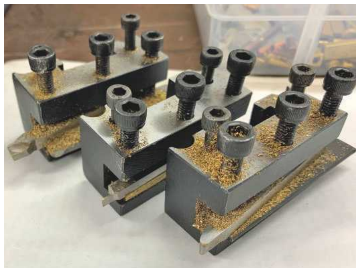
From left to right, knife tool, parting tool (0.025 inch wide) and 0.625 inch radius round nose tool are all the tools required for injector production.
