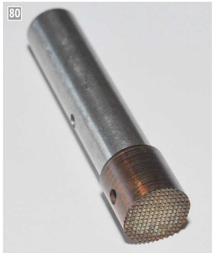
Hardened and tempered matting tool.
