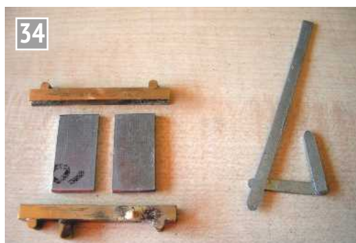
Parts for the firehole door.
