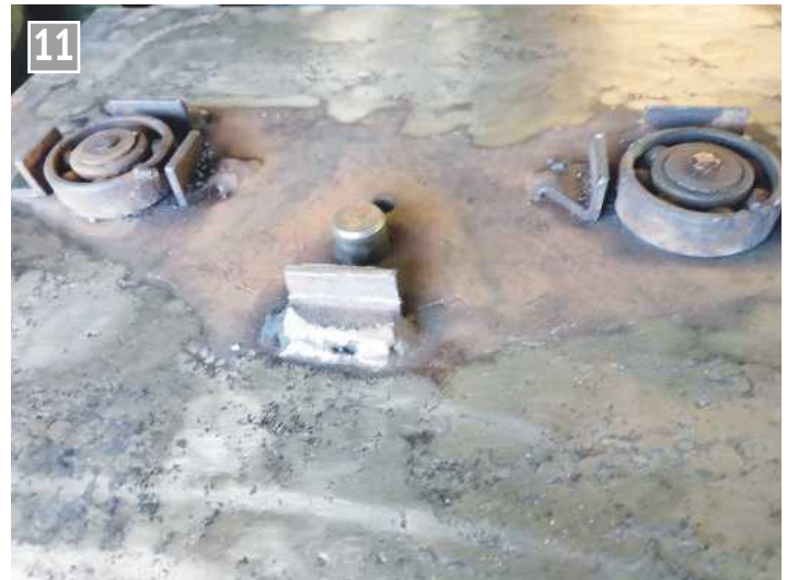
Bogie side frame assembly jig.
