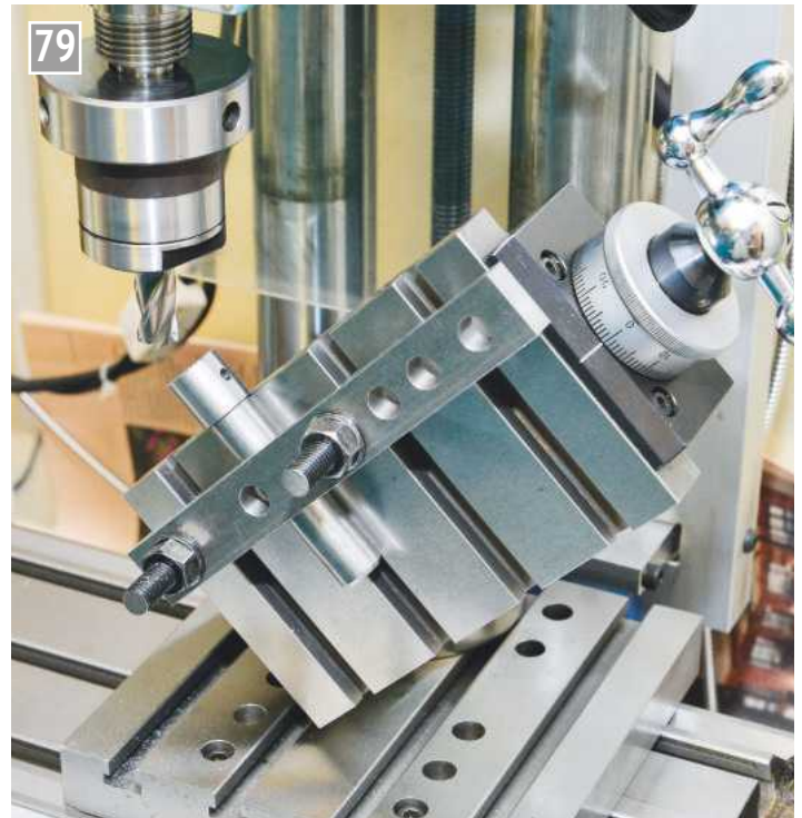
Cutting the pattern on the matting punch.
