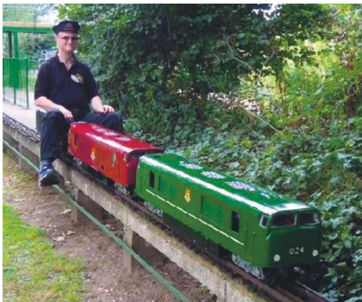
A pair of petrol hydraulic locomotives running in tandem, the creation of Aubyn Mee, Rugby's chairman. The power is provided by Honda industrial engines adapted for this interesting role (photo John Billard).
