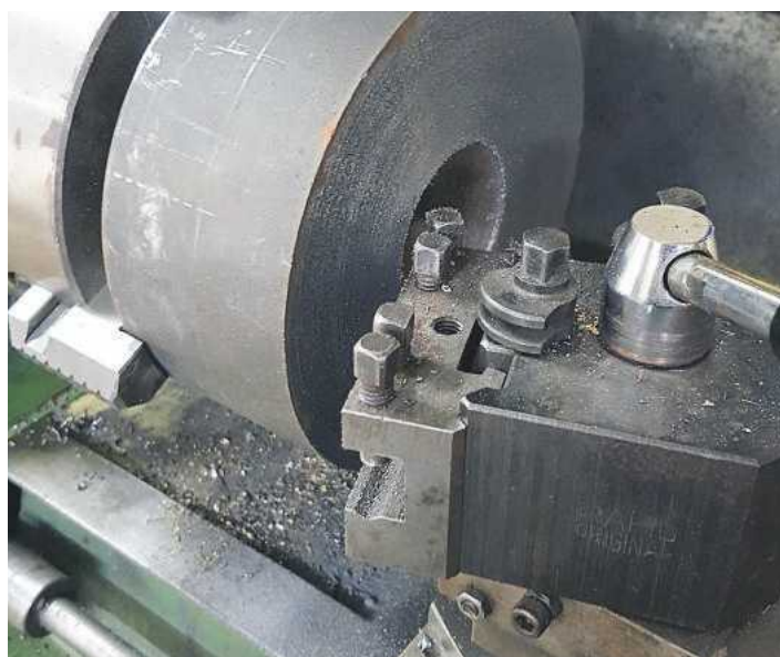
1. This first picture shows the cast iron lump held in the four-jaw chuck having been clocked for concentricity.
