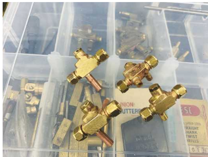
This shows an advantage of designing and making your own injectors. This batch of four are 14oz with 1/4 inch x 40 connections and side water entry. These features are unavailable in commercial injectors, yet ideal for 3.5 inch gauge locomotives.
