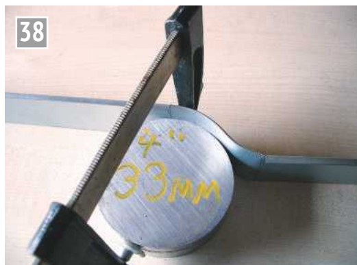
Checking the curve on the platforms.
