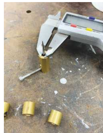
A square reamer with its depth stop holder.
