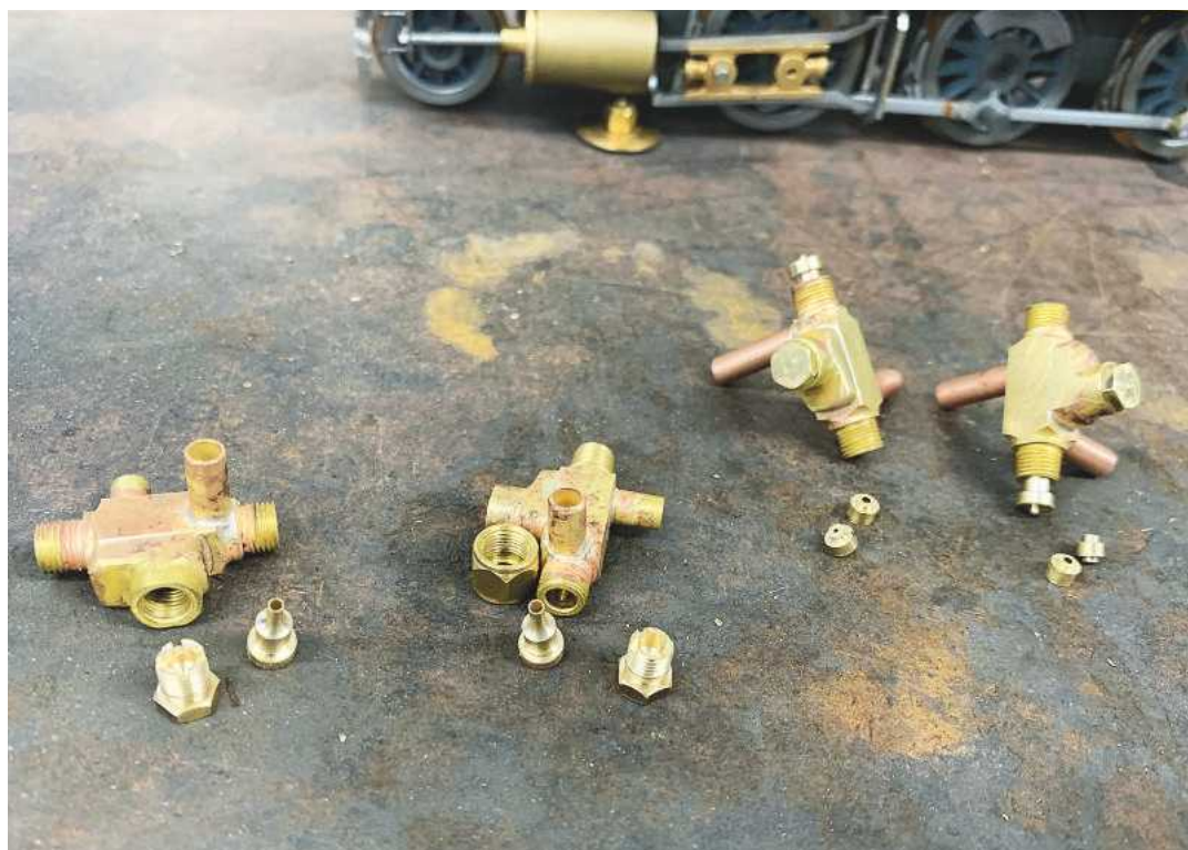
14 oz injector components - note the side water entry.
