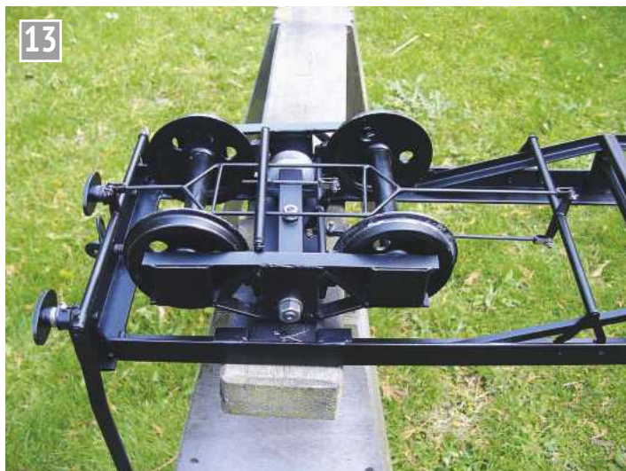
Underside view of the brake gear.
