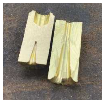
Tests of the taper reamers to check surface finish.
