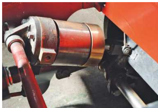
A close-up view of Blyth's steam brake cylinder from between the mainframes.
