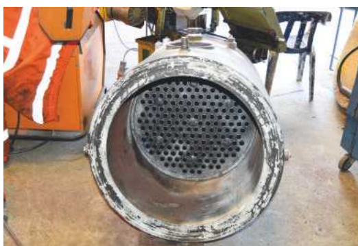
Much of the work undertaken today by N.B.R.E.S.L. is on boilers and not all for railway locomotives. This is a three-quarter (9 inch) scale boiler for a miniature compound Foden steam lorry for a customer in the Republic of Ireland.
