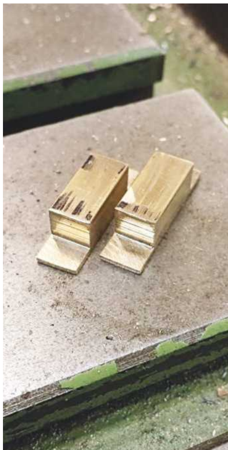
17. Now we come to the oil boxes. The first job was to make the reservoir tanks from \frac{1}{4} inch brass section. Once I had two rectangles of the correct length I machined the end steps that have the holes for the bolts to secure them to the spring plate, as seen here.
