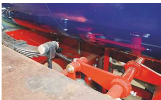
A view looking into the leading left hand area between Blyth's mainframes showing the left hand drop link and overhung leading spring, along with part of the right hand expansion link.
