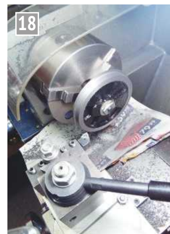
Wheel profile being rough machined.
