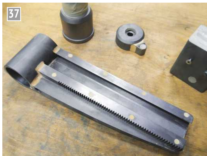
Fillets added using filler.
