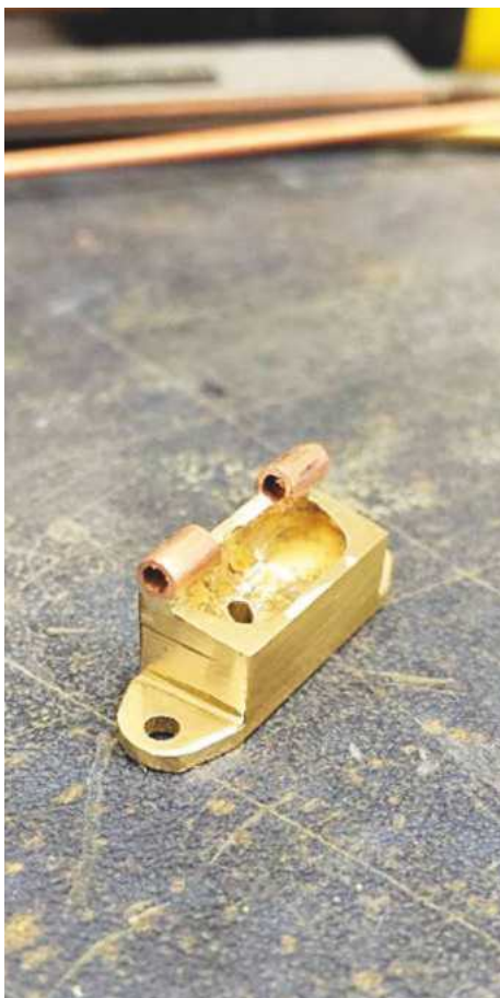
18. After some machining, shaping and silver soldering on the hinge we arrive at the nearly finished tank. The top is sloped 10 degrees, the hinge has been added and the end tabs have been profiled to shape although not quite there yet. I also needed to do a little more draw filing to get the case nice as this isn't a painted item when finished so needs to be good. The small oil hole has been drilled into the bottom of the tank at an angle - this hole will continue through the spring plate and the wedge so that all of those parts get oiled from the one tank. This I did once the tank had been fitted to the spring plate.
