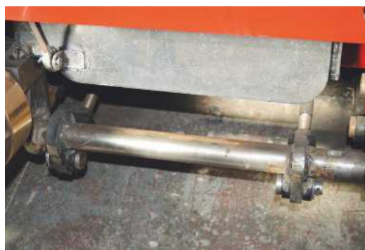
A view of Blyth's brake cross-shaft and the lower part of the rear ashpan damper.
