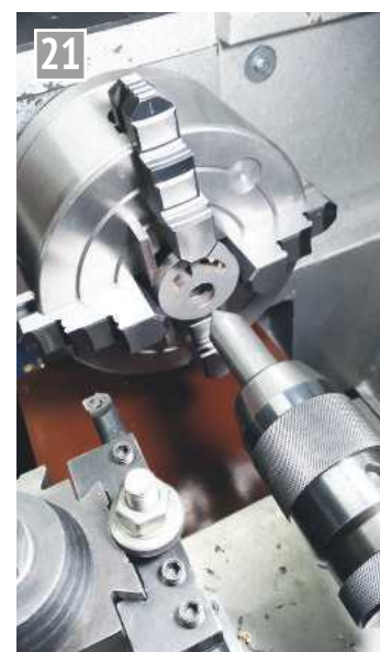
Eccentric shaft hole alignment in the four-jaw chuck.
