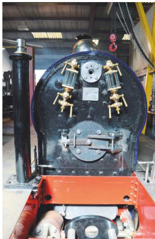
Blyth's backhead area showing the water gauge glasses, firehole door, rear coupling mounting and steam brake cylinder.
