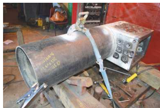
Another boiler job – this time for a 15 in gauge loco of Kerr, Stuart 'Wren' inspiration on the Sherwood Forest Railway. Welding work on this boiler was in progress during my visit.
