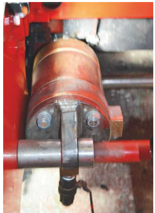
The rear of Blyth's steam brake cylinder and its mounting on the inside of the left-hand mainframe.
