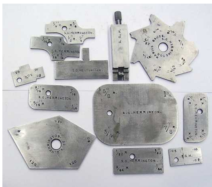
A remarkable collection of gauges all stamped with S.G.HERRINGTON or S.G.H. Also, there is a small tool, the purpose of which I am unsure of except that it looks as though it was designed to grip something – the finish is excellent as are all the gauges.
