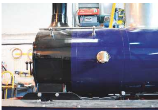
A close-up of the left hand leading area of Blyth's boiler barrel, showing the clack valve and handrail. This view shows well the fact that the smokebox is lagged (hence the cladding) and the fact that the steam pipes have yet to be fitted.
