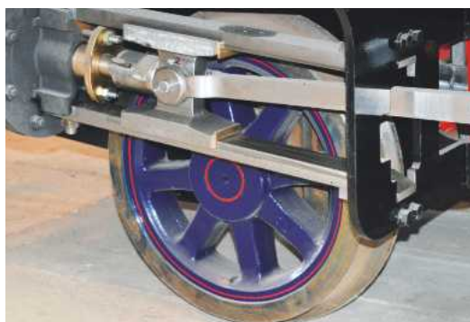
The left-hand leading wheel area of Blyth showing the lower part of the motion bracket, crosshead and slide bars, leading forked end of the connecting rod, securing cotter for the piston rod, gland and rear cylinder cover.
