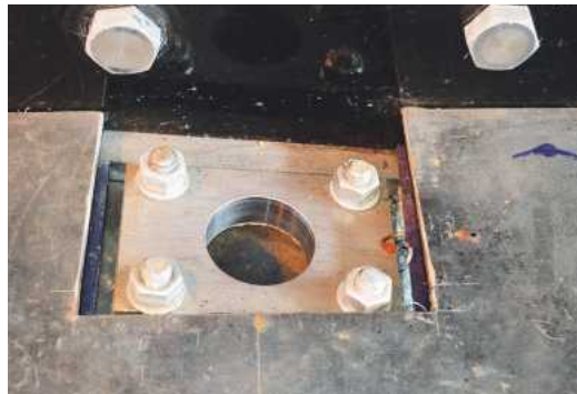
Blyth's left-hand steam chest cover showing the entry point for the steam pipe.
