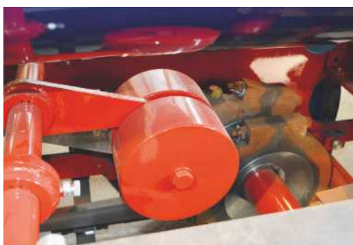
A view of Blyth's weighshaft balance weight and right-hand eccentrics.
