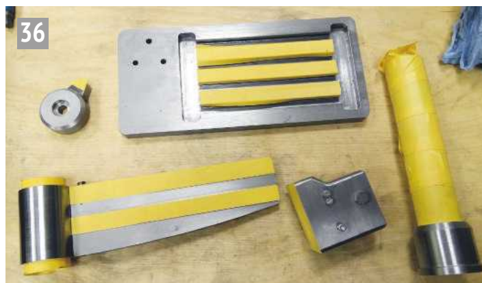
Parts masked up for sandblasting.
