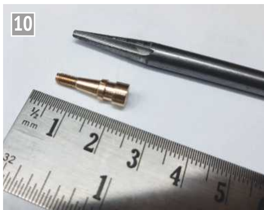
Tapered cock inner and matching reamer.
