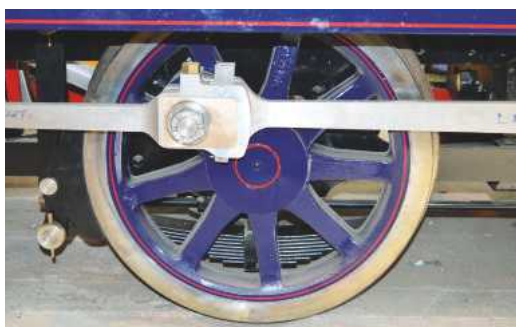
Blyth's leading left-hand coupled wheel showing similar detail to the previous view, but this time also showing the rear of the connecting rod.
