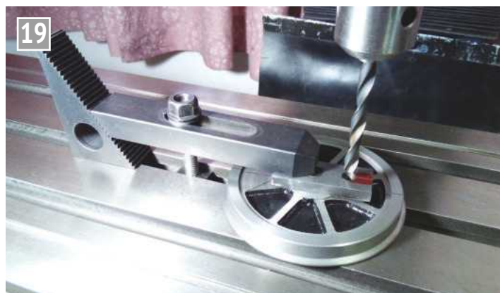
Drilling the crank holes with a drilling jig.
