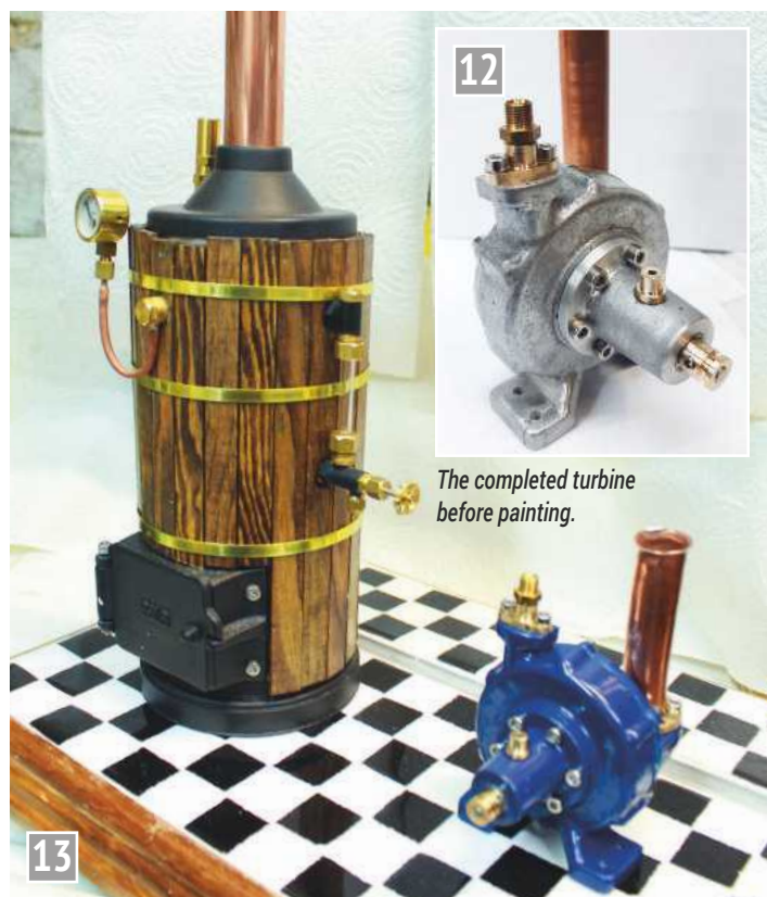
Turbine teamed up with its boiler.
