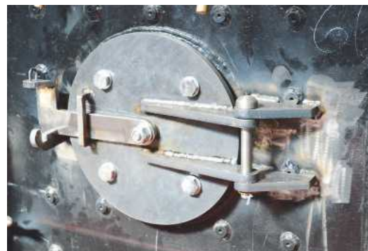
Another close-up view, this time of Blyth's firehole door. Welded construction is once again very much in evidence.
