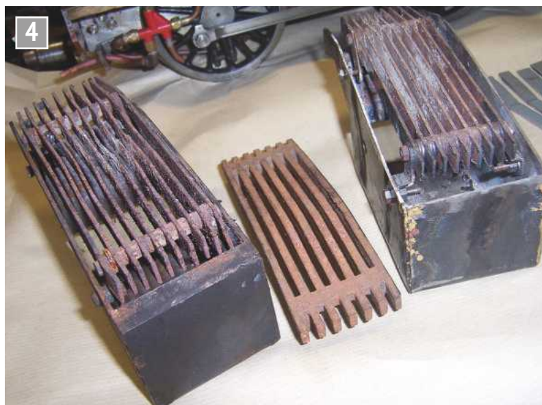
Old and new-ish grates.
