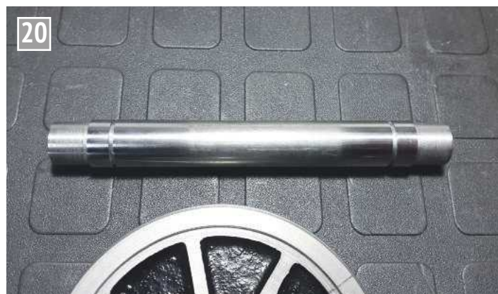
Machined shaft ready for press fit.
