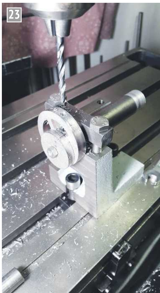
Machining the set screws in a 'V'-block.
