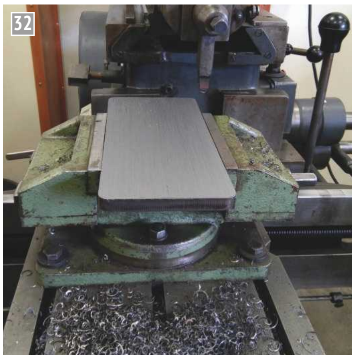
Improving the surface finish on the shaper.
