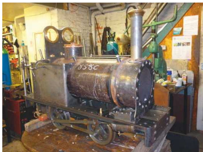
One of the earliest projects undertaken by the company was the construction of this 7 1/4 inch replica of Sir Arthur Heywood's 15-inch gauge 0-4-0WT Effie of 1875. It is seen here, nearing completion in the Scarborough workshops on March 16th 2015.
