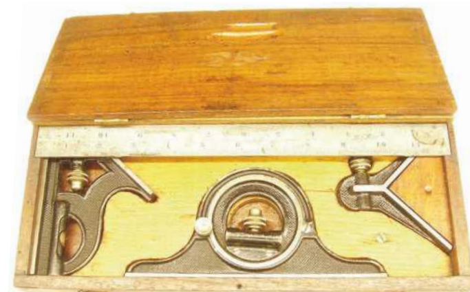
Finally we come to something a little different... A combination square set with a little something extra. It is marked H.J. Fox and made by LSS Co. (i.e. Starrett). The wooden box is very much an engineer's woodworking effort but is still effective. I must have had this for 20+ years and only now have I discovered its extra secret, which, in the best tradition of cliffhanging episodes on TV etc., I shall reveal in the next article!
