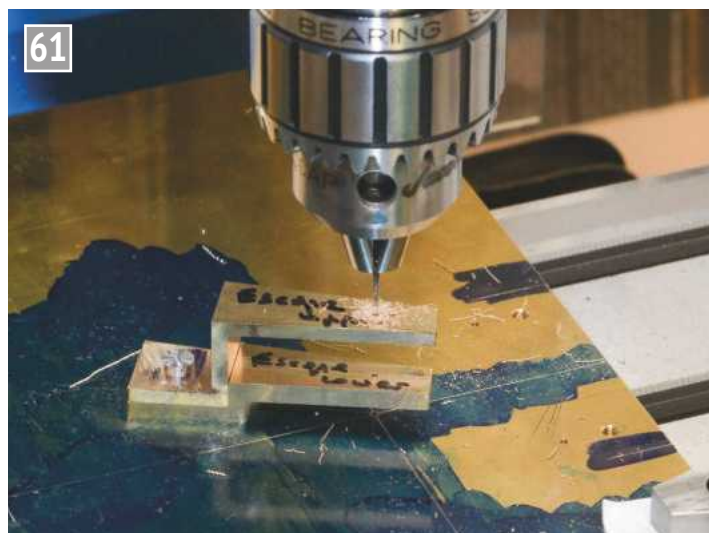
Drilling the double cock in situ.
