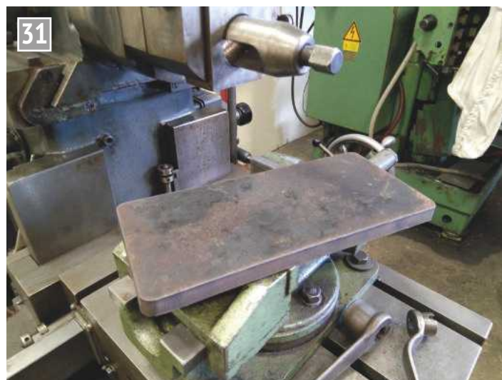
Base cut roughly to shape.
