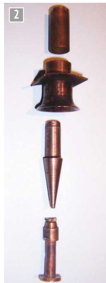
Blast pipe height gauge.
