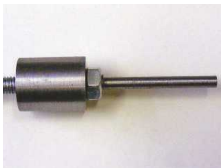
Mike Cox details a spindle back stop.
