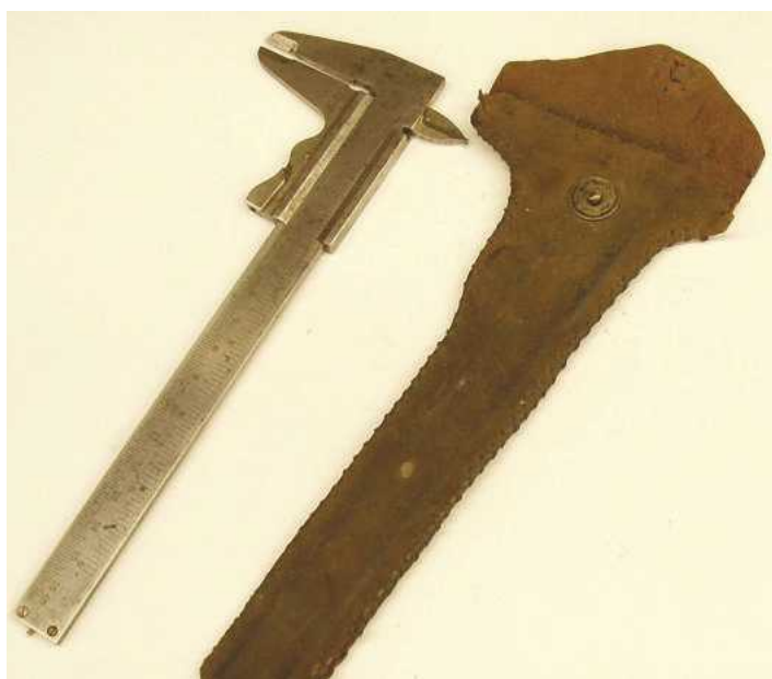
Another of my grandfather's tools - the vernier caliper is calibrated in mm and (look closely) fractional inches. I confess to be not too good at reading them!
