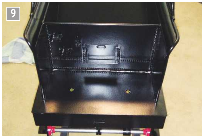
Some corner spraying on the Stirling tender.
