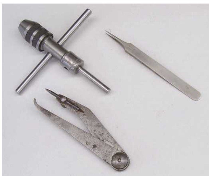
The tap holder is so easy to use, putting the stem into the vertical drill or mill – they should all have one! The jenny calipers I use frequently to get a centre line and the jeweller's tweezers to pick up small items and remove metal splinters....!
