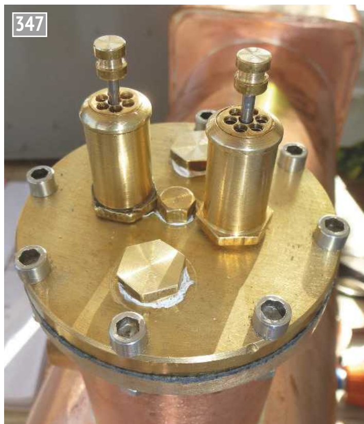
The 0-6 -0 dome and safety valves.
