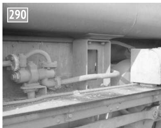
Right-hand injector on 3673 but no water valve.
