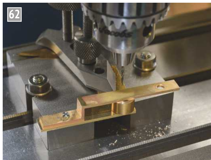
Drilling the swing arm assembly, using a spacer to avoid flexing.
