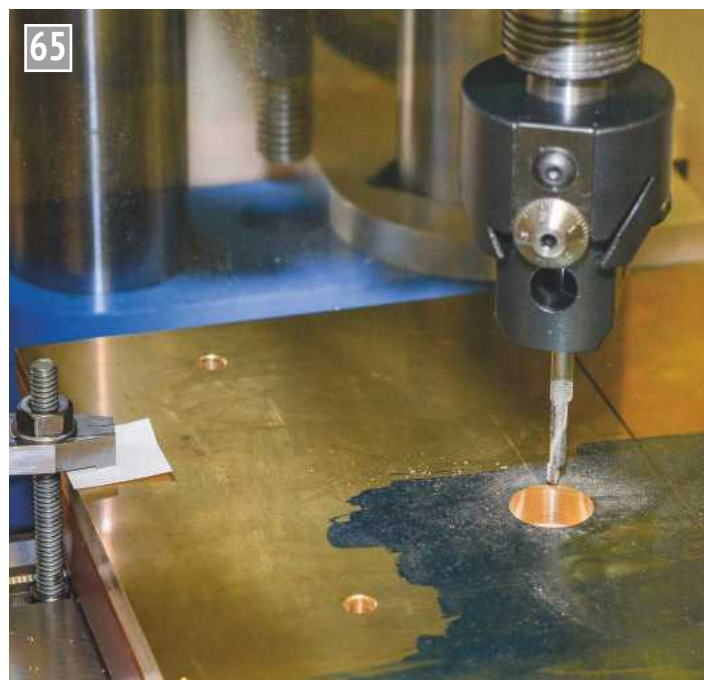
Boring the hole for the fusee ball race mounts.
