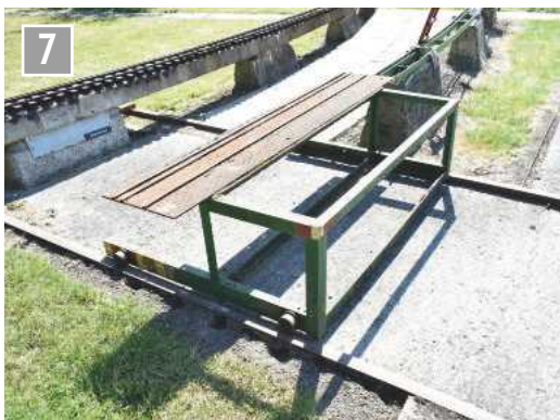
The steaming bay traverser for access to the running line.
