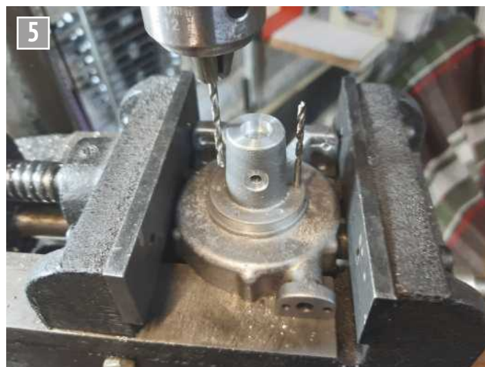
Spotting through the fixing holes on the bearing housing.
