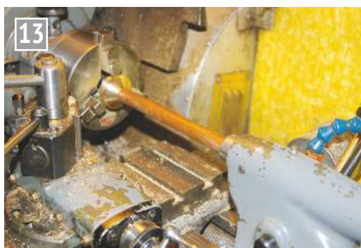
Using the lathe to align the water pipe with the base.
