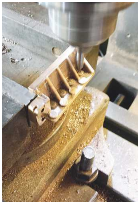
5. I then held the other horn of the matched pair for the one side and placed the horn already drilled on top, aligning it by placing steel blocks to the side and back. This was just to get the hole in its correct position height-wise - its depth is determined as with the first by being held by its machined step in the machine vice. All holes were centre drilled first. I then drilled all of the mounting holes except for those that are on the leading horn closest to the horn cheek as it's not possible to drill these from above due to the angle of the horn.
