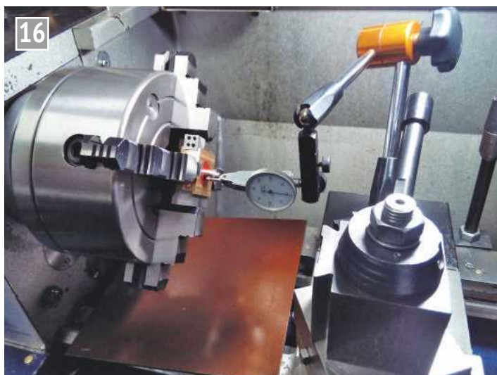
Setting up the shaft hole for the back axleboxes.
