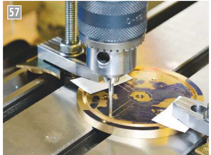
Tapping the holes for securing the pallet keeper plates.
