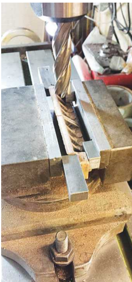
3. Next was to machine the last of the three edges. As can be seen the casting was packed out either side of the horn stay supports and also had packing underneath. It didn't matter that the horn supports hadn't been machined square yet, the important thing was to have all three faces machined so far square to each other. With those three faces done I then moved on to the step to fit the frames. This left the one main face to machine, that being the 17 degree running face for the axle box. The castings were cut into singles and in turn set up in the tilting vice set to the required angle. I left these slightly oversize until the axle boxes were done, then fitted them to the trailing frames and trued them up. It was then back to the machine vice to finish all the other parts.
