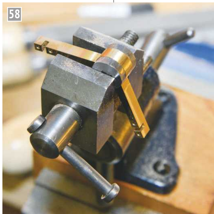
Using filing buttons to form the boss on the rocking arm.
