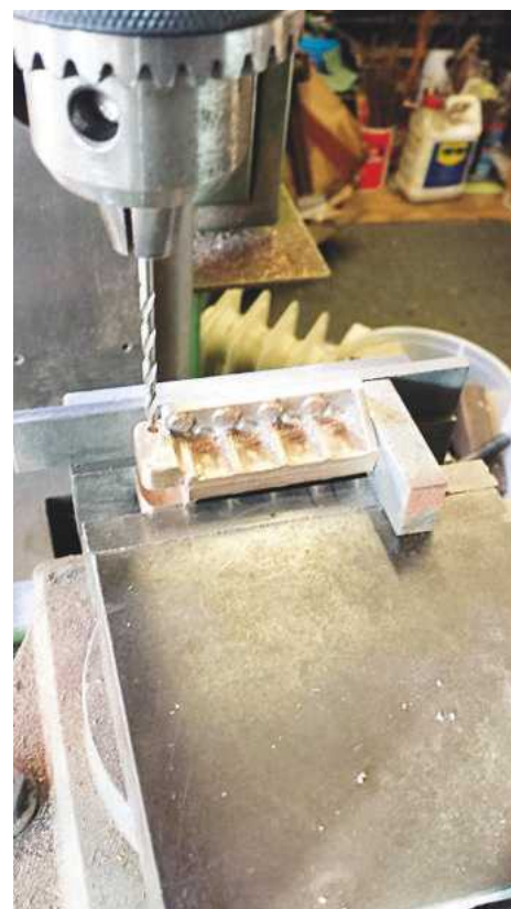
4. On to some drilling. First, I drilled the two holes in two opposing horns for the hornstay bolts to fit into.
