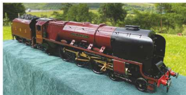
A gauge 1 Aster model of a 4-6-2 London Midland and Scottish Princess Coronation Class tender locomotive No 6233. 'Duchess of Sutherland'
