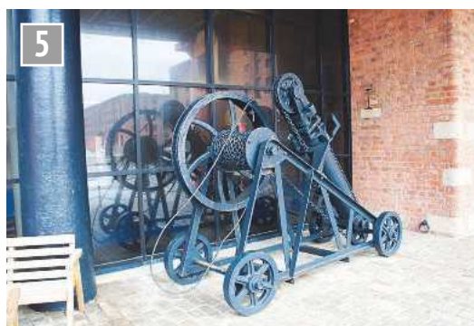
Hydraulic 'jiggers' provided portable lifting power around the docks when connected to hydraulic mains.
