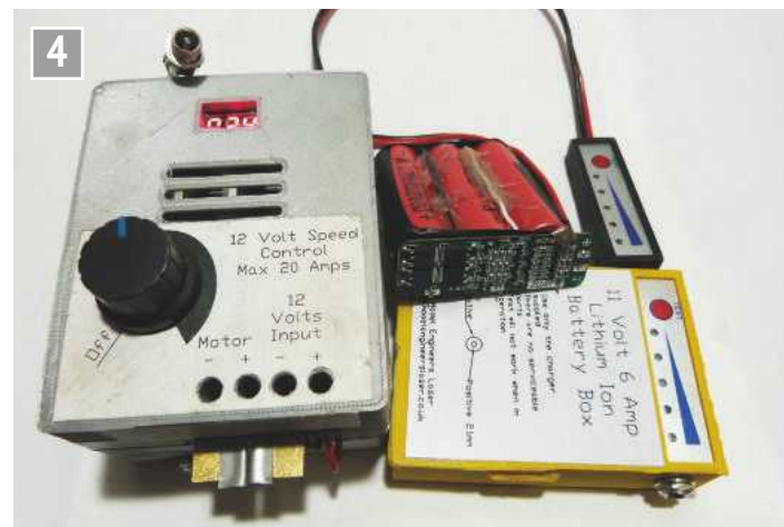
A home-made battery pack, battery checker and speed control.
