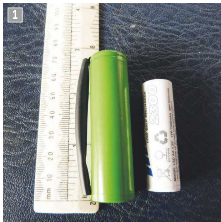
A single 18650 lithium ion cell compared to an AA battery.
