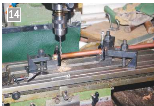
Cross drilling to secure the pipe to the base.
