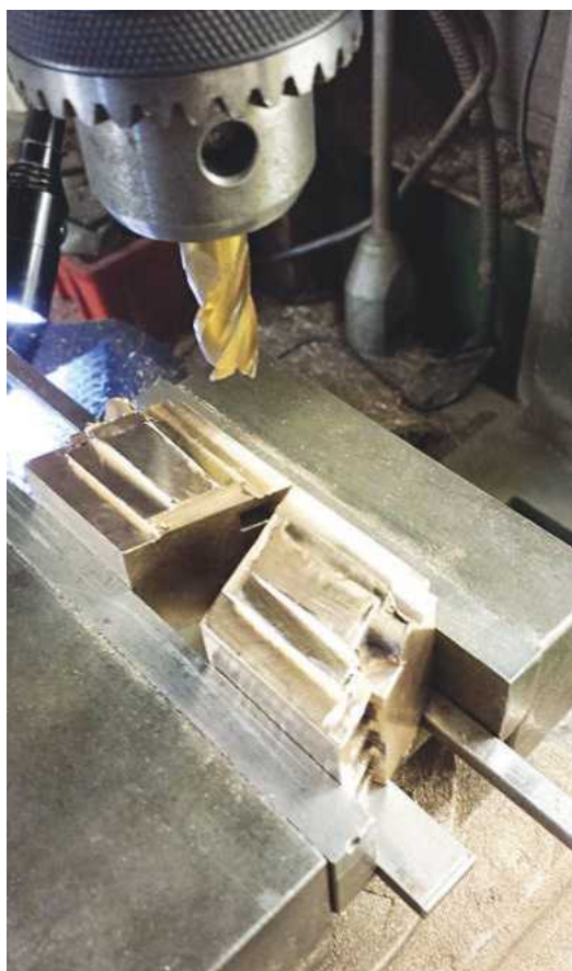
13. Using packing to clear the lower spigots I held both axle boxes in the machine vice to ensure they are both the same size. I was surprised that I only needed to take a couple of thous of the top to keep the wedge at the correct height clear of the step below.
