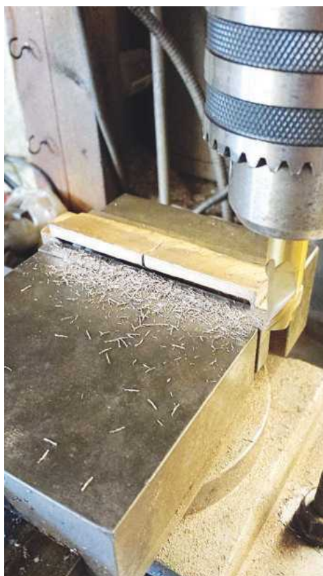
2. With the machine vice checked for squareness to the mill head (I tend to do this now and then for peace of mind), I packed up the horn castings from underneath and behind and machined the opposite edge square.
