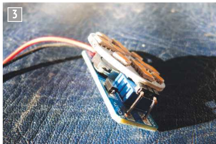
A 12 volt LED with charge pump attached to run on a single cell.
