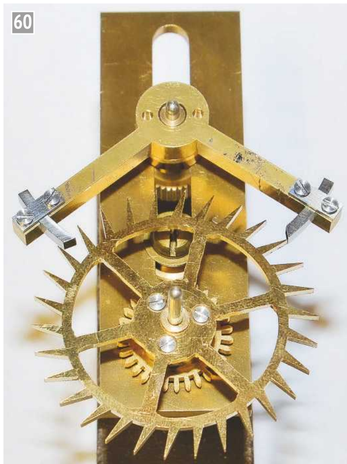
Setting up the escape wheel and pallets in the depthing tool.
