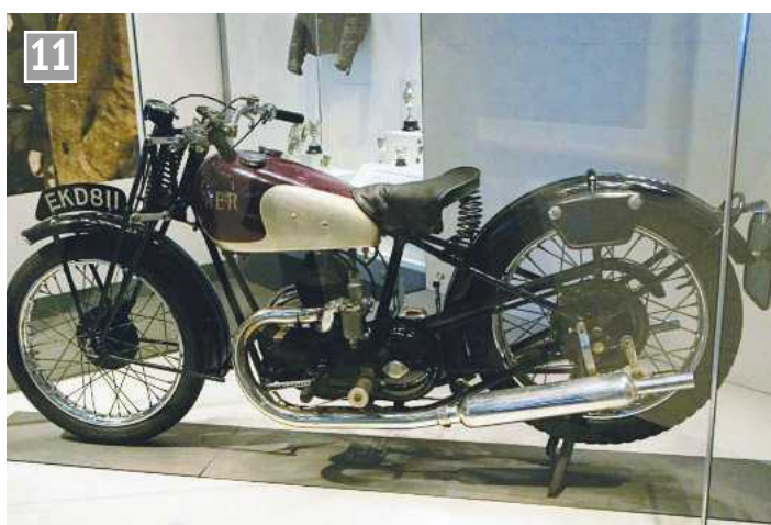
AER 250cc motorcycle made in 1938. Albert E. Reynolds was a motorcycle retailer who branched out into making bikes like this with a 250cc Villiers engine. He supported the TT races and did well with these high quality machines.
