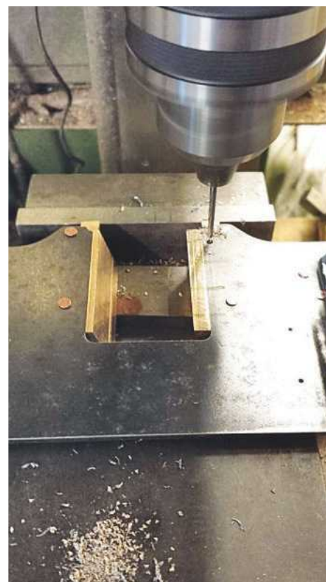
6. I then lined one horn up with its frame, clamped it in position (ensuring it was held tight against the frame opening via the machined step) and drilled through from behind from the two holes mentioned, riveted it in place and then did the same with the other horn, checking height using a depth gauge with a suitable drill bit placed through two of the horn stay bolt holes. Once happy with the horn positions I drilled another hole in each, this time from the front, and riveted in place. It was then back to the machine vice and this time the holes closest to the leading horn cheek were marked out and drilled from the back. With these holes drilled it was a simple task to turn the frame over and drill all remaining holes through the pre-drilled holes in the horns. ➤
