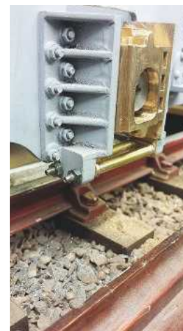
23. Finally the stays are bolted to the horns. I have fitted them with the threads towards the rear. Prototype pictures show them in both orientations so I've followed good mechanics practice - always fit threads to the rear to avoid dirt build-up. I'm sure the same should apply to a locomotive but I stand to be corrected of course...
