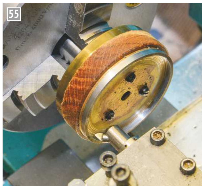
55 Turning the gauge plate ring for the Villaimy pallets.
