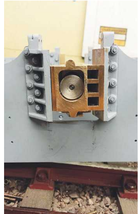
20. Here's one of the axleboxes with its oil tray recess machined using a 6mm long series cutter. For those not familiar with this design the axles have to be pushed in at an angle and then locked in place when they are parallel with the journal. Once the oil tray is in place everything is locked down, so to speak.
