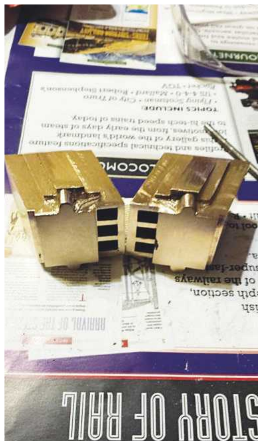
14. The last job for that day was to file off all burrs and clean up the spigots/wedges a little. I finished these once the oil tray covers had been made, using the covers as a jig to get both spigots the same.
