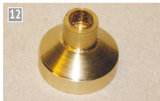
The finished counter electrode base.
