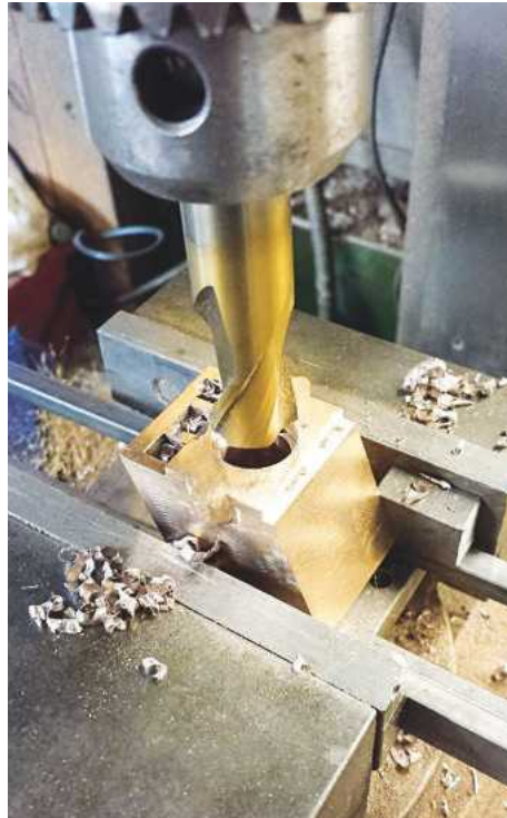
19. Once the bore had been reamed to size it was time to open up each end of the journal for the axle to fit in. This involved using a 'D' bit (I managed to find the same bit as used for the tender boxes), doing the front first and then the back.
