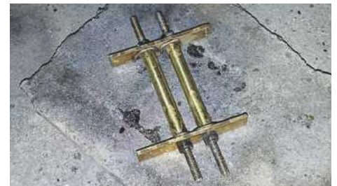
22. Finally we have the hornstays. The drawing has these as steel but I have cheated with suitably sized telescopic brass tube doubled up (two tubes telescopic) both for extra strength and to bring it up to the size needed. I believe this is more than adequate for the job, being held between very substantial horns. Here are the various parts before being silver soldered together.
