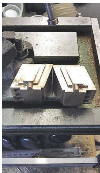
15. The next day, I cleaned up the spigots a little more using a 2mm cutter – the smallest that I had at the time. The spigots are still about 20 thou oversize which will be taken care of once the covers are finished. Mind you these parts won't actually be visible - the prototypes seem to have a dust shield that hangs down from the wedge control plate that sits above. It looks like they are made out of some sort of material, perhaps rubber, I'll see what I can find that's suitable. There's also a metal dust shield that's bolted to the leading horn - I plan to add this detail later too.
