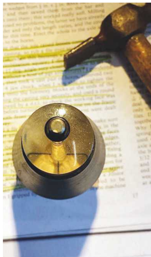
17. Then I did a little 'old school' work using an optical punch to spot the centres. There is an axlebox under there somewhere - honest...
