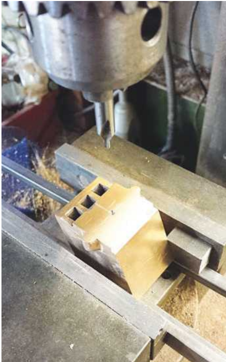
18. With each box in turn back in the machine vice, I drilled the \frac{1}{2} inch hole, first using a centre drill followed up by a series of drills and then the bore finished to size with the reamer.
