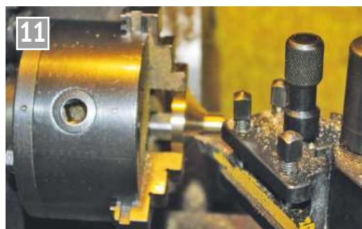
Turning the base for the counter electrode.
