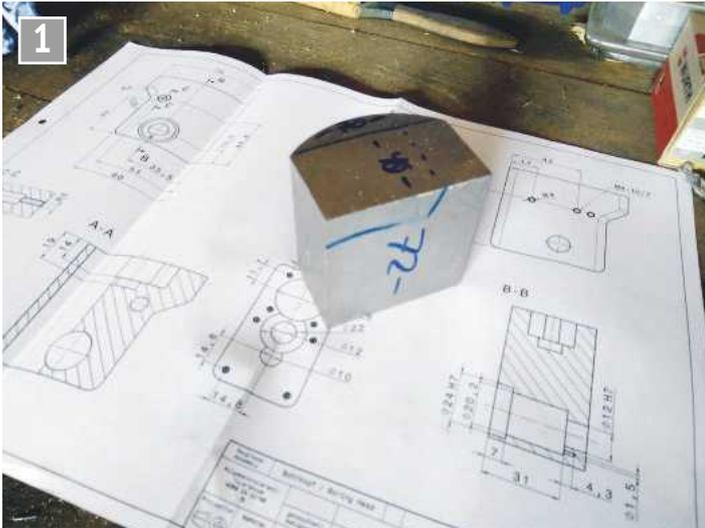
1 The rough shaping of the radial borer body.
