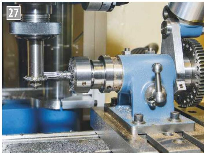
*Cutting around the pinion for the third time.*
