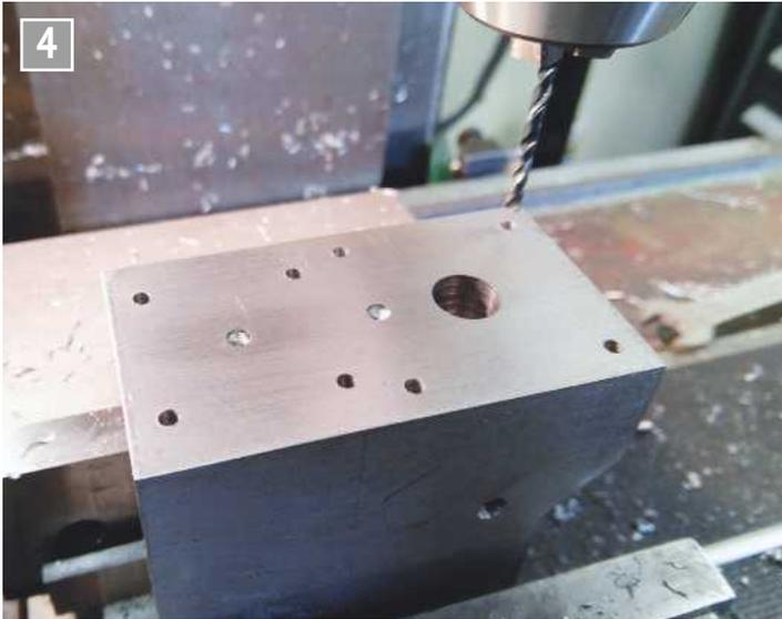
Accurately drilling the fixing and reference holes.
