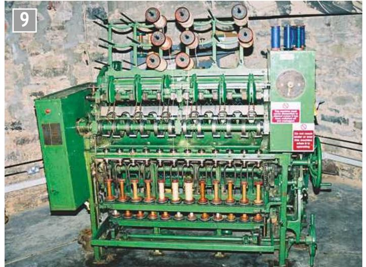
**9** Using the flyer spinning principle, slivers come from the rove bobbins above to be drawn out and twisted.
