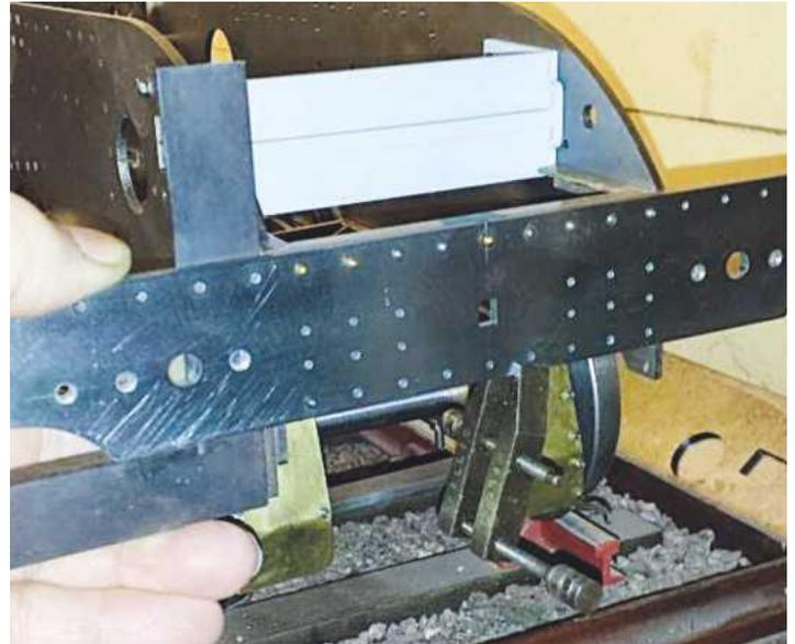
4. Continuing with the front end here's the front buffer beam having had all of its holes drilled and countersunk where needed. The picture shows the beam being checked that it was level and square with the bottom bracket only being used to hold it in place.
