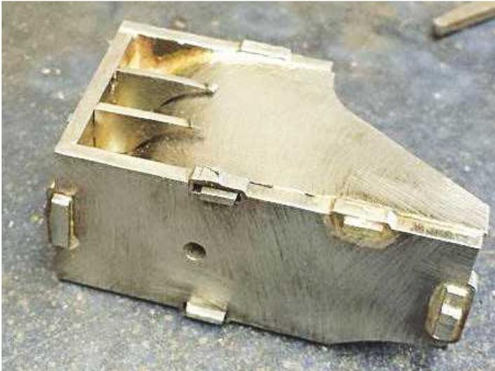
12. After being silver soldered together and cleaned up the webs were checked for fit. These were then soft soldered using a high melting point soft solder as they do not need silver soldering, being tucked away out of sight and harm's way. Note the tab that hasn't penetrated with silver solder yet - this was completed before any soft soldering was done.
