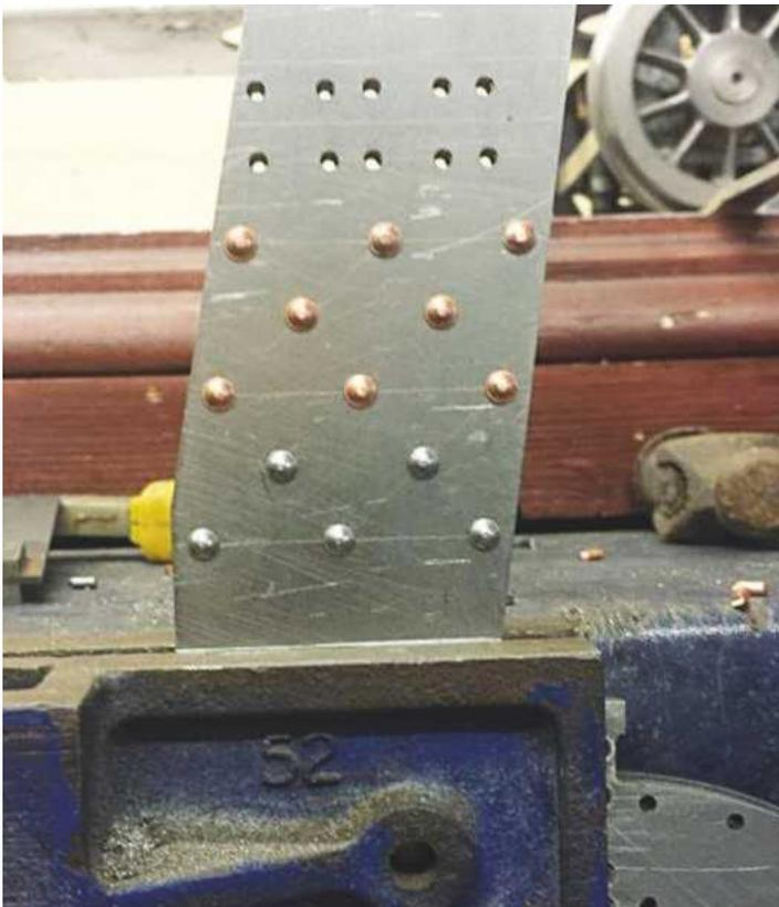
17. Next job was to place the frame in the vice along the marked line and do it up very tightly. A square was also used here to check that the frame was sitting upright. Using a 2lb club hammer and a piece of wood the frame was persuaded to bend to its correct position which is  $\frac{5}{16}$  inch from upright or parallel when assembled and viewed from above.
