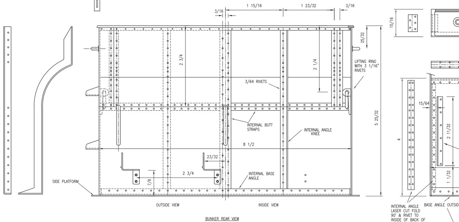
NOTE THAT ALL PLATE SIZES IN LASER CUT SET ARE GOVERNED PRECISELY BY PLATE THICKNESSES SO DIMENSIONS ARE A GUIDE ONLY
