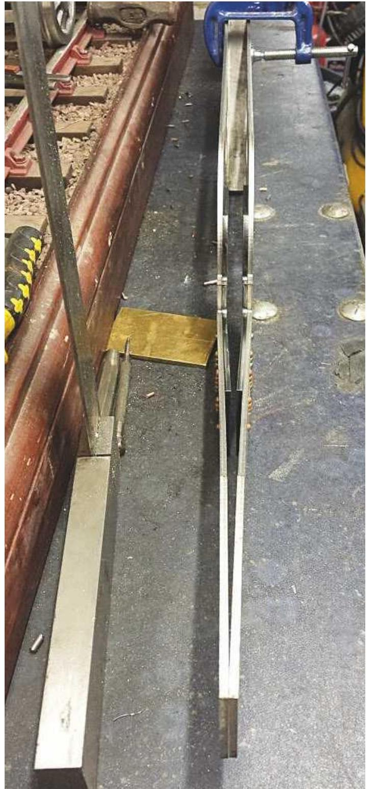
18. Just to check that all was going to plan I held a  $\frac{5}{16}$  inch piece of steel bar between the frames and clamped them together. The method used to form the taper worked very well as can be seen in this picture.
