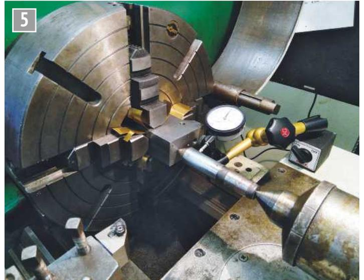
Centering up the body on the lathe.
