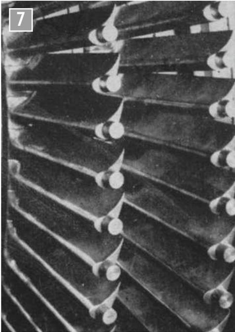
Reaction blades partly assembled in a Westinghouse steam turbine rotor. The blades have very rounded entry edges. The circular extensions on the end of each blade are for attachment of shroud bands which had not been fitted when the photograph was taken. (From fig 7.12 in ref 36)
