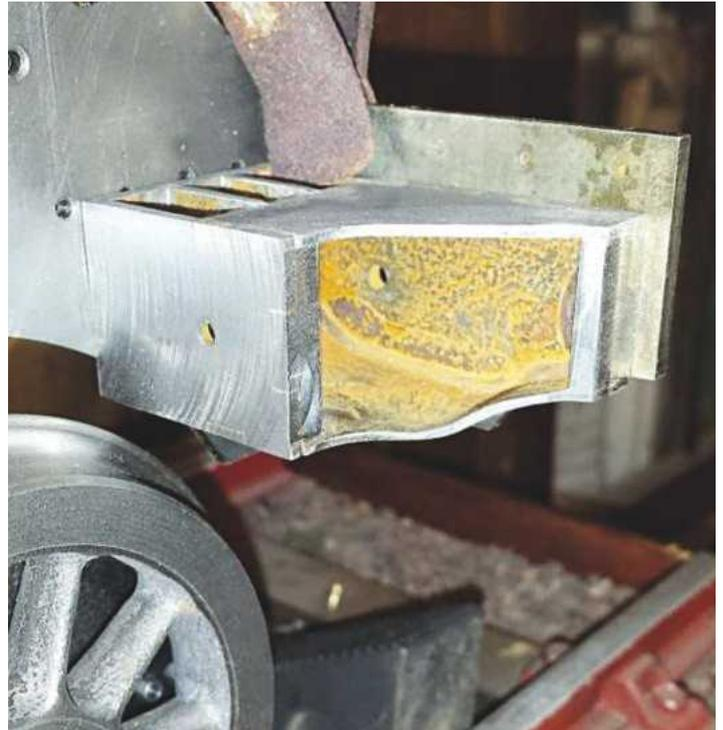
13. Here is the housing after it had been machined square and held in its correct position (the holes half hidden are holes that I drilled wrongly for the top buffer beam support - whoops), I will transfer the mounting holes once the frames have been parted as it's not possible to get a proper alignment as it is. I'm very pleased with how these turned out and even more so when I reached the stage of fitting the buffer stocks and heads.
