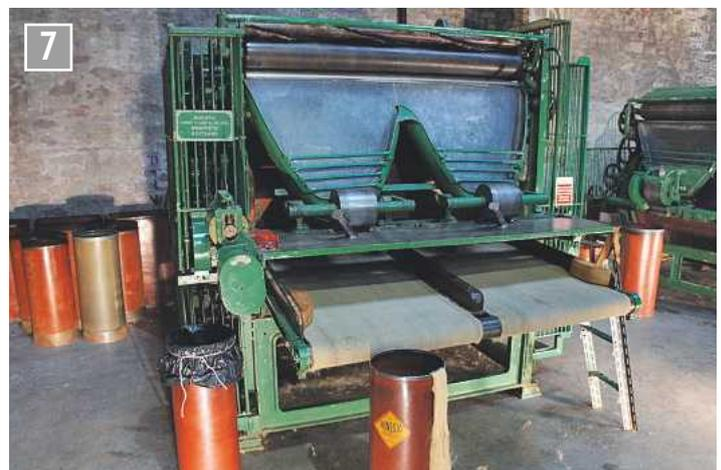
The finisher carder takes jute slivers from the breaker and passes them up the feed cloth to be further mixed and aligned.
