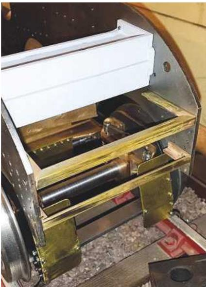
1. Here we see the beam stiffener brackets, made up from  $\frac{1}{4} \times \frac{1}{4} \times \frac{1}{16}$  inch brass angle, fitted between the frames. As usual they only have two holes drilled and tapped for now and they still need cleaning after soaking in the acid.
