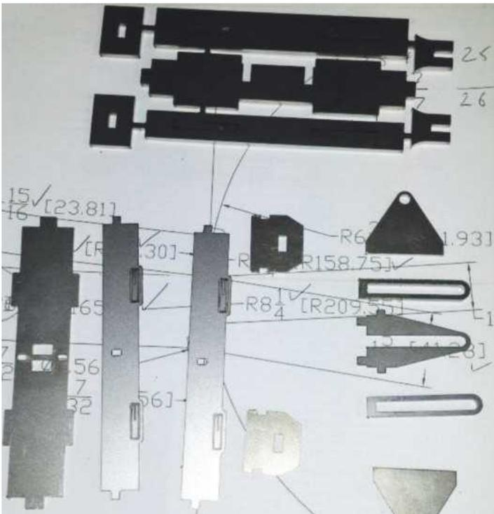
5. This picture shows the kit of parts for the vacuum cylinder stay as supplied by Malcolm. This is a fairly easy part to make but it would have taken some time to cut out these shapes by hand and also been a little bit more involved in holding the parts together for silver soldering. This is where the 'slot and tab' method comes into its own.
