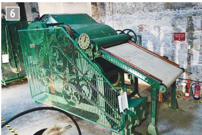
The breaker carder is the first carding machine, aligning fibres in one direction using rows of pins on a giant rollers.
