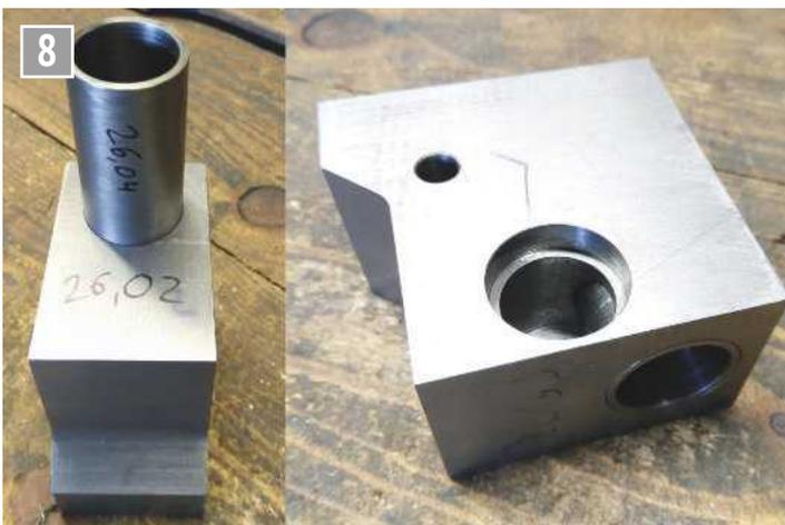
the centre in the tailstock and the midpoint, which I drilled before on the workpiece. After that, I placed an indicator on the dead centre and adjusted the jaws on the chuck until achieving the runout that I wanted. On my lathe I can use
