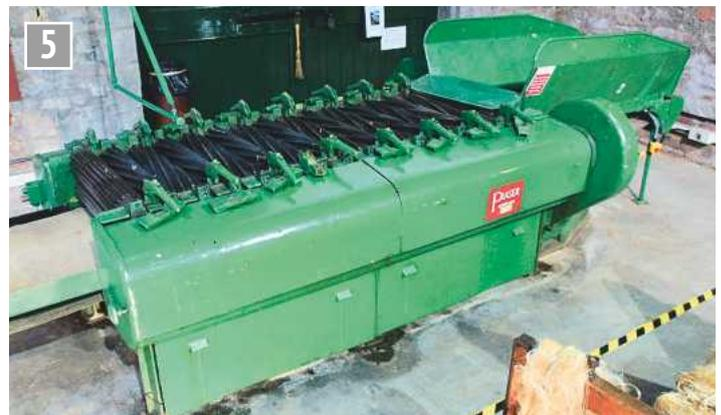
Softener machine. Jute is moved between fluted rollers and sprayed with an emulsion of oil and water. It is then left to soften. Raw material is shown, lower right.
