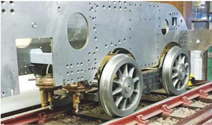
7. Here is a picture of the vacuum stay arrangement to show the overall positioning of the vacuum cylinders in the frames.
