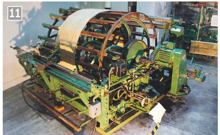
**11** The beaming machine created the weaver's beam holding the warp threads.
