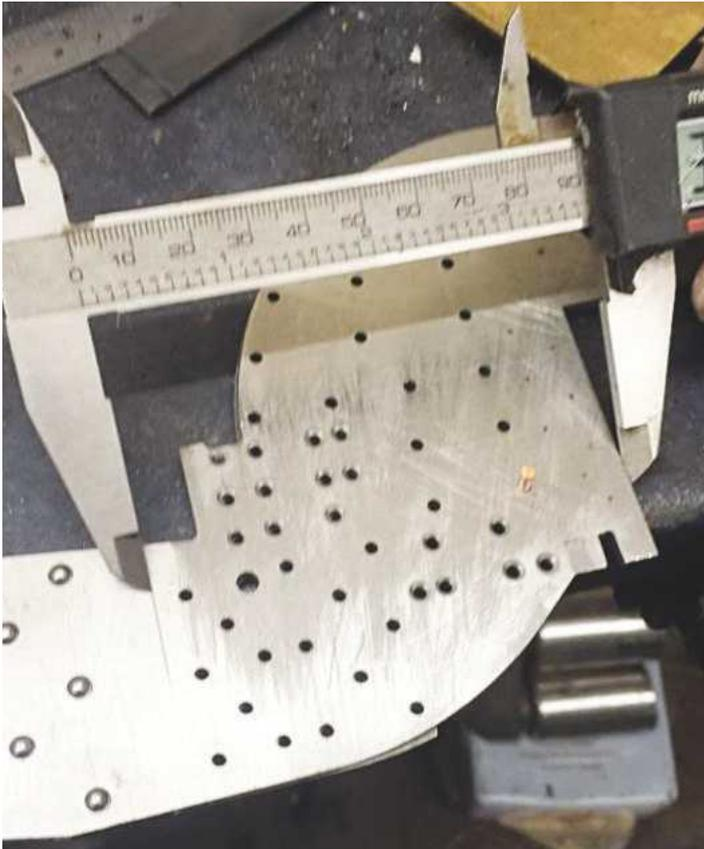
16. With the position for the bend marked I used a vernier caliper to take an accurate measurement from the rear axle slot so that I could duplicate the mark for the other side.
