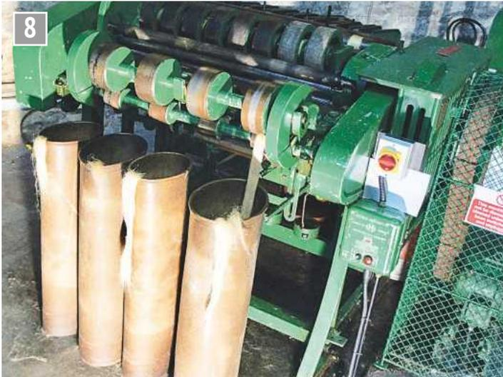
**8** Drawing machines produce slivers for the roving machine. These reduce slivers in size and weight operating with two sets of rollers rotating at different speeds.
