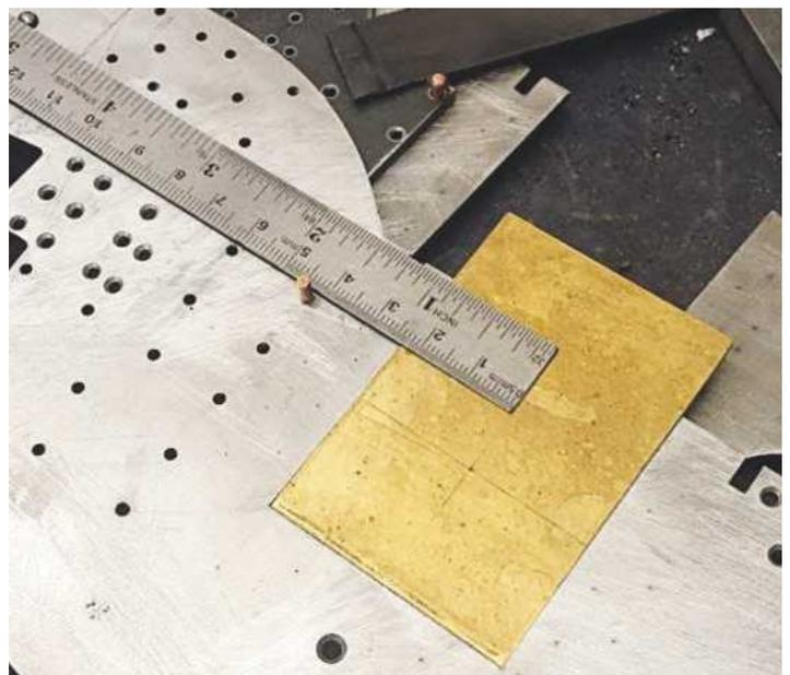
15. I now needed to plot the correct position for the bend which is 4½ inches behind the rear coupled axle centre. Here I reused the jig that I had previously made for marking out the crank axle centre, for plotting the 7° angle required for the centre cylinder incline.
