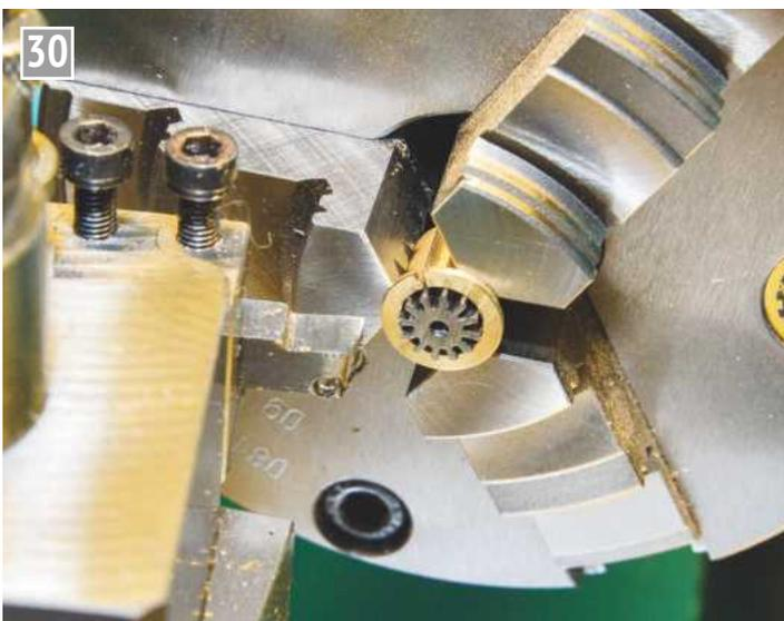
A homemade collet holds the pinion for facing off.
