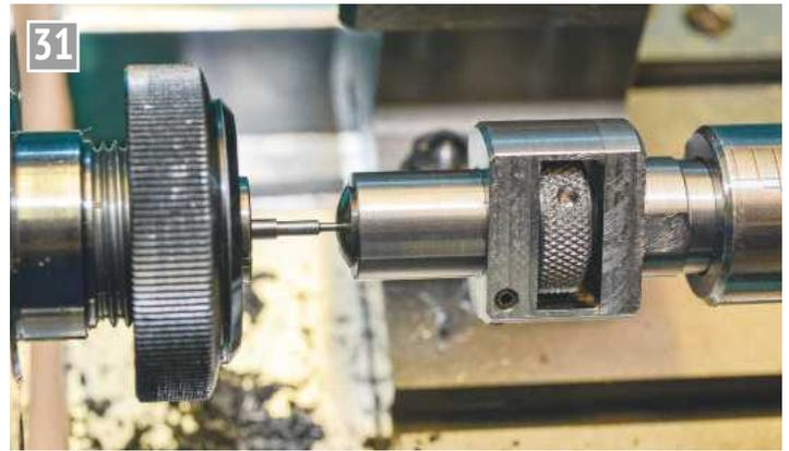
31 Holding an insert in alignment while the glue sets.
