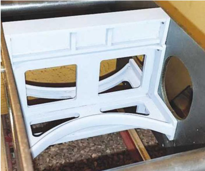
3. Another one of the stays. This shows the boiler intermediate stay fitted to the frames on top of the star stay. Now this is certainly different to 4472 today as the star stay is taller and comes up to the top of the frames and thus there is no intermediate stay as shown here. Again, this may be due to changes over the life of a Gresley Pacific or perhaps a one off on Flying Scotsman today. The works drawings of 1470 in 1922 show the arrangement as seen here.
