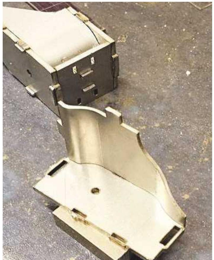
11. In this picture we have one housing with its main components assembled and the other with the bottom plate shaped and dry fitted to the front section. The curve nearest the camera follows the shape of the front buffer beam cutout and was formed by hand on the rollers.
