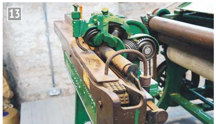
**13** Sack stitching machine, creating an overhead stitch which isn't easily unravelled. Useful for heavy duty coal sacks.
