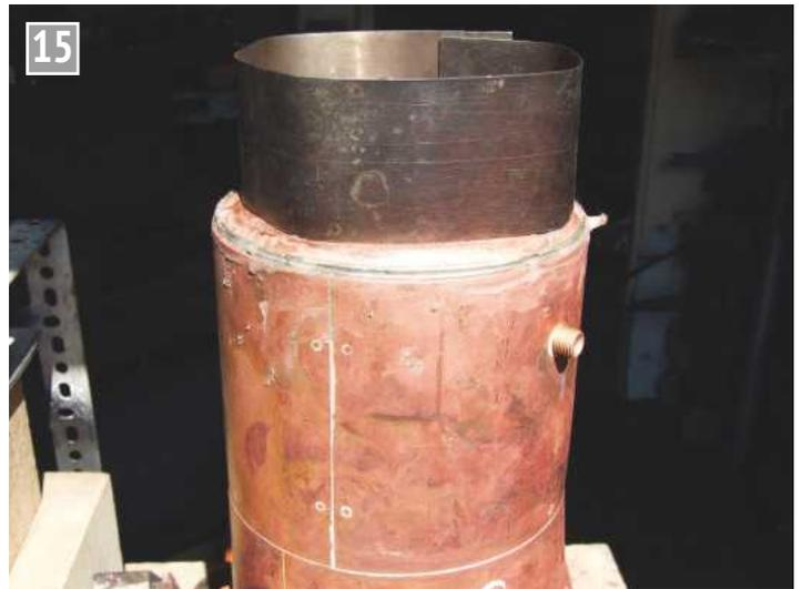
A simple heat shield protects the ends of the tubes.
