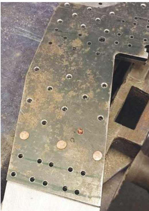
14. This picture shows the rivets completed for the rear of the doubler plate and filed down. I've left them a little proud at this point in case there was any movement during bending - as it turned out there was no perceivable movement of the plates.
