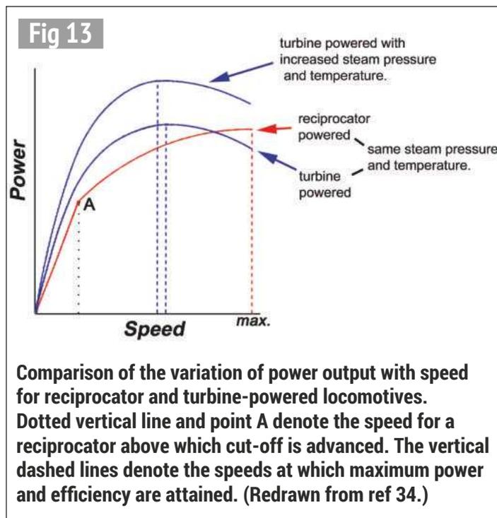
**Comparison of the variation of power output with speed for reciprocator and turbine-powered locomotives. Dotted vertical line and point A denote the speed for a reciprocator above which cut-off is advanced. The vertical dashed lines denote the speeds at which maximum power and efficiency are attained. (Redrawn from ref 34.)**
