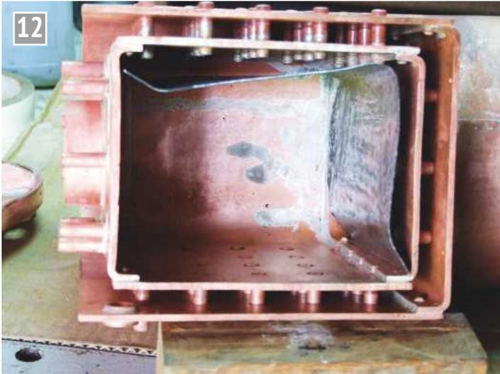
Heat shield in use while soldering inner stay ends.
