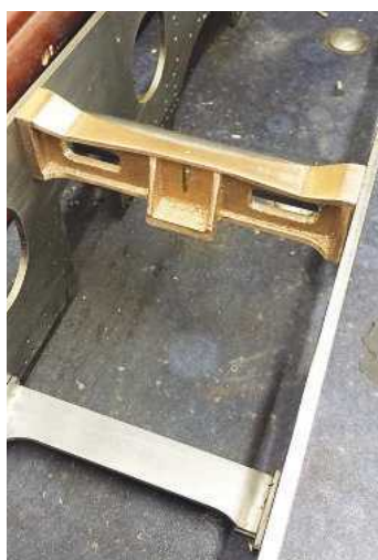
13. This is the inside motion stay and for this one a casting was supplied and used. The first job was to tidy up the stay as the casting was pretty rough. The bottom is machined flat leaving the centre angled section for later. The casting was then flipped over and machined - first the two ends close to final size, followed by machining the centre section flat. This just left the two wings which were lined up by eye, measured so both were the same and then the centre section was machined flat to join with the wings. I then machined the two end flanges to size.
