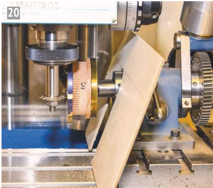
Cutting teeth on the vertical mill.
