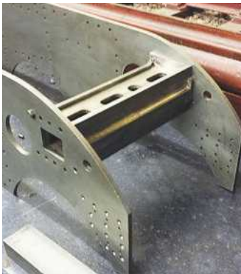
9. Following the same principle as with the frame stay I drilled one hole each side for holding the 2:1 gear stay in place. An aid in this case to ensure the stay sits where it belongs was the use of a suitably sized piece of steel that closely fitted the rectangular slot in the frames and the corresponding slots in the stay - once pushed through, trapping the stay between the frames, it wasn't going anywhere. The height was set by first scribing a line along the top edge of the stay sides to show where the bolts go through and then marking another line across it when sitting in place to give the correct position for the two holes. This tunnel is where the 2:1 arm runs through as part of the operating mechanism for the valve timing on the outside cylinders so its position is critical as Don rightly states in his words.
