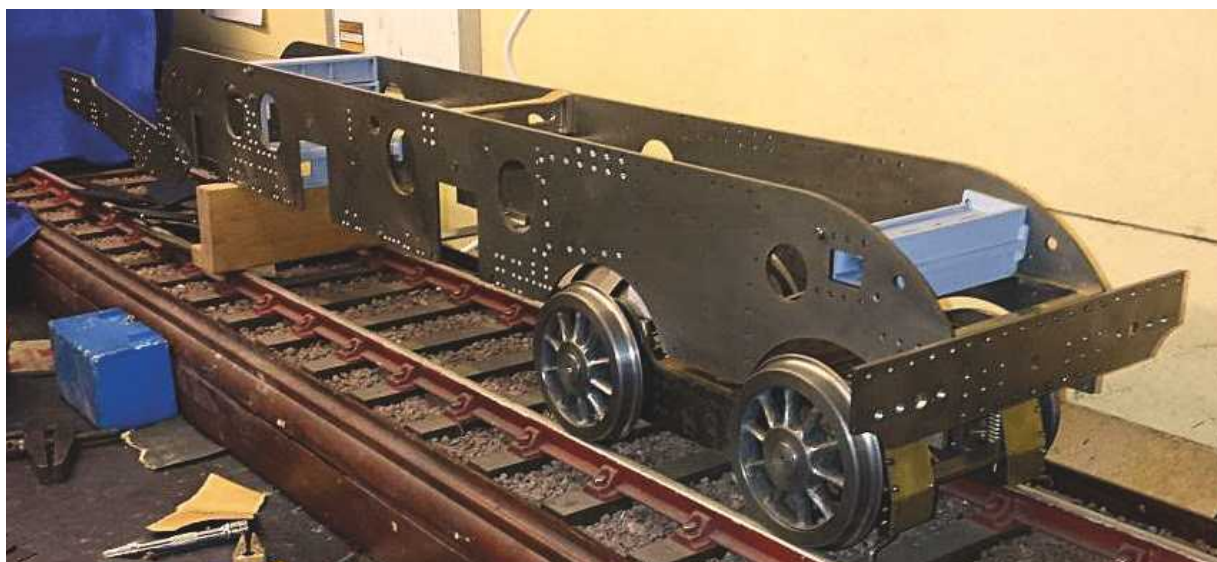
16. Here are the frames so far, posing with the front bogie.
