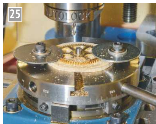
Using a rotary table to mill the inside of the outside circumference.
