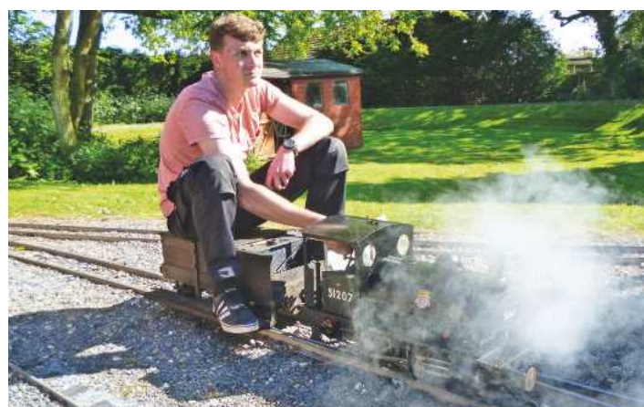
LMS Pug 51207 owned by Stuart Duncan reeled off lap after lap of our track, in sharp contrast to previous years. I understand that she is now fitted with a Rosebud grate, which has clearly made a big difference to this little engine's performance.
