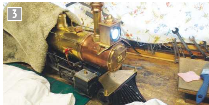
Ralph's torch-powered locomotive lantern. (Photo courtesy of Ralph Meanly.)
