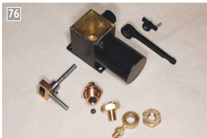
The left side lubricator; an enlarged Modelworks body with new pump mechanism according to the Ewins design.
