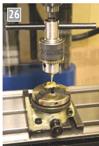
Drilling the three 10BA mounting holes.
