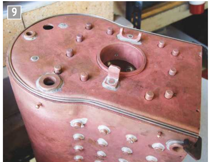
The backhead joint requires a surprisingly large amount of filler.
