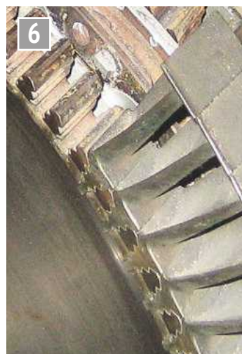
Side entry blading in a Bristol Proteus gas turbine.
