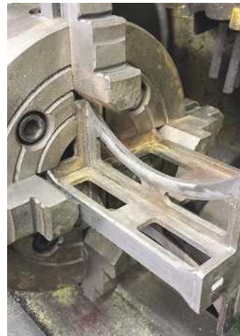
11. The picture shows how the stay was held in the chuck. I first clocked the stay to get it as true as possible, faced off and then tackled the other side. With no DRO on the lathe I took off just enough so that all of the face had been machined and then removed it from the chuck and checked the four corners and the centre for size. This showed a maximum discrepancy of 8 thou between all four corners. I noted all of the measurements, marked the stay accordingly, placed it back in the chuck, clocked it so that I had the corners sticking out by the amount they were over size to each other, held my breath and machined to size - and it worked.
