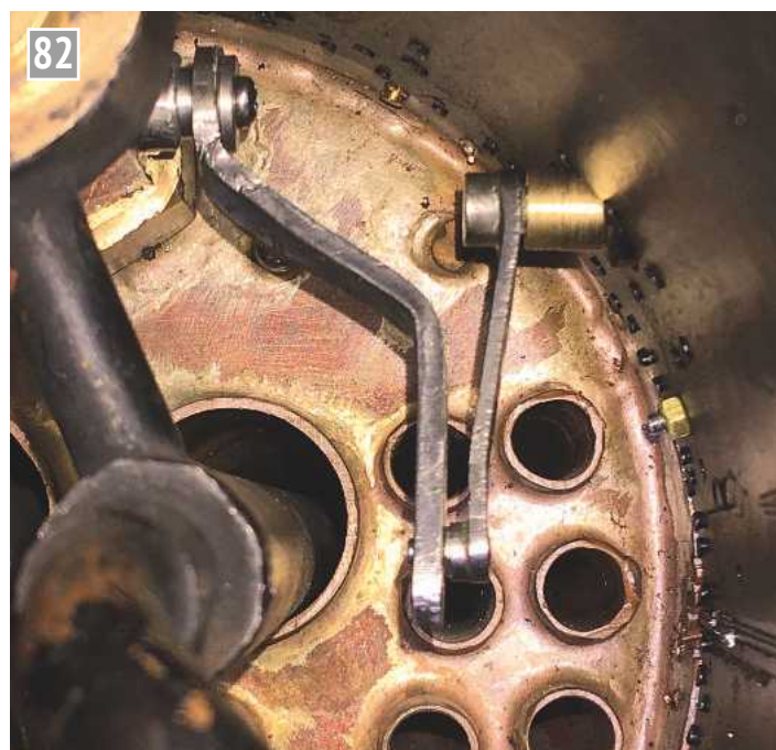
Regulator levers on the inside of the smokebox, with a pin locating in a slot to drive the crank affixed to the ball valve. All parts made from silver soldered stainless steel.
