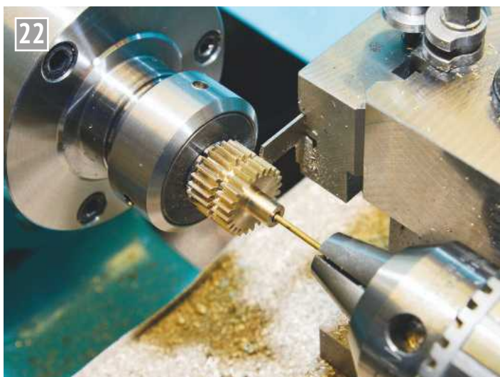
Parting off a pair of wheels.
