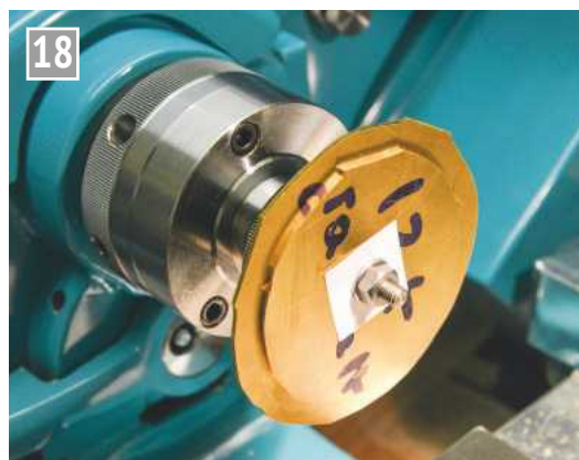
Wheel blank mounted on a true running mandrel.
