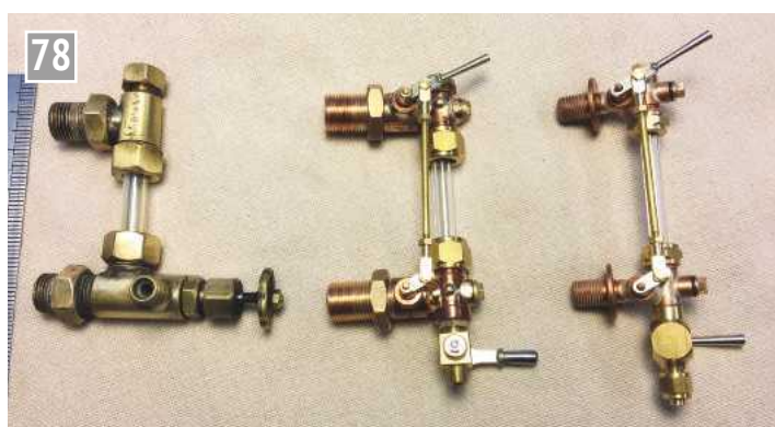
Three alternative water gauge styles: left to right - Modelworks 6mm glass; my design 5mm glass; Dave Noble production 4mm glass.
