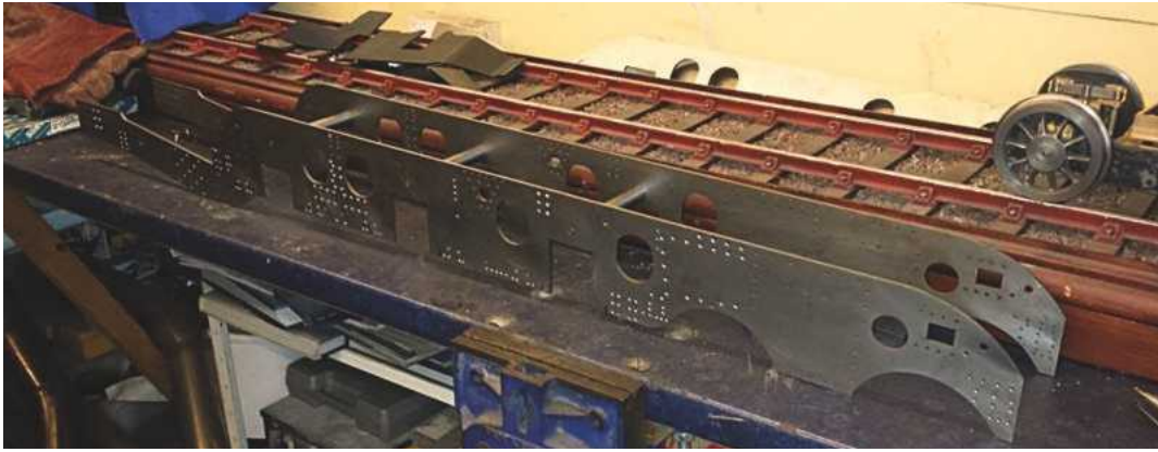
7. Here are the frames with the three spacers holding them apart at the correct separation.
