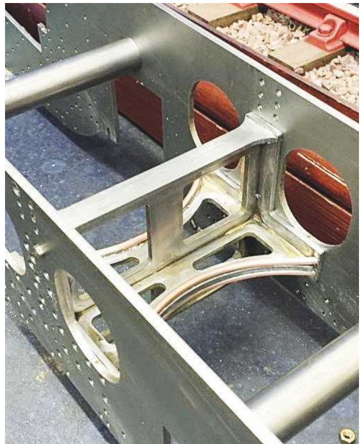
12. The last job was to solder on the beading. The stay as seen here still needed a little filing and a good clean to finish. Fitting the stay to the frames followed the same procedure as with the others.
