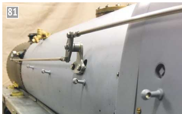
Alignment of the regulator rods down the boiler. The bracket height and stand-off were adjusted to get this right.
