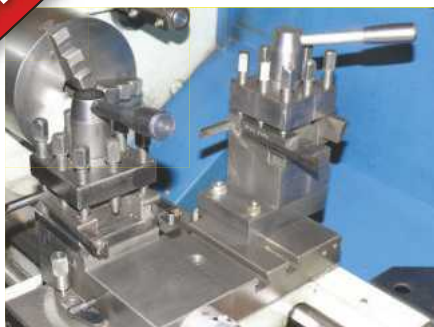
Howard Lewis explains how to make a heavy duty rear toolpost.
