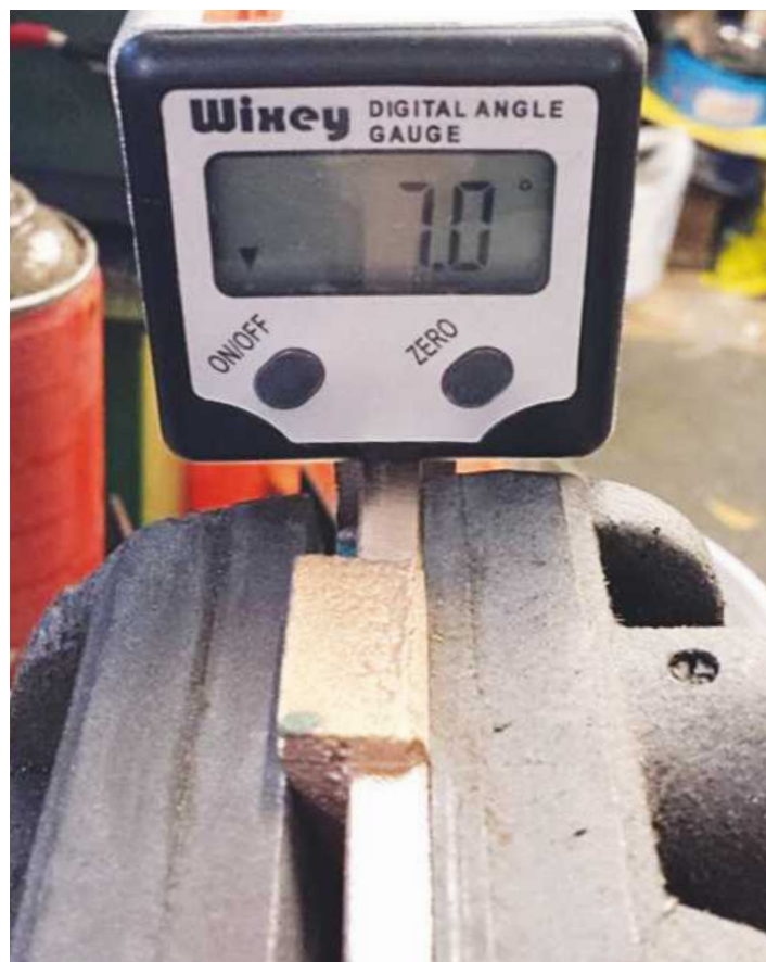
14. Here we see the casting held in the tilting vice to have the centre cylinder slide-bar support machined at its correct angle of 7 degrees. My new digital angle finder came in handy for doing this. I also used the gauge to check the other axis to ensure all was square before machining as even though the casting was chocked up with a piece of steel to keep it square I wanted to be extra careful here as this part is very important.
