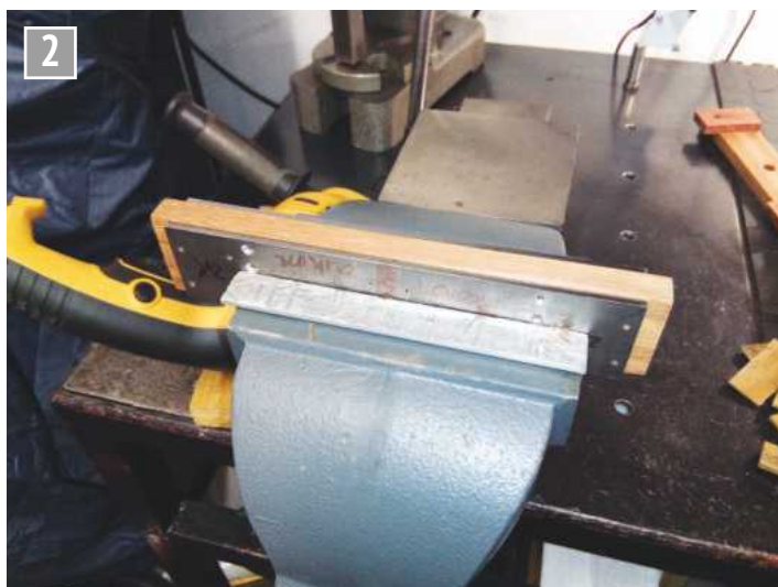
Drilling the wooden buffers.
