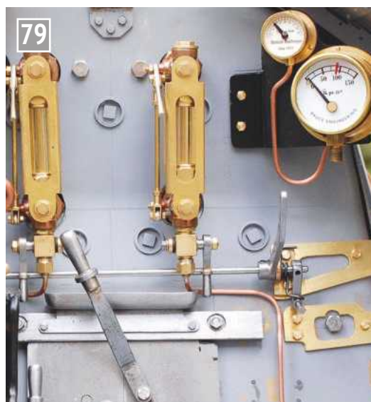
Water gauge glasses mounted on the backhead. The glasses are twice the height of true scale from the prototype which makes the bottoms much lower and closer to the fire door top.
