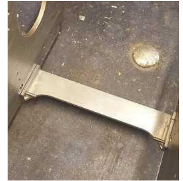
8. The first stretcher made and part fitted in its correct position with just temporary bolts.
