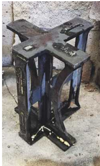
10. The STAR stay - this is a monster and a very prominent fixture on a number of Gresley's locomotive designs. Here is the star after soldering up. I had noted that the width was just under the required size, only by a few thou but that's enough to cause problems later on, so I packed out the two end pieces with some brass shim equally either side. I'd rather do it this way to create a small fillet in the gap created than use shims later to space the frames correctly. This gave me a fixture slightly oversize as required to be able to later machine the two side faces square.
