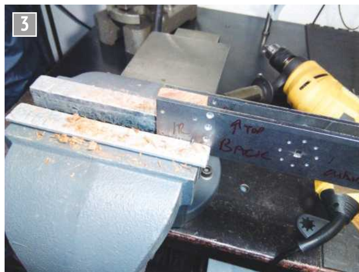
Drilling the wooden buffers extensions.
