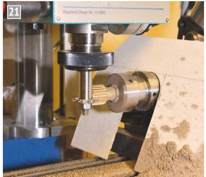
Cutting the 24 tooth wheel.
