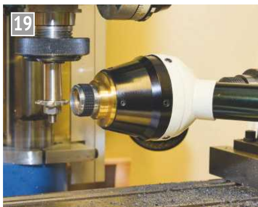
Using a microscope to set the cutter centre height.
