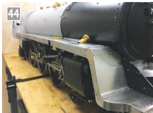
Locomotive side platforms (running plates) fitted close to the boiler cleading.
