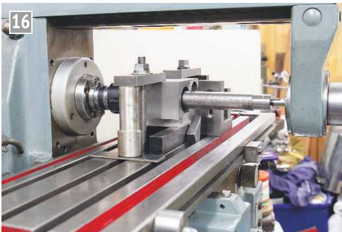
16 Boring through one of the outside cylinder blocks, this time viewed from the opposite side of the milling machine.
