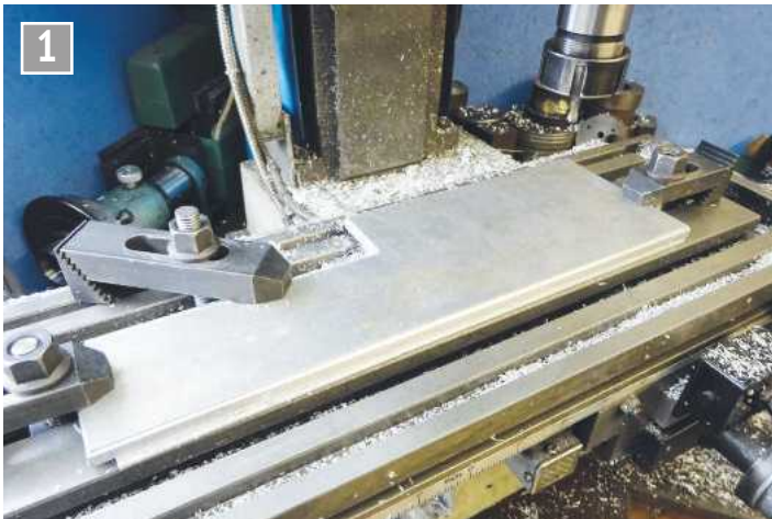
Machining the quarter round decorative moulding around the base.
