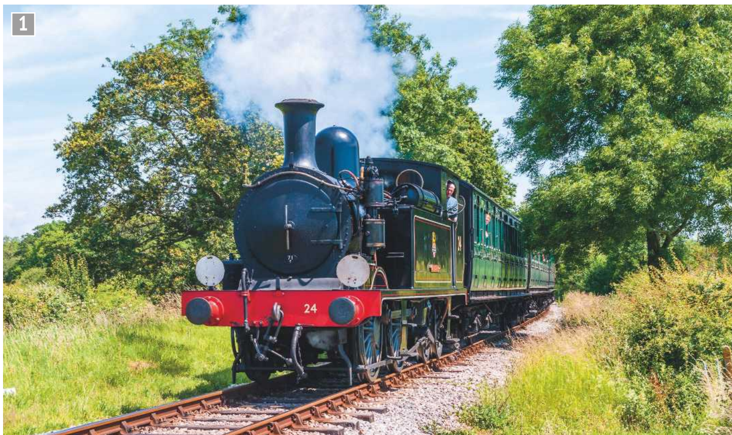
Edwardian elegance on the Isle of Wight Steam Railway; Calbourne with vintage carriages. Note the Westinghouse brake pump.
