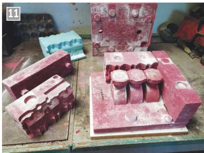
Crankcase sand moulds.
