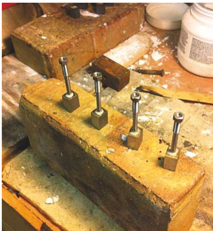
2. With the parts fitted together they were then silver soldered and so two parts became one, ensuring a good fillet was achieved around the collar.
