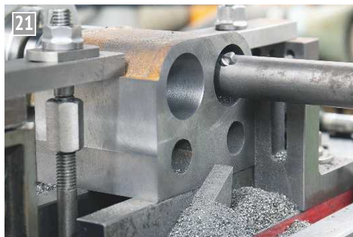
Work on one of the castings, showing slightly different clamping arrangements.
