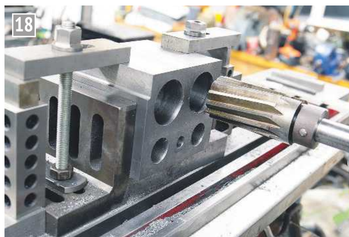
18 Shell reamer used for the main bores, viewed from spindle side of machine.
