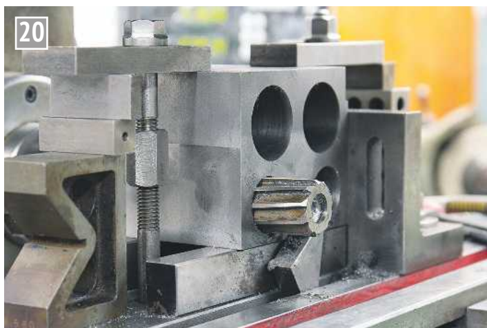
Smaller shell reamer emerging from one of piston valve bores.
