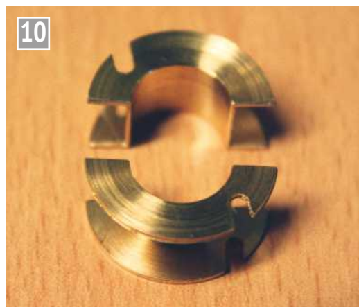
Finally, the big end bearing shells are split.
