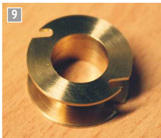
Big end bearing shells with slots.
