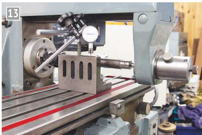
Setting the angle plate true to the Y-axis on the milling machine.
