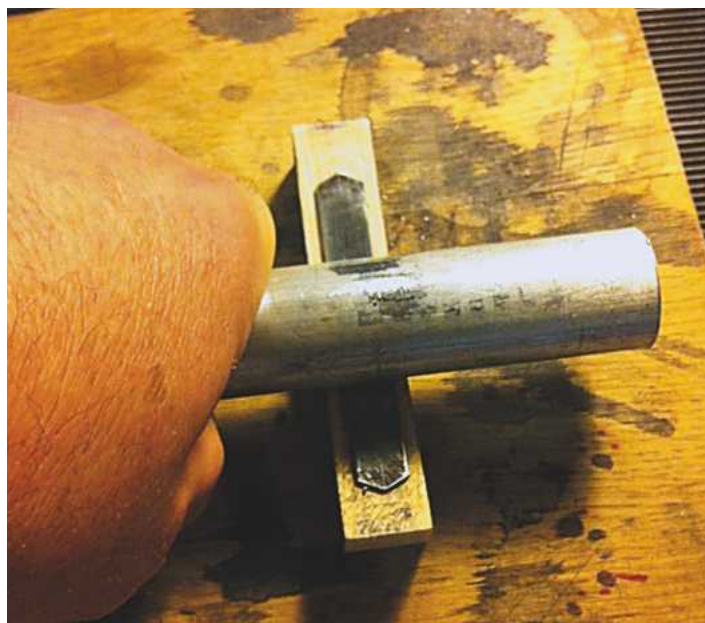
6. This picture shows me using the bottom profile piece, and rubbing a suitable piece of alloy bar across each leaf to form its shape. For the large leaves I used this method (using both hands of course) but for the small ones I used a small hammer to rapidly tap the alloy while moving it along the length of steel.
