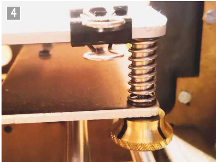
Heated bed adjustment screw.
