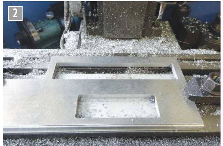
Forming cut-outs for flywheel and crank disc clearance.
