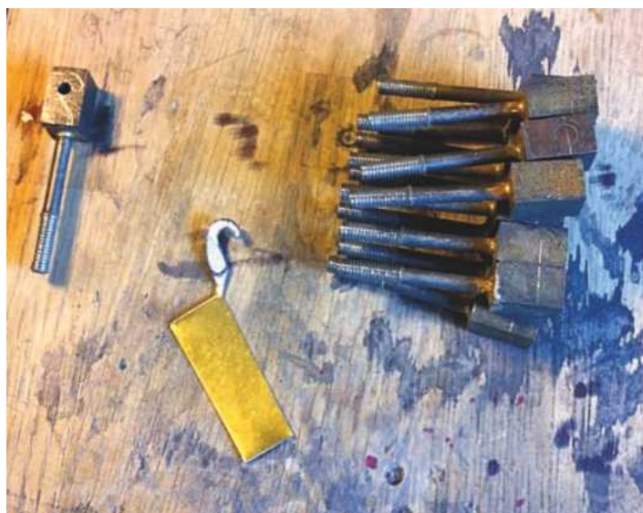
3. After retrieving the parts from the acid dip (note to self, don't leave things with fine threads in acid for too long as they get eaten away - although the threads are slightly damaged, on doing a small stress test the threads are still capable of doing their job - live and learn) I cut a small template for the gripper and scribed around it for each hanger. I used the small casting of a grip for reference but I just can't recall where it came from after 10 years.
