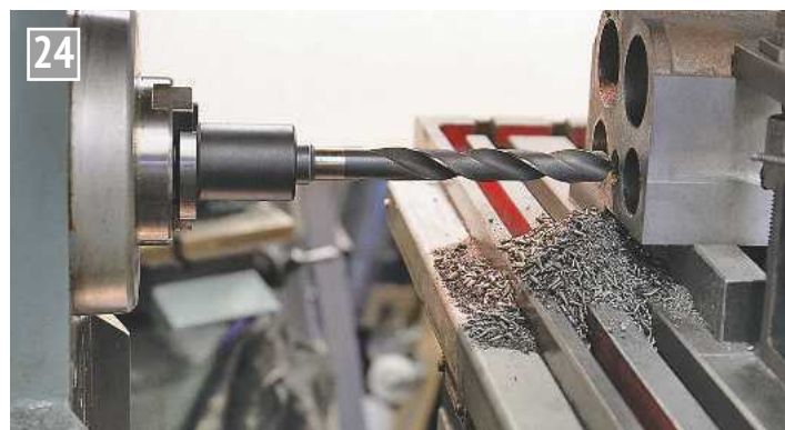
Drilling \frac{1}{16} inch for the exhaust steam passage through the block.
