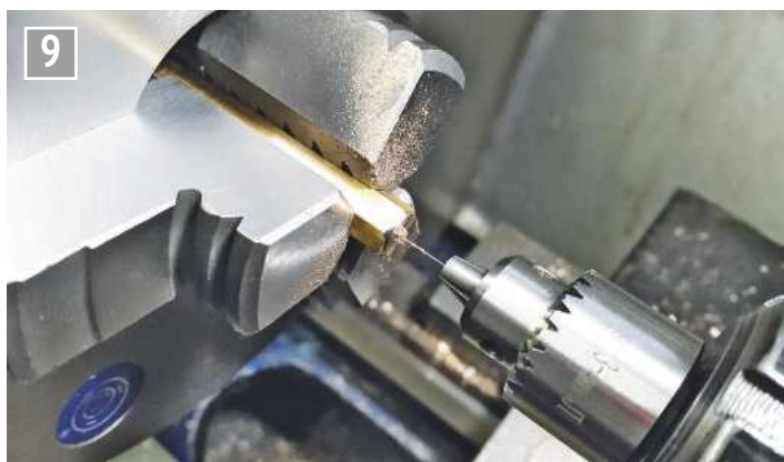
Drilling the 0.3mm nozzle hole.
