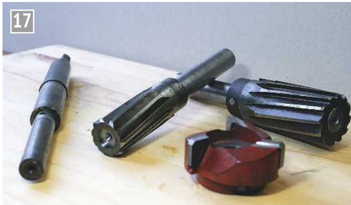
17 Shell end mills mounted on home-made shanks, the original MT3 shank being on the left. Also shown is the face mill used for much of the early machining to square up blocks and bring them to size.
