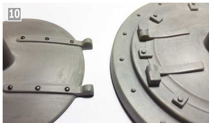
Detail added to the pattern after printing and as printed.
