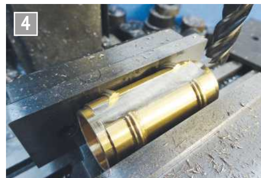
Milling a 10mm wide flat for the valve chest.
