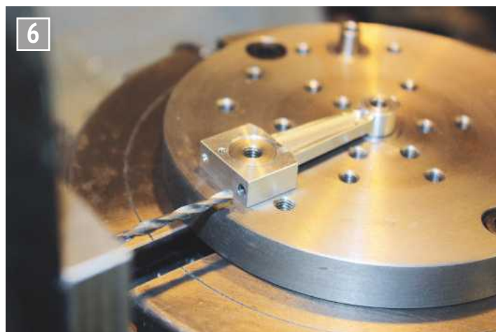
Drilling for the bearing cap screws.
