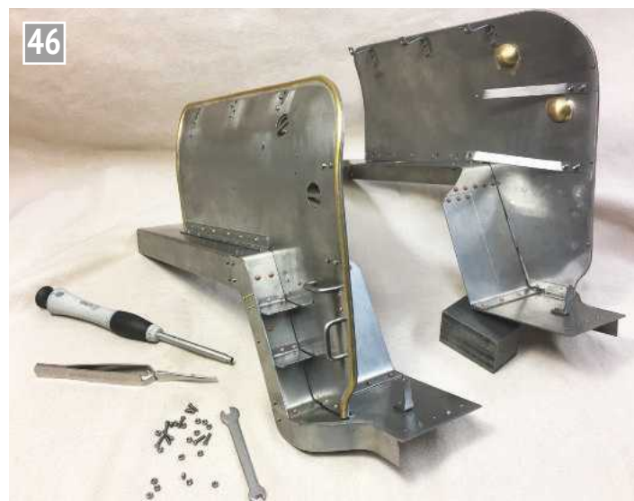
Smoke deflectors fixed to front platforms.
