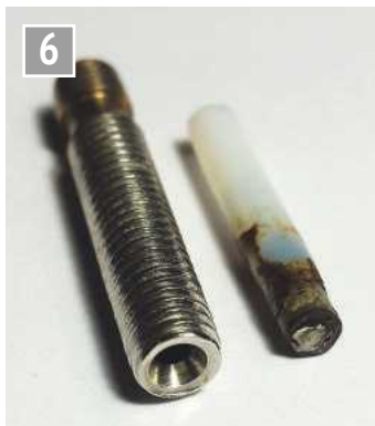
Failed PET tube and new stainless feeding tube.
