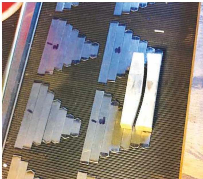
5. Seen in the picture are the various steel components cut to size ready for bending to shape. They are, of course, in the annealed state. The piece of wood seen is a piece of 2 x 1 that I have cut to the profile needed for the 1/4 inch camber as drawn - this will be used to shape the steel so that all leaves are correct.
