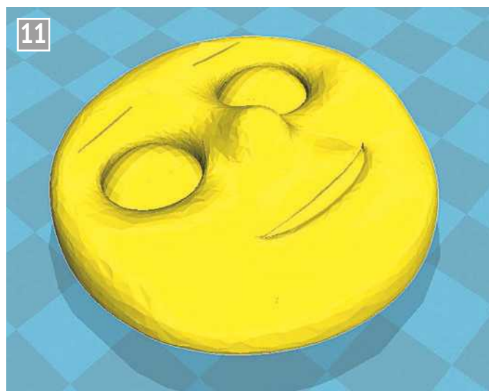
A faceted geometry - STL tolerance set too high.
