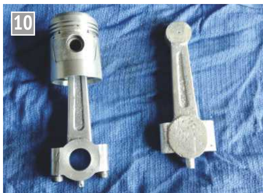
One of the pistons and a connecting rod casting.
