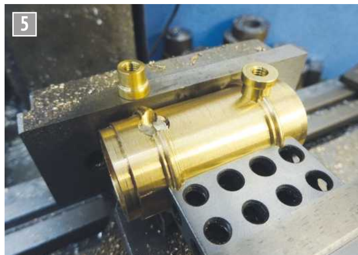
Plunge cutting pockets for feet.
