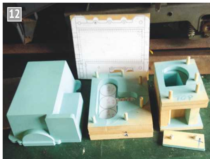
Pattern and core box for the sump.
