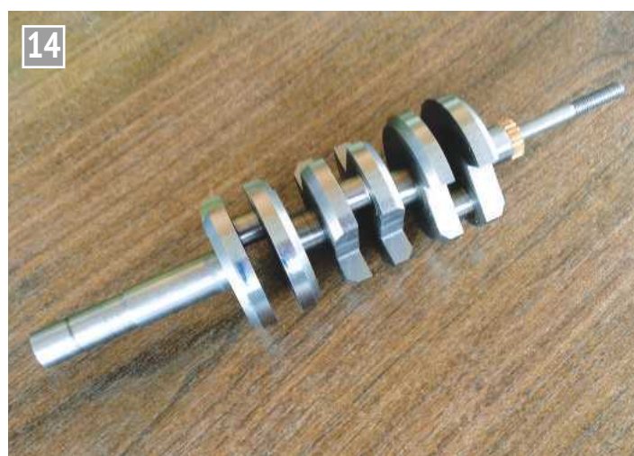
The crankshaft is machined from the solid.
