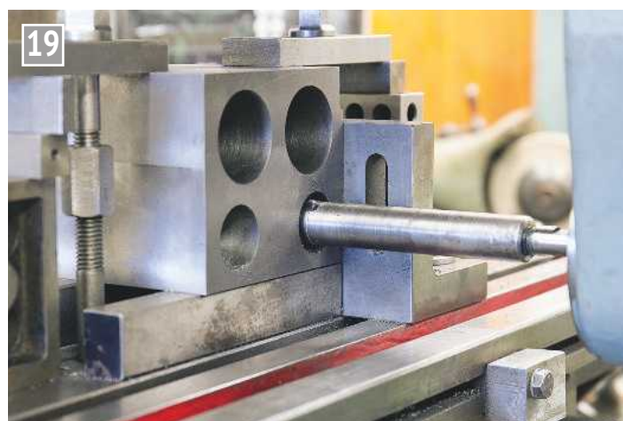
19 DRO used to reposition block and small boring bar in use machining the smaller piston valve bores.
