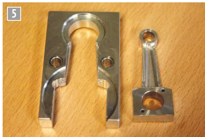
Conrod separated from the parent stock.
