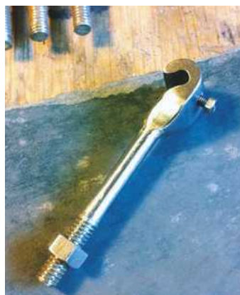
3. After retrieving the parts from the acid dip (note to self, don't leave things with fine threads in acid for too long as they get eaten away - although the threads are slightly damaged, on doing a small stress test the threads are still capable of doing their job - live and learn) I cut a small template for the gripper and scribed around it for each hanger. I used the small casting of a grip for reference but I just can't recall where it came from after 10 years.
