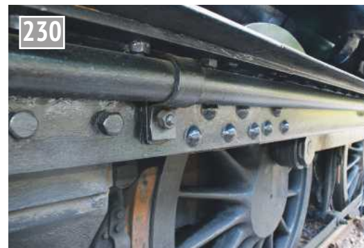
Vacuum pipe neatly tucked away under the platform.
