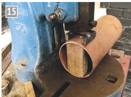
Curving the steam dome flange to fit.
