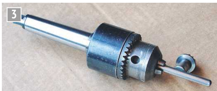
Ideally a smooth bodied chuck should be used.
