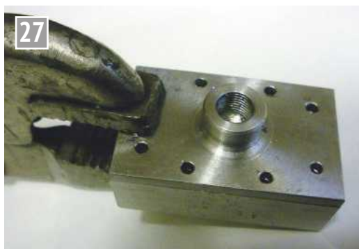
Spotting the fixing holes through the steam chest.
