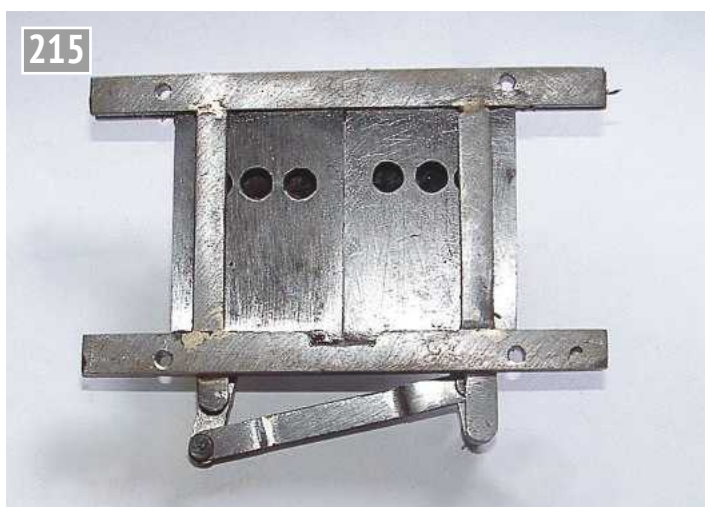
Y4 fire hole doors (cack-handed!).
