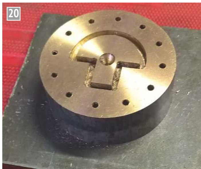
Forming the base of the steam dome.
