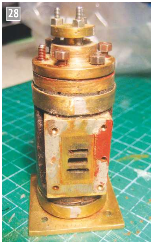
The cylinder, showing the port face.
