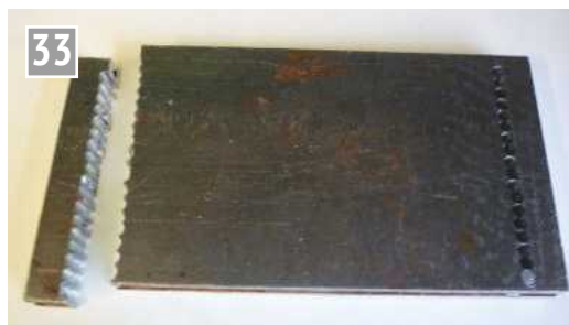
Cutting strips for the steam chest outriggers.
