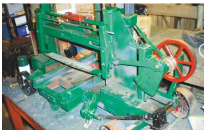
Crank driving the saw blade.
