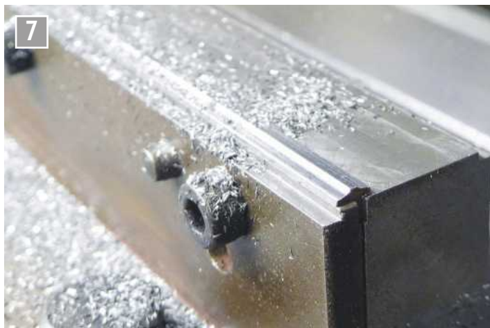
Part-way through generating the profile – still 11 more passes to do!
