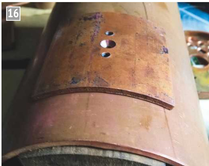
16 Steam dome flange nicely fitted.
