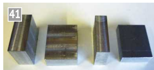
Blanks for the rocker shaft bearings.
