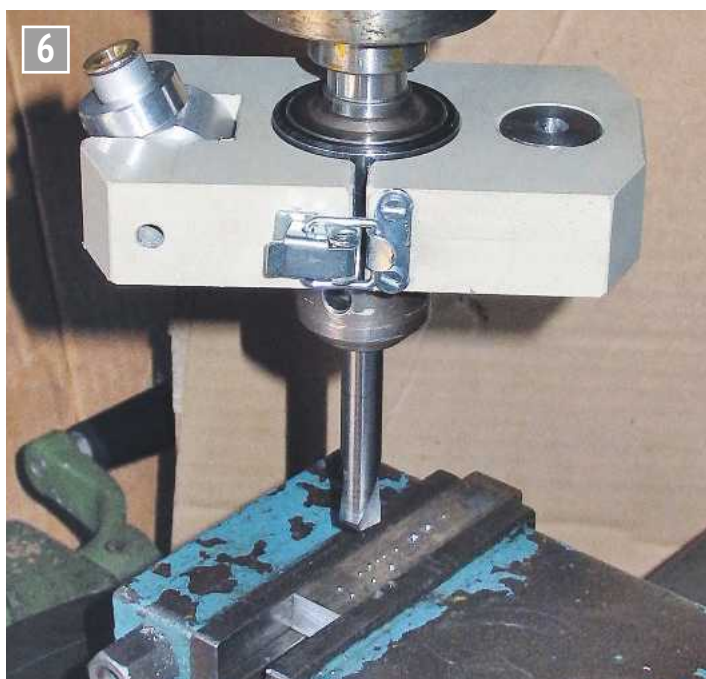
The centre finder mounted ready to centre a drill.
