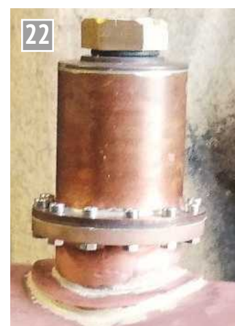
The completed steam dome.
