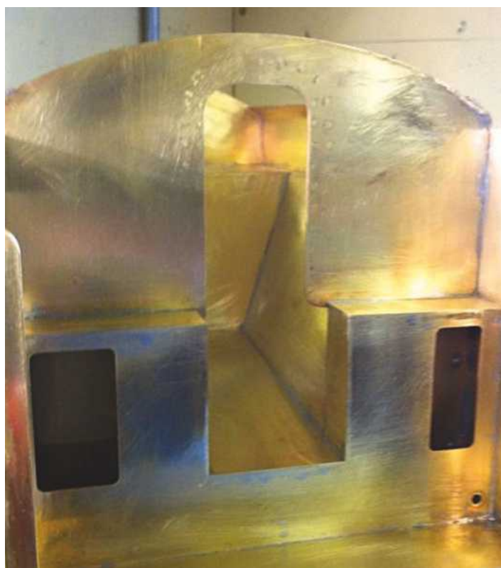
And now we have the locker panel and its shelf soldered in place. The hole, bottom right, is where the water gauge fits.
