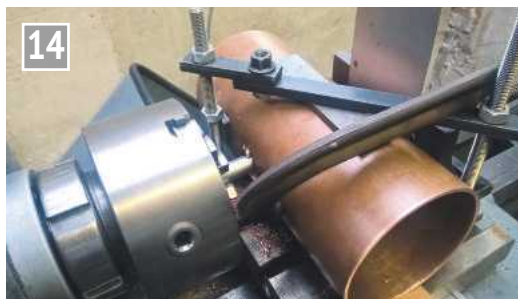
Boring the steam dome hole.
