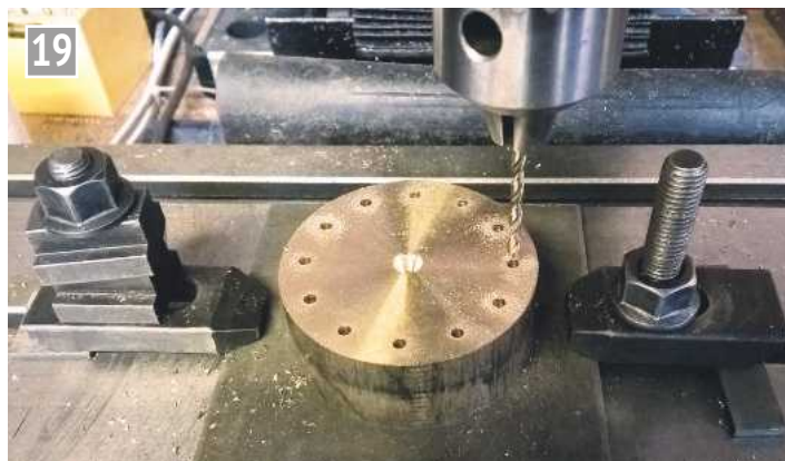
19 Drilling the dome fixing holes.
