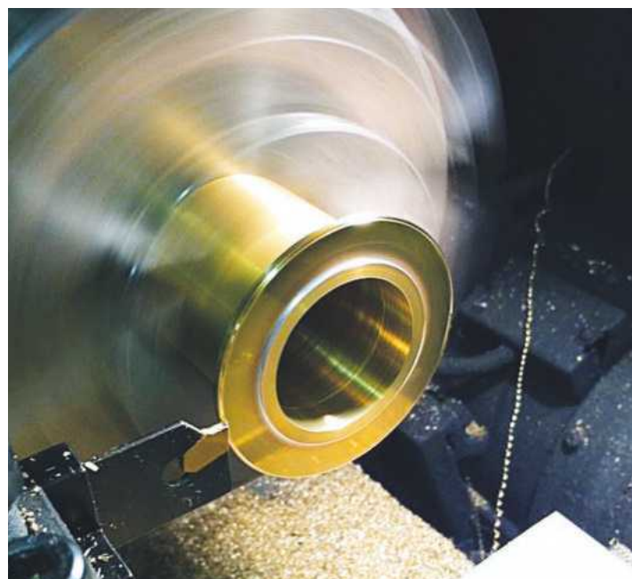
With the ring securely fitted to the tube it was mounted in the three jaw chuck and the outside radius was machined to size.
