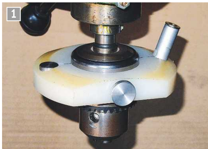
The centre finder attached to a Jacobs chuck.
