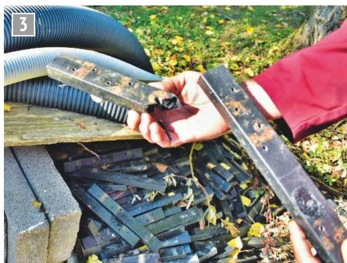
One of the replaced plastic sleepers showing the brittle cracking and the burn damage.
