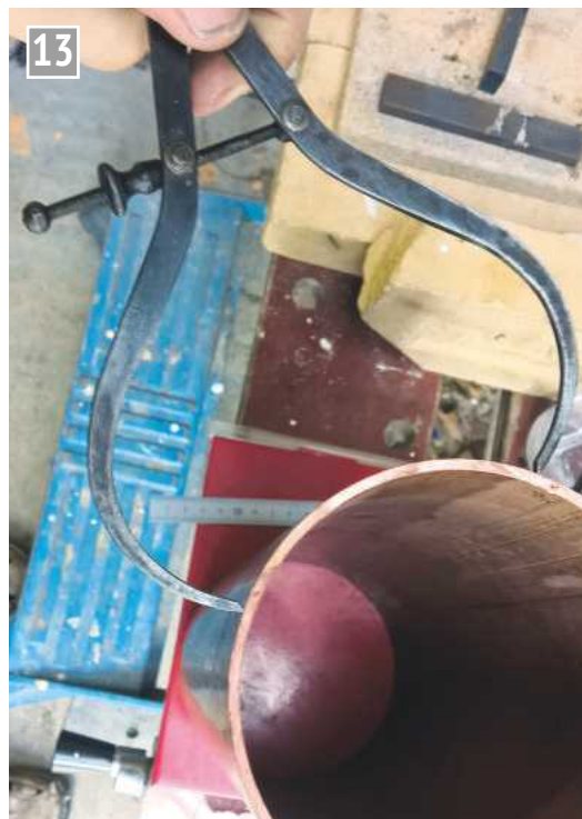
Marking off quarters around the boiler barrel.
