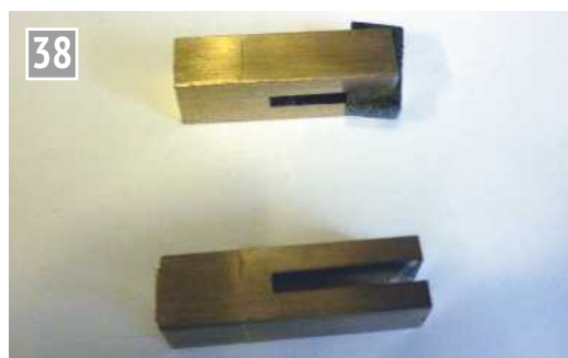
Slots formed in valve rod ends.
