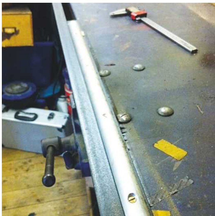
The picture shows the former/jig that I used. I might add that this length of alloy was first cut down the middle using my small band saw. It's a good job I had a very good blade made for it some time ago.
