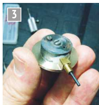
3 Backing plate drilled and ready for soldering.
