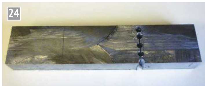
Preparing the blank for the steam chest.
