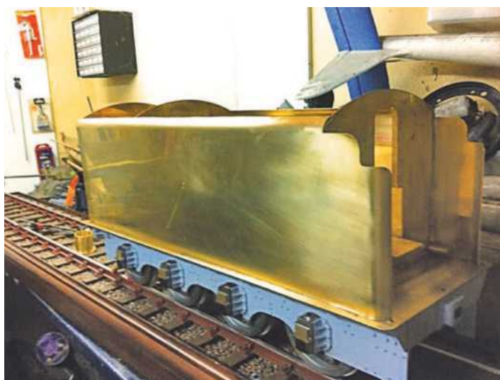
With the sides rolled I could now make a start on assembling the panels. The rear was done first, followed by the front after I had first turned up a short length of brass which was drilled, tapped, stepped and brazed into a matching hole for the step in the front panel. This can just be seen bottom right. This is for the working water gauge once it's fabricated; the drawings weren't very clear here as they only show the hole for the gauge on the locker panel, which, yes, has to be done too (I did both at the same time while clamped together) but since it's a locker and not part of the water tank I can only assume that there is some sort of connection pipe running through the locker from the tank to the gauge. Anyway, I've tackled it with my brass tube which the gauge will screw into later. Finally the side panels were soldered on and I finally had something that looked like a streamlined non corridor tender.
