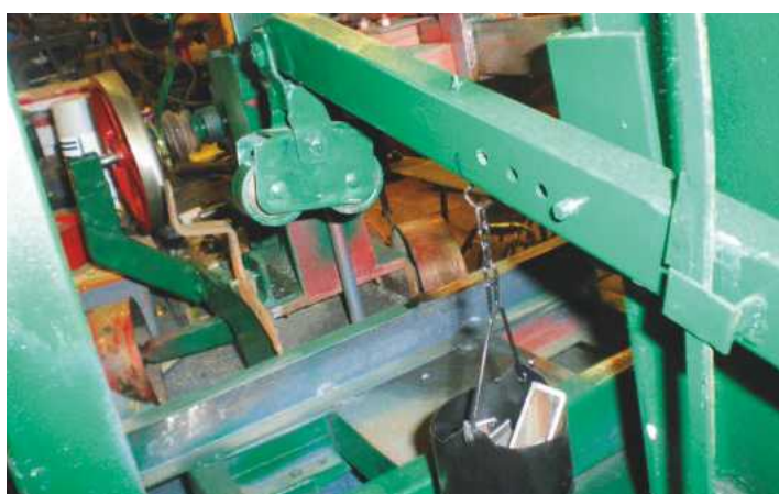
Weighted rollers keep the wood on the carriage.
