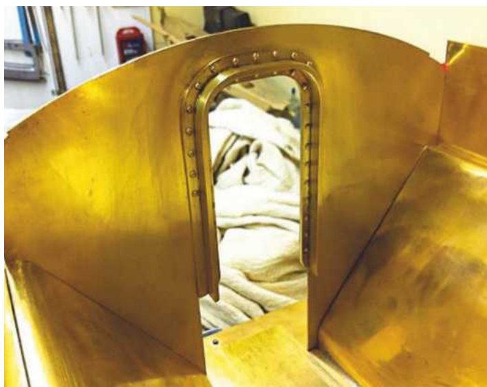
Here the door frame has been fixed in place.
