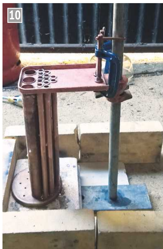
Silver soldering the tubes into the firebox tubeplate.
