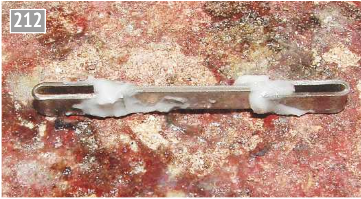
Preparing to silver solder the connecting link.
