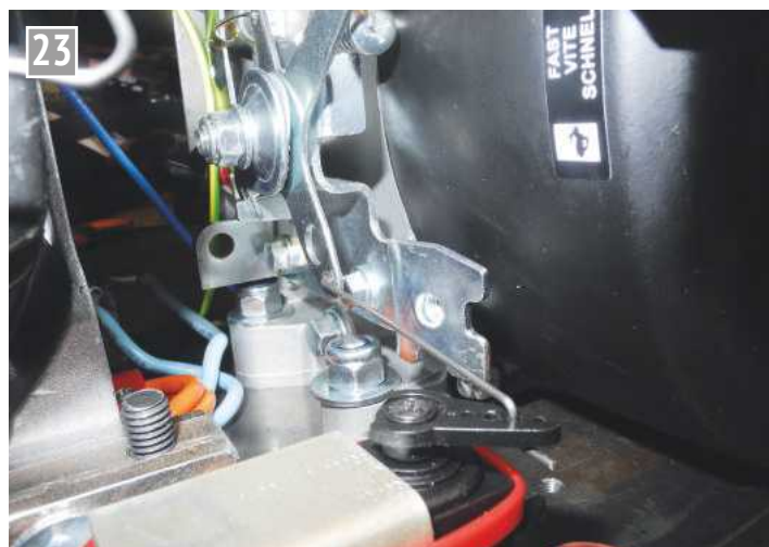
Engine control servo and linkage.
