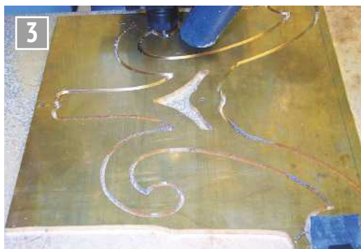
Cutting the second half with CNC after flipping the material over.
