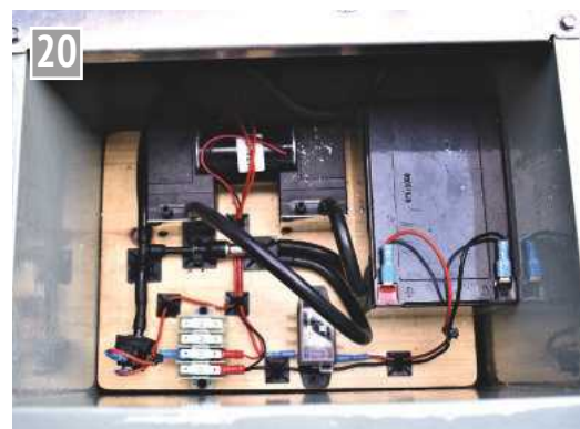
The auxiliary vacuum assembly fitted to the new baggage carriages.
