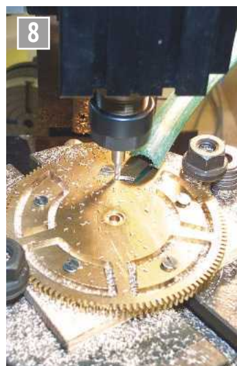
Cutting the crossings (windows).
