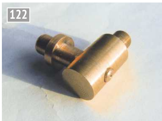
The ends of the holes through the body have been chamfered and the two parts assembled ready for silver soldering.
