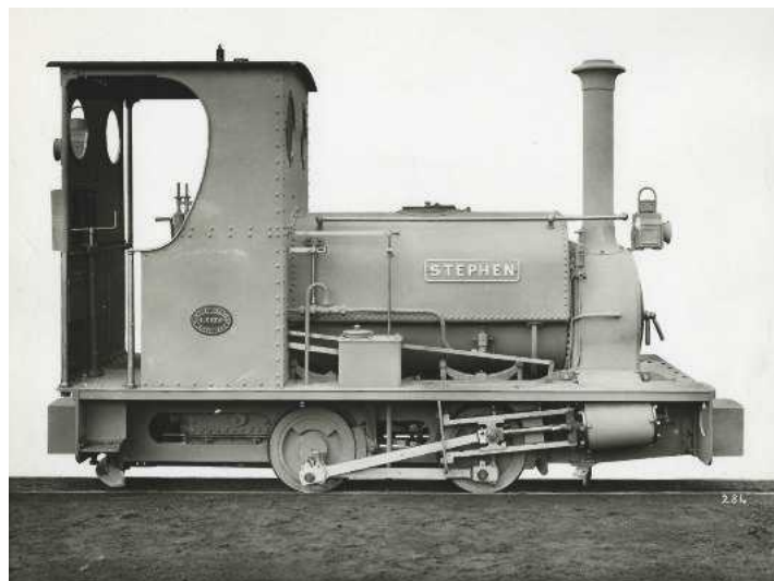
Perhaps the best-known wider gauge relatives were the four 3ft gauge locomotives built for Penmaenmawr Granite Quarries. This maker's photograph shows Stephen (W/N 771 of 1902). Unfortunately, all four locomotives were scrapped by 1951, being outlasted in their workplace by De Wintons. As with Velinheli the feed pump was on the left-hand side.
