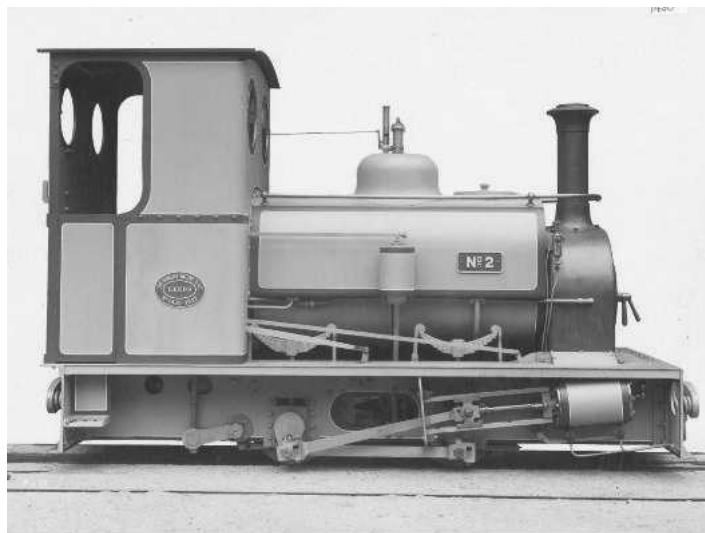
This maker's view is of the Dinorwic system's second 'Port' class (W/N 1430 of 1922, originally No.2 later Dolbadarn). This design was built to basic Alice class proportions but the illustration clearly shows the higher pitched boiler (updated from Peep-o'-Day); cab derived from Dorothea short chimney; kidney buffers; plain rectangular mainframes with no lower extensions, and rectangular buffer beams with cylinder access holes.
