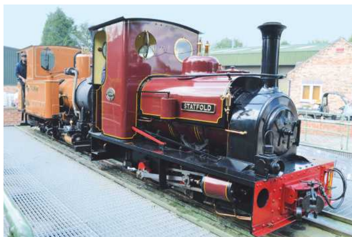
Michael's design, sans buffers and with revised drawgear, was repeated in 2005 for a new locomotive, Statfold, constructed in Statfold Barn's workshops as Hunslet W/N 3903. The locomotive is seen here on Statfold Barn's turntable on August 8th 2020.
