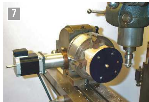
Cutting the great wheel teeth with the dividing head on the big miller.
