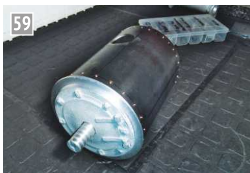
Trial assembly of machined smokebox door.
