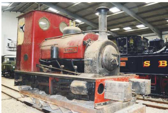
The final member of the Dinorwic second 'Port Class', Michael, was built in 1932 for quarry work, with appropriate buffers and drawgear. It subsequently lost its cab but this was restored prior to shipment to Canada. It is seen here at Statfold Barn on April 9th 2016 and, as with King of the Scarlets, no restoration work has taken place since repatriation. The original pattern sandboxes are still in place.
