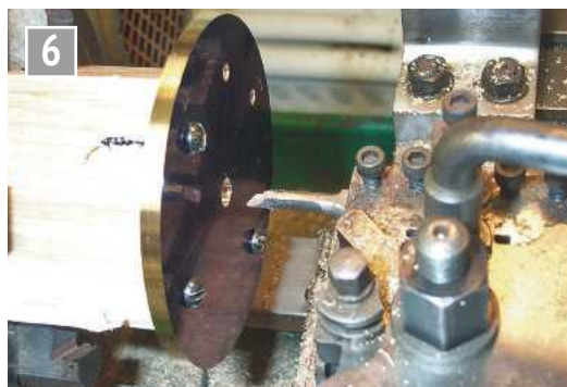
Turning and boring the great wheel.
