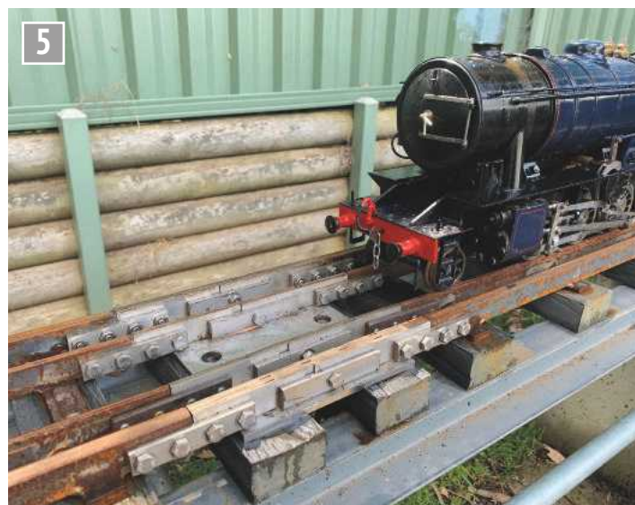
Warwick Allison's rail expansion joint (photo courtesy of Andrew Allison).
