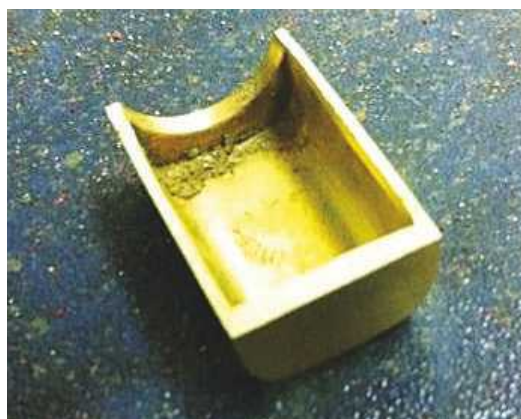
First tray brazed together with the rear panel shaped to clear the axle.
