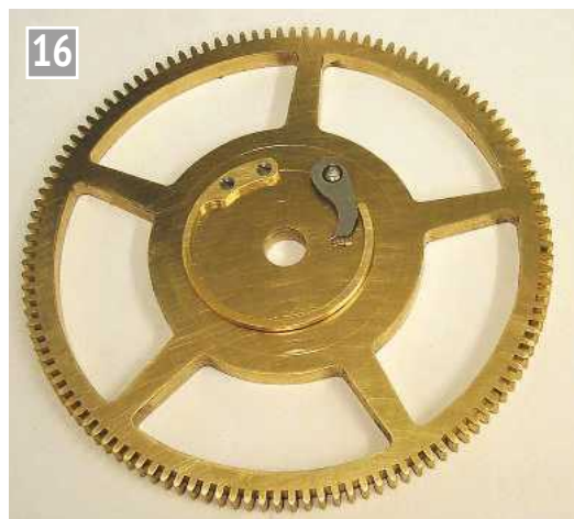
The winding click and click spring fitted.
