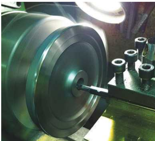
The first tender wheel having the back machined and then bored out.
