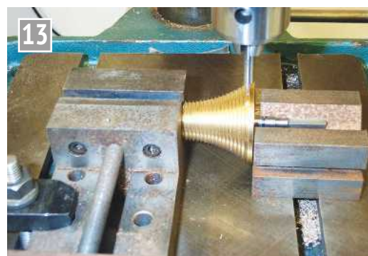
Drilling for the fusée wire.
