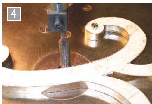
Using a file in the fret saw to clean up the frames.
