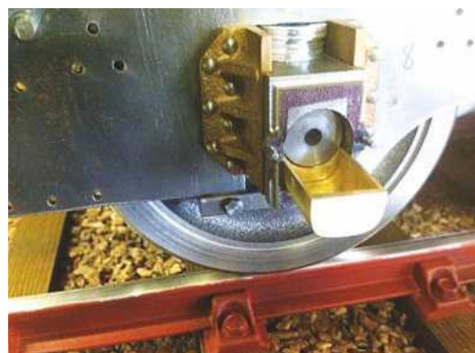
Test fit of a tray to an axle box making sure it's a good fit for the axle. I still need to make the oilway blocks which will then fit through slots in the covers when machined later.
