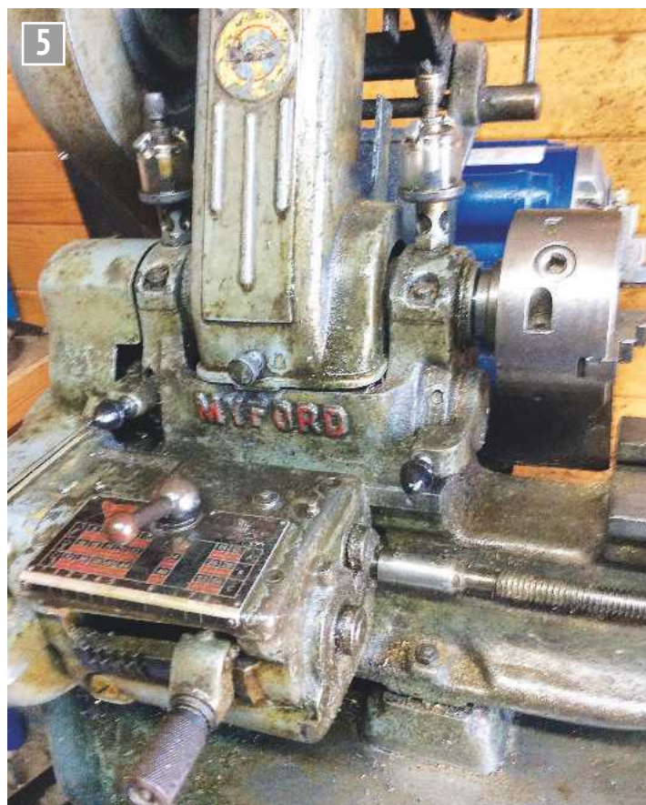
The old Myford gearbox and new motor.
