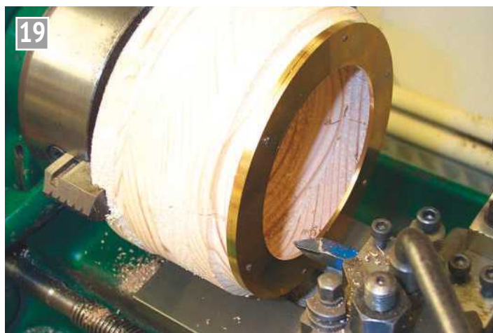
The annulus blank mounted ready for tooth cutting.
