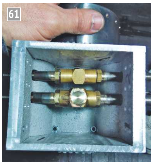
Plumbing fitted to the smokebox cradle.
