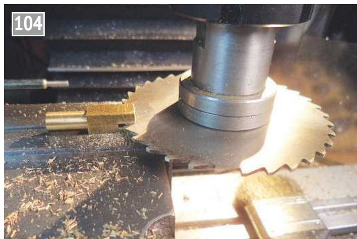
Cutting a slot for the whistle valve lever.
