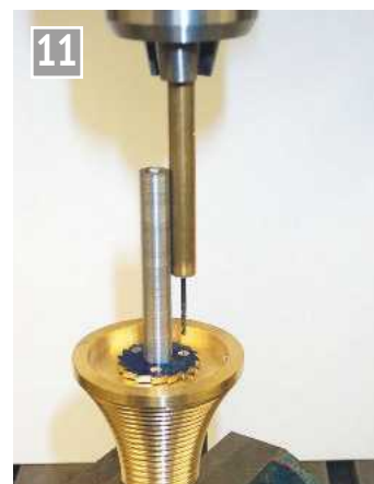
Tooling in use to drill and tap for the winding ratchet fixing screws.
