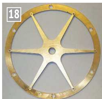
The six-legged spider attached to the blank prepared to become the annulus gear.
