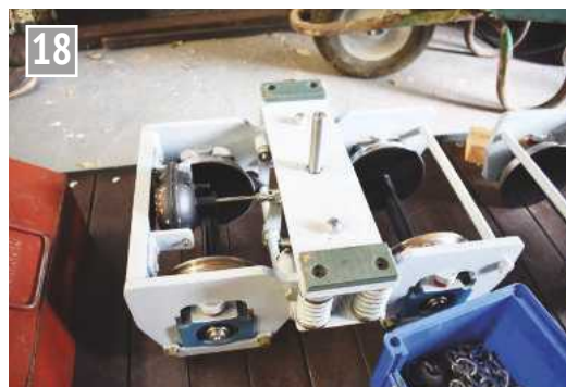
One of the new passenger carriage bogies built on site by members.
