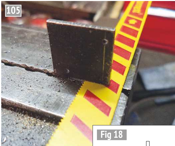
105 A crafty hack using two blades to cut a slot.
