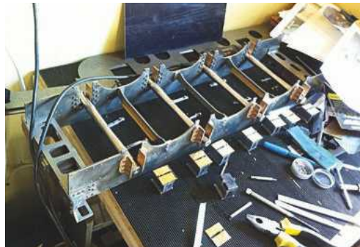
Tender frames erected, axles turned, horns fitted, axle boxes being constructed.
