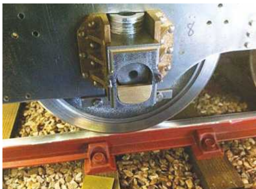
Tray in place. The washers above the box are just there temporarily holding the chassis at the correct height.
