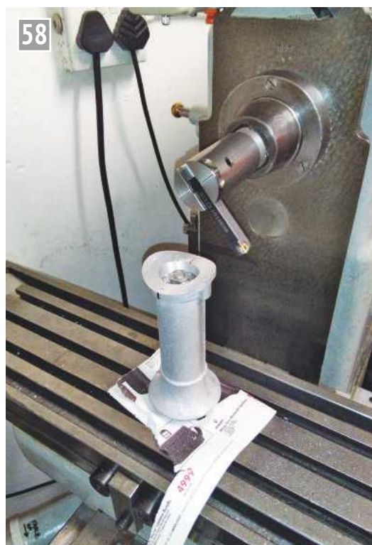
Machining the chimney base using a fly cutter.
