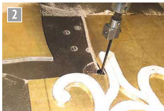
Sawing out the frames.
