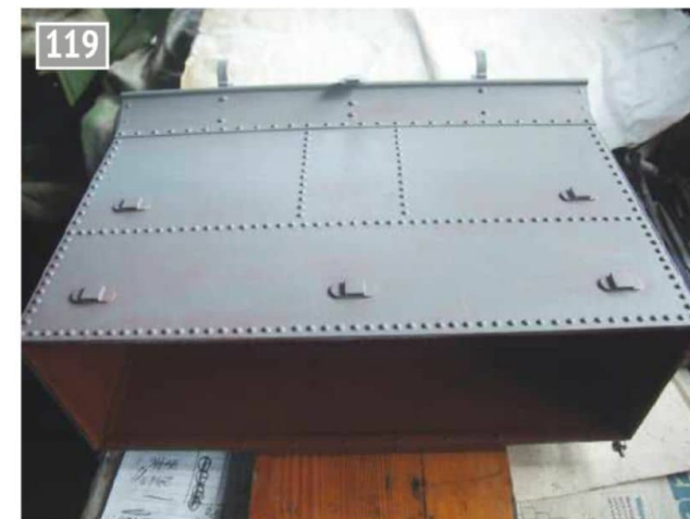
119 The outside of the rear bunker primed and undercoated with all the early design of lamp brackets fitted.
