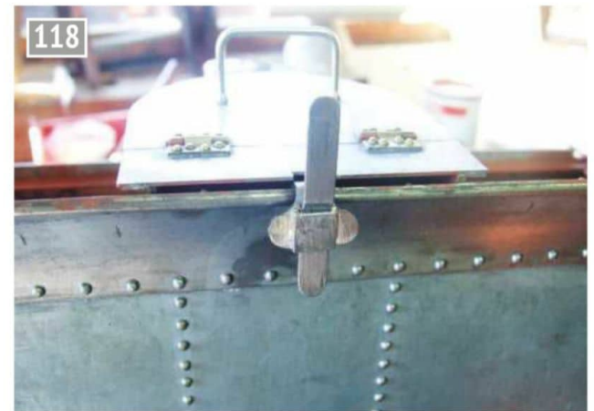
118 The top bracket in position but only one bolt added.
