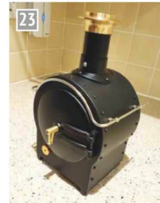
Completed smokebox assembly.
