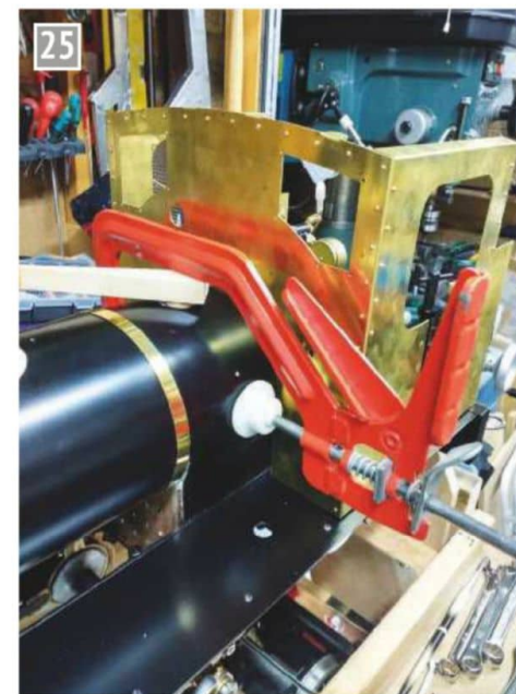
Squeezing the cleading to fit the boiler into the frames.
