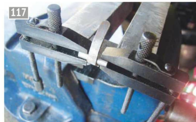
117 Now the steel forming plate is held horizontally and the tail of the bracket formed with small plain nosed pliers.
