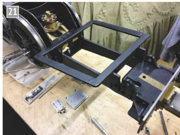
Square frame for ashpan and firebox support. After this picture was taken the support was lowered by \frac{3}{8} inch to position better the boiler.
