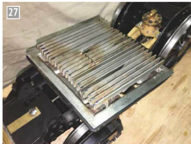
Three grate sections mounted on the ashpan cross bars.
