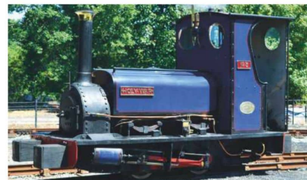
Classic second generation Alice class locomotive, Holy War is seen here at Minfordd during the Hunslet 125 Gala. The chunkier mainframes (as pioneered on George B ) when compared with Velinheli and the current Maid Marian will be immediately apparent, as will the authentic block buffers. A cab has been fitted but sadly the need to fit a cabside number plate has resulted in the distortion (i.e. a straight portion) being incorporated into the otherwise curvaceous cab cut-out.
