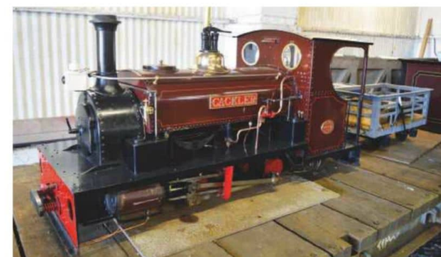
A lovely 5 inch gauge model of Jerry M's 1898-built sister, Cackler on display at Minfordd in May 2018. This view shows the neat outlines of the design to advantage, including a cab cut-out profile similar to several Thomas Green and Hudswell Clarke products of the engine's period of construction. The access holes for the cylinders in the leading bufferbeam are also evident.
