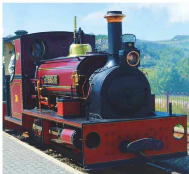
Lilla's basic proportions were used for two new locomotives constructed in 1895-8 for the Dinorwic Mills tramway, although the design was heavily modified with two injectors (no pump); dropped rear footplate; round cab spectacles and altered cut-outs; dome mounted safety valves; Dinorwic 'Port' pattern drawgear and rectangular (as opposed to radiused) bufferbeams. The hole for the linkage to operate the uncoupling mechanism for the leading set of drawgear can still be seen in this May 2018 view of Hollycombe -based 1895 vintage Jerry M (formerly Vaenol ) on the W.H.R. road at Harbour Station, Porthmadog.
