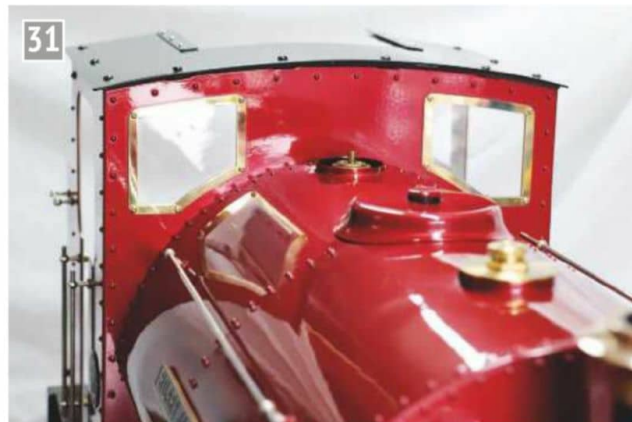
Window frames in position.
