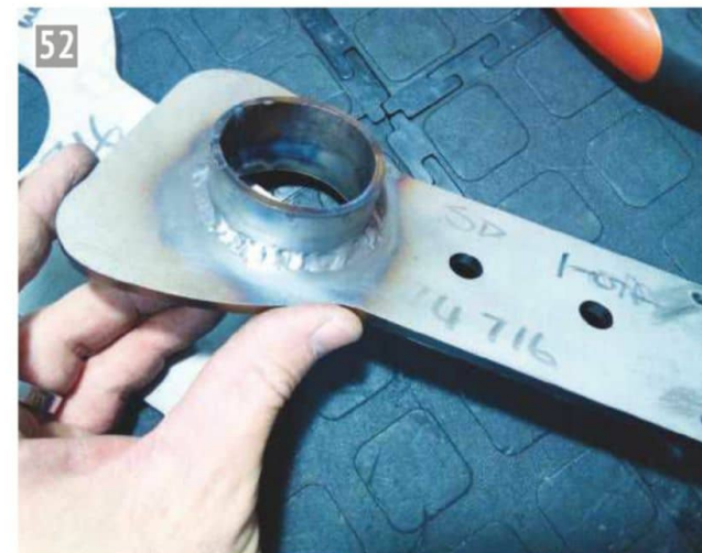
Firebox fillet weld.
