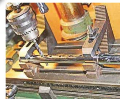
John Garnish offers advice on accurately drilling holes across a diameter.
