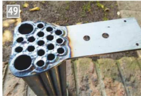
Tubes welded to the firebox tubeplate.
