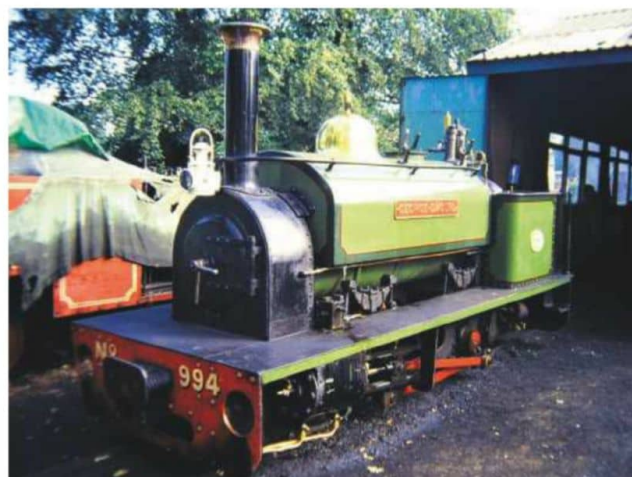
Another 'on shed' view, but this time showing classmate, George Sholto at Bressingham in July 1999. The Penrhyn -pattern buffer beam, without buffers (in contrast to Dinorwic Quarry and Port practice) is very much in evidence although the cab had yet to be fitted at this stage.
