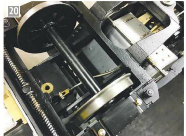
Stainless steel ashpan obscured by the pony truck and frame extensions.
