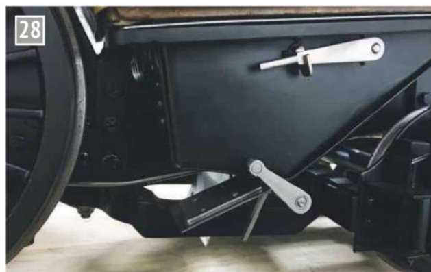
Ashpan levers. Grate drop door lever above and shutter closing lever at the bottom.
