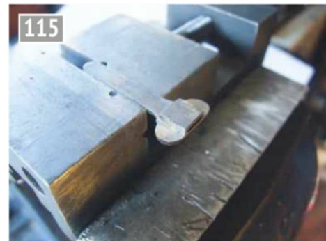
115 The central lamp bracket has been cut out with the channel silver soldered and the slot for the blade opened out to ensure it is functional.
