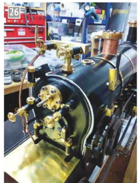
Fittings assembled on the backhead.
