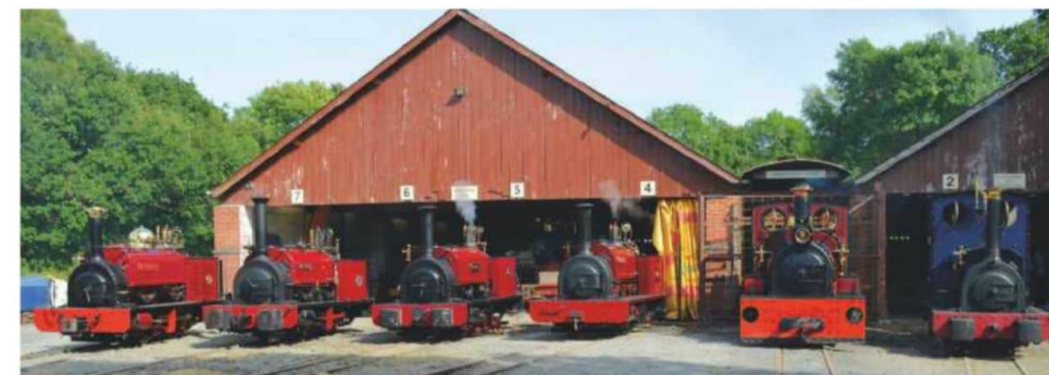
The Dinorwic 'line-up' at Minfordd during the Hunslet 125 Gala. From left to right can be seen Velinheli ; Alice ; George B ; Cloister ; Jerry M , and Holy War . Note the fixing holes where the buffers have been removed from Velinheli and Cloister during the preservation era.
