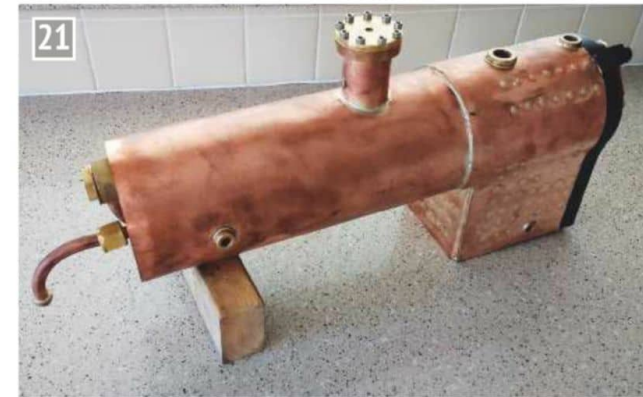
Boiler assembled with superheater pipe.
