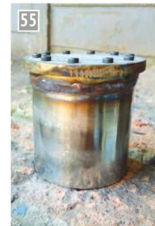
Regulator boiler dome.
