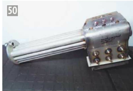
Firebox and tubes welded.
