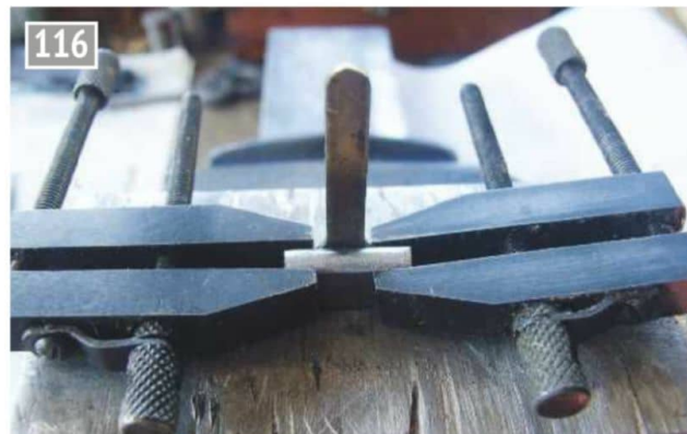
116 Here the central lamp bracket is being formed over a steel plate which has been given a \frac{3}{16} inch radius.
