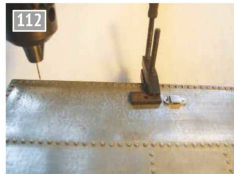
112 This picture shows the first off-set rivet hole drilled and the rivet held up from underneath with a small clamp and pieces of steel packing for one of the lower brackets.
