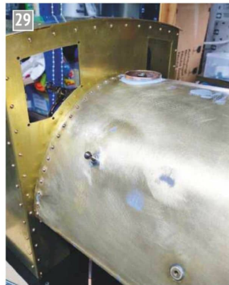
Saddle tank ready for painting.
