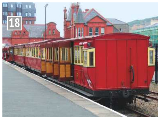
Typical carriage with Guard's side look out. Built by Metropolitan Carriage and Wagon Co. in 1913. The railway adopted bogie carriages early on.
