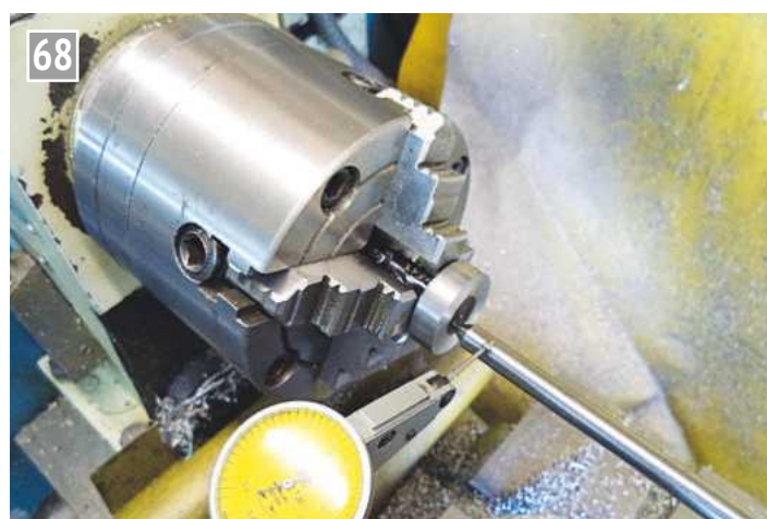
68 Setting the throw in the lathe.
