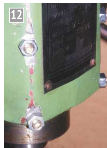
ME Pressure pad screws installed.
