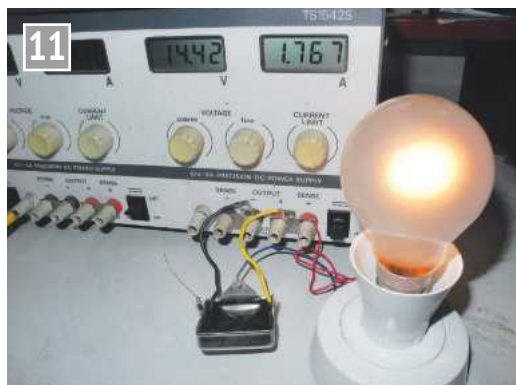
Regulator bench test.
