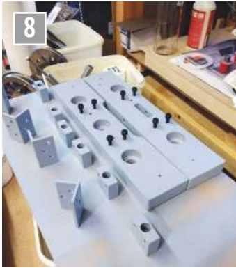
Component parts sprayed with acid etch paint.
