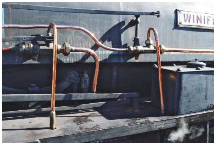
A view for modellers – Winifred's injectors, both on the right hand side. This feature did not find its way on to Pearl.
