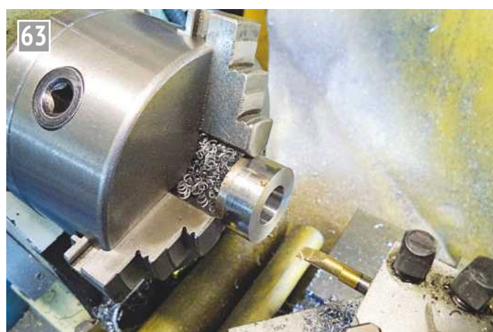
63 Boring the eccentric outer.
