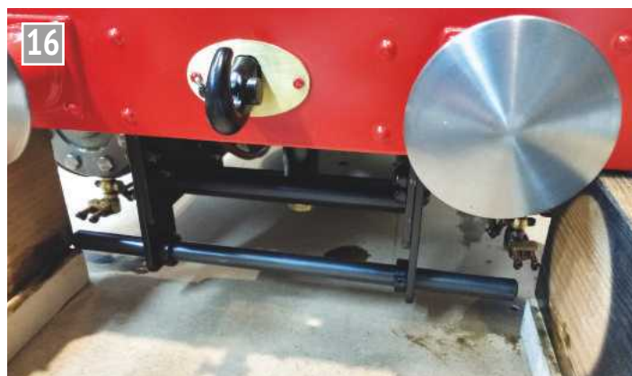
Derailment support bar.
