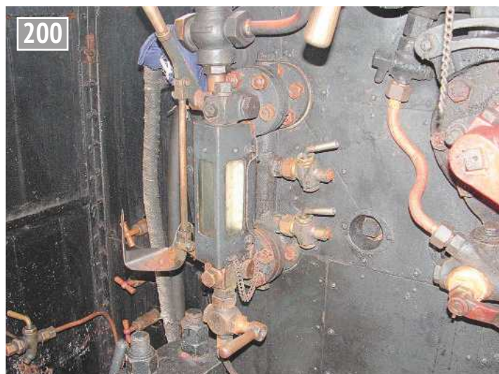
The water gauge, or 'gauge frame'.
