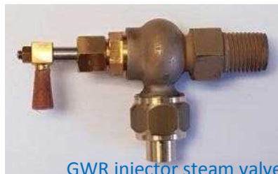
GWR injector steam valve
