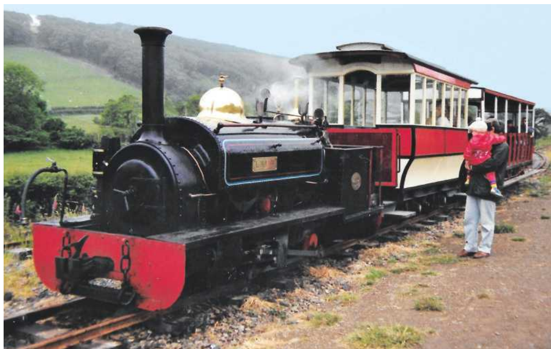
Penrhyn Railway 'Port' class 0-4-0ST Lilian is seen here at Canna Park on the Launceston Steam Railway in June 1990. The locomotive had first been restored to working order by Nigel Bowman in Surrey in 1968.
