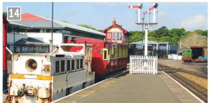
1994 built former Channel Tunnel and Jubilee Line extension Hunslet locomotive, renamed Ailsa stands at Douglas semaphore signals. Restricted vision limits it to shunting and works duties.
