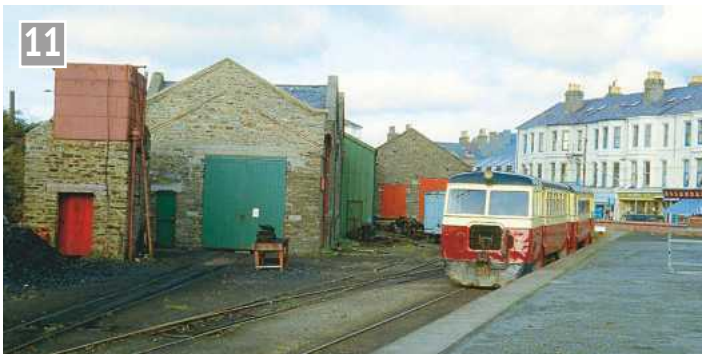
Former County Donegal Joint Railway railcars built by Walker Brothers of Wigan. Seen at Port Erin in 1980. Cars were used back to back, sometimes with a parcel van between. (Photo: Roger Backhouse 1980.)
