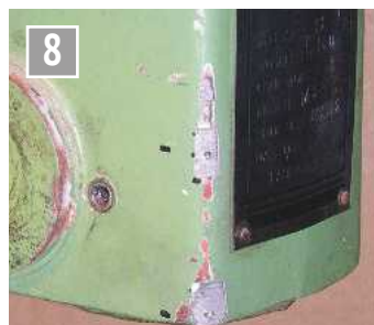
Marking out for the pressure pad screws.
