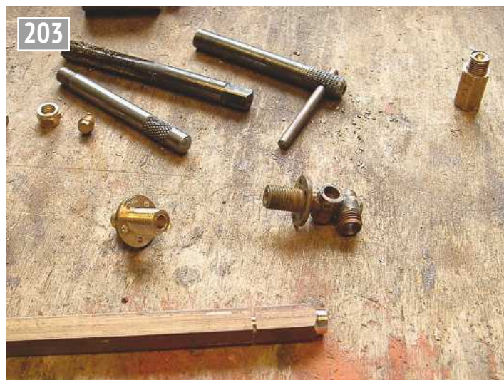
Fabricating parts for the water gauge.
