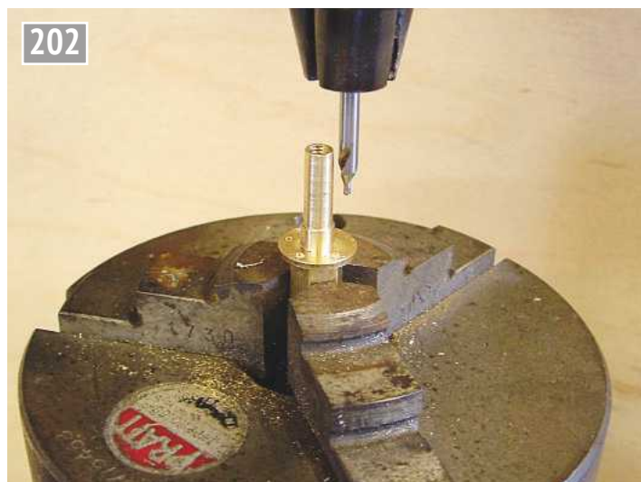
Drilling the five holes for the water gauge studs.
