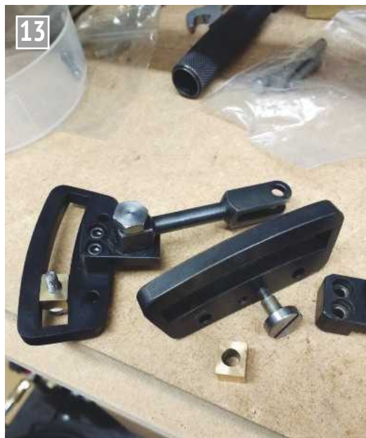
Completed expansion links.
