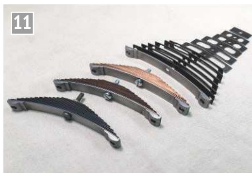
Leaf springs with leaves of four different types for test.
