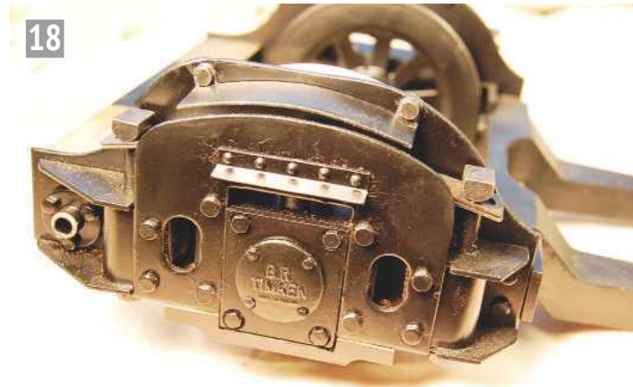
Pony truck top two leaves visible with semi-circular spring hangers. These tops could be replaced with the more prototypical pin through the vertical shaft.
