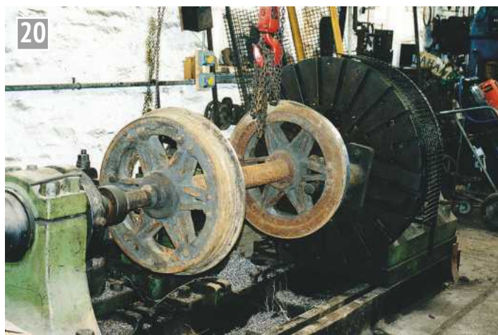
Wheel lathe in the workshops.
