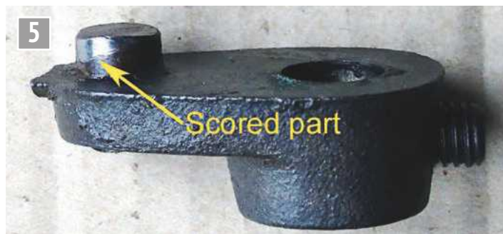
Wear in the tensioning system.
