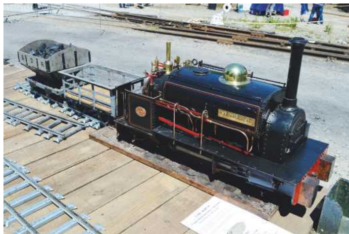
This fine 5 inch gauge model of the basic Penrhyn 'Port' class locomotive by Steve Milns of Shropshire appeared at the Hunslet 125 Gala in May 2018. Despite being constructed substantially to Winifred's configuration (note the injector configuration and early pattern smokebox door with which this engine was built), the model has Dinorwic-pattern buffers and the name (and worksplate) of Lady Madcap.
