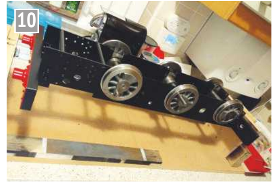
Chassis mounted in assembly jig.
