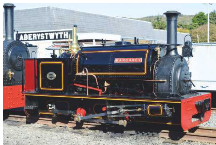
A right hand view of Margaret taken at Aberystwyth during the 'Forgotten Engines' Gala of 2016. Note the loss of the upper flared portion of the safety valve 'trumpet'.
