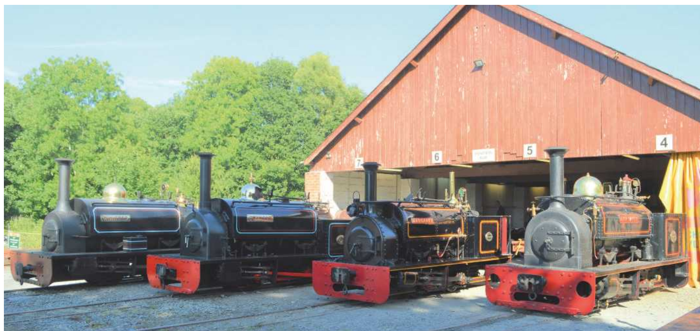
Ex-Penrhyn locomotive line-up at Minfordd during the Hunslet 125 Gala. From left to right we have Winifred; Gwynedd; Margaret, and Hugh Napier. The effect of the 1980s re-boiling on Gwynedd is very much in evidence, namely the higher pitched boiler (in comparison to Winifred) with later pattern smokebox and door, although Salter safety valves were retained.
