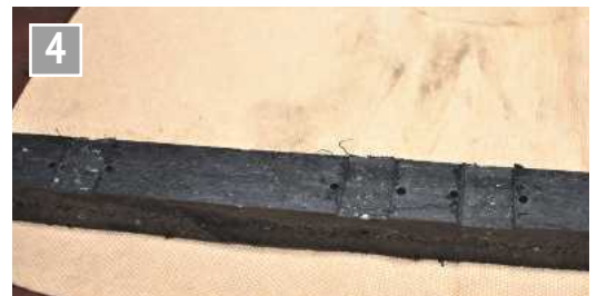
A machined sleeper showing the rail seating and drilled holes for the fixings.
