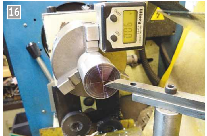
Marking up the front and rear covers.
