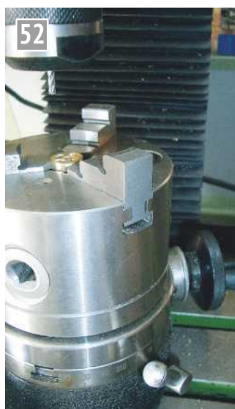
Milling the ports for the steam brake valve.
