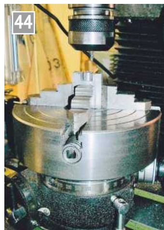
Profiling a crosshead on the rotary table.
