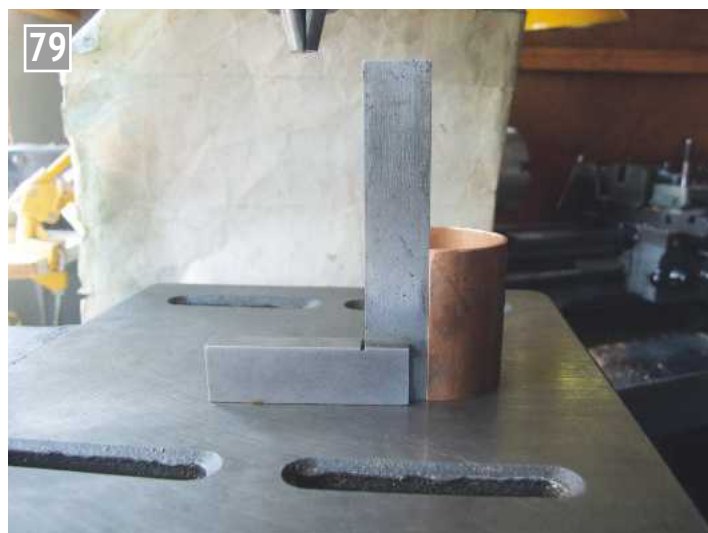
Checking the cut ends of the casing tube are flat and square.
