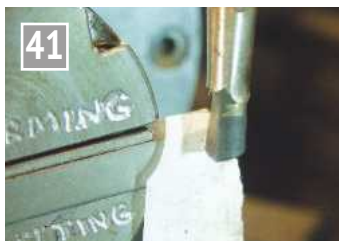
Using cigarette paper to set the first boring head datum.
