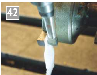
Finding a second datum on the other side of the blank.
