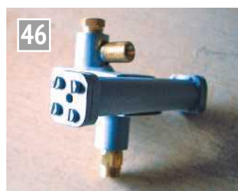
Water feed pump.
