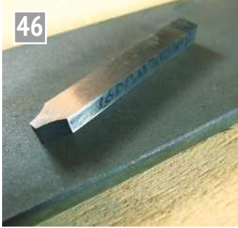
The finished tool after heat treatment.
