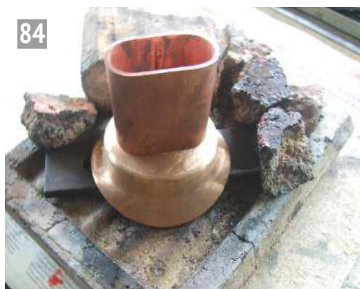
This is the set-up for the silver soldering operation to attach the upper casing to the bonnet casting; the curved lower edge is sitting astride a piece of steel bar.
