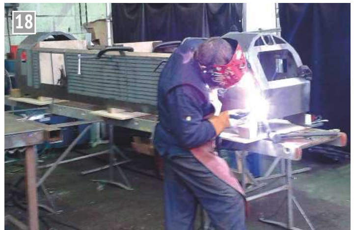
Stainless steel rods were used.
