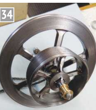
Rope pulley attached to the flywheel.
