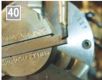
Lining up the tool blank to set the datum.
