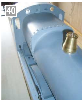
Cab roof and spectacle plate in place.
