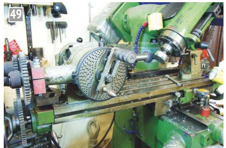
The setup used to cut the helical gears.
