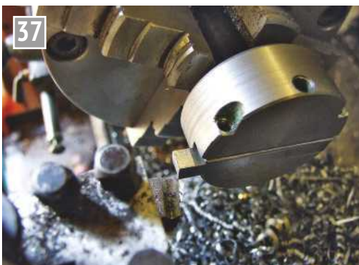
Machining the end of the blank.
