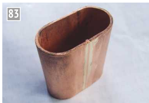
Here the edge of the joining strip has been carefully filed away to leave a flat surface.
