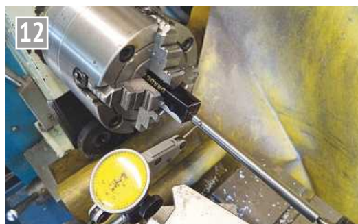
Trueing up the valve chest using the wobble bar.
