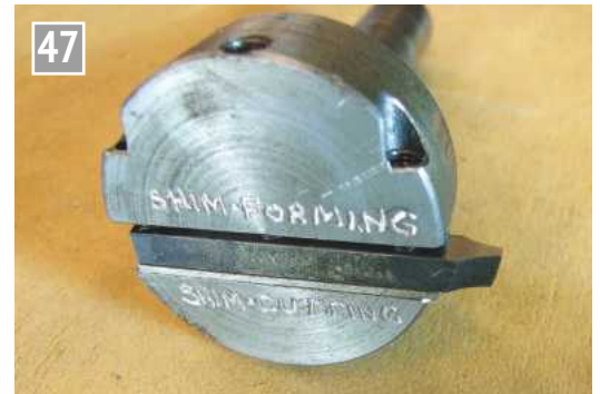
The tool fitted into the flycutter holder.
