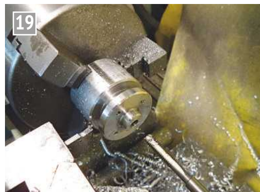
Tapping for the piston rod gland.
