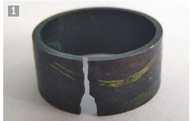
An un-annealed section of brass tube exposed to ammonia.
