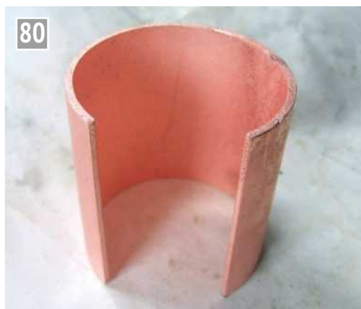
The casing tube cleaned and ready for the forming operation.
