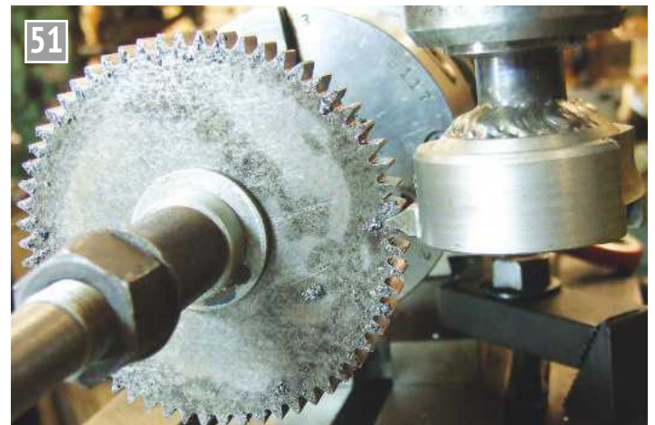
Cutting a 60 tooth gear as an encore.
