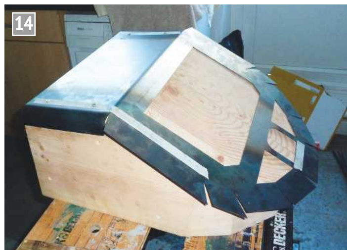
Nose panel on the wooden former.
