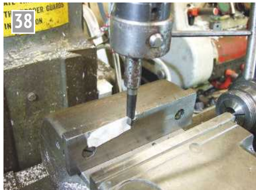
Setting the boring head to the correct radius.
