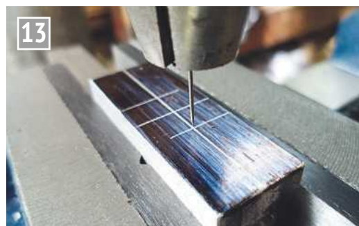
Centering on the inlet and exhaust ports using a 'sticky pin'.
