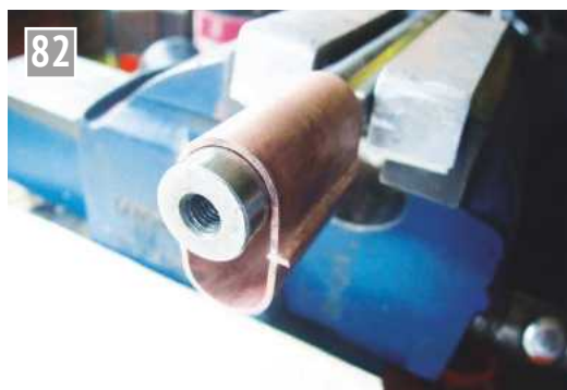
A final adjustment was made to the radii by inserting the forming bar and using a soft rubber mallet around each end.
