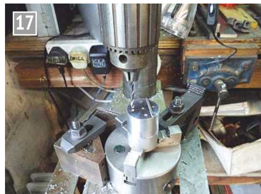
Drilling on the pitch circle diameter.
