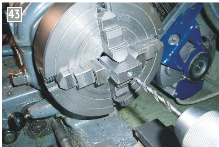
Drilling a crosshead for the piston rod.
