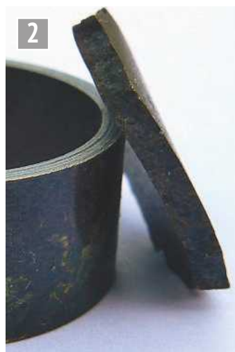
A fragment of a deep drawing brass cup, un-annealed and exposed to ammonia, which has cracked and failed, showing the failure surface.
