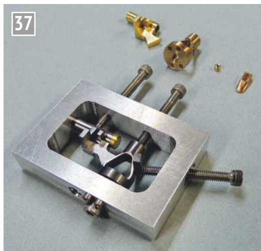
Soldering fixture for the governor.
