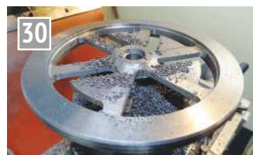
Machining the barring teeth in the flywheel.
