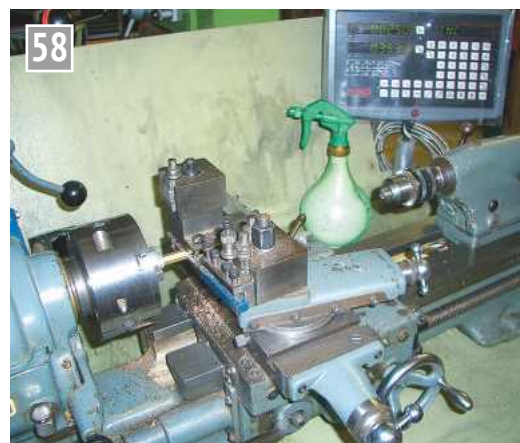
Turning out fittings with the help of the DRO.
