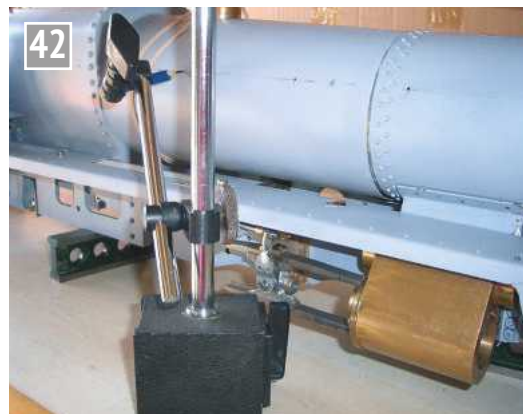
Marking out for the handrail stanchions.
