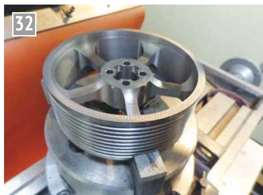
Machining the rope pulley.
