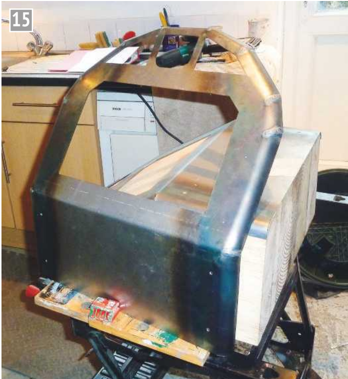
Nose panel formed and welded.
