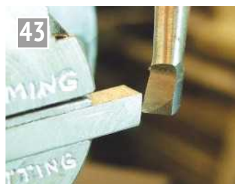
Touching the cutter against the end of the tool blank.
