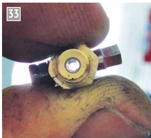
Taper cock hole perfectly aligned.
