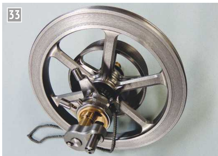
Machining the barring teeth in the flywheel.
