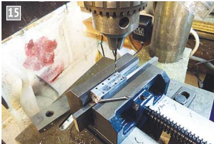
Drilling the clamp down holes.
