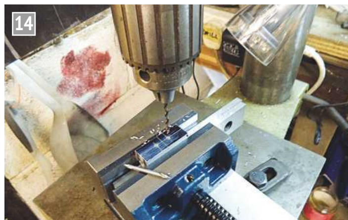
Drilling the inlet and exhaust ports.
