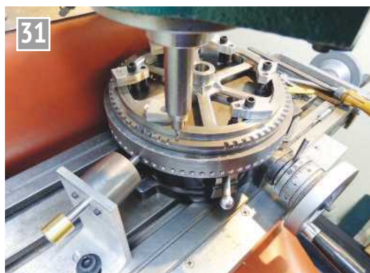
Machining the barring teeth in the flywheel.
