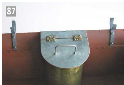
Here the brackets are attached to the bunker plate work.
