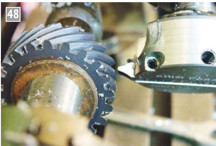
Using the tool to cut a helical gear.
