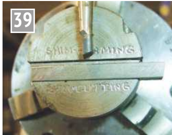
Setting the boring tool height.
