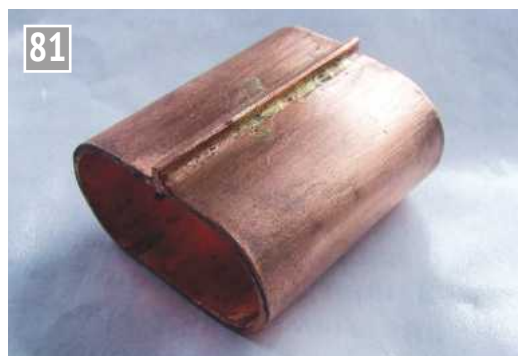
To join the ends of the casing, a narrow strip of copper was inserted to be just protruding on the inside. The joint was hard silver soldered as it must not be disturbed when the second heating is carried out.
