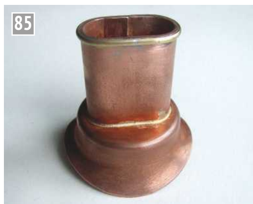
The beading successfully added to the top of the safety valve casing and secured with soft solder.
