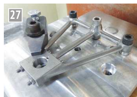
The yoke mounted on a fixture for machining.
