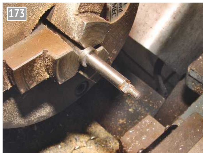
Putting the square on the end of the regulator shaft.
