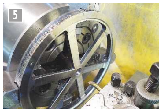
Boring the flywheel.
