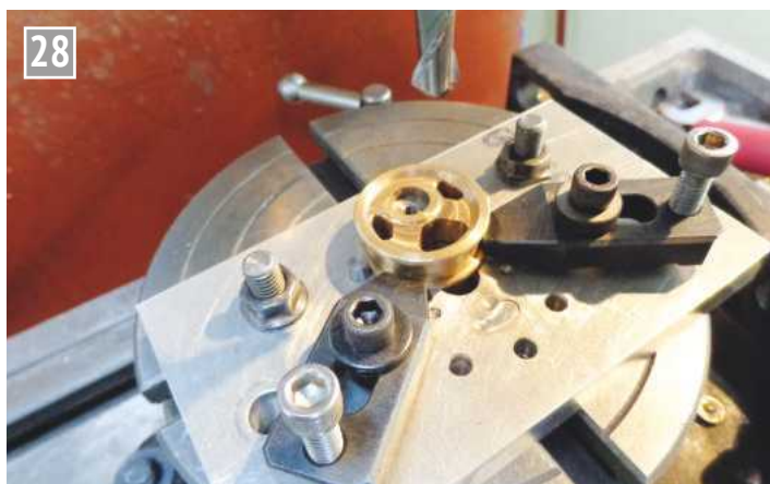
Machining a sheave.
