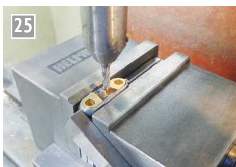
Machining a link.
