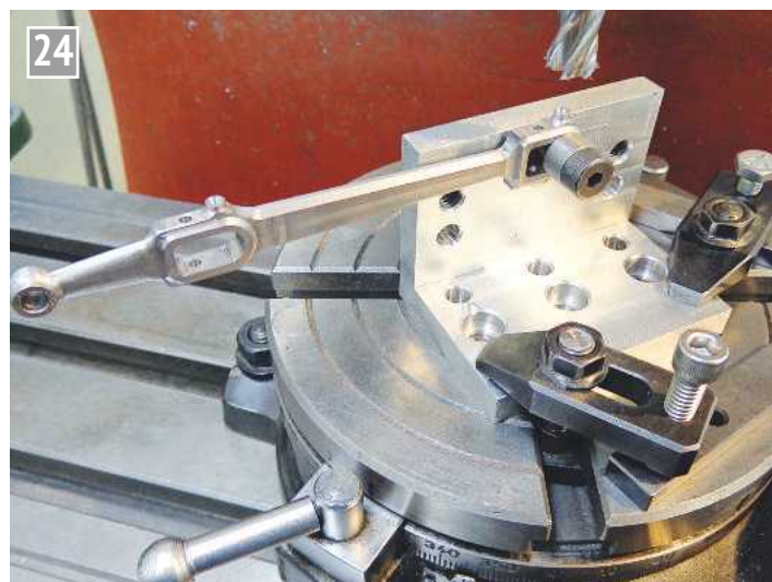
Setup for machining the rocker arms.
