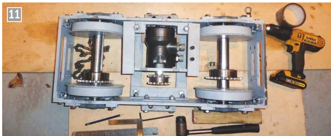
Placement of the motor.
