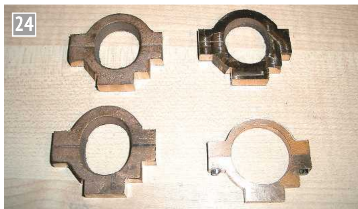
A casting becomes an eccentric strap.
