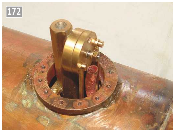
The regulator installed in the author's Y4.
