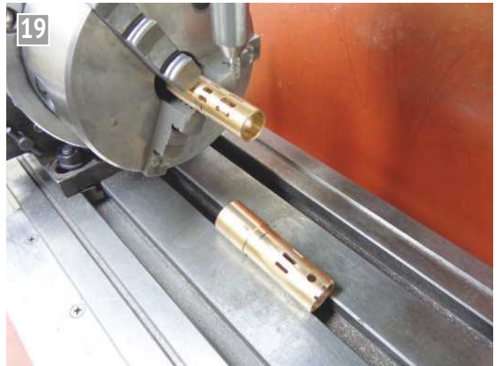
Rotary valve sleeves – note extra hole in the LP sleeve.
