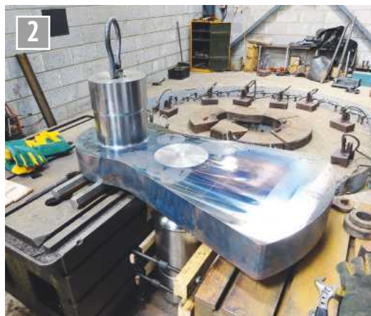
Assembling the crank axle at Darlington Locomotive Works (photo: David Elliott).
