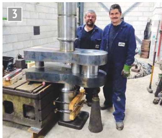
The crank axle fully assembled (photo: David Elliott).
