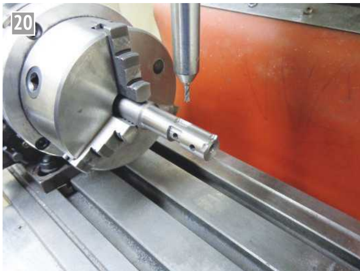
Machining a rotary valve.
