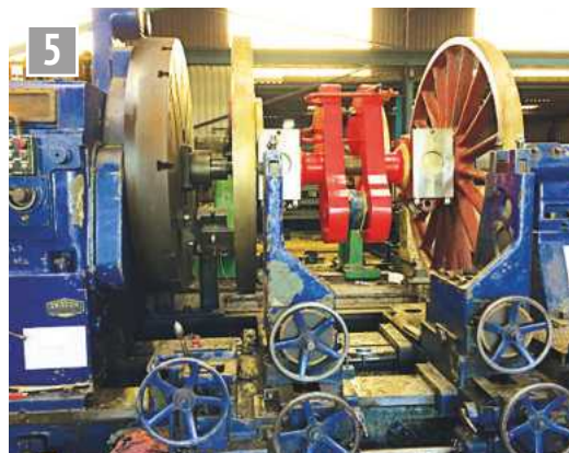
The crank axle wheelset is set up in the wheel lathe to turn the rims (photo: Rob le Chevalier).
