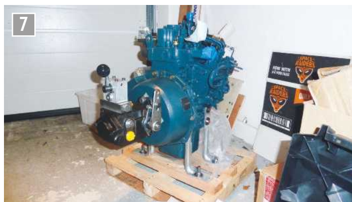
The water cooled, two-cylinder Diesel engine used in Queen's Messenger.
