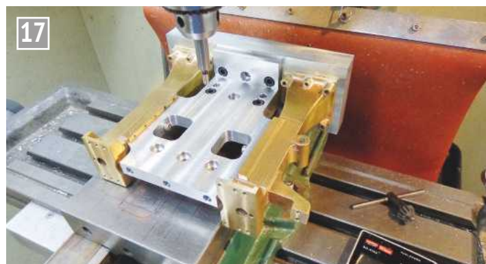
Picking up the position on the fixture.
