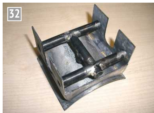
Smoke box saddle fabrication.
