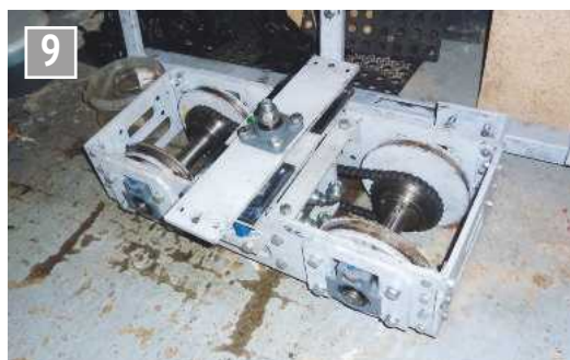
View of the bogie showing the chain drive.
