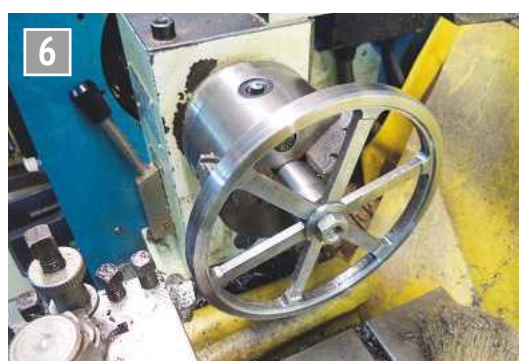
Truing up the rim with the wheel mounted on a mandrel.
