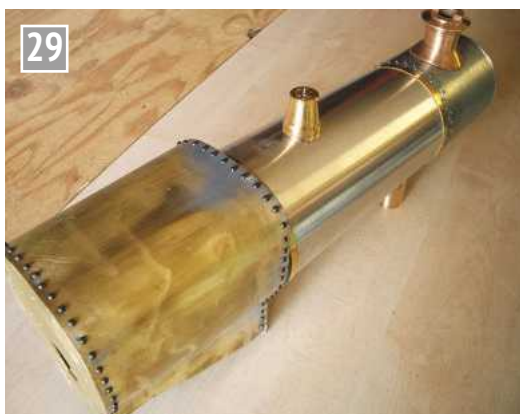
Complete boiler assembly.
