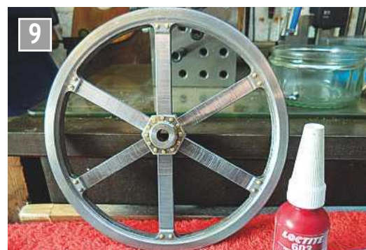
Flywheel assembled with Loctite.
