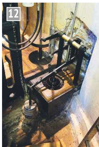
The cataract or timing device was derived from a water clock and enabled automatic operation.
