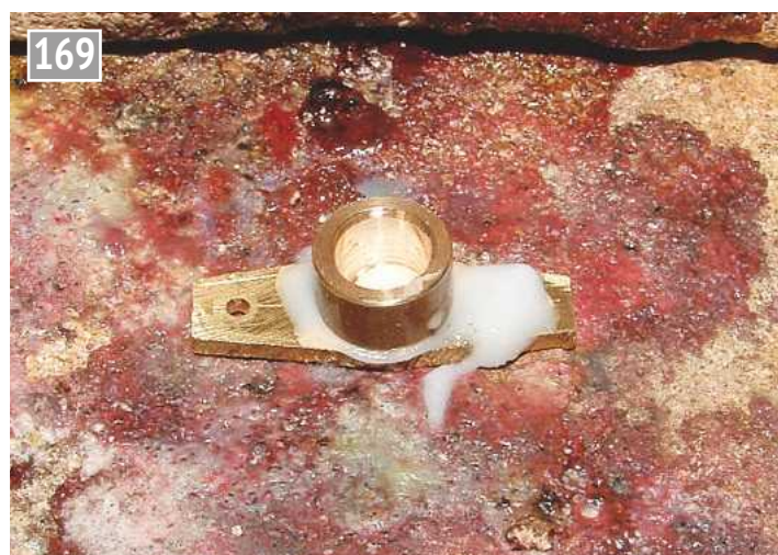
Making the regulator crank.
