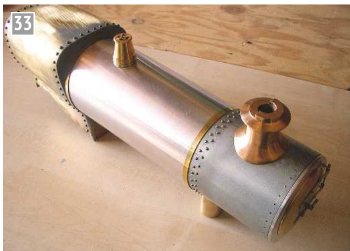
Smoke box door fitted.
