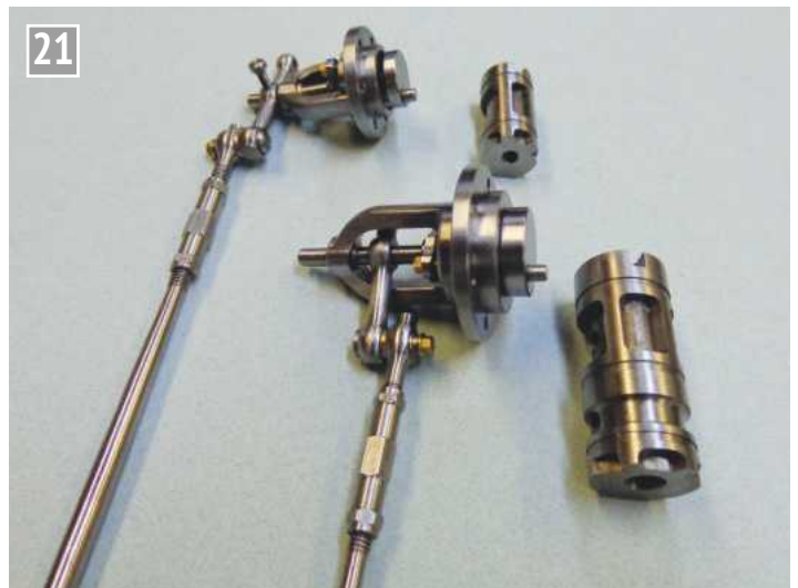
Valve operating linkage.
