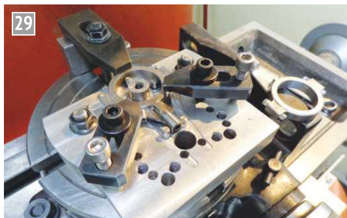
Machining a strap.
