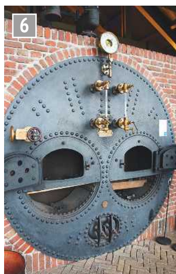
Re-erected Lancashire type boiler front obtained from Belgium gives a good idea of how the boilers once looked. These had twin flues.
