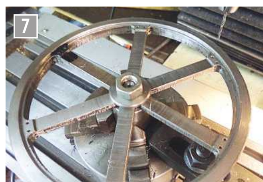
Drilling the flywheel for dummy rivets.
