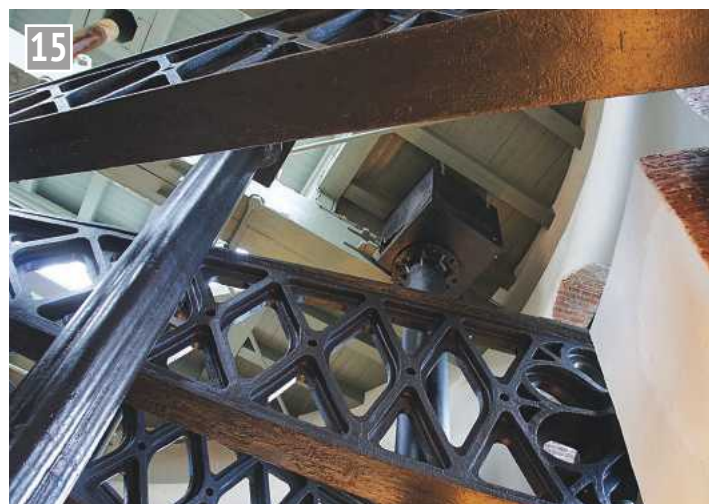
'The hydraulic' - one of the two columns visible through the beams. This held the great cap in position while pump clacks had time to close.
