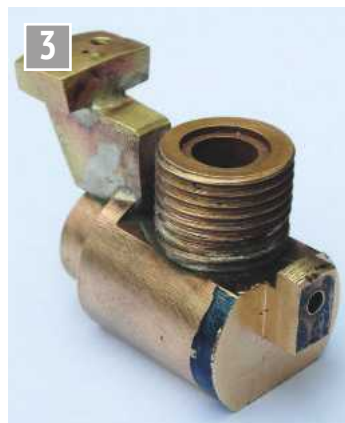
The completed block.
