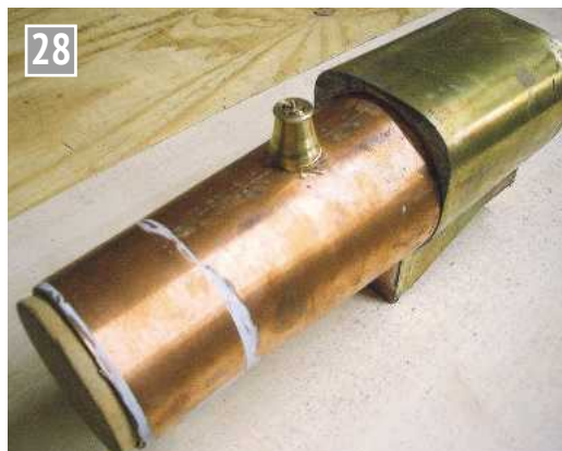
Old boiler barrel given a new lease of life.
