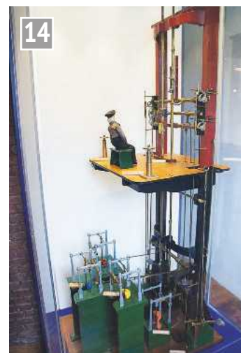
For an engine as big as this, a model is sometimes the best way to show the controls and interlocks.
