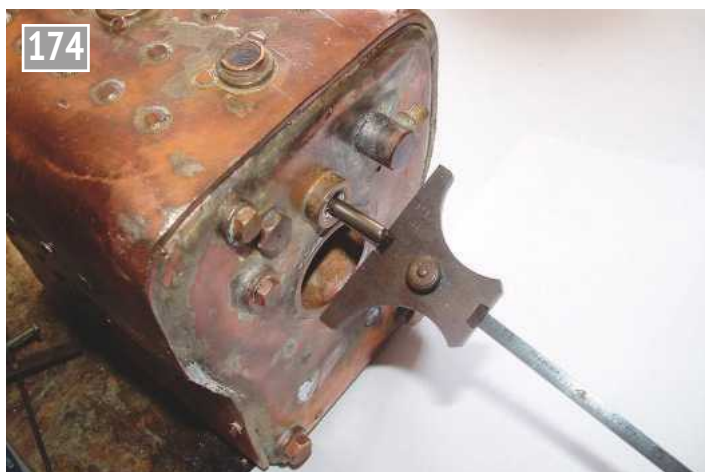
Checking the length of the regulator shaft.
