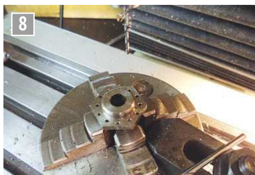
Drilling the hubs for the dummy rivets.
