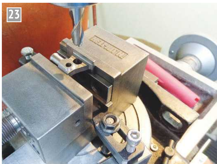
Machining the crosshead.
