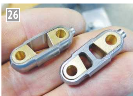
Two links at different stages of machining.
