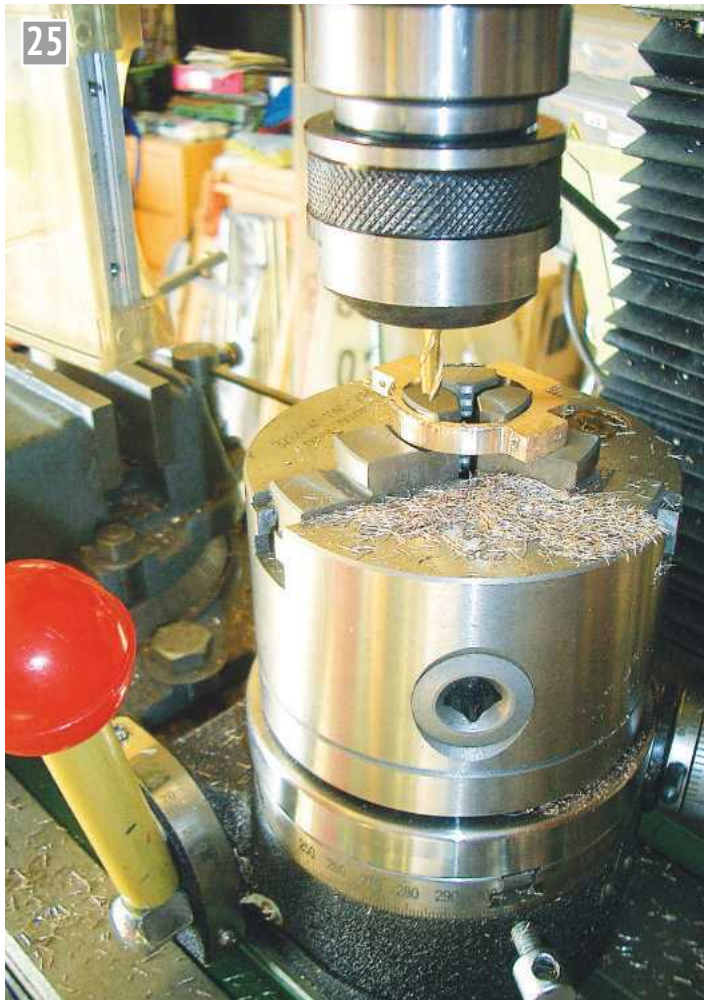
Shaping the outside of a strap.
