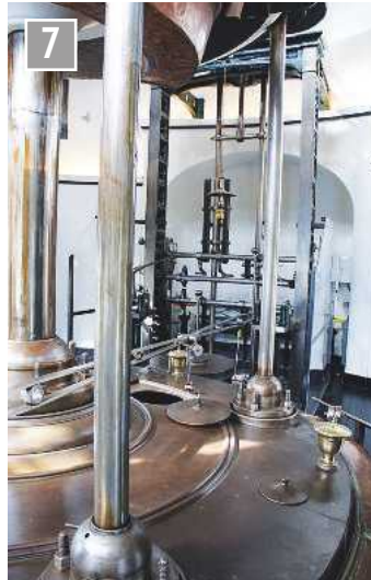
The great cap weighs 82 tons. Inner ends of the beams link to the cap which is lifted by both HP and LP pistons inside the annular cylinder.
