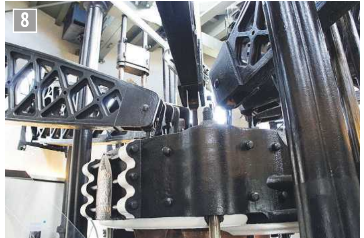
The great cap weighs 82 tons. Inner ends of the beams link to the cap which is lifted by both HP and LP pistons inside the annular cylinder.
