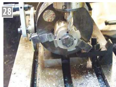
Cleaning out the gash.
