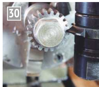
Cutting the gear.
