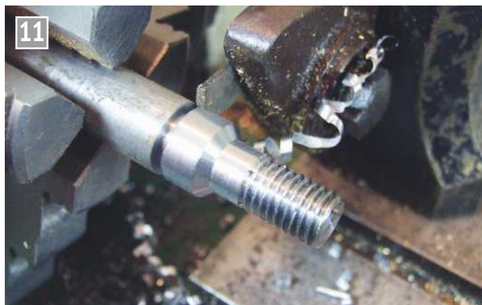
Parting off a button blank.
