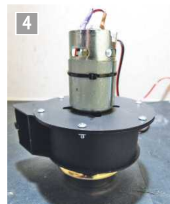
The small blower unit.
