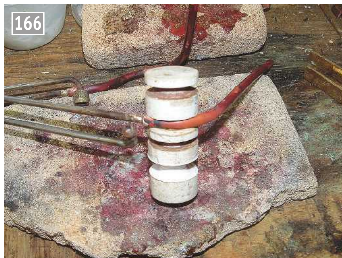
Pipe bending former.
