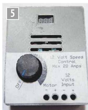
Blower speed control.
