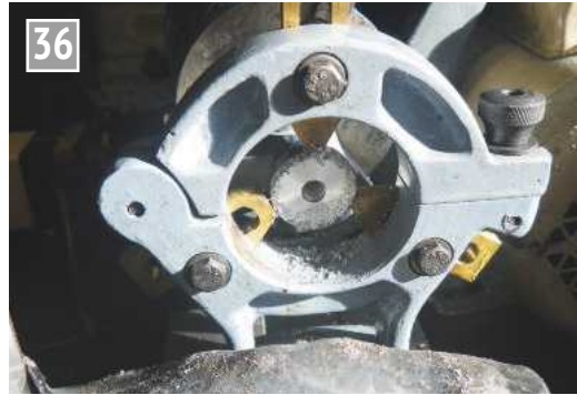
Drilling the passageways with the help of a fixed steady.
