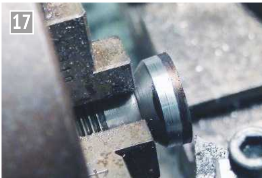
17 Forming the clearance angle on the button.
