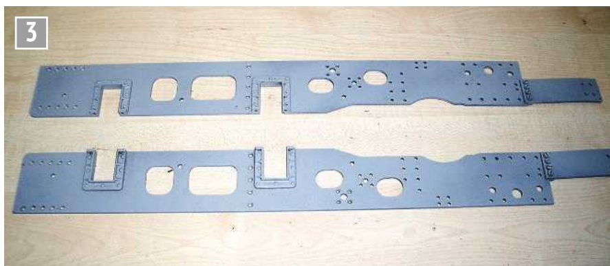
The restored main frames.
