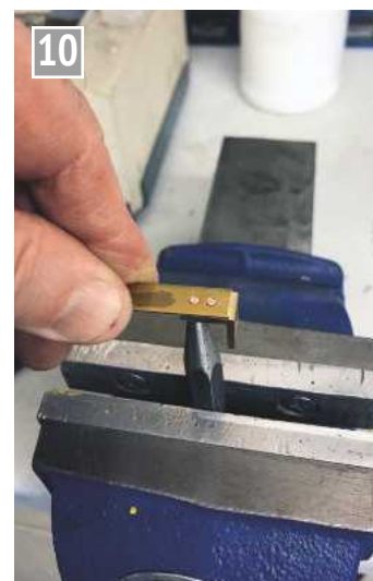
Attaching the angles to the bands.
