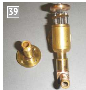
The steam control valve.
