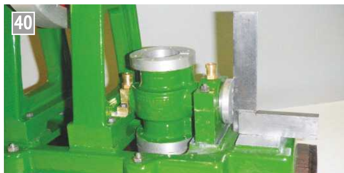
Checking the squareness of the port face.
