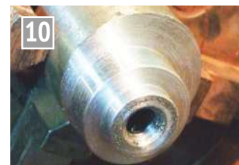
Initial machining on the eccentric cutter blank.
