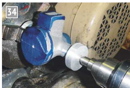
Machining the valve block between centres.
