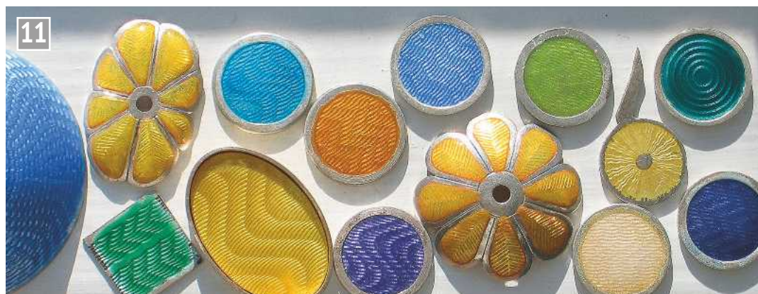
Trial samples of transparent enamels to assess their suitability together on the patterned silver surfaces.
