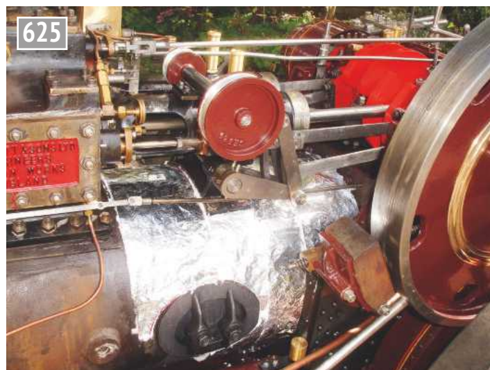
Lagging part complete.
