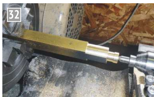
Rounding the sides of the piston rod.
