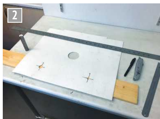
Cutting out the insulating material.
