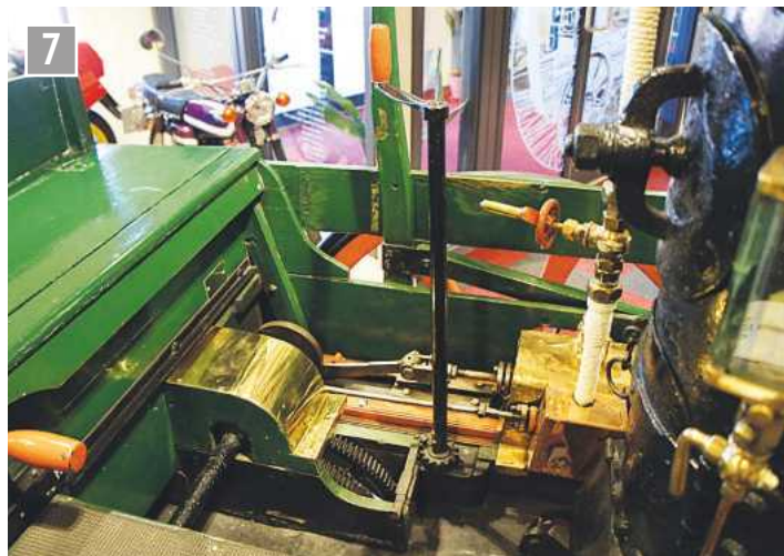
A vertical pillar with a short-handled lever is the steering gear linked to the front wheel; the machine must have been difficult to control.
