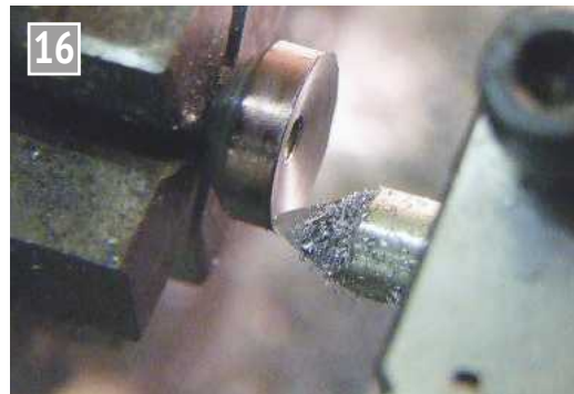
16 Forming the top rake angle on the button.
