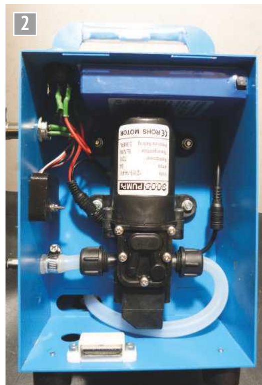
Pump and battery mounted in the box.
