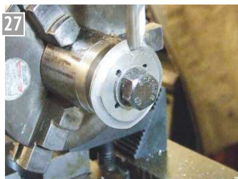
Gashing out the profiled cutter blank.
