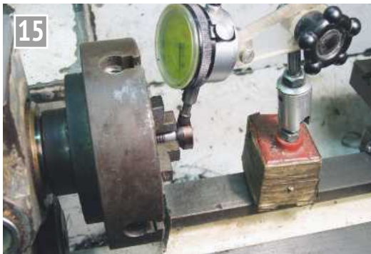
15 Setting the button to run true.
