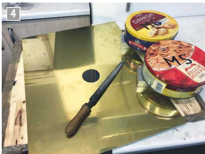
Filing out the hole for the dome.
