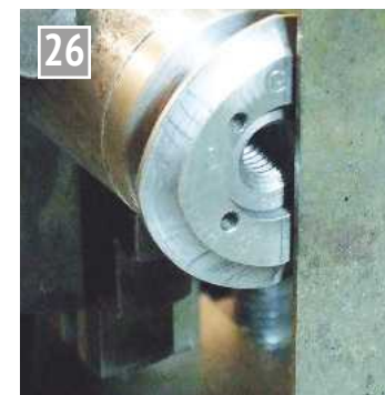
Lining up the high points on the cutter blank. ➤
