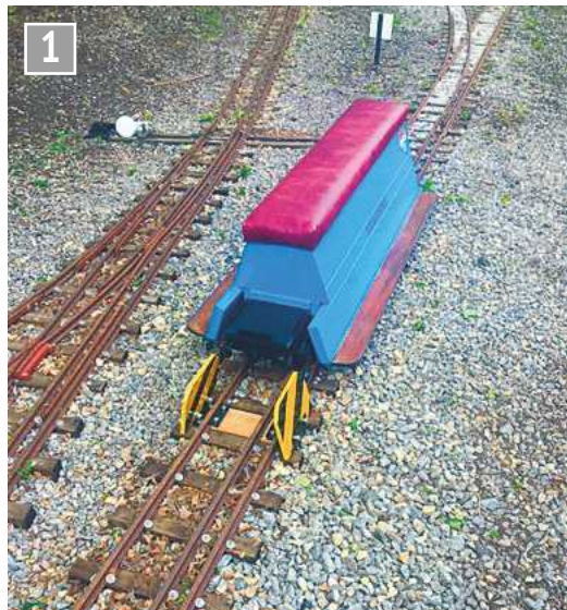
The device, when deployed, prevents incursion of unwanted vehicles.
