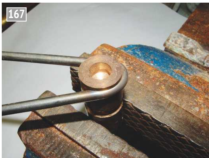
Bending the pipes is a simple job.
