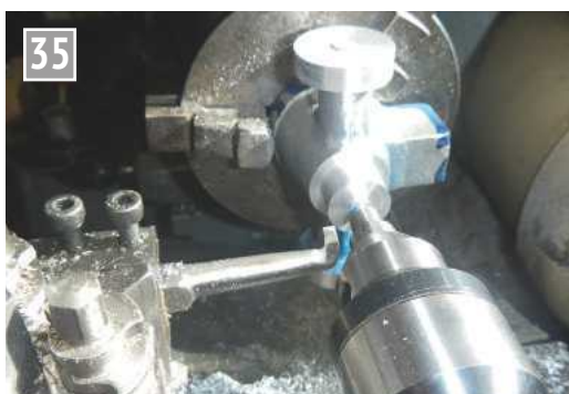
Finishing the bolt end profile.
