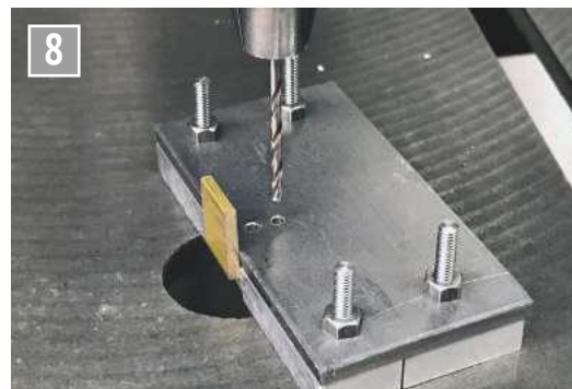
Using a jig to drill the holes in the angles.
