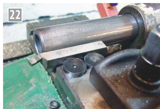
Truing the button tool in the toolpost.
