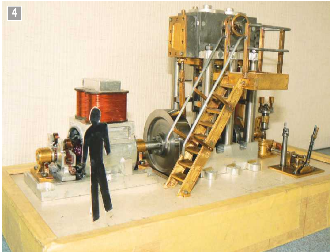
Vertical engine and generator, Stamford MES (photo courtesy of Richard Wright).
