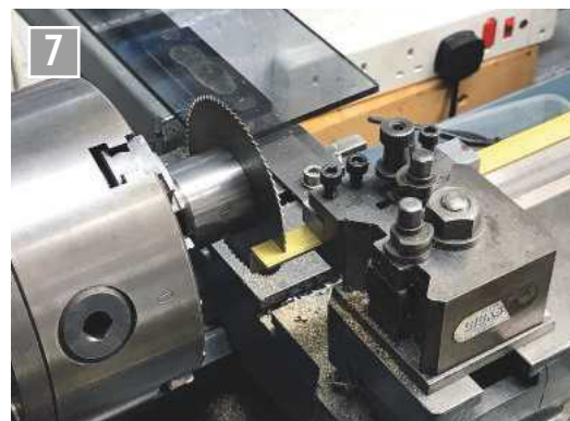
Mass production of the little bits of angle for the ends of the bands.
