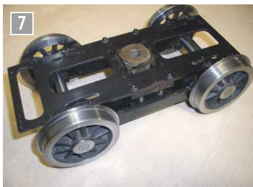
Front bogie after cleaning.
