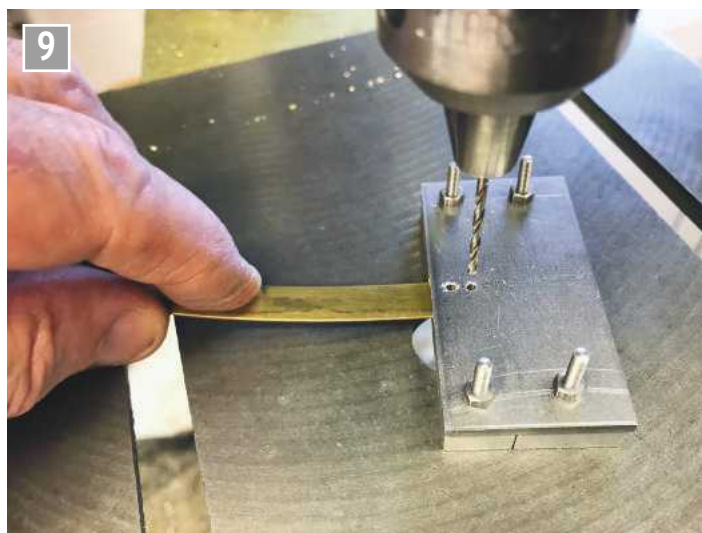
Using the same jig to put the corresponding holes in the bands.
