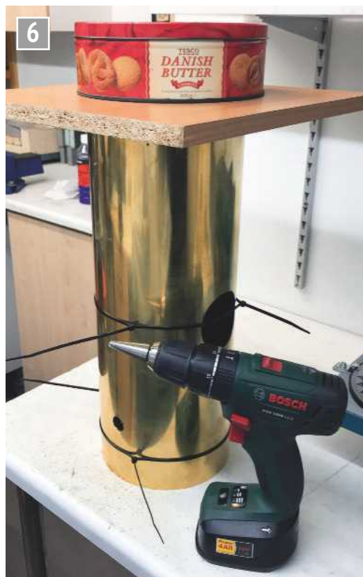
Enlarging the holes for the clacks.
