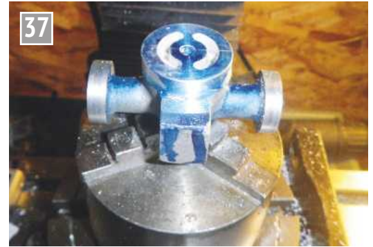
Milling the steam ports on a rotary table.
