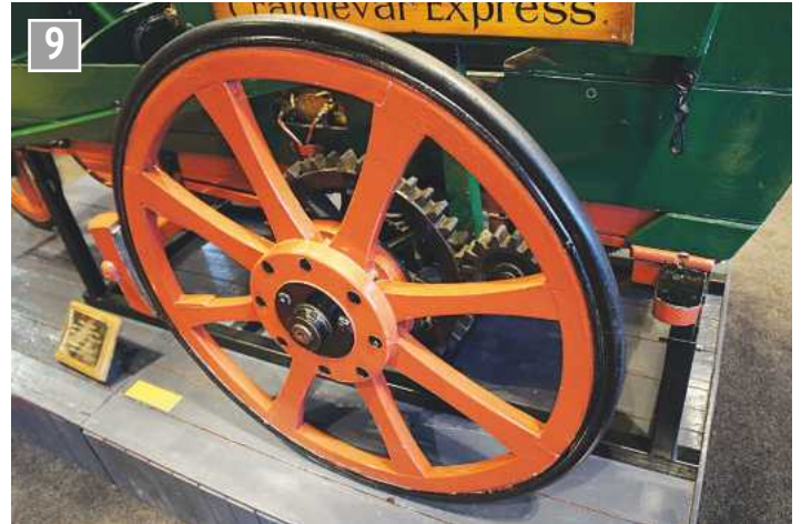
Rear wheel with a simple rim brake to the left. Solid rubber tyres replaced iron in the 1960s restoration.
