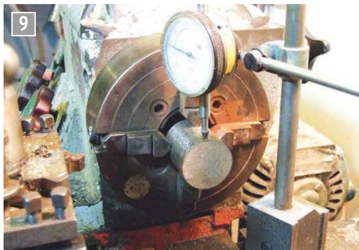
Truing up the plain cutter mandrel blank.
