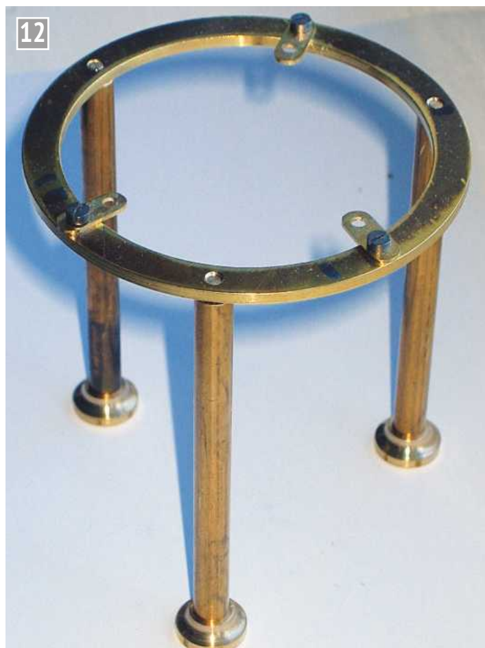
In this assembly/display stand the removable legs could be screwed into the top or below for easy working on any part of the complex mechanism; important where considerable trial and error of mating parts is required.
