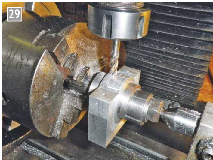
Forming the curvature on the top of the bearing block.
