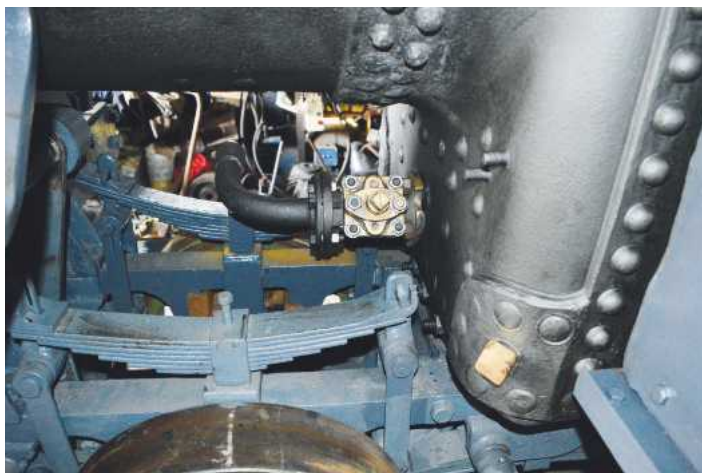
LEFT: The bogie used on these Baldwin locomotives is quite sophisticated and was described by the makers as being of the 'swing bolster' type. The housing for the control spring (which is within the central pivot) was anchored to the lower part of the 'fore and aft' swinging arms as shown here, with the upper pivots attached to the bogie itself. Limited provision was also made for vertical deflection of the bogie axleboxes to cater for inequalities in the road, a common occurrence on the Western Front! RIGHT: On the extreme left of this illustration can be seen the transmission bellcrank for the handbrake linkage.
