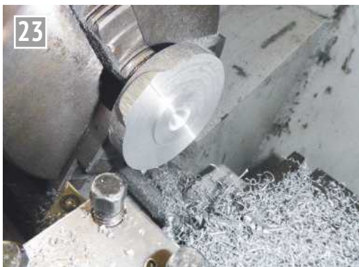
Turning the cylinder bottom cover.
