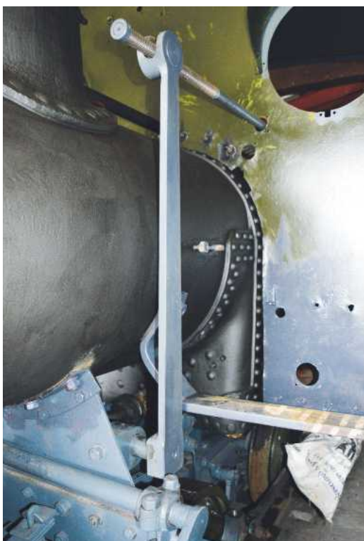
LEFT: The tank supports are bolted to the boiler in the manner shown here. RIGHT: This is a detail much of which is not normally visible on the Baldwin 10-12-D locomotives as shown in working condition. The handbrake is actuated by means of a mechanism consisting of a horizontal screw and a vertical lever, which has had to be completely renewed during the restoration work.
