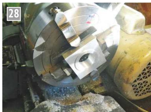
Finishing the profile of the bearing block.
