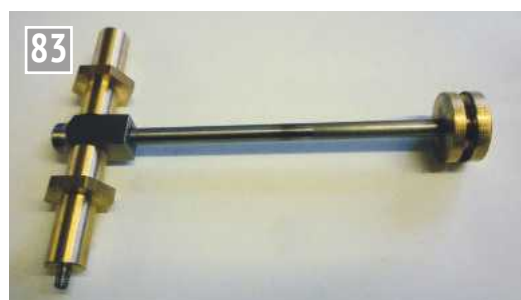
A pair of crosshead guides mounted on their piston rod.
