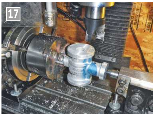
Facing off one end of the cylinder.
