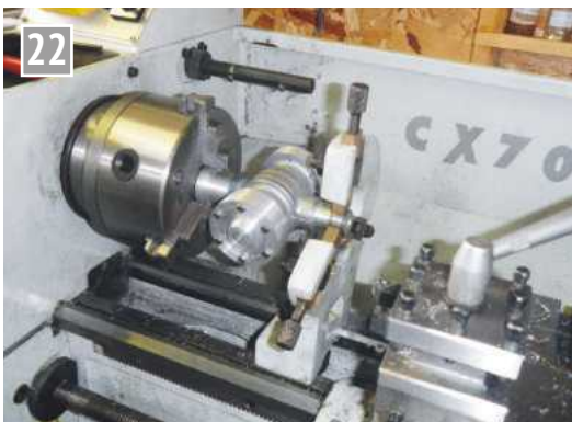
Drilling the hole for the rotational dowel.
