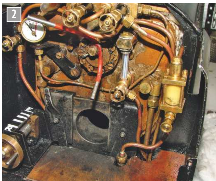
A sight glass full of mayonnaise - no hope of seeing the oil feed rate.
