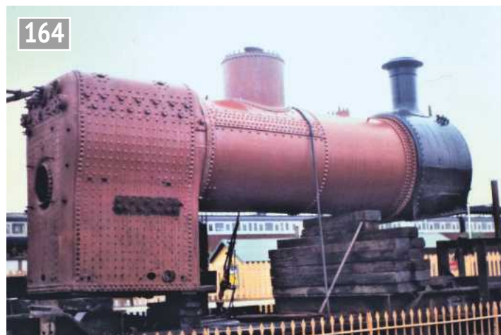
Pannier boiler, showing the inner dome.
