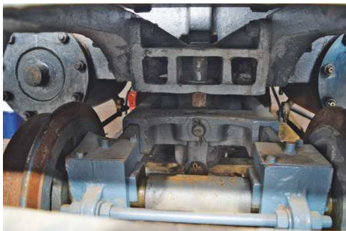
LEFT: The bogie used on these Baldwin locomotives is quite sophisticated and was described by the makers as being of the 'swing bolster' type. The housing for the control spring (which is within the central pivot) was anchored to the lower part of the 'fore and aft' swinging arms as shown here, with the upper pivots attached to the bogie itself. Limited provision was also made for vertical deflection of the bogie axleboxes to cater for inequalities in the road, a common occurrence on the Western Front! RIGHT: On the extreme left of this illustration can be seen the transmission bellcrank for the handbrake linkage.
