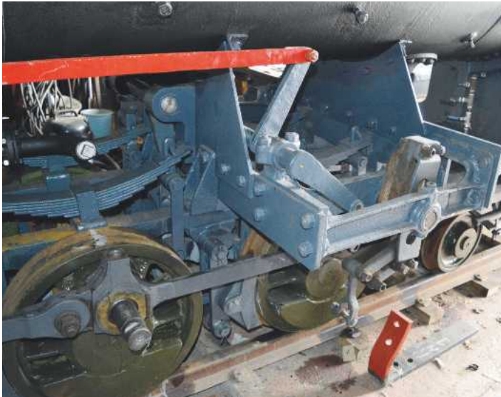
At the time of taking the photographs, the valve gear components had yet to be fully assembled on either side of the locomotive but the bracket holding the expansion link is clearly visible here. Note that, as with other components of the locomotive, such as the boiler support plates, much use is made of bolts rather than rivets as an aid to interchangeability of components. The reversing lever, reach rod and its associated bellcrank are located on the right-hand side of the locomotive. The handbrake cross-shaft can also be seen in this view with its bearings anchored to the rear of the trailing boiler support plate.
