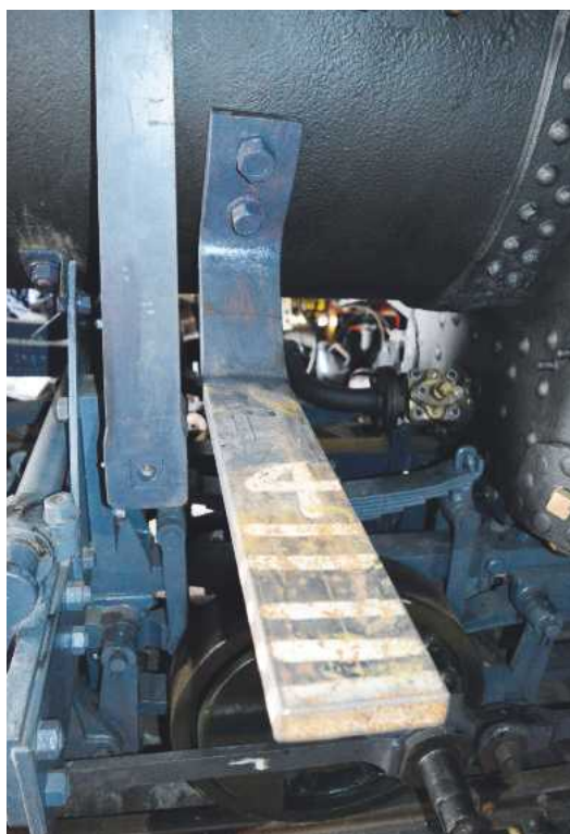
LEFT: The tank supports are bolted to the boiler in the manner shown here. RIGHT: This is a detail much of which is not normally visible on the Baldwin 10-12-D locomotives as shown in working condition. The handbrake is actuated by means of a mechanism consisting of a horizontal screw and a vertical lever, which has had to be completely renewed during the restoration work.
