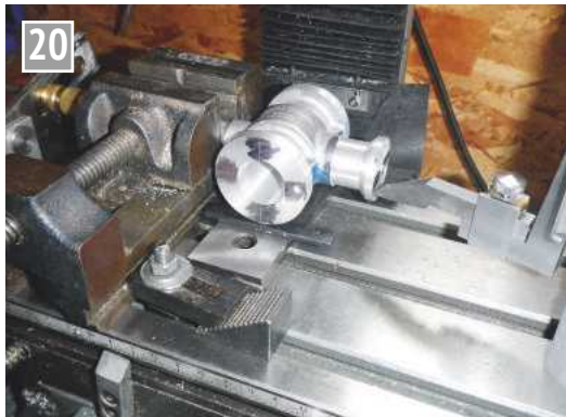
Transferring the cylinder centreline to the port flange.
