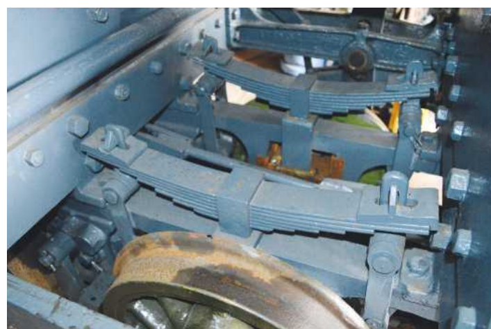
This view shows the upper frame area and suspension associated with the leading coupled wheelset. The bar-framed construction of the chassis is shown to advantage here, as is the arrangement of springing; on the right-hand side (nearest the camera), the fixed anchorage of the leading spring hanger can clearly be seen, whereas on the left-hand side, the bottom of the trailing spring hanger is just visible, connected to its compensating lever.
