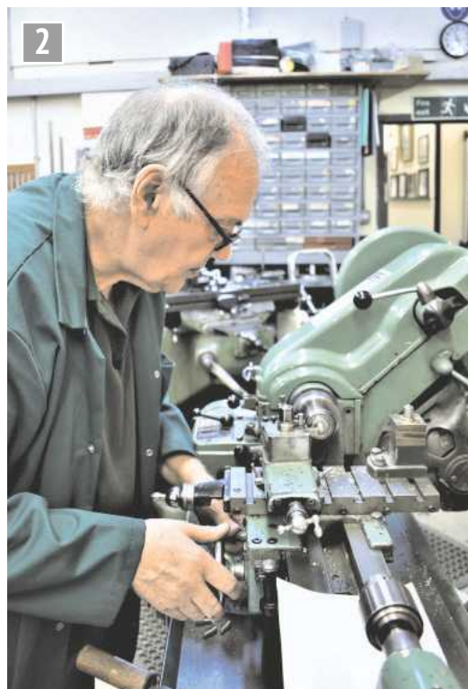
The Myford put to good use, busy making signal pins.
