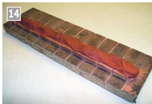
The mould needs to be over filled to ensure the bricks are full.
