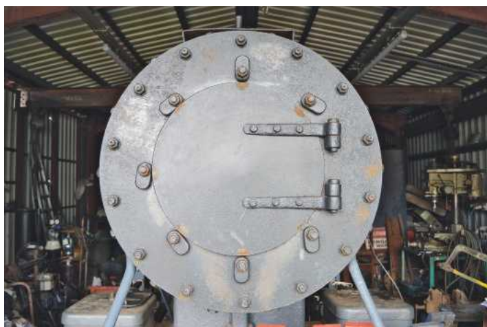
The new smokebox and door are shown head-on in this view, which illustrates well the dog-catch arrangement for securing the door.
