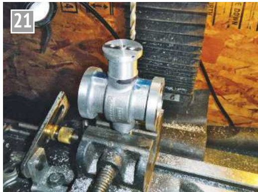
Drilling the steam ports.
