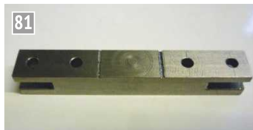
Roughing out two link arms, back to back.
