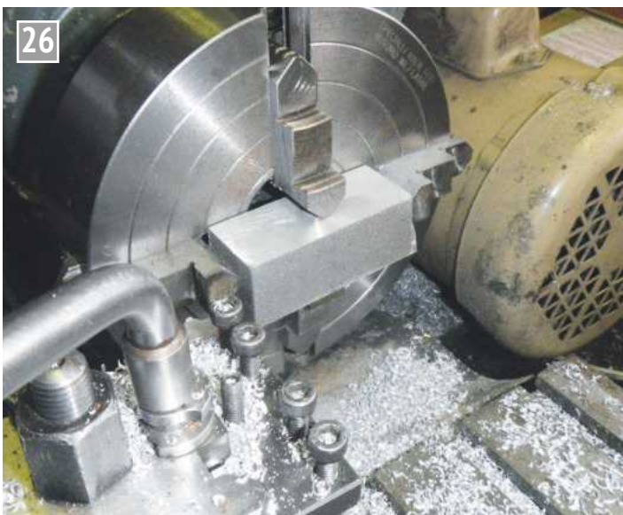
Squaring up the cylinder bearing block.
