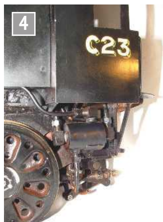
Location of the heat exchanger tank on C23.
