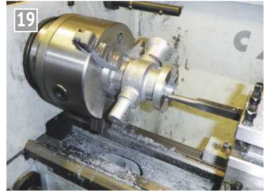
Boring the cylinder.
