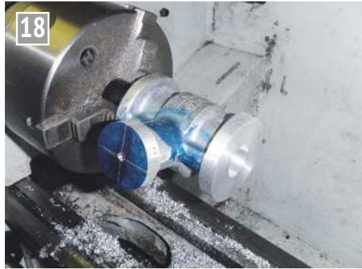
Facing off the other end of the cylinder using an arbor.
