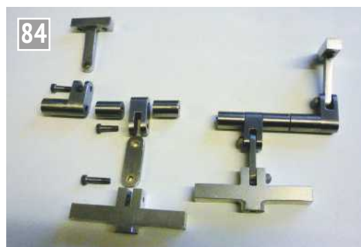
Operating arm assembly, showing the links.
