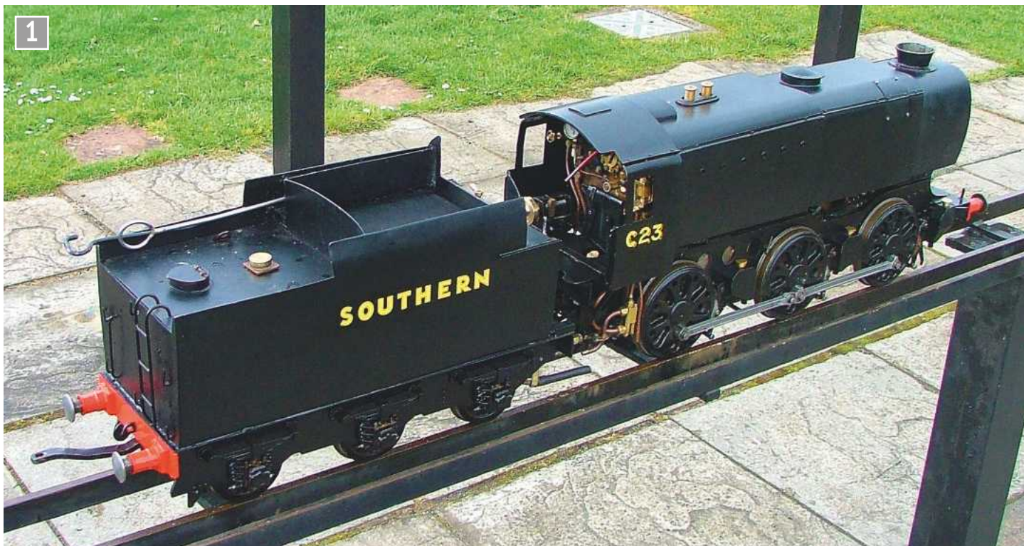
C23 freshly outshopped on the steaming bay at Bournemouth DSME - sight feed glass visible through cab side window.
