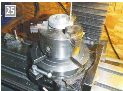
Drilling the fixing holes in the cylinder covers.
