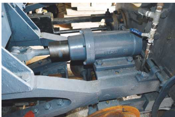
As mentioned in the main text, most of the locomotive's braking and associated linkage components had been removed during its spell of service in India. However, the steam brake cylinder was the exception and restoration of this item proved possible. It is seen here, anchored to the mainframes immediately ahead of the leading boiler support plate, with its piston rod centre left of the picture.
