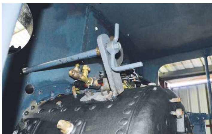
LEFT: The tank supports are bolted to the boiler in the manner shown here. RIGHT: This is a detail much of which is not normally visible on the Baldwin 10-12-D locomotives as shown in working condition. The handbrake is actuated by means of a mechanism consisting of a horizontal screw and a vertical lever, which has had to be completely renewed during the restoration work.
