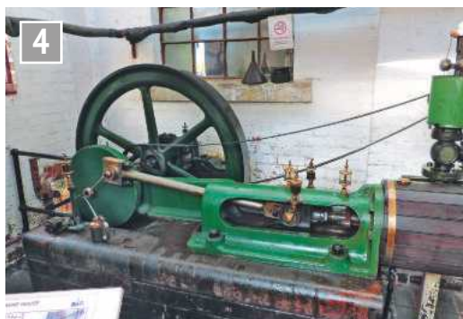
Small steam engine at Clay Mills Pumping Station (with an amazing array of lubricators!).
