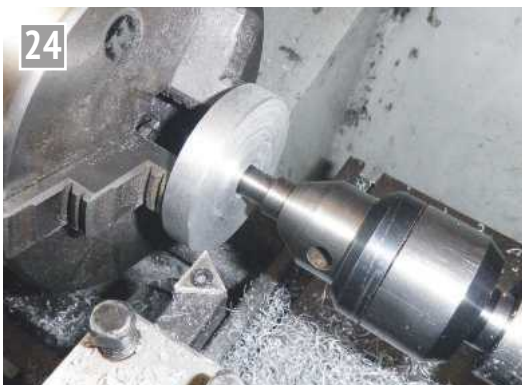
Turning the bottom cover to the finished diameter.
