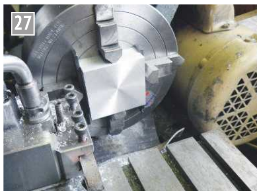
Machining both bearing halves to the finished width.
