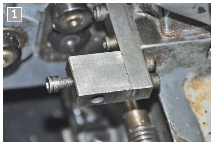
Depth stop installed on the lathe.
