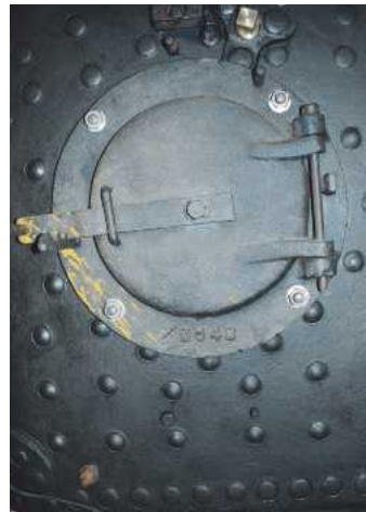
LEFT: The firehole door and its seating are both castings, as is readily apparent here. A washout plug can also be seen centre-right uppermost in this illustration.
