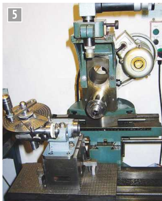
Machining small, accurate components such as watch size pinions requires a set-up or machine with substantial rigidity and with means of accurate centring and indexing such as this Swiss machine (originally for patterning using a high speed diamond). The milling spindle is 55mm in diameter.
