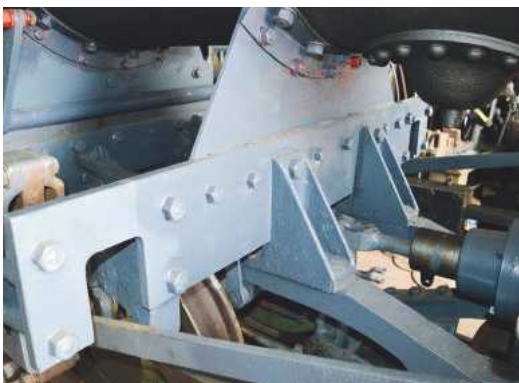
LEFT: A close-up view of the leading boiler support plate, again emphasizing the extensive reliance upon bolts rather than rivets during construction. Note the apertures for the valve rods and the fulcrum (just visible) for the steam brake linkage lever.
