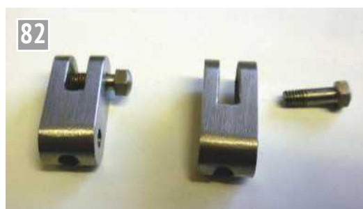
A pair of completed link arms.
