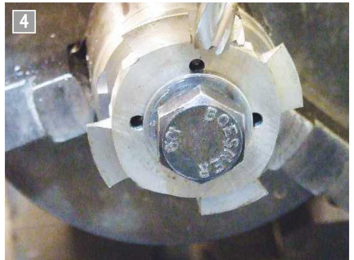
Gashing the cutter to form the teeth.
