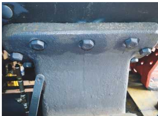
LEFT: A close-up view of the leading boiler support plate, again emphasizing the extensive reliance upon bolts rather than rivets during construction. Note the apertures for the valve rods and the fulcrum (just visible) for the steam brake linkage lever.
