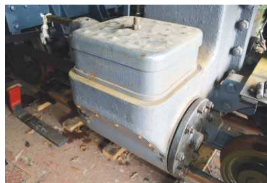
LEFT: This is the flange for the main steam pipe in close-up. RIGHT: A close-up view of the Baldwin locomotive's right-hand cylinder, once again showing the typically U.S.-pattern outline of this component. In the background can be seen part of the flange that facilitates the connection of both halves of the cylinder/smokebox saddle assembly.
