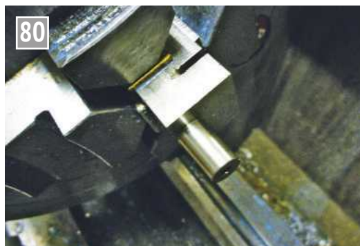
Turning the pin on the valve operating arm.
