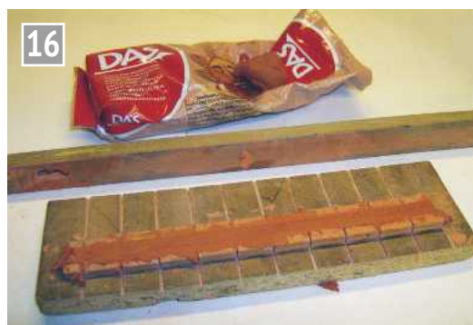
Smooth the upper side of the bricks with a piece of wood.
