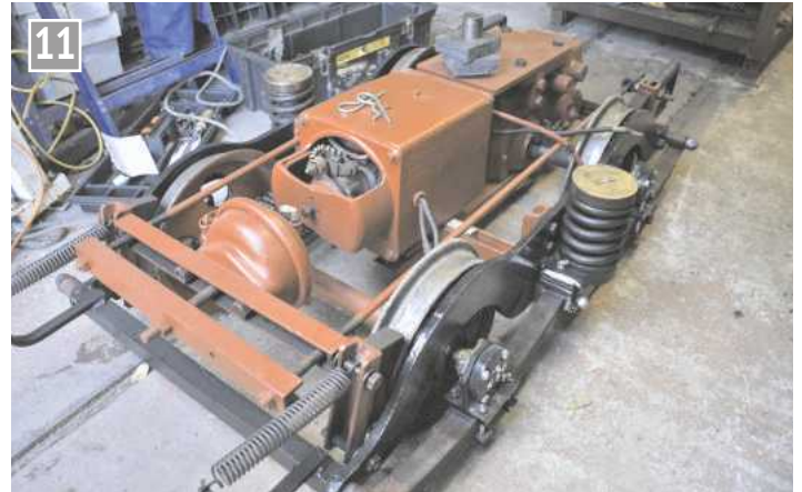
One of the tram bogies with Bostock & Bramley gearboxes ready for installation onto the tram.
