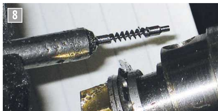
Thread type milling on the Myford of an endless screw, without tailstock support (peeling), is a very satisfying process once set up for the correct thread angle and depth. Pivots are cut at the same setting for maintaining truth. Easy to make some spares at the same settings from roughed out blanks.
