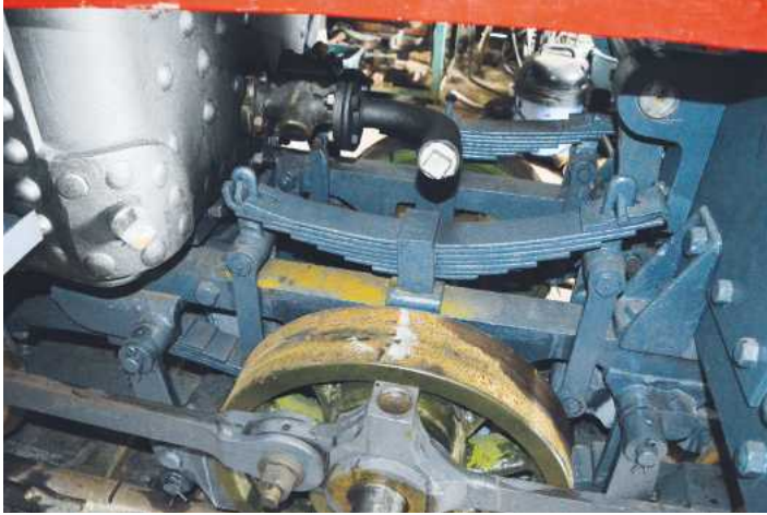
LEFT: The driving wheelset is flangeless, as can be seen here. Further detail of the bar framing is also evident, as is the fact that the springs and hangers associated with this wheelset effectively form a 'bridge' between their adjacent pairs of compensating levers. The rear wheelset has two pairs of leaf springs, each pair linked by beams centred over the axlebox. A portion of the leading right hand spring can also be seen in this view. Other details illustrated here include the brake hangers and the big-end crankpin with the return crank for the Walschaert's valve gear yet to be fitted.
