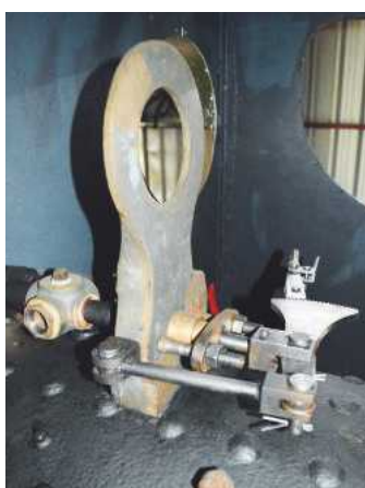
LEFT: The tank supports are bolted to the boiler in the manner shown here. RIGHT: This is a detail much of which is not normally visible on the Baldwin 10-12-D locomotives as shown in working condition. The handbrake is actuated by means of a mechanism consisting of a horizontal screw and a vertical lever, which has had to be completely renewed during the restoration work.
