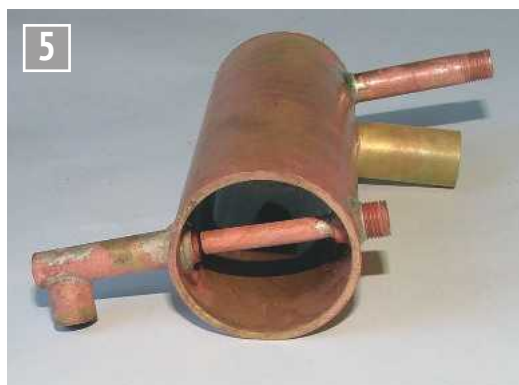
The copper oil reservoir for C23 under construction.
