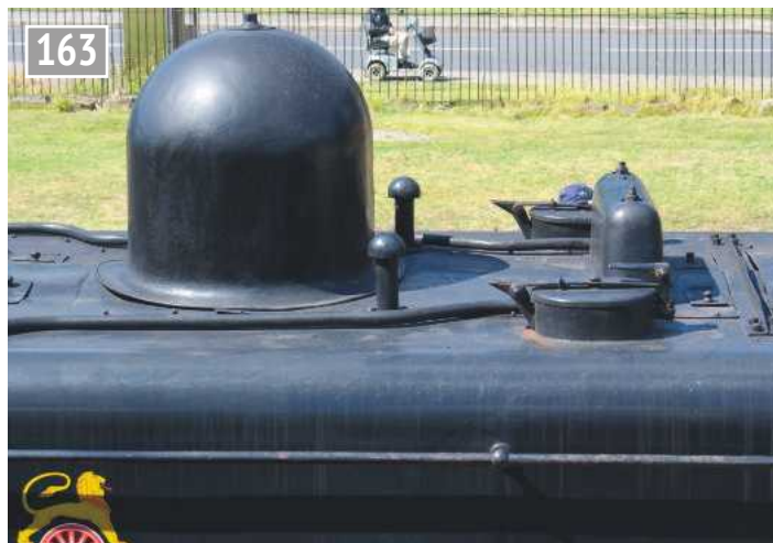
Outer dome – badly fitted on full-size locomotive!
