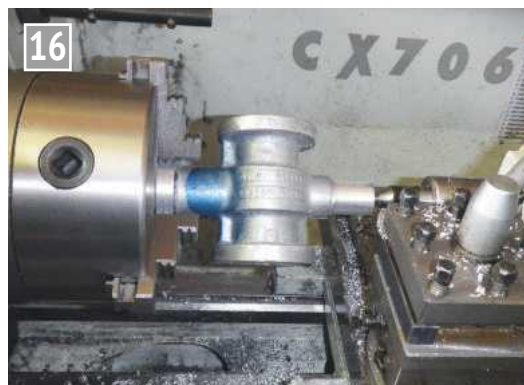
Machining the spigot end of the oscillating cylinder.
