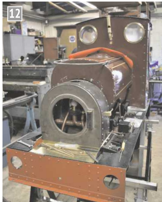
The re-built Hunslet tank locomotive under construction.
