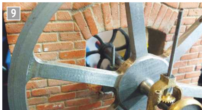
Arch, made using brick slips.
