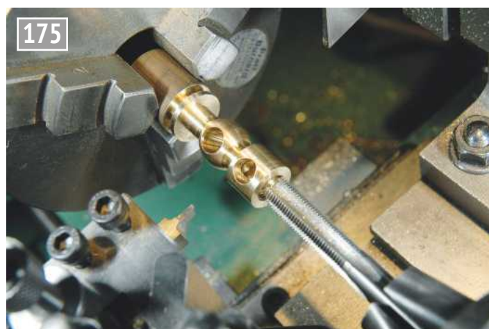
Tapping the throttle joint.
