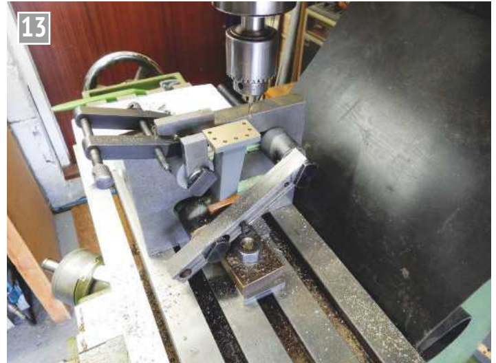
Set-up for flycutting the bottom of a standard.
