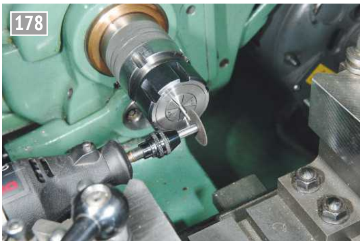
Splitting the throttle shaft.
