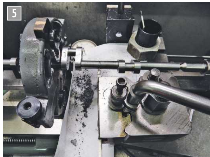
Final machining of the crankshaft.
