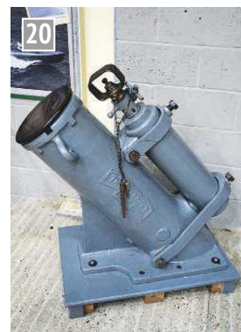
First making steam launch engines, Thornycroft moved into other branches of naval engineering. They made over 3000 of these depth charge throwers during the First World War.
