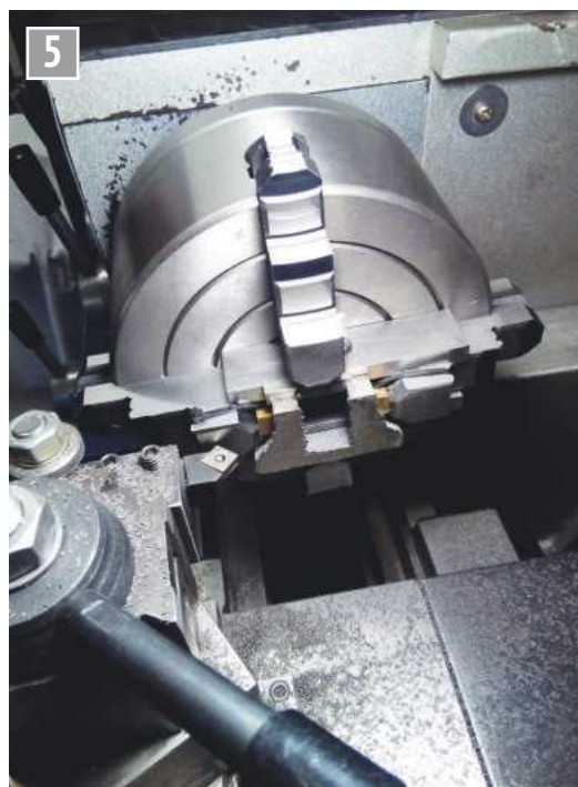
Facing the backs of the bogie pedestals.
