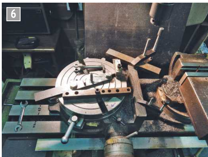
Milling the ends of the connecting rods.
