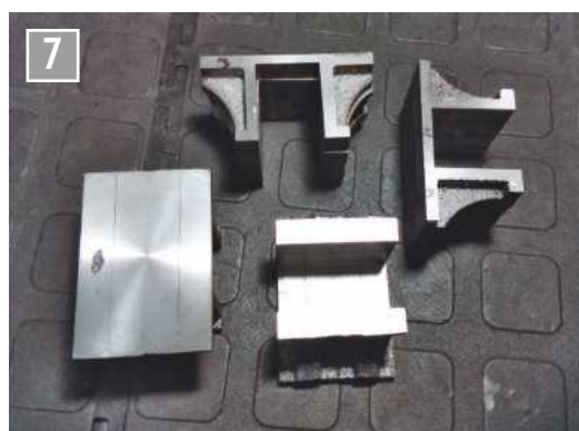
Completed bogie pedestals.
