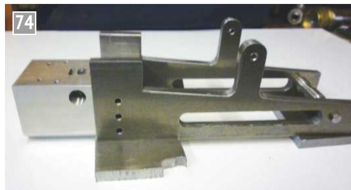
Matching the frames up to the cylinder.
