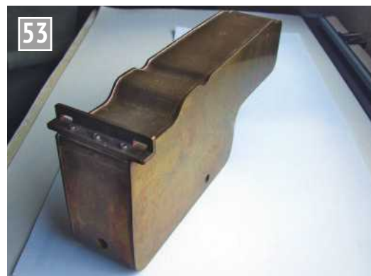
This is the rear view of the forward well tank showing the holes for the \frac{1}{4} inch pipe connections and the vent hole towards the front at the top. The bracket at the rear engages with the tabs on the light stretcher over the driving axle.
