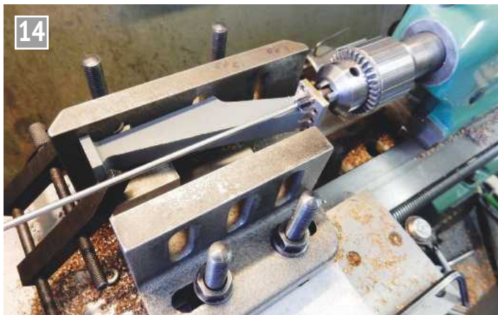
Long spot face cutter for reaching the base of the standard.
