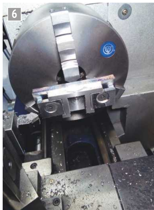
Bogie pedestals clamping jig.
