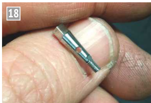
Stainless steel taper spindle.
