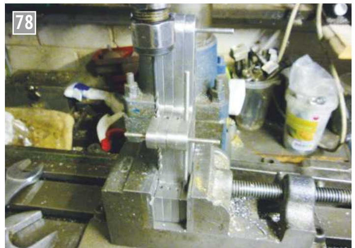
Drilling for the valve guide rods.
