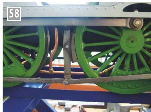
This view is taken from outside the chassis to show the fettled union block for the vertical feed to the donkey pump. The corners have been filed off the block to give the appearance of the more usual pipe junction.
