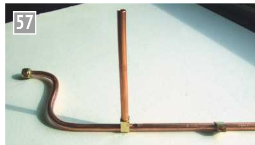
Preparing the main pipe run with the two junction blocks in place. The pipe for the feed up to the donkey pump is ready for soldering but the second one, for the feed to the injector water valve, will not be positioned until the upward bend at the rear has been made.
