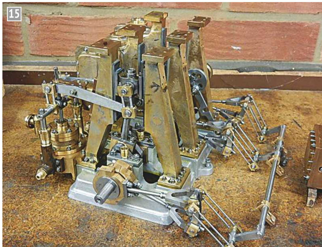
Partly assembled engine showing the crossheads.
