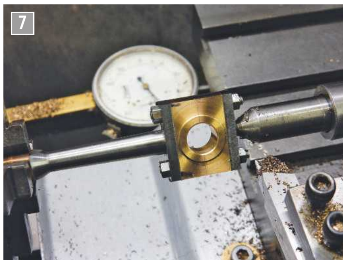
Bearing brasses fitted to the connecting rod.
