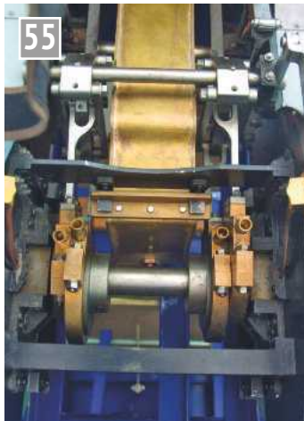
For those unfamiliar with the build of the model, this is the view from above the front well tank showing the way the suspension bracket engages with the tabs on the cross-stretcher but with minimal clearance between the valve gear. The water connection on the rear of the tank can just be seen.
