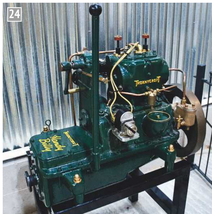
24 Besides vehicles, Thornycroft made smaller portable engines like this 'Handy Billy' much used in small boats during the 1930s.
