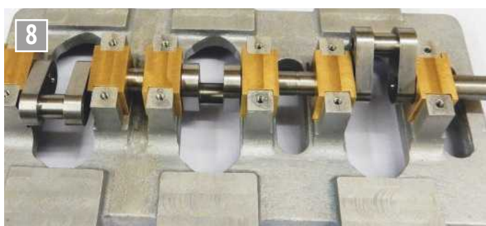
Machined base plate with bearings and crankshaft installed.
