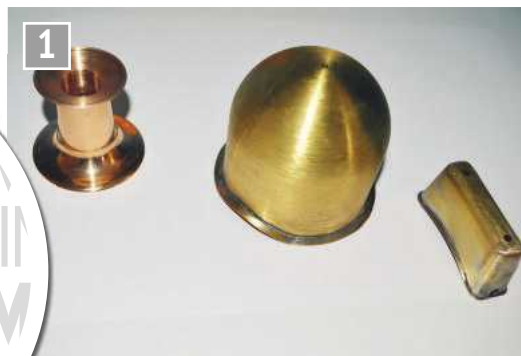
Covers for the safety valve, inner dome and top feed.
