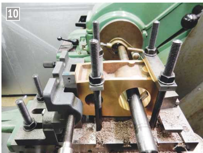
Boring the IP cylinder.
