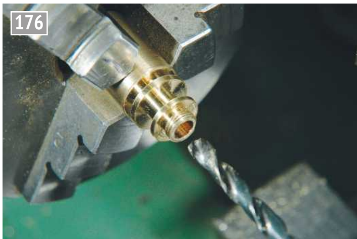
Drilling the throttle extension.
