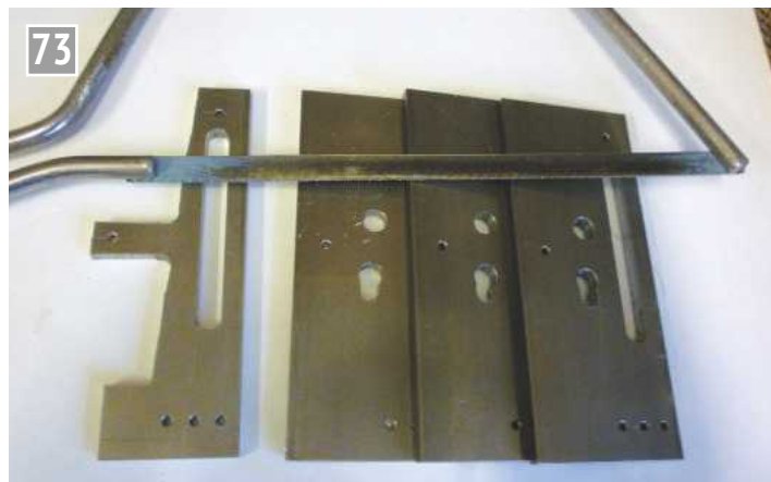
Machine the slot then cut the frame sides to shape.
