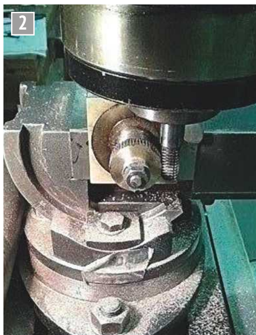
Cutting the reverser wheel.
