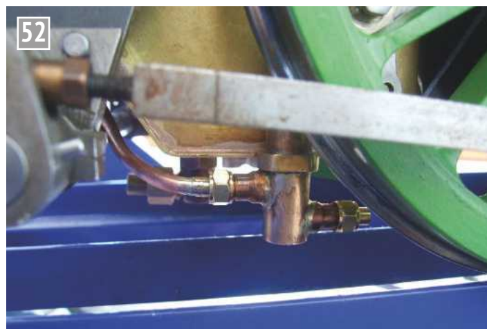
Here the right hand pipe is fitted to the valve again once the tank is down in position.
