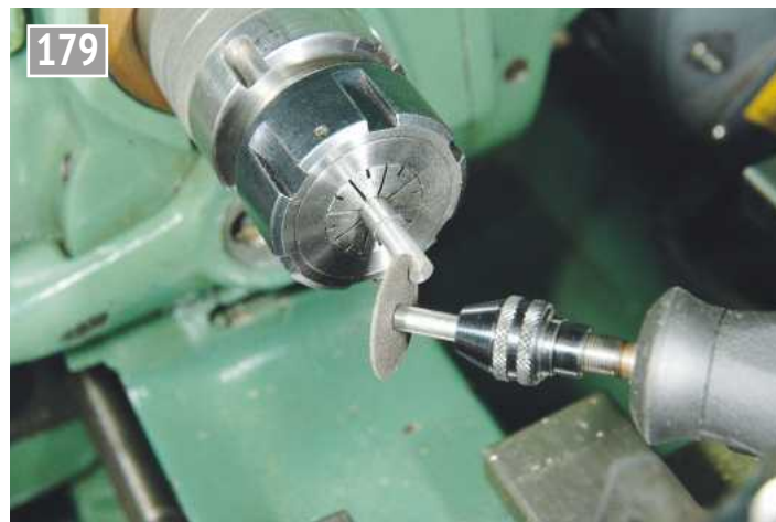
Cutting the butterfly disc.
