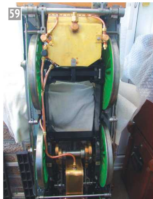
This view from underneath the chassis shows the routing of the pipework described. It is important that the main pipe sits underneath the chassis frame so it does not hamper the fitting of the boiler as the ash pan is alongside the main pipe.
