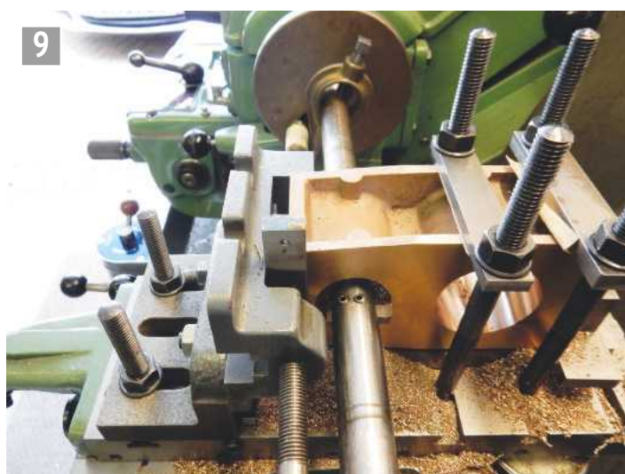
Boring the HP cylinder.
