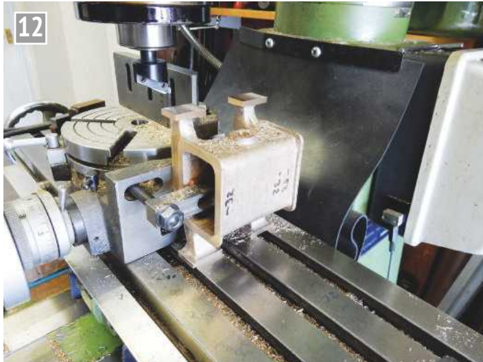
Flycutting the standards integral with the condenser frame.
