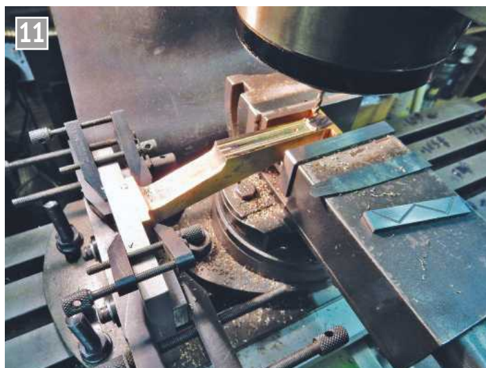
Machining the standard.
