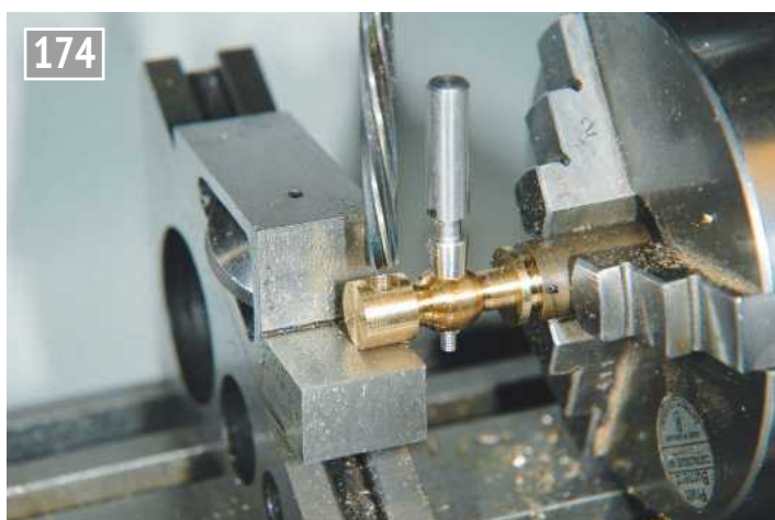
Reaming the throttle shaft hole.
