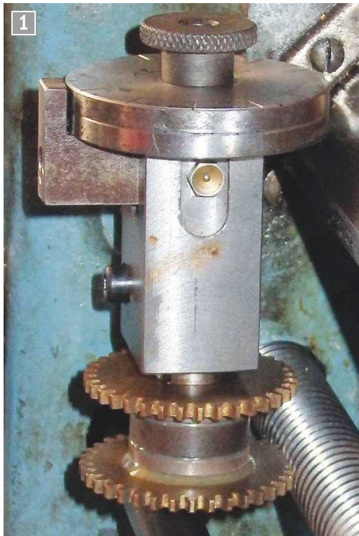
TDI engaged with lead screw.
