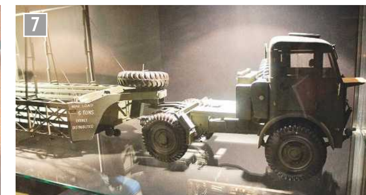
Demonstration model for Taskers patent automatic coupling, much used on semi-trailers like the Queen Mary aircraft transporter.
