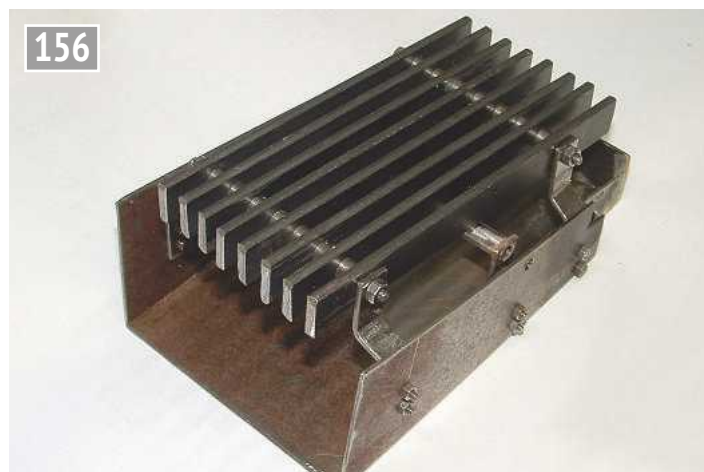
Completed grate and ash pan.
