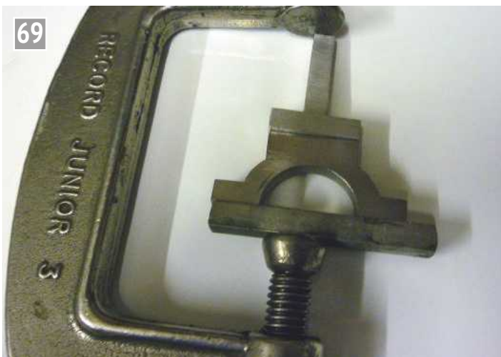
Spotting through for the fixing holes.
