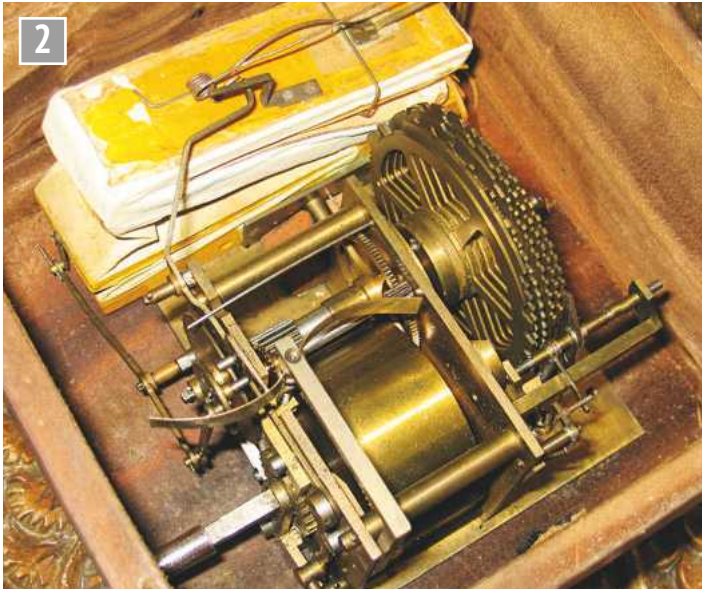
Research is essential prior to design, such as into this nightingale box (in which song cams are selected in a pre-set varied sequence, for teaching a caged bird to sing), and can provide a good guide to many of the proven design principles in a singing bird mechanism. Only by fully understanding the principles is it possible to adapt them to the actual design.
