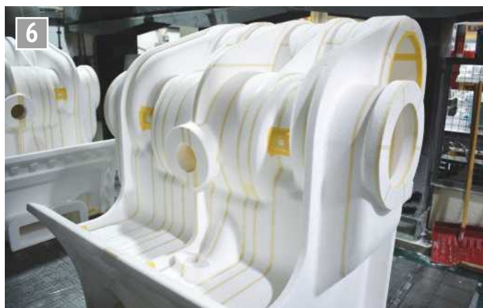
Outside view of the steam inlet from the smokebox and snifting valve boss.
