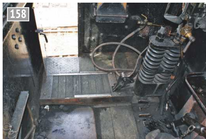
Damper levers (just by the firehole door).
