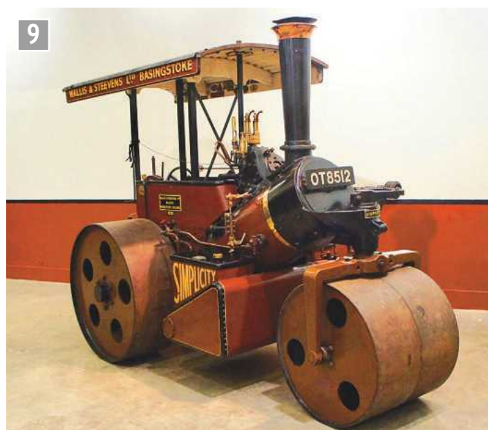
With a sloping boiler the Simplicity roller was a radical attempt by Wallis and Stevens to rethink conventional steam roller designs.
