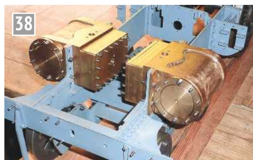
TOP RIGHT: Cylinder patterns and core. RIGHT: The finished Metro tank cylinders.
