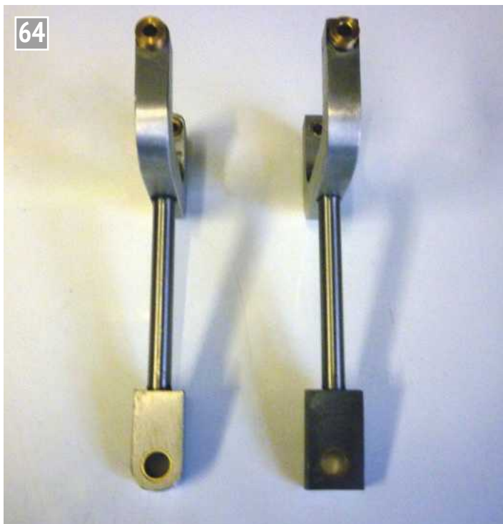
The secondary connecting rod top end – after and before.
