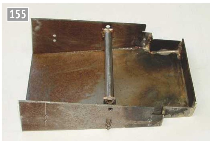
Dump pin tube attached to ash pan.
