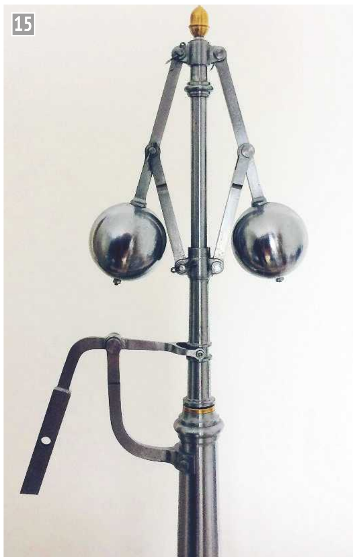
This is a typical Watt governor of the later type as used towards the end of their career in the mid-19th century - in fact this one is now nailed to a Major Beam.
