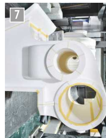
The pattern - photo orientated to show how it would look bolted to the frames.
