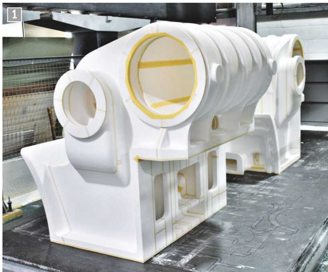
The main cylinder blocks ready to send to the foundry.
