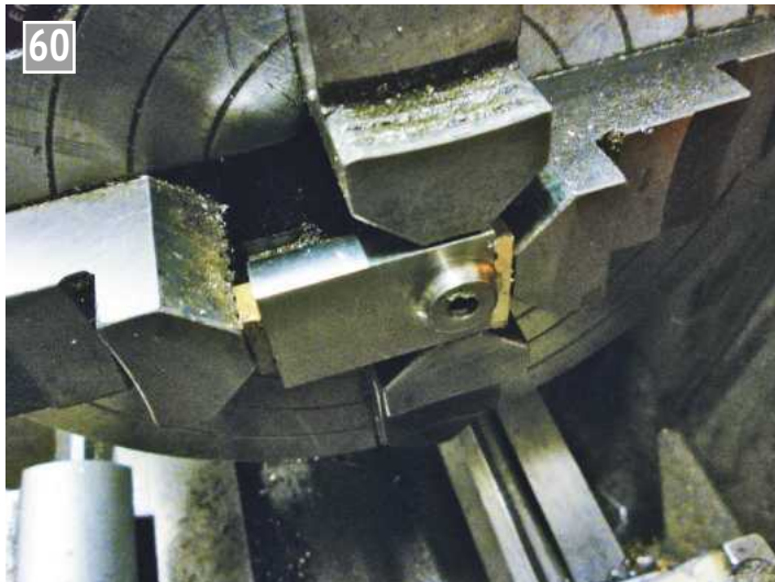
Turning the boss of the crank.
