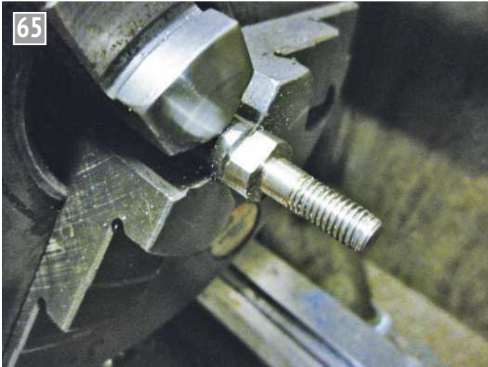
Putting the flats on the crank pin.
