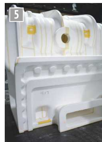
Saddle section with bolt pads and exhaust flange.
