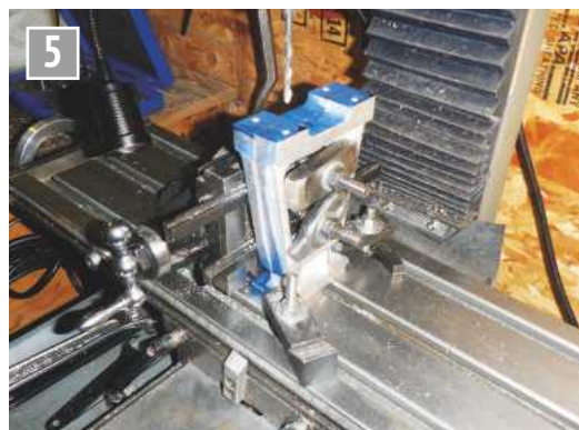
Drilling the fixing holes for the stands.
