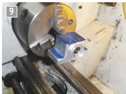
The bearing block mounted on a mandrel for facing off.
