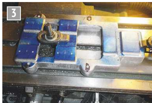
Machining the topside of the base.
