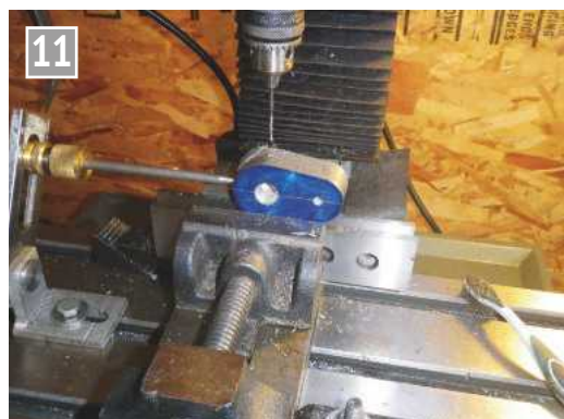
Drilling the holes for pinning the web to the shaft.
