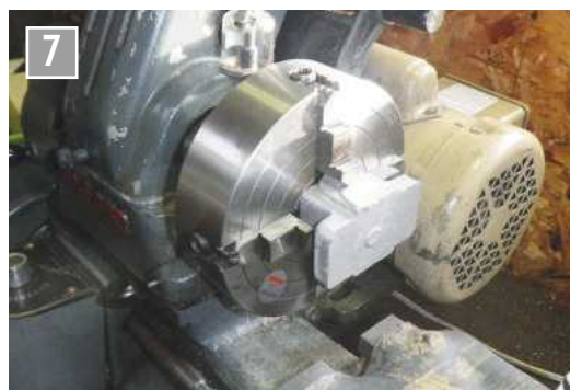
Machining the base of the bearing block.
