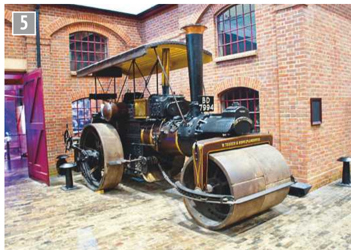
Tasker and Sons Type B steamroller made in 1923 and believed to have been used in Northamptonshire. The firm made their last steam roller in 1926 and that is also in Milestones.
