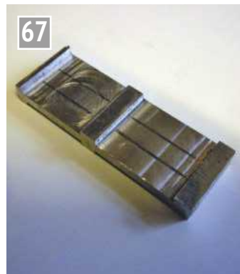
Roughing out for a pair of eccentric strap units.
