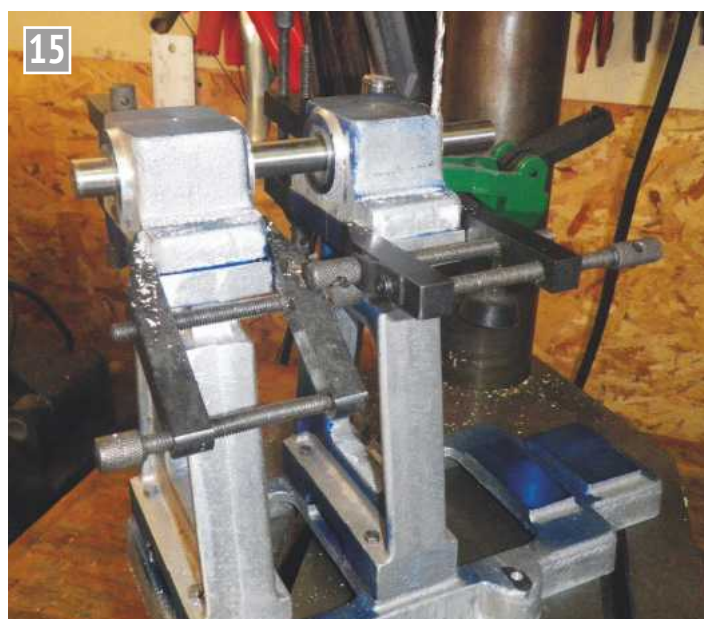
Aligning the shaft before fixing the stands to the base.
