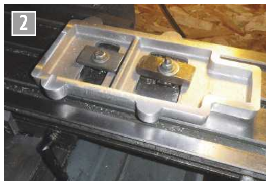
Levelling the underside of the base.
