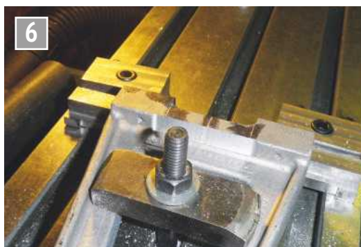
Machining a flat to accommodate the bearing.
