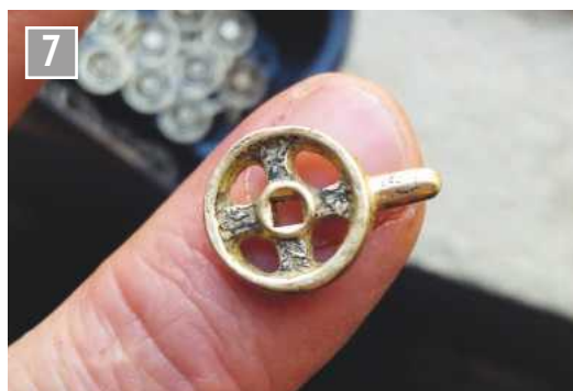
7 Square hole cut with the back end of broken tap.
