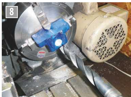
Drilling then boring the bearing block.
