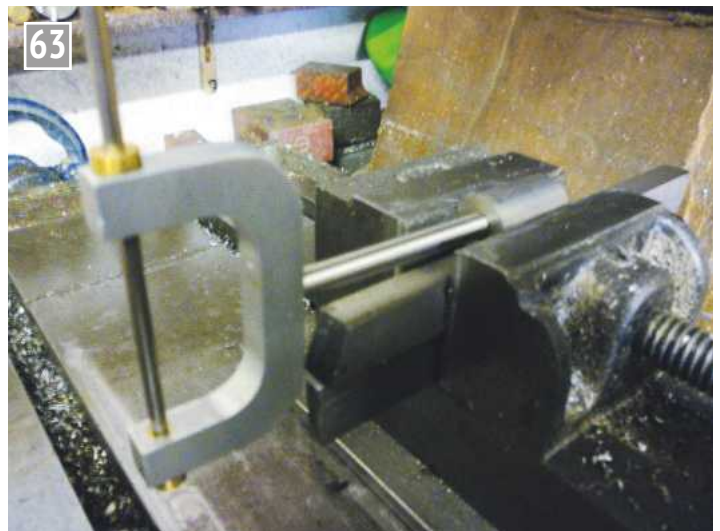
Squaring up before machining the top end.
