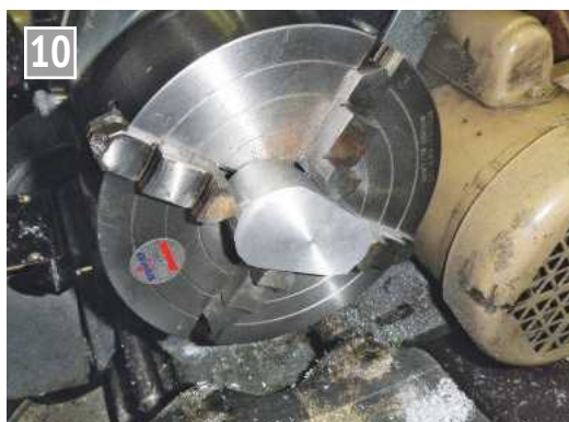
Machining one face of the crank web.
