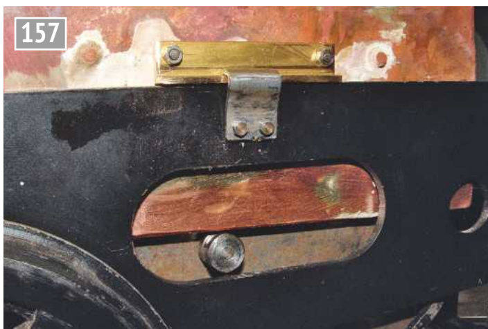
The dump pin is accessible through an aperture in the frame.
