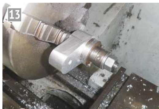
Final finishing of the web.
