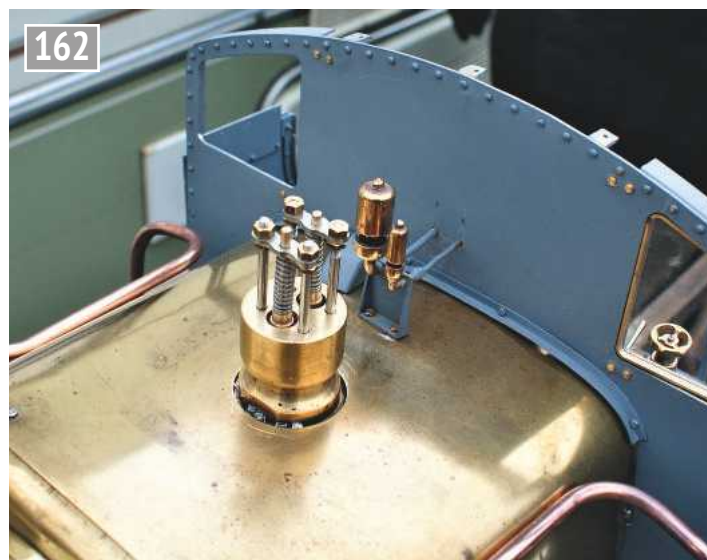
Proper twin GWR safety valve on Frank's pannier.
