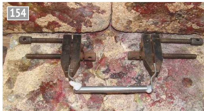
Fabricating the dump pin tube.
