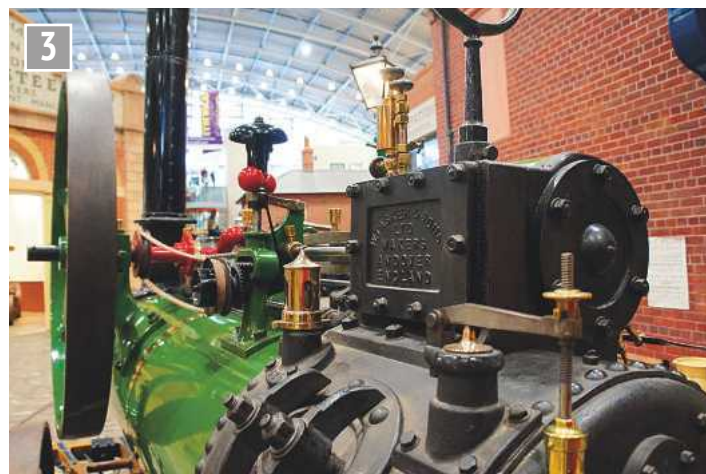
A Tasker portable engine, of a type much used on farms to power threshing machines. Contractors would move these engines from farm to farm.
