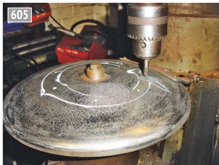
Drilling smokebox door.
