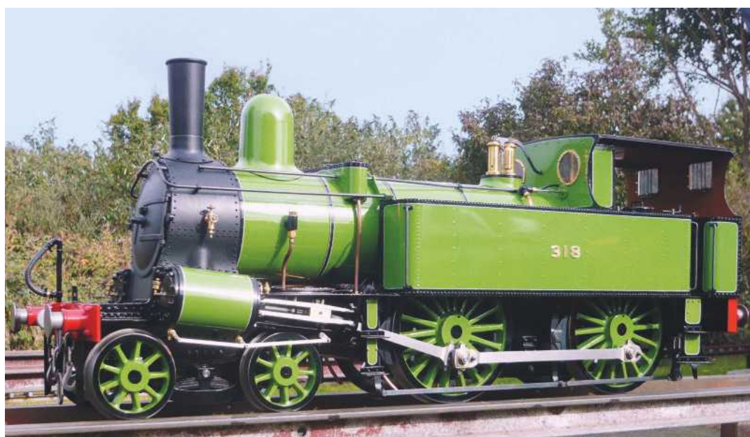
Completed 5 inch gauge LSWR 'Metropolitan' tank locomotive.
