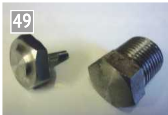
49 Making a bespoke dome screw.
