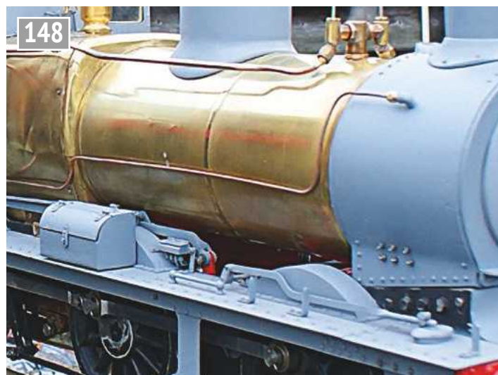
Frank's model showing the sanding gear linkage.
