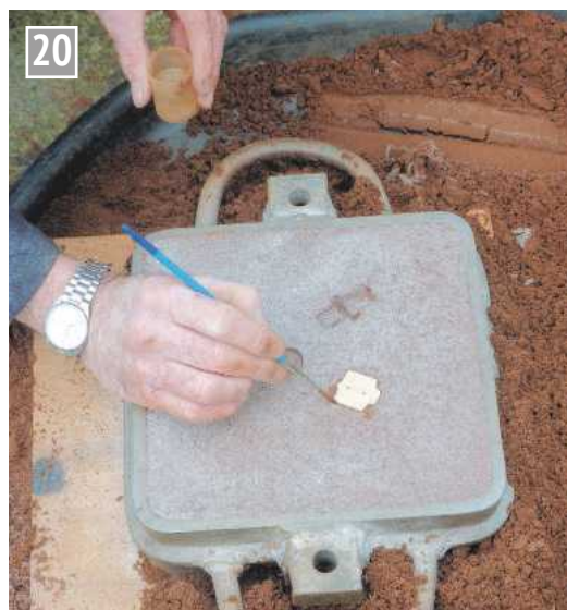
Reinforcing the sand.
