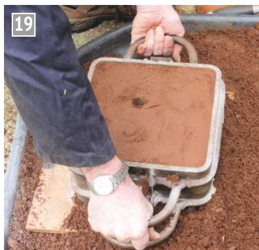
Lift the cope.
