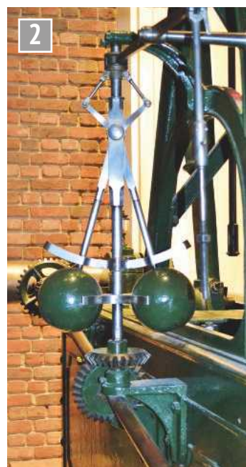
A Watt type governor by Hall and Co. on their Woolf compound beam engine in London's Science Museum. The operating lever is activated at the top of the governor on this example which is of the earlier crossed arm variety.
