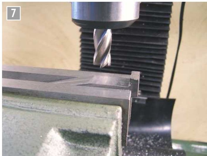
The flat fully machined.
