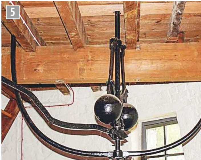
An application predating the Steam Engine: here is a governor in Brixton Windmill.
