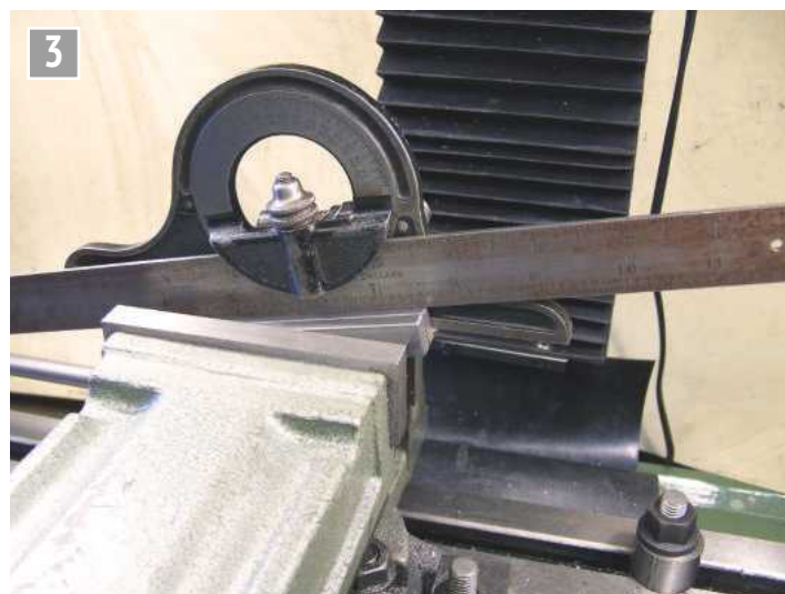
Setting the claws at 12 degrees.
