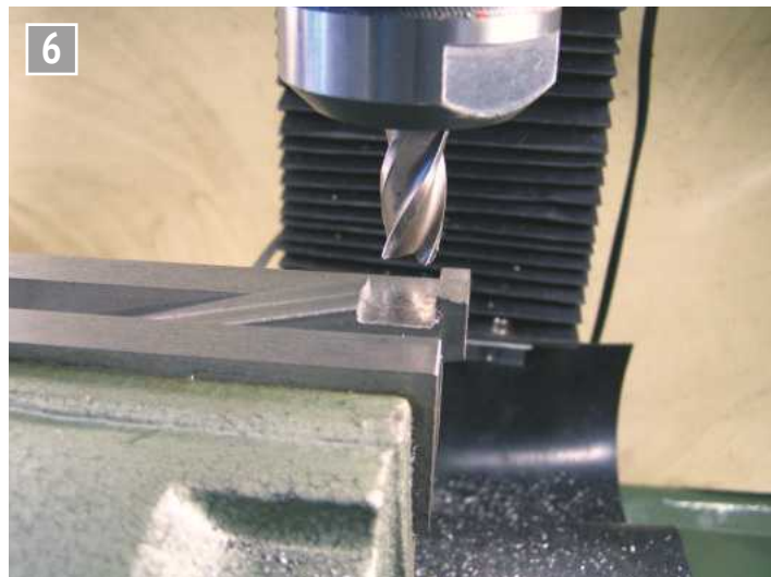
The first slot cut to 5mm depth.
