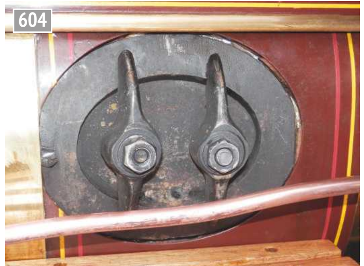
Completed mud hole.
