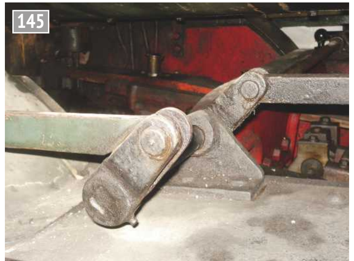
Linkage cross shaft.
