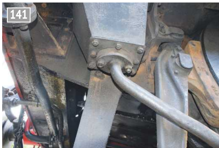
Attachment of sanding pipe.
