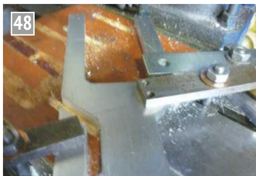
Engine platform profile almost complete.
