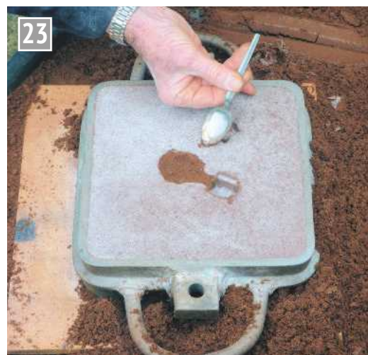
Cutting a gate in the drag.
