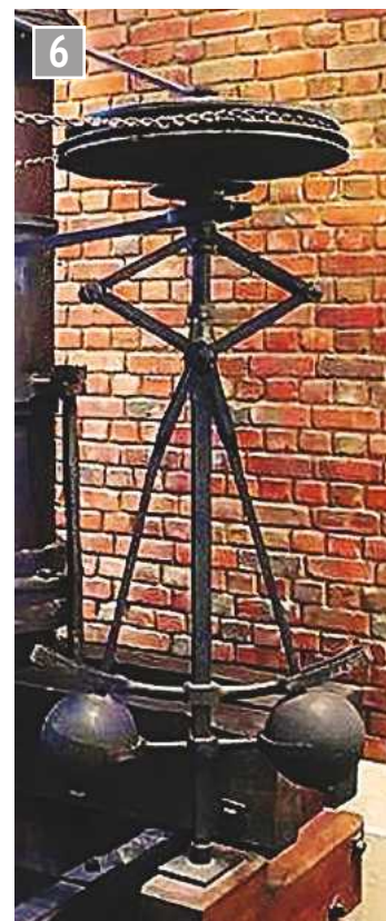
And here it is: the very first governor ever applied to a steam or any other engine, on the Lap Engine of 1788, in London's Science Museum.
