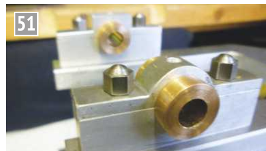
Main bearings in place.
