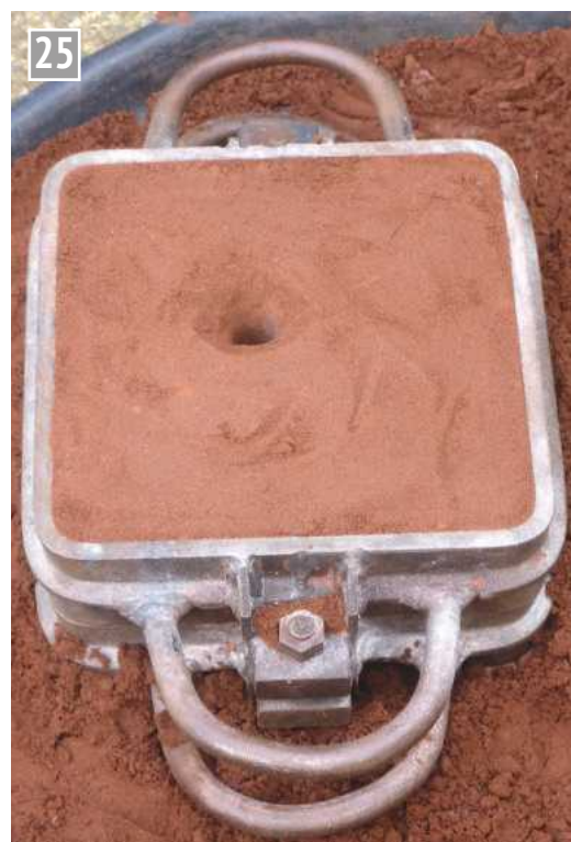
Cutting a gate in the drag.
