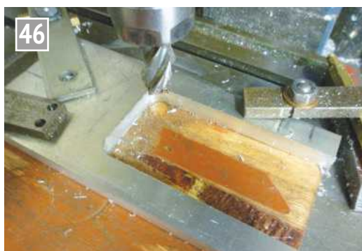
Milling out the engine platform.
