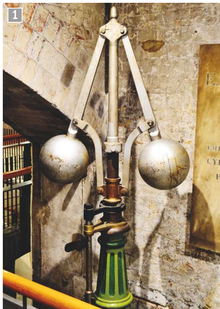
Perhaps the most evocative symbol of the Industrial Revolution, the 'Watt' Governor. This one's history is unknown but thankfully it is now being preserved at Kew.
