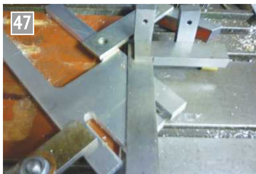
Forming the profile of the engine platform.
