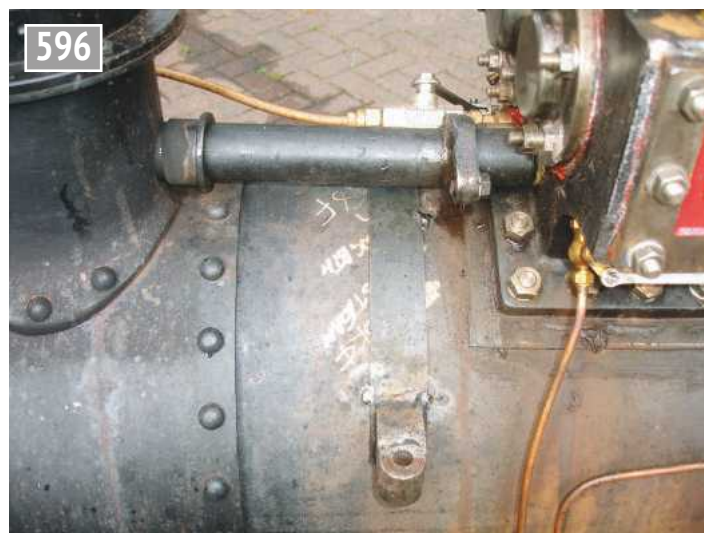
Finished exhaust pipe.
