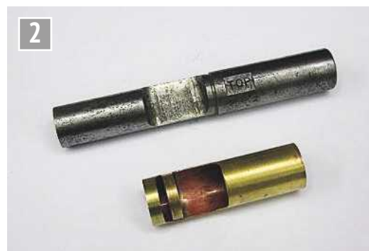
Use a hardened jig to make it easy to cut out the voice slot.
