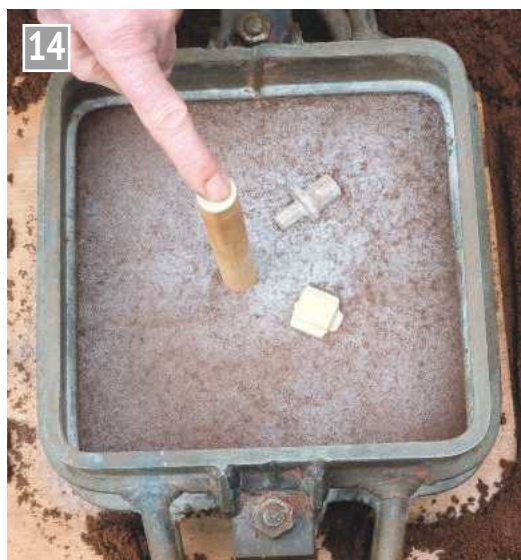
Position the cope and sprue stick.
