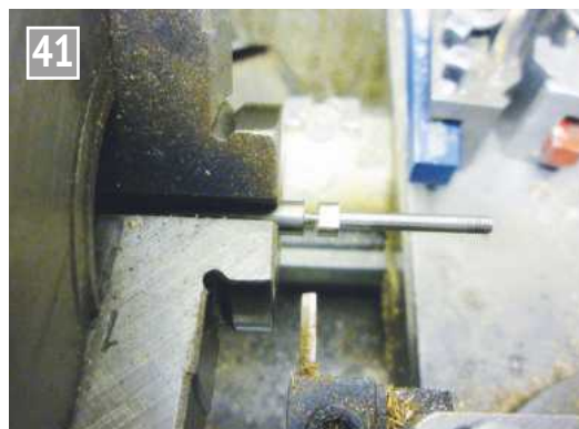
Parting off after filing flats on the pin.
