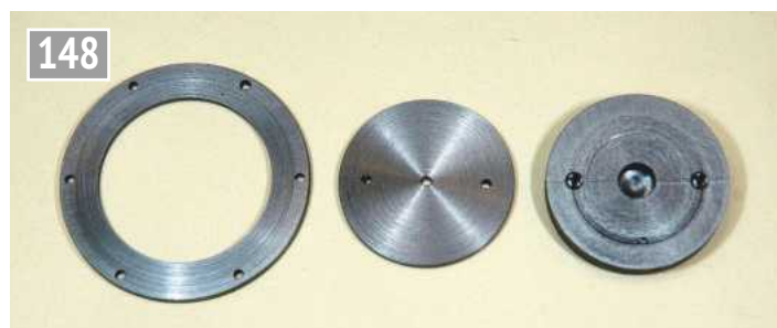
Two templates and cylinder plug.
