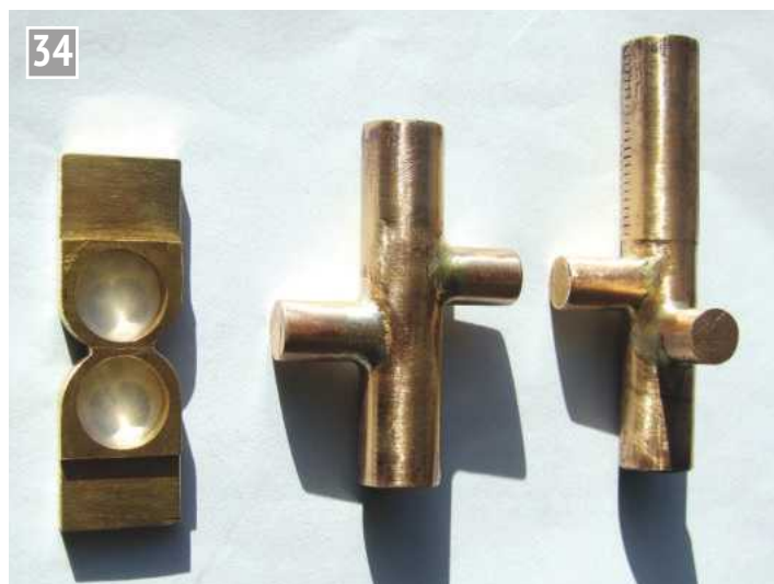
The two fabricated water control valve bodies which have been left long for the machining operations. Also shown is the machined brass plate that will provide the two mounting brackets for the plates.
