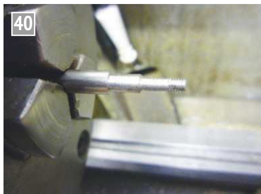
Machining a securing pin.
