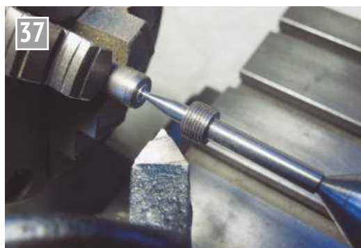
37 Machining the valve stem in stainless steel. The text describes how the task is done in stages and here the valve cone itself is being turned with a sharp pointed tool ready for polishing.
