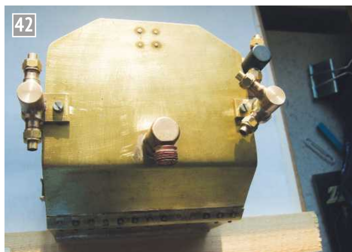
These four pictures show the assembly of the valves on the tank from all four directions to confirm the details. I had to use stainless cheese head screws temporarily for the assembly!
