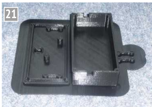
3D printed DC-DC converter box on its 'raft'.
