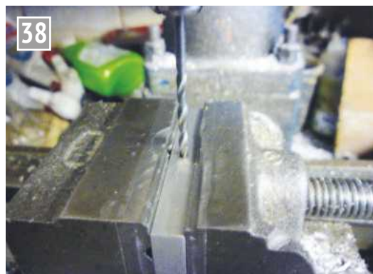
Drilling for the connecting rod.
