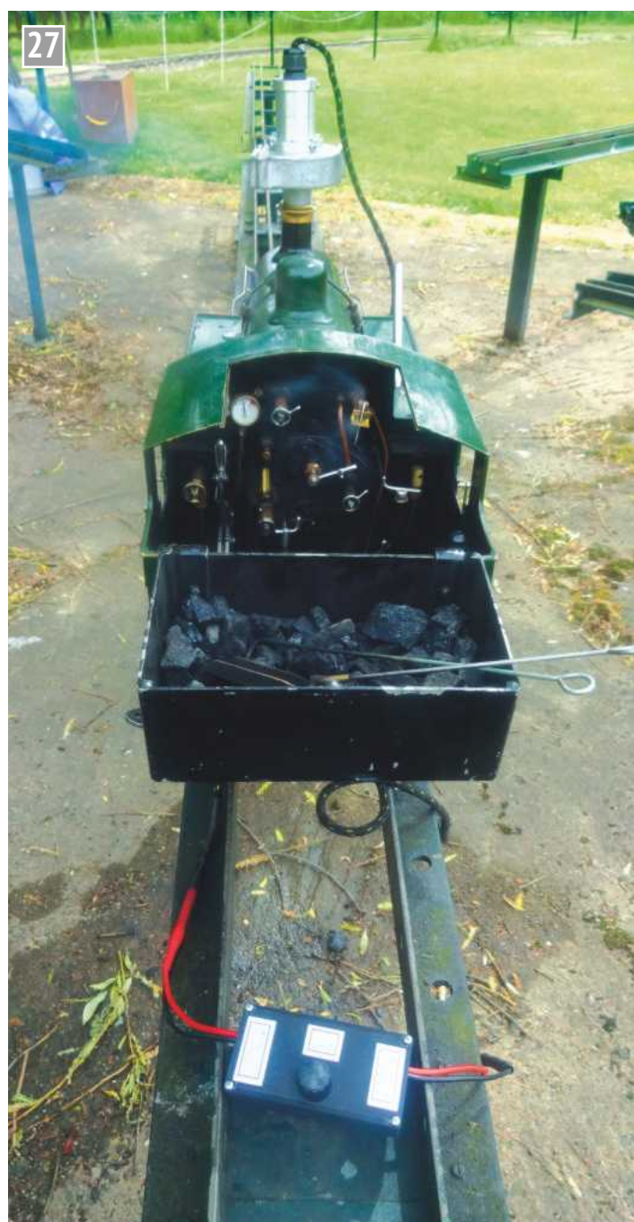
Blower control system in operation at Hereford SME's raised-track steaming bays (using a 24V supply provided at the bay). The locomotive is my 5 inch gauge Super Simplex.
