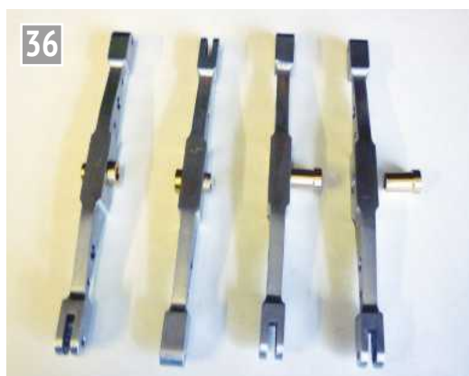
Bushes pressed into the main beams.
