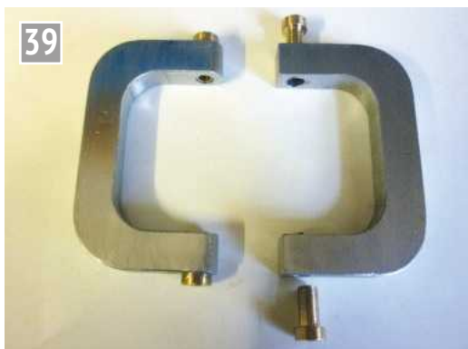
Pressing bushes into the bottom end of the connecting rod.
