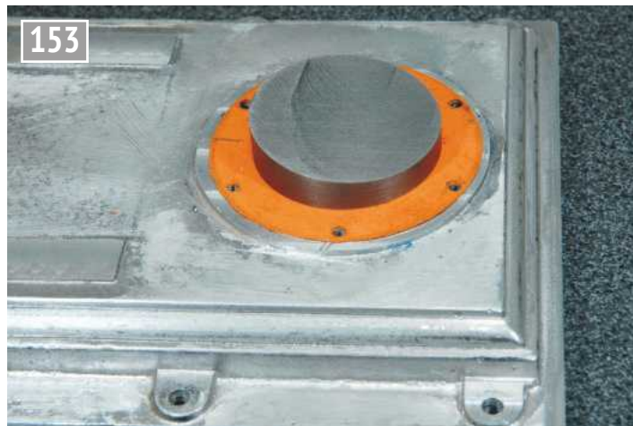
Iron plug bolted down through the gasket.
