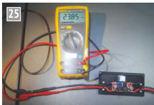
Testing the installed circuit: at maximum voltage.
