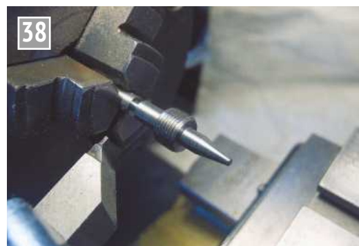
38 After turning the valve spindle round in the chuck, the top section of the stem is being machined for the sealing groove with a fine parting tool.
