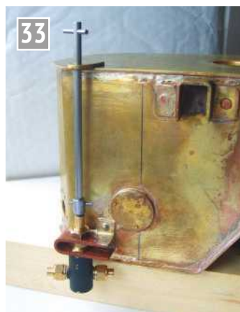
The injector water valve mounted on the left side of the well tank; the fireman's side! The inlet pipe will be fed from the main inter-connecting pipe that goes to the front well tank and the outlet pipe will dive behind the water control valve to the injector to be fitted at the rear.
