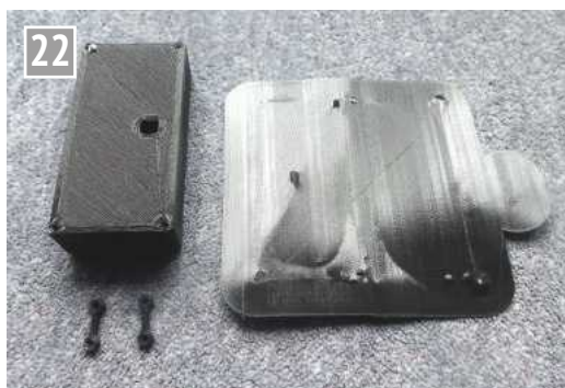
Box, cable-clamps and raft once separated. The raft was very easy to separate from the box and left only a tiny amount of material (see the screw-hole surround on the top left-hand corner), which was then removed by light filing and sanding.
