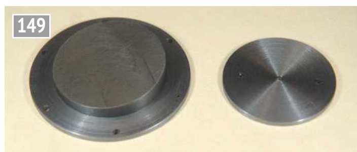
Drilling cylinder mounting template.
