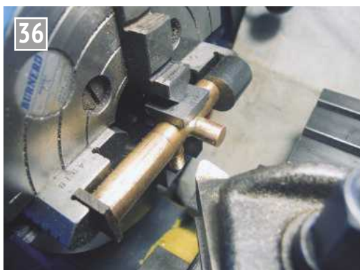
Two views of the valve body fabrications being held in the four jaw chuck to machine the pipe union stubs. The bodies are cast bronze but the stubs are phosphor bronze which gives an excellent thread form.
