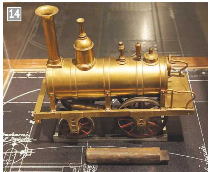
'Poker' engine used to promote Chesterman and Bottom's measuring tools. A red hot iron bar in the firebox generated steam.
