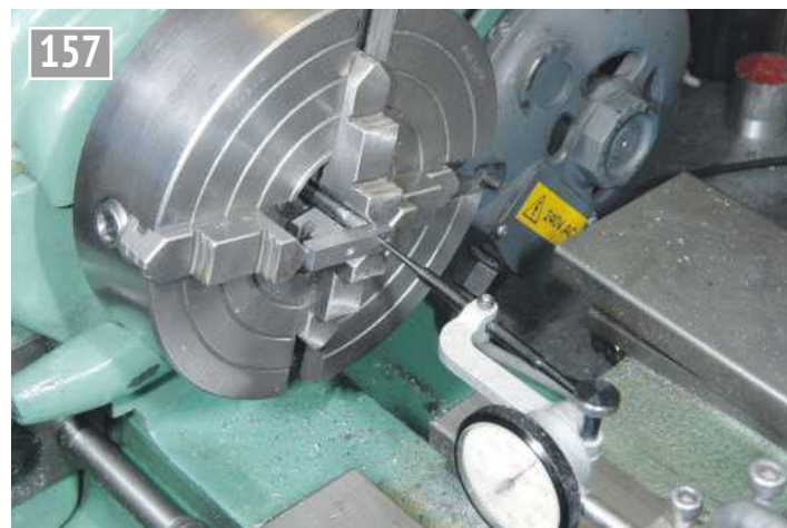
Centring the shaft hole.
