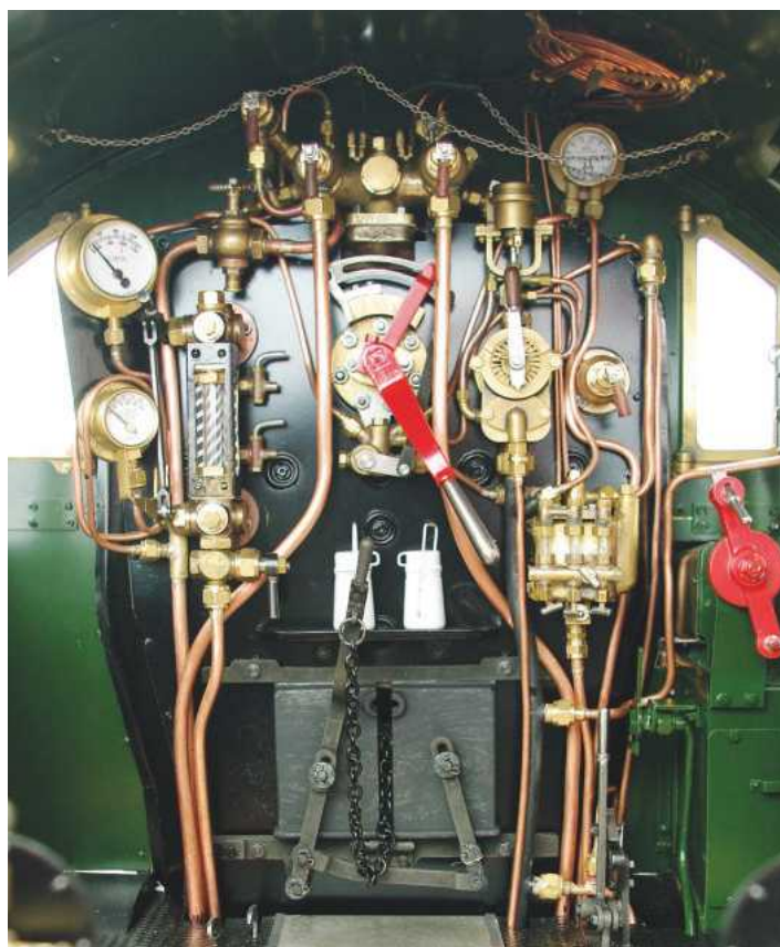
Backhead cropped. The detailed backhead of Pete's 7 1/4 inch gauge Collett Goods.
