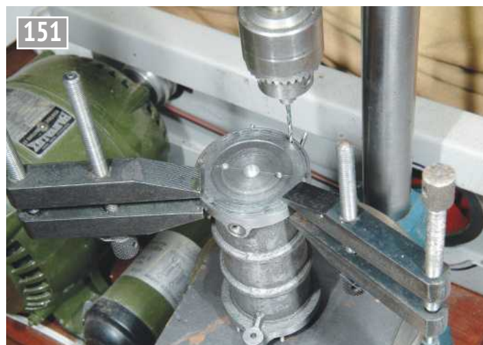
Spotting through 8BA tapping size.
