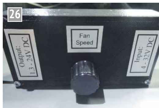
Completed blower fan speed control unit in its 3D printed box.
