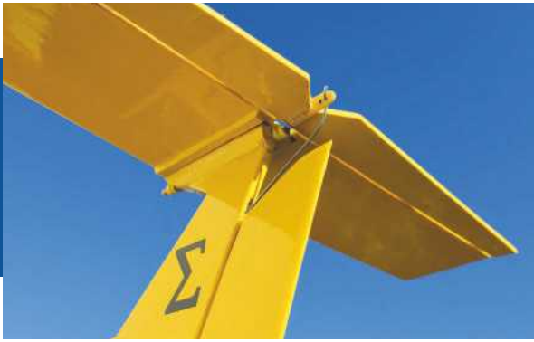
My elevator pushrod and horn set up. The horn was made from thin glass fibre board but 1/16" ply could also be used. I know it looks a little strange, but it works. Take your time so it is bind free.
