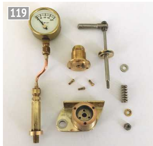
Brake valve component parts with mounting for air pressure gauge, also shown.
