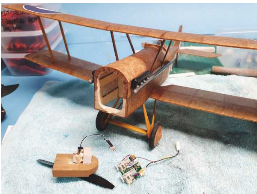
Left: Elevator and rudder separated from the model. Hinged with diskette internal film. Below: Motor fitted to nose block and Rx brick ready for fitting.
