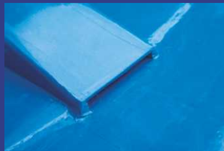
Leave the slot open at the back of the fuselage to let the cooling air escape.
