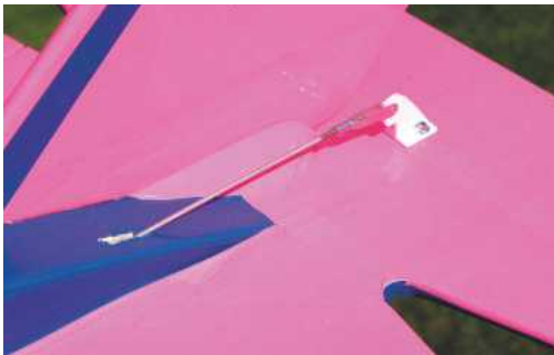
Elevator pushrod has a straight run too.
