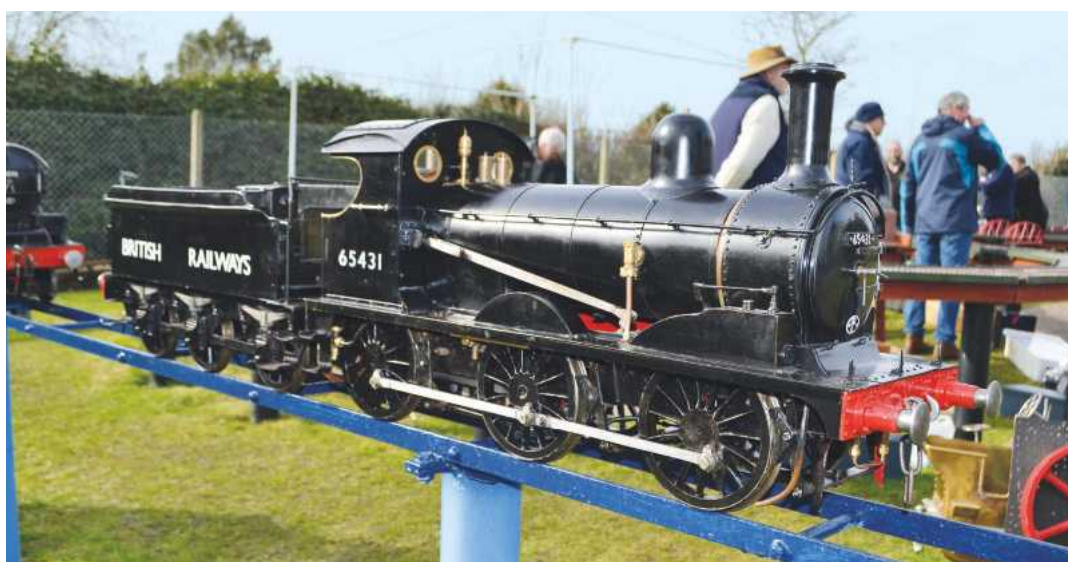
Terry Woodward's 5 inch gauge J15 locomotive, built mainly from photographs, with a chassis based on the Metro tank. This locomotive took 5 years to build.
