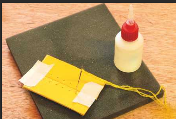
Mock-up surfaces to develop your sewn hinge skills. Use cyano to seal the knots.
