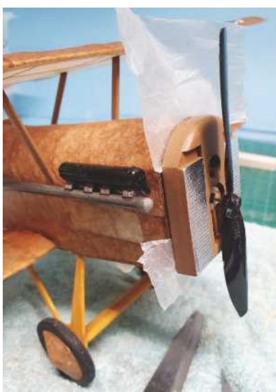
Above: Very popular AR6400 Rx brick positioned on a small shelf. This is a 3-channel unit, with a built-in brushed ESC and two linear servos Left: Polythene sheet keeps the magnets from sticking together when glued in place
