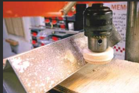
Sanding block set over at an angle to sand a chamfer on the wheel trim blank.
