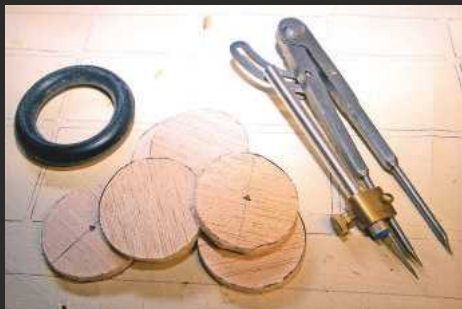
Balsa wheel blanks are scored or cut from sheet with dividers or compasses.
