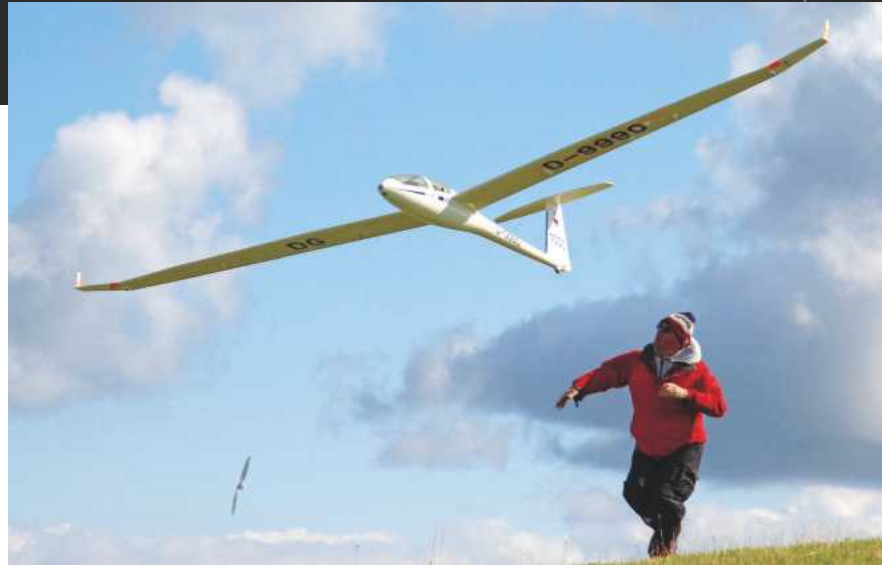
Below: My mighty DG-1000 loses its prop and spinner, which is visibly departing at this moment. The aircraft only just escaped disaster.
