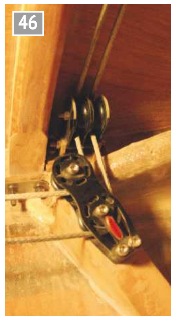
Some tricky routing is needed to get the tiller ropes to the quadrant.
