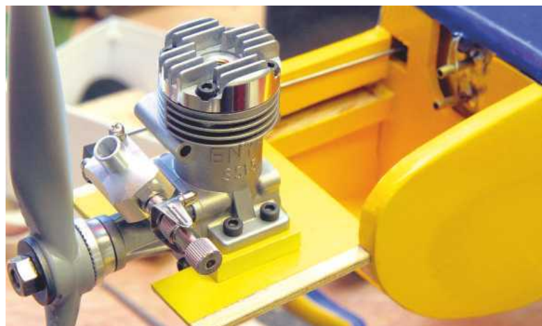
Ply engine plate slides into a tight slot between beech bearers.
