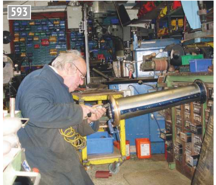
Drilling chimney cap holes.
