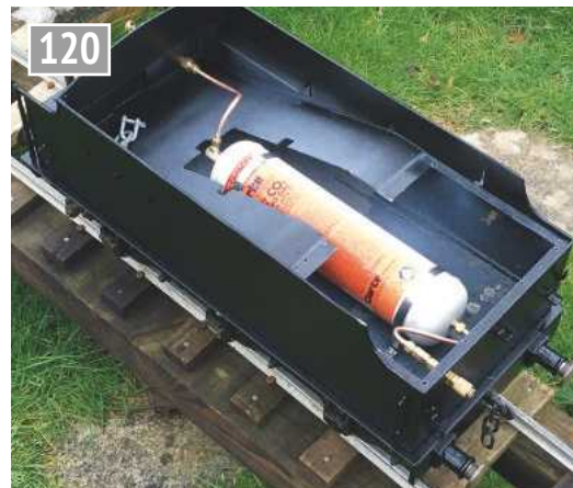
Driving truck with seat removed to show the air reservoir and connection for charging from the workshop compressor. The reservoir is formed from a suitably modified MIG welding CO2 bottle.
