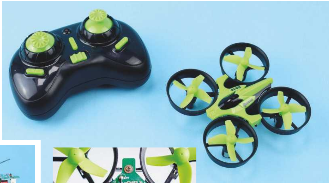
Above: Just one of the many suitable mini drones for a Whoover conversion. I used an inexpensive Eachine Eo10 to great effect. Left: The motors on the Eo10 control board are soldered on so these will need temporarily and carefully removing to install on the Whoover (or Tiny Wing). The ducts and battery box are cut off the frame to be reused.
