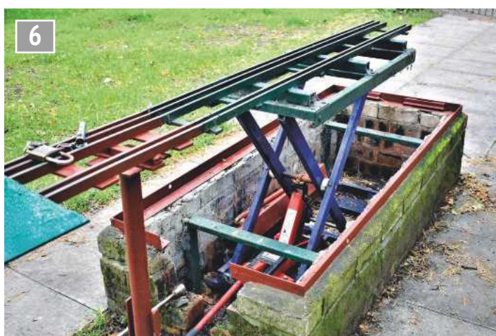
The lift table ready to receive a locomotive.
