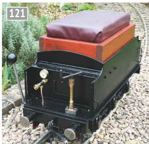
Driving truck showing air reservoir pressure gauge and shut off valve.
