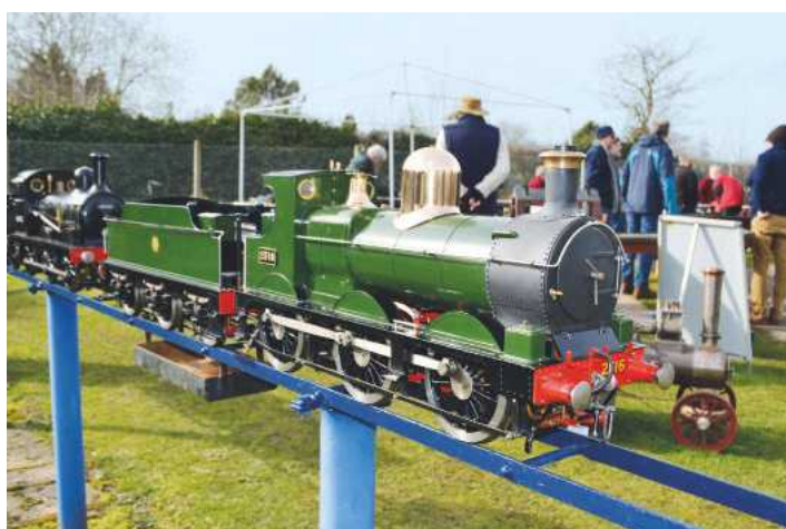
A 5 inch gauge Dean Goods by Dudley Deas. This model was finished 6 months ago, having taken just 2½ years to build, but has not yet been steamed.
