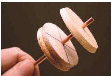
Wheel (left) has a seat for the tyre cut with a rat-tail file, with chamfered wheel trim on right.
