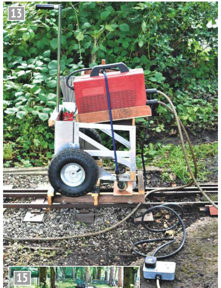
Another useful road/rail generator set.
