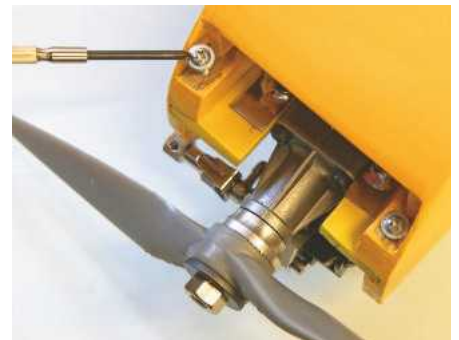
These screws retain the plate in the tight slot, facilitating easy engine swaps.
