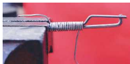
Clevis piano wire matches the servo output arm hole. Keeper is thinner wire.
