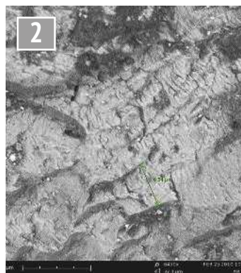
SEM photo of a fatigue fracture surface - the dimension is across two striations. Magnification 6450 times. (Photo taken at Anglia Ruskin University when I worked there.)
