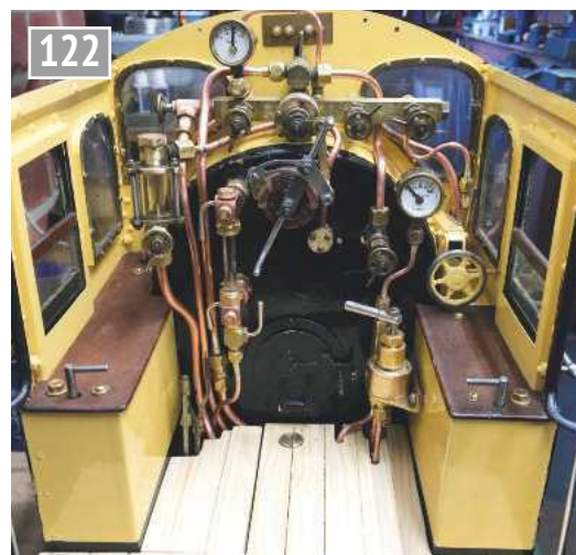
Cab view of No. 1870. Both pressure gauges are faulty and temporary, awaiting replacement.
