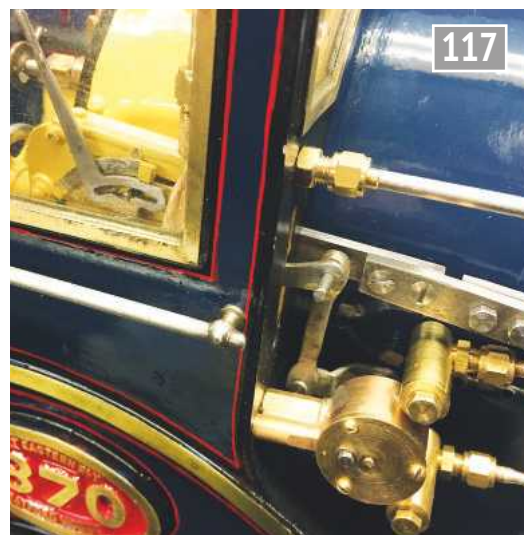
Control valve for power assisted reverser. The valve is operated by the lever on the side of the screw reverser. Both the reverser and lever inside the cab are close to scale but the control valve outside most definitely is not. I anticipate that it will be less obvious when the Westinghouse pump is fitted; although there is provision for a steam supply via the union connection in front of the handrail the pump will be a dummy.
