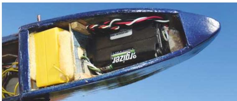
Like the servos this retro receiver is a big lump and it's only two-channel! It was a squeeze to get it in. Using four AA cells the C of G came out spot on. I didn't use a switch, just plugging the battery into the receiver as required.
