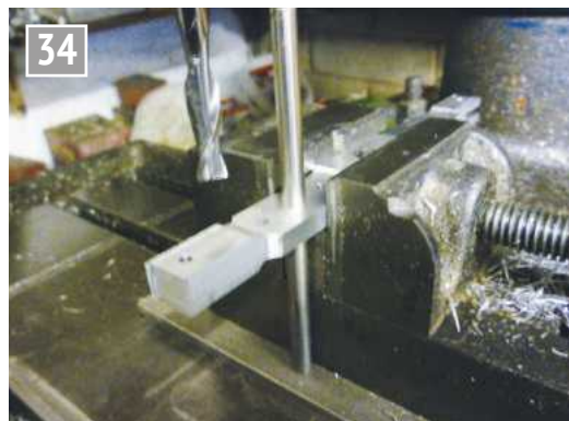
Making a start on the beam profile.
