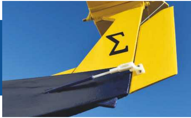
Traditional tube in tube set up for the rudder. When modifying for an elevator the rudder area needs increasing as shown due to the section that's removed to accommodate the elevator push rod.
