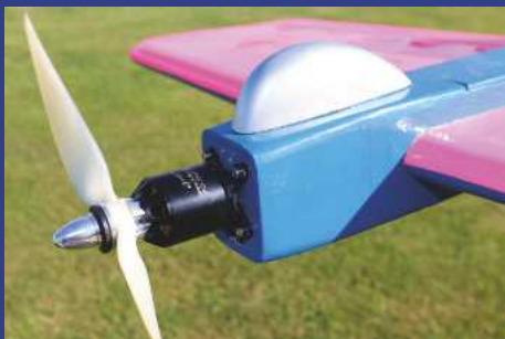
Simple firewall mounted motor suits electric or a .25 glow engine.
