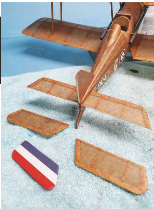
Left: Elevator and rudder separated from the model. Hinged with diskette internal film. Below: Motor fitted to nose block and Rx brick ready for fitting.
