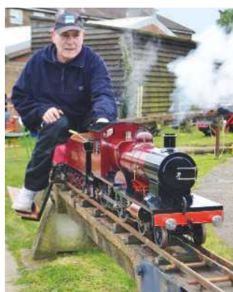
Tom Rose's 5 inch gauge 'Maid of Kent' locomotive. This took 23 years to build, with a lot of redesign along the way. It self-identifies as a Midland compound.
