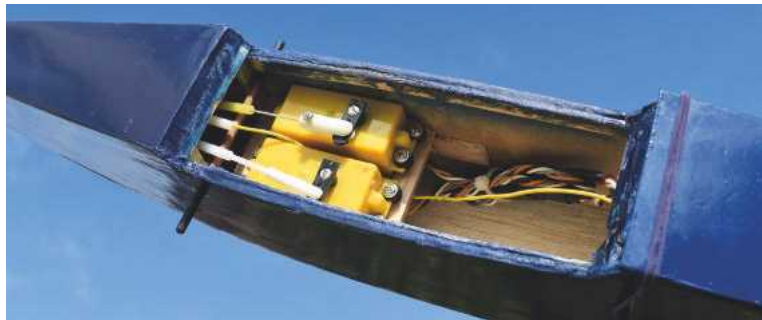
Old school servos are huge in comparison to modern types. For current radio gear 9g servos will be fine, but metal geared examples are worth the small additional cost to survive the rough and tumble when landing on a slope.
