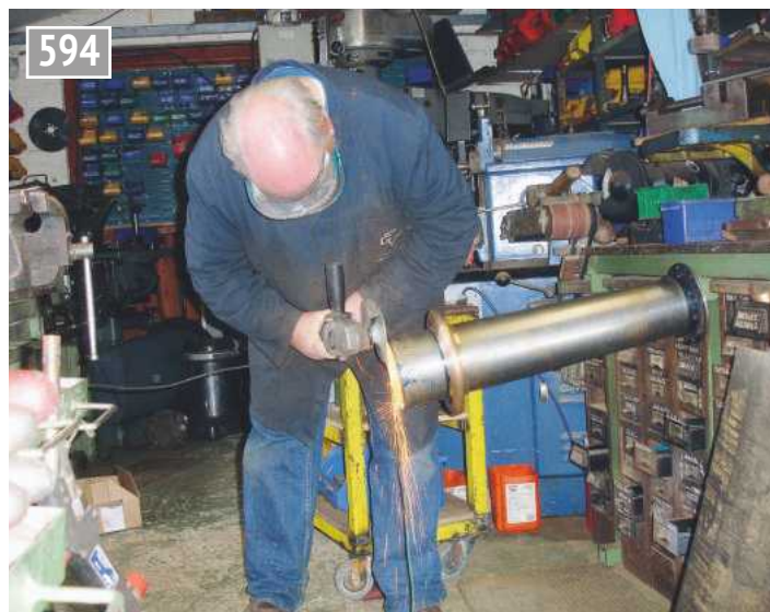
Cleaning up chimney end.
