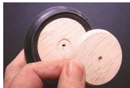
Wheel with tyre fitted and wheel trim ready to be glued on.
