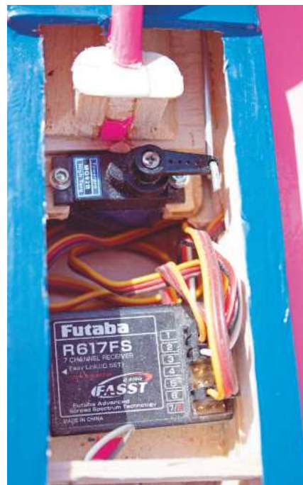
Elevator servo and receiver are located at the back of the R/C bay.
