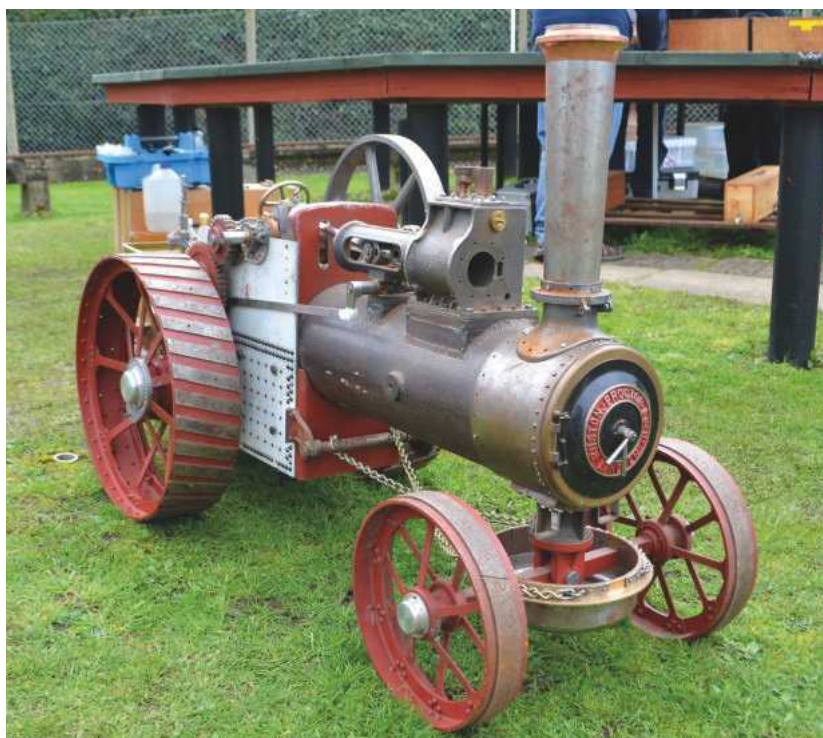
A 3 inch Ruston Proctor engine, being constructed by Alan Burrows. This is a model of Alan's grandfather's engine, still on display at Thursford, and is a replica of the original. Alan made the patterns for the castings himself. This is an ongoing project, having been started in the mid 1990s.
