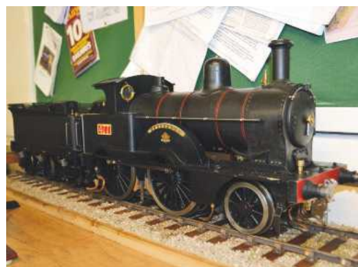
John Bloom's 3½ inch gauge LBSC 'Mabel' Caractacus, an LNWR 'Jumbo' locomotive. This model took 5 years to make and the tender is John's own design, taken from the original at Shildon.
