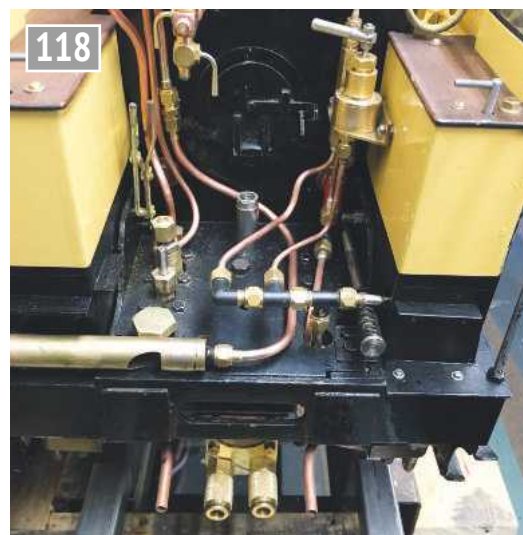
View showing the pipework under the cab floor with the compressed air manifold and brake valve prominent. Below the footplate the offside pressure connection is for the tender hand pump, the nearside pressure connection is for air with injector feed pipes either side. The oil reservoir for the hydrostatic lubricator is below the drag box on the near side. The spring loaded push rod on the offside operates the drop grate.
