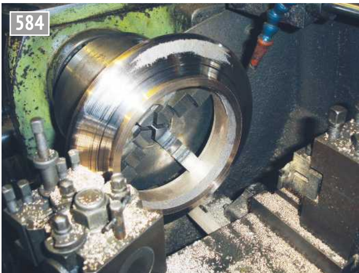
Machining chimney profile.
