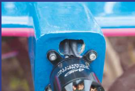
Open up the wiring access hole to get some cooling air to the LiPo.
