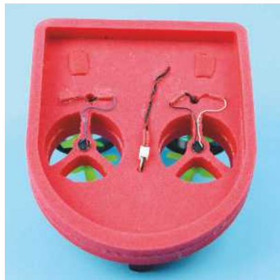
Front motor wiring on the Eo10 needs extending but may not be necessary with other drones. The central wire with a connector is the power cable for the camera and video Tx.
