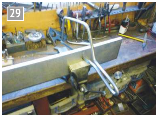
Precise hacksawing of the blanks for the beams.
