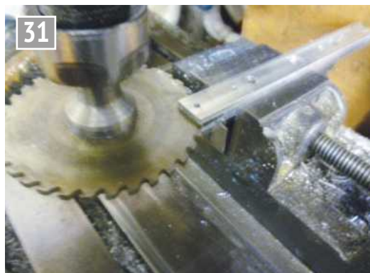
Sawing out a slot in the beam.
