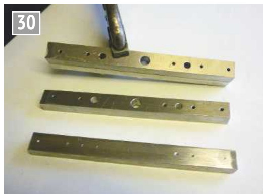
Spotting through the holes in the beams.
