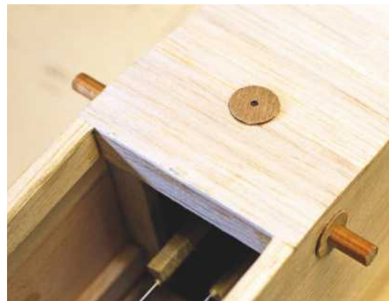
Above: Doughnuts provide local strength where needed for wings, undercarriage and aials.
