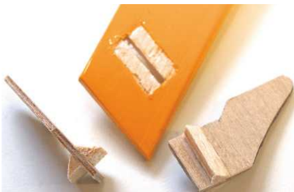
Hardest bit is cutting the neat slot for the blade through the control surface!
