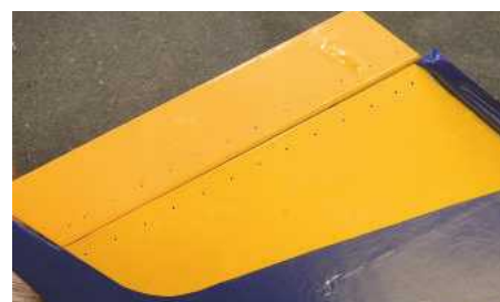
Rudder and fin with staggered holes so the thread will zig-zag down the hinge.
