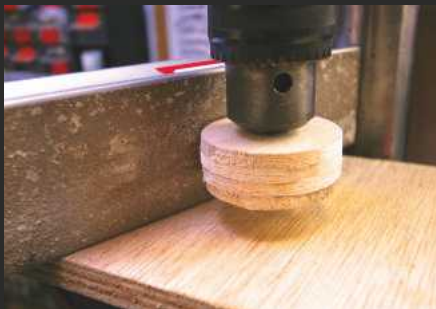
Balsa blanks on a set-screw mandrel are trued up in the drill chuck with a sanding block.
