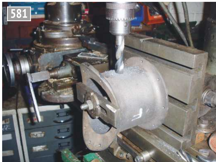
Drilling chimney for blower.
