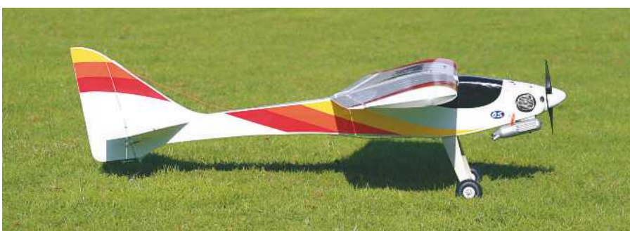
Mk.3 was released in 1992 with a tapered wing and a restyled fuselage.
