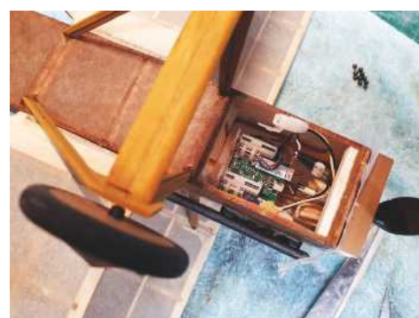
Above: Very popular AR6400 Rx brick positioned on a small shelf. This is a 3-channel unit, with a built-in brushed ESC and two linear servos Left: Polythene sheet keeps the magnets from sticking together when glued in place
