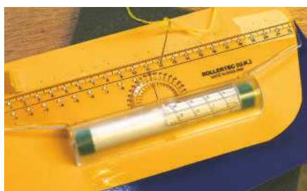
I used my trusty Rollertec drawing instrument to mark out the hinge holes.
