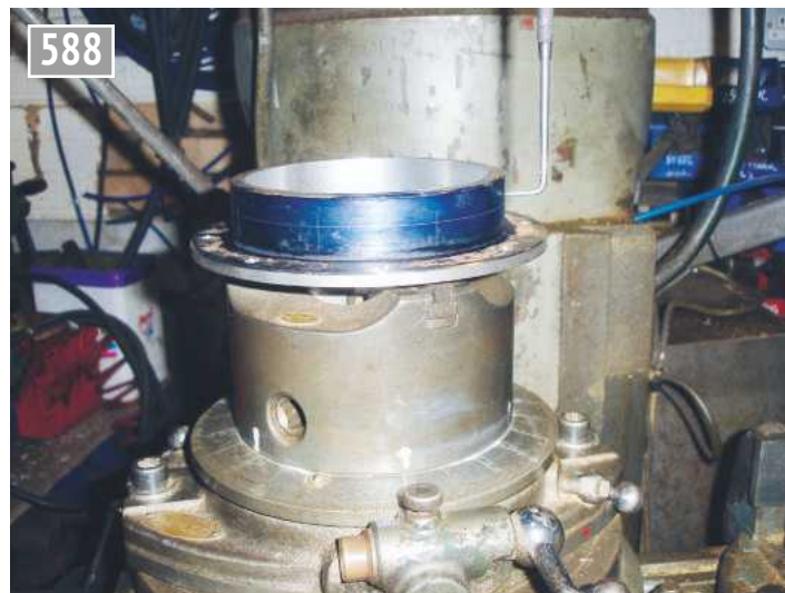
Marking out chimney base.
