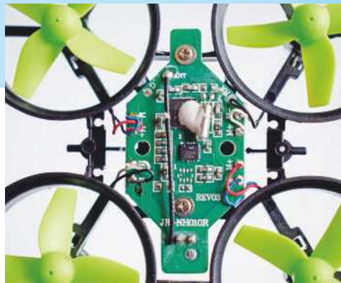
Above: Just one of the many suitable mini drones for a Whoover conversion. I used an inexpensive Eachine Eo10 to great effect. Left: The motors on the Eo10 control board are soldered on so these will need temporarily and carefully removing to install on the Whoover (or Tiny Wing). The ducts and battery box are cut off the frame to be reused.
