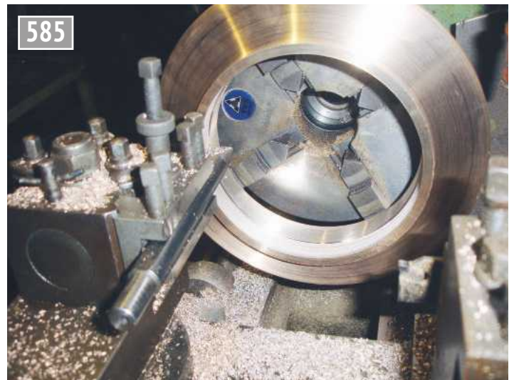
Machining chimney profile.
