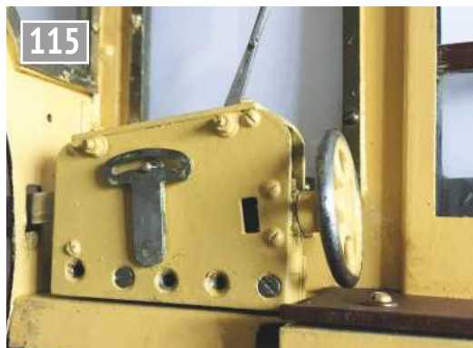
Reverser mounted on cab platework.
