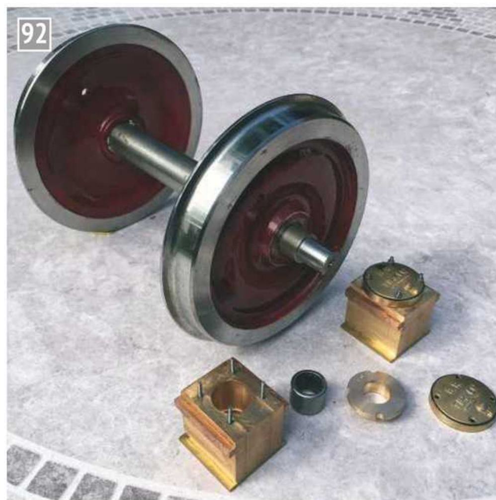
Tender wheelset showing axle box components.
