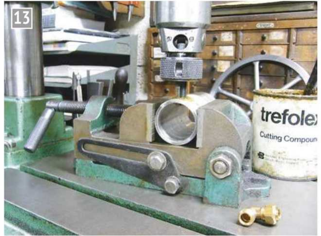
Tapping the power cylinder for the transfer pipe.
