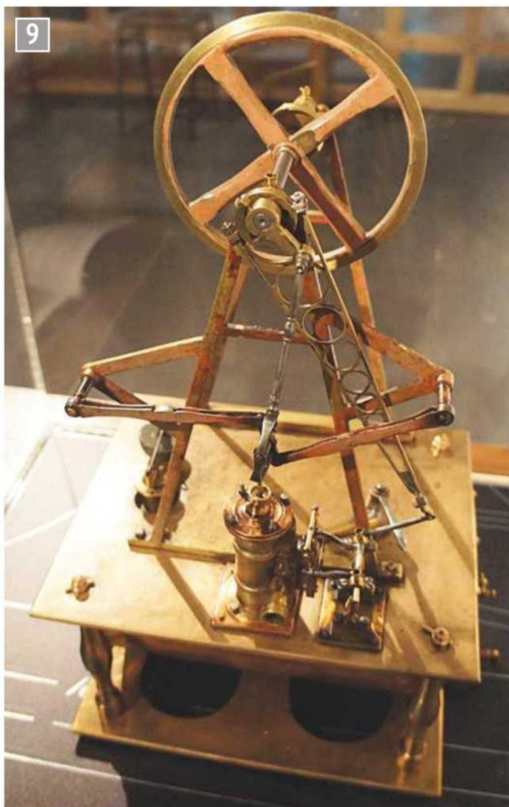
Model of an incline winding engine built by 16 year old Thomas Greener of Etherley, County Durham. It is the oldest working model steam engine.
