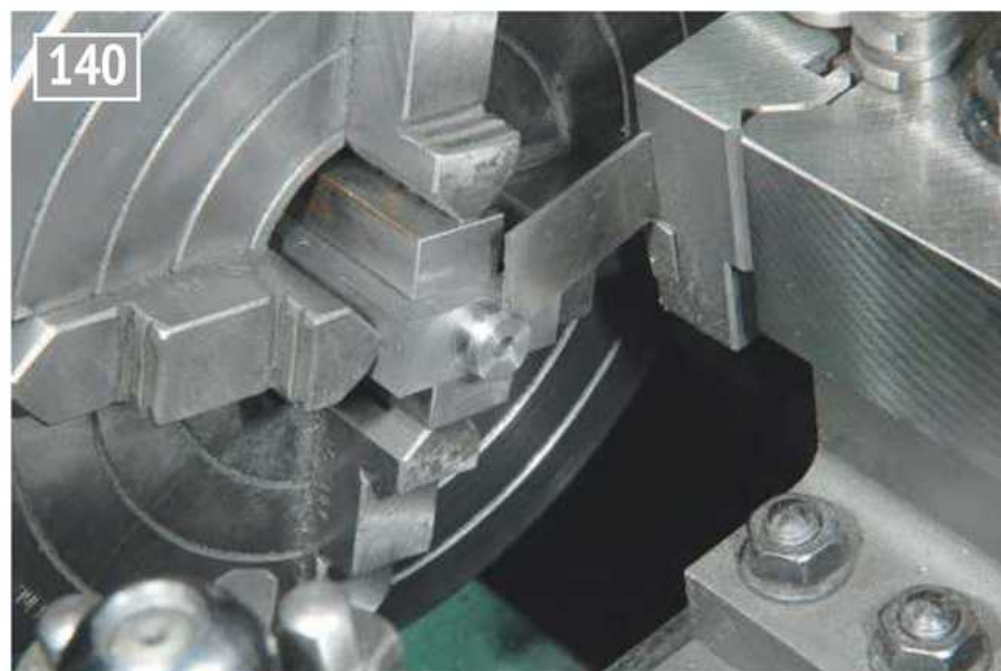
Turning the valve rod flange on the steam chest.
