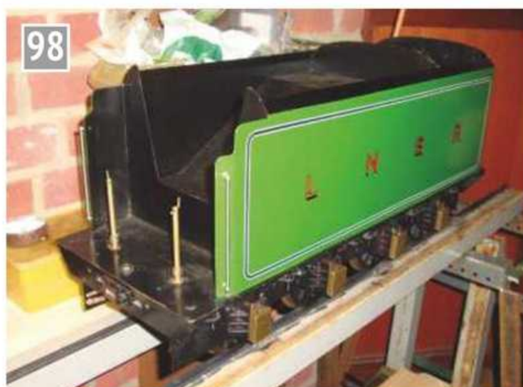
98 The tank on this very basic tender was used as a basis for the new corridor tender.
