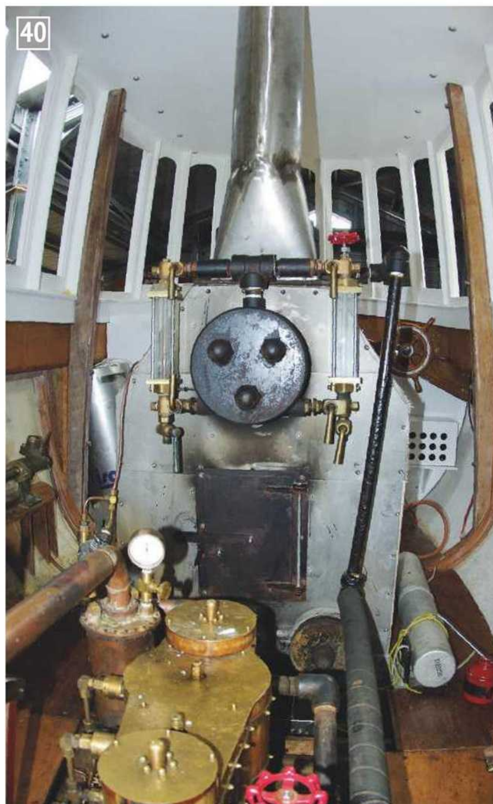
The boiler fitted to the hull.
