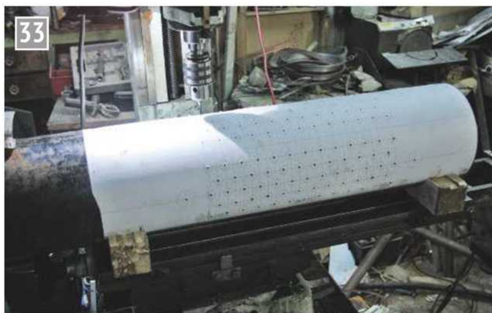
Paper pattern wrapped around the drum for drilling holes.
