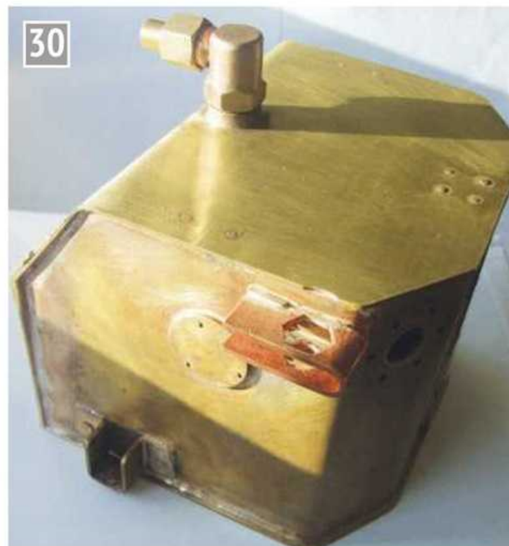
30 The final assembly of the adaptor fitting in position on the tank. The pipe union can be blanked off with a machined brass pipe union added or just a fibre washer inside the union nut.
