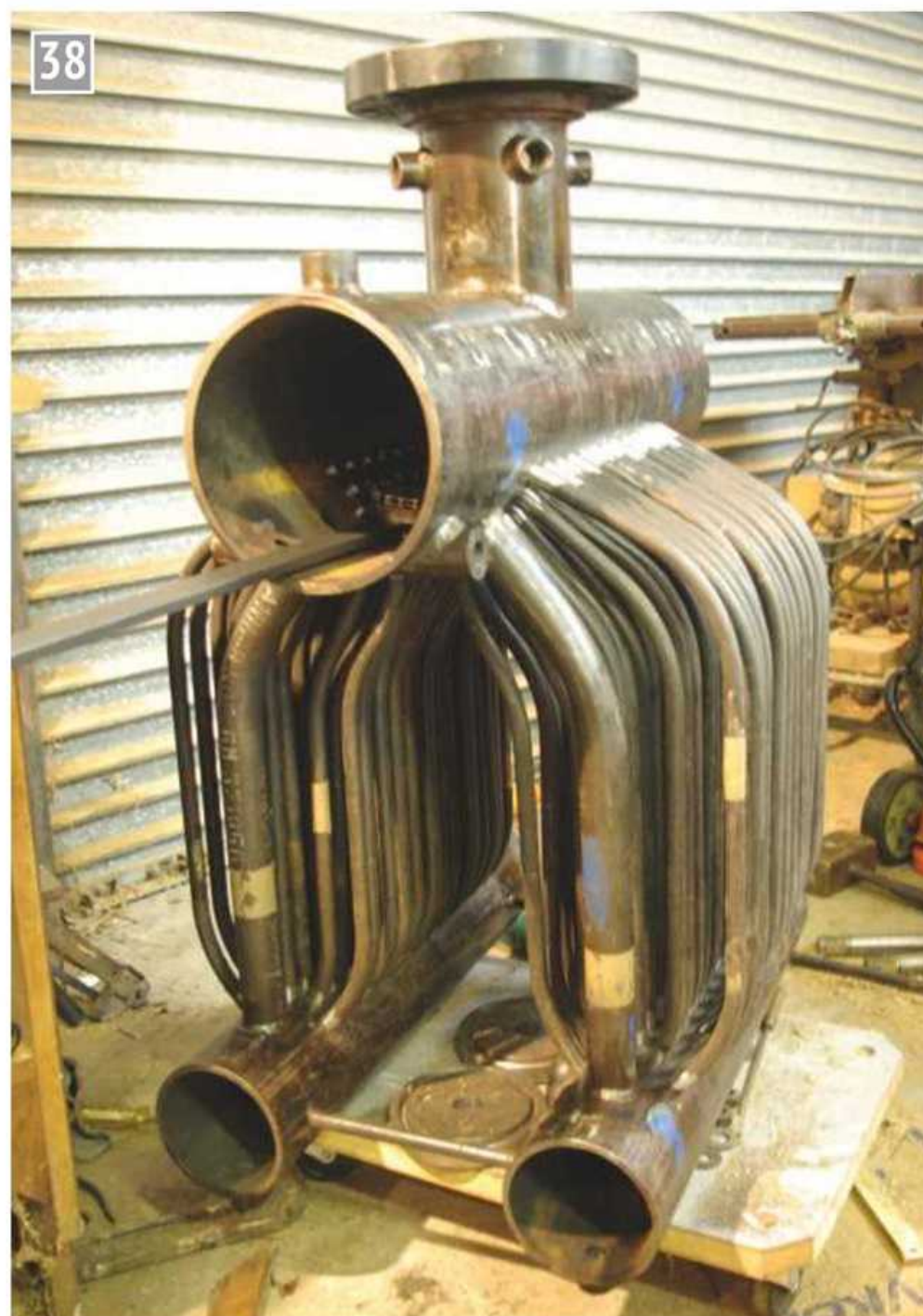
All tubes installed and expanded, ready to fit the end covers.
