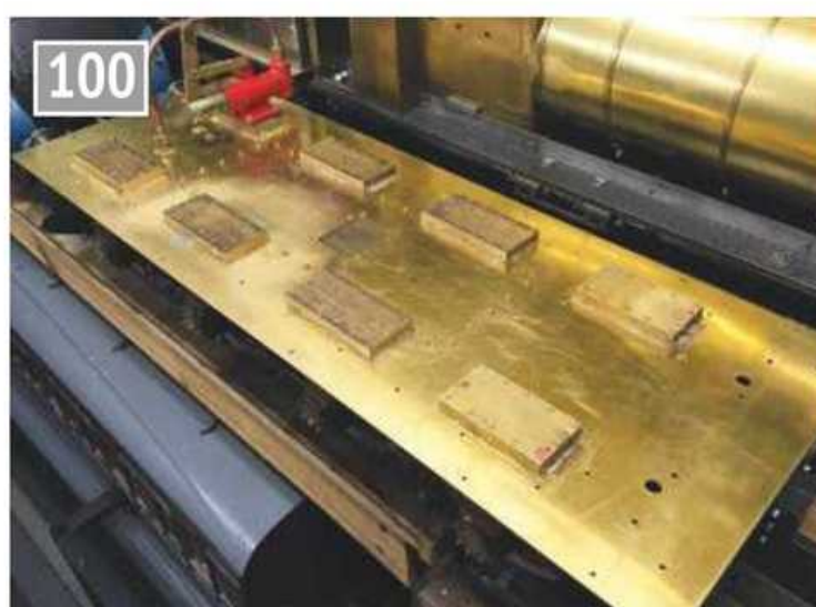
100 The new tender soleplate showing splashers, filter and hand pump.
