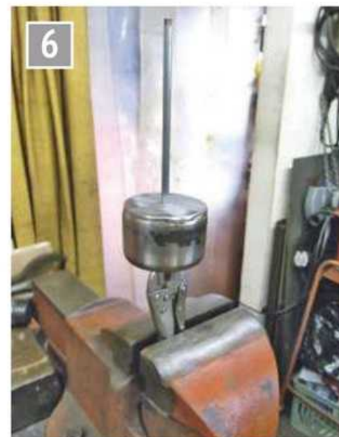
The displacer piston is a stainless steel sugar basin.
