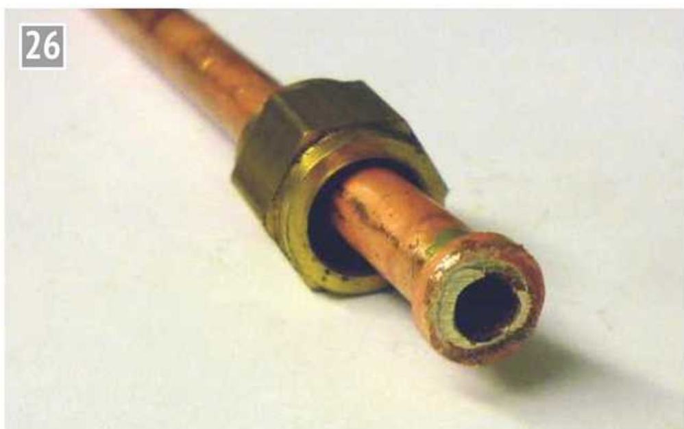
After a final touch with the file, the union is ready for use.
