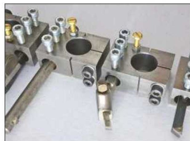
David Smith makes a set of holders for a Myford M lathe.
