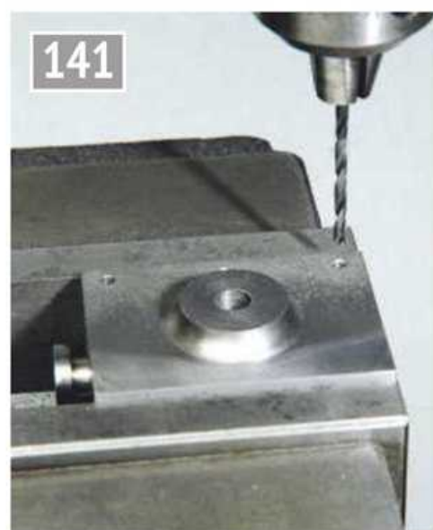
Drilling holes for the studs.
