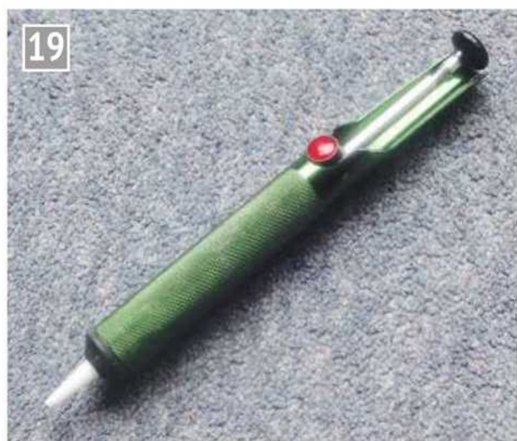
Solder sucker – depress the latching plunger, hold close to the joint whilst melting the solder with a soldering iron and then press the release button. Hey presto, no more solder! Note that the plastic tip is heat-proof.
