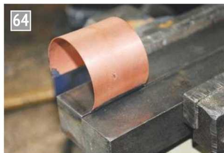
Forming the bends in the ends of the cladding.
