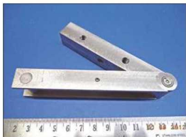
Stew Hart explains how to make and use a 'sine protractor' for setting accurate angles.
