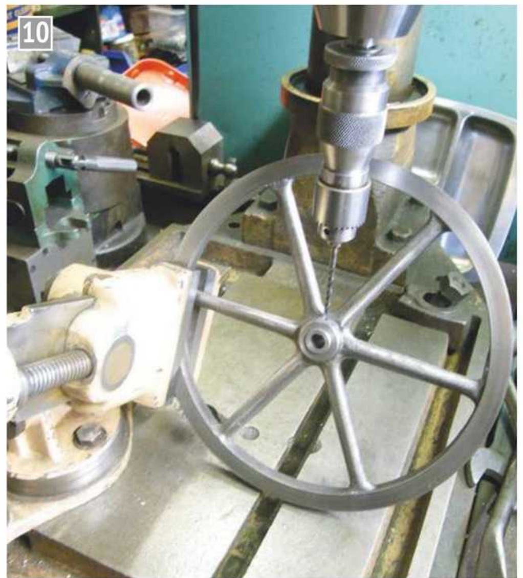
Drilling the flywheel for the grub screw.
