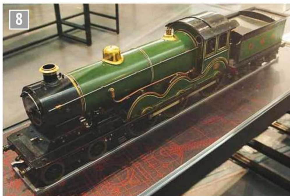
Cosmo Bonsor built by Bank of England clerk, Jim Crebbin in 1903 to test ideas about superheating and compounding. It hauled the first train at the first Model Engineer exhibition in 1903 and ran there until 1950.
