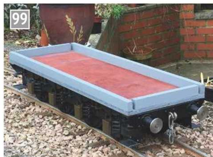
99 The original chassis was modified to create a very useful flat wagon.
