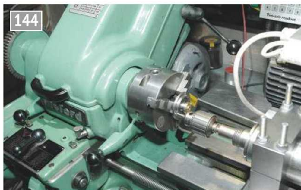
Drilling the cylinder cover.
