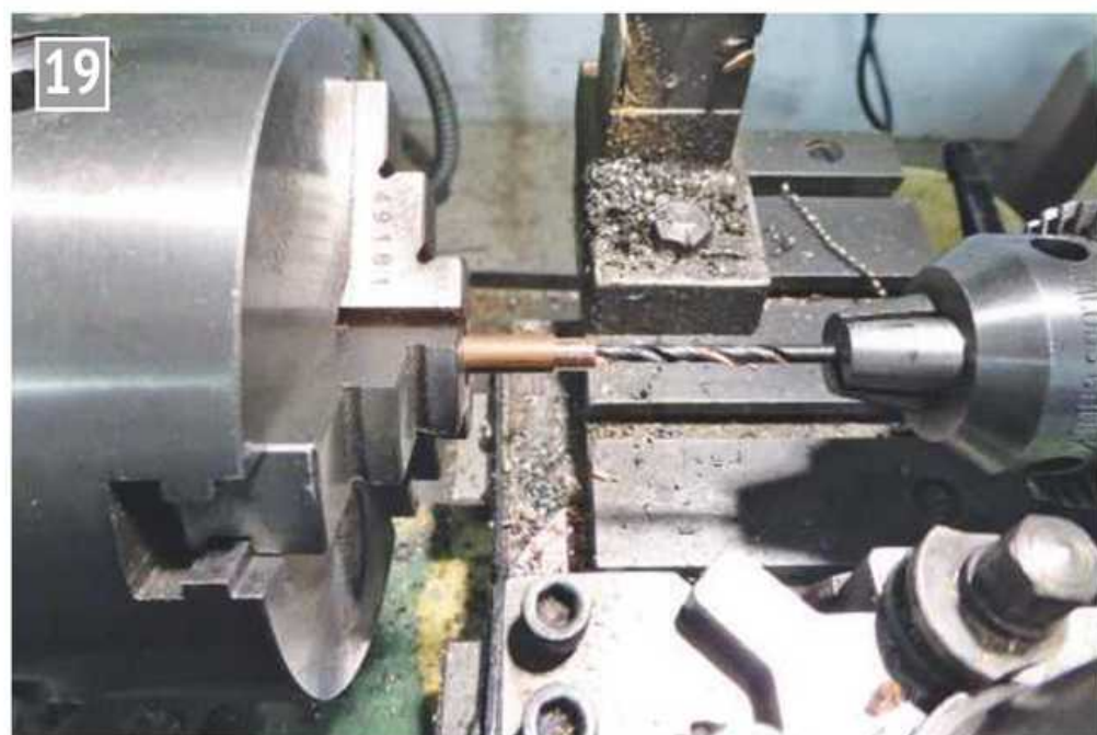
The copper is centre drilled and then drilled for the pipe.
