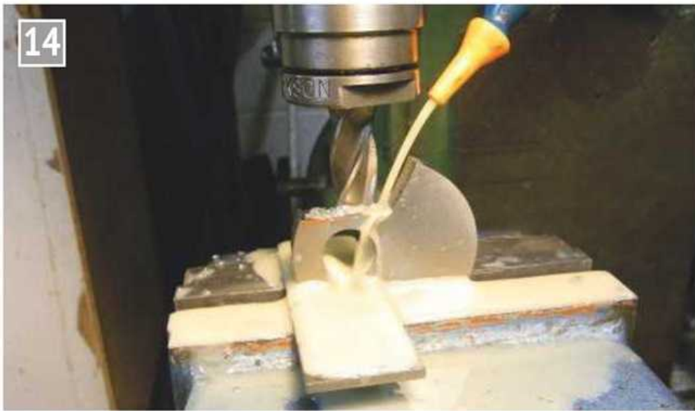
Milling the extra balance weight.
