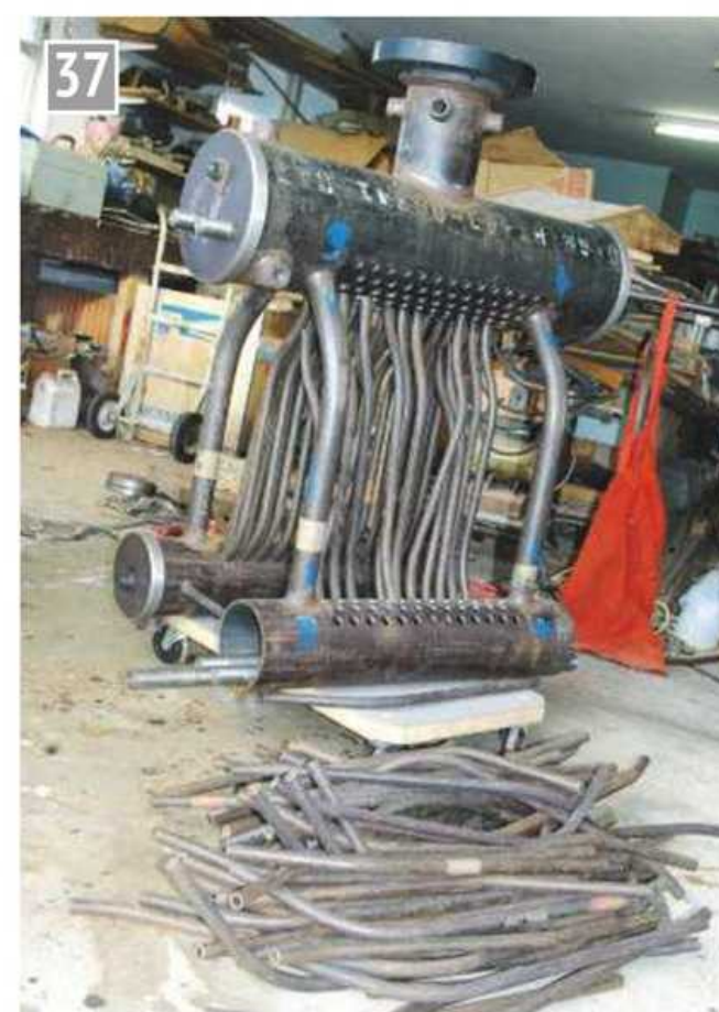
The inner tubes must be installed first.
