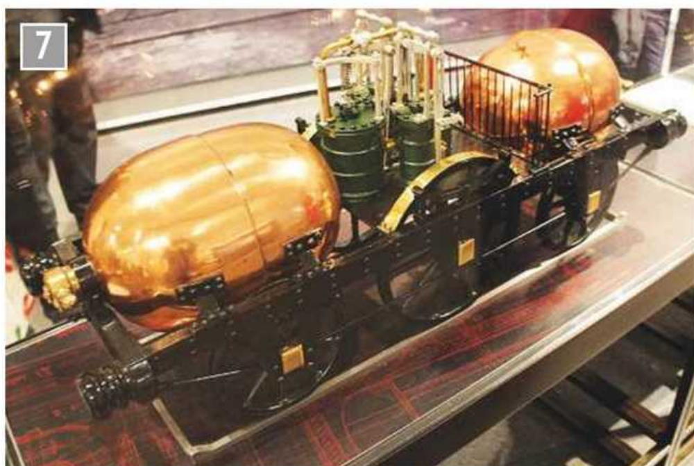
Another locomotive experiment; Arthur Parsey's idea of a compressed air locomotive. Though the Great Western Railway did not take up the idea, such locomotives found favour in underground workings.
