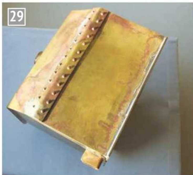
29 The final piece of ⅛ inch thick plate with its angled jointing lap strip in place. One edge of the strip was riveted and soldered first, then the plate was lined up and the second row of holes added and cleaned up. The plate was then silver soldered in place with loose rivets through the other half of the strip to ensure the rivets did not fall out.
