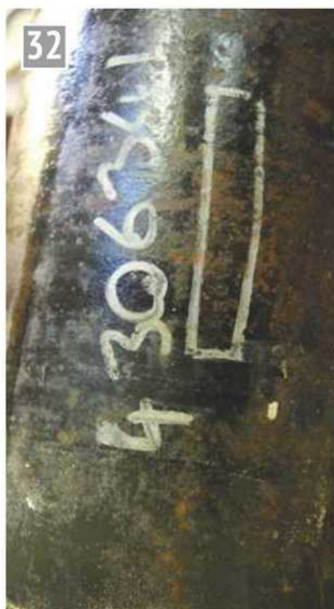
The heat number is stamped on the tube and then outlined with a white marker so that it can be found easily.
