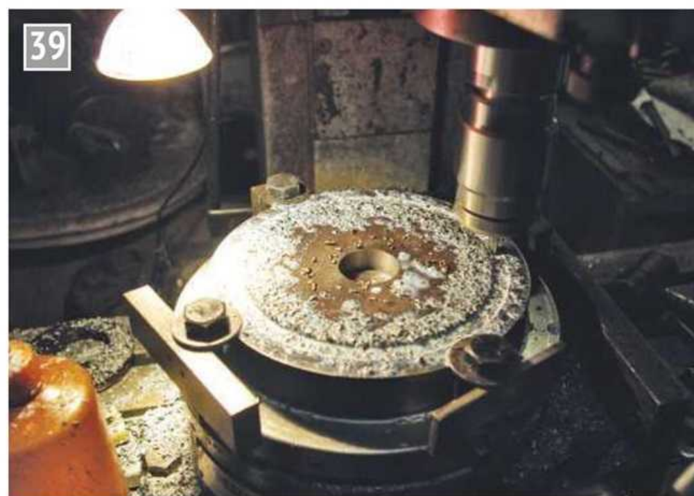
Milling the groove in a mud drum cover for the gasket.
