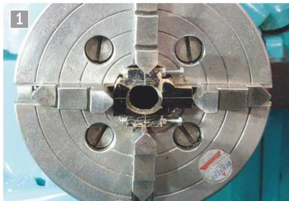
Rough hole in centre of the casting.
