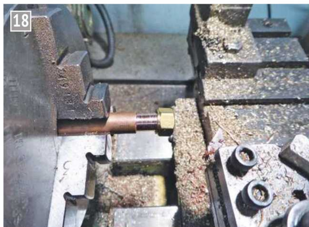
The bevelling tool used to turn the outside diameter of the olive so that it is an easy fit onto the nut.
