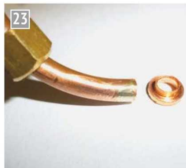
The pipe is carefully cleaned prior to silver soldering.
