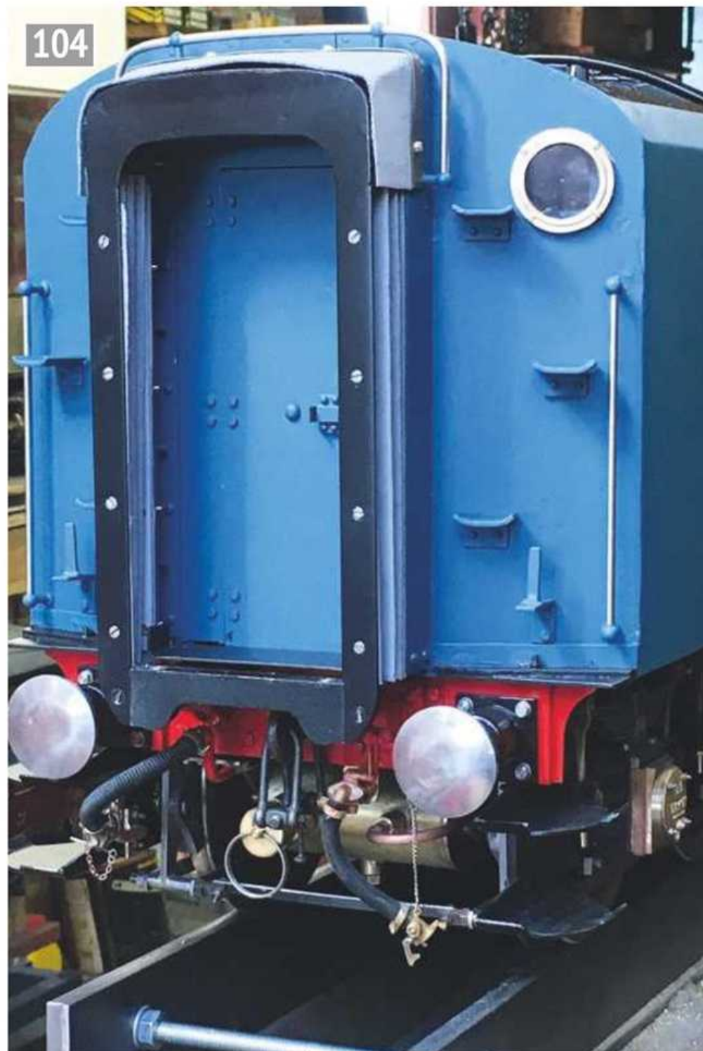
Tender rear view showing corridor vestibule. The Buckeye coupler has yet to be fitted.
