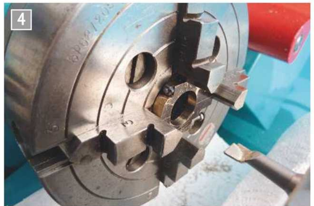
Boring the hole.
