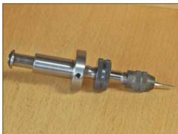
Graham Meek introduces his special attachment for tapping small threads.
