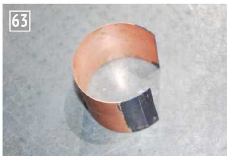
Cladding rolled to the correct diameter.
