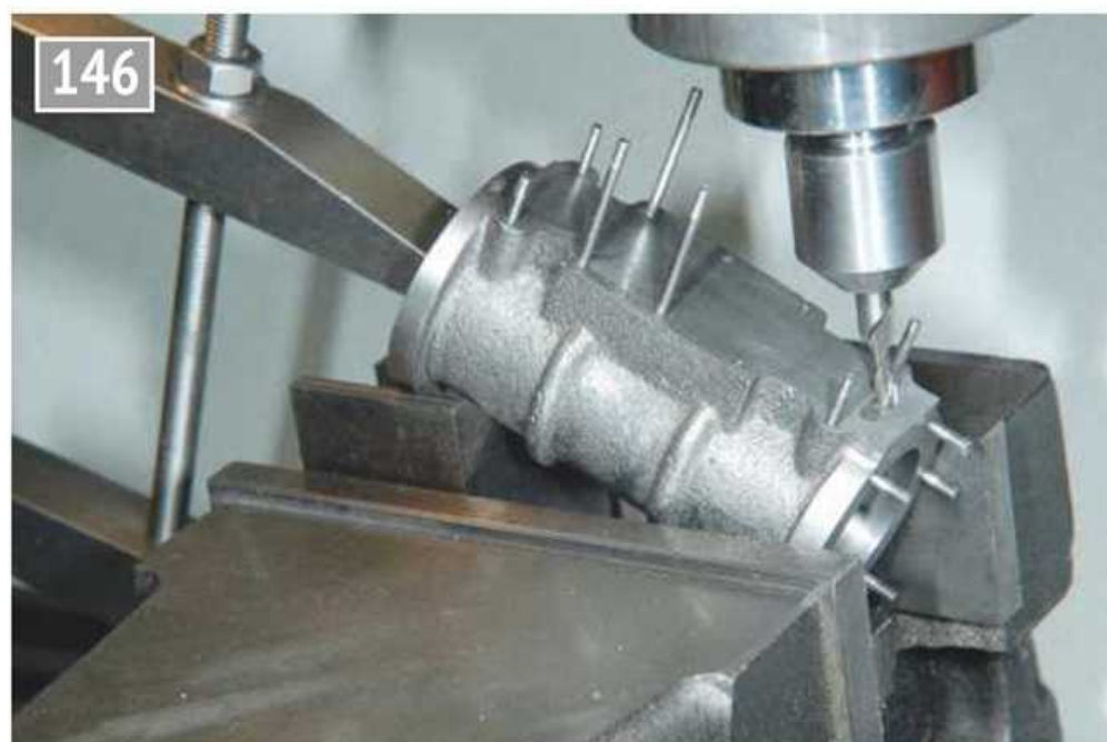
Milling the cylinder ports.
