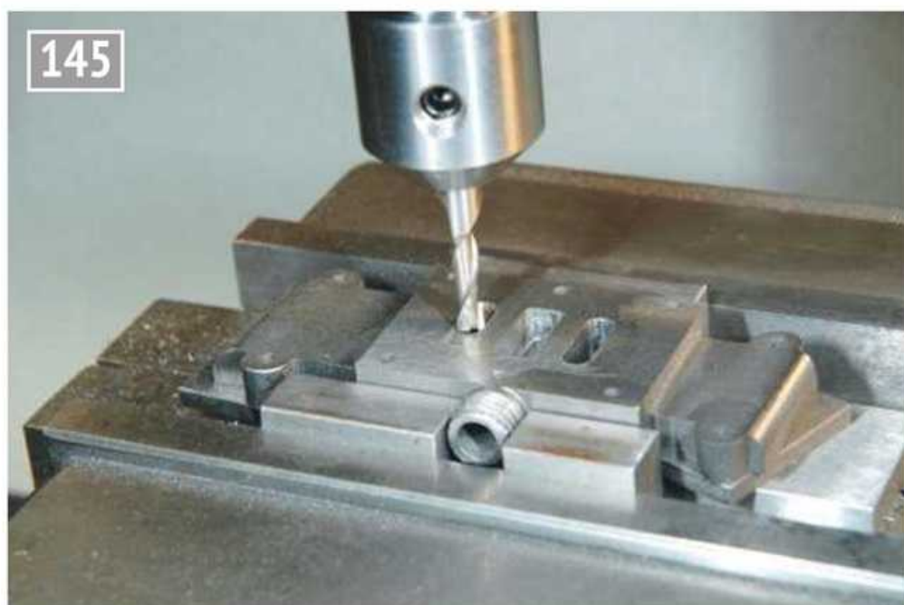
Milling the steam ports.
