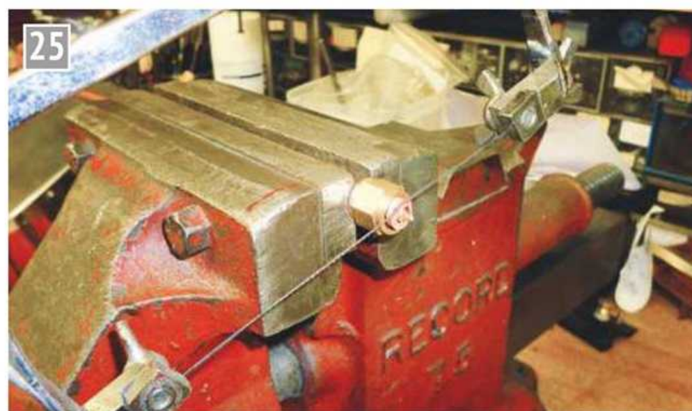
The remnants of the parting off burr, which we used to position the olive, is sawn off.
