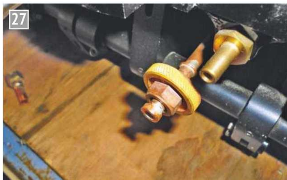
I find this modified union nut helpful in lining up the tender hand pump joint.
