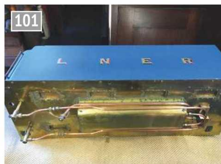
101 No. 4497: The tender soleplate from below showing the well tank and the gravity and hand pump feed pipes. The hand pump draws water from the main tank, not the well.
