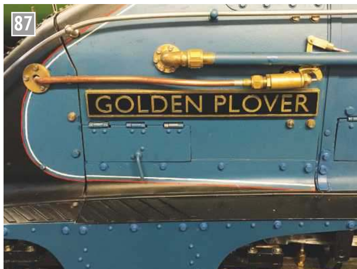
Smokebox near side showing operating valve and feed to whistle.
