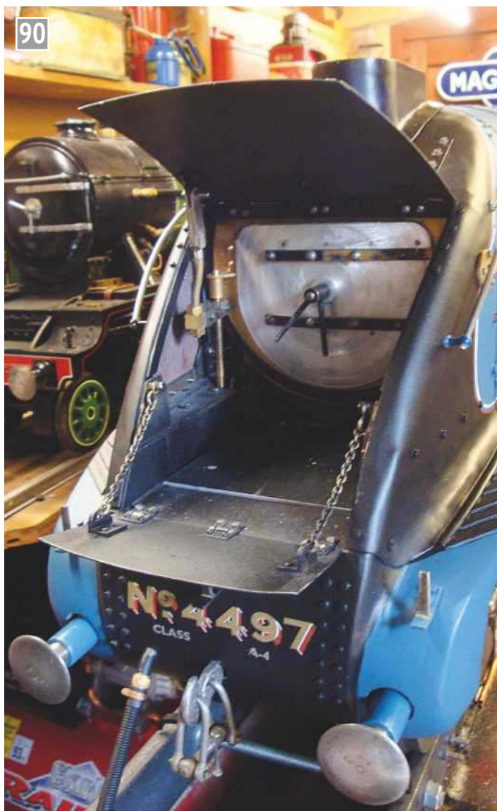
'Cod's mouth' doors in the open position.
