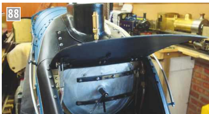
View from the other side showing where the whistle steam is Tee'd off to the dummy in front of the chimney. The photograph also shows the upper connection of the 'cod's mouth' door operating mechanism.
