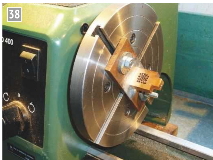
Machining the valve chest on the faceplate.
