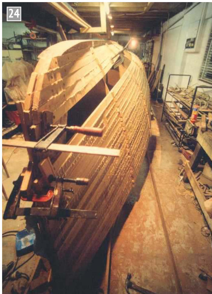
Planking almost complete.
