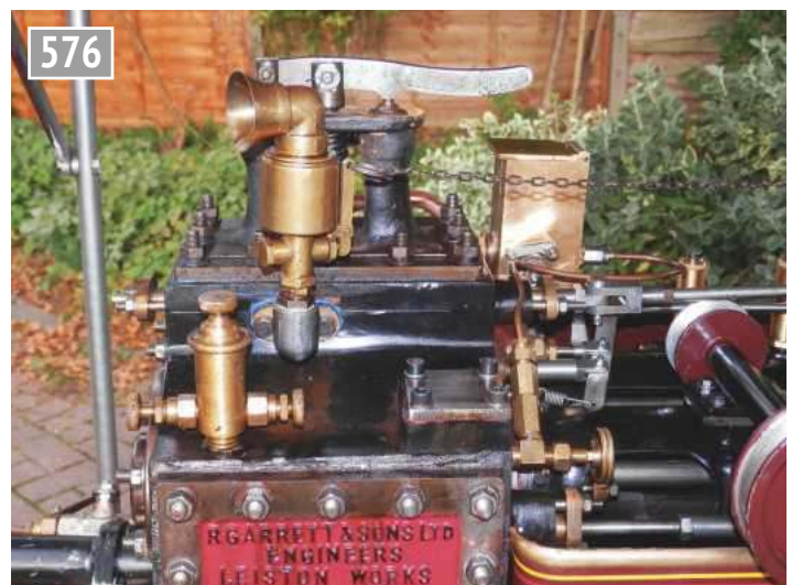
Lube steam valve.
