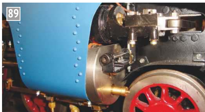
Operating mechanism for the upper door of the 'cod's mouth'.
