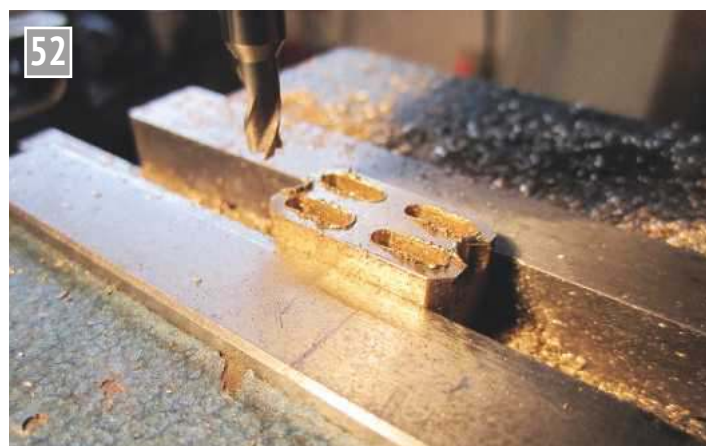
The pilot valve. In need of a little deburring!
