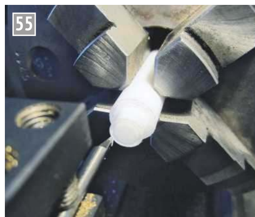
Photo 55: Turning the water piston from PTFE rod.
