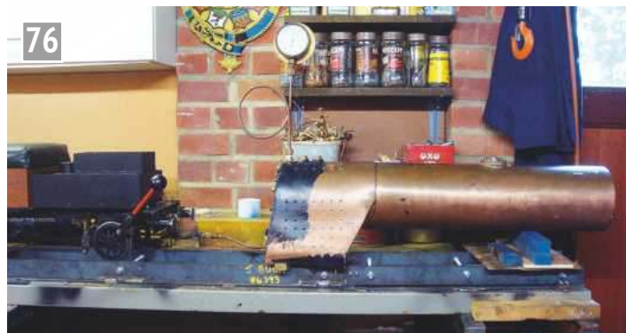
Boiler under test. 160 psi was sustained with no weeps or detectable deformation.
