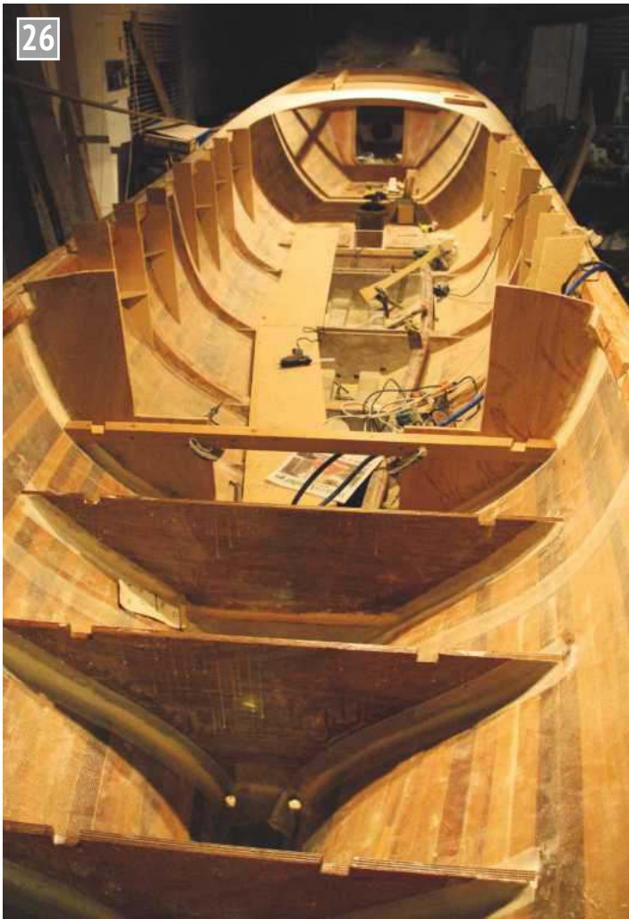
Ribs and bulkheads fitted.
