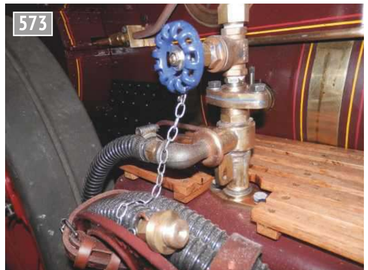
Water lifter and valve.
