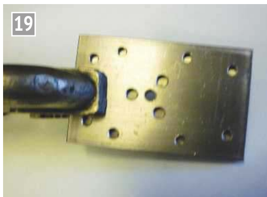
Steam chest cover, drilled for the steam inlet.
