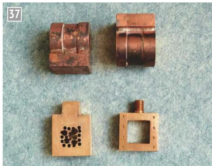
Cylinders and valve chests at various stages of manufacture.
