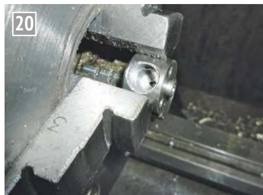
Turning the steam inlet gland.
