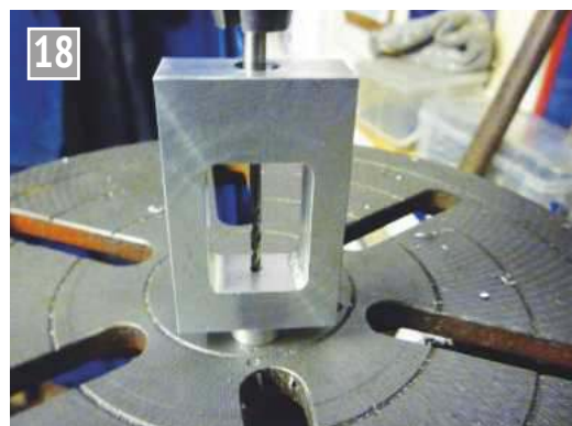
Drilling the valve rod guide.
