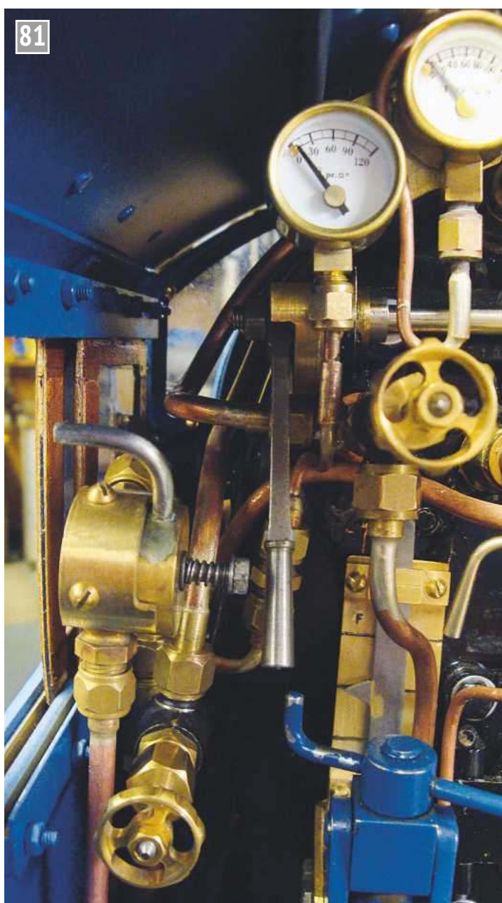
81 View from the Driver's seat. The vacuum brake valve is prominent. Steam chest pressure gauge on the left, boiler pressure on the right.
