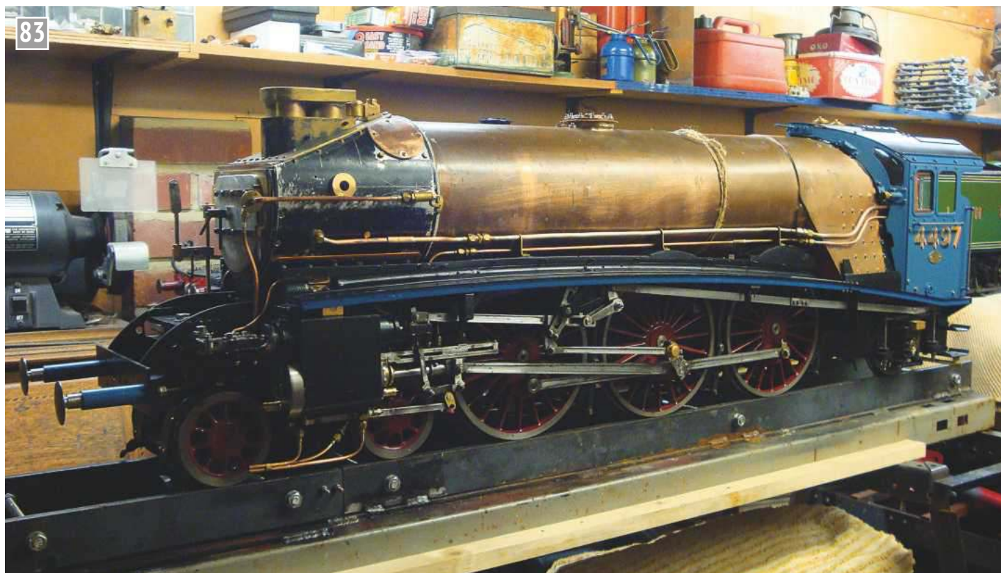
Before the streamlined casing was fitted, the underlying pipework including the snifting valve behind the chimney is visible.
