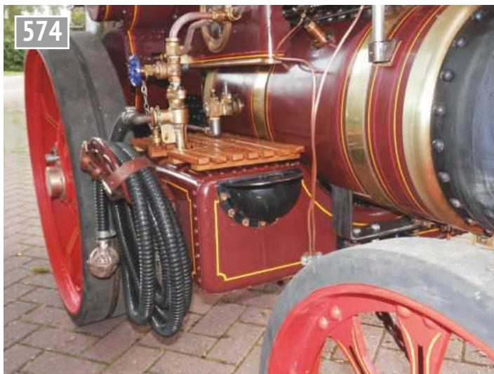
Drain cock pipes.
