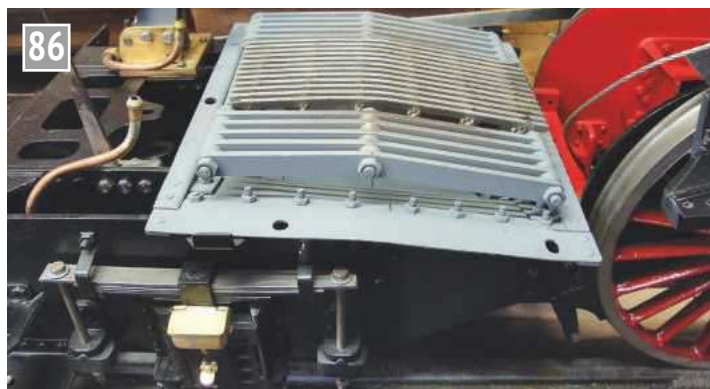
Ashpan installed showing grate. Outer sections are fixed; centre section can be dropped through the hopper doors.
