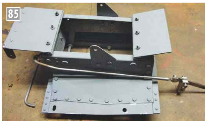
Ashpan assembly inverted showing hopper doors and control linkage for front damper.
