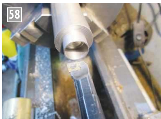
Boring the inner diameter of the piston ring blank.
