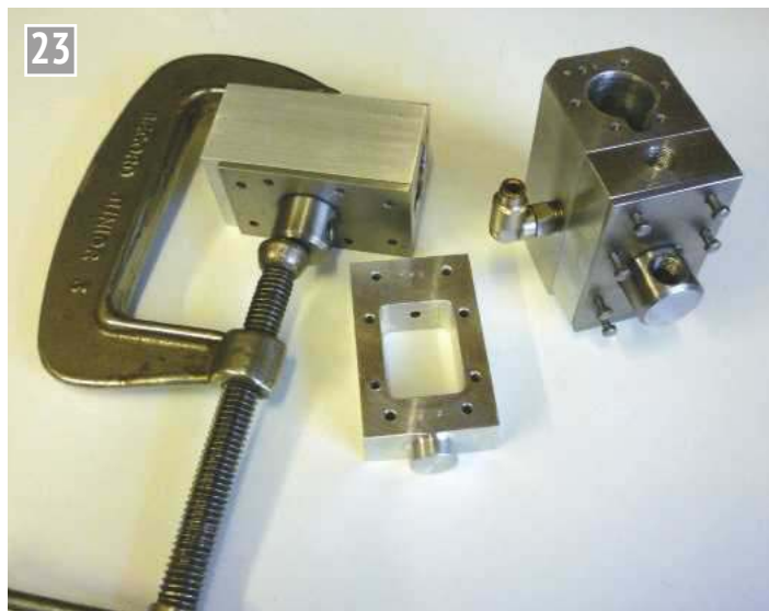
Spotting through to the cylinder.
