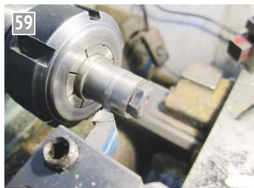
Skimming the outside diameter of a piston ring.
