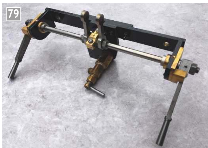
79 Regulator assembly. I found that three bearings were essential for smooth operation. The subframe also serves to support the blower valve.
