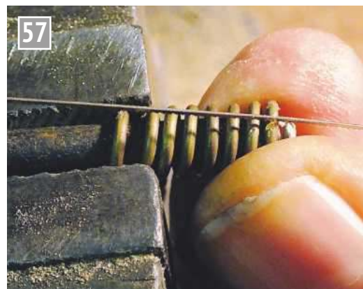
Cutting the links of a chain.
