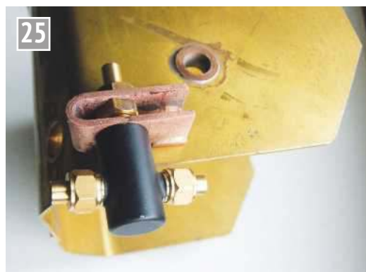
This view shows the water valve in position on the left side of the tank and a top fitting will steady the operating rod once the body of the tank has been fully silver soldered.
