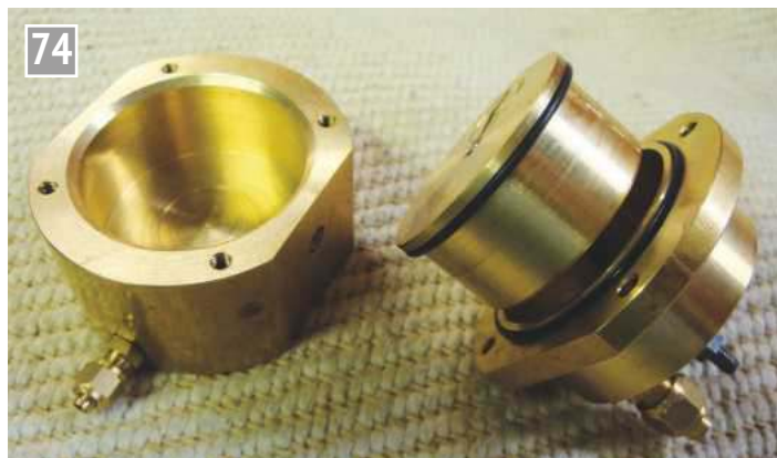
A4: Vacuum cylinder parts showing the rolling ring.
