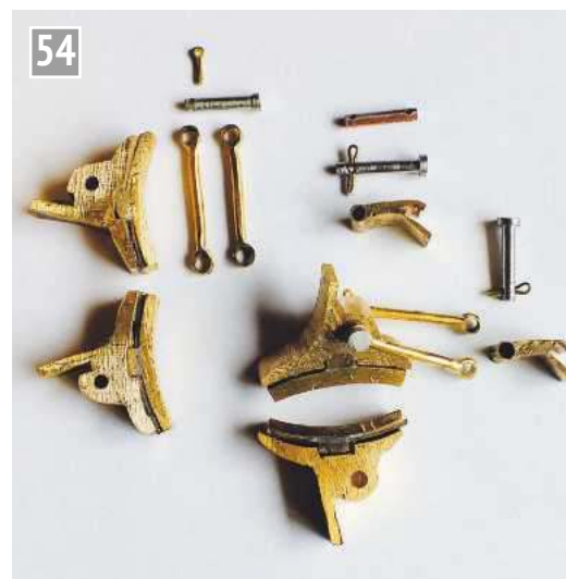
Shoes are glued or soldered to the holders.
