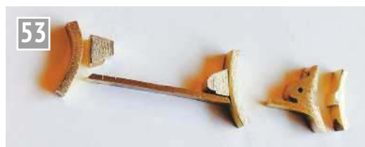
Fabricating a brake shoe holder.
