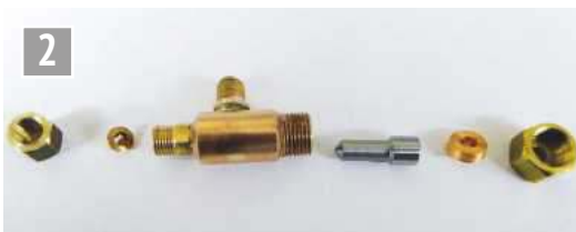
Nuts and olives of different sizes are basic parts of this steam operated drain cock.
