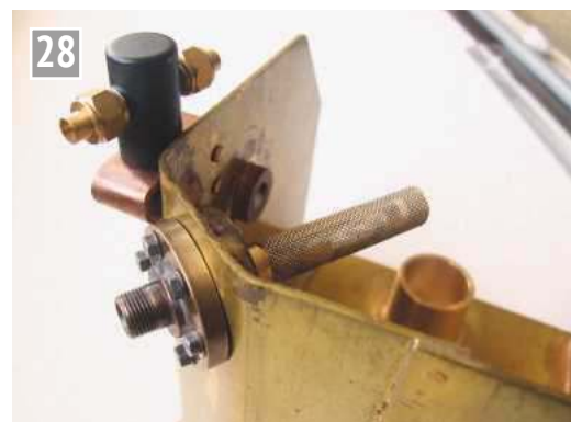
The completed water outlet adaptor mounted on the tank with the filter tube and its gauze in place. Stainless bolts will be fitted on final assembly.
