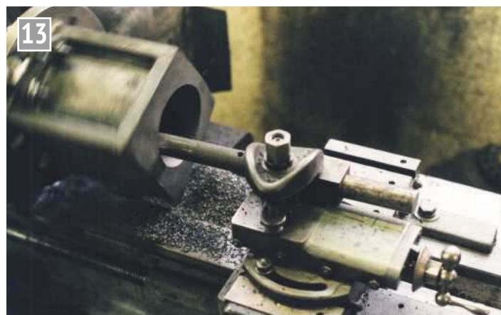
Boring the high pressure cylinder on a Myford ML7.
