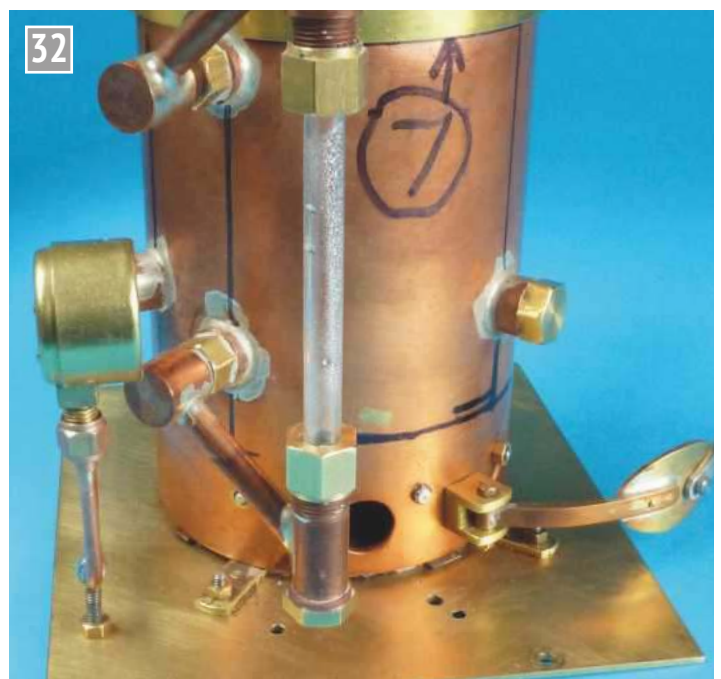
This plate supports the boiler.
