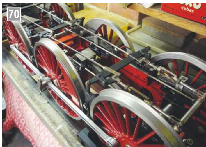
A4: Fully compensated brake rigging viewed from underside.
