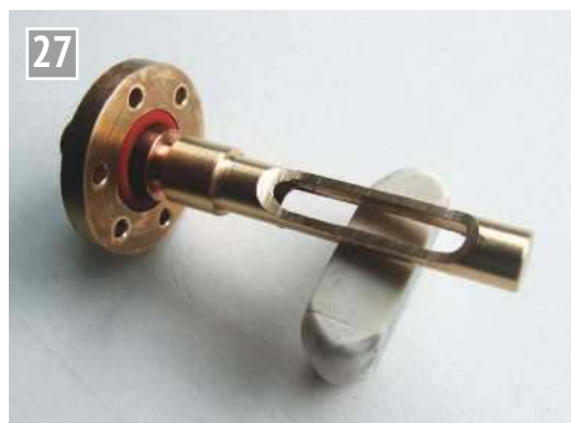
This is the adaptor assembly with the filter support tube in place.
