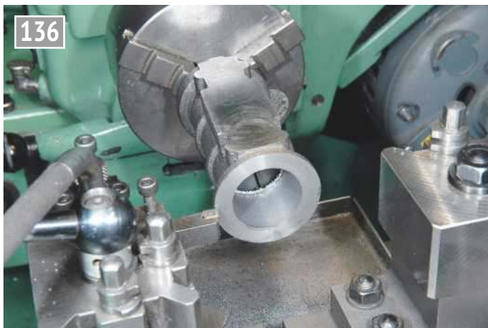
Facing the cylinder, mounted on a mandrel.
