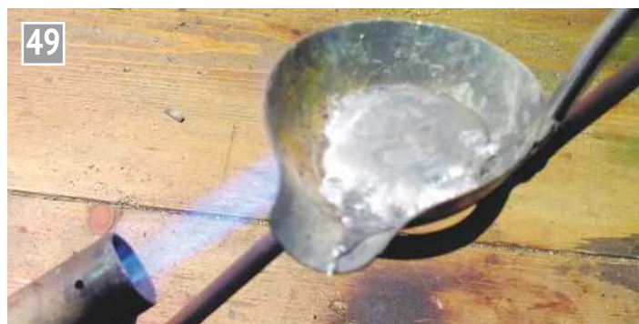
Casting: melting the white metal.
