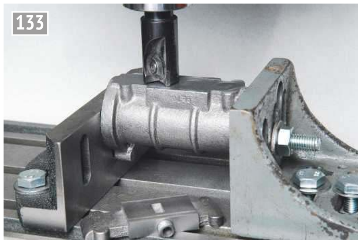
Machining the mating surface for the port face casting.
