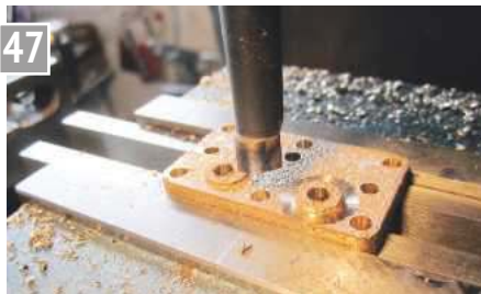
Cunning use of a boring head to cut a recess around each boss.
