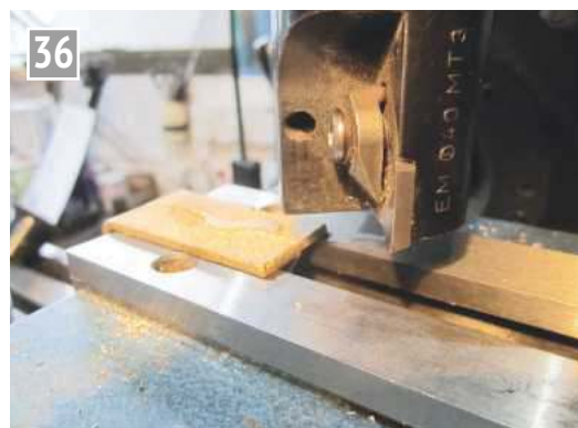
Machining the base of the coupler.
