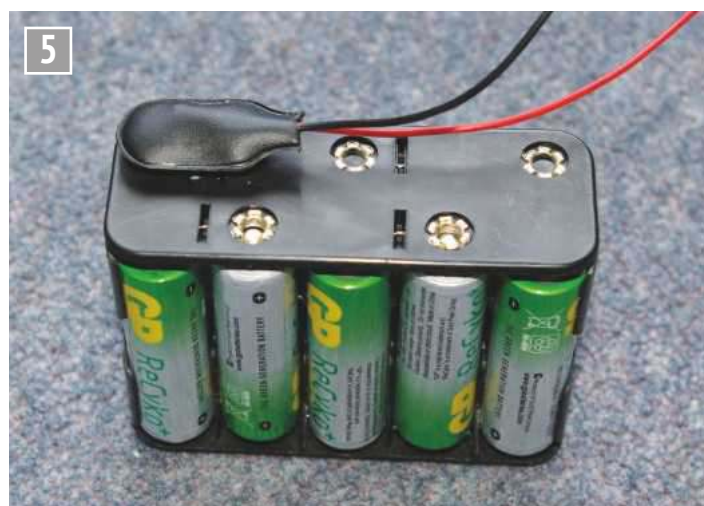
Populated battery case with PP3-style connector attached.
