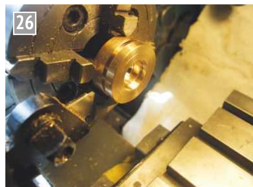
Turning the brass adaptor flange and marking off the PCD for the fastening holes.
