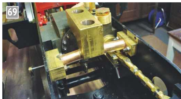
A4: The inside cylinder valve cannot be accessed from the front after installation of the outside cylinder exhaust pipework.
