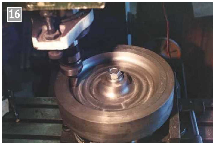
Machining the flywheel with rotary table and milling machine.
