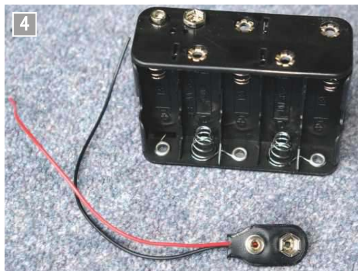
Empty 10-cell battery case and PP3-style connector. Note that these cases are also available in a 'linear' configuration, i.e. with all 10 batteries sitting side-by-side. It is a matter of personal preference as to which is chosen.
