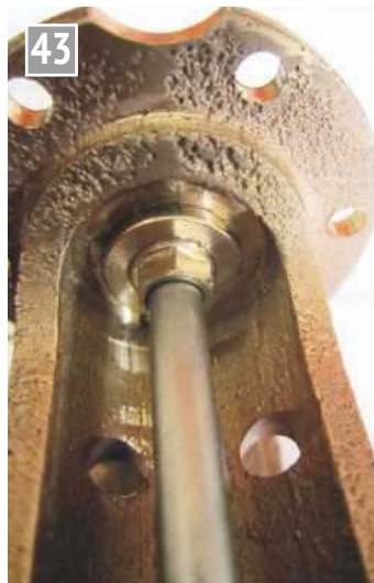
Steam gland and gland nut fitted.
