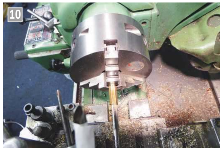
Tapping the thread - I usually pull the belt round by hand but it could be cut under power.
