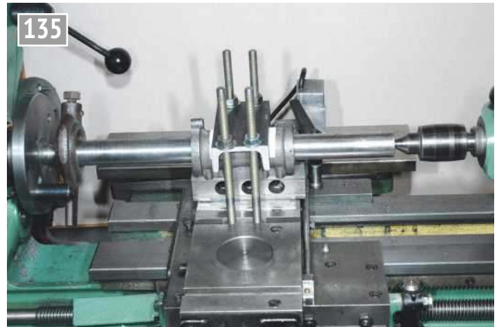
Boring between centres.
