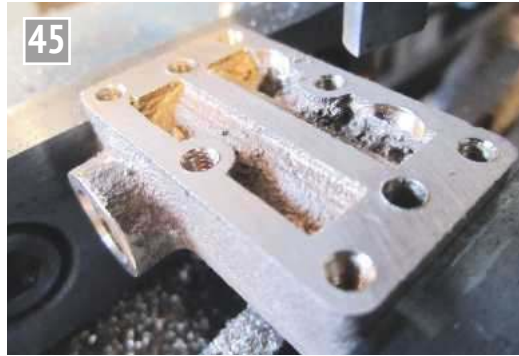
Machining the pump body.
