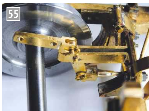
Fabricating a brake shoe holder.
