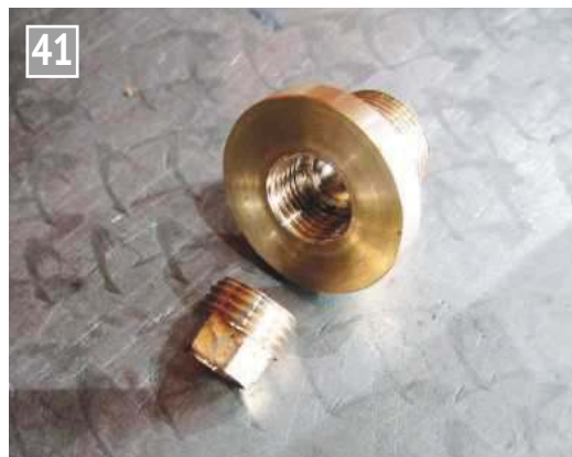
The pump retainer with its gland nut.
