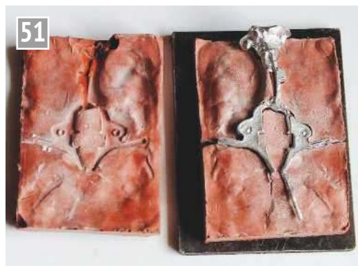
Casting: moment of truth – opening the mould.
