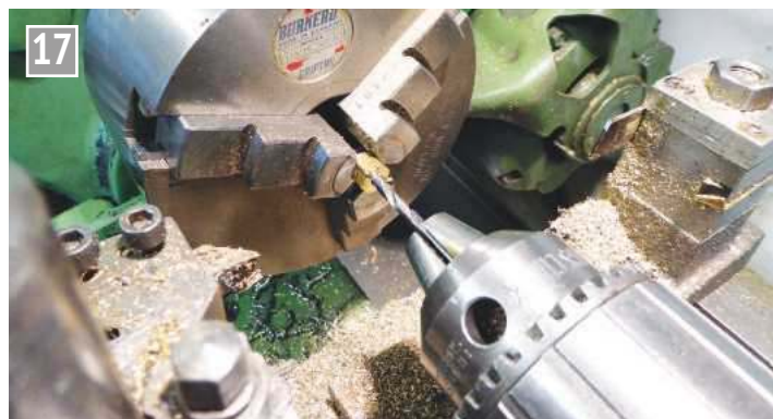
Cleaning out the hole through which the pipe will pass.
