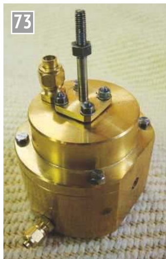
A4: Vacuum cylinder prior to installation.
