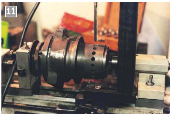
Dividing ports for the Edwards air pump using a Unimat 3.
