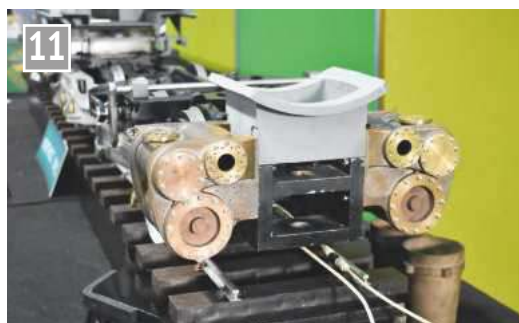
The front end of the inner engine on Big Boy under construction by Alan Antiss.
