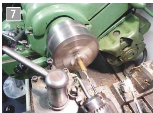
Six tool turret rotated and here is the drill for the pipe size.
