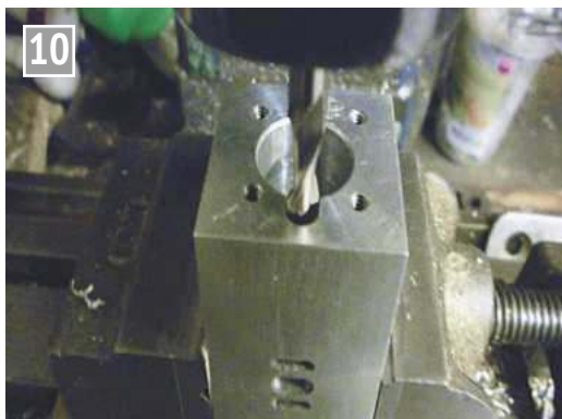
Milling out the steam inlet passage.
