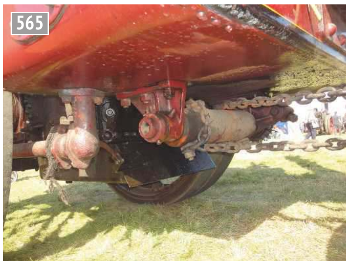
Belly tank connection.
