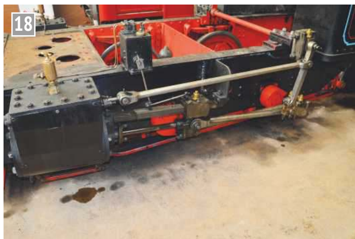
Detail useful for prospective modellers of Stanhope can be seen in this view, namely the cylinders, Hackworth valve gear and the displacement and mechanical lubricators. It is difficult to believe from this view that the frames had once been cut in half and were welded back together during the 1990's.
