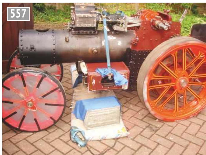
Belly tank assembly.
