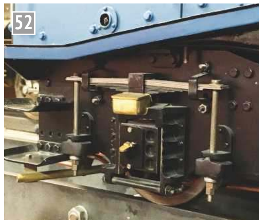
Trailing axle showing Cartazzi axlebox and leaf springing. The upper oil box feeds the Cartazzi inclined slides and the horn cheeks. The lower oil box feeds the axle to the underside, as it should, of the journal. The offside injector overflow pipe is visible below the footstep. The pipes behind the trailing wheel are the vacuum brake train pipe (lower) and connecting pipe between the vacuum reservoirs on engine and tender (upper).
