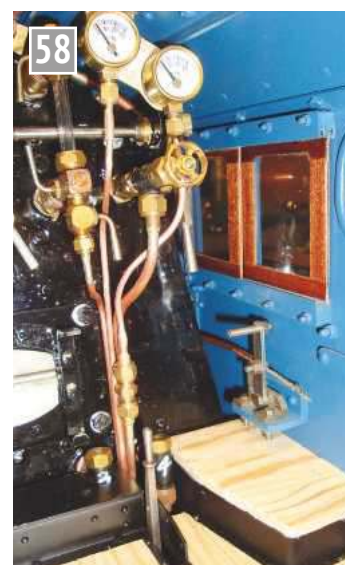
58 Cab view showing the drain cock operating level bracketed off the cab side sheet. Also prominent are the vacuum gauges for train pipe and reservoir. The lever projecting above the cab floor controls the ashpan damper.
