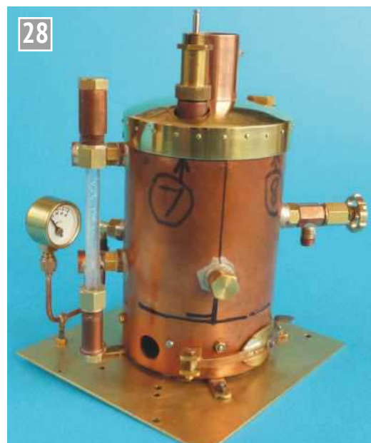
More boiler fittings – gauges from the front.
