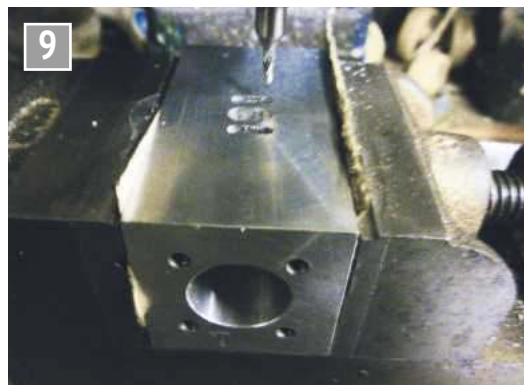
Drilling the port slots.
