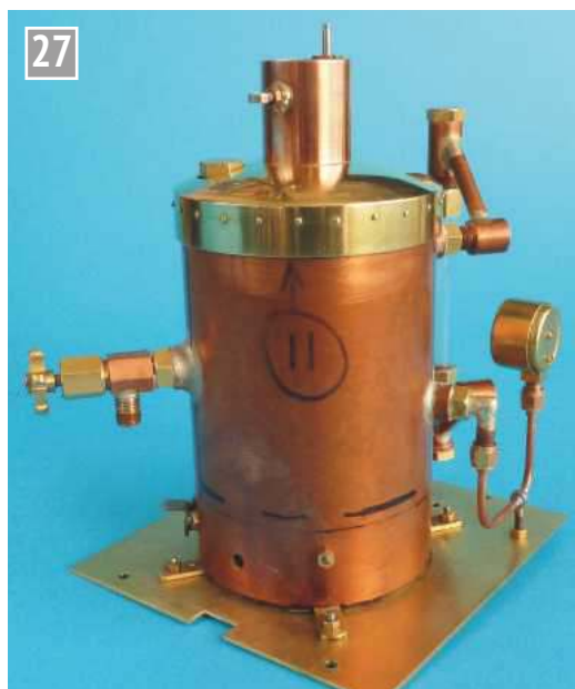
More boiler fittings – gauges from behind.
