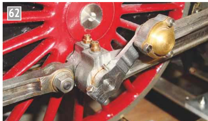
Return crank and more motion details.
