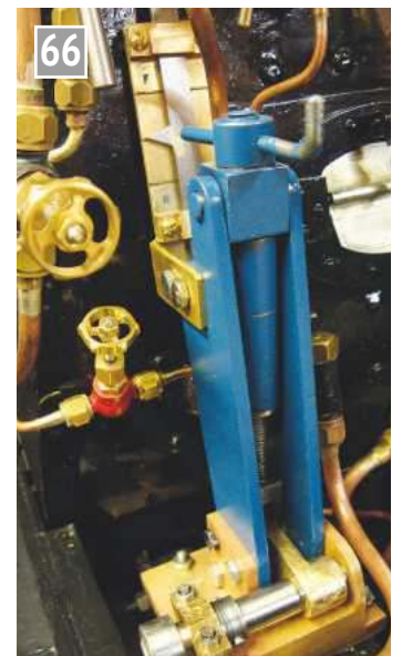
Reverser. Not visible are the stops that determine full forward and reverse gears. The fit up between the cranks and the cross shaft had to be perfect to prevent unacceptable 'wagging' of the lifting links.
