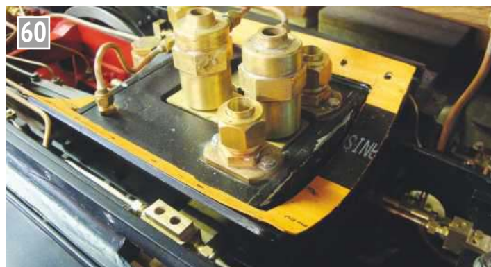
60 View on smokebox saddle showing live steam connections from superheater to saddle. ➤
