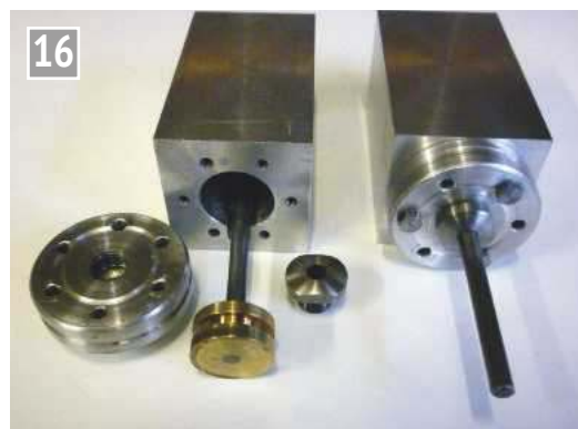
Completed cylinders and pistons.
