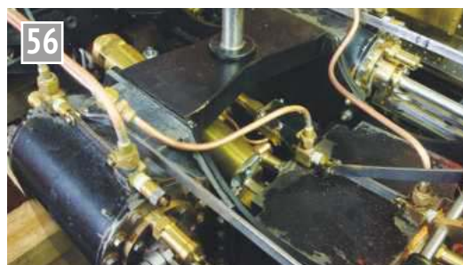
56 Underside of cylinders showing the drain cocks and operating linkage. The pistons are in the 'closed' position. The PTFE insert in the piston has an annular groove which, when in the 'open' position, lines up with the passage in the body.
