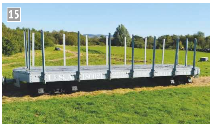
The contribution made by the other allied powers to narrow gauge WW1 rolling stock development has not been overlooked by the MRT and one of the items in the collection is this U.S. bogie 'Pershing' flat wagon dating from November 1917.
