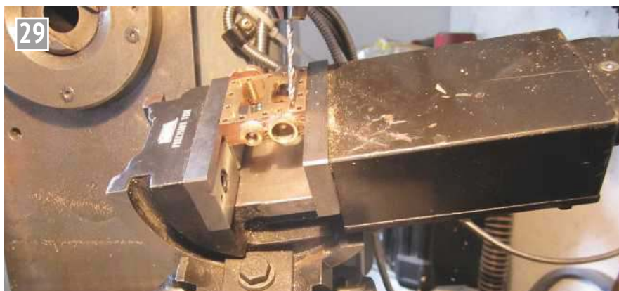
Drilling through into the shuttle hole.
