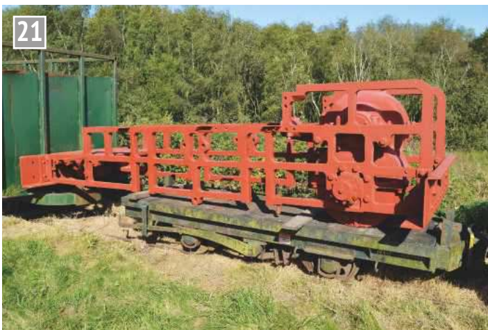
21 A challenging restoration project for the MRT team is a Baldwin 50 HP 7 1/2 ton 4-50-1-C tractor locomotive imported from Switzerland in the spring of 2016 as a standard gauge Diesel conversion. The stripped-down mainframe, carrying the gearbox, was on display as a wagon load at the gala, but much work is still required, not least in sourcing and fitting a suitable engine unit.
