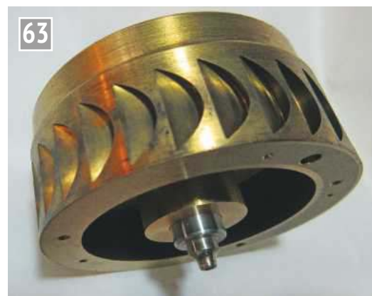
Rotor from the Sperry artificial horizon shown in photo 62. (The rotor diameter is 2.065 inches.)
