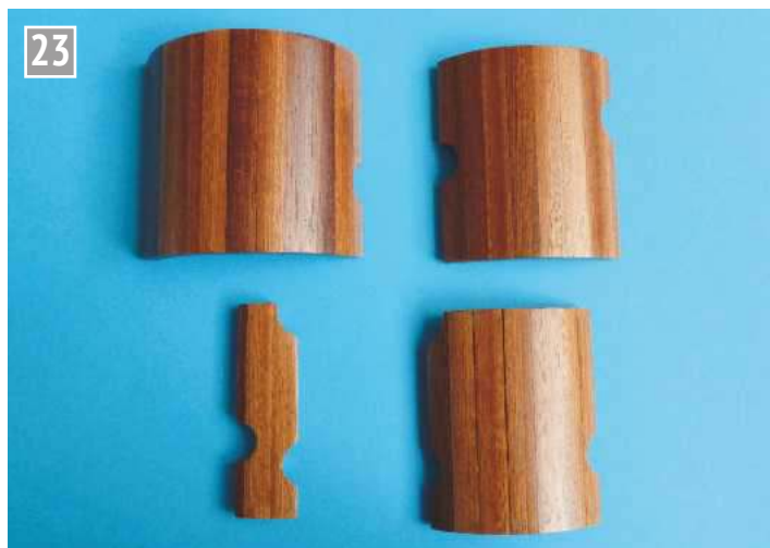
Boiler lagging – in four pieces.
