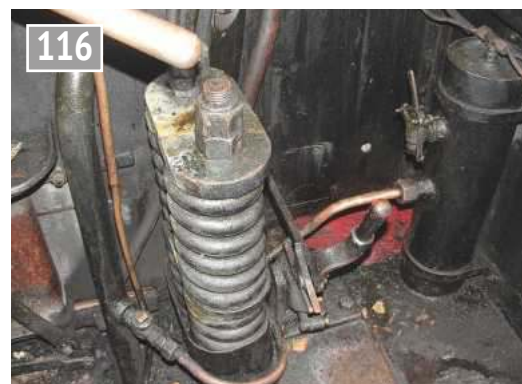
Better view of the drain cock lever.
