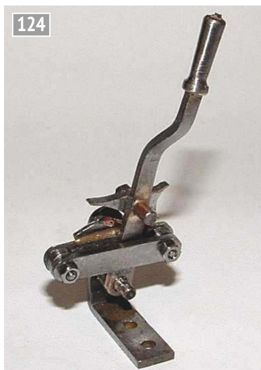
The complete operating lever.
