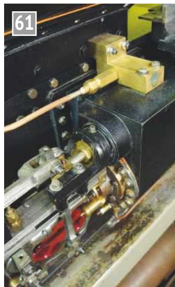
Live steam connection from saddle to outside cylinder showing also oil feed and check valve.
