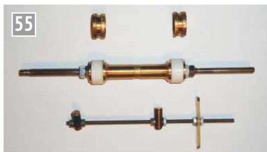
55 Piston valve bobbin, after lengthening to match the near side cylinder ports, with PTFE 'rings' which control steam entry and exit. The original rings can be seen in the background. The jig that I used to determine the actual port positions is in the foreground.
