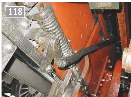
The linkage is taken up to platform level.
