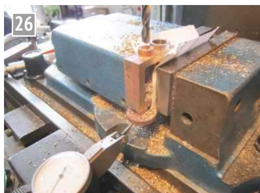
Drilling and tapping into the valve chest.
