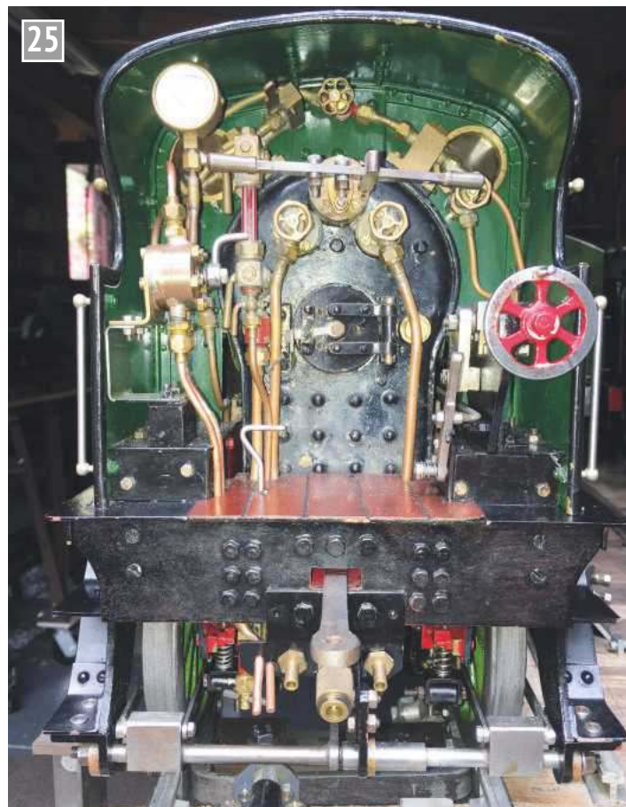
25 Backhead and cab controls are rather let down by the steam brake valve.
