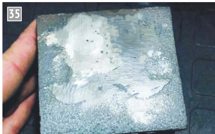
Welded casting defect.
