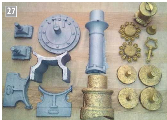
Some aluminium and brass castings showing the detail from 3D printing.
