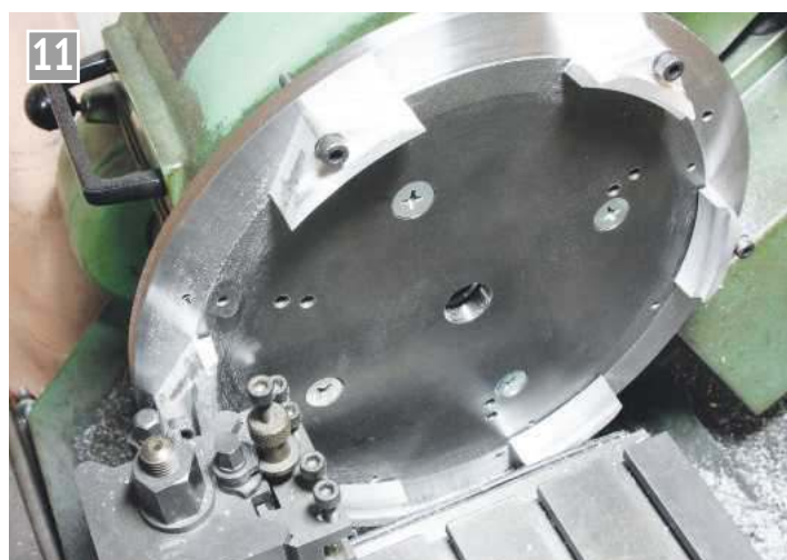
Cutting the driver brake block profile.
