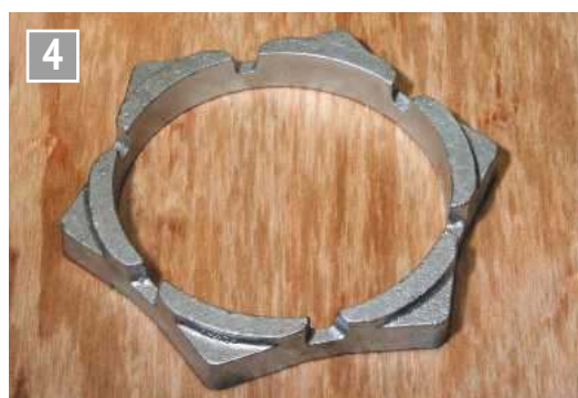
Brake block castings for the bogie wheels.
