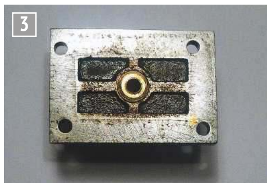
The valve chest cover. Notice the brass plug, bottom right.
