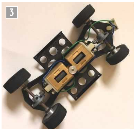
Russkit 'black widow' 1/24 metal slotcar pan-chassis with two motors.
