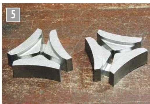
Brake block castings for the driving wheels.
