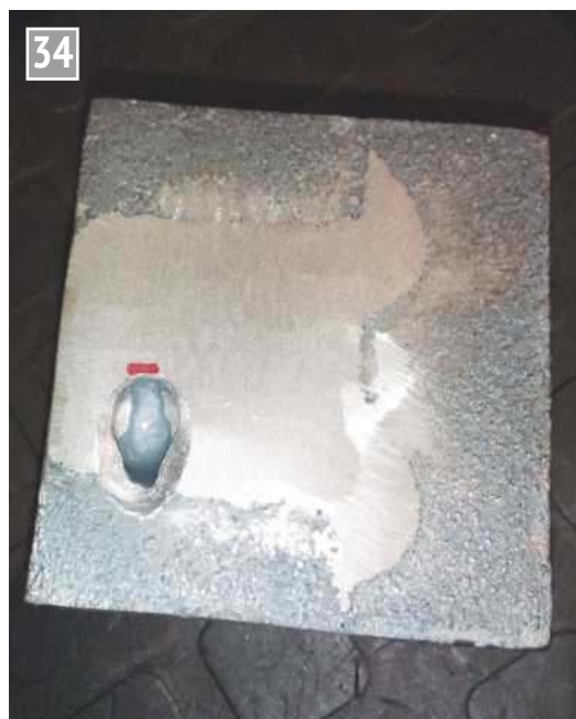
Casting defect to weld.
