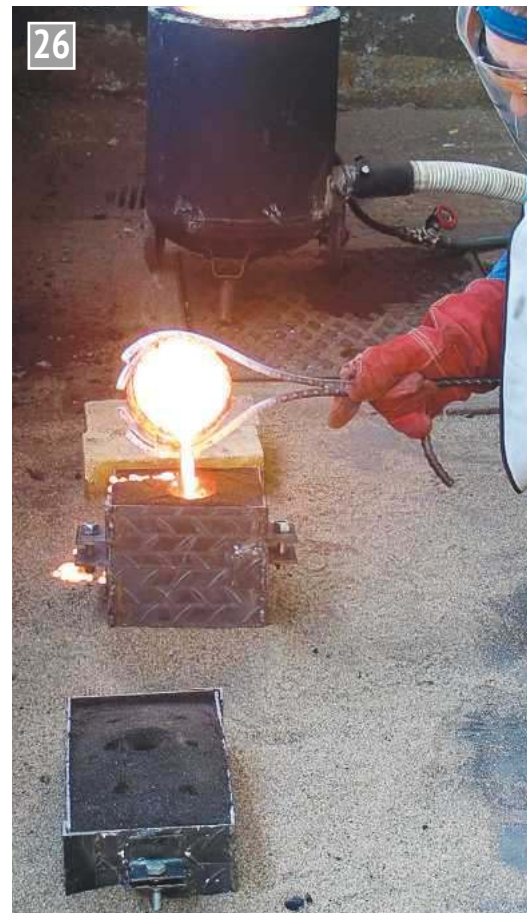
Pouring steadily and safely to the side.
