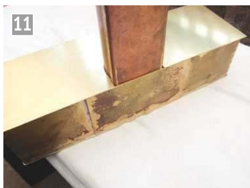
The top plate with an opening made to fit around the filler pipe and ready to be silver soldered in place in due course; note the overhang for the soldering operation.
