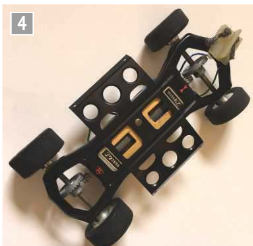
Russkit 1/24 'black widow' slotcar chassis underside.
