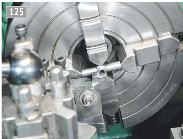
Turning the crosshead boss.
