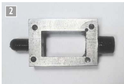
The valve chest, complete with poorly drilled holes.
