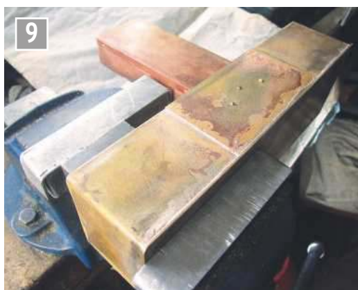
Two views of the tank so far with the lower joint trimmed back to allow the assembly to fit the bunker. The fabrication is held in the vice with a steel block to remove the outer edges of the bottom plate.
