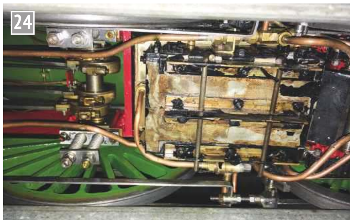
24 View of the ashpan from below showing drop down doors. This view also shows, partly hidden by the brake rigging, the blowdown valve bracketed off the side of the ashpan and fed by an external pipe from the lowest point of the foundation ring.
