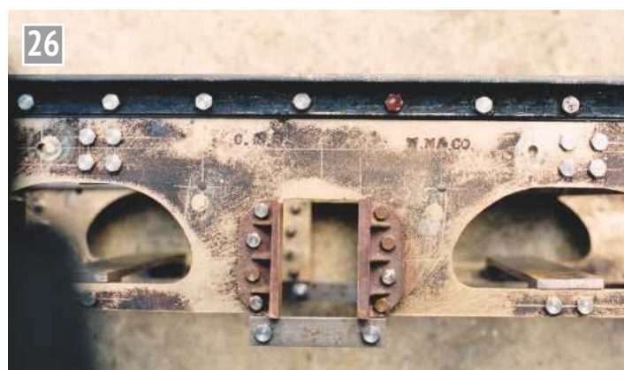
26 Cast tender frame. Original holes have been plugged and silver soldered. Open holes are for the spring hangers and the brake rigging. New hornblocks are fitted with bolts in close tolerance holes. The angle on the near side is bolted through the casting to a steel sub-frame.
