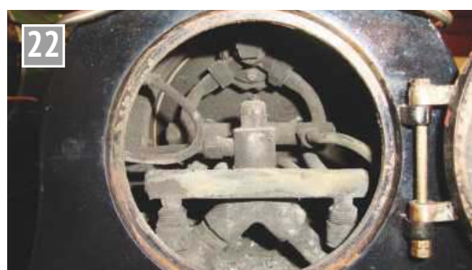
22 Inside the smokebox. Access for sweeping the flues from the front is very limited. The multi-jet blower is integral with the blast pipe and fed from the pipe on the left. Steam is delivered to this through the handrail on the offside of the boiler. The pipe on the right is to the snifting valve. This is tucked away behind the frames just in front of the tubeplate which is set back from the rear of the smokebox wrapper.
