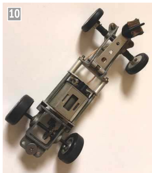
Tamiya 1/24 slotcar chassis underside.
