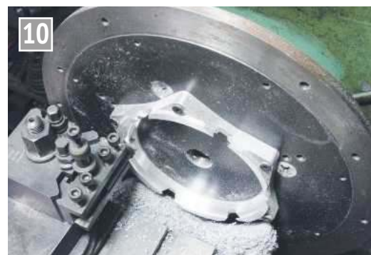
Cutting the bogie brake block profile.
