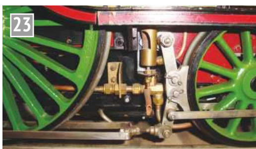
23 Nearside injector with delivery pipe bracketed off the ashpan. Above the injector is the bottom end of the whistle which extends up into the dummy sandbox. The dump pin for the drop down doors of the ashpan can be seen below the injector support bracket. As in all of my engines, except No. 8783, the whole ashpan cannot be dumped.
