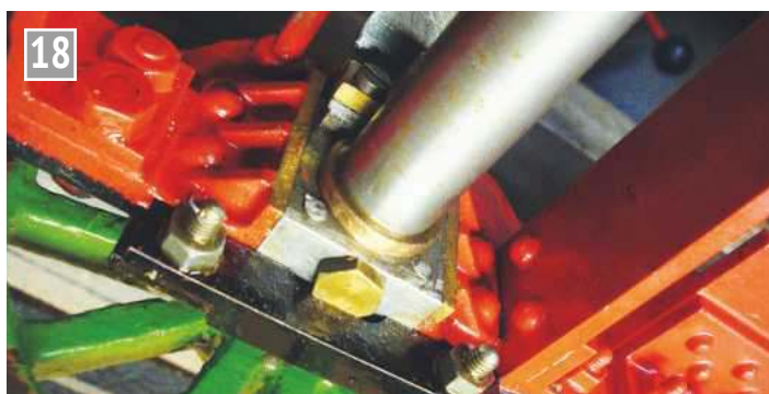
18 Bogie wheel set from below. The bronze bearing surface in the steel axle box is evident. The original plan was to have a spring loaded felt pad to direct oil to the underside of the journal. Lack of space and inaccessibility proved to be intractable so a simple plug was substituted. The horn stay had to be recessed to accommodate the plug.
