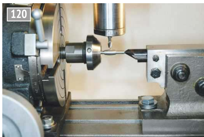
A normal collet chuck interferes.
