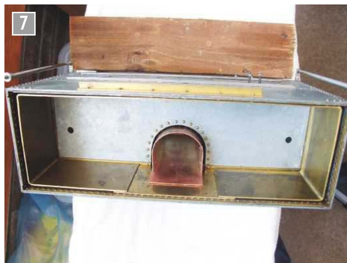
The tank sides and the water filler pipe have been fitted into the bunker space to check the clearances and mark out where the attachment should be made. There is some sideways movement for the tank - just centralise it but the filler pipe needs to be at right angles.
