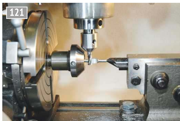
Milling the central panel.
