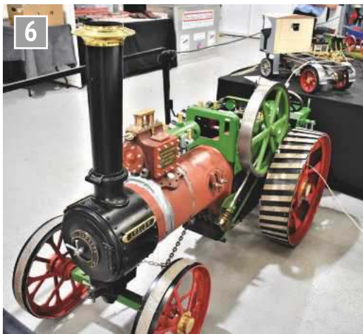
Richard Betts, a member of the Black Country Live Steamers, is building this 4 inch scale Garrett traction engine.
