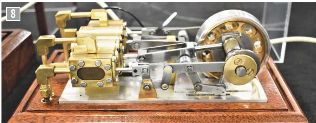
The Twin Cylinder Oscillating Engine in 1/8th scale built by Laurence Drybrough.
