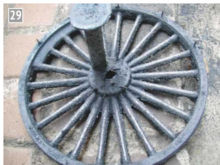
Largest casting - 4kg Stirling single wheel.
