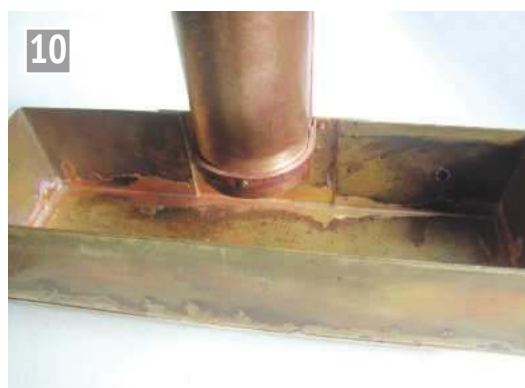
This view shows the supporting copper strip formed into a hoop and attached to the filler pipe casing and the rear side. It will provide a secure soldered joint for the tank top plate when it is fitted.
