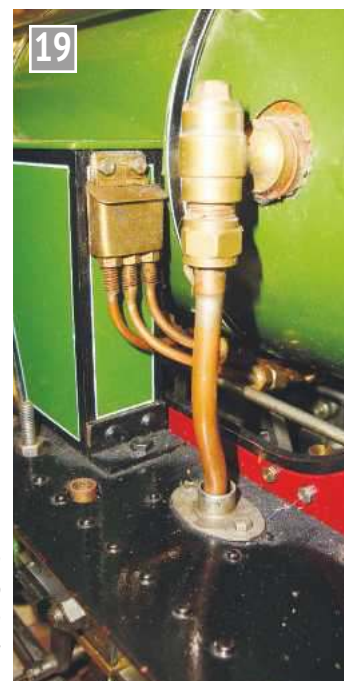
19 Oil boxes mounted on the forward sandbox for driving axle journal and horn guides, and two eccentrics. Two further oil boxes can also be seen, one for the upper slide bar, and one for the bogie rear wheel journal and horn guides. Between the frames can be seen some of the more accessible parts of the Stephenson's valve gear. Some of these are very difficult of access for the oil feeder.
