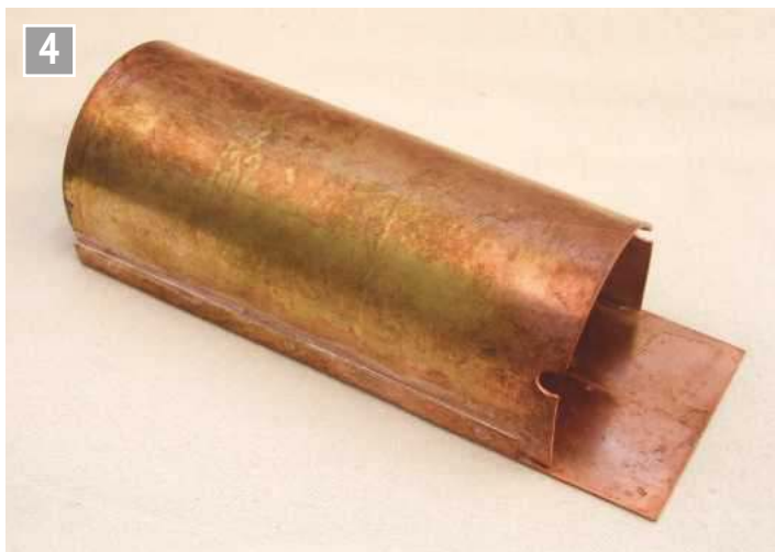
This shows the completed water filler casing - note the \frac{3}{16} inch slots added at the base to act as a location for the two return water pipes from the crosshead pumps.
