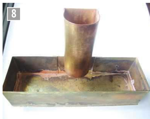
Two views of the tank so far with the lower joint trimmed back to allow the assembly to fit the bunker. The fabrication is held in the vice with a steel block to remove the outer edges of the bottom plate.
