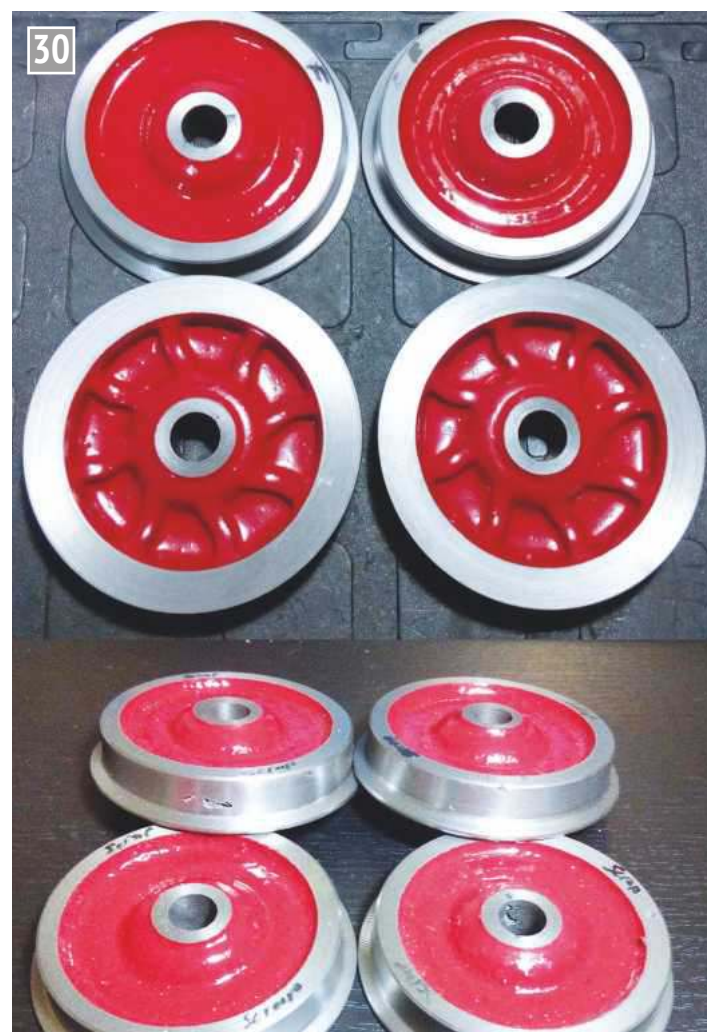
Proper risering and no risers causing draw holes.
