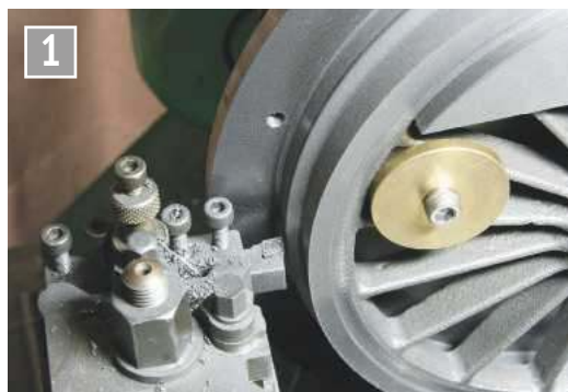
1 Cutting the flange.
