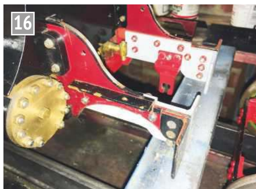
16 Modifications in progress to the front end framing in order to accommodate more side play for the bogie wheels. The bracket against which the side control spring bears is prominent.
