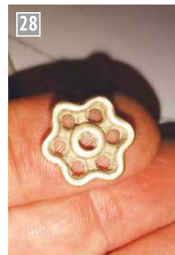
Smallest casting - a 2g steam valve handle.
