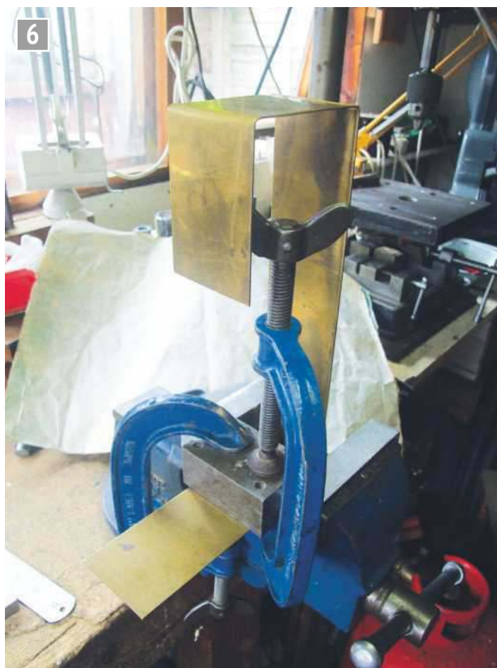
Two views showing the way the side strip for the bunker tank body was clamped against a steel block in the vice to form the right angled bends. A folder would have made life easier but I do not have room for one!
