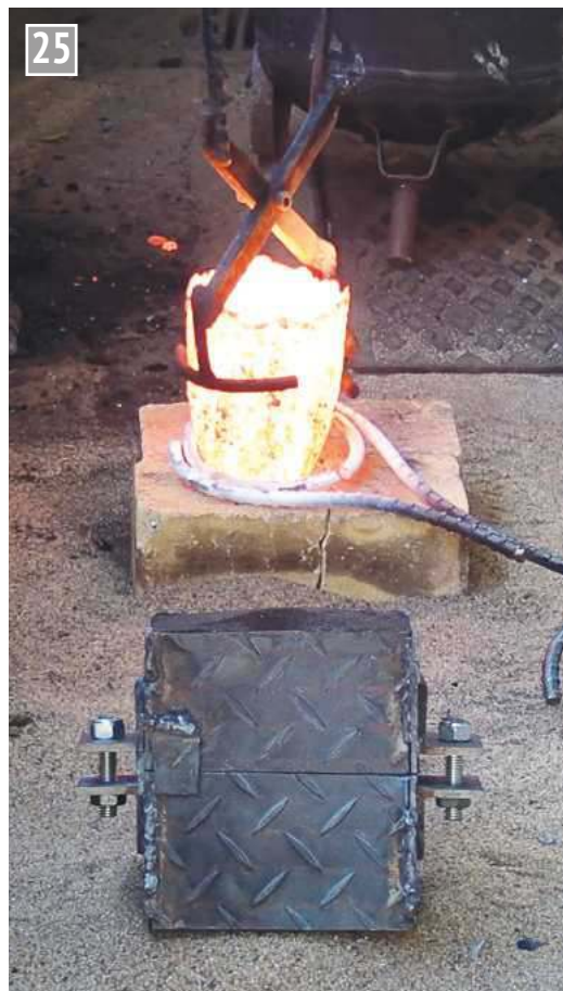
Placing the crucible in the pouring ring.
