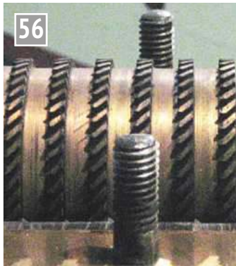
56 Blades of Parson's first turbine, made in 1884 and now in the London Science Museum (image from Science and Society Picture Library).
