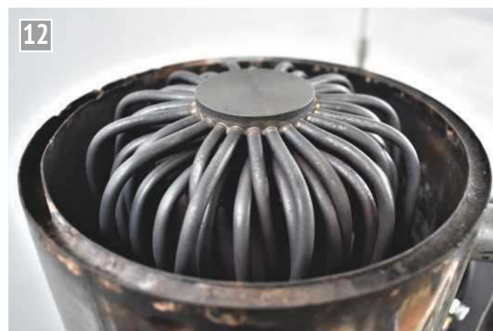
The heater tubes on the four lever Stirling engine.
