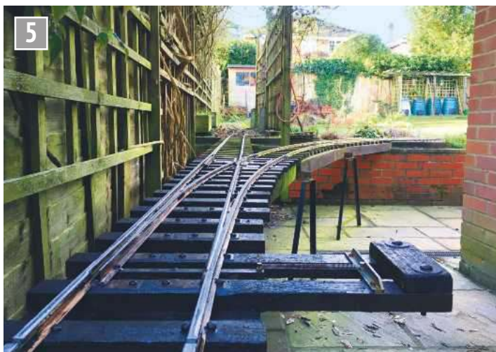
Point at the entrance to the 'balloon' loop, showing the spring control.
