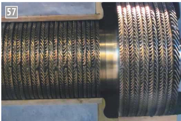
57 Blades in turbine No. 261 made in 1889 by Clarke, Chapman, Parsons & Co. It was originally installed in HMS Gleaner and is now in the National Museum of Scotland, Edinburgh (photograph is included by kind permission of the museum).
