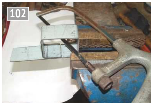
Trimming the tank.
