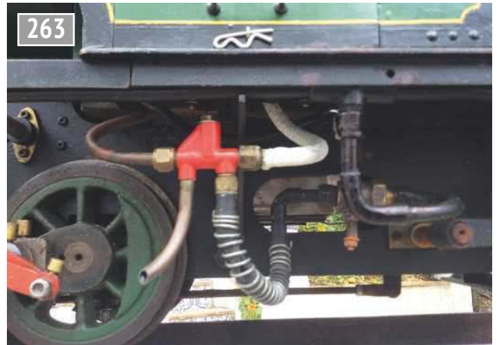
Close-up of fireman's injector water feed.
