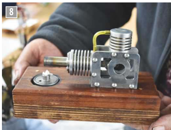
David Laycock used a traditional engraving machine to machine the side plates for his engine.
