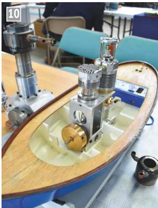
Tony Goodger is constructing this free piston engine for his model boat.
