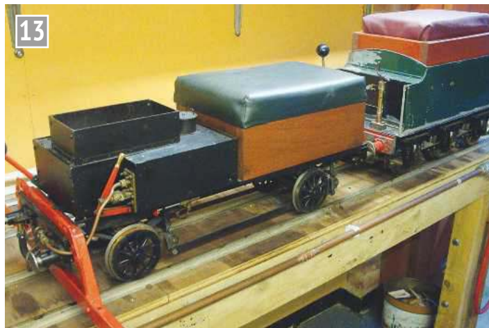
The Y4 driving truck in front with water tank (hand pump feed only) and coal bunker. The driving truck behind was built for the Stirling Single but can be used with all of the tender locomotives. It has no water or coal capacity.
