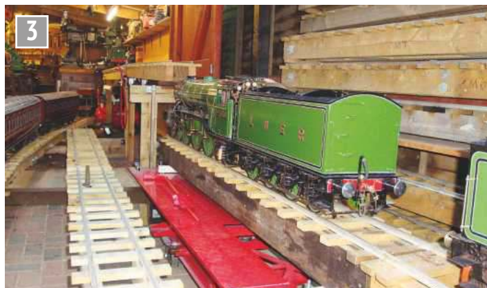
The lifting table at main line level.
