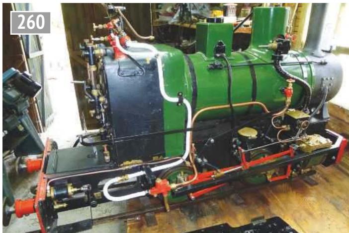
Driver's injector pipework.
