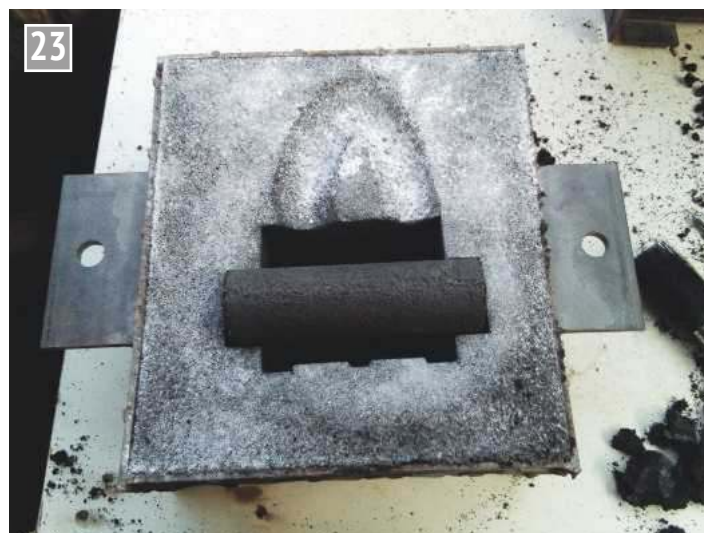
Cylinder – bottom box with cores fitted and ingates cut in sand.
