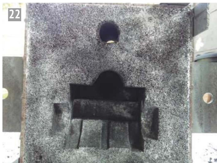
Cylinder – top box with riser and pattern removed.
