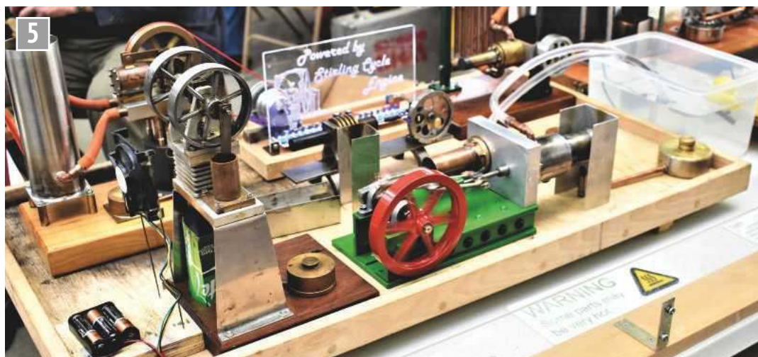
Bob Cannon provided this example of Gamma and Henrici hot air engines.
