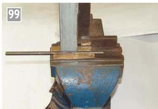
Wrapping up the tank for the lubricator.
