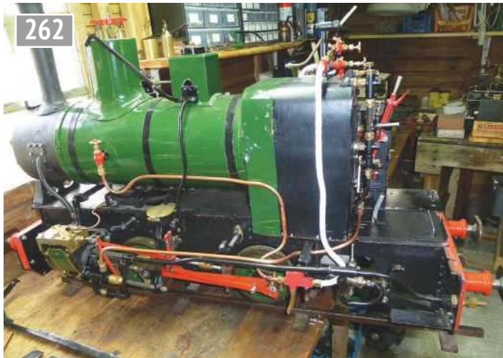
Fireman's injector pipework.
