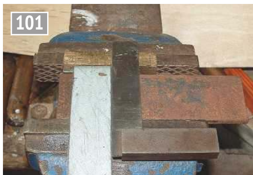
Checking the tank is square.
