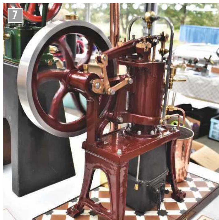
A well made example of the popular Ryder-Ericsson Hot Air Engine built by Andy Badman.
