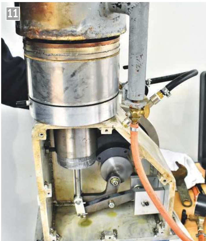
Norris Bomford built this four lever Stirling engine for use in a small boat.
