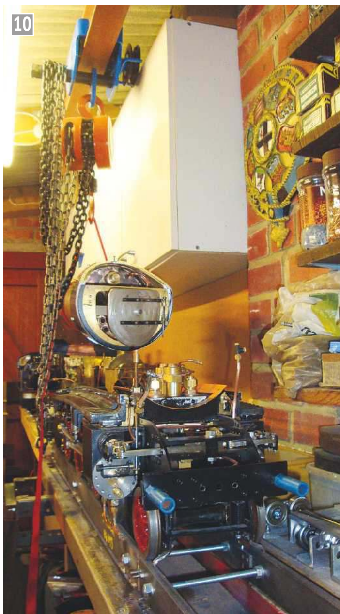
Chain block in use during assembly of the A4.
