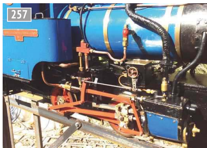
Driver's injector on ACC No.1.
