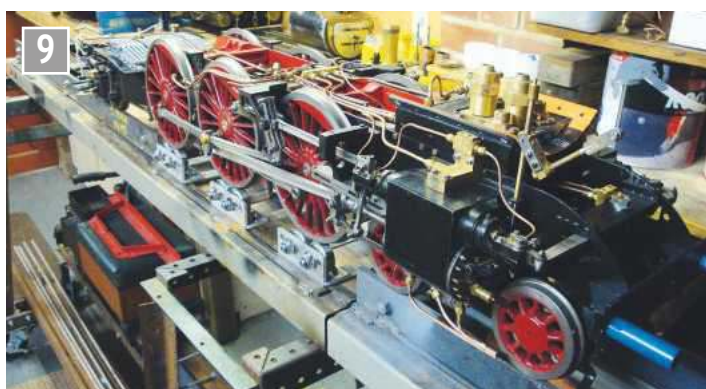
Mobile bench with rolling road installed and A4 being set up for valve setting.
