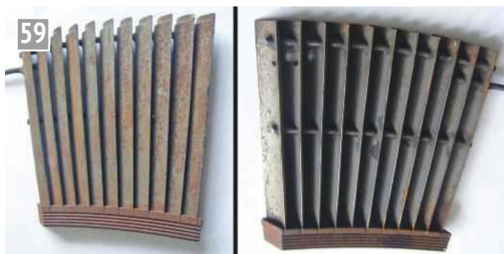
59 Section of Parsons rotor blading photographed from both faces. This was constructed by brazing together blades and spacers cut from drawn strips. The wires that can be seen passing through the blades are lacing wires and were brazed to each blade to improve stability. Note the thinned tips to reduce effects of any rubbing that may occur against the cylinder.
