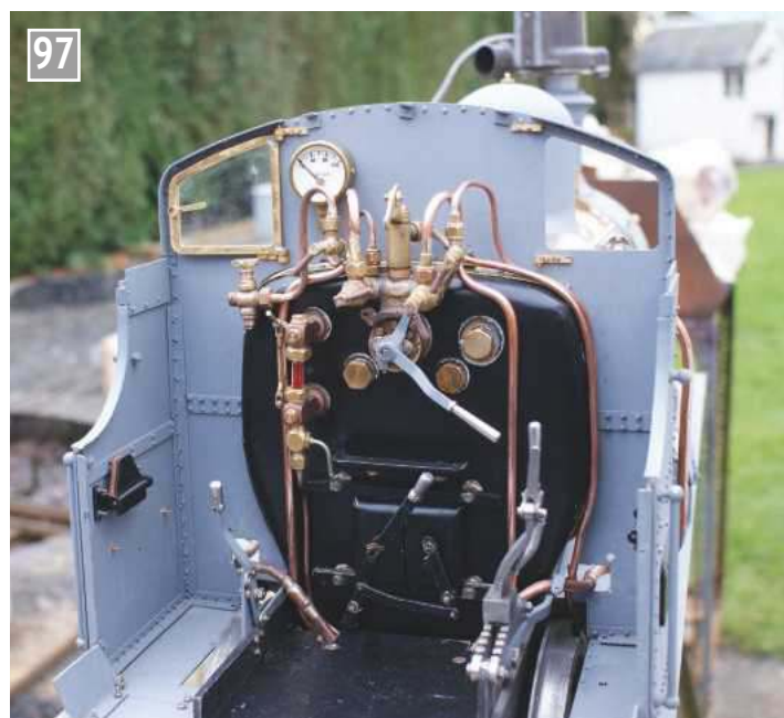
The location of the reverser in the cab.
