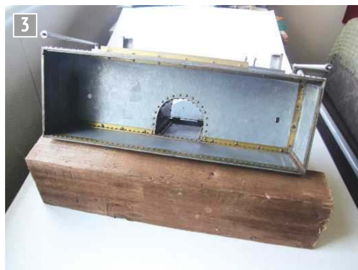
Two views of the locomotive bunker showing the water entry casing, which passes through the coal space, and the bunker tank space itself underneath. Note how the construction of this assembly left the rivets protruding and so the sizing of the water tank parts has to be carefully determined.
