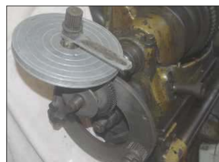
Terry Cleife's Lathe Dividing Attachment.
