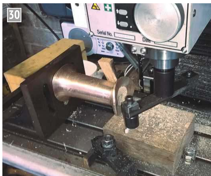
Fly cutting the base of the chimney.
