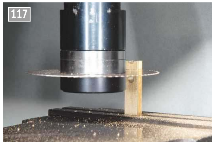
117 Separating the parallel bearings.
