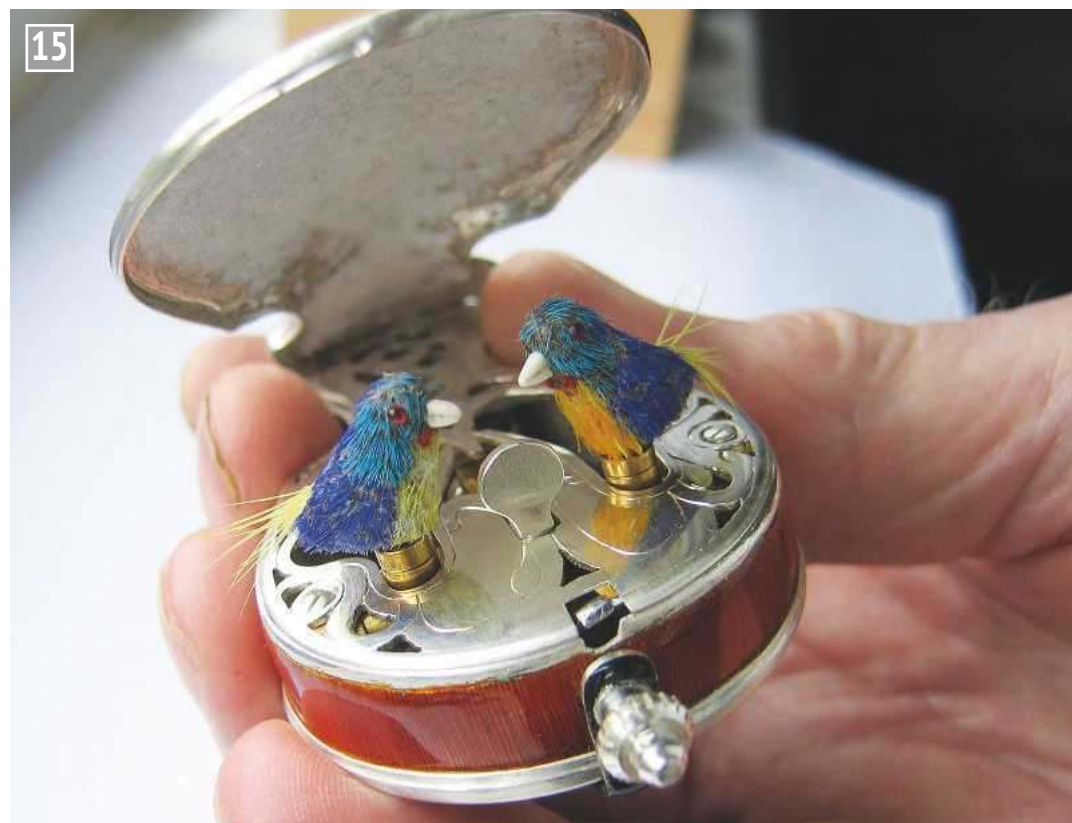
The open position showing silver operating button and the engraved and pierced silver grille.
