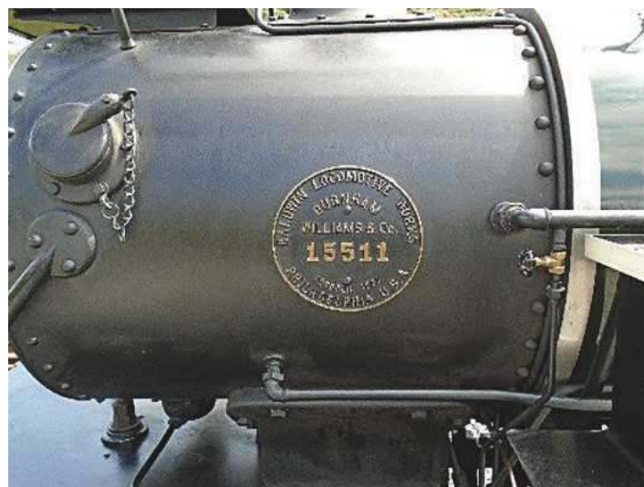
The left-hand side of No. 1's smokebox showing, lower left, the steam pipe to the char removal device. On each side of the smokebox are bars linking it to the front footplate. Above the three rivets attaching the top end of the left-hand bar to the smokebox can be seen the access hatch for inserting a paddle to move char into the removal device.
