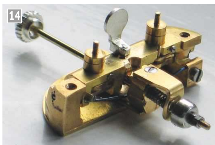
The carriage assembly on the sub-base plate, in the open position.
