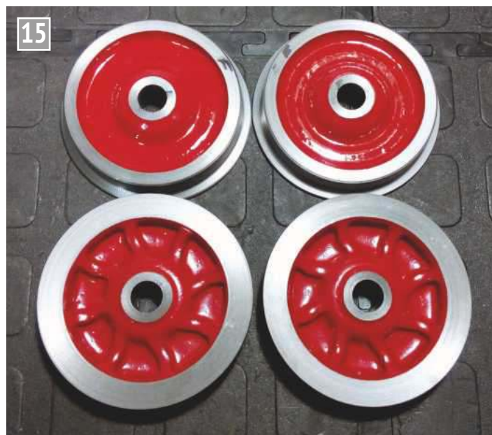
Wheels properly risered with no defects.
