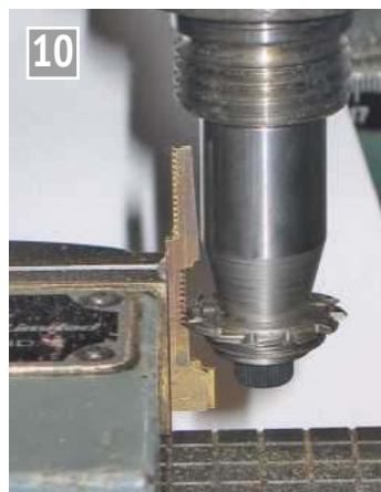
10 Milling the teeth on the second side of the rack.
