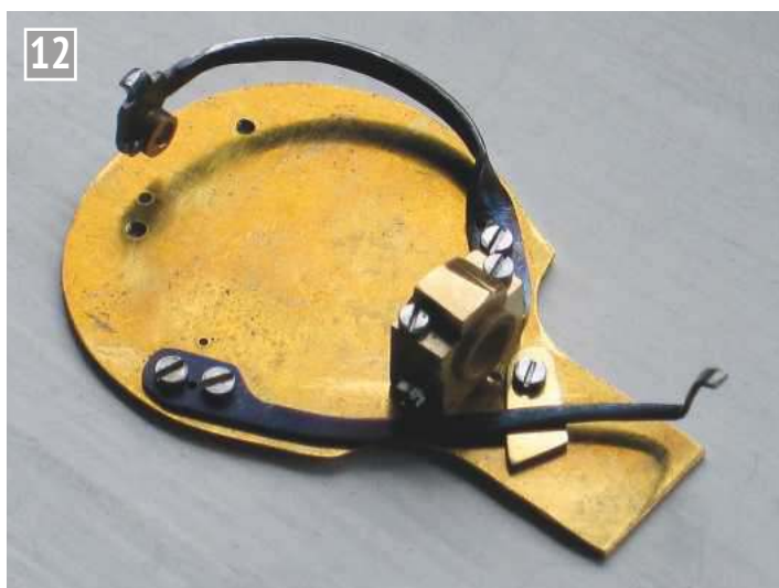
Main base plate with lock and fly springs screwed in position.
