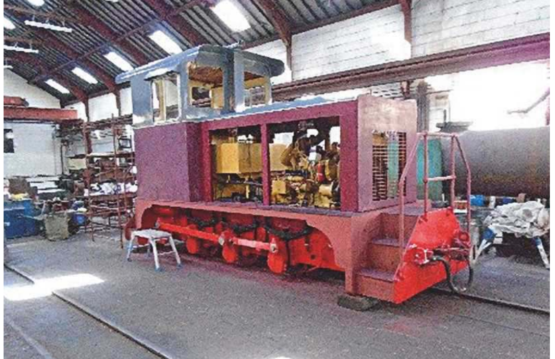
Diesel 001 which was built by the BMR in 1987 using parts obtained from the liquidation sale of Baguley, locomotive builders in Burton-on-Trent (these parts were for a locomotive order for Sena Sugar in Mozambique). This is a 140HP 0-6-0 Diesel hydraulic locomotive weighing 13T. The locomotive is fitted with a four cylinder turbo Caterpillar engine and a Twindisc single speed torque convertor. This locomotive is currently undergoing a general overhaul and re-paint.
