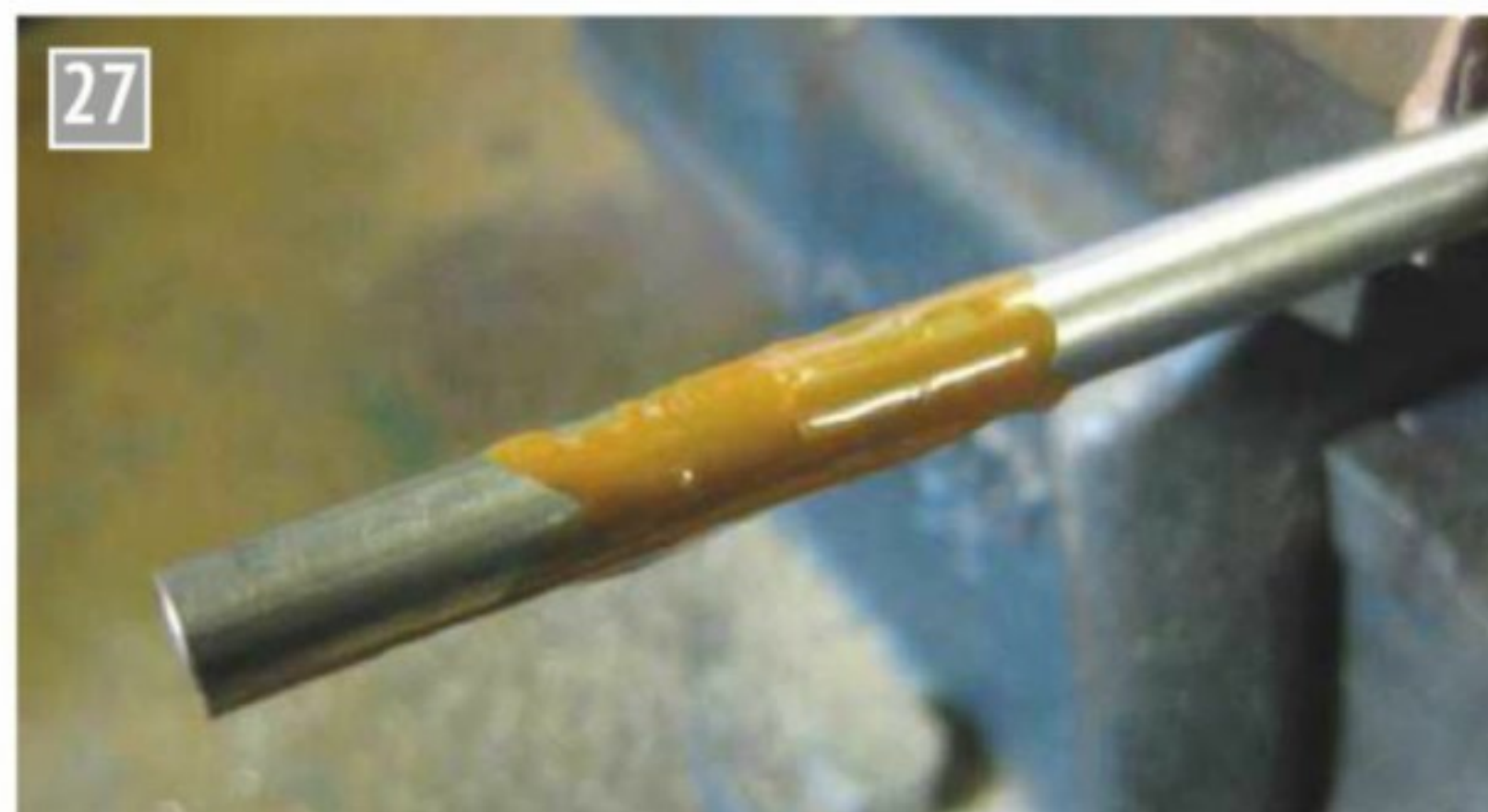
Steel rod mandrel with shellac applied.
