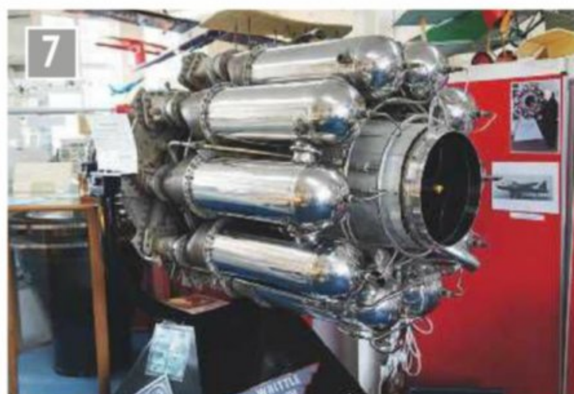
7 Frank Whittle designed this jet engine, the W2 model fitted to the Gloster Meteor in 1943.
