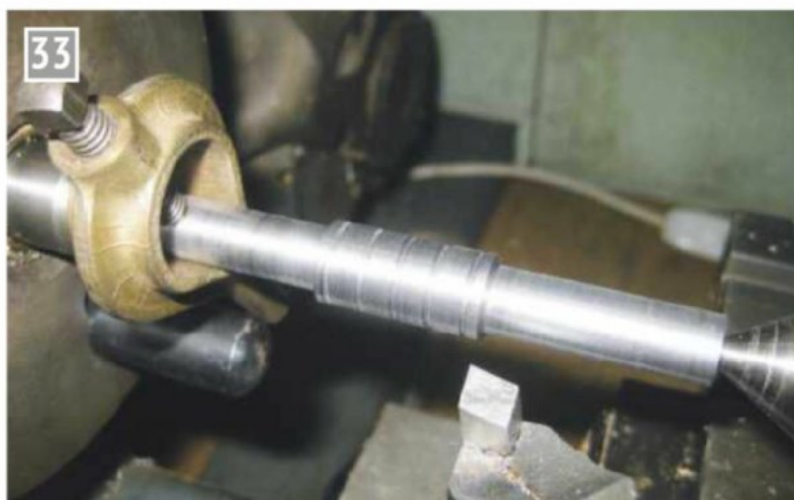
Machining the cylinder mandrel.
