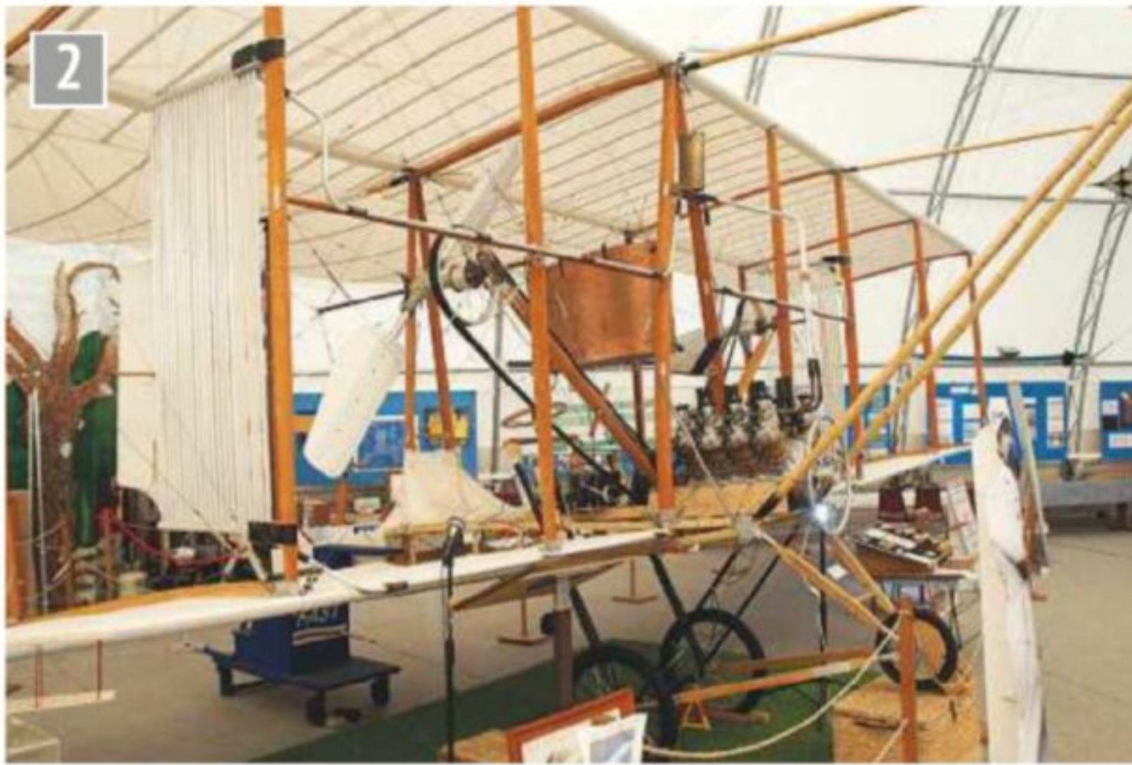
2 Replica of Cody's first aircraft, which had a French built 'Antoinette' engine. Materials included cambric, piano wire, bamboo and pinewood.
