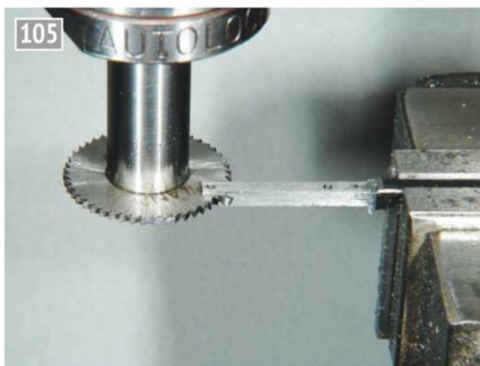
Machining the groove in one of the lower arms.
