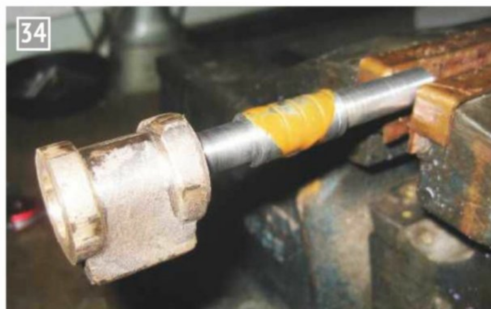
Melted shellac on the mandrel.
