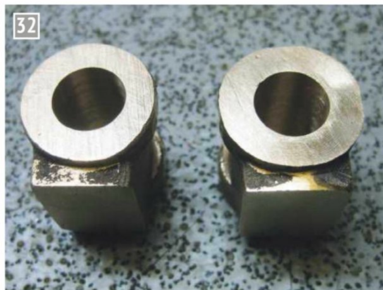
Cylinders with completed bores.
