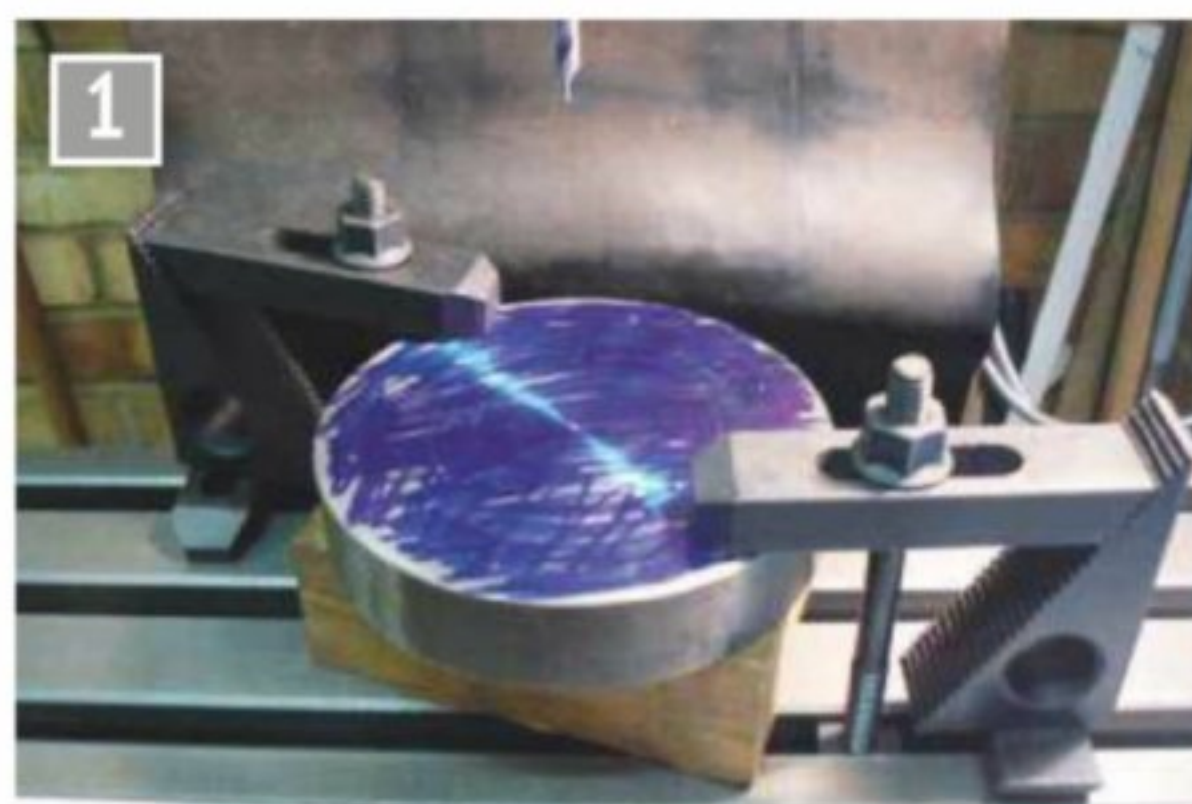
The blank on the mill prior to drilling.
