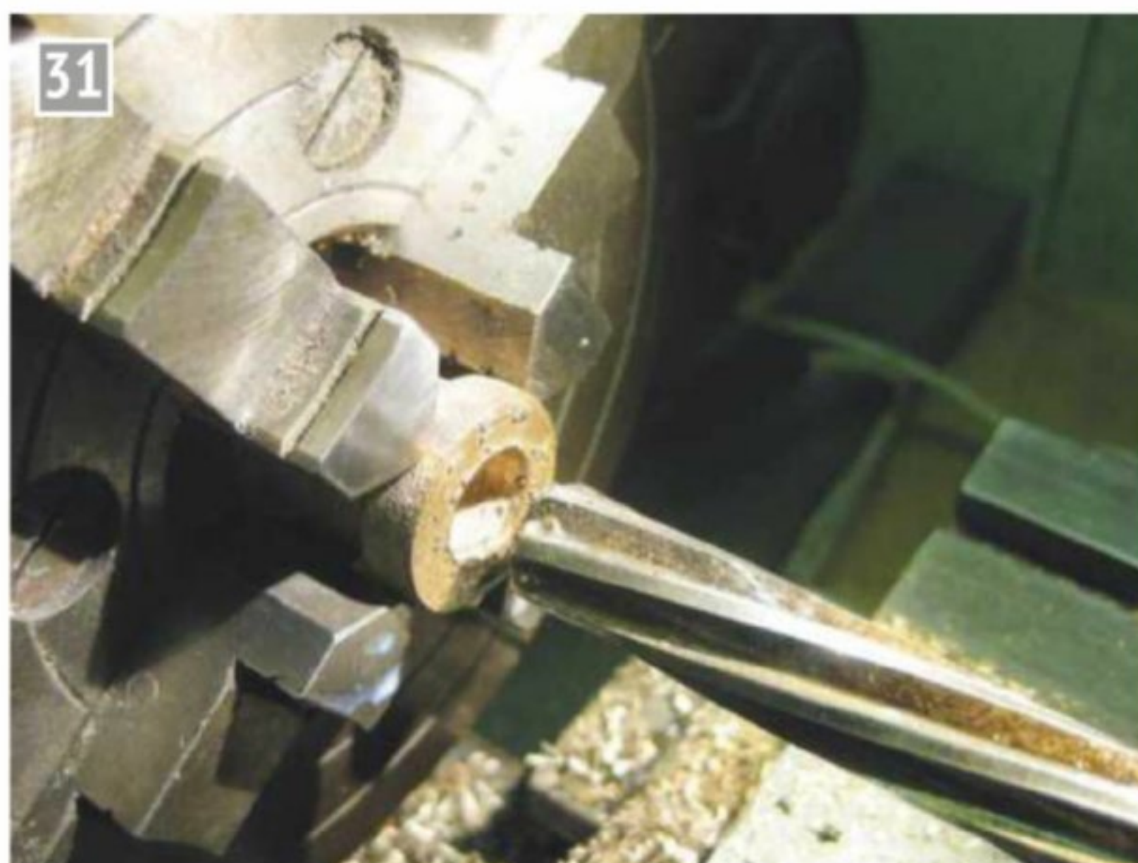
The cylinder is bored and reamed.
