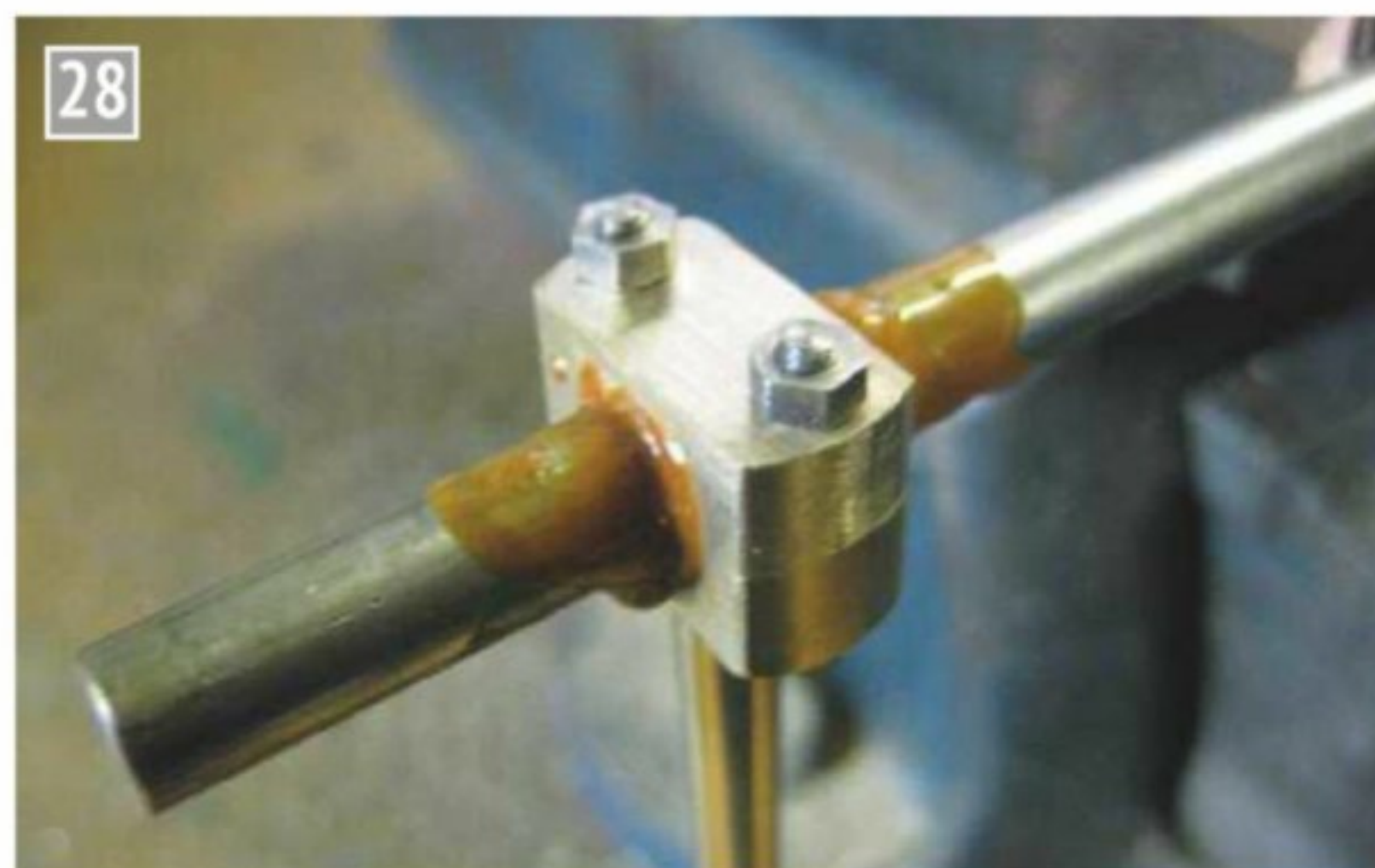
S50 connected rod mounted on the mandrel.
