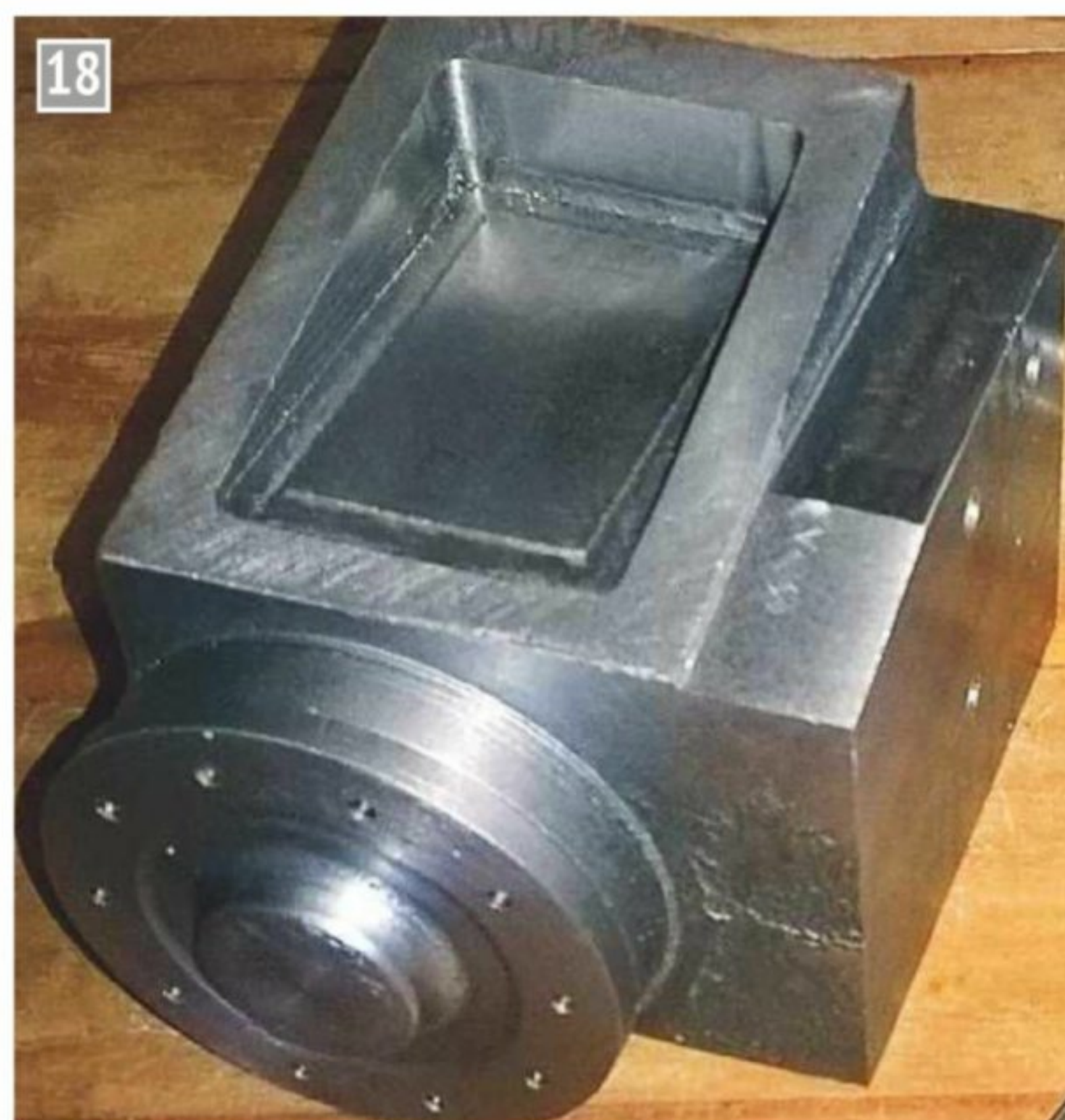
The port face before cutting the ports.
