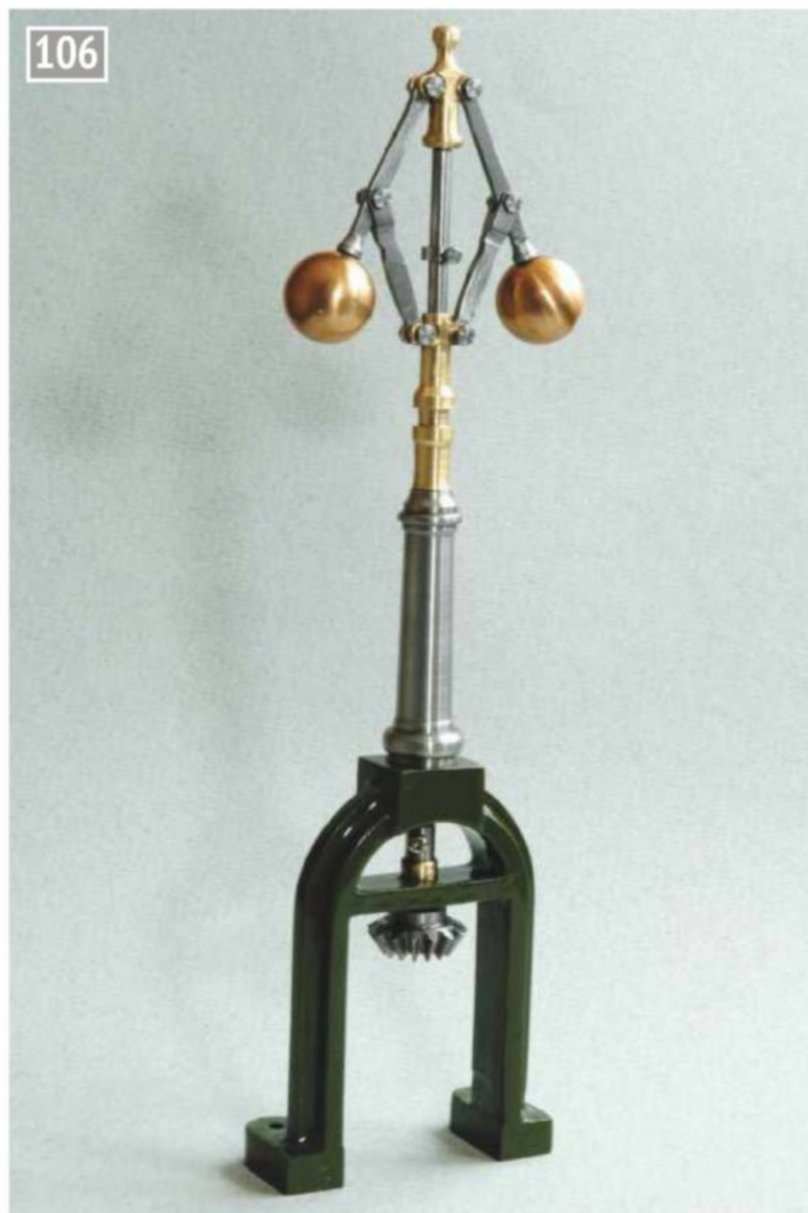
The arms and balls are fitted to the governor.
