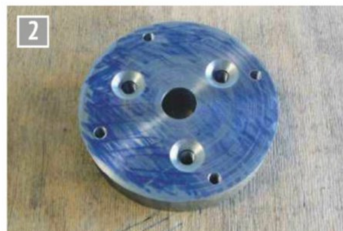
Completed drilling and tapping.
