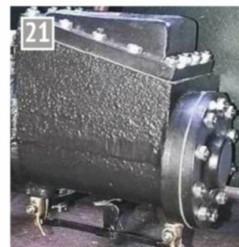
Drain cocks fitted.
