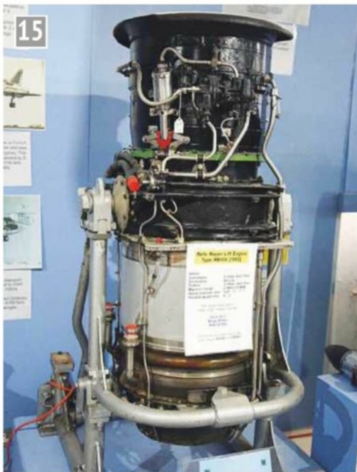
Rolls Royce test vertical takeoff and landing jet engine. The RB108 built in 1955. Work like this eventually led to the development of the Harrier jump jet. (Example outside the museum.)
