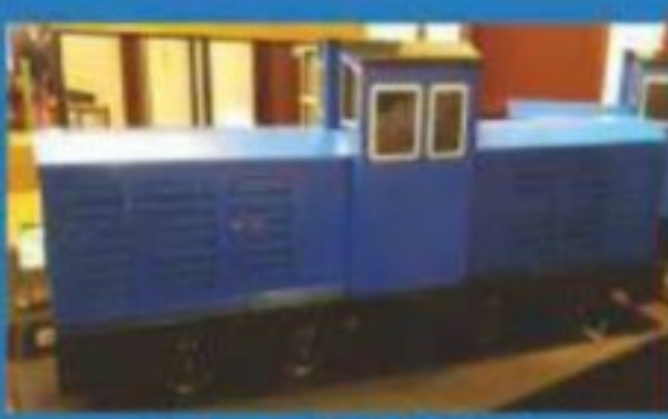
"Imp" £1650 4x motors 4x batteries 100A controller
