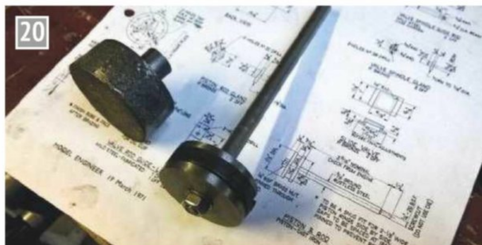
Piston, before and after machining.
