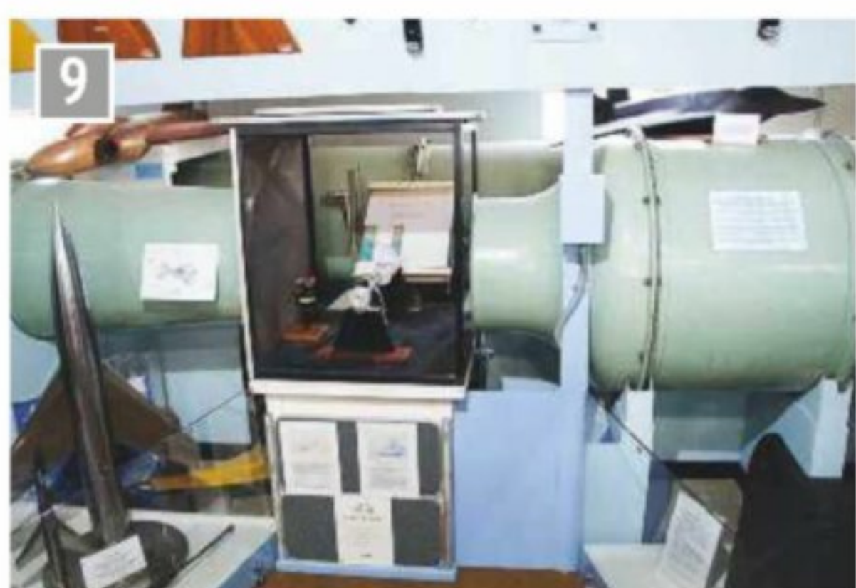
Open type wind tunnel brought in as part of war reparations from the University of Göttingen.
