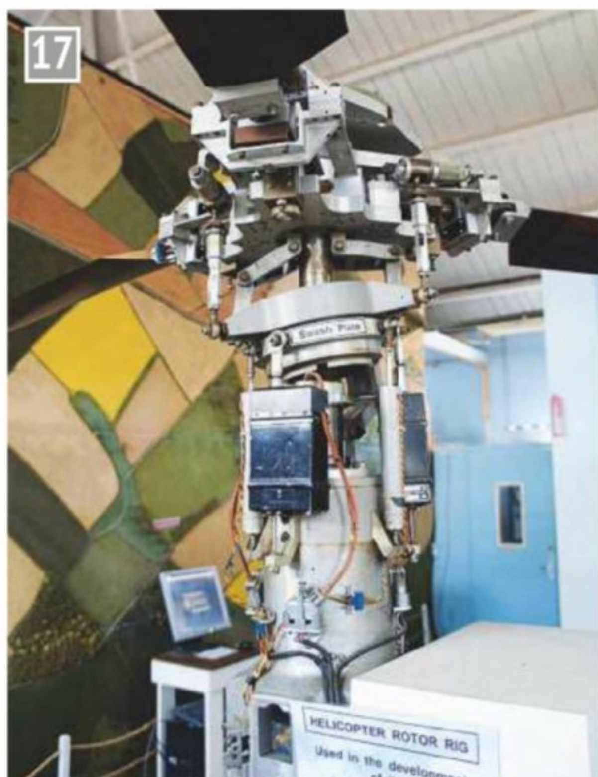
Swash plate mechanism used in research on helicopter rotor blades.
