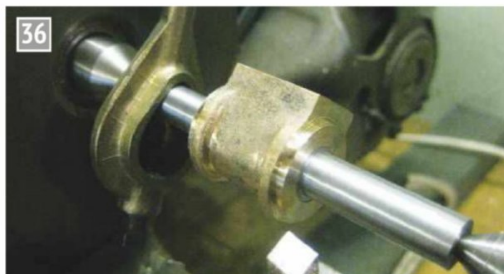
Machining the ends of the cylinder.
