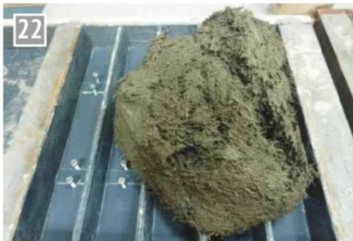
This shows the stiffness to aim for. It looks too stiff but actually flows into the mould easily. Some bleed water then rises to the surface before being reabsorbed during setting.
