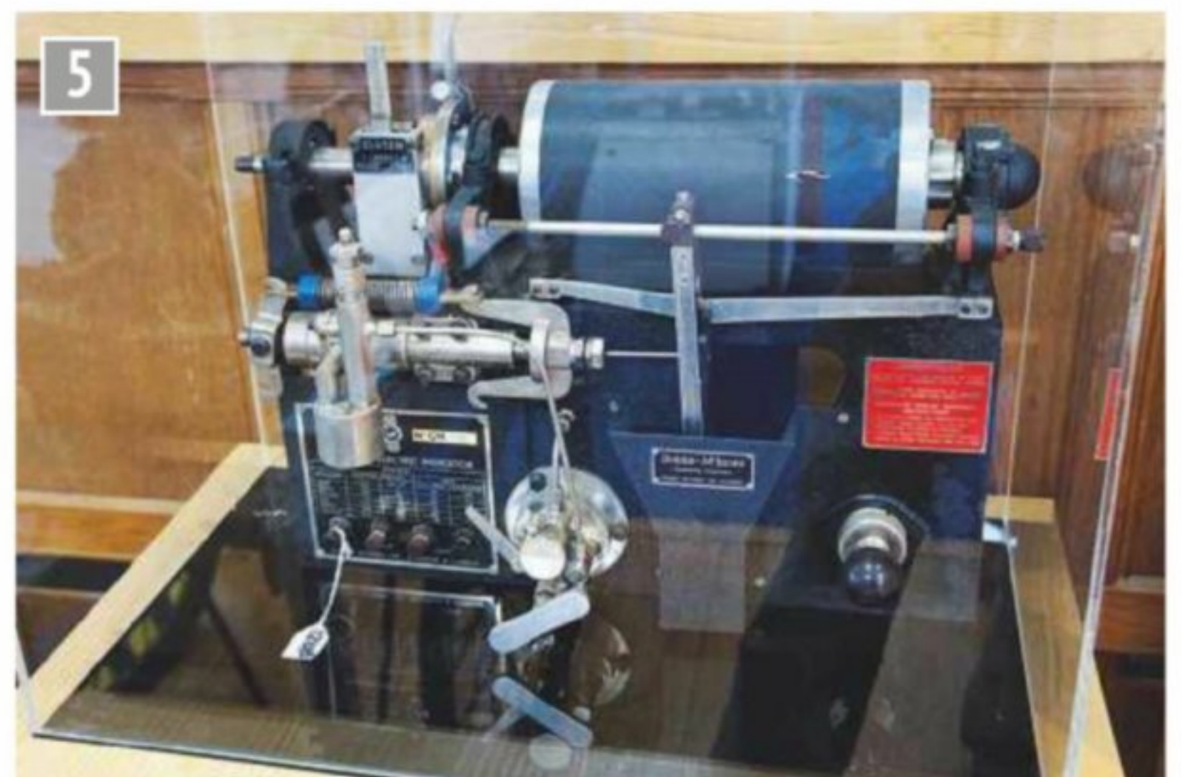
5 'Farnboro' indicator devised at the RAE and made by Dobbie and MacInnes of Glasgow.
