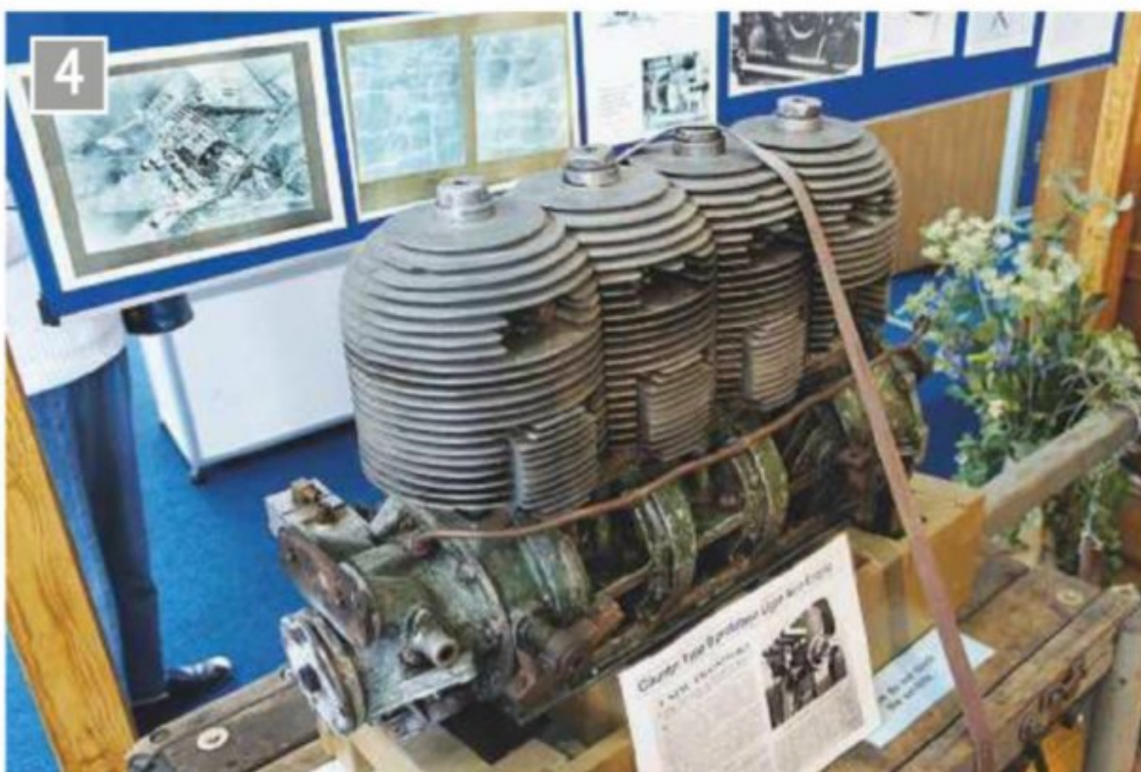
4 Caunter engine designed as a lightweight two stroke aero engine. Undergoing restoration.
