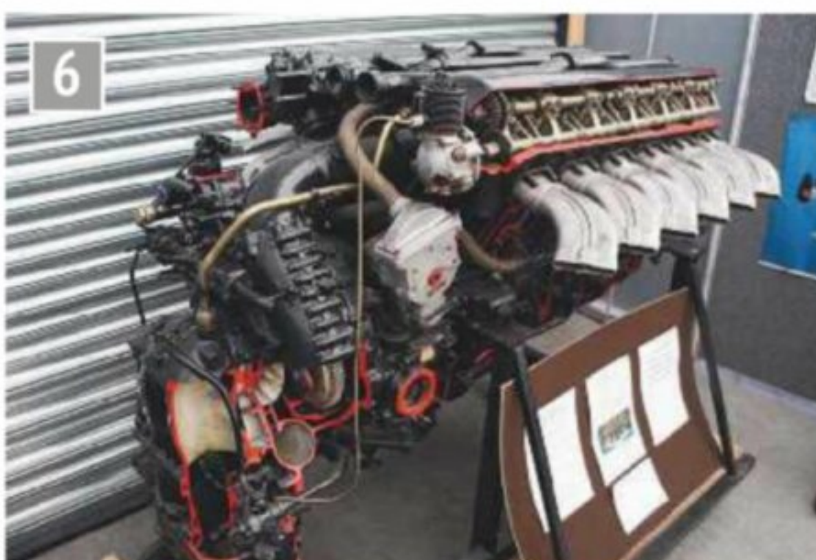
6 Rolls Royce Merlin engine as used in the Hurricane, Spitfire and Lancaster aircraft.
