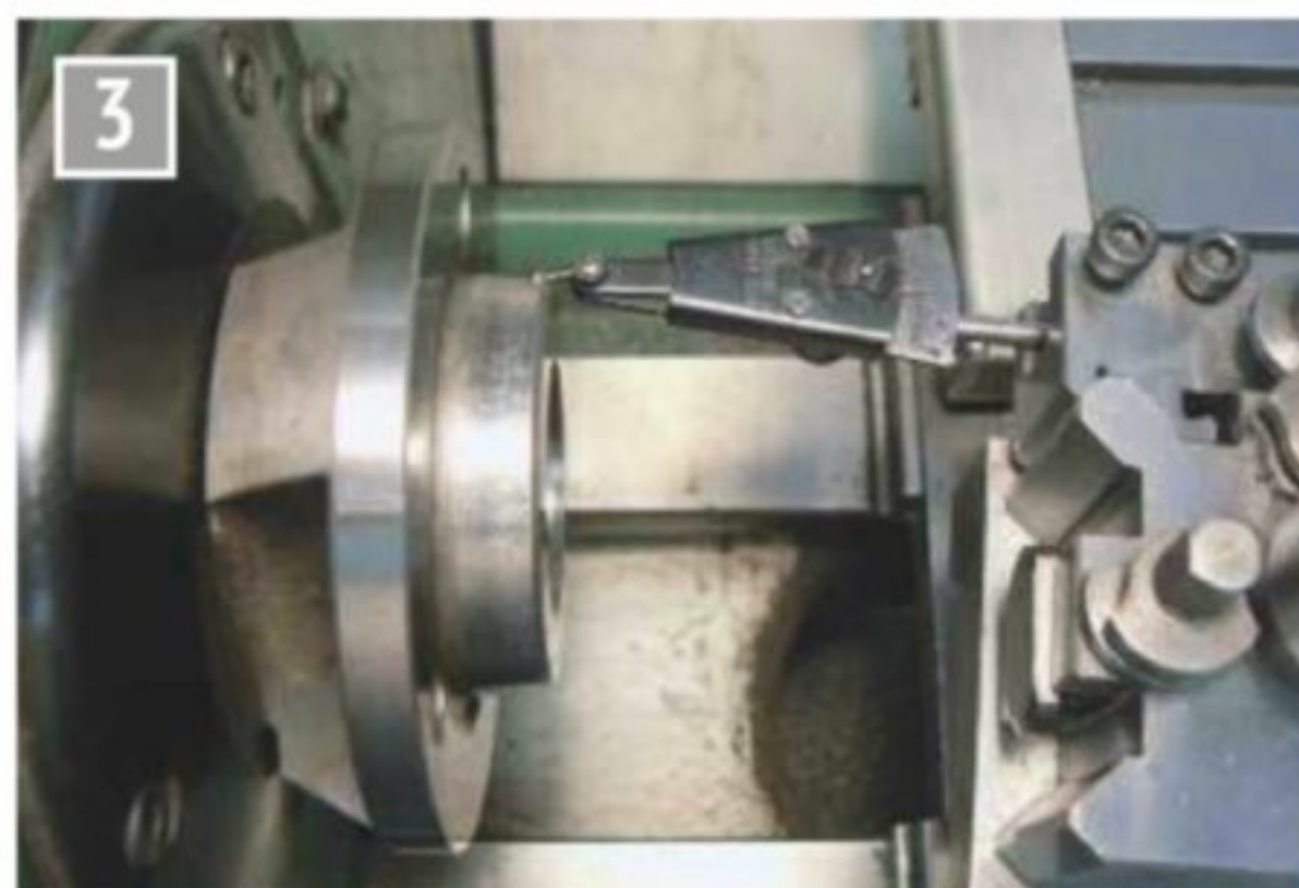
Setting the compound slide to the correct angle.
