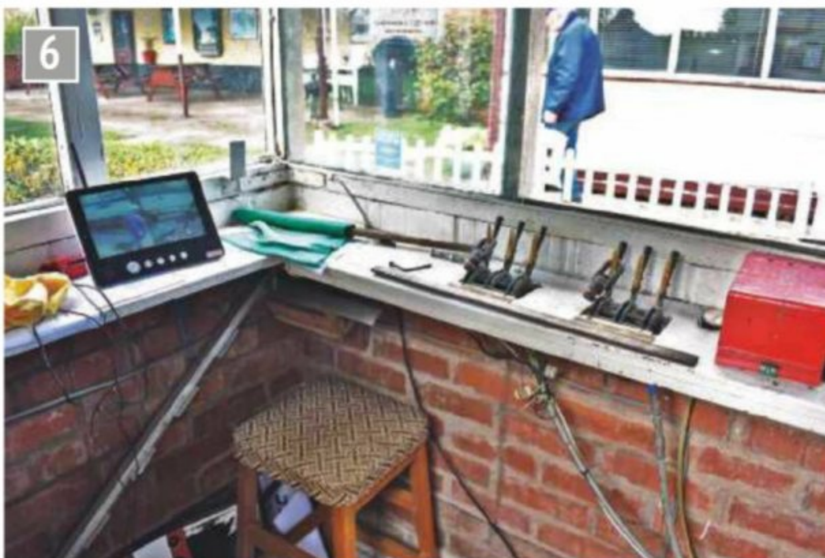
The small lever frame in the signal box.
