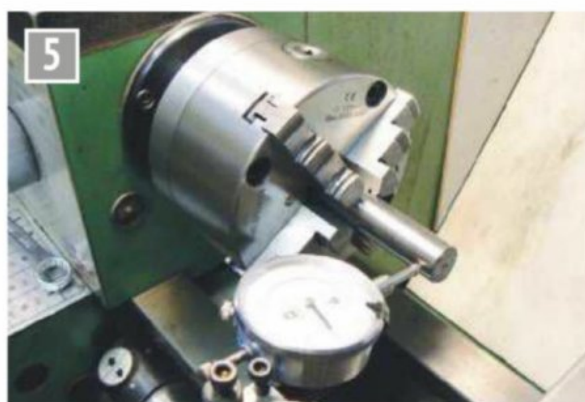
Testing the chuck assembly.
