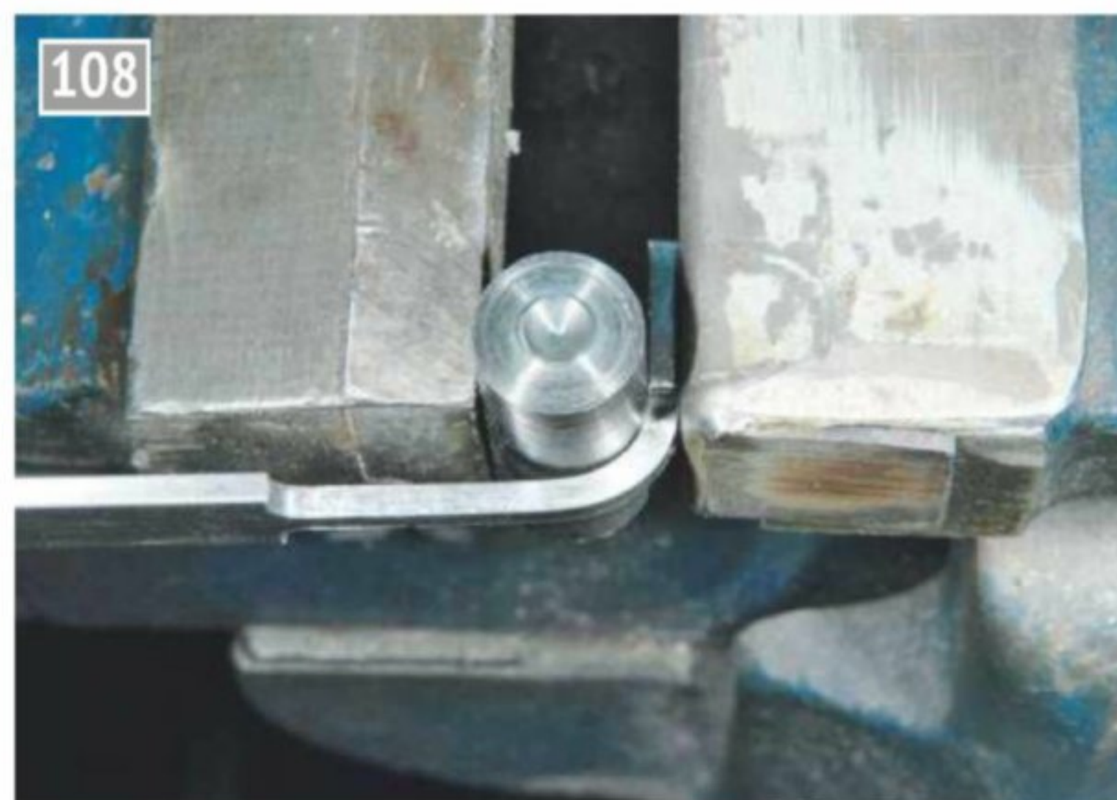
Putting the bend into the bracket.
