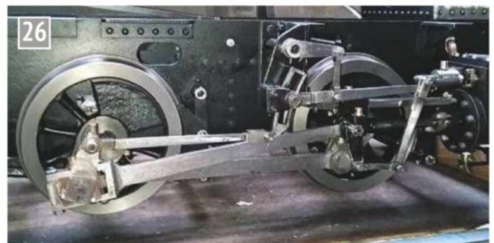
The complete valve gear.
