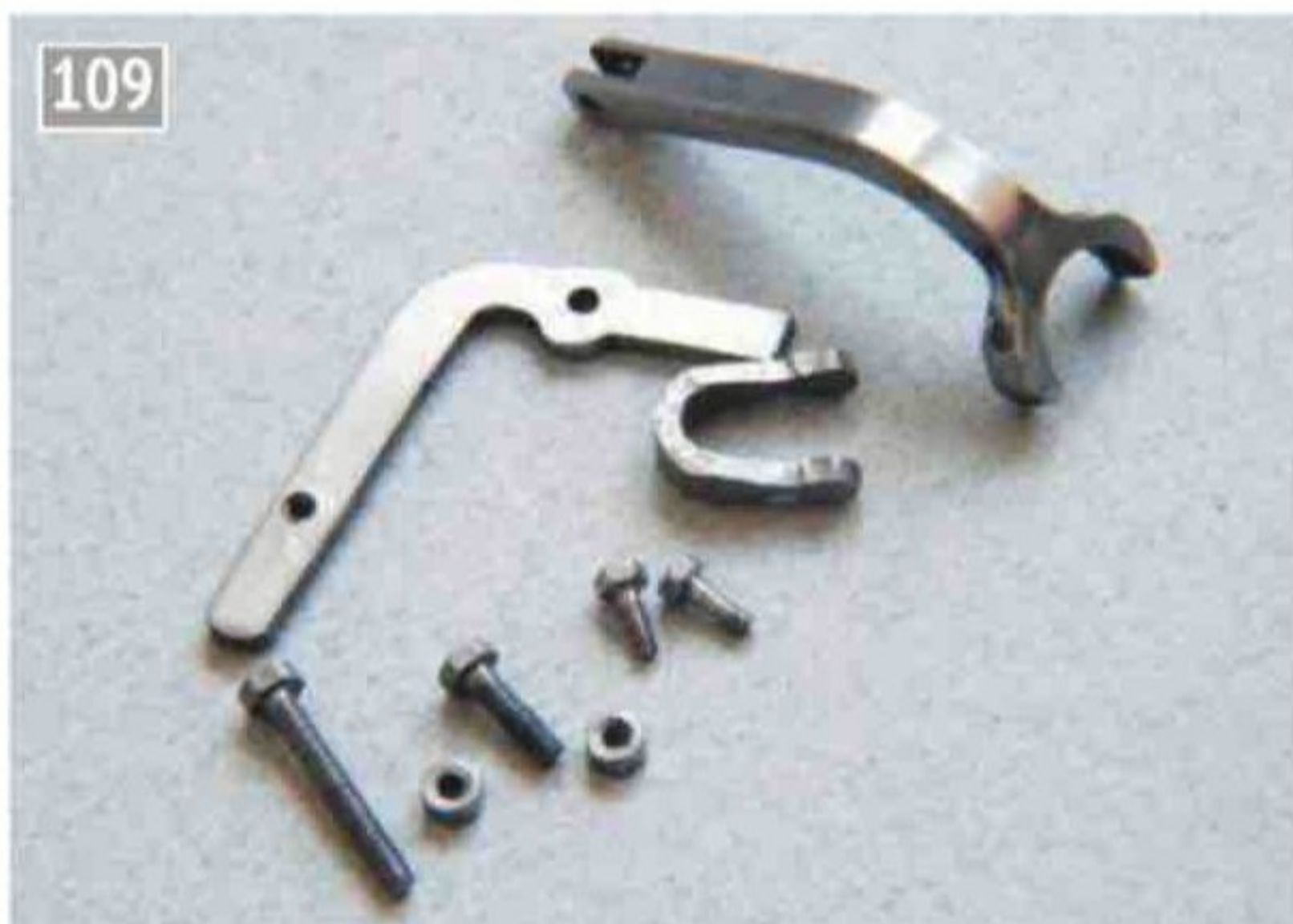
The completed bracket.
