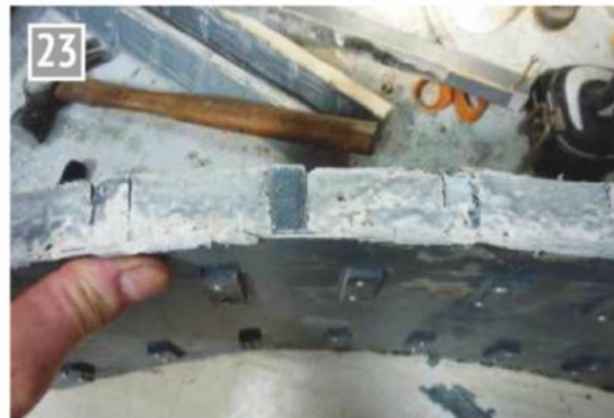
Flexing the mould base loosens the castings. When the mould is inverted they drop out.
