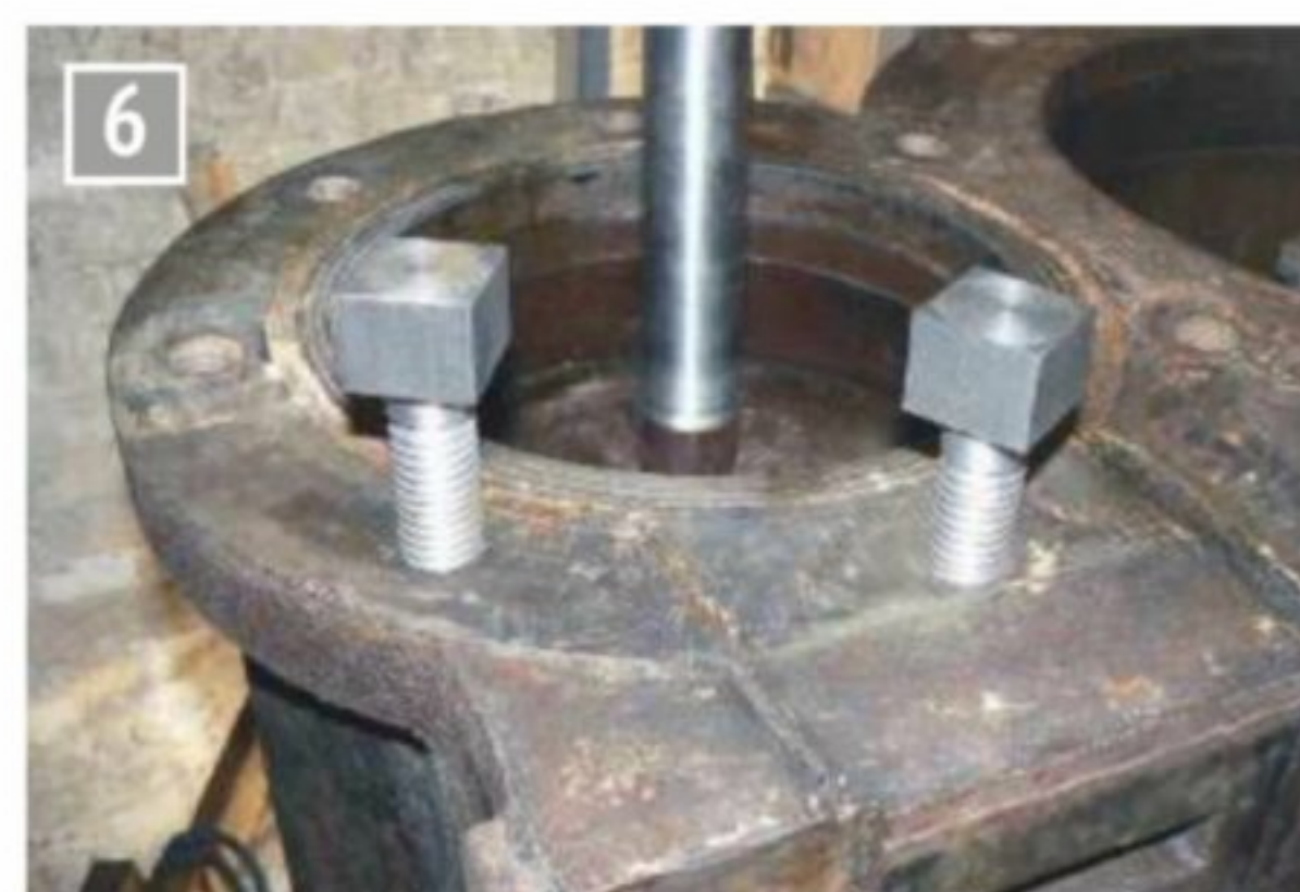
Two of the bolts in the mill engine awaiting assembly of the cylinder covers.
