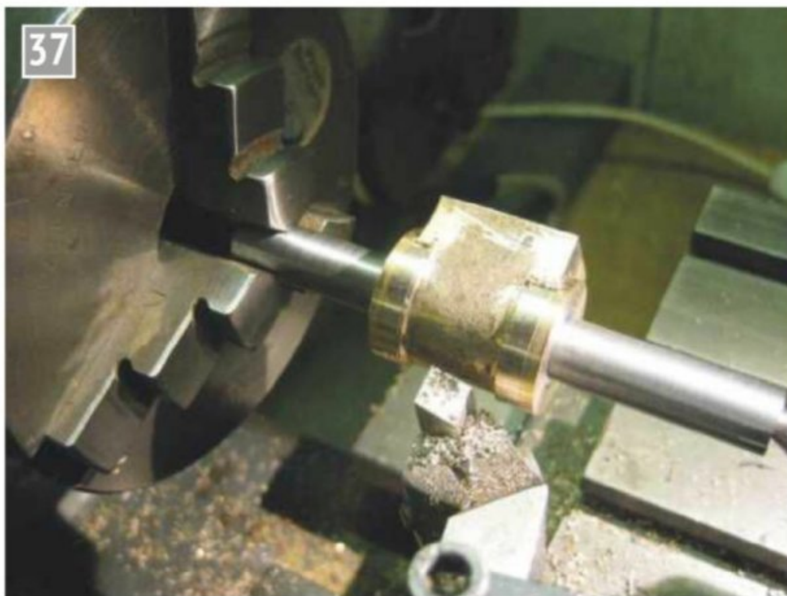
Completing the shaping of the cylinder by hand.
