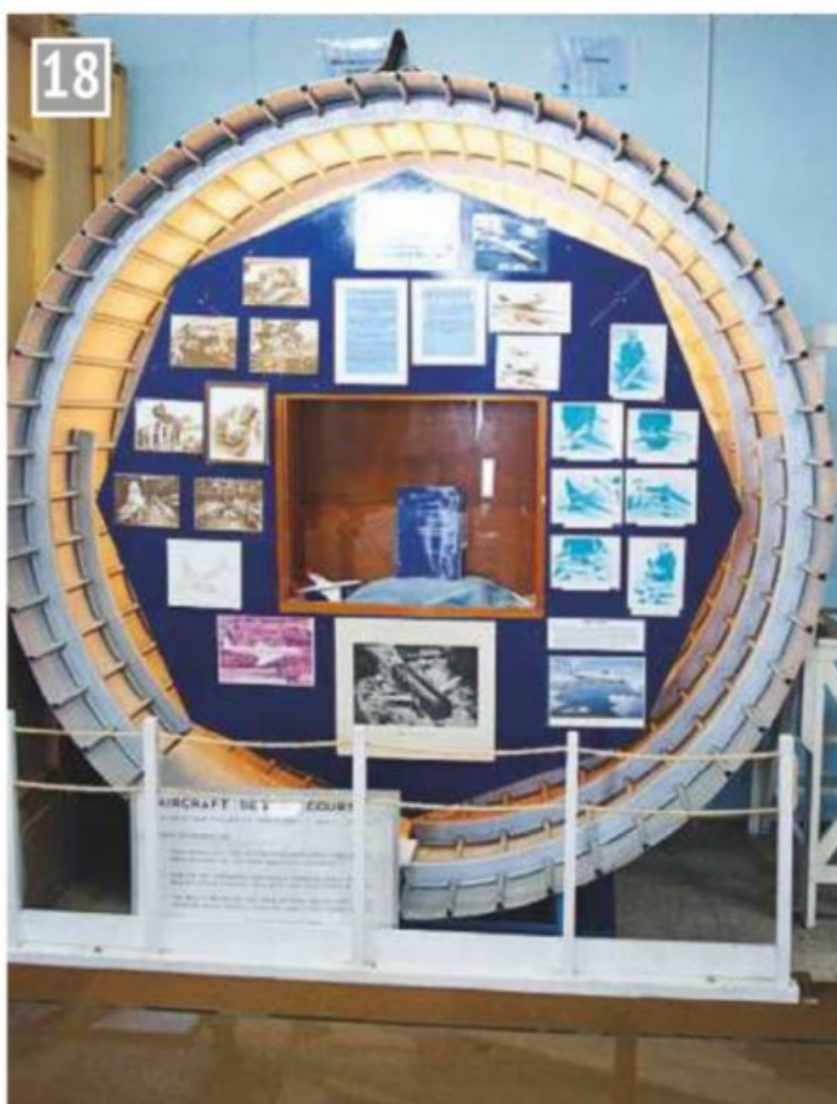
Comet display with fuselage section. Aircraft mostly use strong adhesives. Early Comet failures led to a major investigation by the Air Accident Investigation Board.
