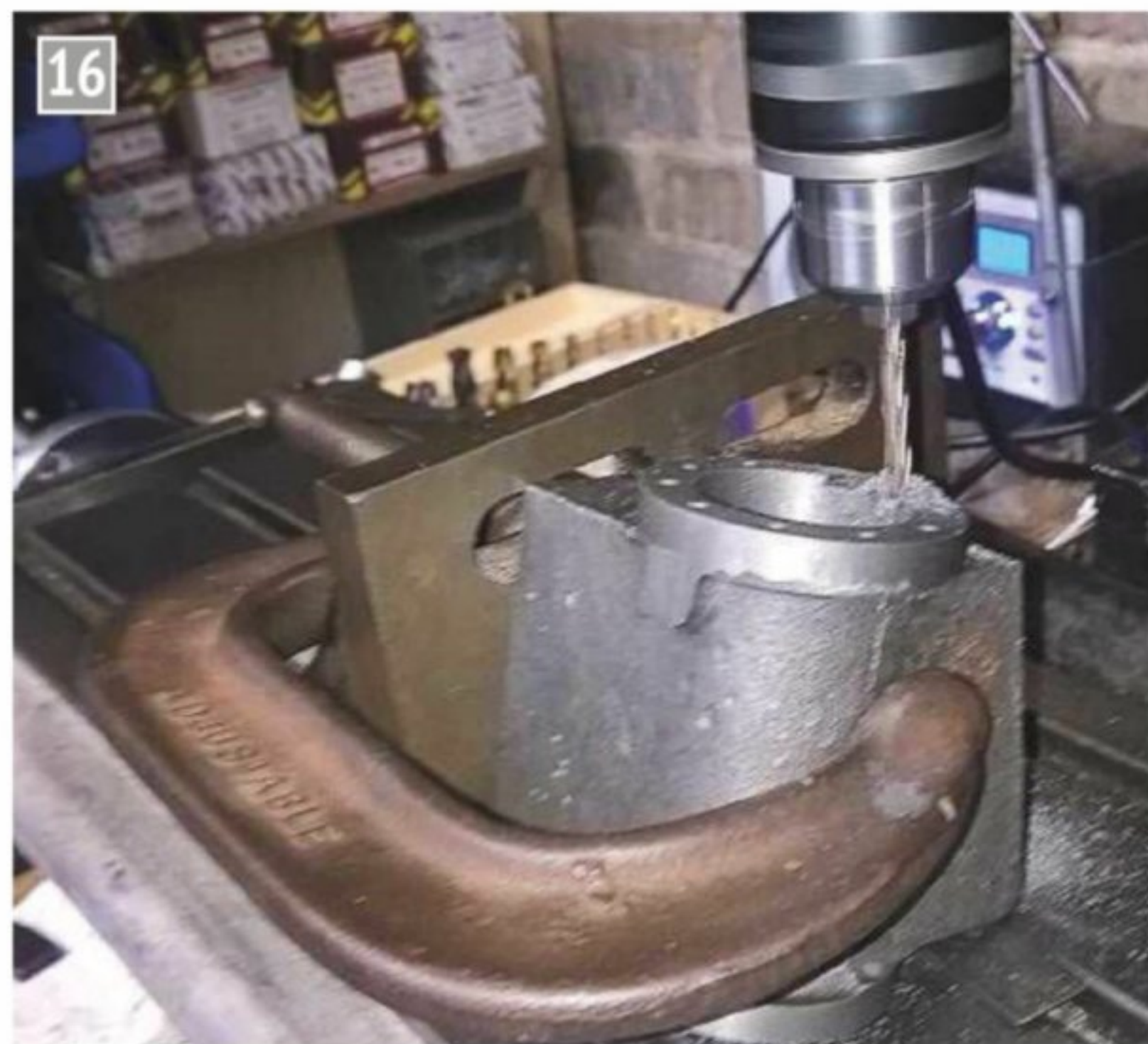
Drilling a port in the cylinder block.
