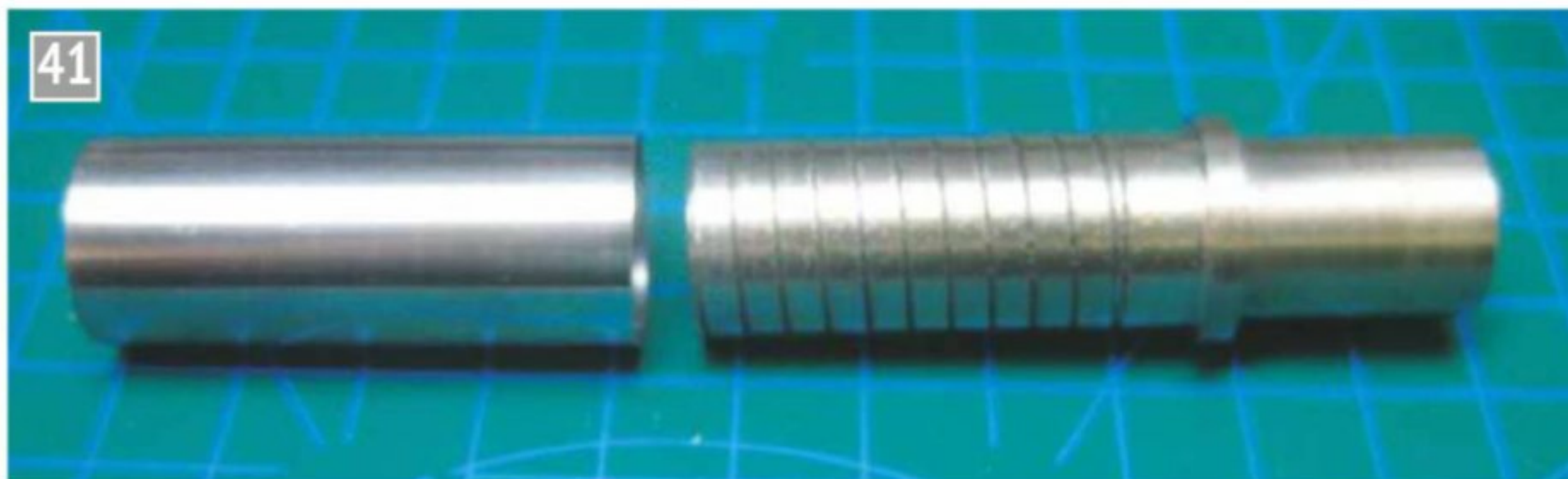
Mandrel for a Stirling engine displacement piston.
