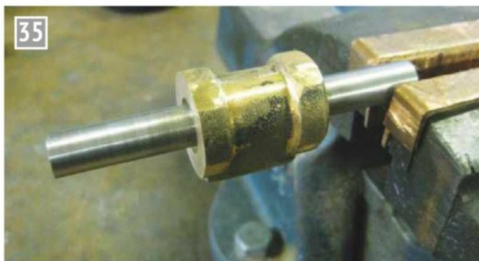
Cylinder secured on the mandrel.
