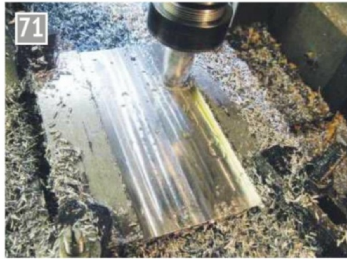
Machining the seating for the pin vice.
