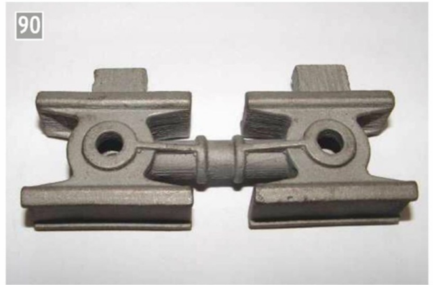
90 Crossheads, as supplied, as lost wax stainless castings.
