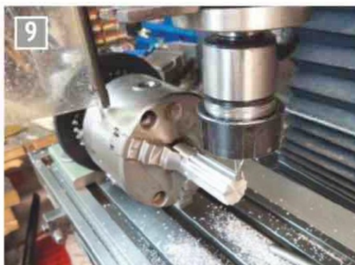
Cutting the finger grips.
