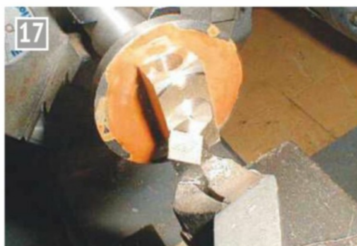
Turning a relief on the centred oscillating cylinder.
