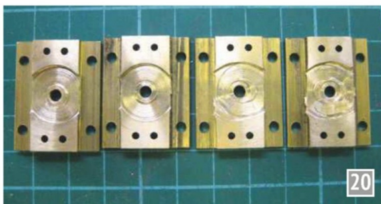
Correcting badly machined commercially made Mamod type port blocks.
