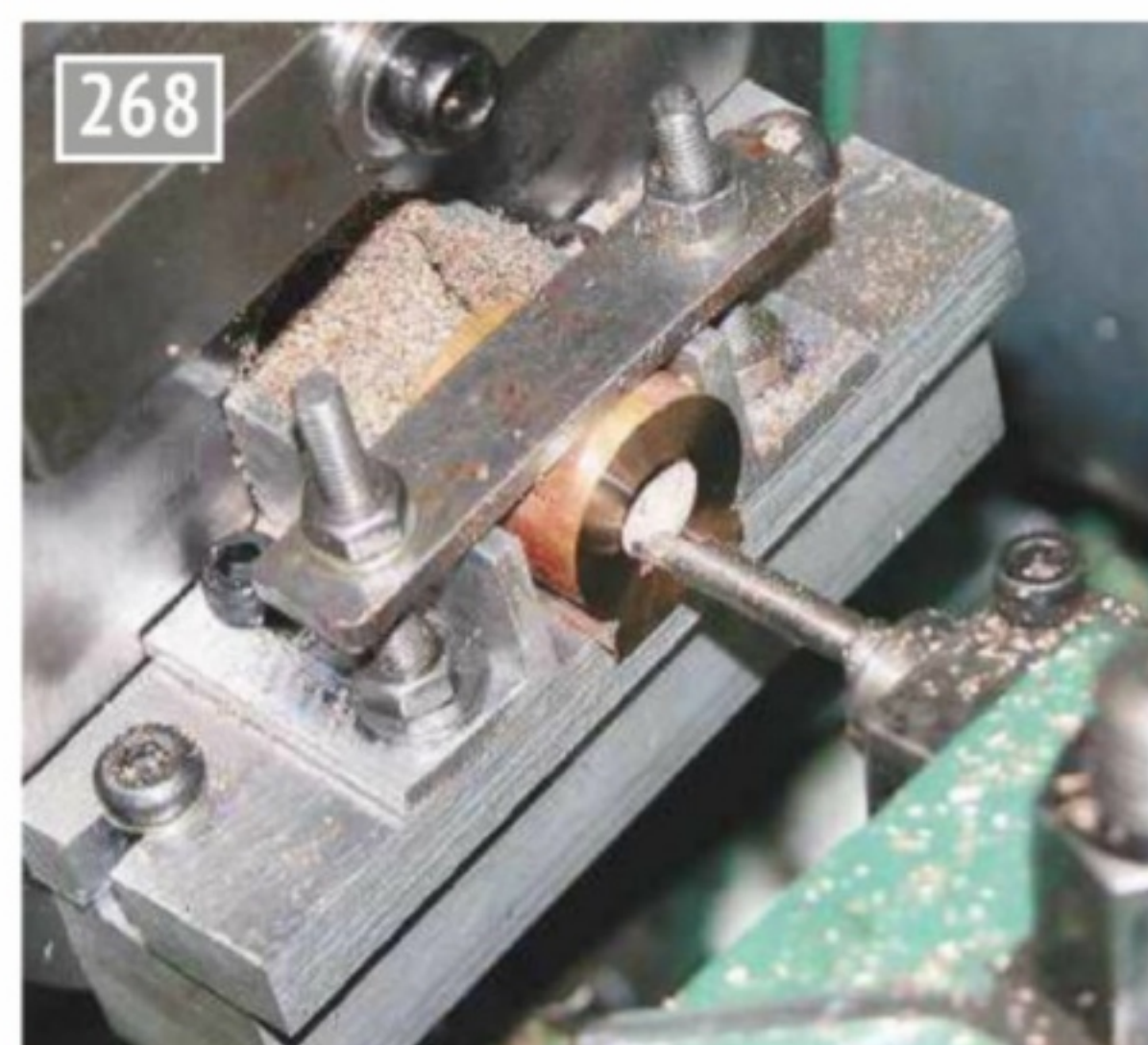
268 Boring and facing the cylinder.
