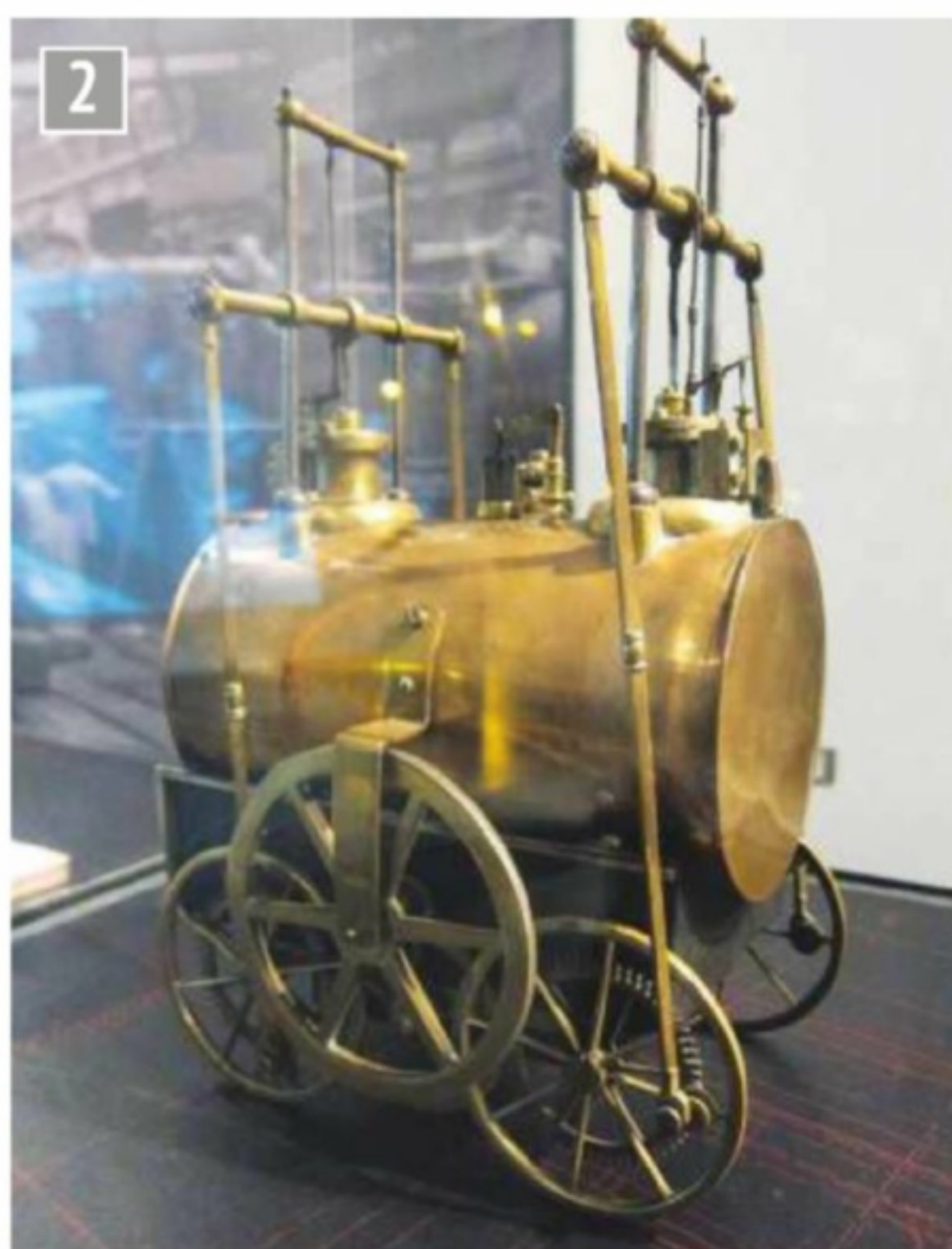
A clockmaker's model demonstrating William Hedley's idea for a two-cylinder locomotive; c. 1810.
