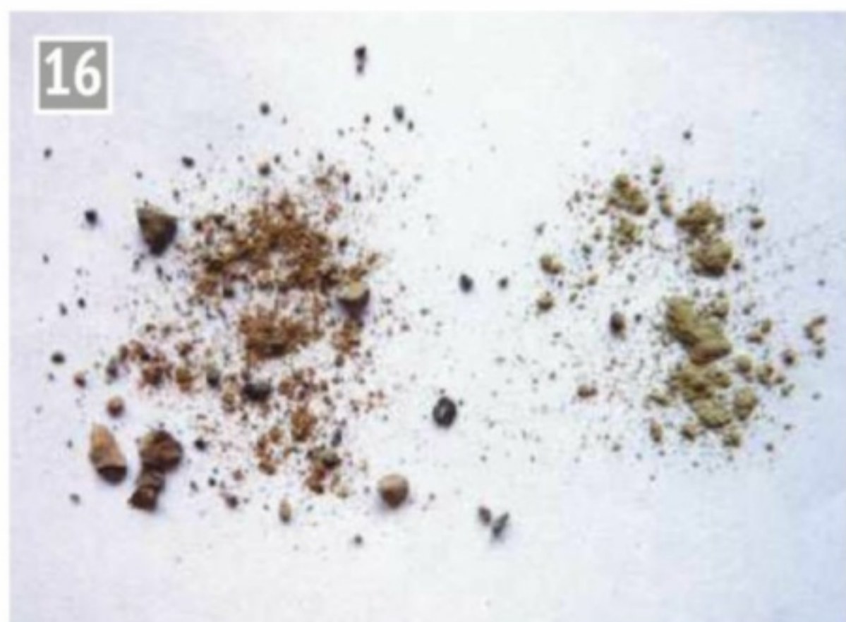
Washed sharp sand. The larger particles are about 3 - 4mm.
