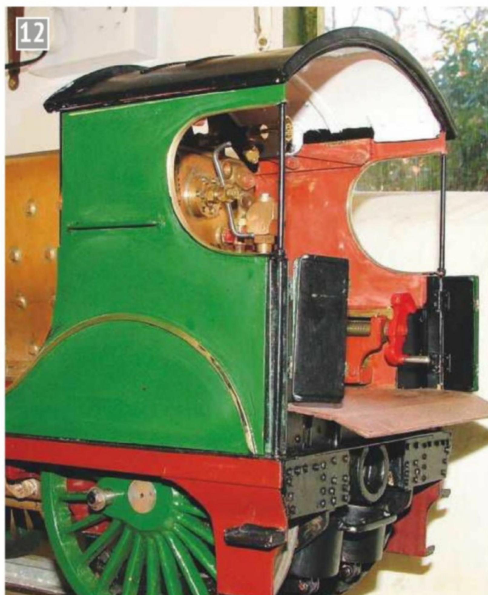
Once painted the hinge will be inconspicuous in the closed position.
