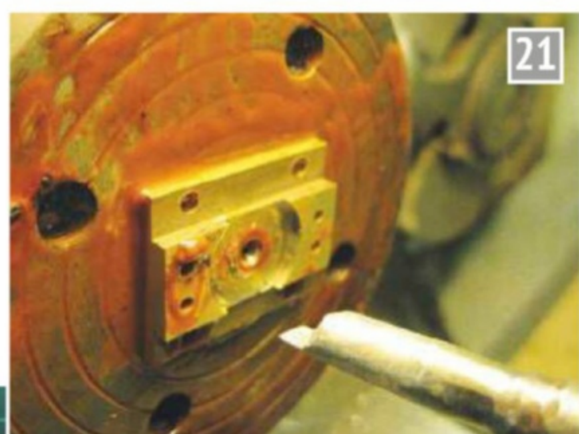
Correcting badly machined commercially made Mamod type port blocks.
