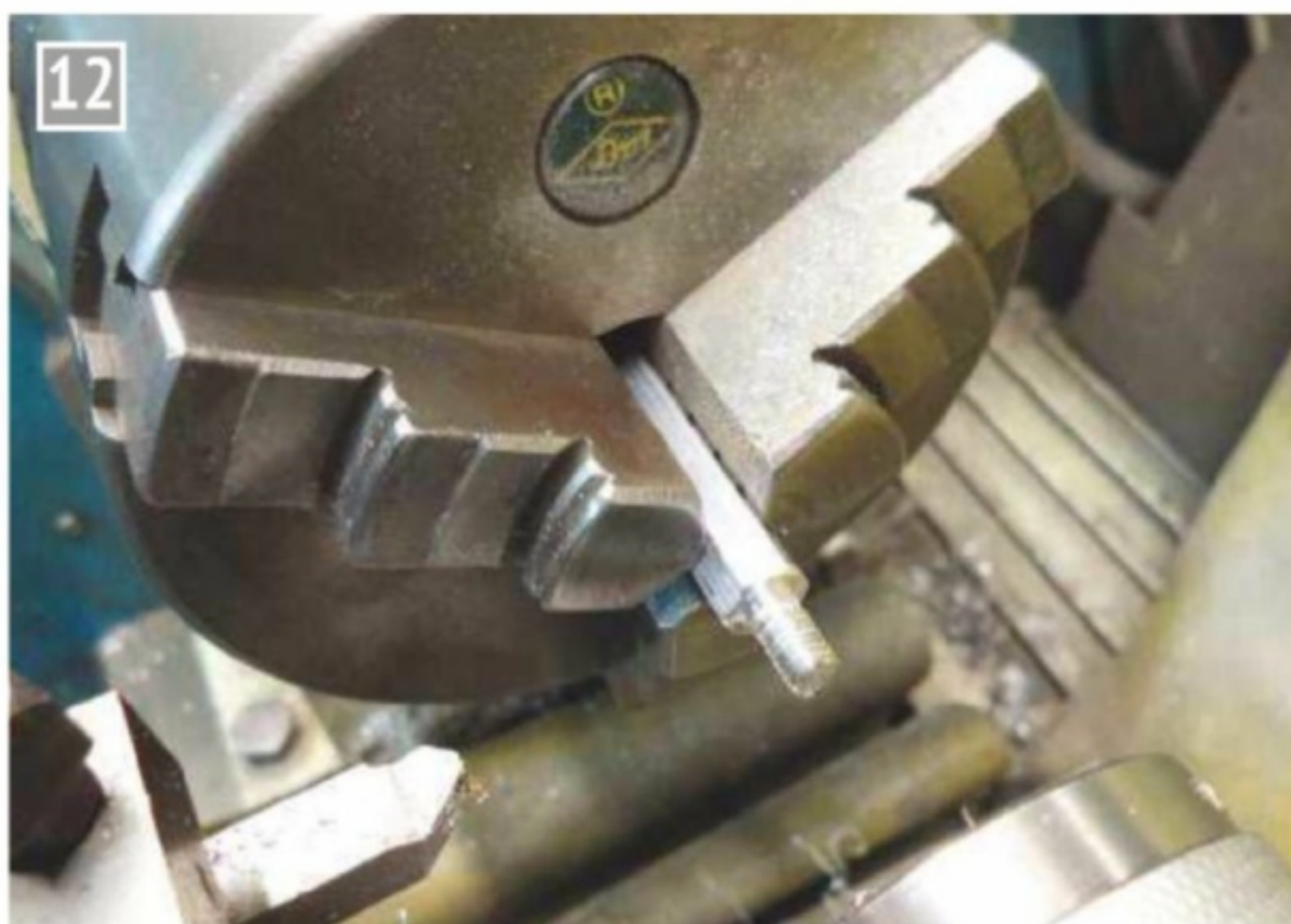
Thread the beam M5.
