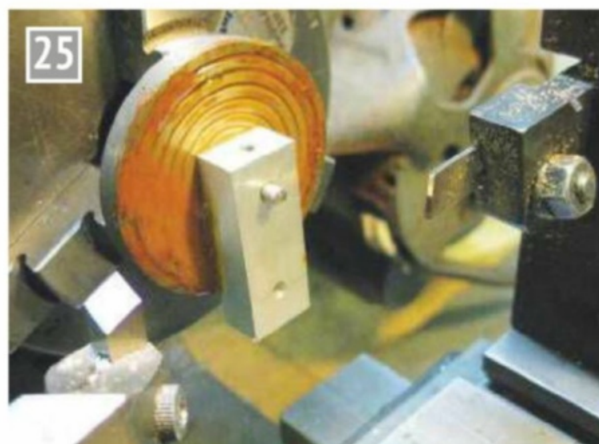
Using a centrally mounted pin; a crank being machined.
