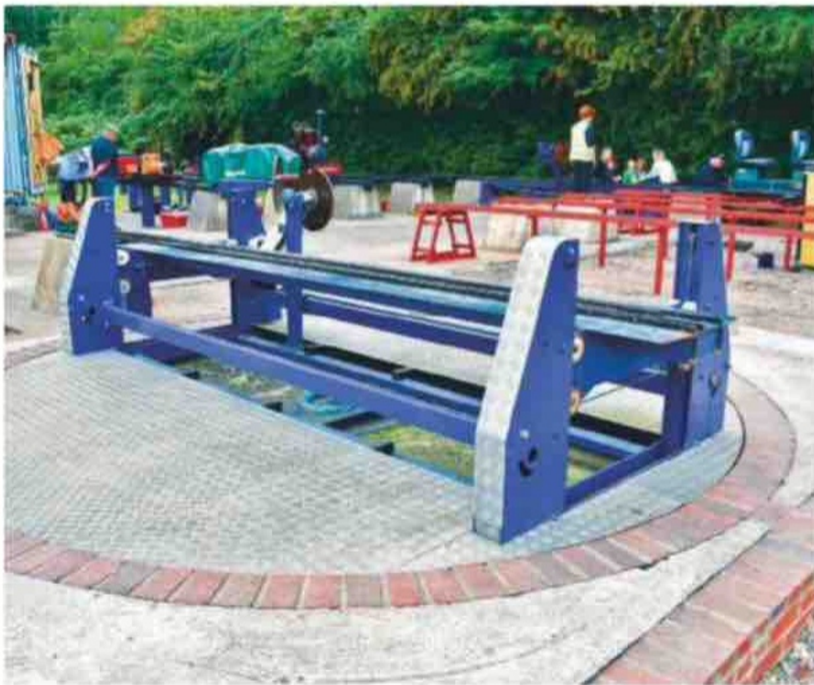
The splendid fully adjustable turntable designed by Eddie Atree and built by the Newport members.
