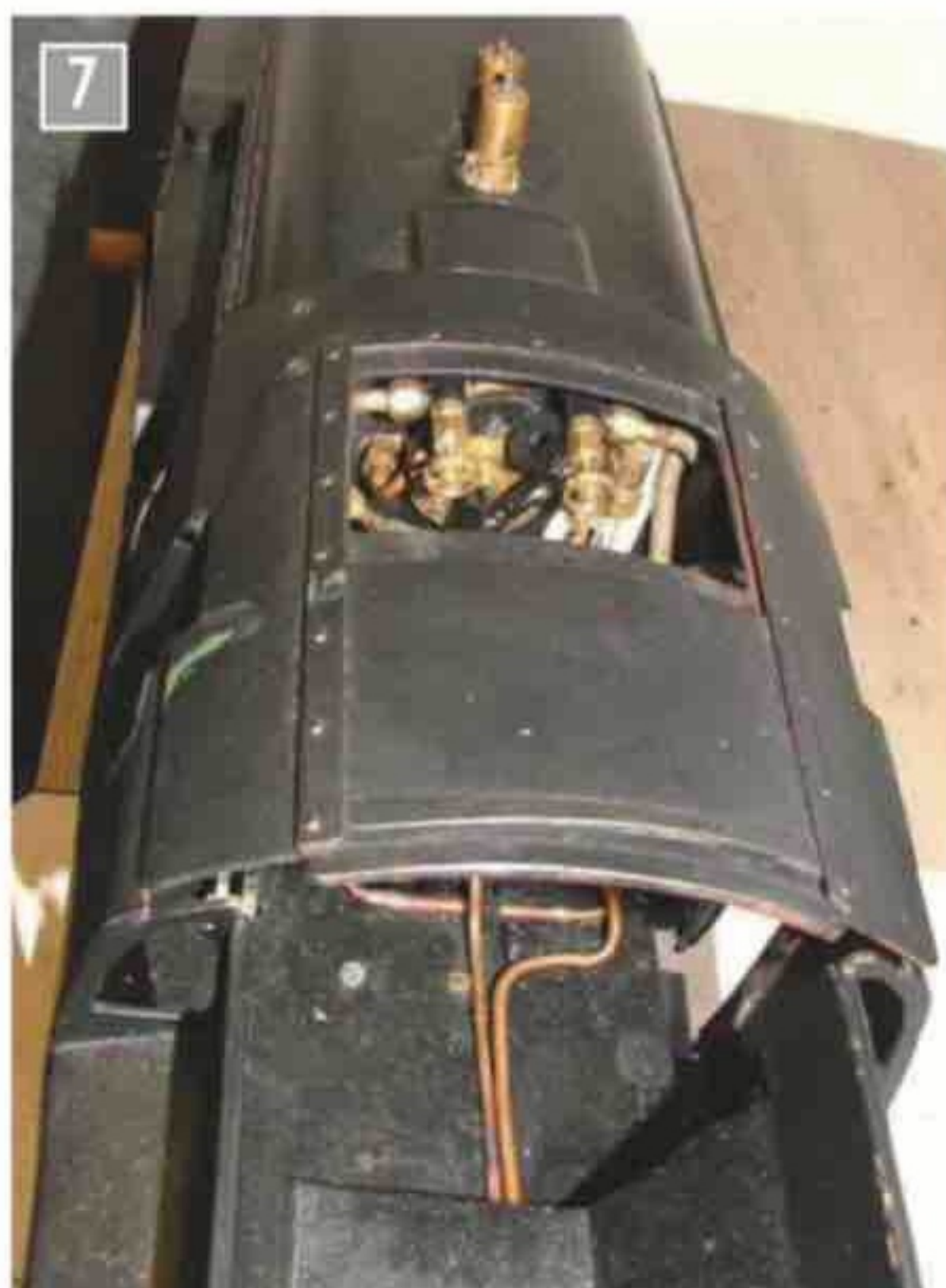
With the ventilator open it is possible to keep an eye on the water level and pressure gauge, just out of sight on the lower right side of the backhead.
