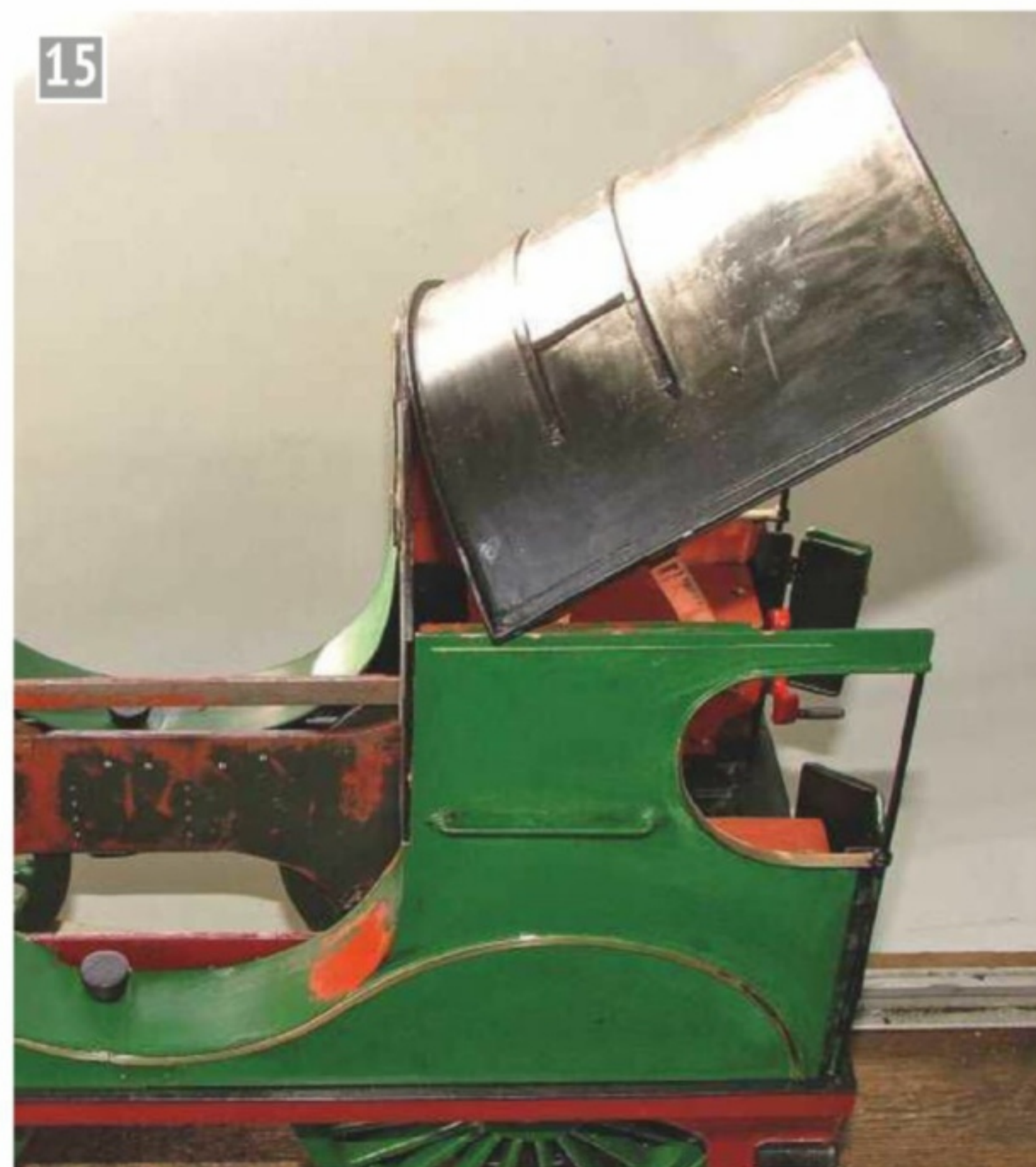
It would have been possible to make a sliding roof on this locomotive but the roof is then prone to being dropped and damaged as it is then fully detachable.
