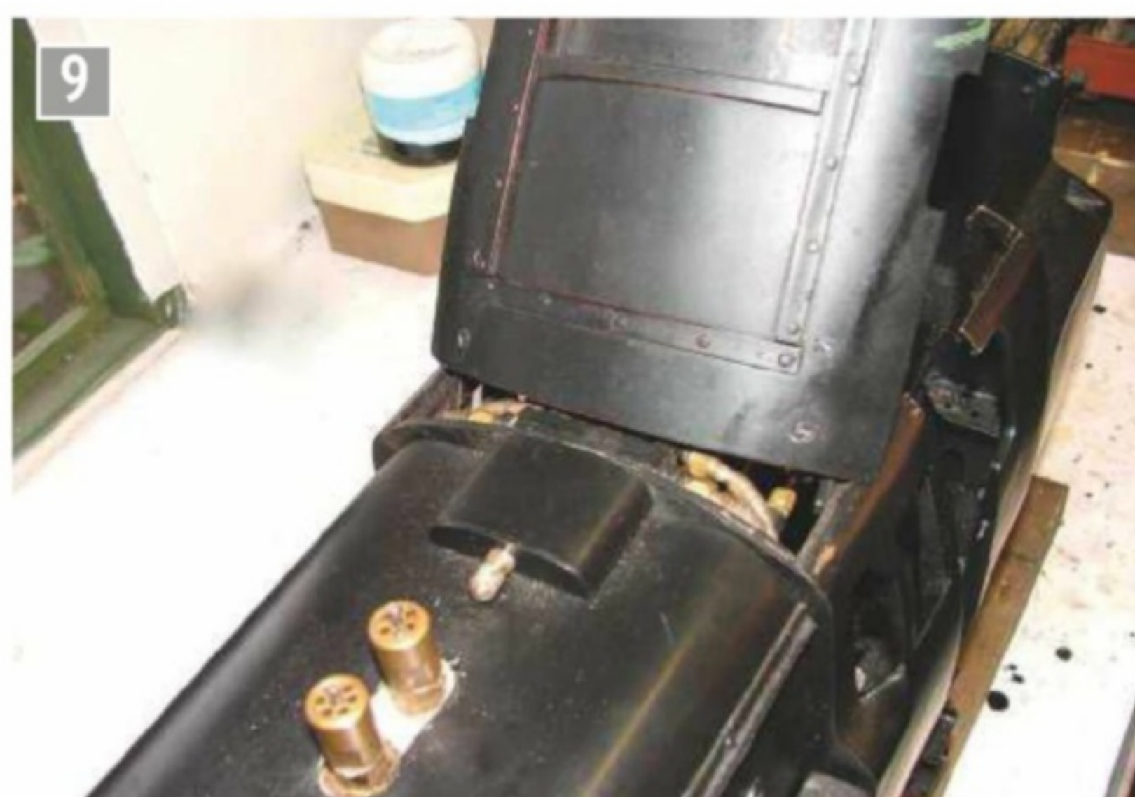
From this angle the way the hinge operation allows the roof to clear the steam turret, which is very close to the top of the cab front, can be seen.
