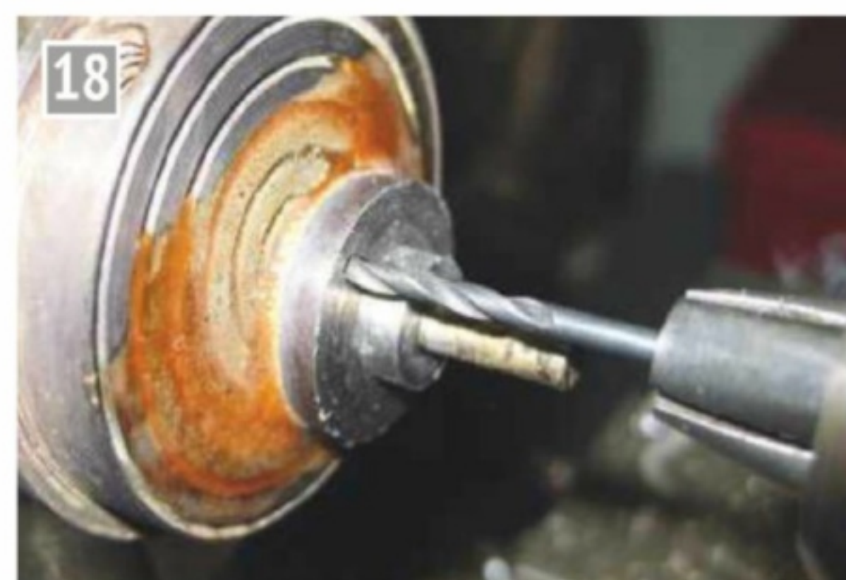
A fly crank mounted on an off-set pin on a wax chuck to drill its crank pin hole.
