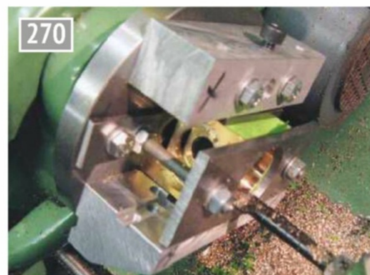
270 Machining the cube, I machined the block true 10 years before I got to this stage! (It looked in focus on the camera).
