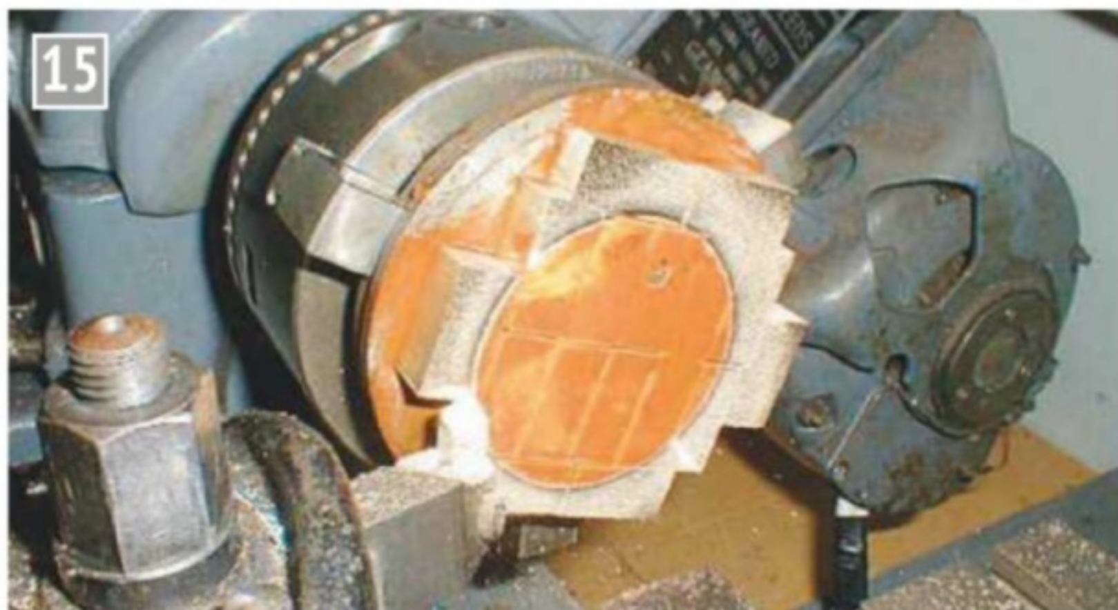
Machining 16 small brass rectangular oscillating cylinder blanks.
