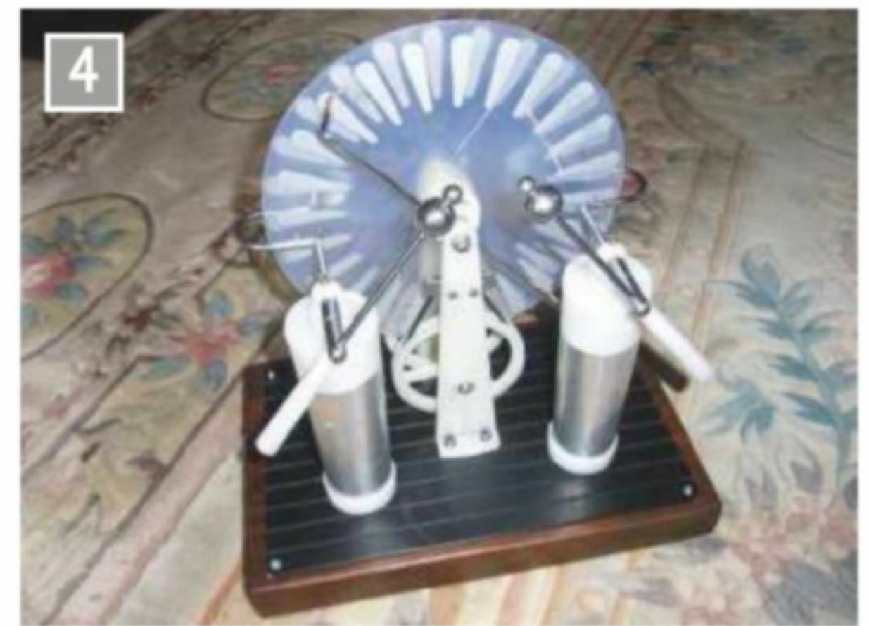
Rear view of the machine, showing the crossed belt, spark gap and Leyden jars.
