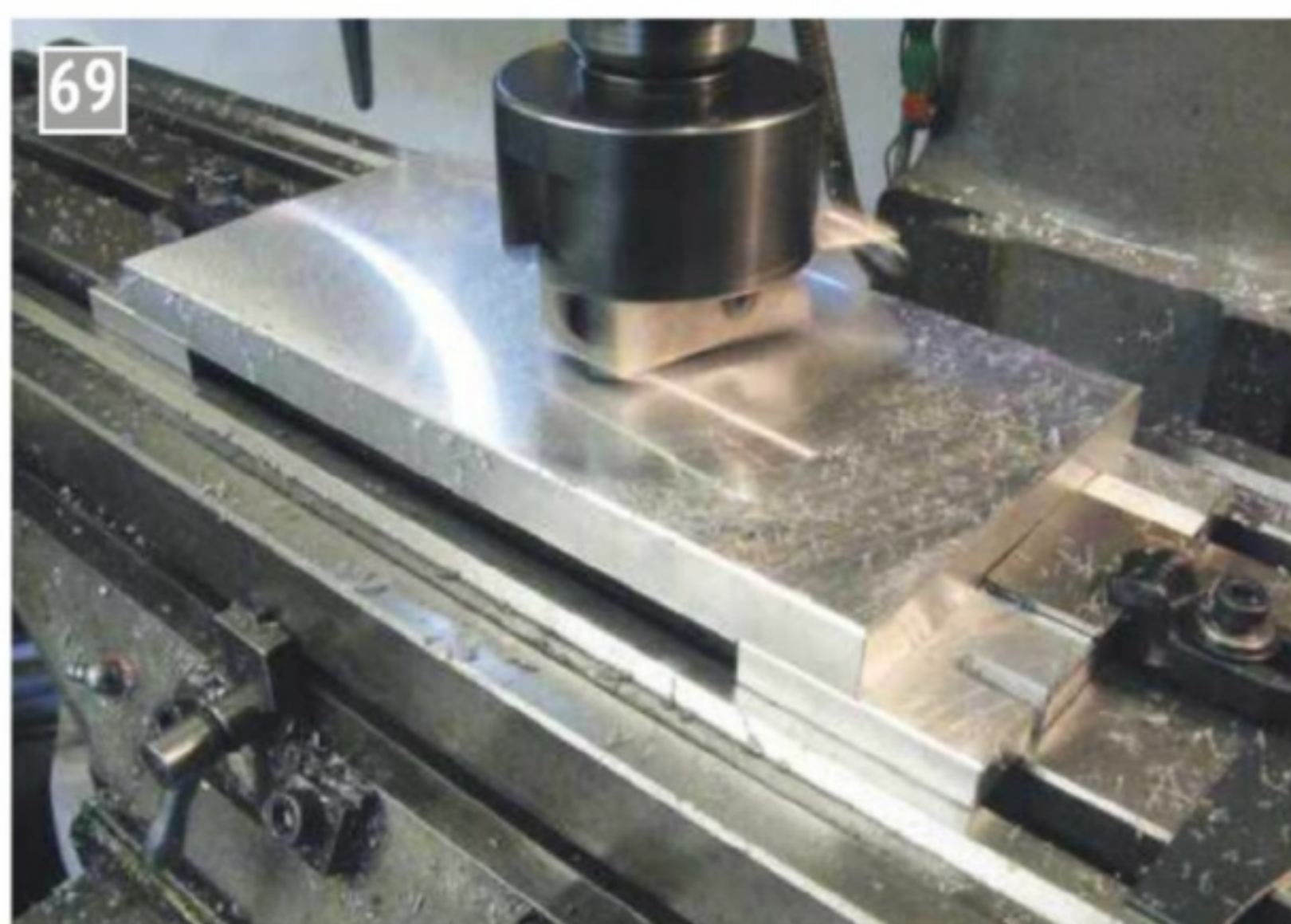
Fly cutting the sub base.
