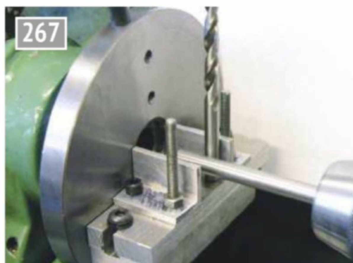
267 Setting the side location stop to position a cylinder. Each one of the batch will fit straight into the jig and be accurately positioned. I used a bar in the tailstock here as it is a fixed diameter; the setting pin is used only with top plate positioning.
