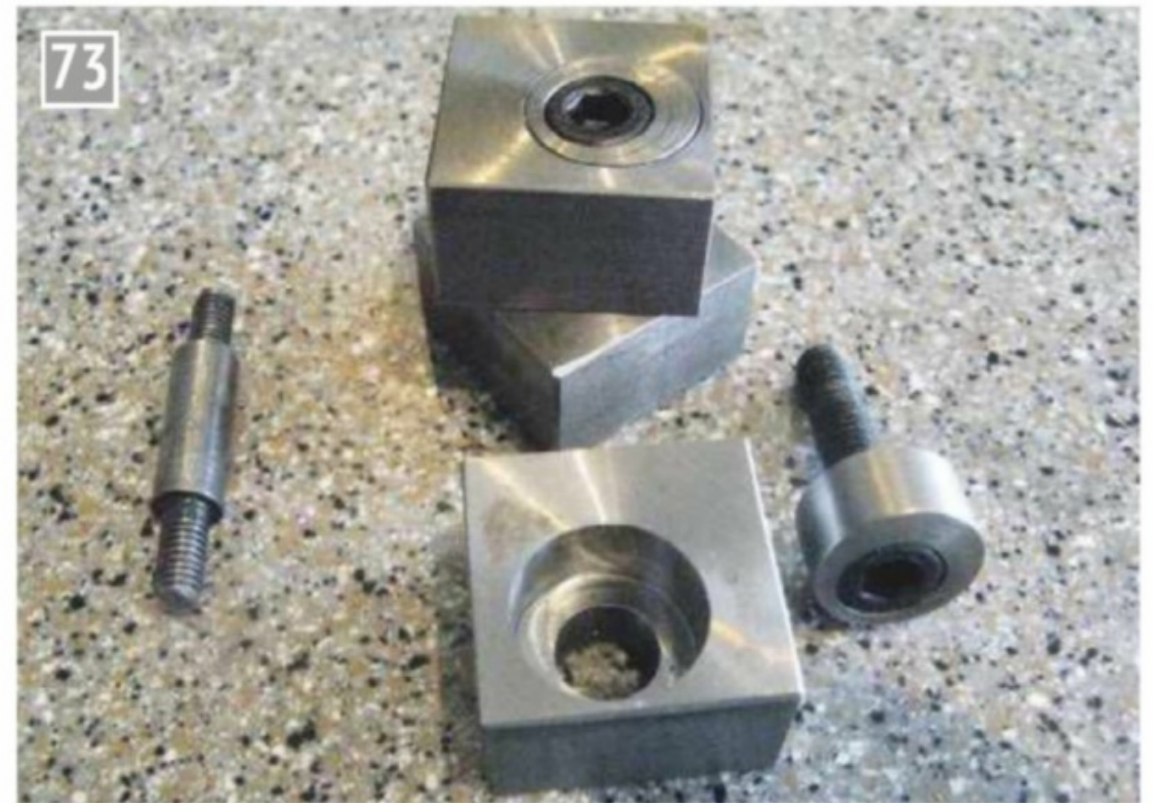
The eccentric low-profile cam blocks and the mounting pillar used for the radius rods.
