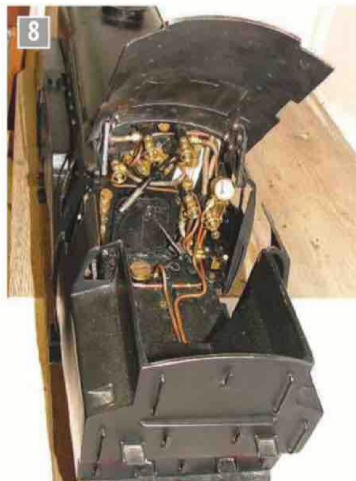
With the roof up, all controls are easily accessible. I have experimented with 'butterfly' firehole doors, as on the full size Bulleid Pacifics.
