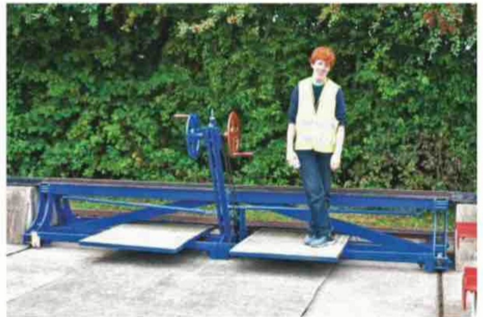
The versatile cable operated traverser, again designed and built by the Newport members.
