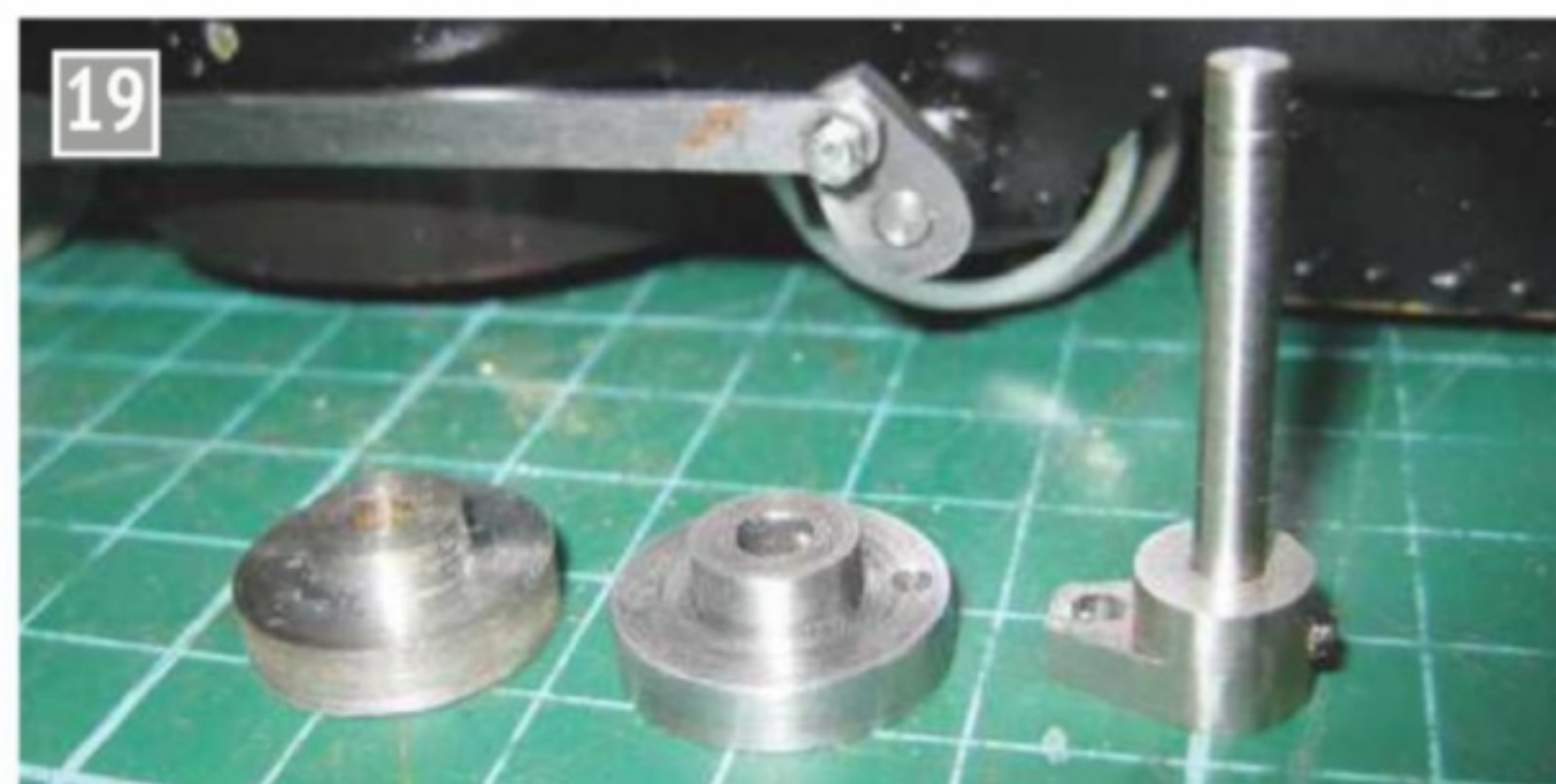
Sequences of making a small crank pin.
