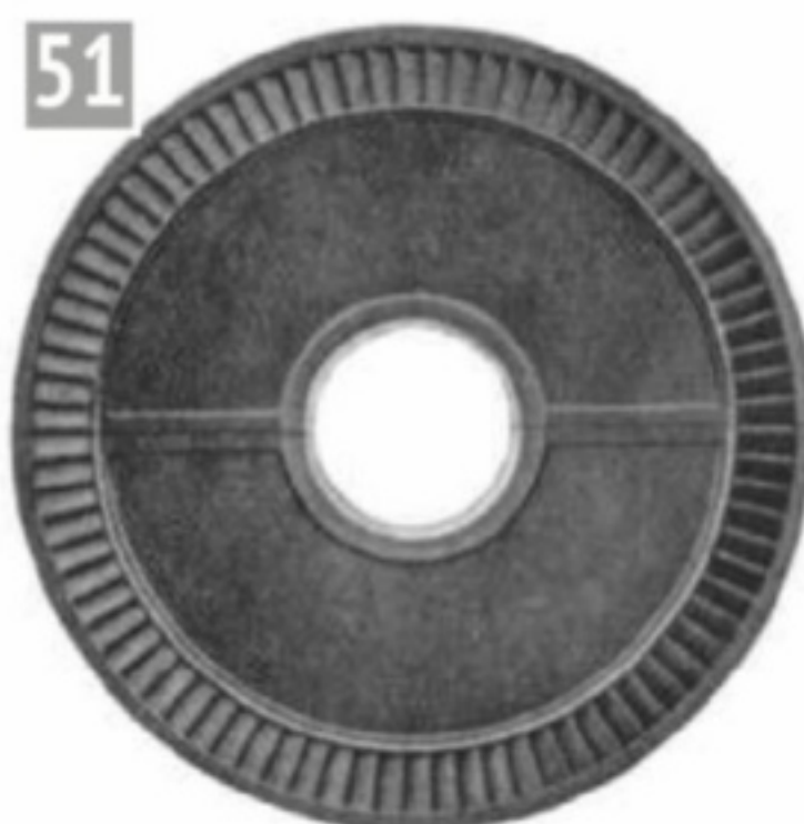
Large diaphragm disc consisting of sheet steel guides embedded in a cast iron body.
