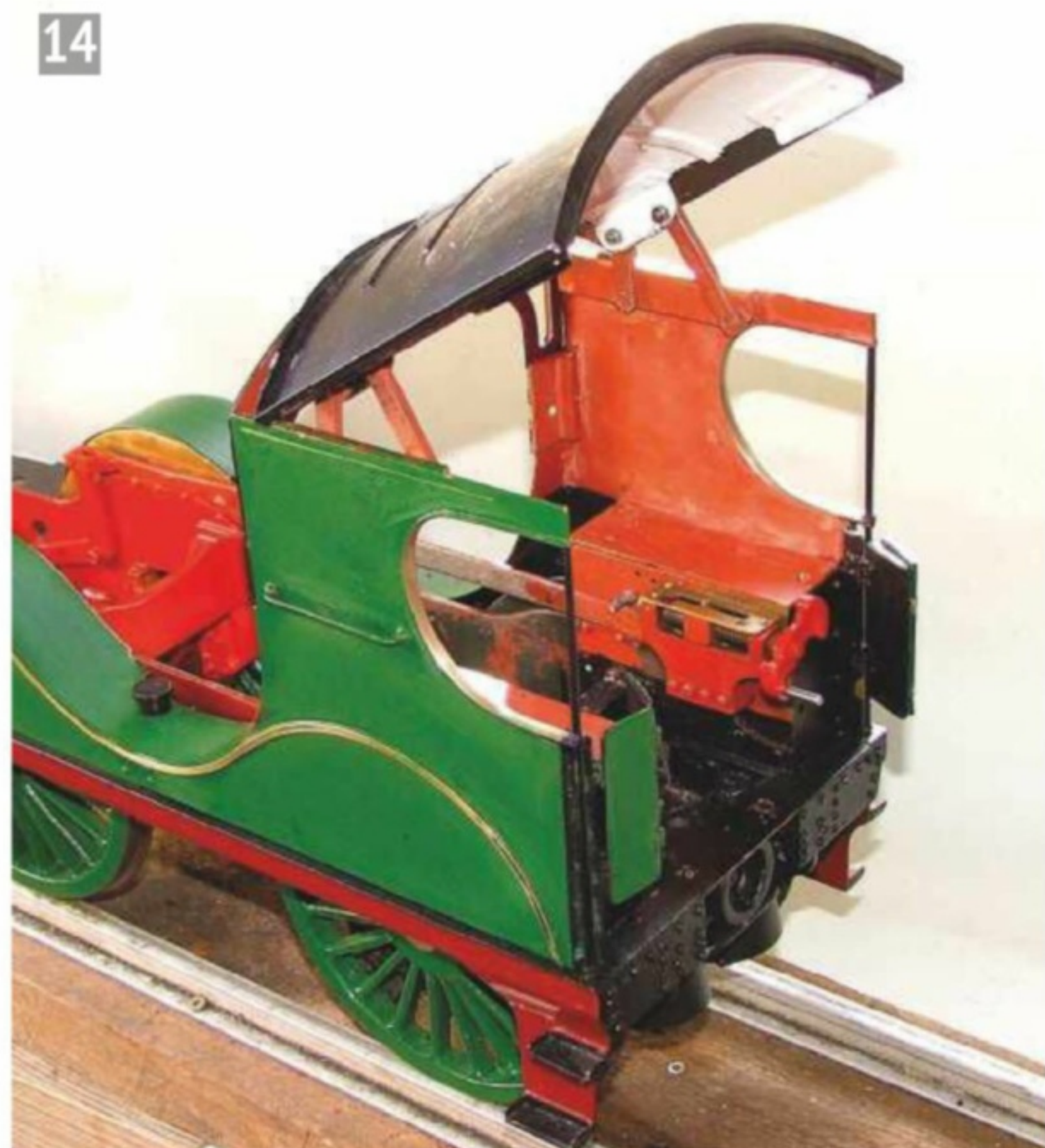
Roof raised, ample access to the controls. The locomotive is correctly built with right hand drive but incorrect in having a screw reverser. A steam reverser was standard on the SECR on almost all classes.
