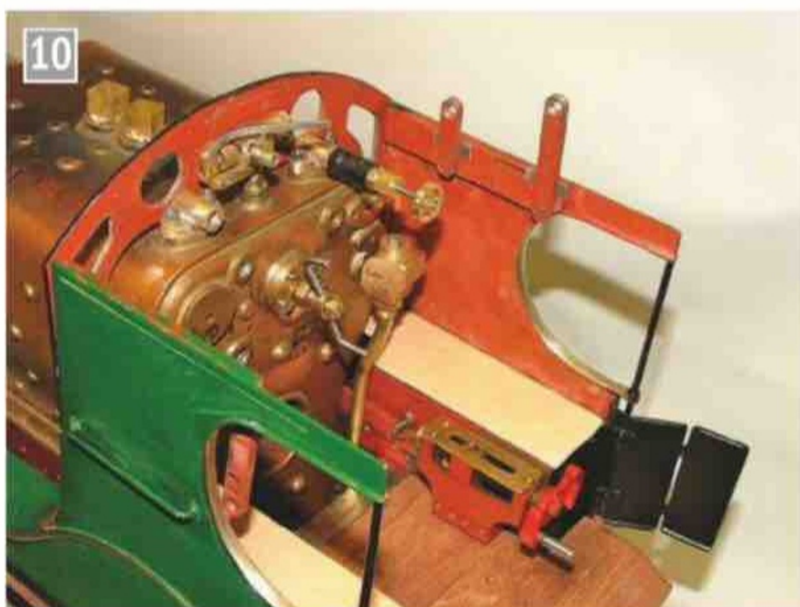
On the L class it was possible to fit the frame of the hinge to the cab sides as these are flat.
