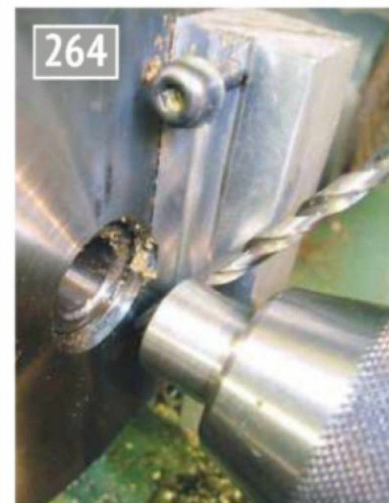
Using a drill to set the centre of the Tee to the lathe axis, rotated for clarity in the photo.
