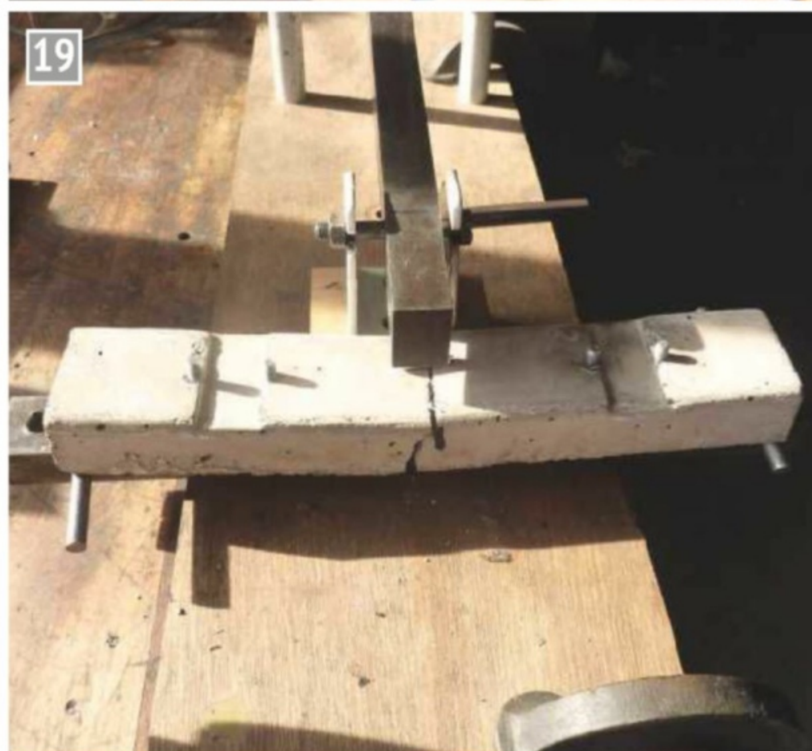
Test rig for flexural strength. Load is applied by a screw attached to the top of the balance (out of shot). It is magnified x 10 by the steel bar. This sleeper broke at 110kg when supported by two rollers placed right at the ends, 9 inches apart.
