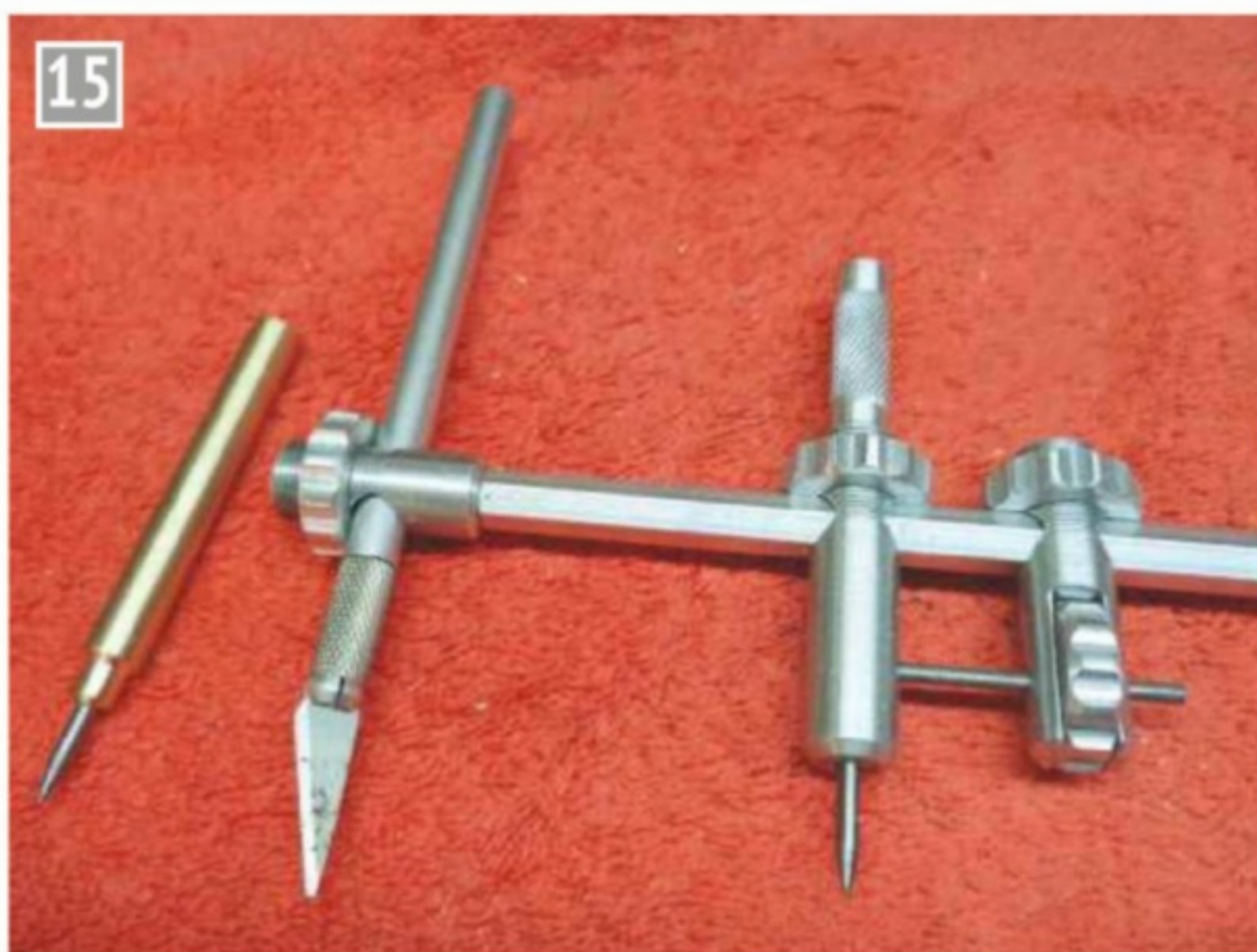
Trammel with scalpel for cutting out gaskets.
