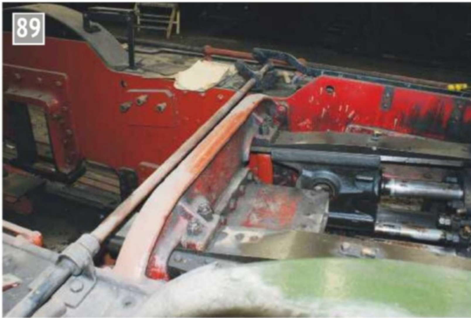
89 Crosshead on 7754 – note, con. rod is missing.
