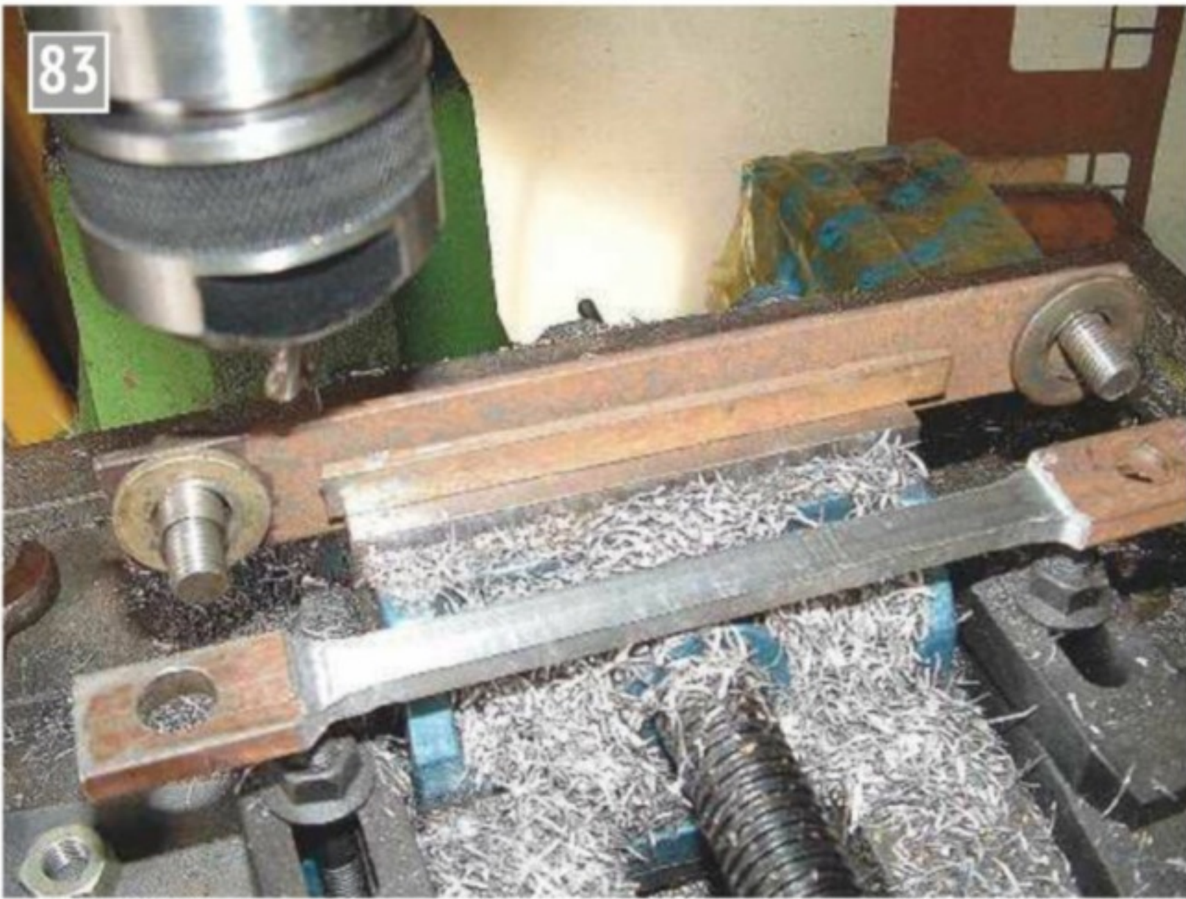
Roughing out completed.
