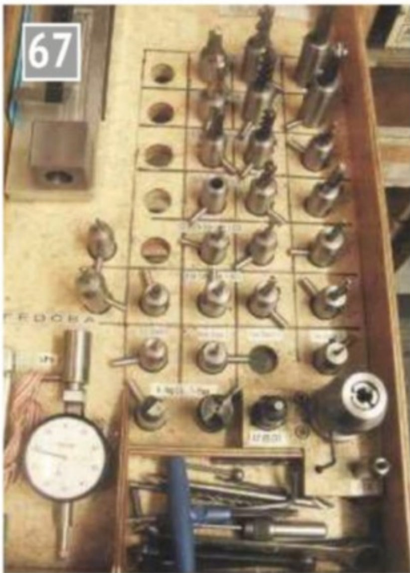
The CNC tool drawer, mounted in filing cabinet type runners directly under the miller.
