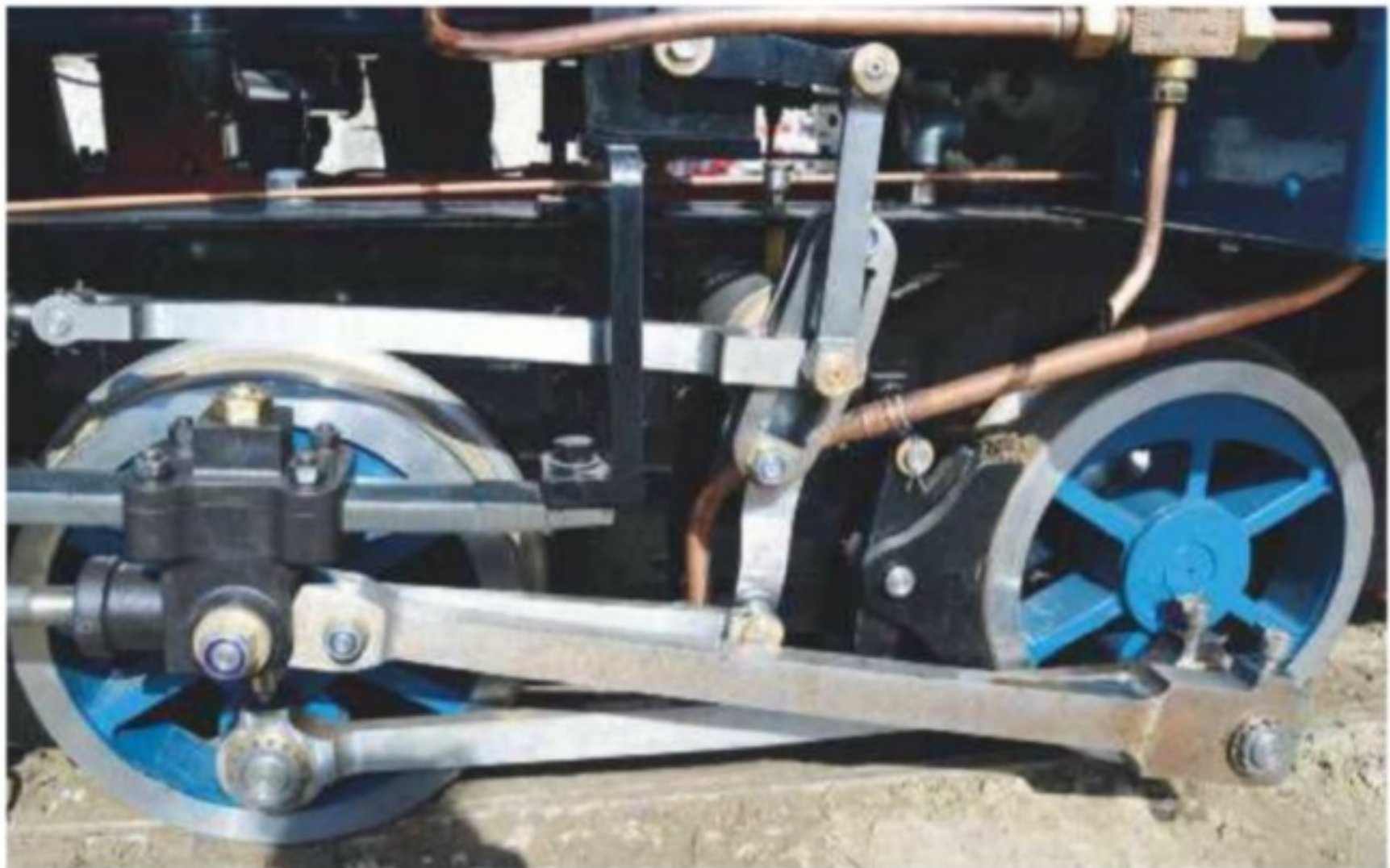
This is a close-up view of the left hand external components of Otter's Bagnall-Price valve gear. From top to bottom, we have the weighshaft bellcrank; the drop-link; the expansion link; the die block (with 'wobble' bearing behind) and valve rod; the combination arm; the crosshead, correcting link and connecting and coupling rods. Note that the general design philosophy of this valve gear is very similar to Walschaert's with its reliance on a primary eccentric (or return crank) driven motion 'combined' with a crosshead driven correcting (lap/lead) motion. Note also the shape of the connecting rod in the big end region – there is blank metal where a cotter pin spit bearing would have been on the original Sipat design.
