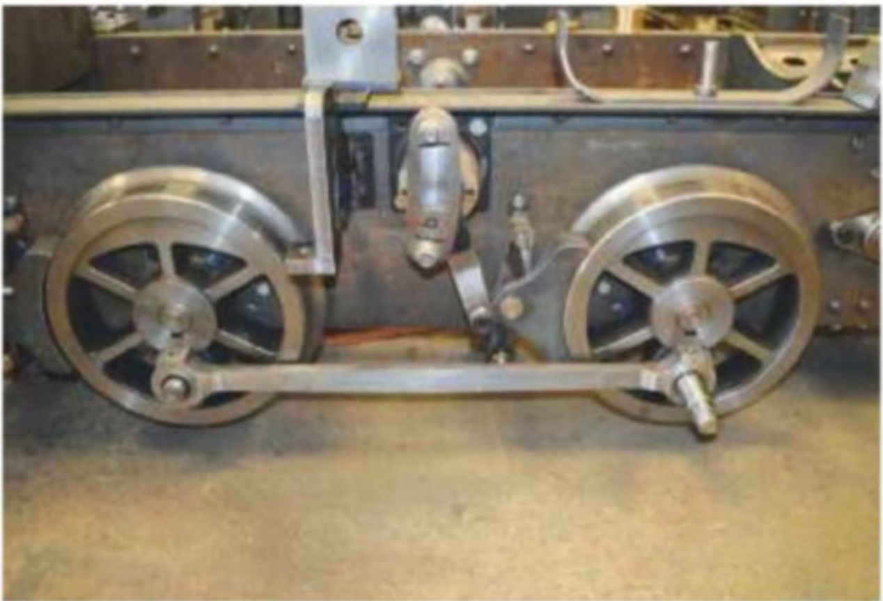
The external parts of the Bagnall-Price valve gear had yet to be fully assembled at this stage, but in this left-hand view the expansion link and combination arm (fixed to the 'wobble' bearing) can be seen.
