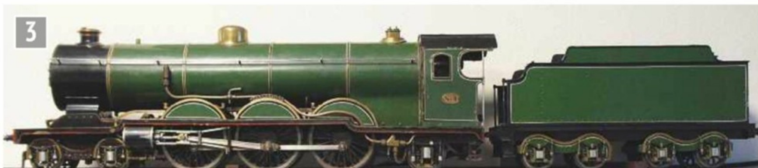
Conversion, formerly Charles Aldington, as it is today. Though outwardly little changed this was built as a four cylinder compound but later altered to simple expansion (© SMEE 2019).
