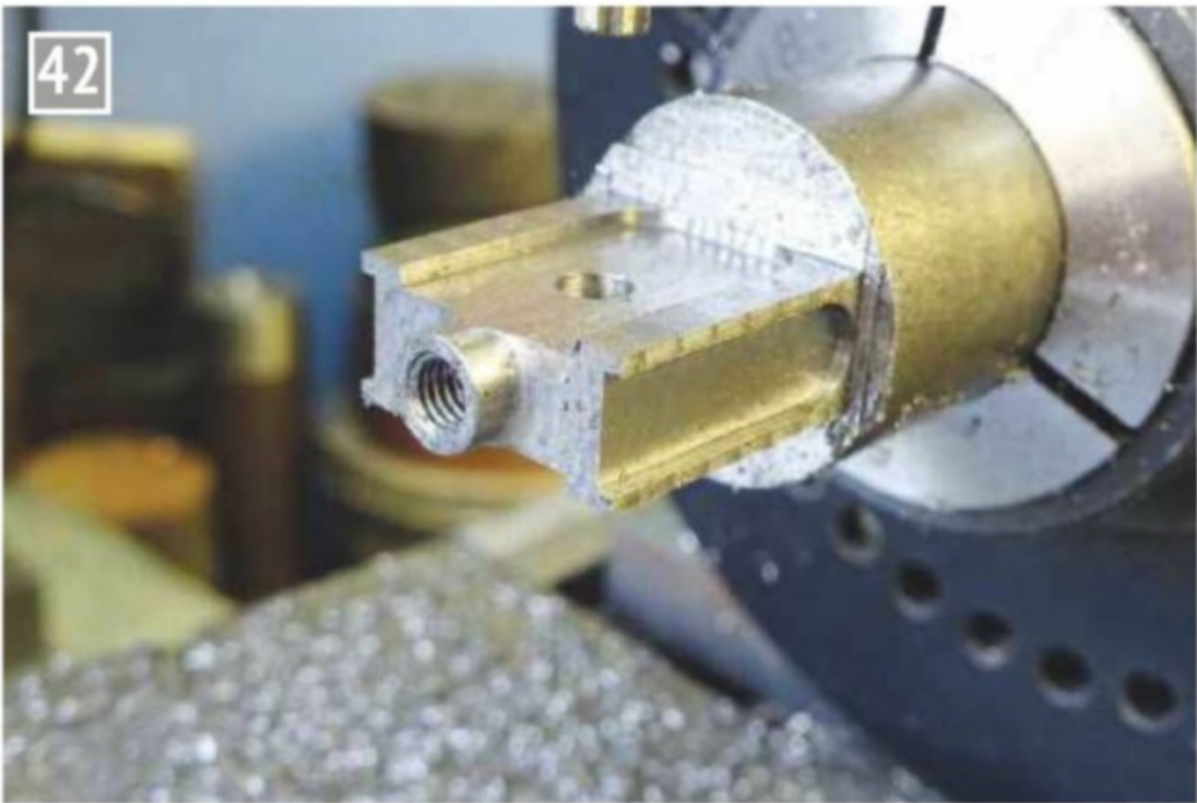
Reaming the crosshead pin hole after milling.
