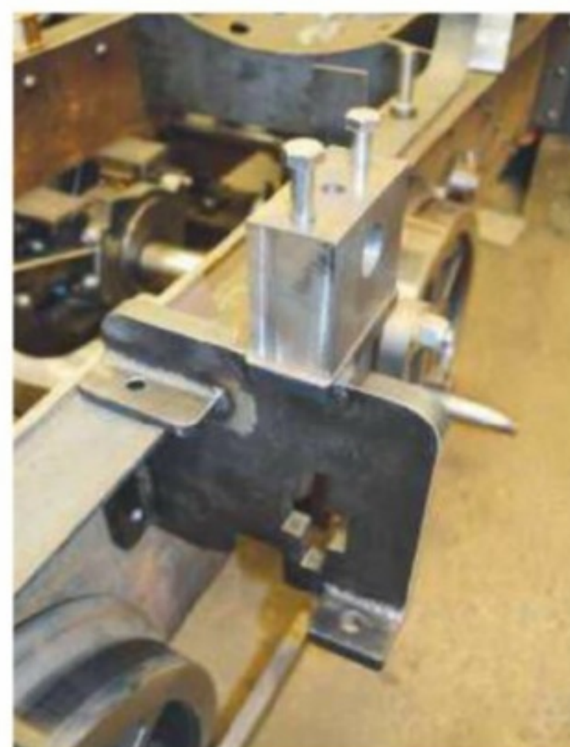
A close-up view of the left hand motion bracket and weighshaft bearing.
