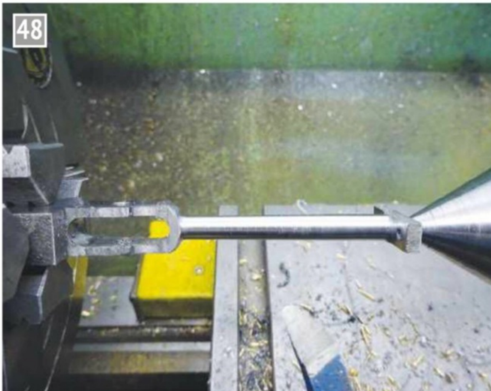
Rough turning prior to doing the taper.
