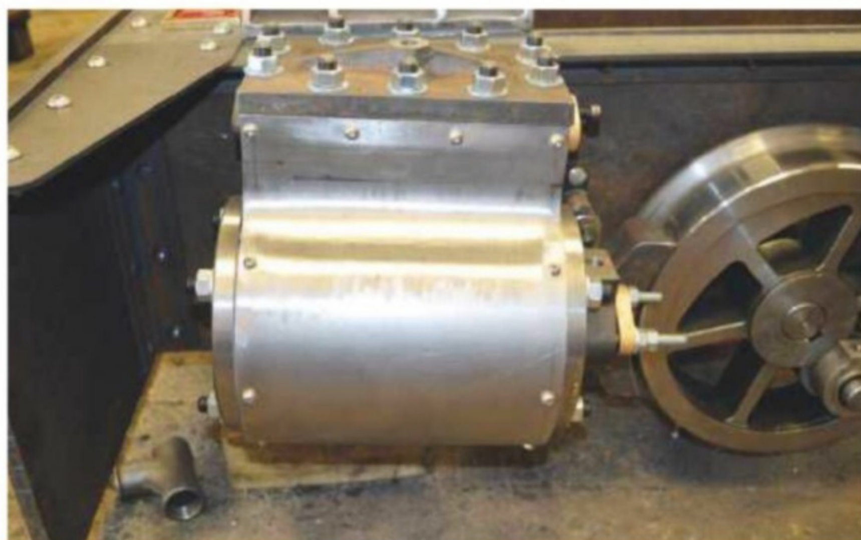
A close-up view of the left hand cylinder. This was cast from the same pattern used to produce the cylinders for the G.G.R.'s other new Bagnall-pattern steam locomotive, 2-4-0T Brown Bear.
