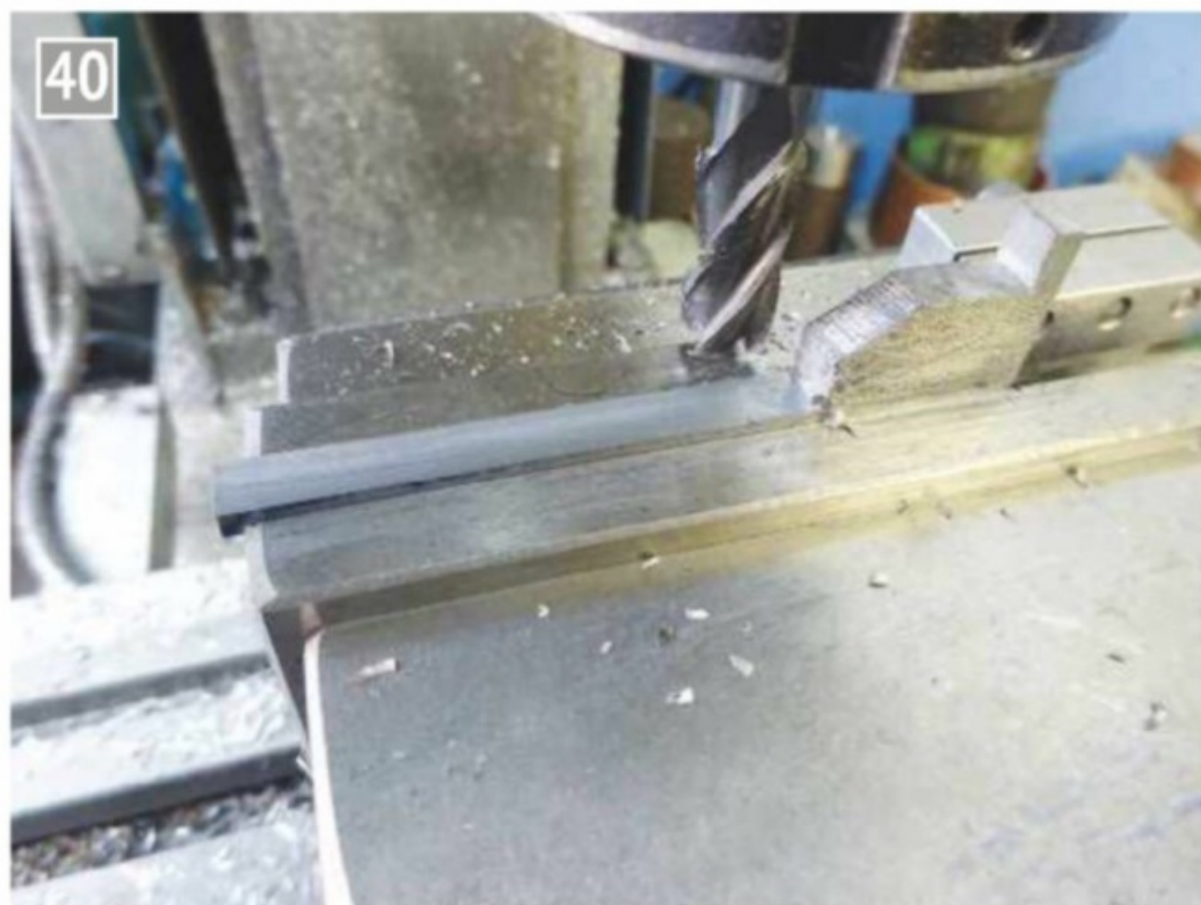
Milling the lower leg of the guide to thickness.
