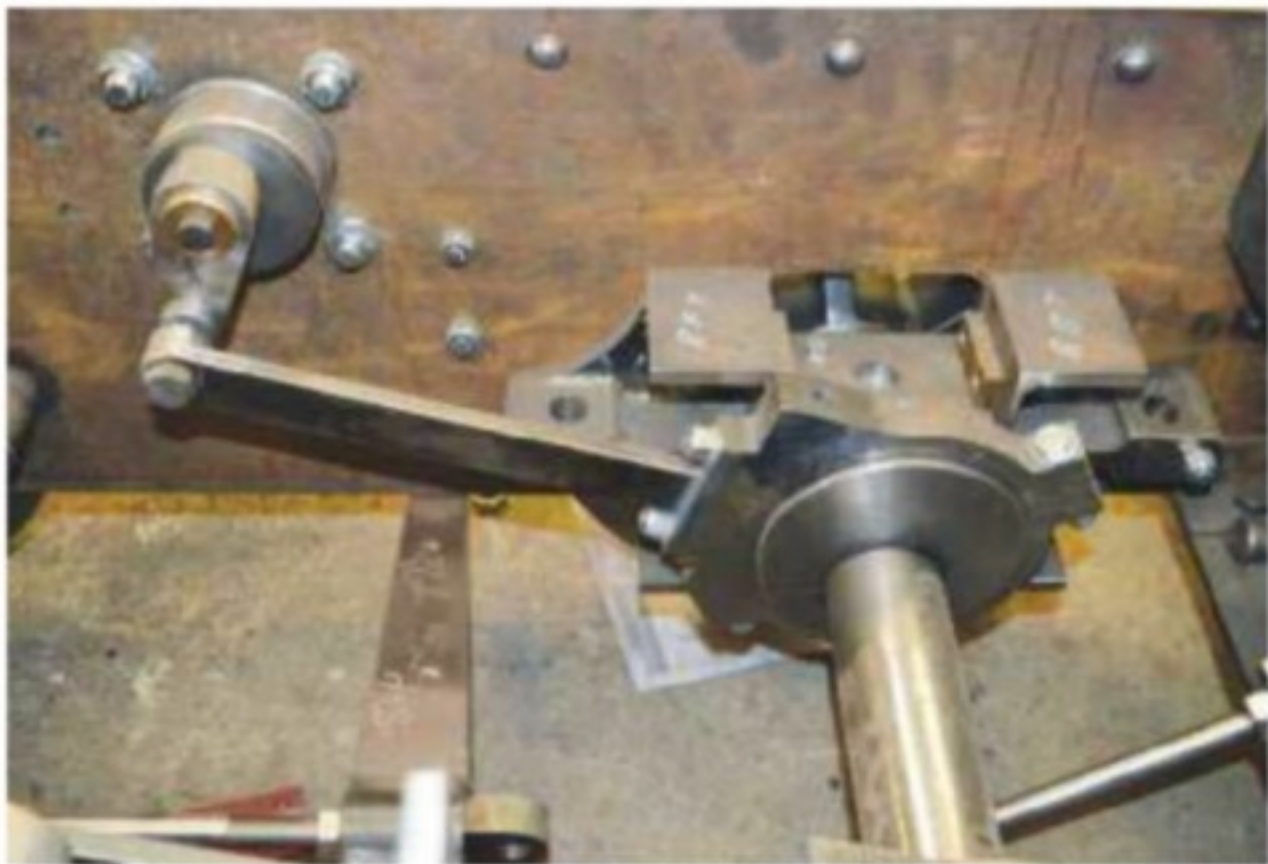
By May 2017, the eccentric rods had been connected up to the bellcranks carried by the 'wobble' (combination) bearings associated with Bagnall-Price valve gear. This is the right hand eccentric, eccentric rod, bellcrank and 'wobble' bearing.
