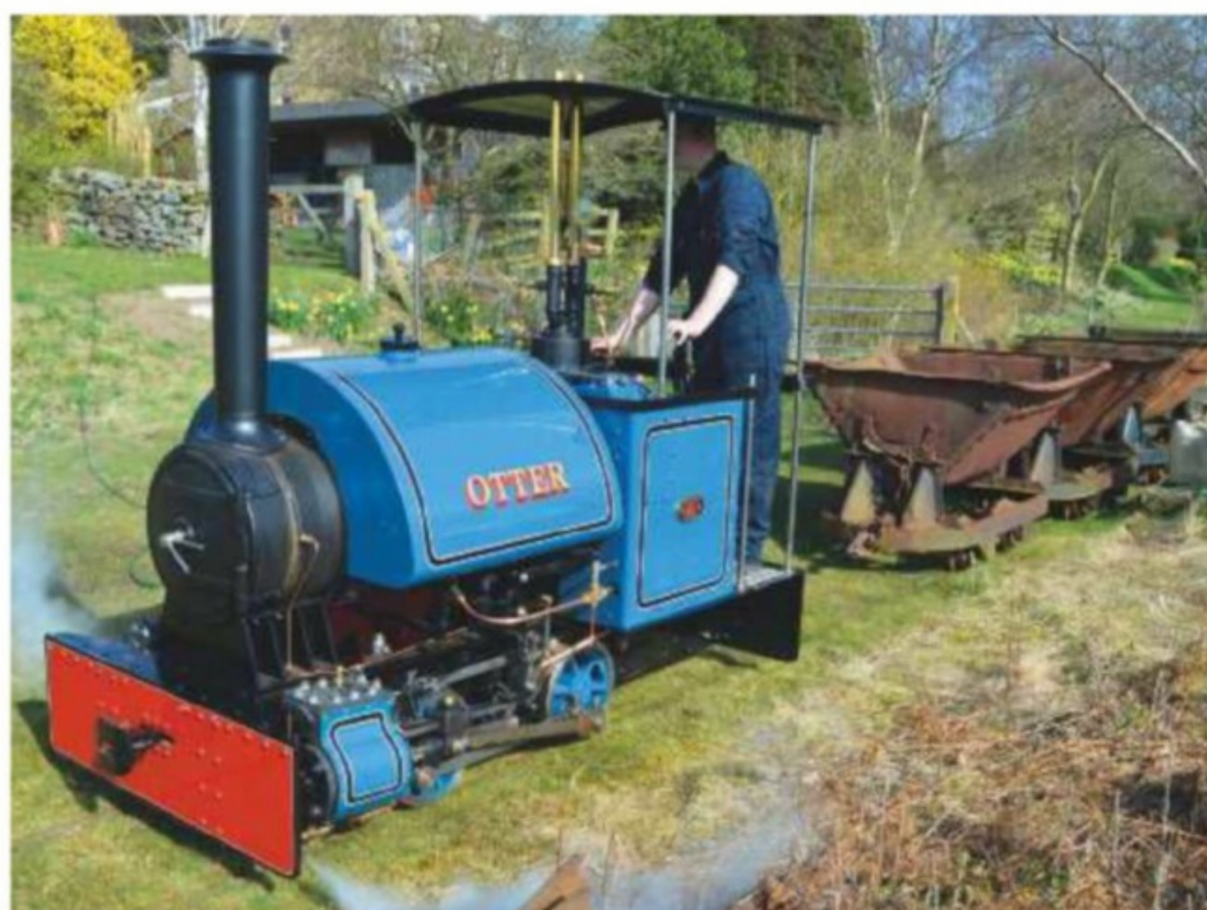
Otter moves off away from the test track's watering facilities following the re-filling of its 35 gallon capacity saddle tank.
