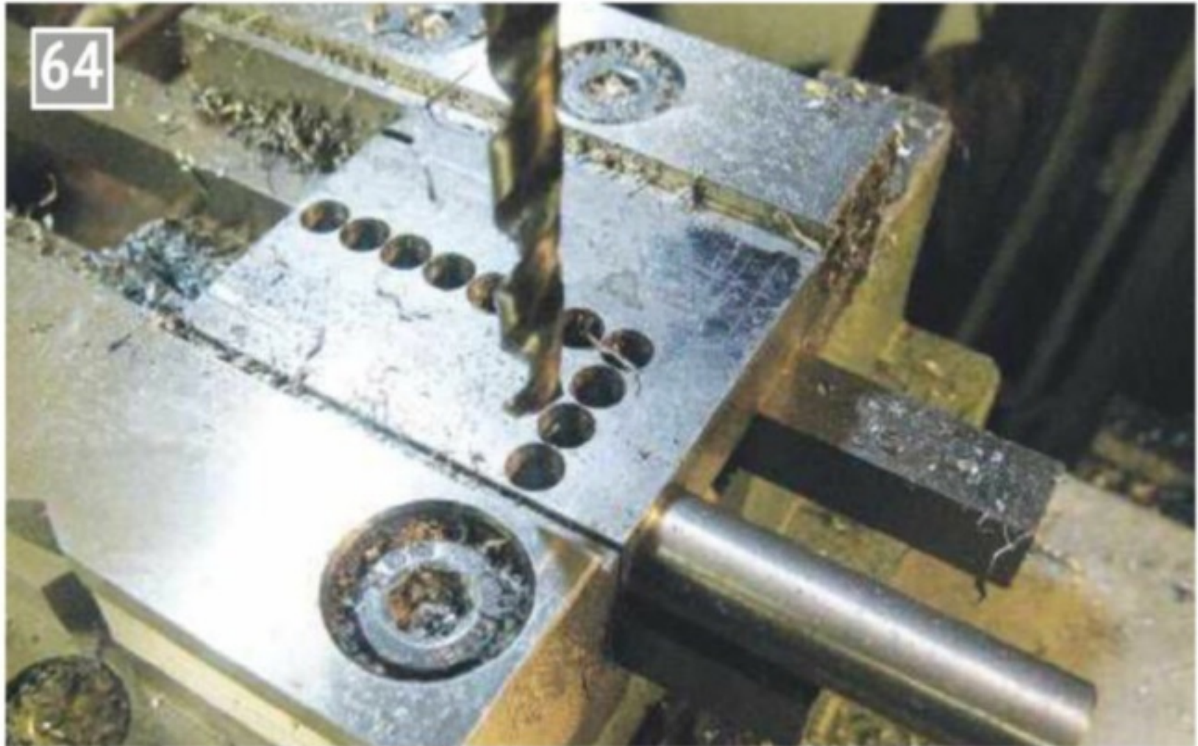
Chain drilling the waste.
