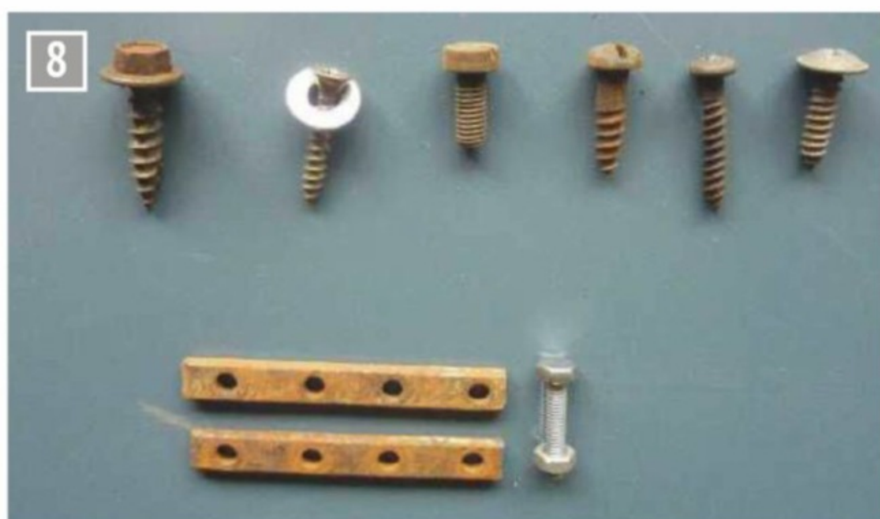
Some rail fixings. The coach screw at left is now favoured mainly for its hexagon head. Flat screwdriver slots are a pain while posidrive slots soon fill with silt making them hard to remove. Note there is no need for stainless steel. Some of these fixings are more than 30 years old.
