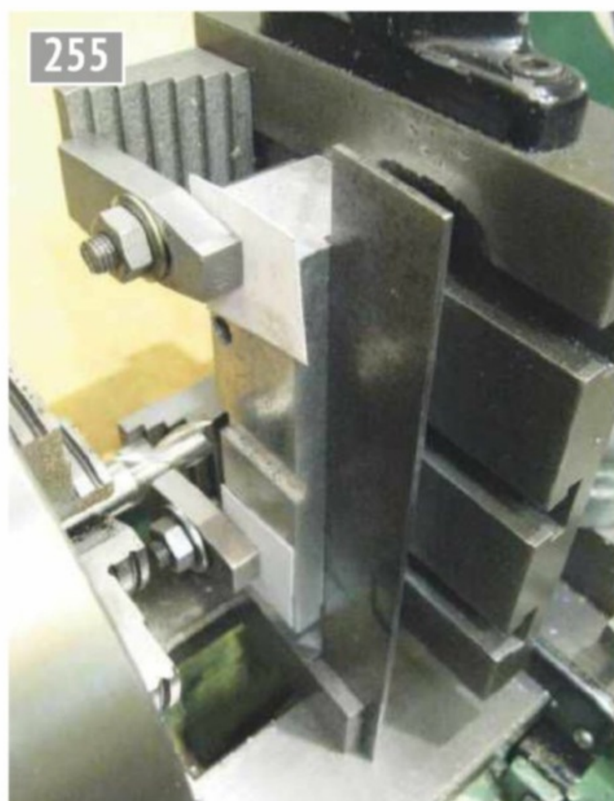
Setting the bar vertical to machine the tenon slot.
