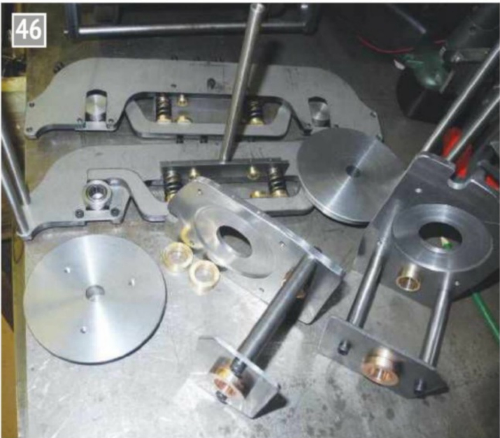
Bogie parts gathered together for assembly.
