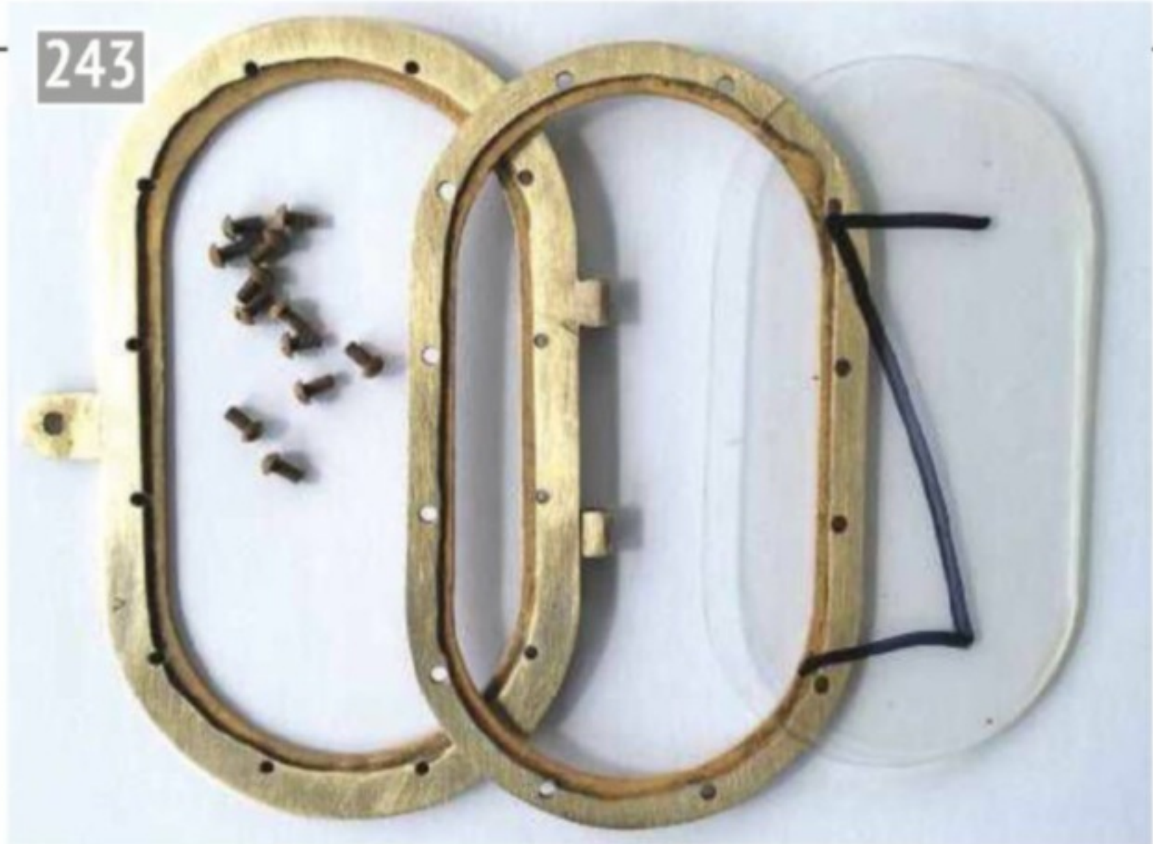
Window frame components.
