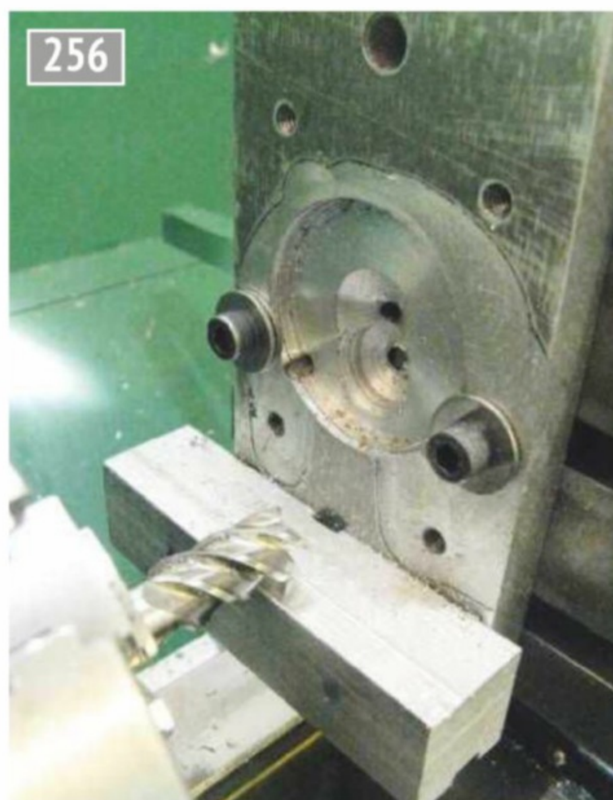
One setup for finishing the angle bar true. The setting plate is well used! This would be better done by clamping the bar onto the cross slide.
