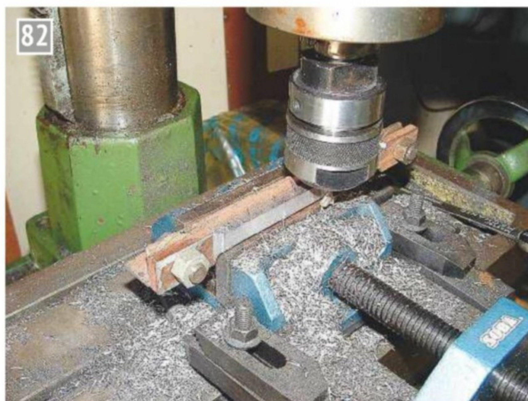
The rod is turned through 90 degrees to be thinned down.
