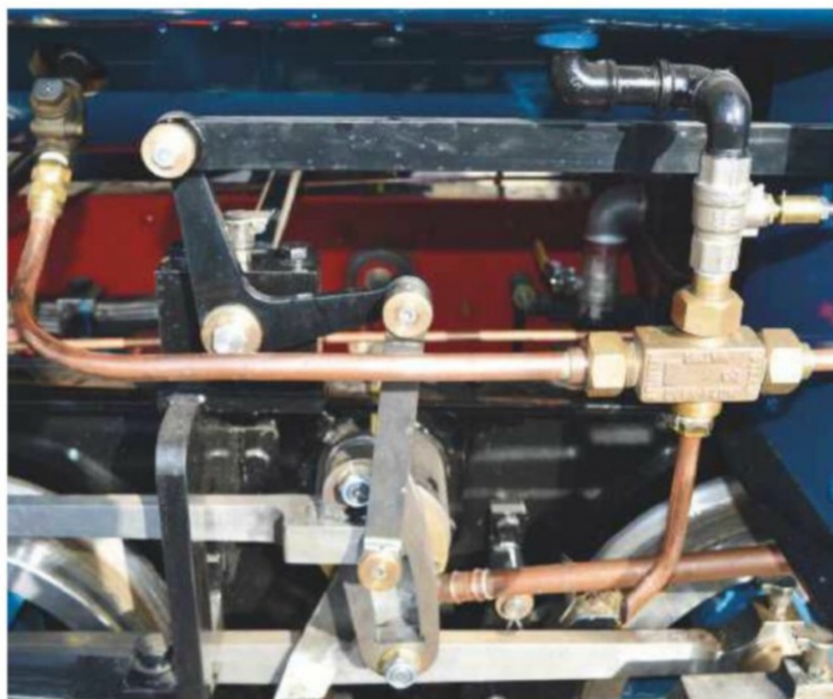
A close-up of the injector pipework, reach rod and upper part of the valve motion on the left hand side.
