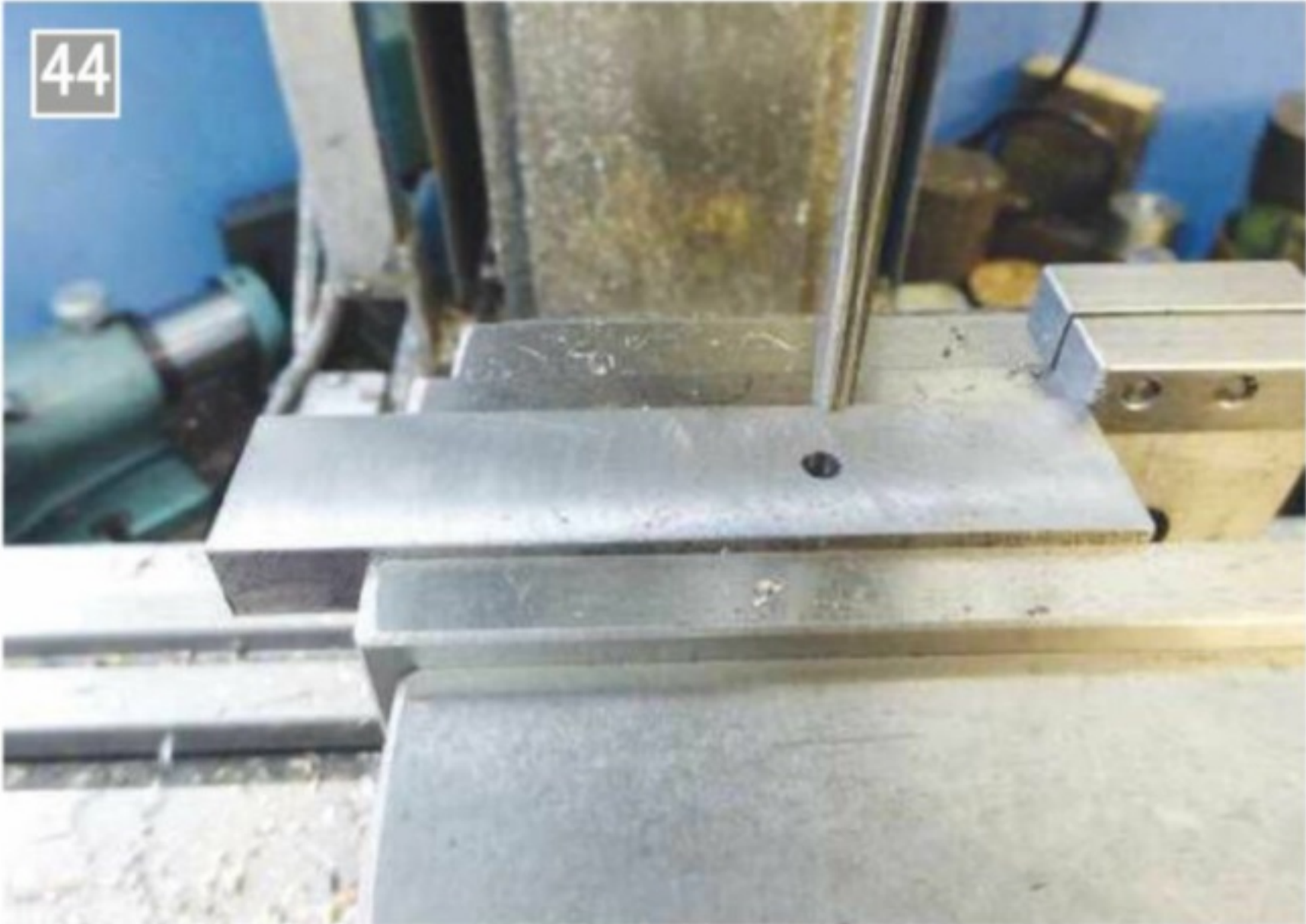
Reaming the conrod for the crosshead pin.
