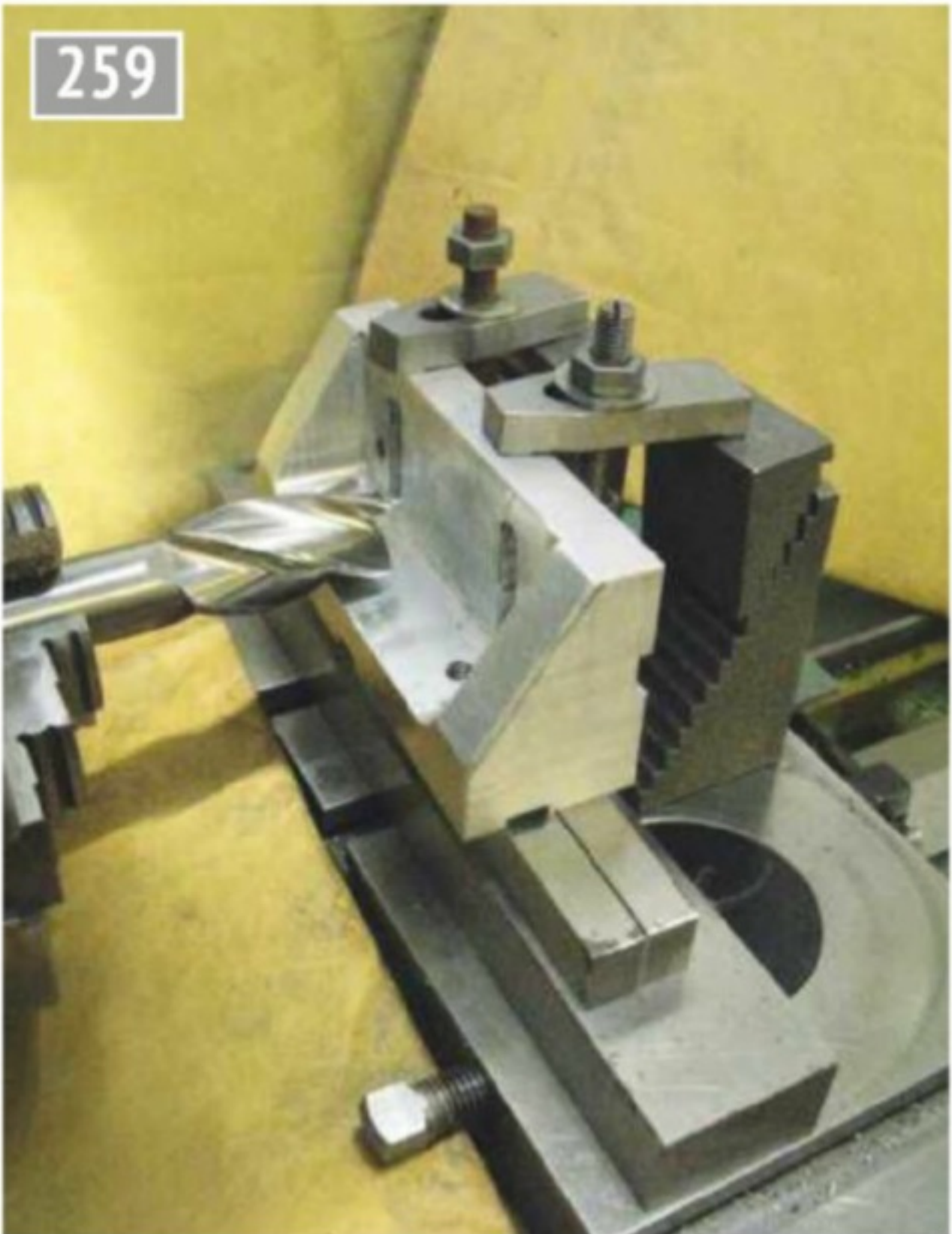
Removing mass from the large angle plate. This will need several setups and perhaps finishing by hand.
