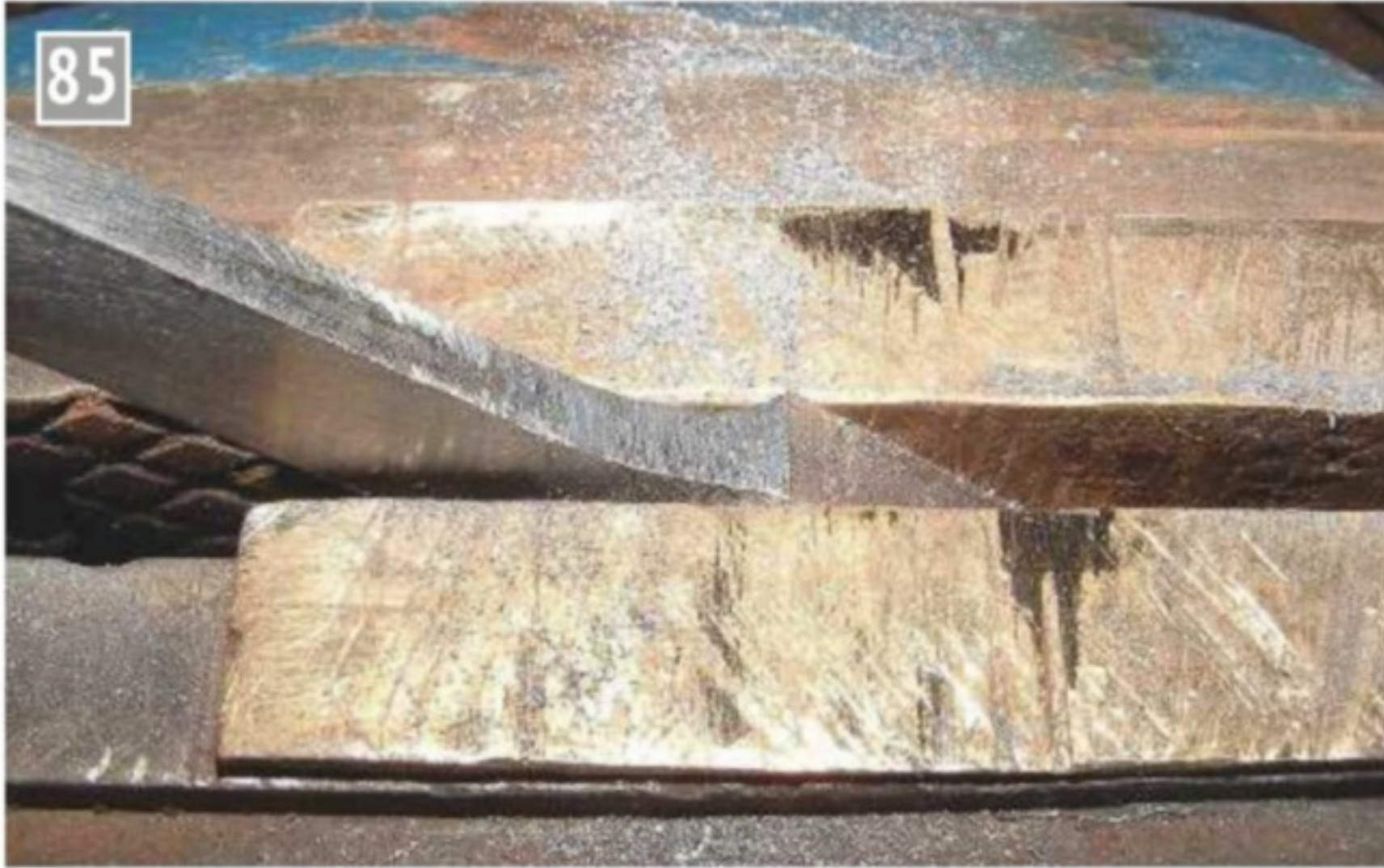
Rod gripped carefully in the vice for shaping the end.
