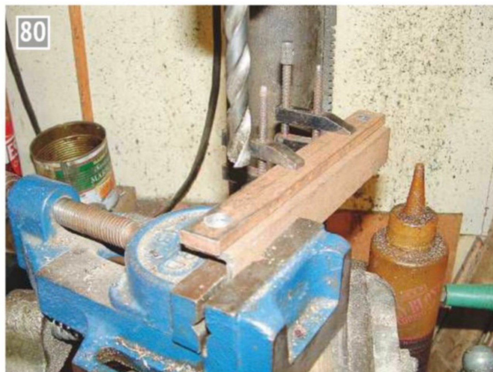
Making a coupling rod drilling jig from a piece of angle.
