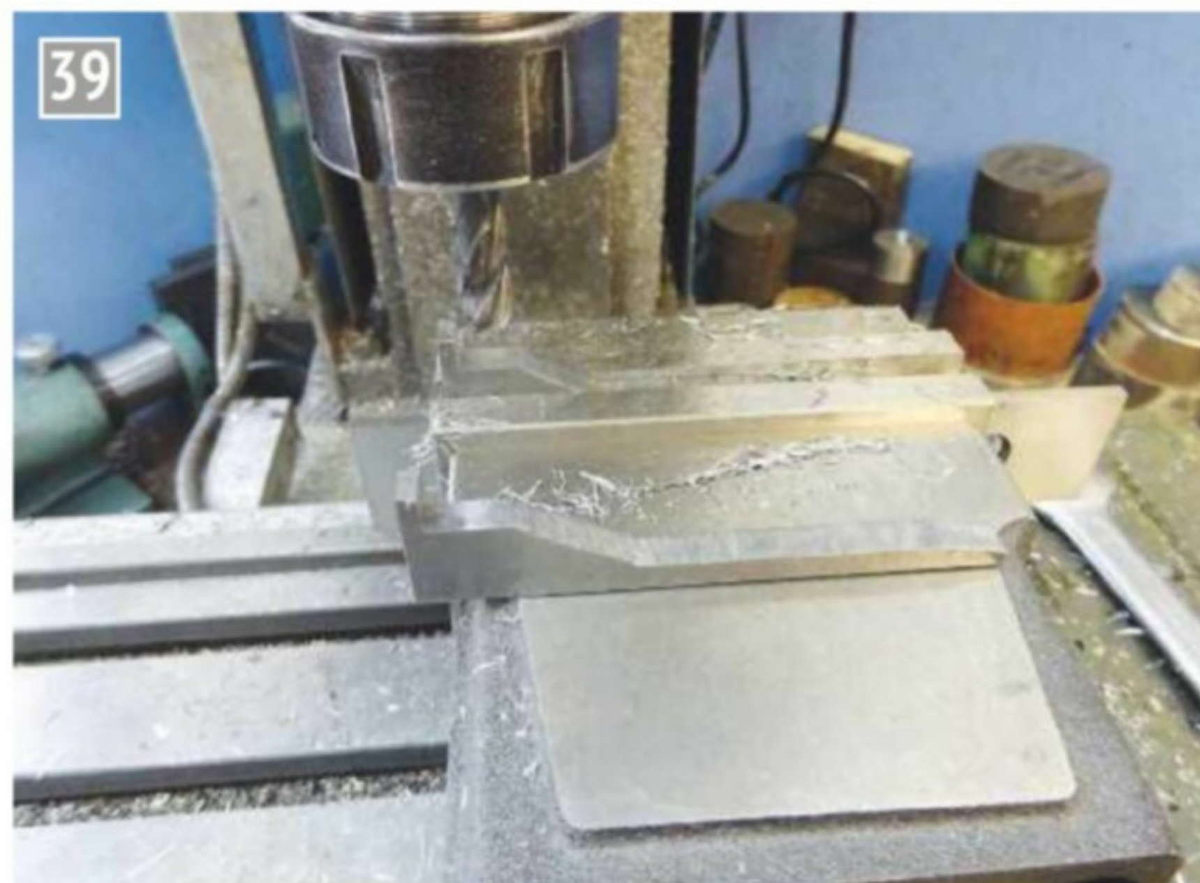
Milling the top leg of the guide.
