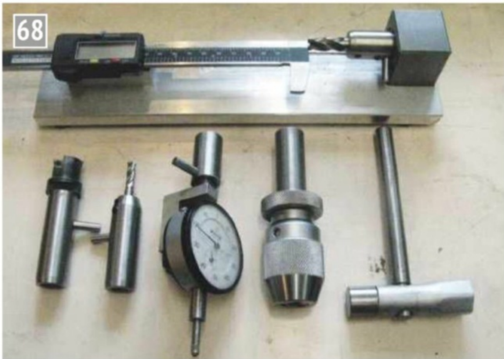
The complete system. Setting jig with tool holder being measured, fitted with my tool no. 4 (6mm end mill), indicator setting probe, drill chuck and spindle box spanner. Note the hammer weight on the spanner, which is stored in a tube on the miller head.
