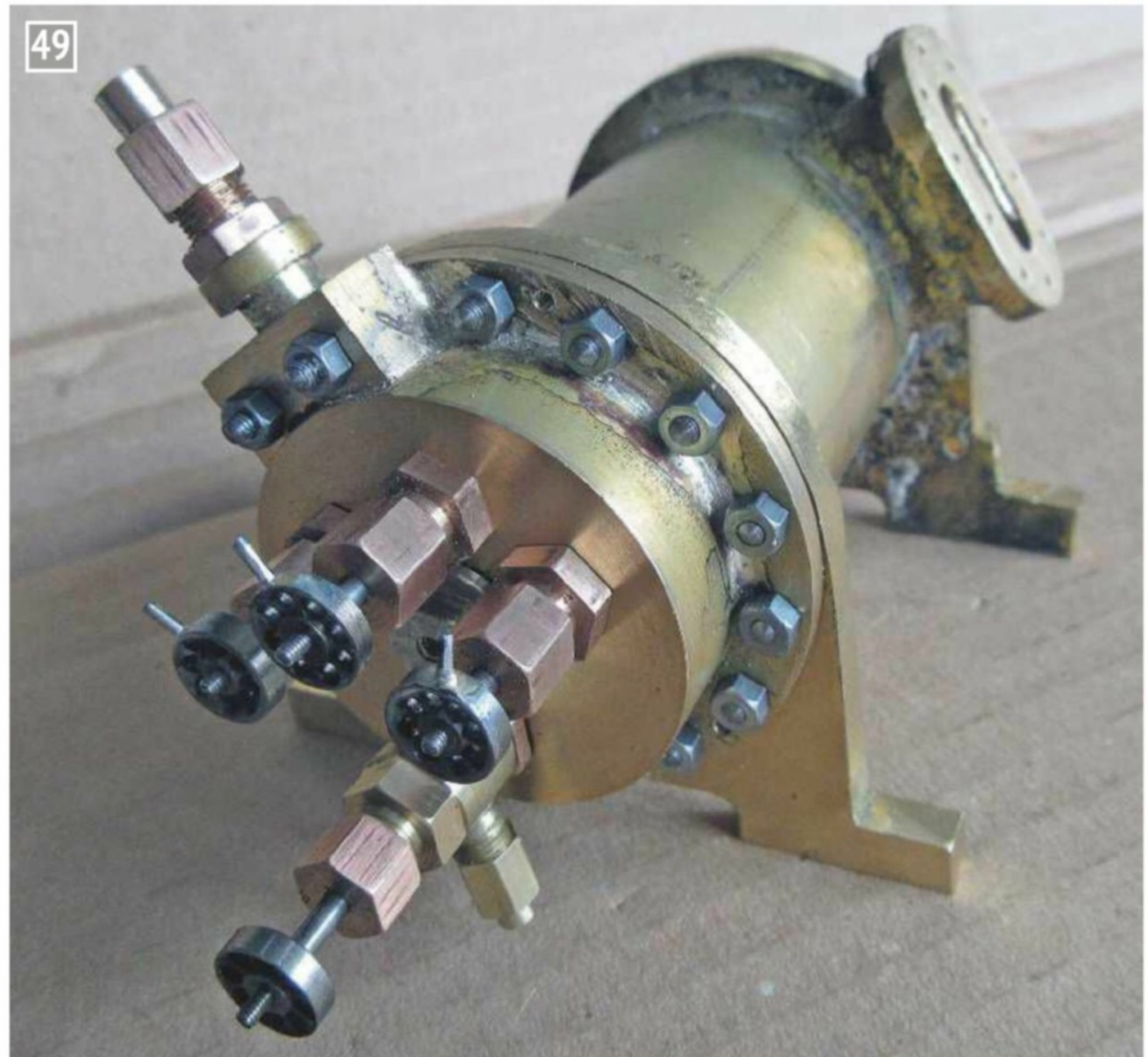
Partly constructed multi-stage turbine.
