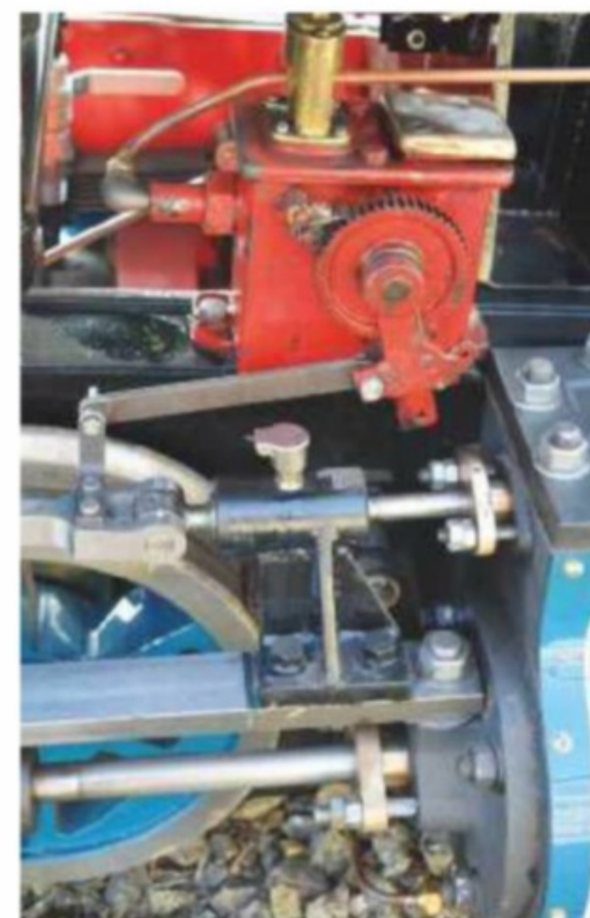
This mechanical lubricator, fitted on the right hand side close to the leading wheelset, was not a feature of the original design.
