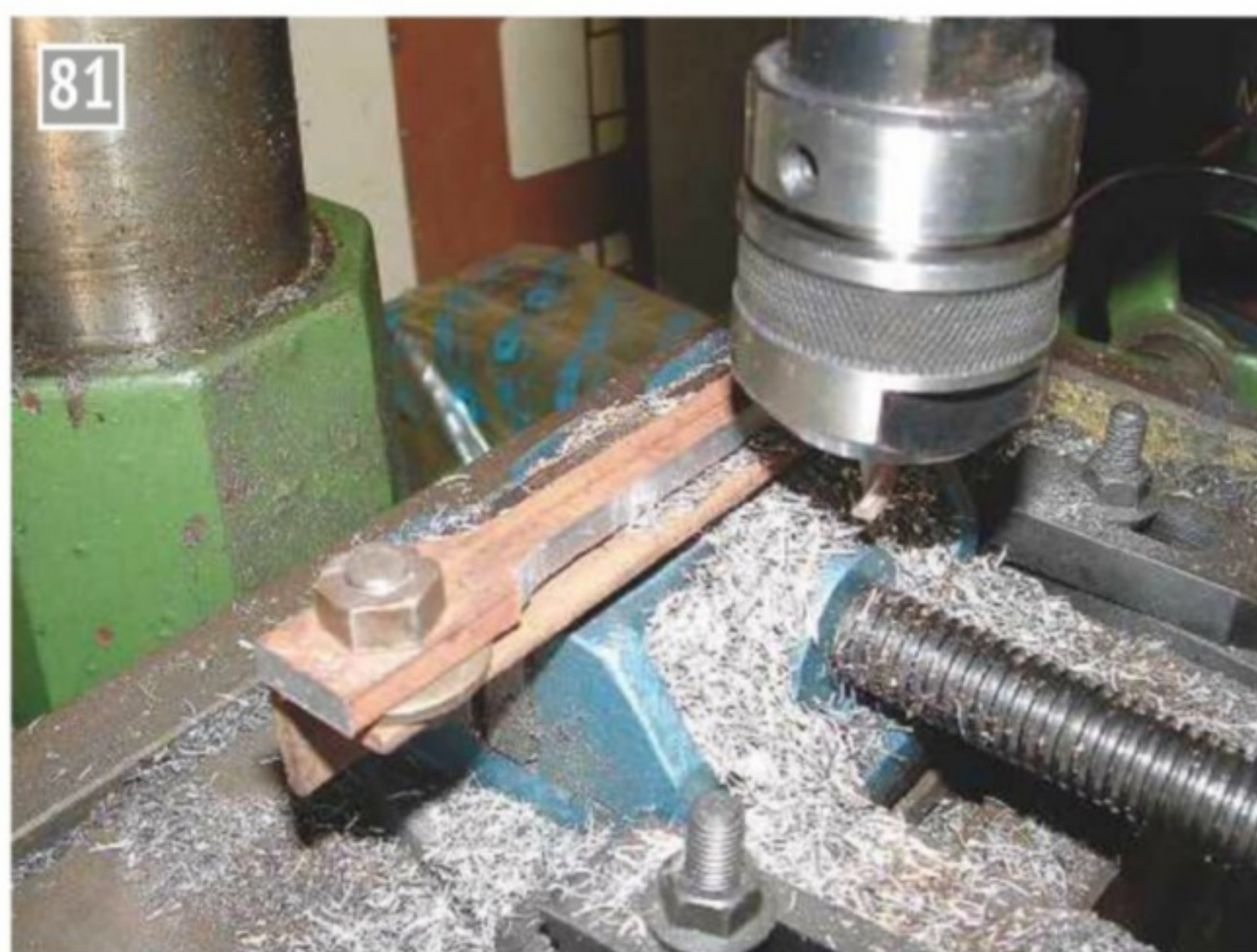
Starting to form the outside shape of a coupling rod.
