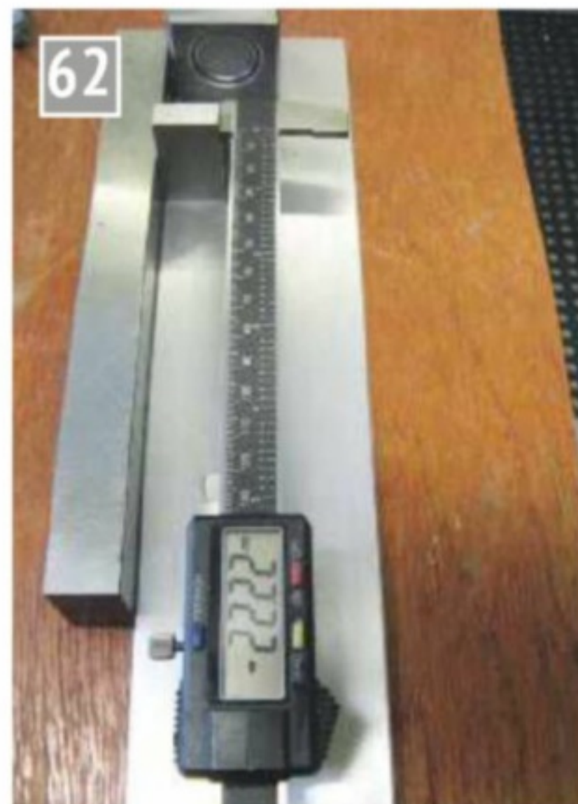
Setting the gauge scale parallel.
