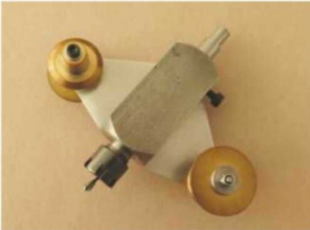
Make Keith Johnson's Pointmaster jig for sharpening small drills.
