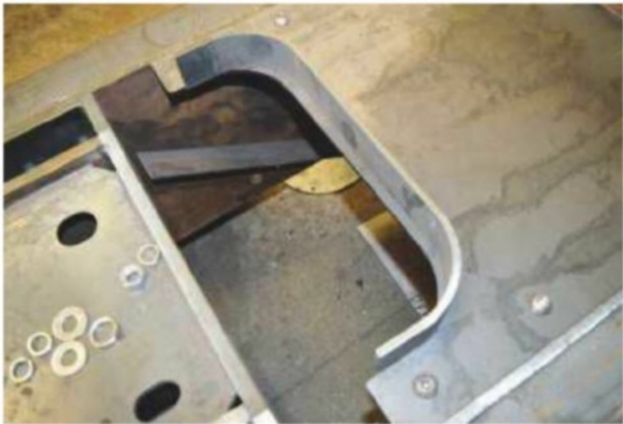
The rear portion of the firebox stretcher can be seen to advantage in this view, together with the leading central part of the footplate and ash shield. With this type of boiler, ash can only be removed from the rear of the firebox.
