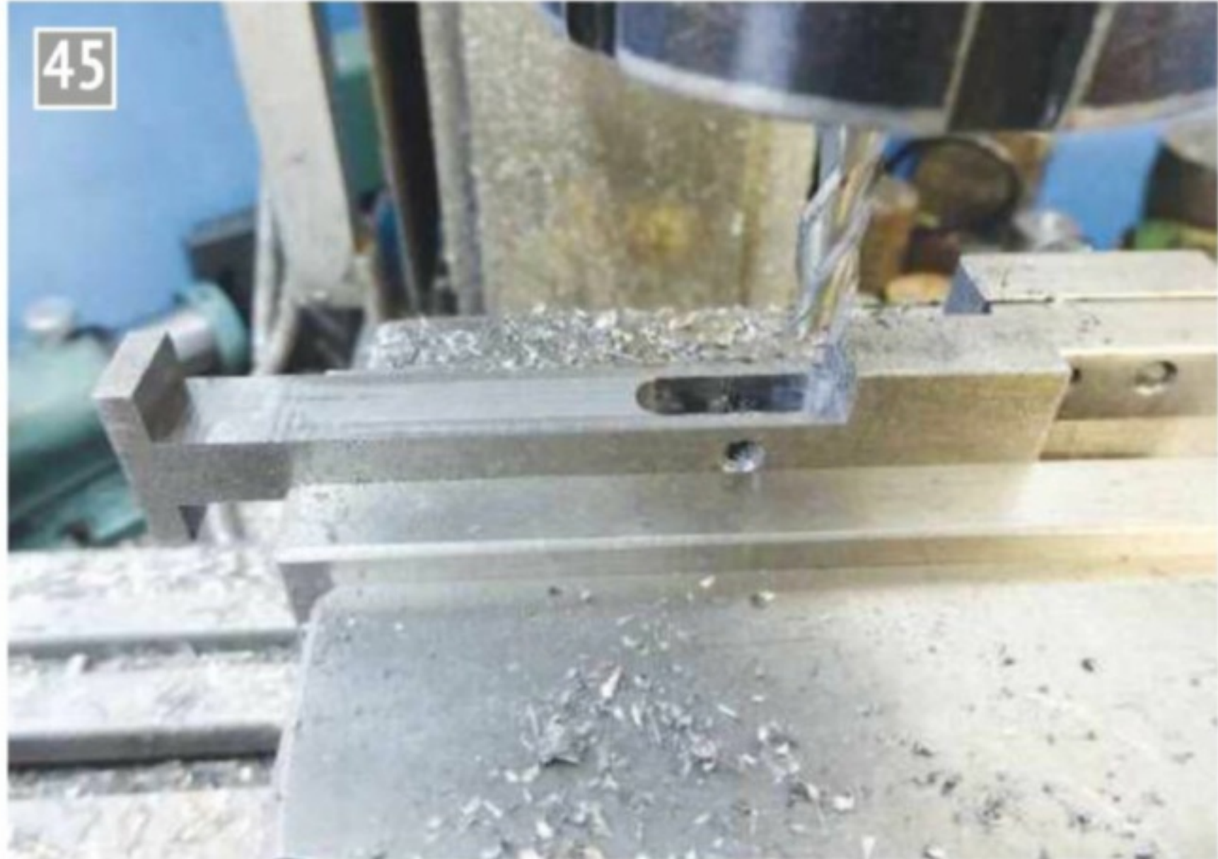
Milling a fork slot in the conrod.
