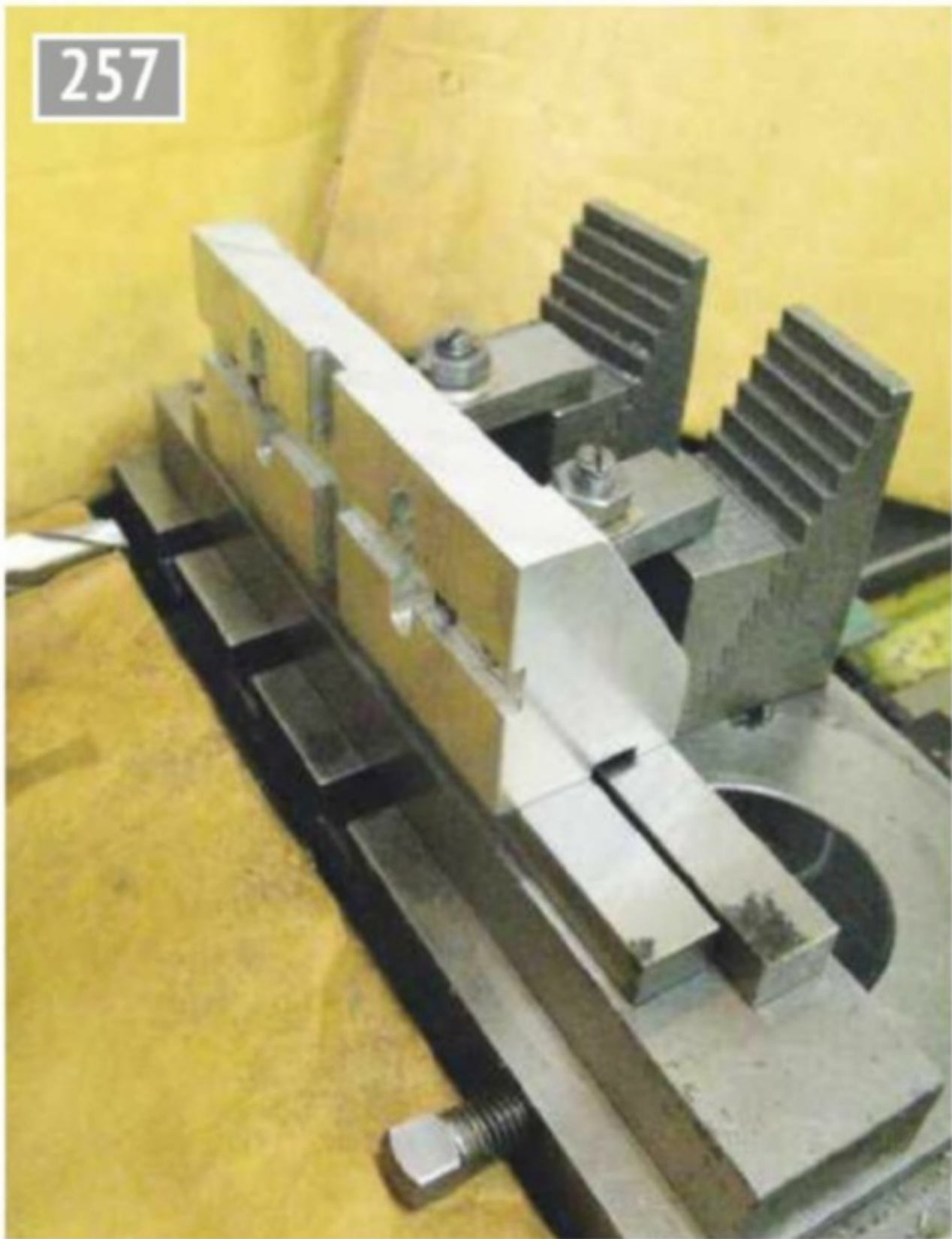
Facing then cutting the tenon slots in the angle plate - do this before cutting the pocket.
