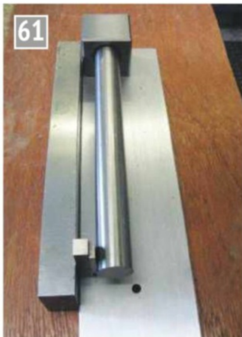
Setting the block parallel on the jig.
