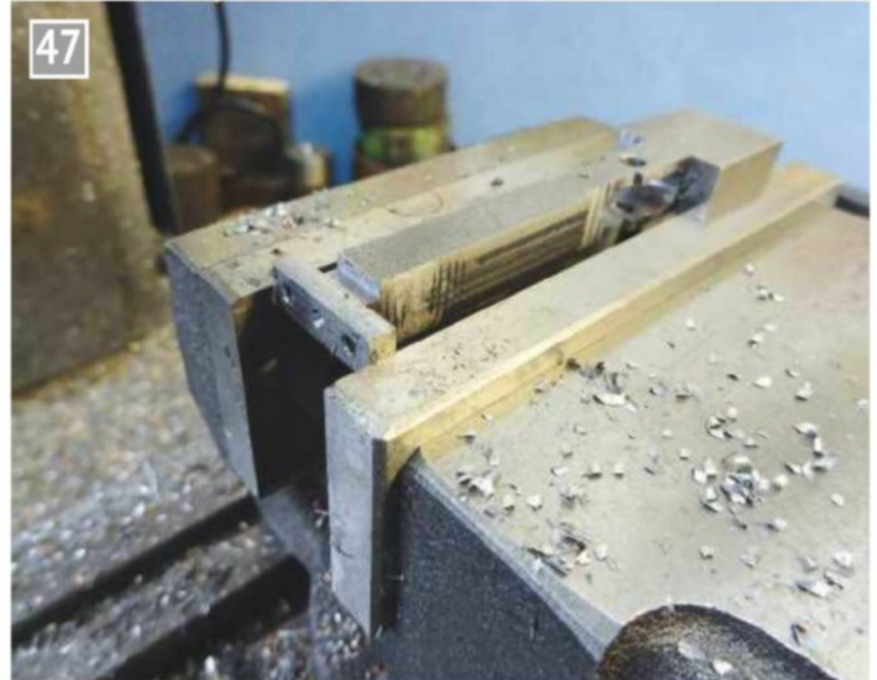
Cutting the palm down to thickness.
