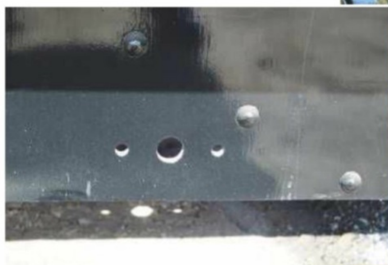
The original plans of the Sipat mainframes were followed closely with the result that this set (mirrored on the other frame) can be seen at the rear end. They should be noted by prospective modellers of the original design as they originally carried the bearings for the hand-worked cylinder draincock control cross-shaft.
