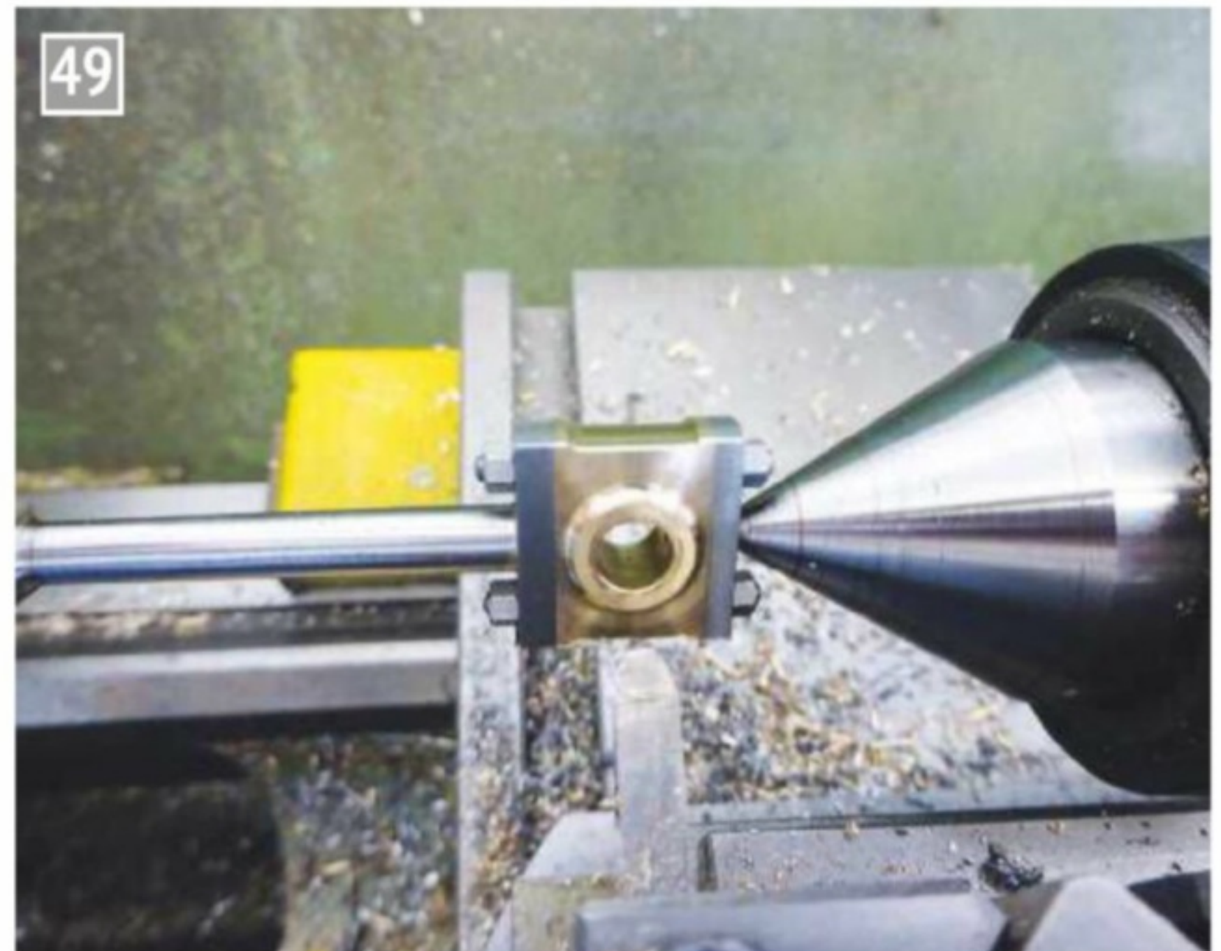
Rounding the assembled big end parts.
