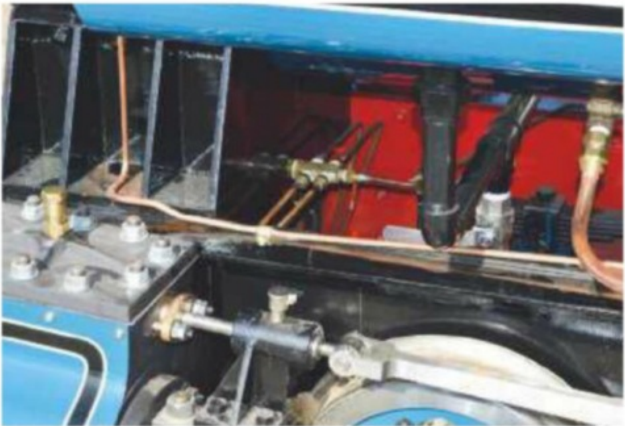
Unlike the original Sipat design, Otter is fitted with steam operated cylinder draincocks. The pipework for these is seen in this view, taken on 21 April 2019. Also visible in this view is the pipework for blower and the tank level equalisation and drain pipe.
