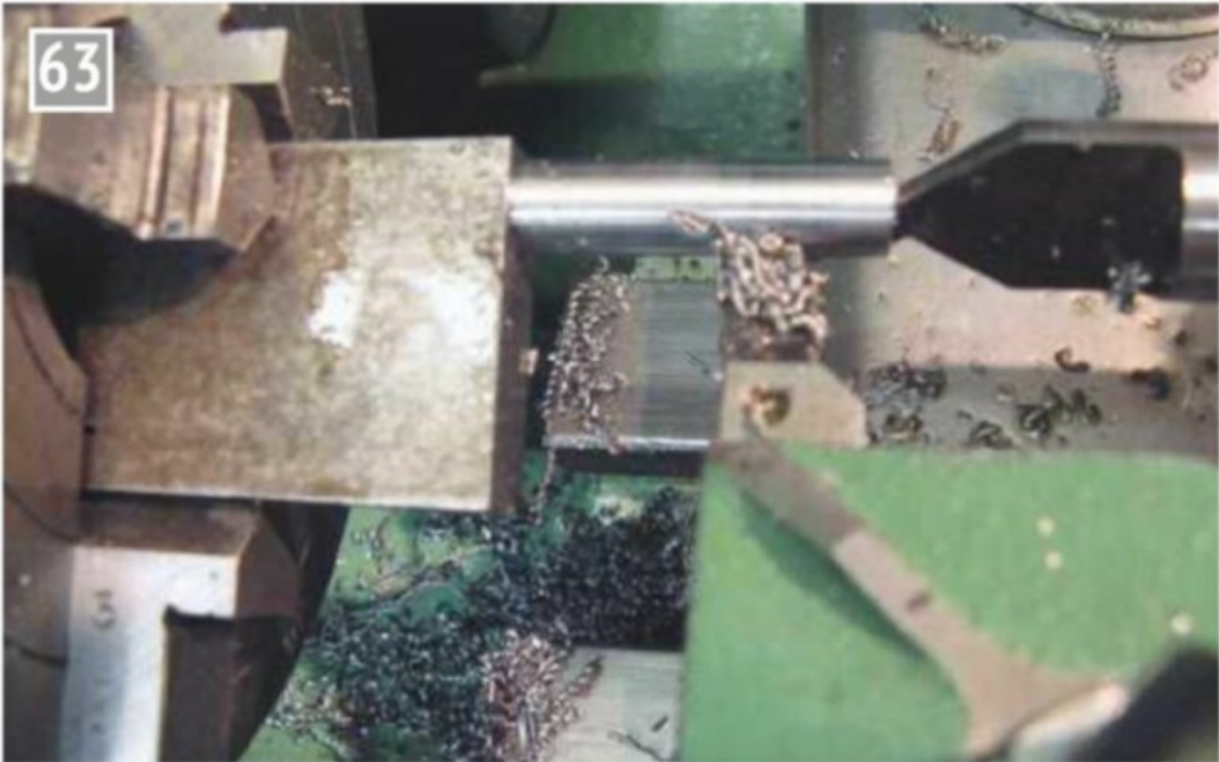
Turning the spigot on the DTI mount.
