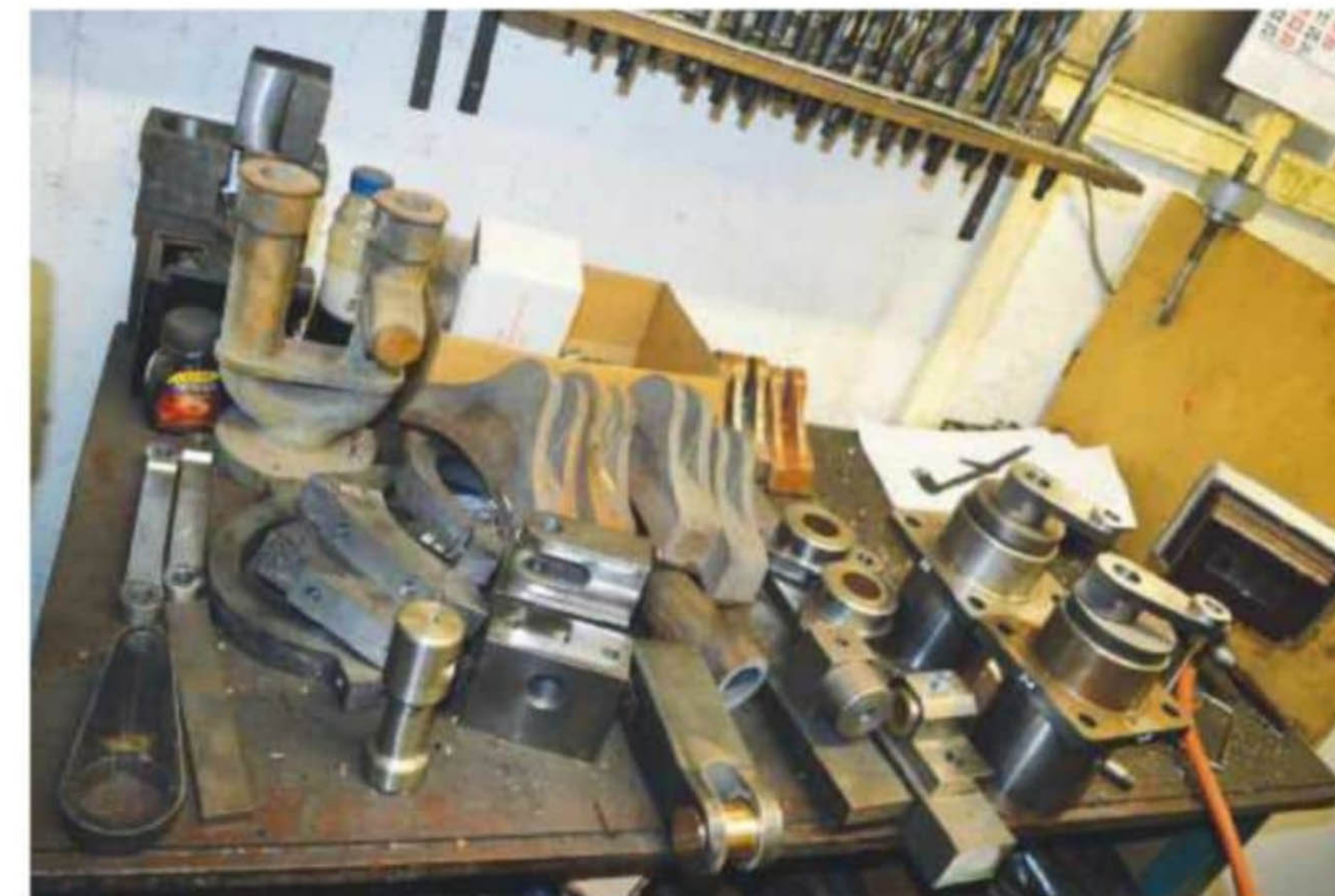
Various components that were later to be incorporated into Otter are seen here in January 2017 in the N.B.R.E.S.L. Machine Shop in Scarborough. They include brake blocks, brake shaft bearings and bellcrank, eccentric sheaves and the safety valve body casting.
