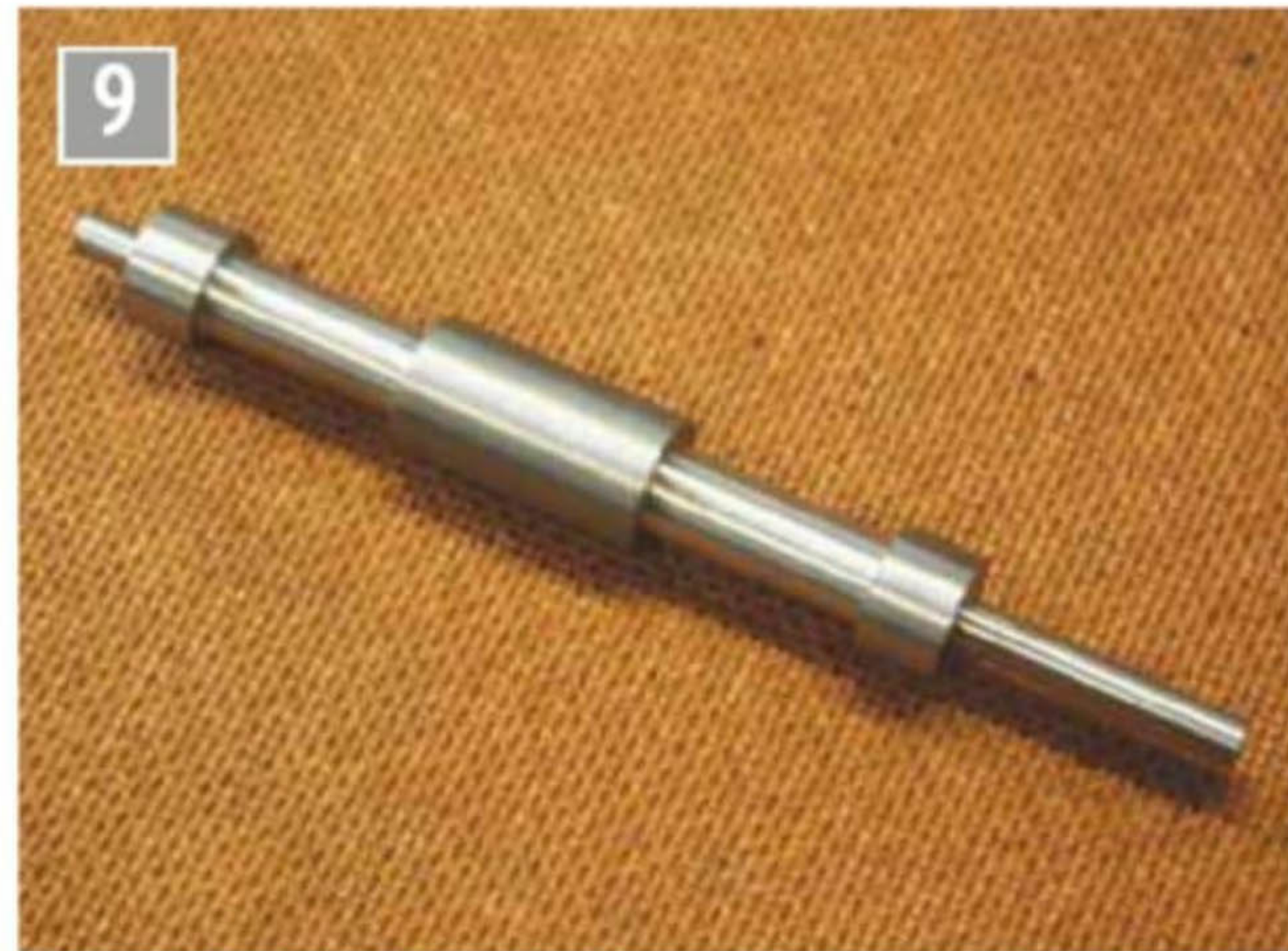
Gear blanks turned double ended.
