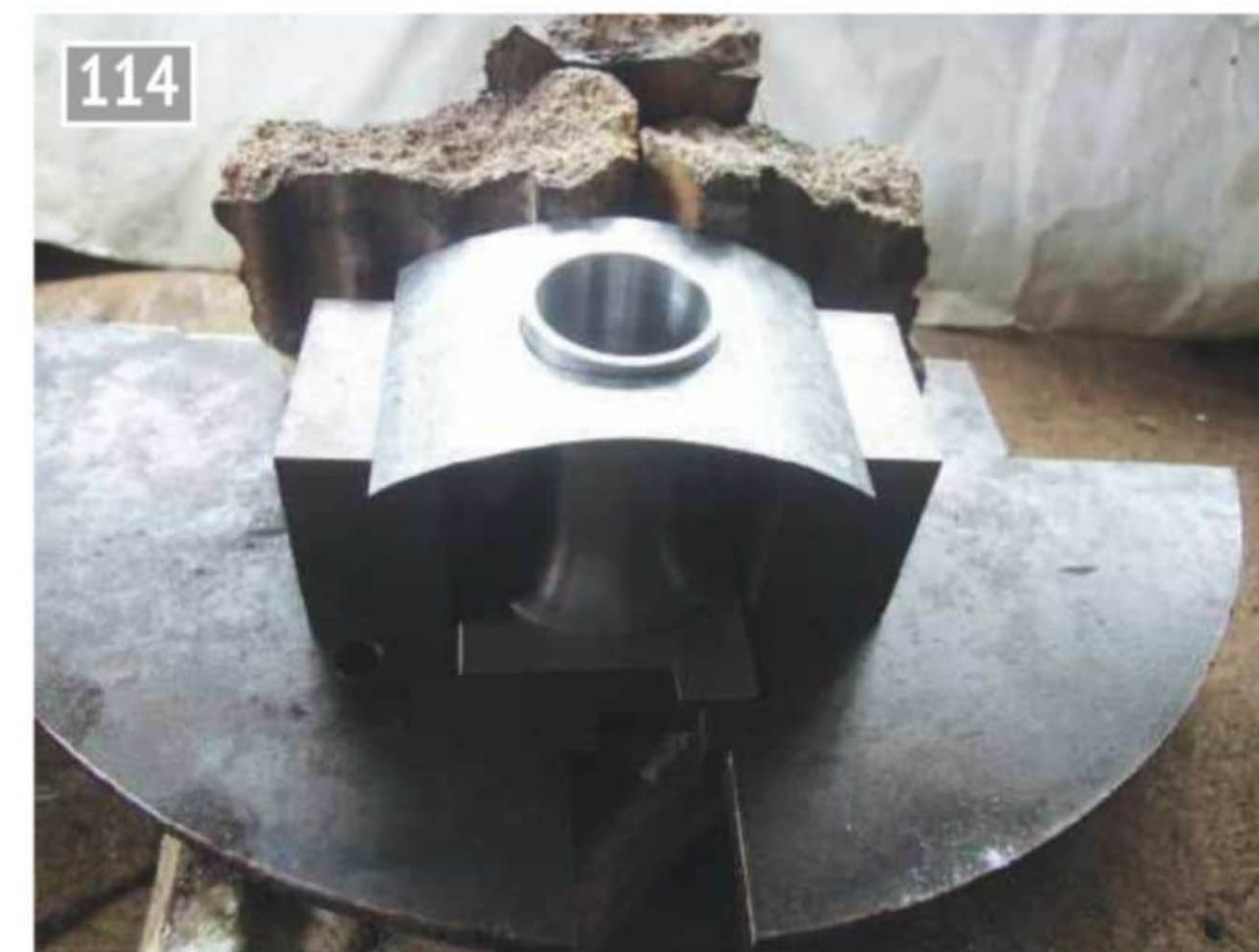
114 Here is the set up for the silver soldering of the petticoat pipe to its mounting plate and the tidy ring of solder at the expense of a very black pipe.
