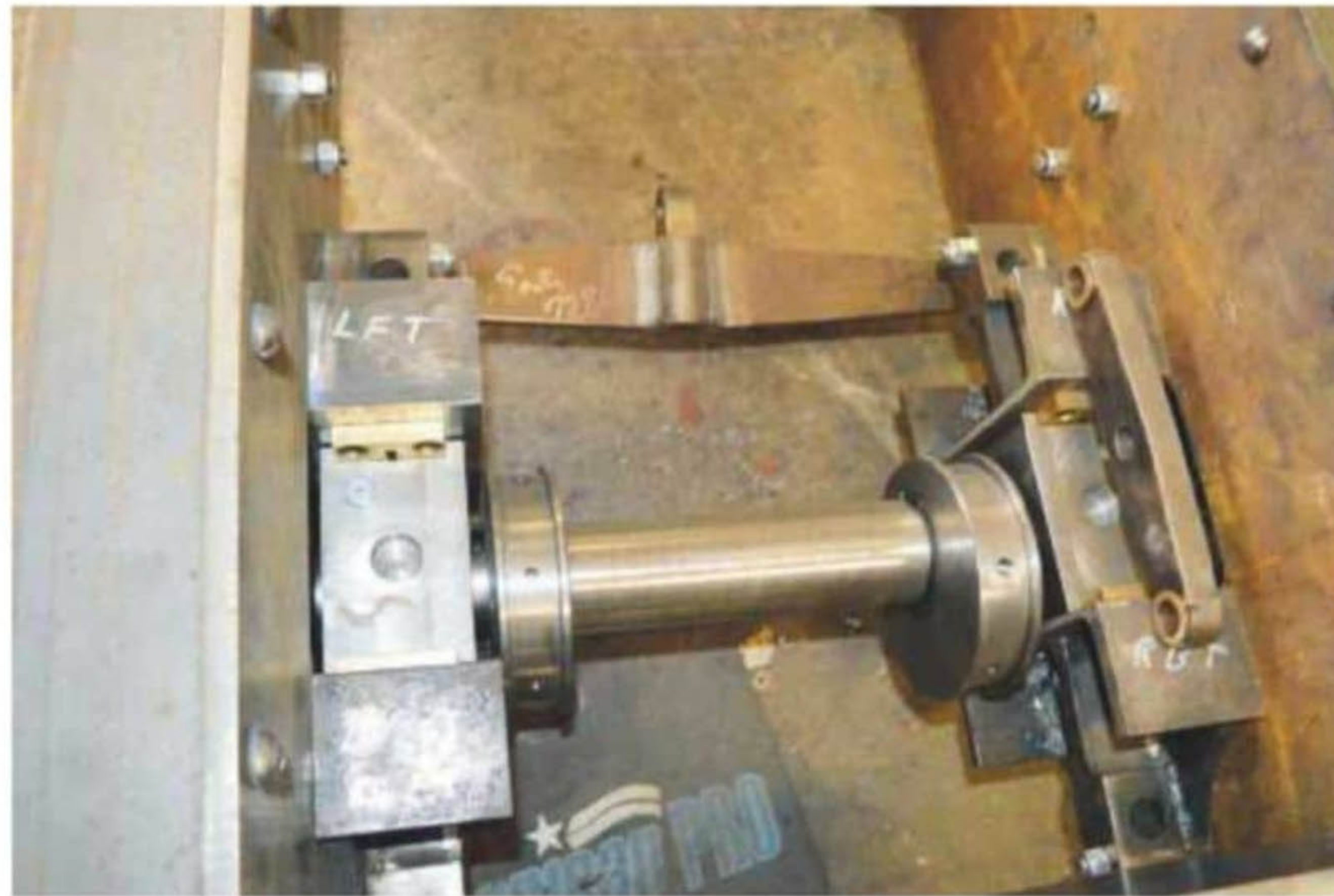
This view shows the trailing axle fitted with the eccentrics, along with its associated axleboxes and hornblocks (again fabricated items) and the rear right hand brake hanger resting on top of its associated hornblock.
