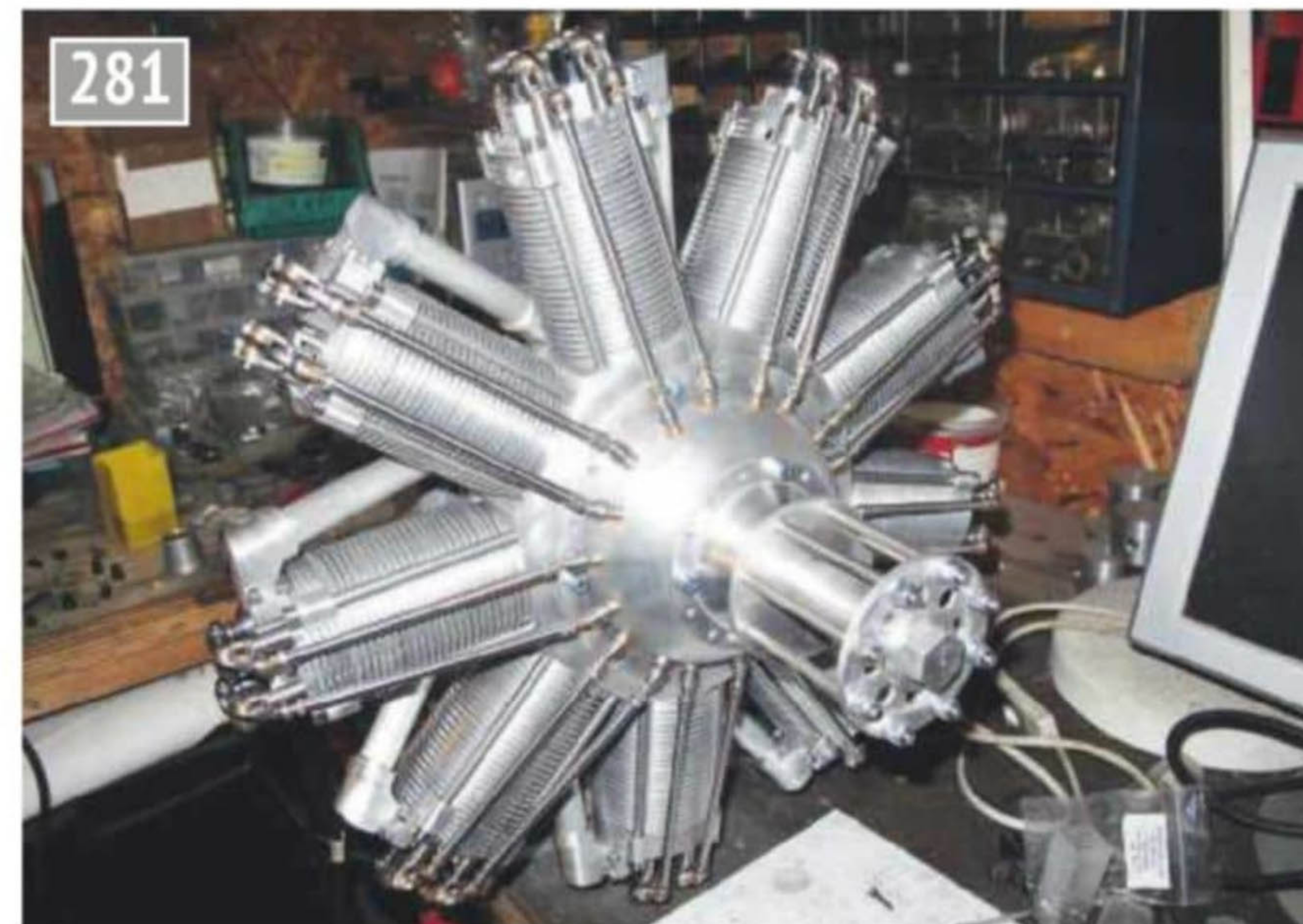
First full engine assembly.
