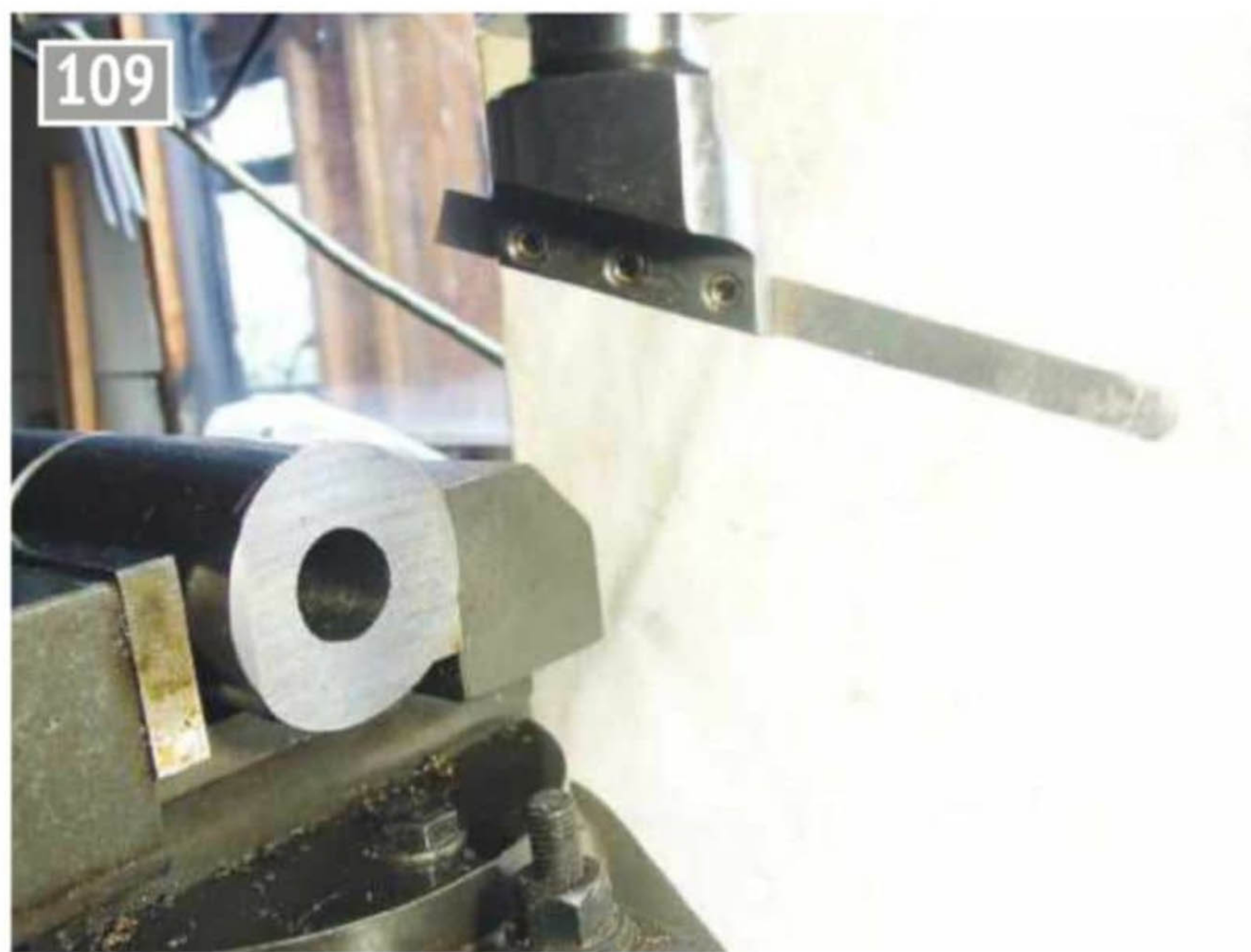
109 The steel bar in the milling machine vice and the rather long fly-cutter used to create the radius under the chimney section. The cutter had to be made from silver steel plate as the standard tool was not long enough!
