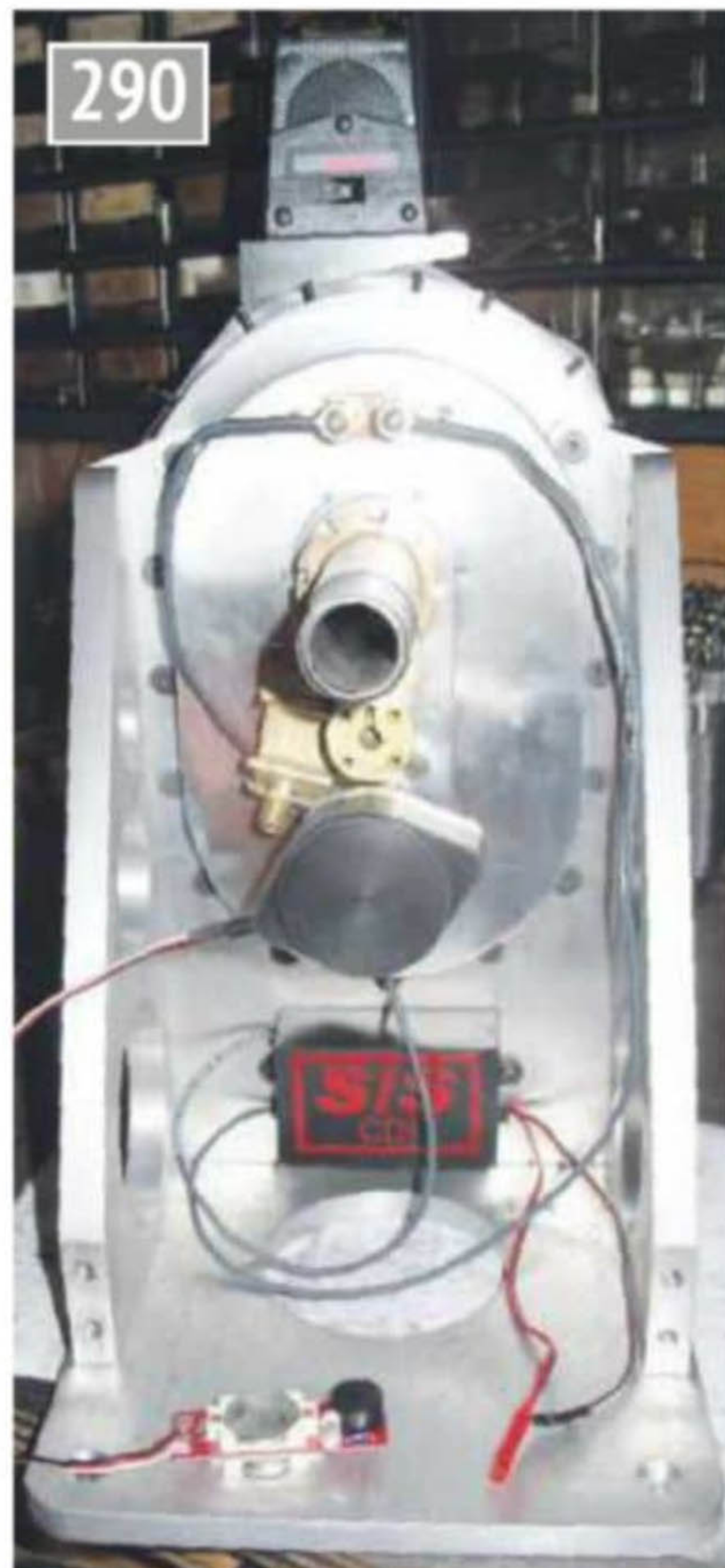
Crankcase set at ten degrees before TDC with timing light attached to the Hall sensor.
