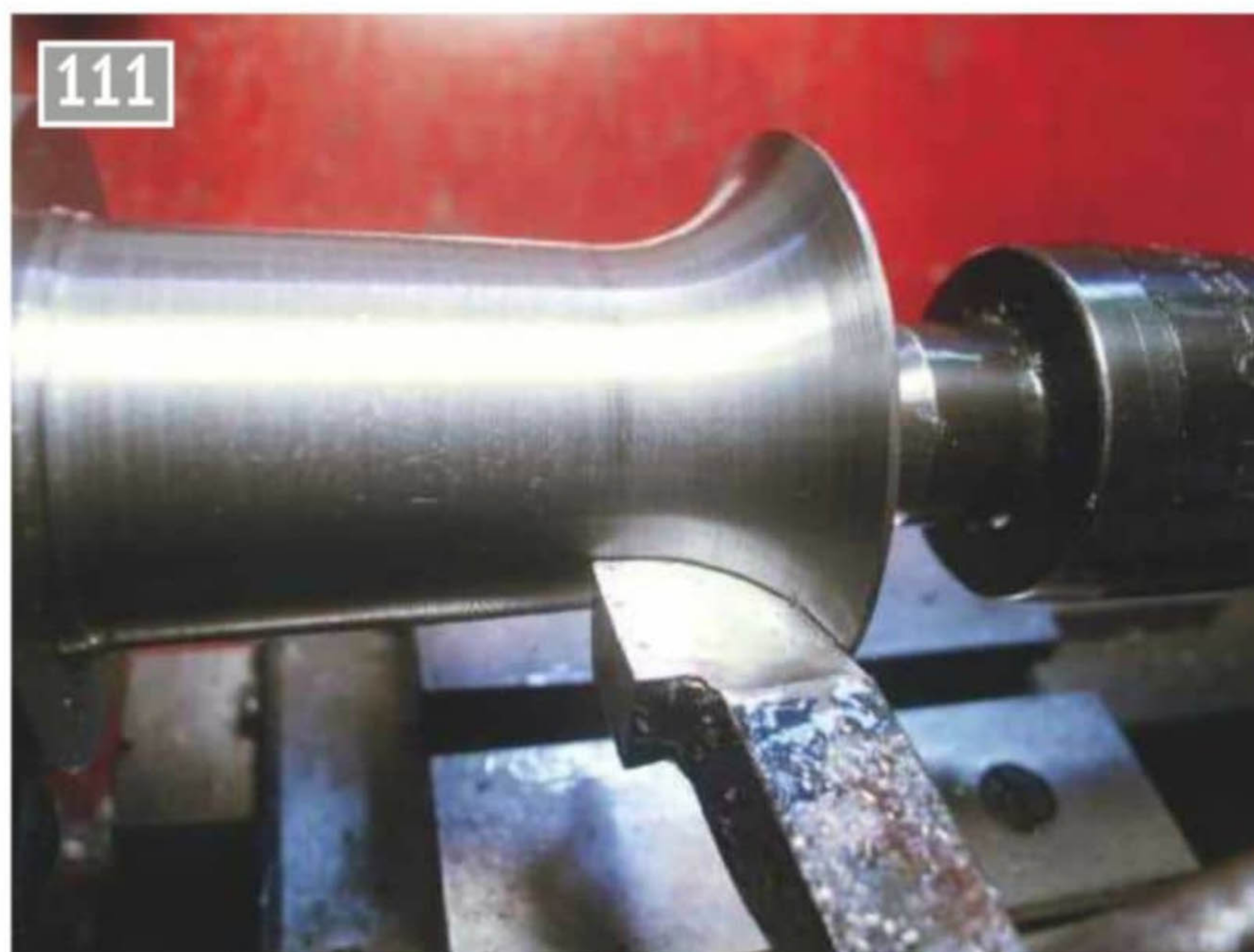
111 The external profiled form tool used to produce the radius on the outside of the flare. This tool was easily made from a standard left-hand tool on the hand grinder.
