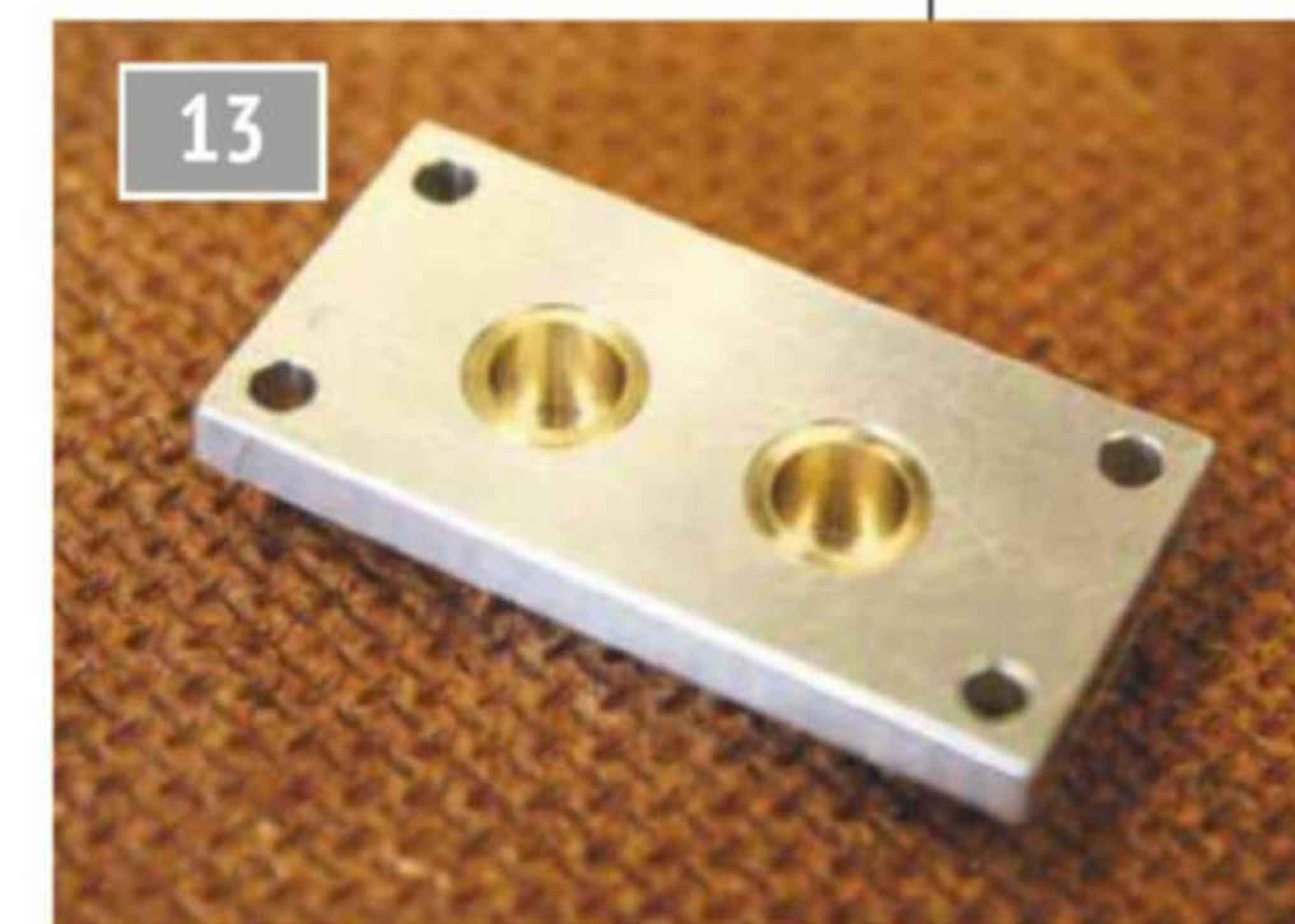
Bushes pressed into gear cover.
