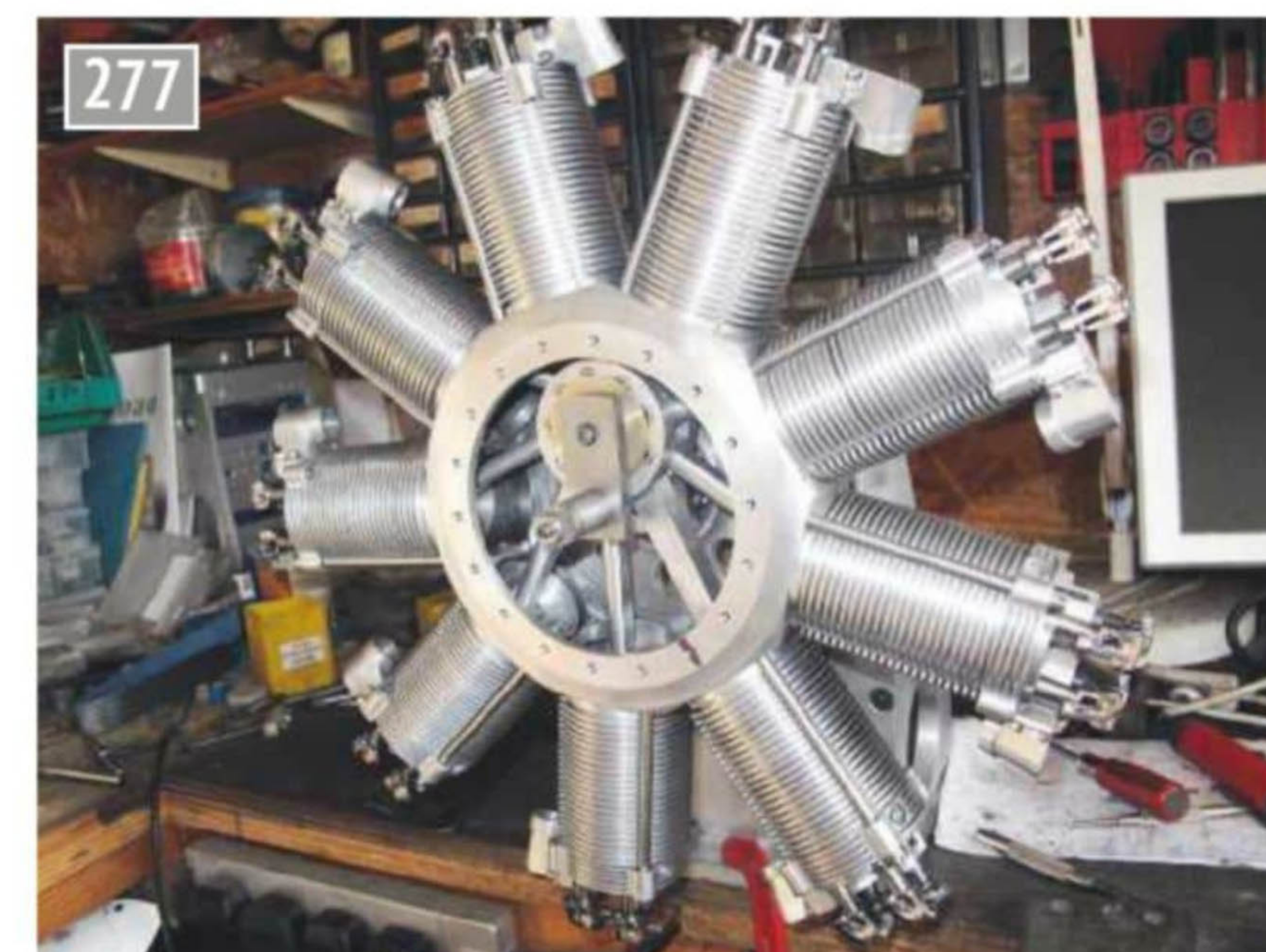
Cylinder heads in place.
