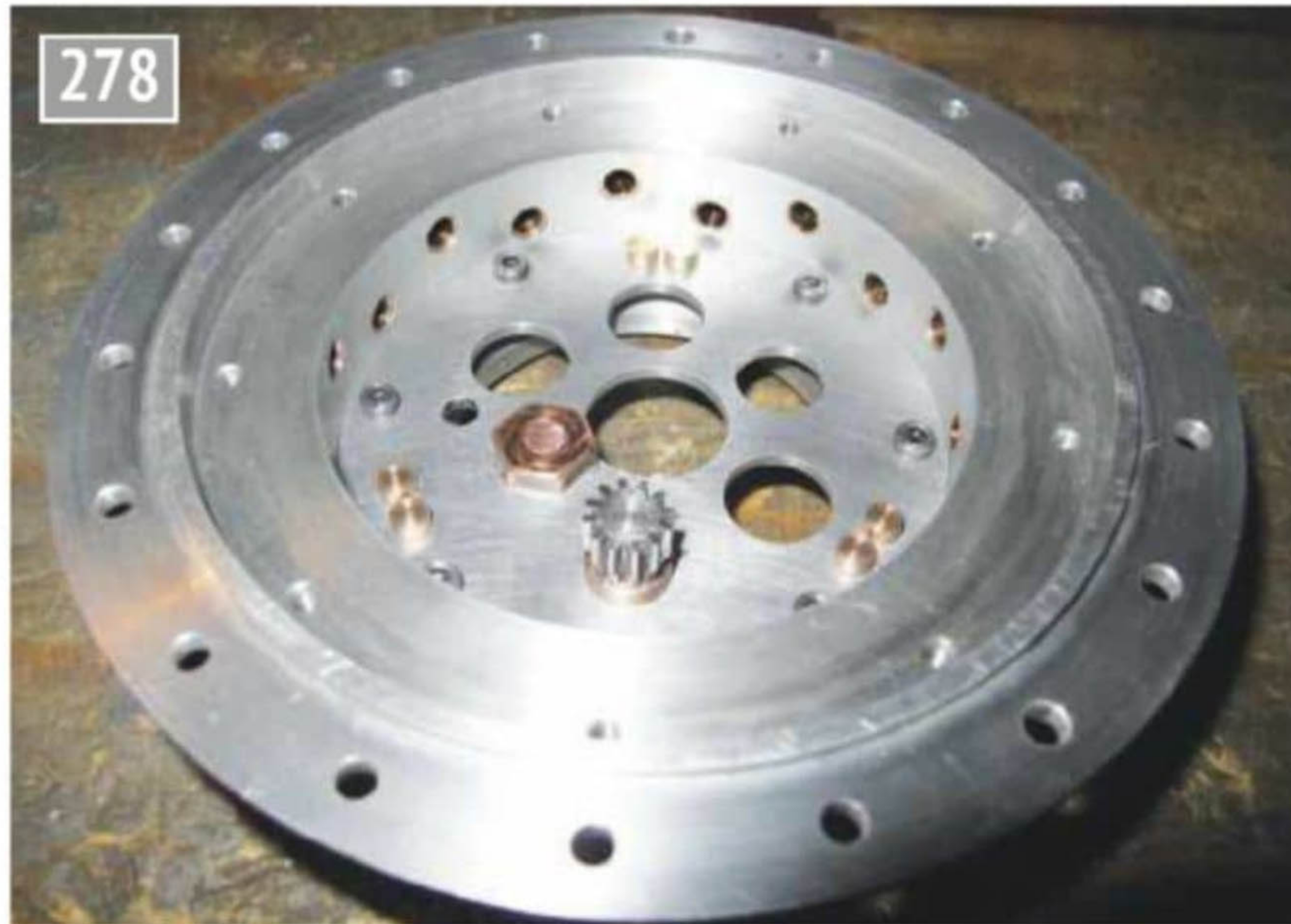
Front cover with its bronze rotary cam positioning pads.
