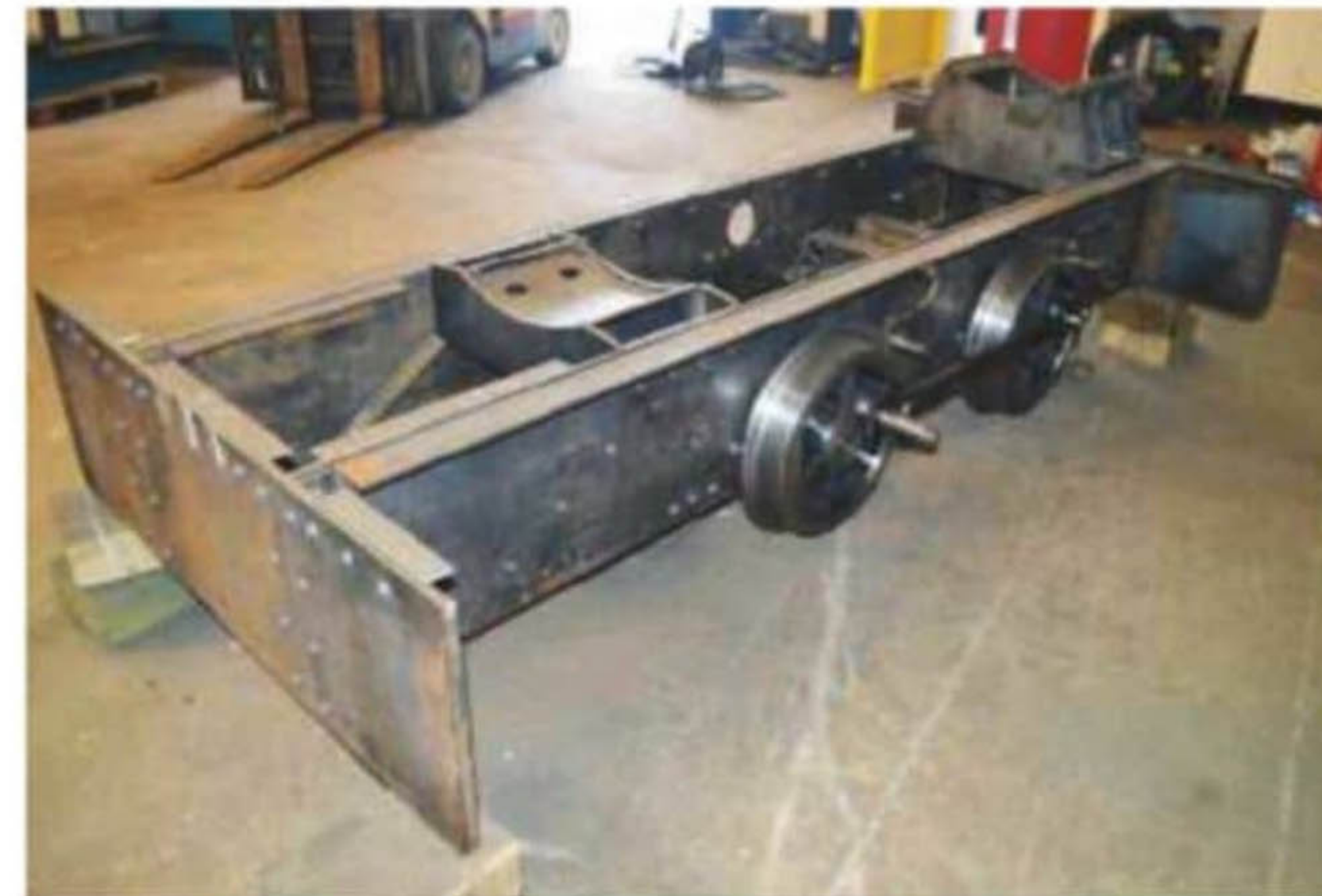
A rear right hand three-quarter view of Otter's chassis in January 2017. This picture gives a good idea of the relative positions of the rear stretcher, the leading axle stretcher and the smokebox saddle.
