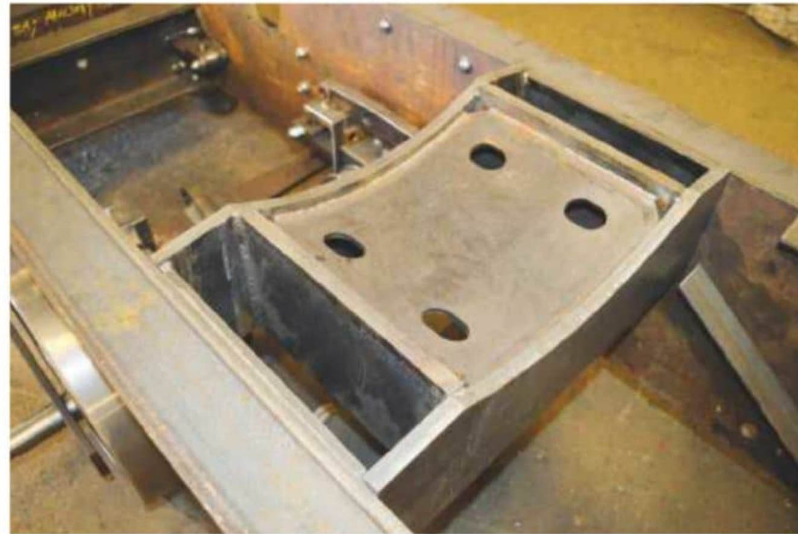
This is the rear stretcher, which supports the 'bullhead' firebox. It is yet another fabricated item.
