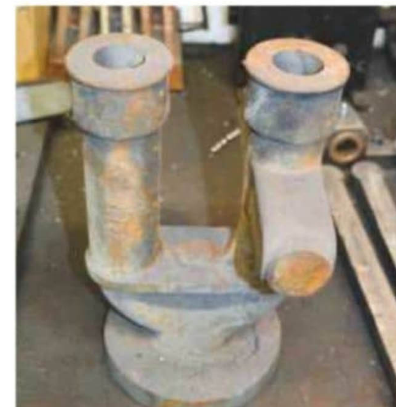
The casting for the locomotive's Ramsbottom safety valve column can be seen to advantage in this photograph.
