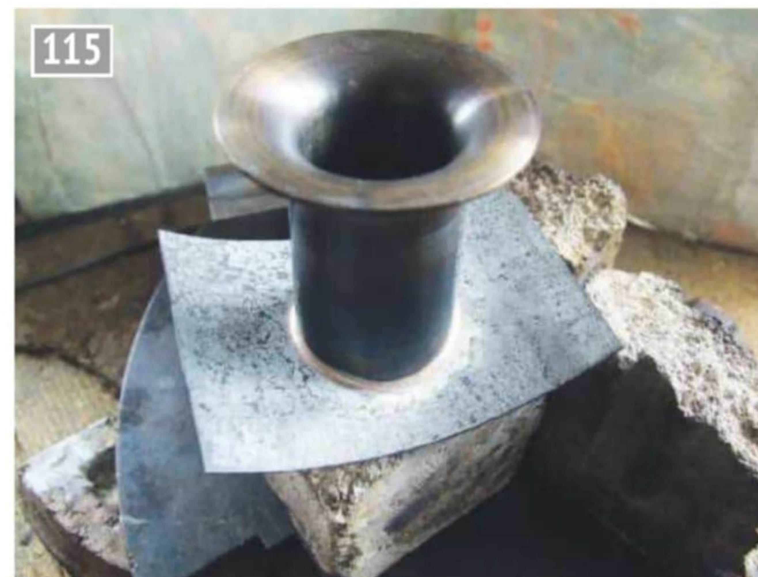
114 Here is the set up for the silver soldering of the petticoat pipe to its mounting plate and the tidy ring of solder at the expense of a very black pipe.
