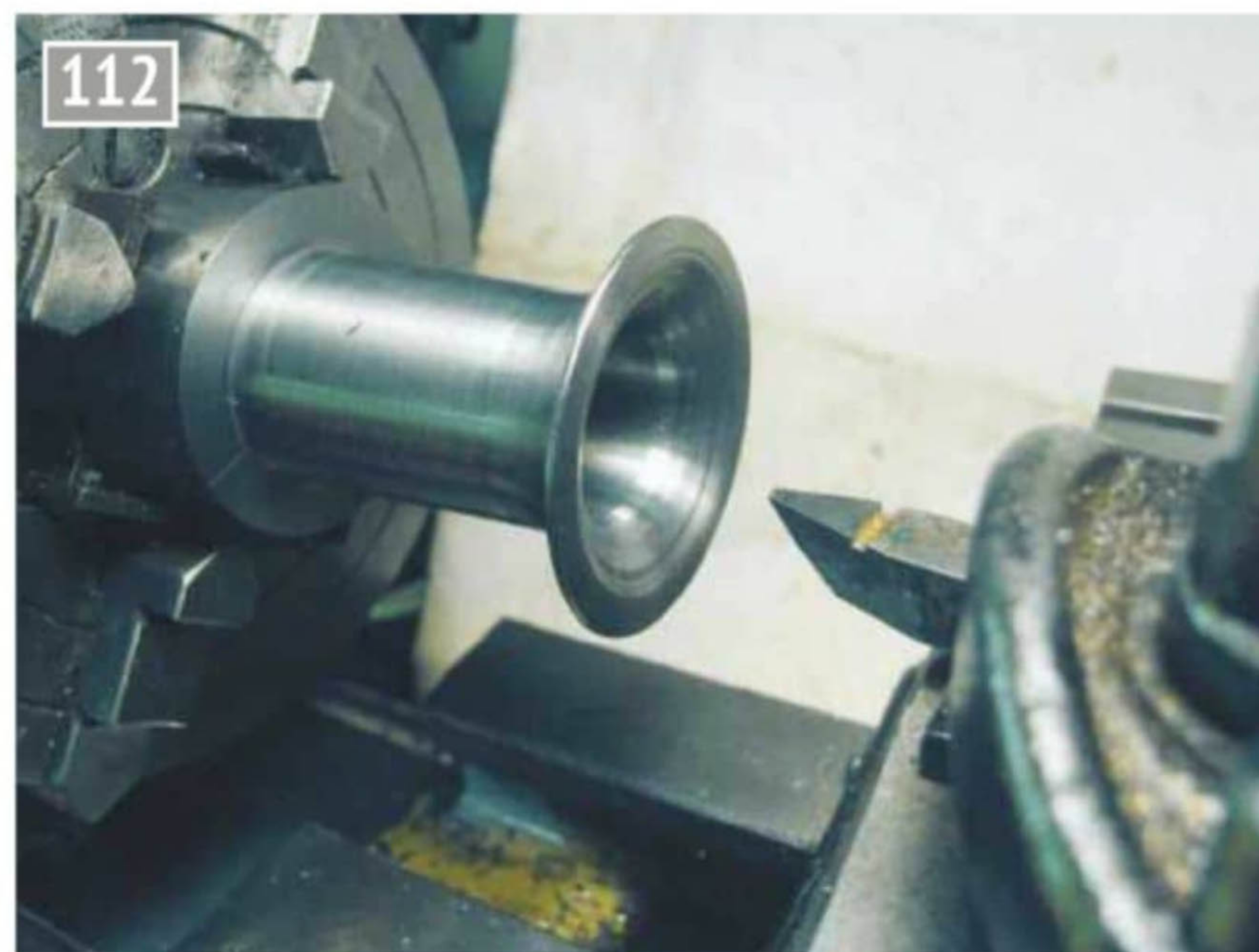
112 Taking off the bulk of the material from the inside radius of the flare before using the form tool and finishing the curved edge.
