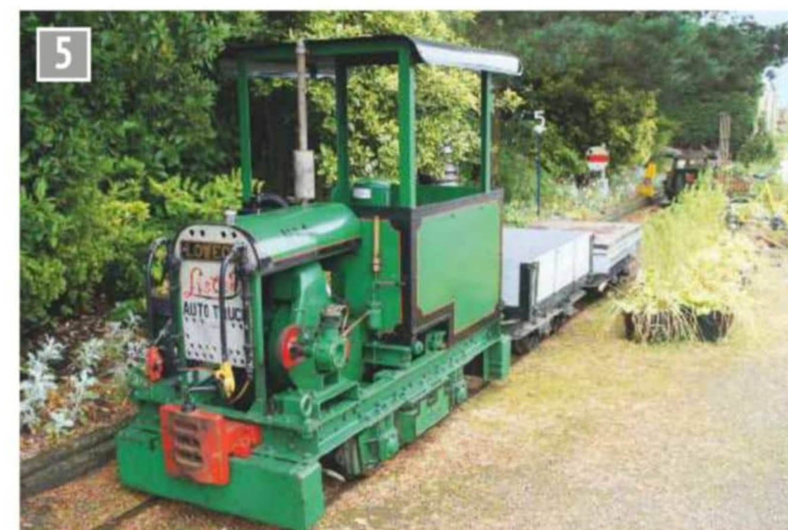
Bob Brooks' Loweco diesel has a Lister engine. It came from the now closed Abbey Light Railway in Leeds.
