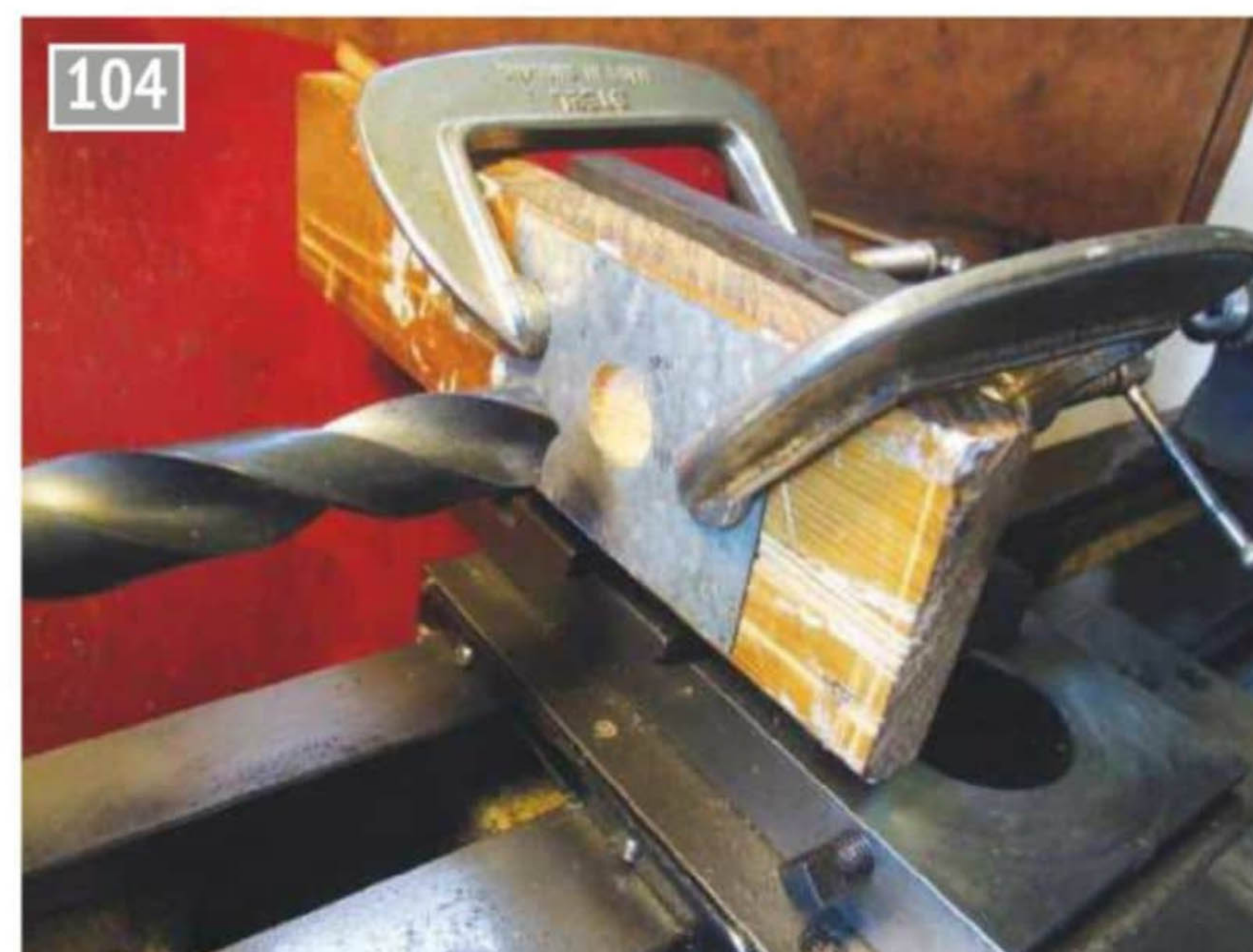
The set up used to produce the large hole for the petticoat pipe plate showing the drilling and boring operations.
