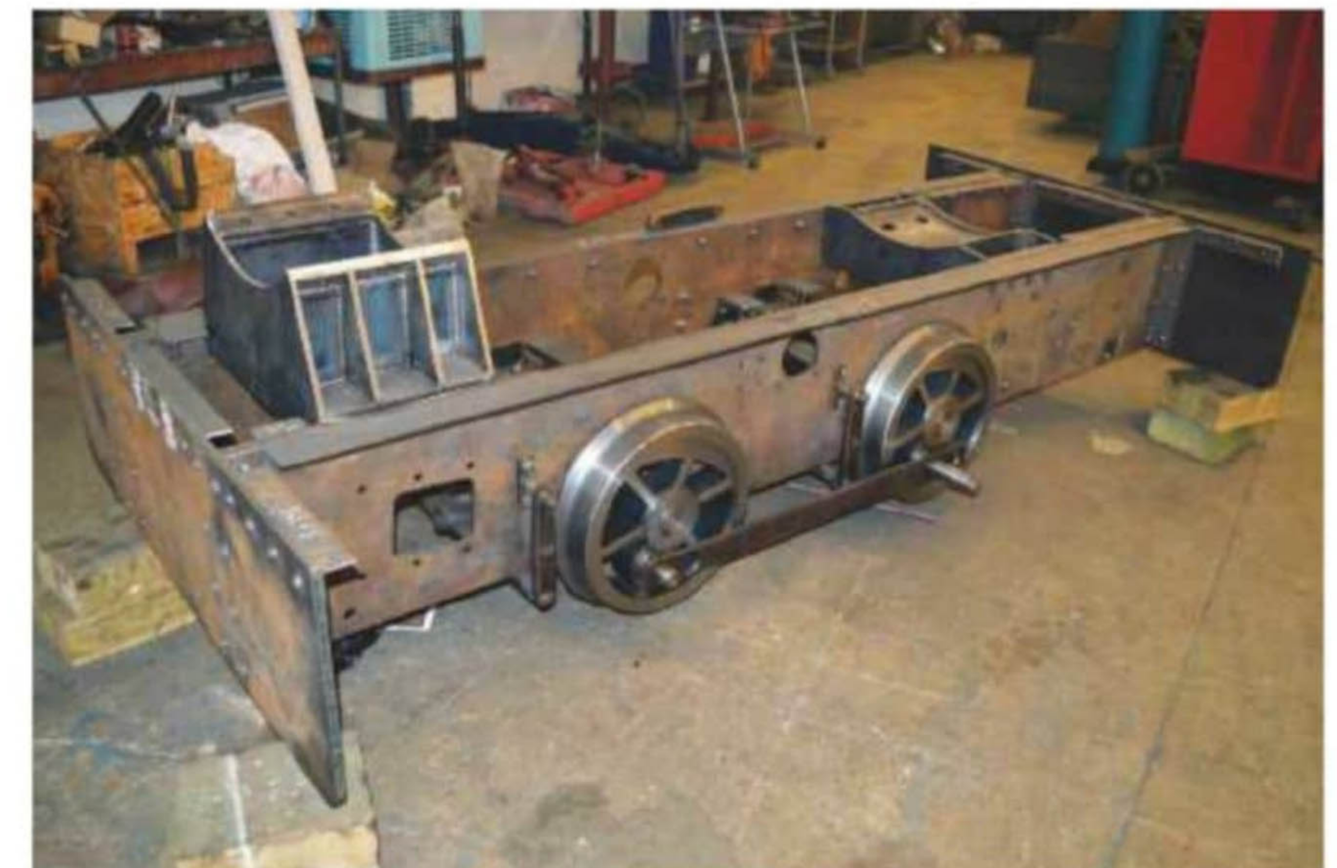
This is a front left hand three-quarter view of the chassis of Otter in the Erecting Shop on the outskirts of Scarborough in January 2017. By this time, the chassis was at the 'rolling' stage with both of the left hand brake hangers and associated transverse rods already fitted.
