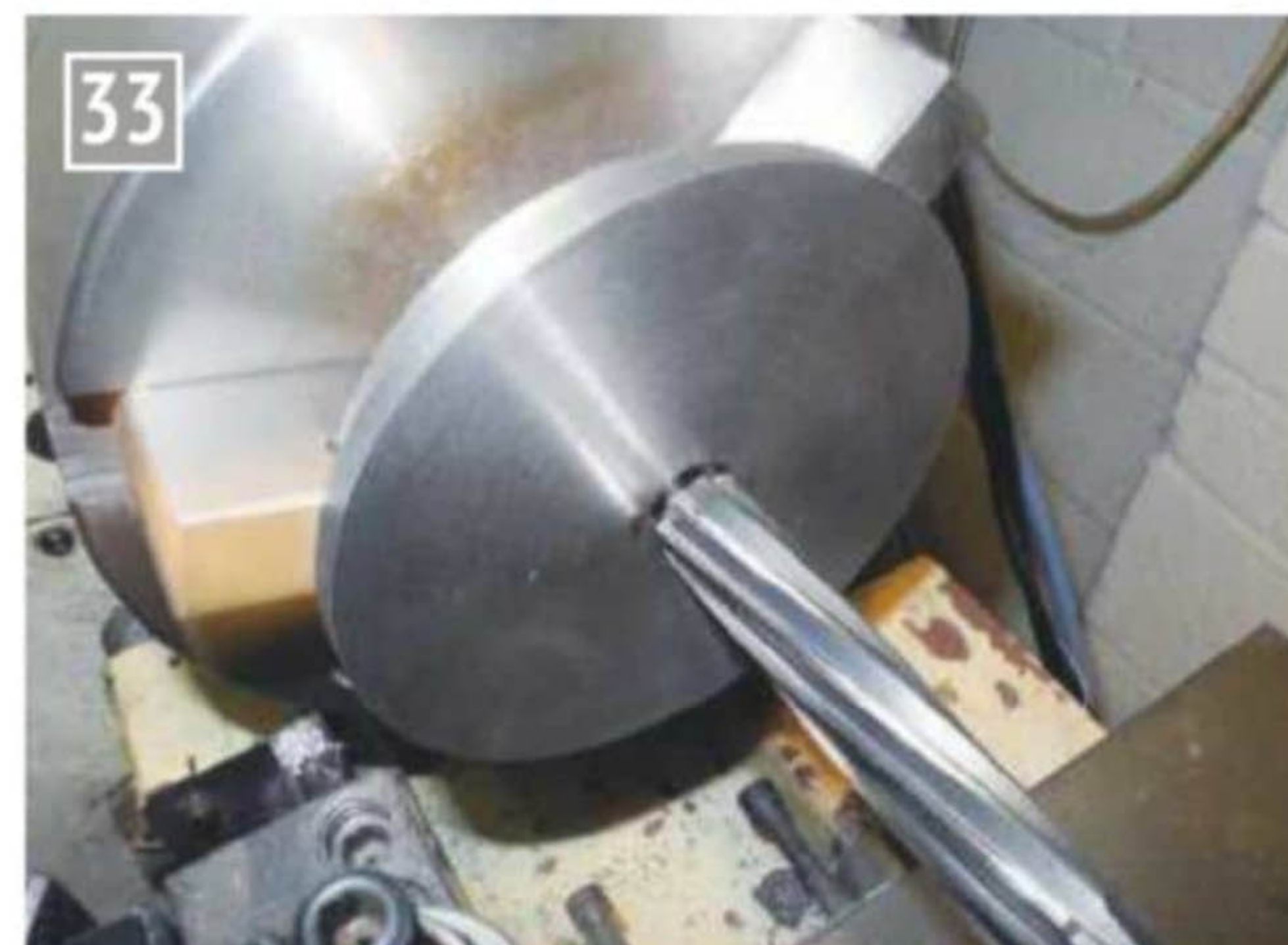
Reaming a wheel for its axle.
