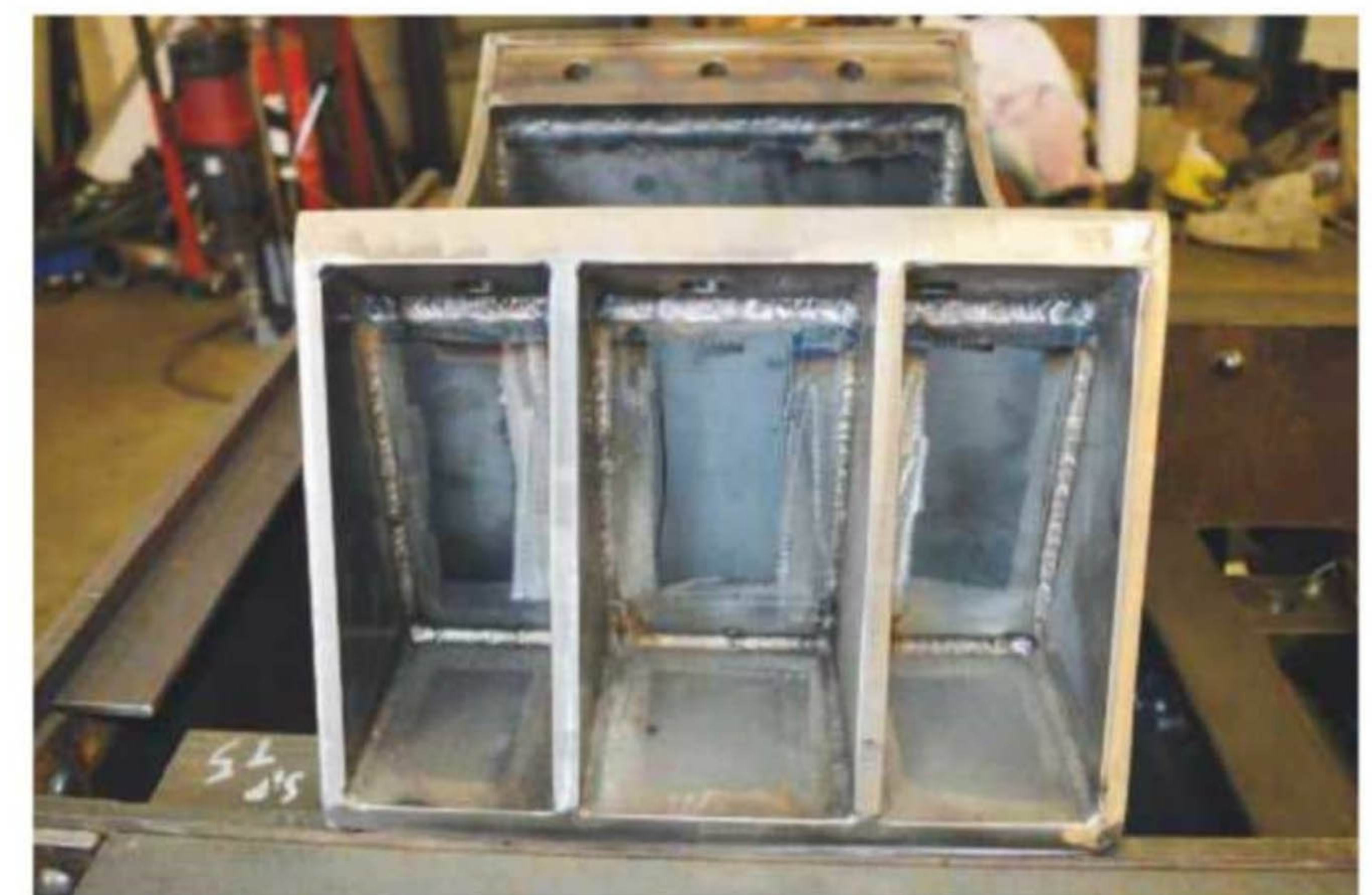
The ribbed smokebox saddle referred to in the text in relation to the Sipat design has been faithfully reproduced on Otter but, in line with the general constructional principles of the new locomotive, it is of fabricated rather than cast construction. For a good illustration of the movement from plain to ribbed smokebox saddles on these small Bagnall locomotives at the turn of the 19th/20th Century, compare the Groudle Glen Railway 2-4-0T Sea Lion and Polar Bear designs.
