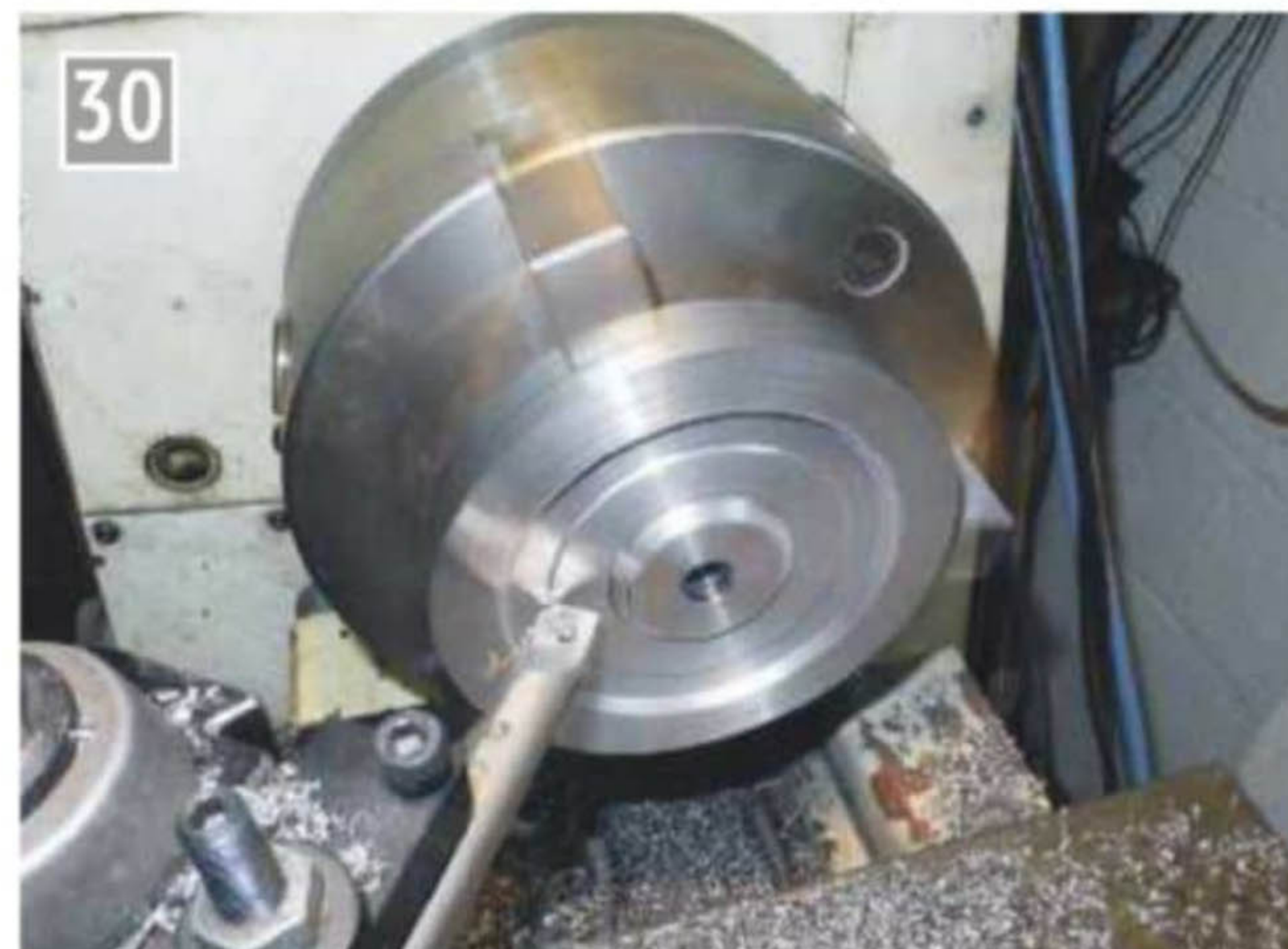
Boring tool angled to recess the front of the wheels.
