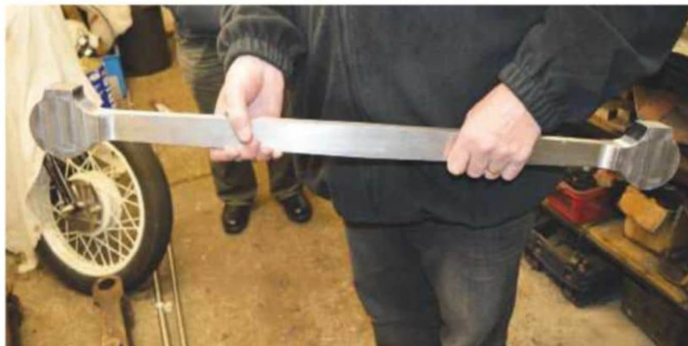
This is one of the blanks for Otter's coupling rods as seen in the Machine Shop in January 2017.
