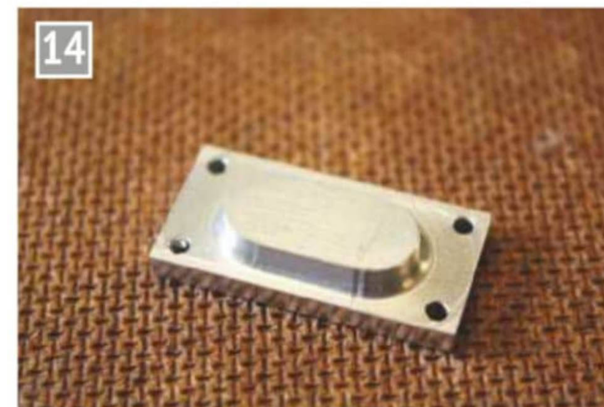
Cover with outside contour milled.
