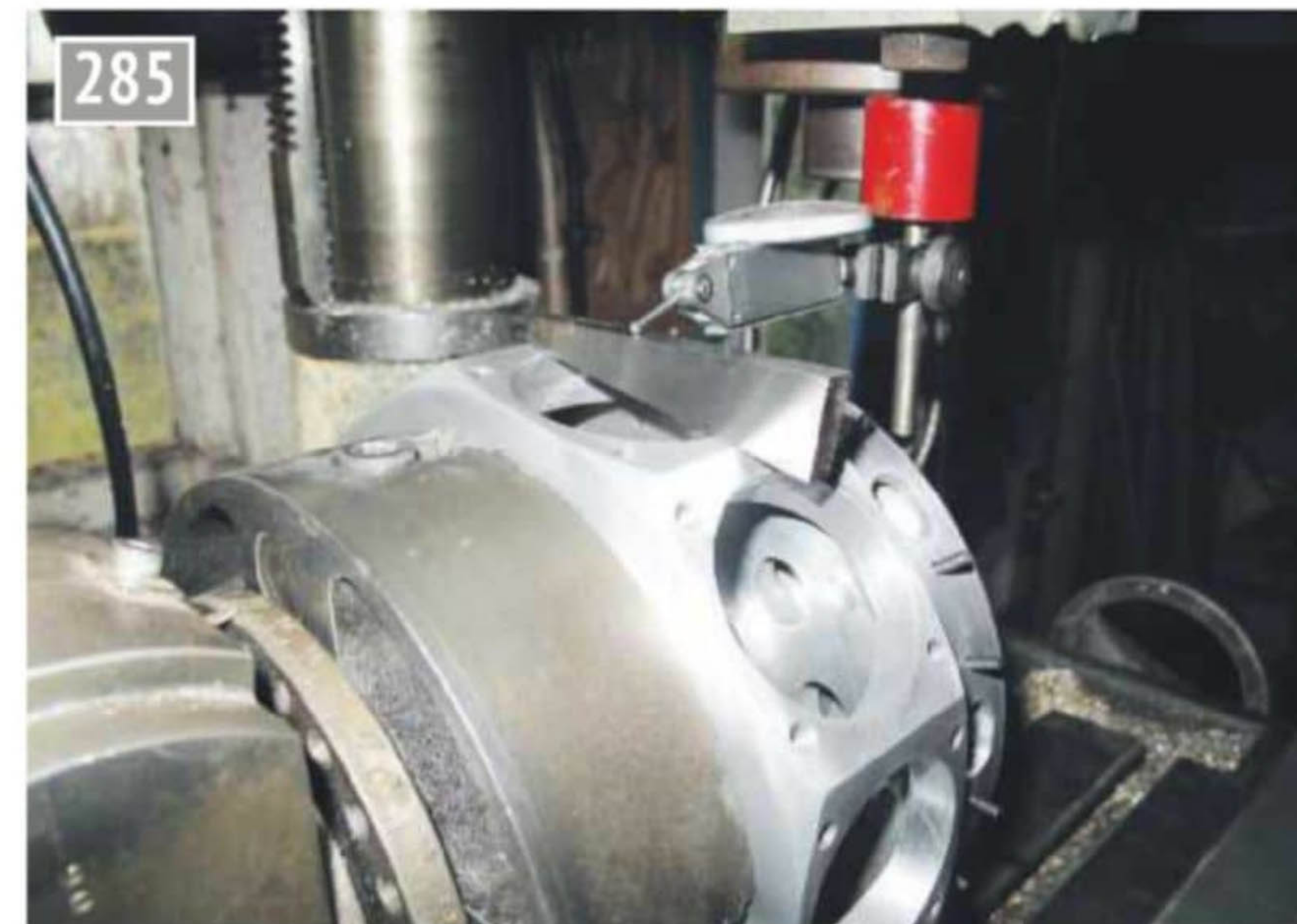
Setting No. 1 cylinder at 10 degrees before TDC.
