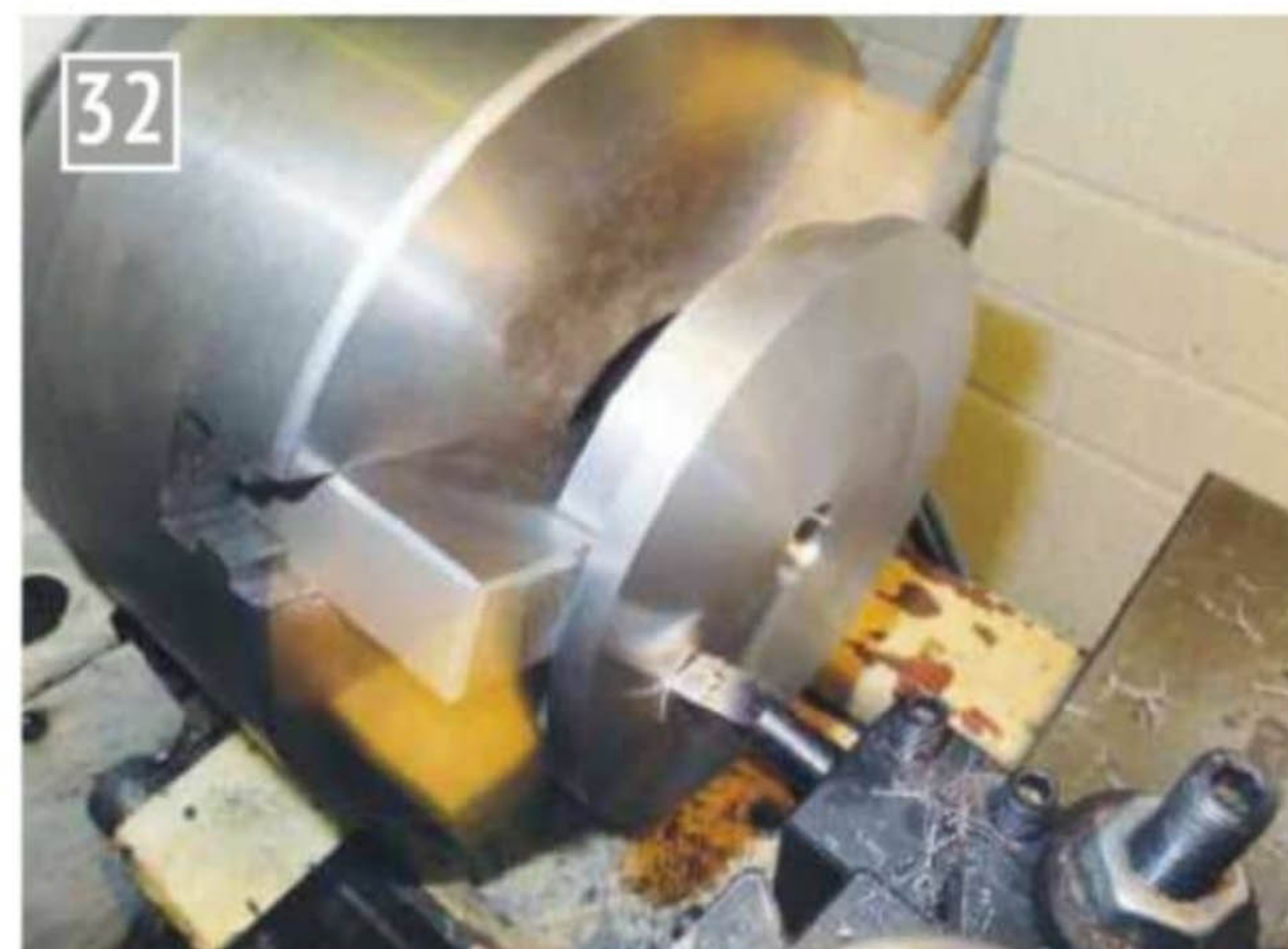
Facing the back of the wheel.
