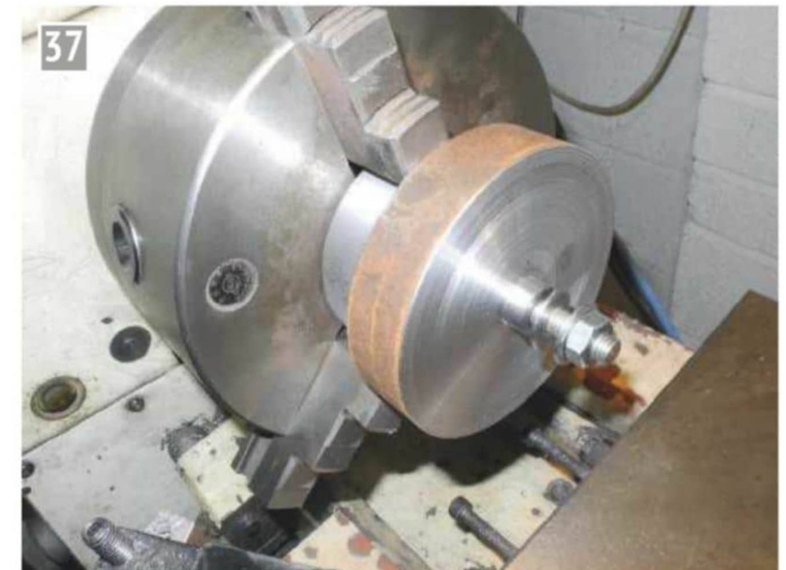
Wheel turning jig.
