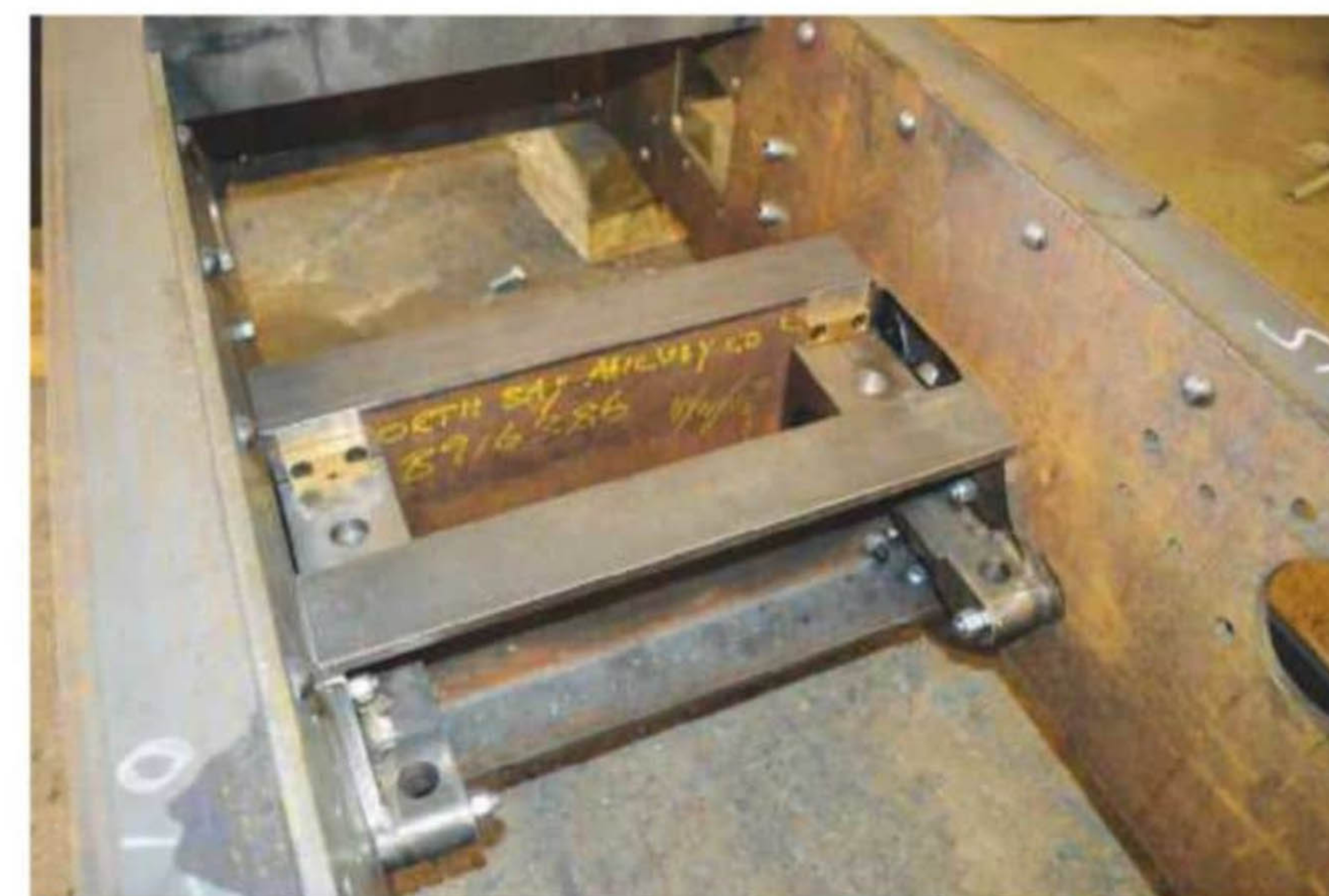
This is Otter's leading axle stretcher which effectively envelops the axle. On the original Sipat design this would have been a casting, but on the new locomotive it is a welded fabrication.
