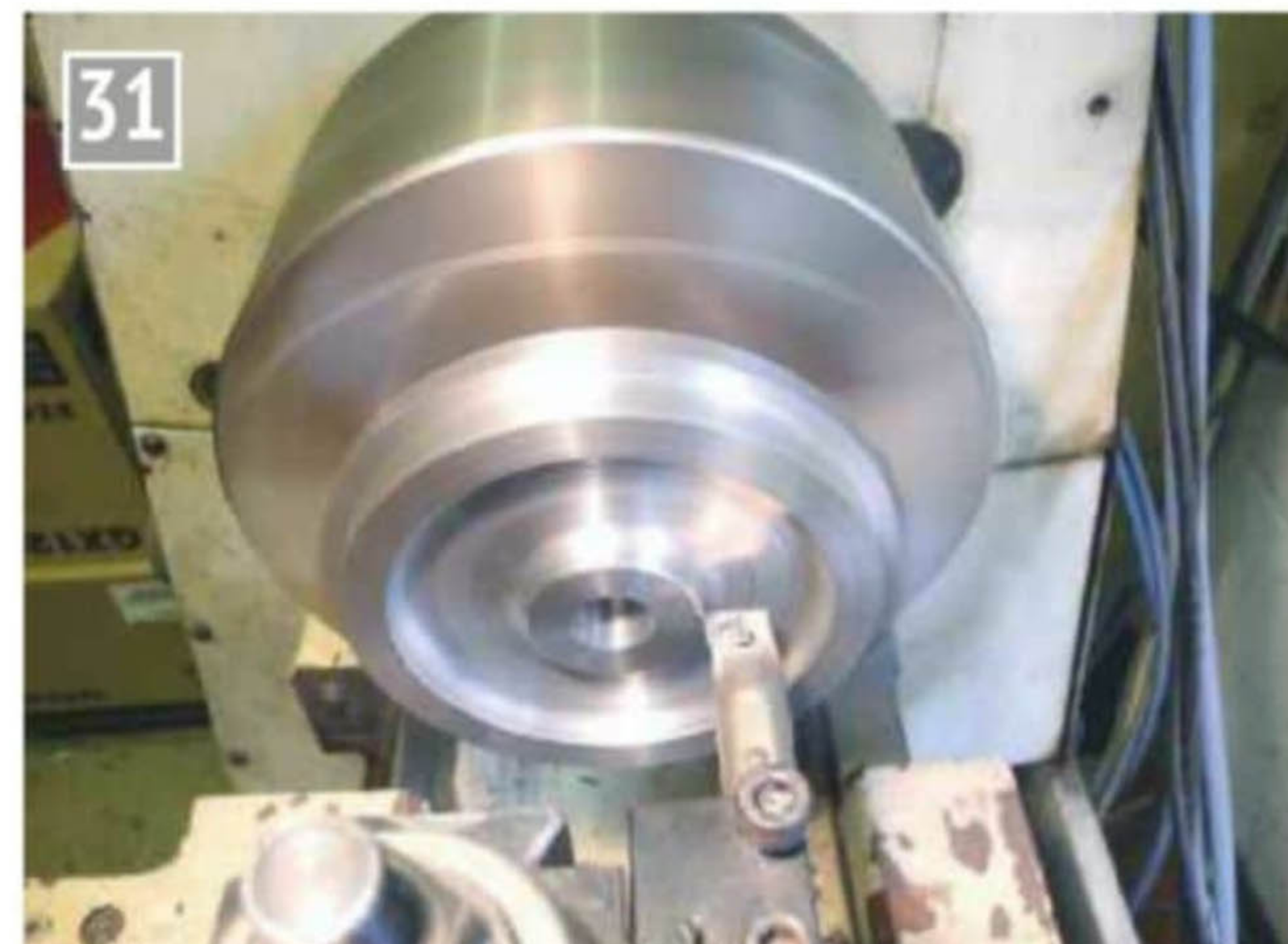
Profiling the hub by using the tool 'wrong side'.
