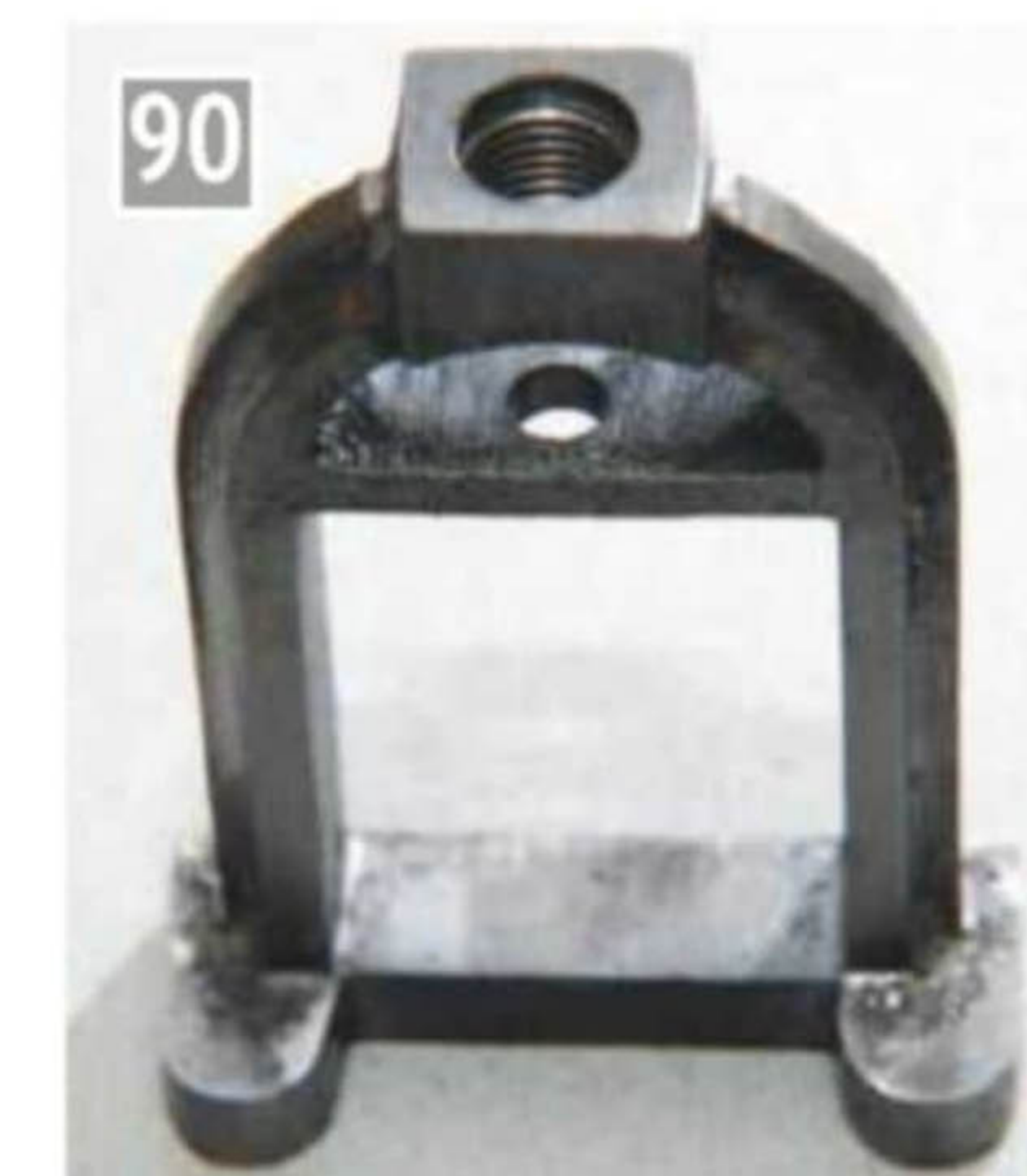
Governor stand with cast-in bridging piece.
