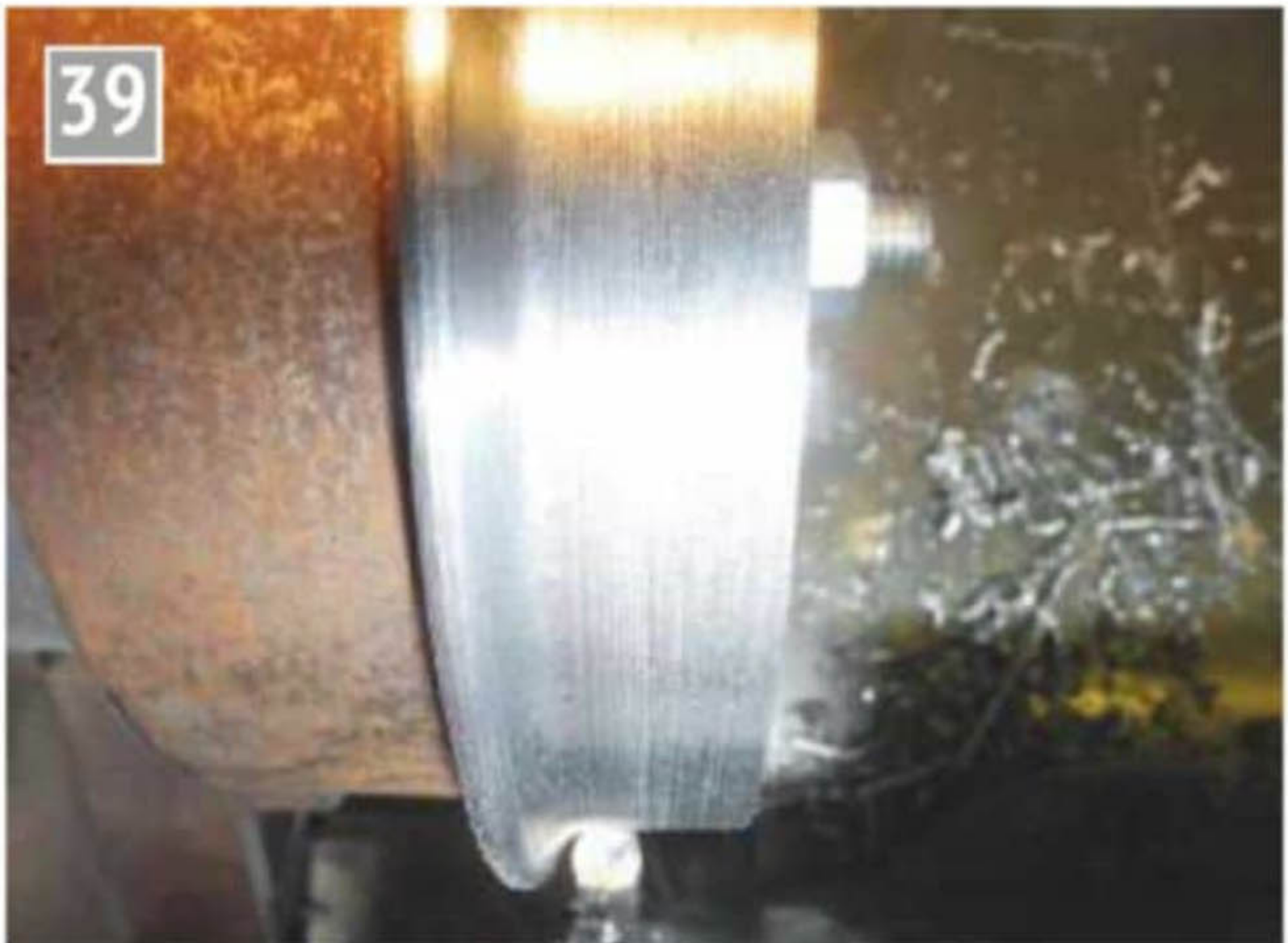
Finishing the wheel profile.
