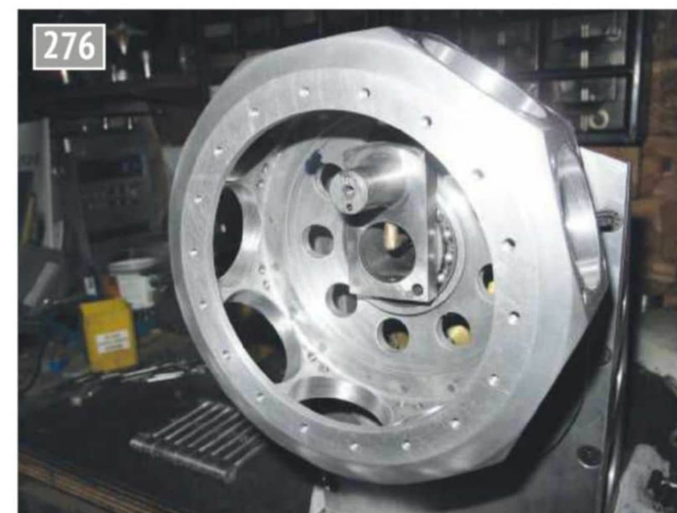
Crankcase secured in the running frame.
