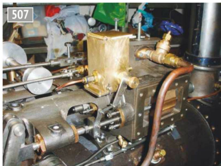
The lubricator mounted on the engine.
