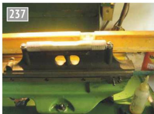
237 Spirit levels to set the bed horizontal - note removed leadscrew.
