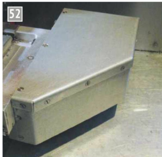
52 The X motor cover. Angled to clear the door shown earlier.
