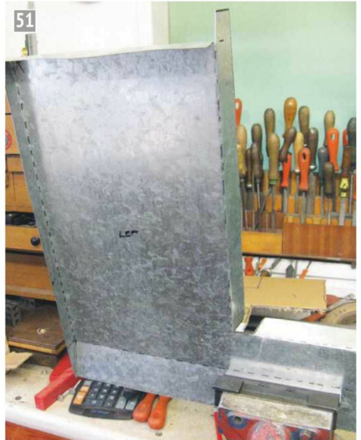
51 Forming the right-hand half of the upper drip tray, which drains into the oven tray shown earlier.
