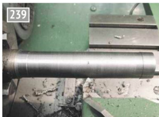
Turning the bobbins for the levelling of the lathe bed.
