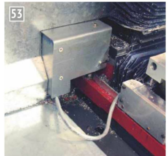
53 The Y motor cover built into the left-hand splash back, which is fixed to the back of the column.
