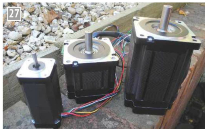
Three different sizes of brushless motor.
