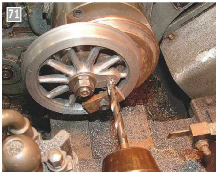
71 Drilling the crank pin.
