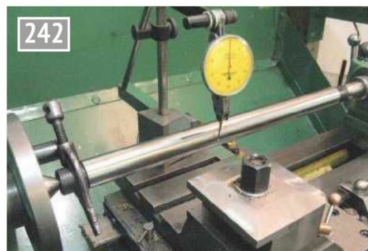
Checking the alignment with an accurate test bar, also showing the use of a catch plate and carrier to turn the bobbins on your test bar. The clearance between the bobbins is needed so a very fine cut at the same setting can be made on the ends. Once made, and with the ends at an identical diameter, it can be used in the same way as my ground version.
