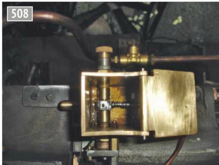
Top view of the lubricator with the pump piston uncompressed.
