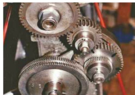
Eric Clarke cuts metric screws on a very Imperial Drummond Lathe
