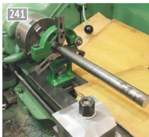
Setting up a three point steady to enable centre drilling the tailstock set-over.
