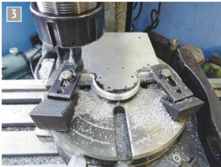
'D' shaped end machined and profiled on rotary table.
