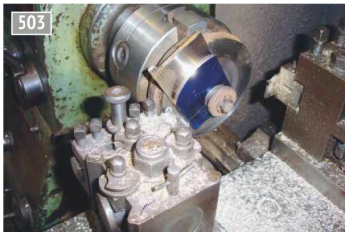
Turning the lubricator side plate.
