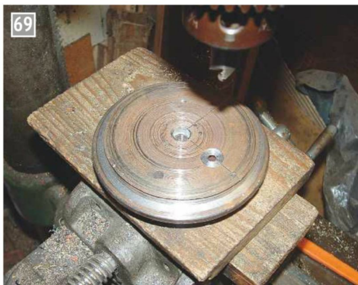
69 Drilling the offset spigot for locating the crank pins.
