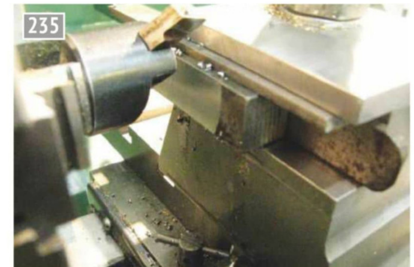
Fly cutting the \frac{5}{8} inch jig square end blocks true.
