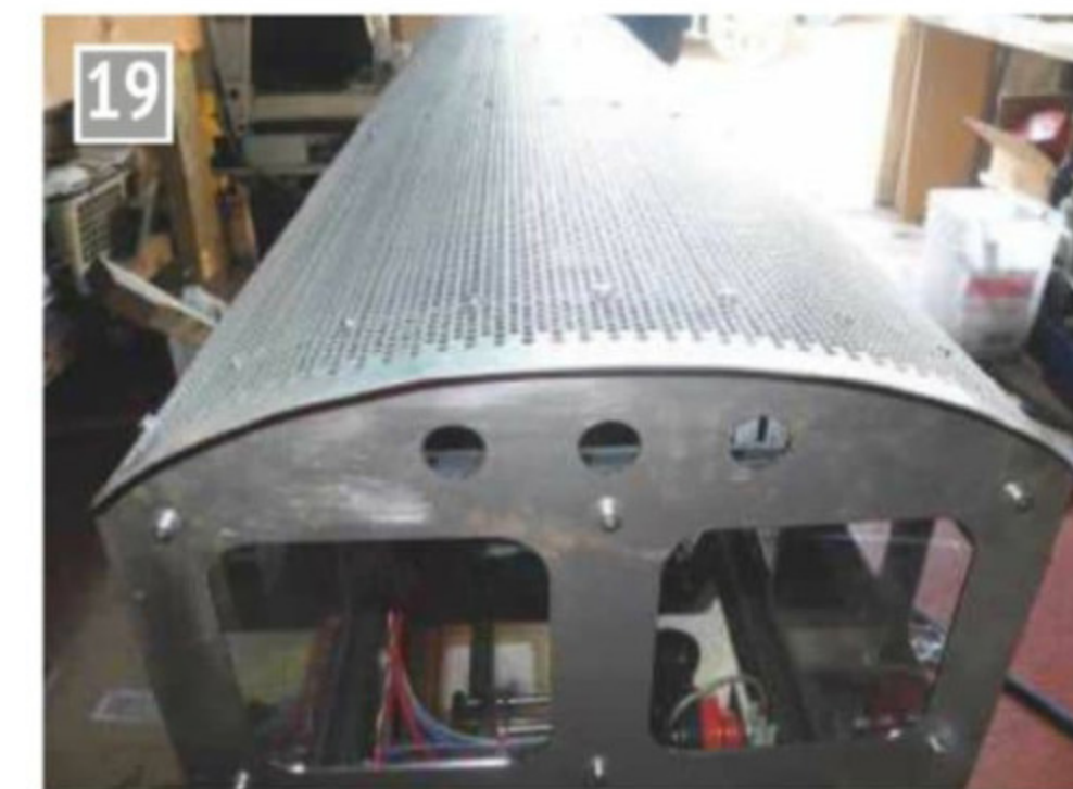
The roof is screwed to the 'coat hanger' supports.
