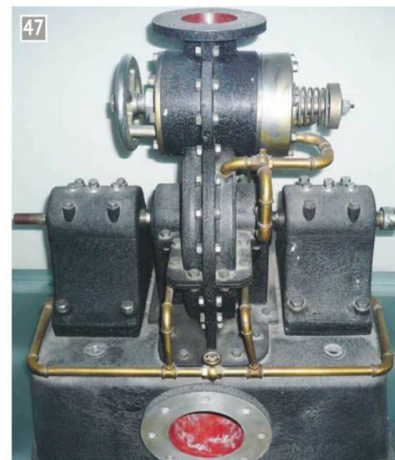
Turbine built by Nikolai Tesla. In the Tesla Museum, Belgrade.
