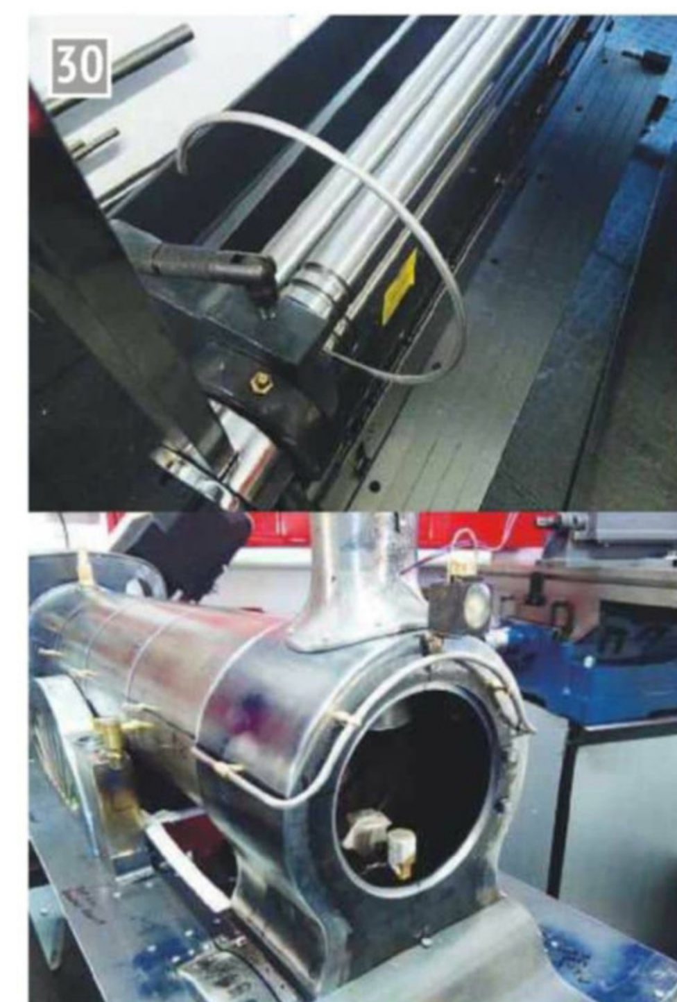
Large stainless steel bend for the blower line in front of the smokebox.
