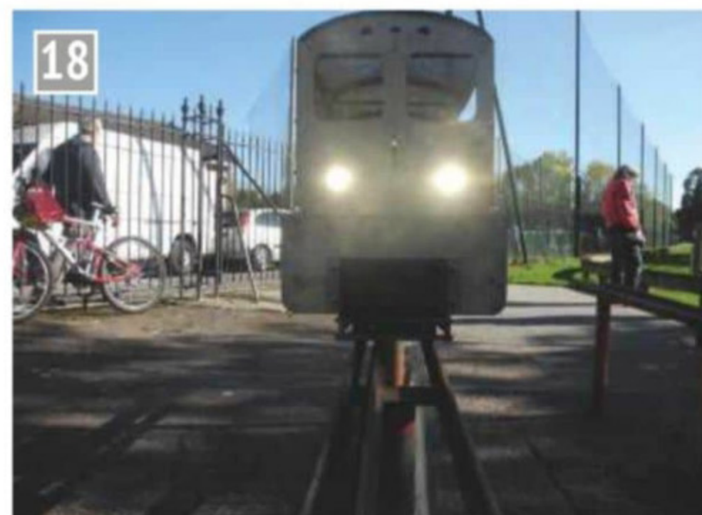
Front view – through the windows can be seen the 'coat hanger' supports for the roof.
