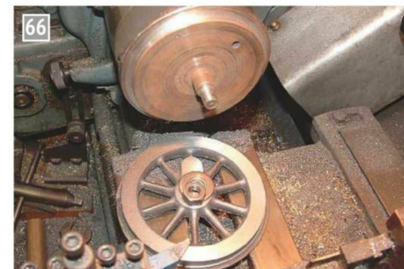
Special faceplate, with slightly raised edge for gripping the flange.
