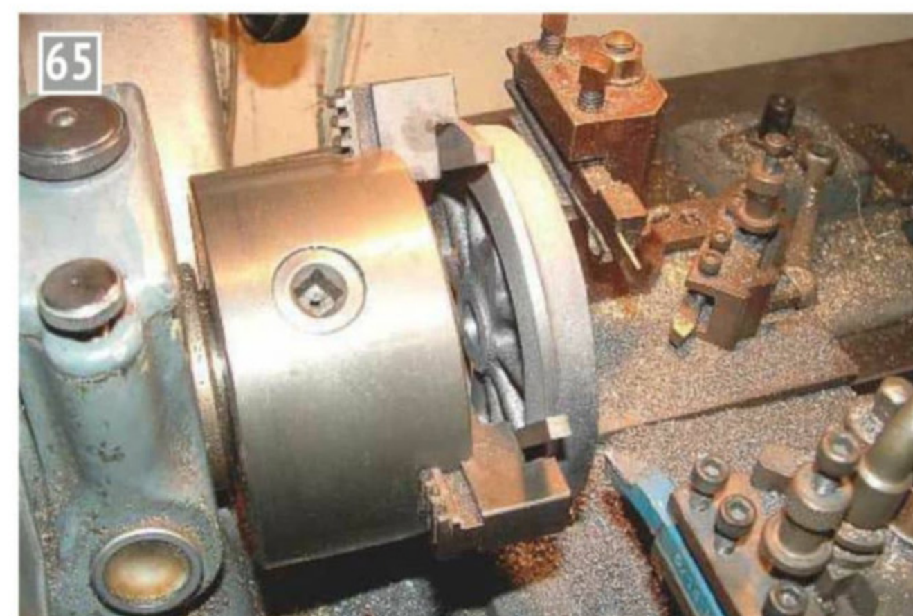
Spacers, allowing the entire tread to be machined.
