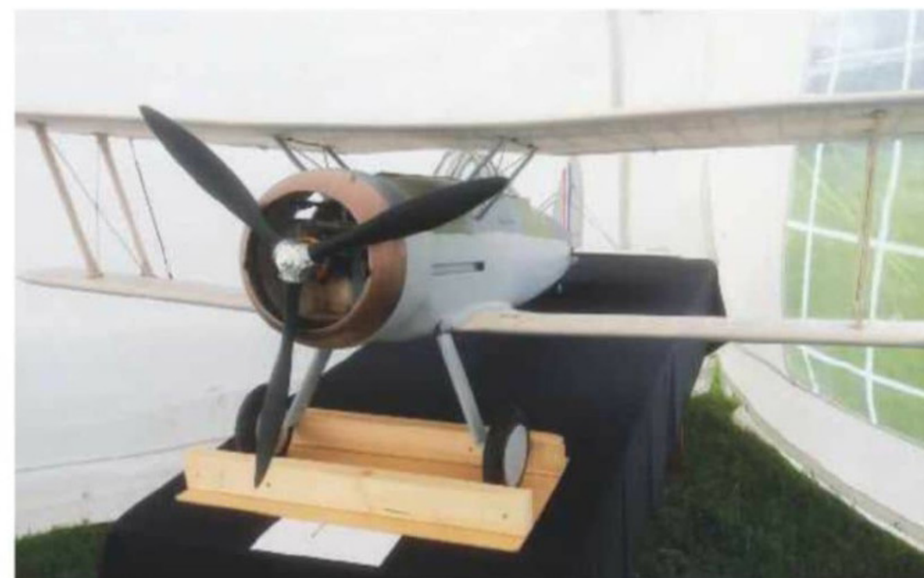
One fifth scale Gloster Sea Gladiator by Trevor Main. This is propelled by a 3kW electric motor and two Li-Po batteries each 22 volts and 5800mAh.
