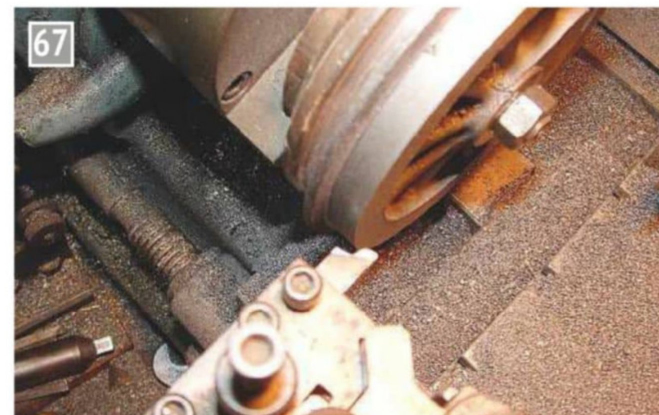
Using the special tool to form the tyre profile.
