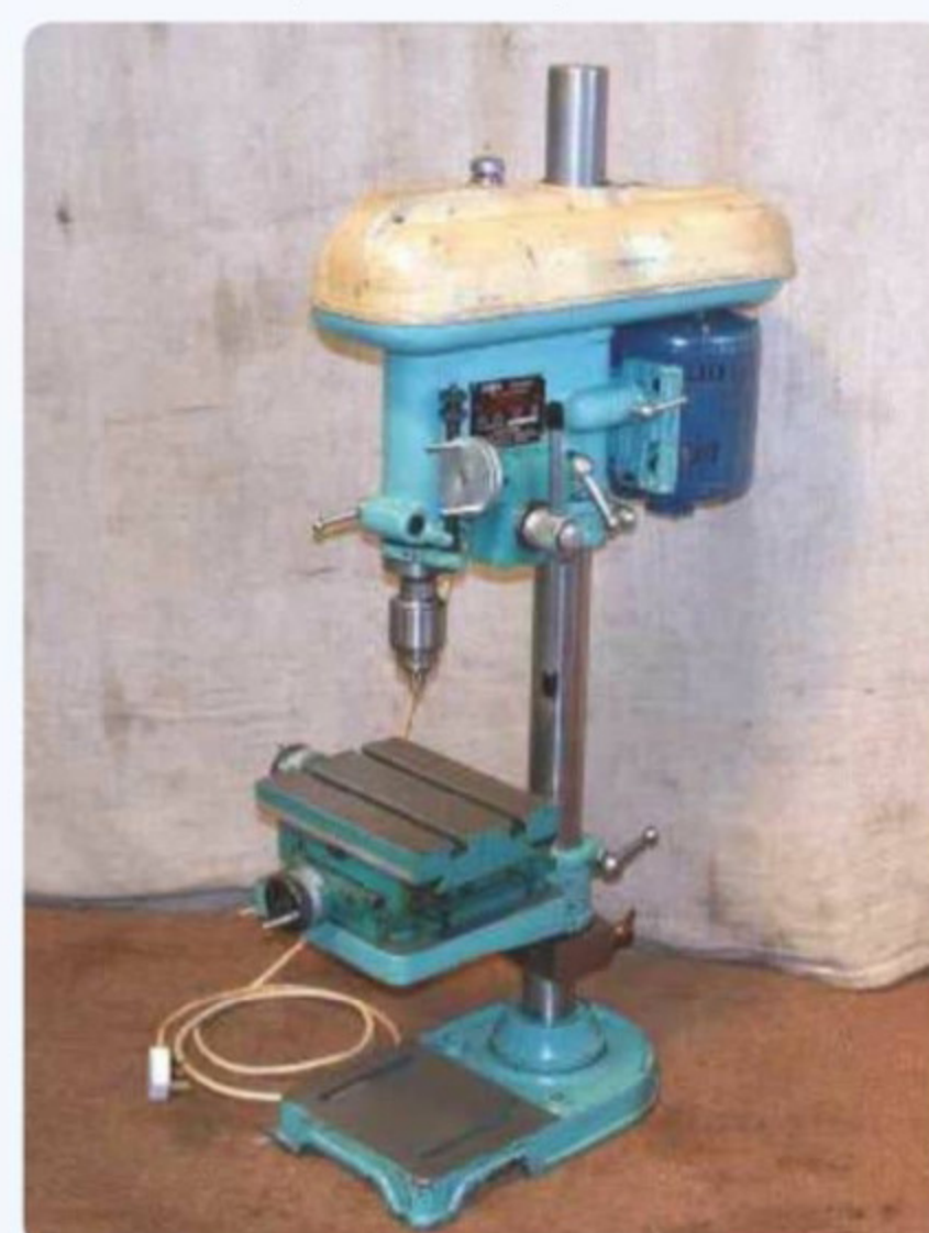
Fobco Universal bench Drilling Machine with Coordinate Table, Fine Feed Quill, Excellent Condition, 1ph, £1250.00 plus vat.
