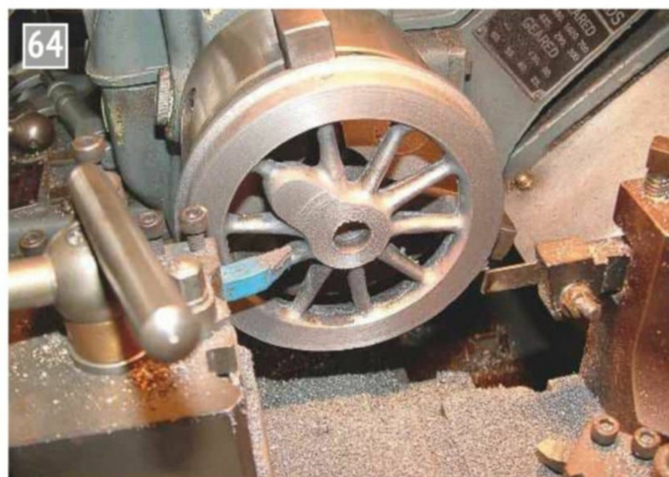
The wheel mounted for facing the front.
