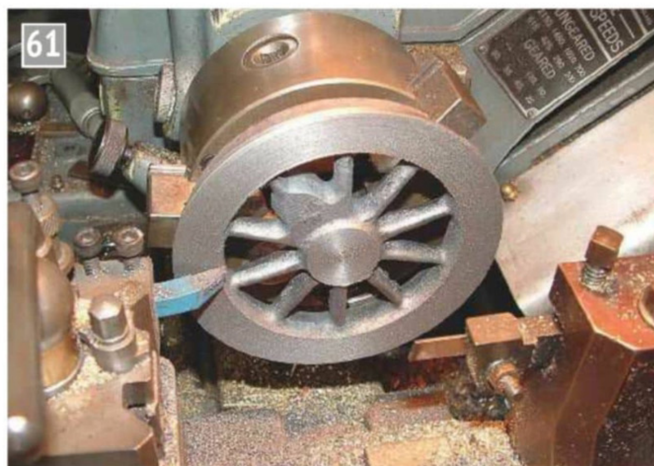
Facing off the back of the wheel.
