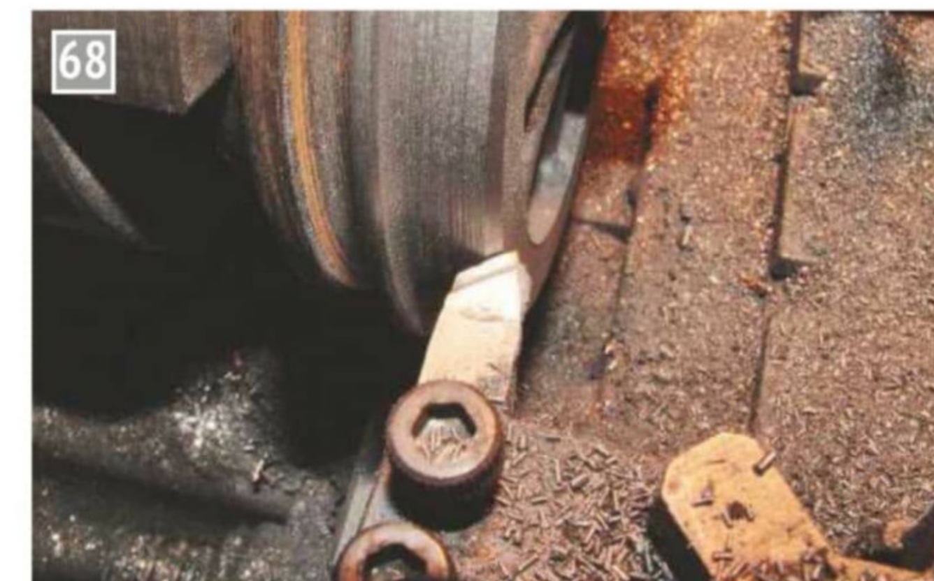
A special chamfering tool.
