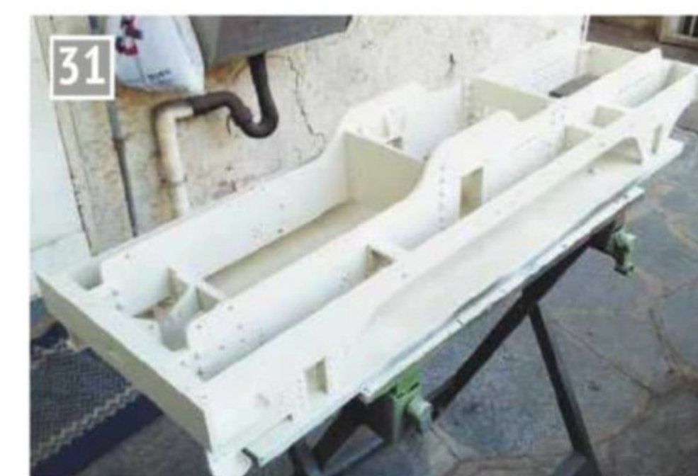
Main frames primed and ready for painting.
