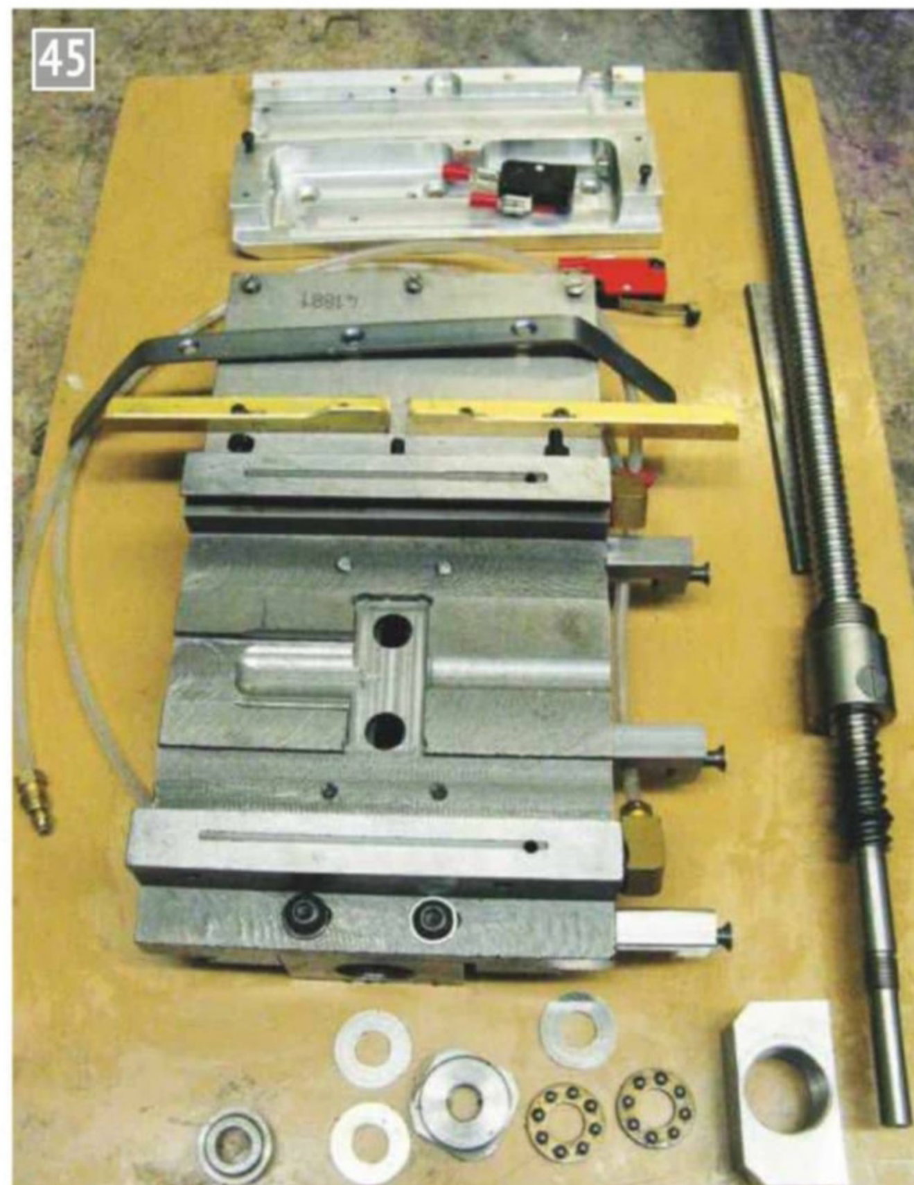
Saddle components, showing microswitch actuating blades.
