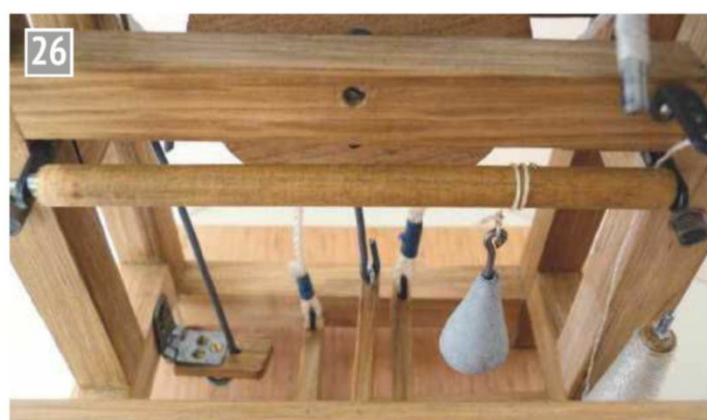
This shows the two fine adjustment screws for the sinker position.
