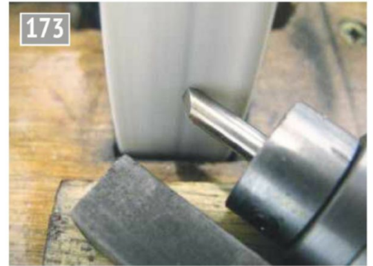
Rotate carrier 12 to 15 degrees (6 to remove the angle created by the curve of the wheel) invert the block and grind the trailing face.
