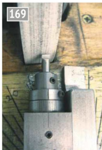
Grinding bore side clearance to 5 degrees in both directions.
