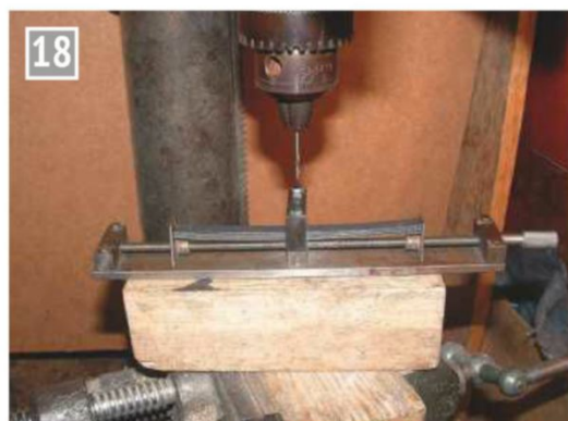
Jig for centring the hole in spring leaves.
