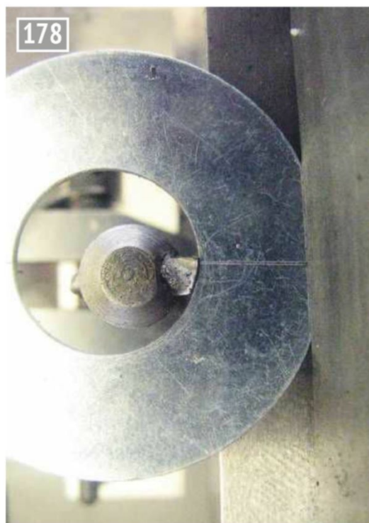
This 10mm short bar with bar locking does not have clearance.
