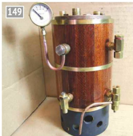
Pressure gauge 'U' tube fitted.
