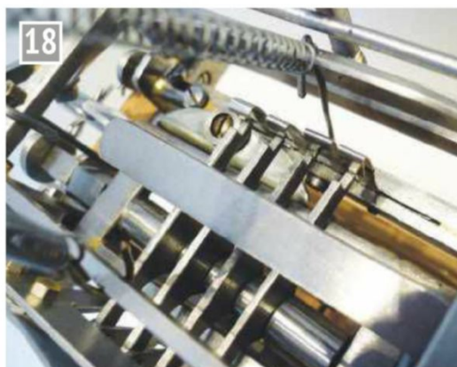
The slurcock roller is about to release the springs.
