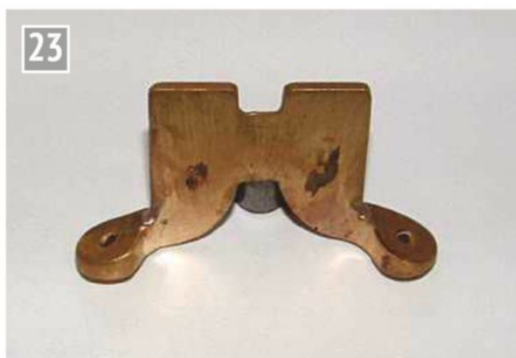
Two leaf spring hangers, back to back.
