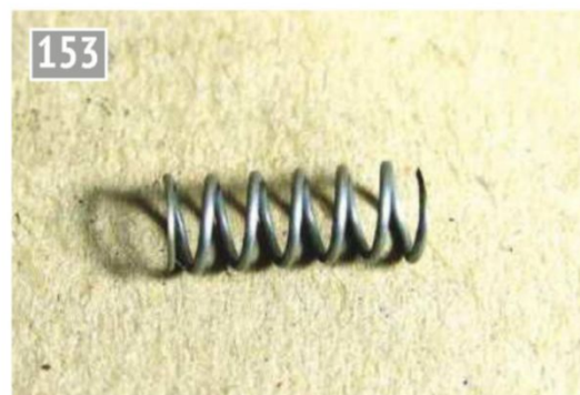
Ends ground on safety valve spring.
