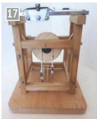
The slurcock and its operating pulley.
