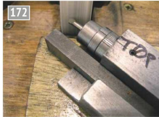
Angled bit for large bars. Set at 50 degrees to give clearance on front and side. See fig 37 (item 8). Note the extension to the highly angled slider fence.
