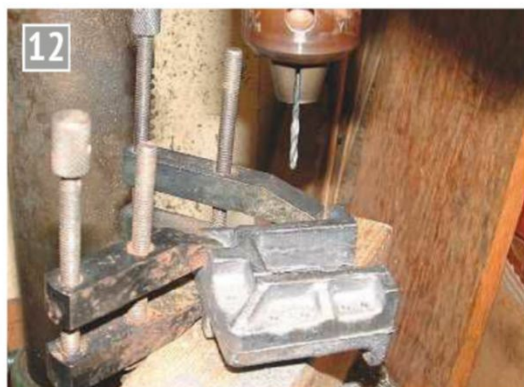
Spotting through the horn blocks back to back.
