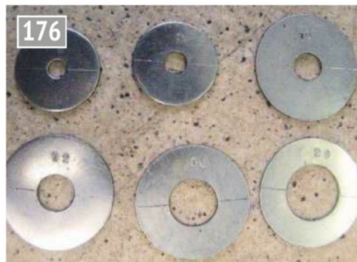
Washer set to check clearances of bits. Stamp the diameter and add a central line with the centre height scriber.
