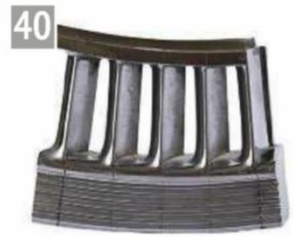
Blades from a high pressure stage of a large Parsons turbine. (Blade, courtesy of Fred Graham. Photograph by Izel Photography/ Duncan Andison.)
