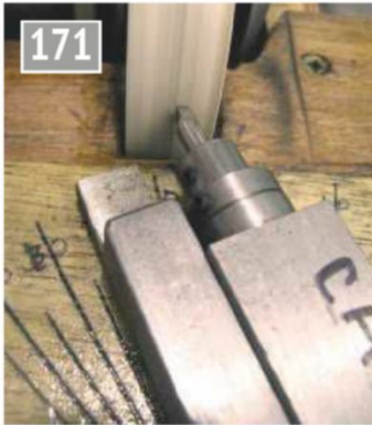
Grinding secondary clearance. Angle as required.
