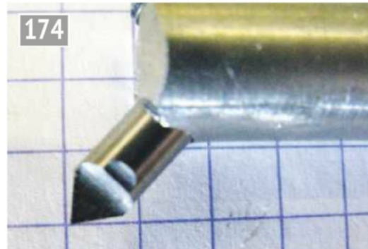
Finished angled cutter, making the clearance stand out on the background. Not rounded on the end yet. The cutter must be as close to the bar in order to use in a small diameter hole. Here it is extended for clarity.
