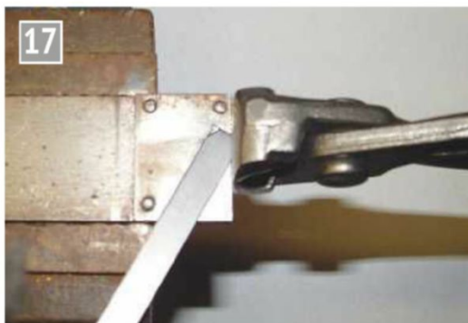
Jig for cropping the corners off spring leaves.
