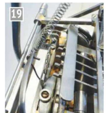
The locker bar is about to force the jacks back under the springs.
