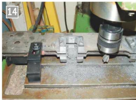
Accurately spacing the horn block openings on the mill.
