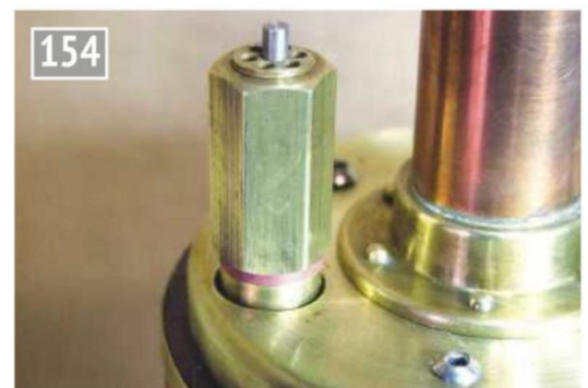
Safety valve assembled.
