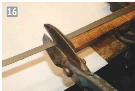
Cutting spring leaves accurately to length.
