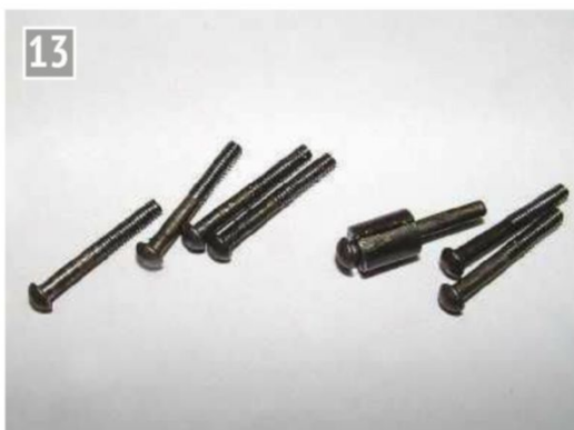
Threaded horn block bolts.
