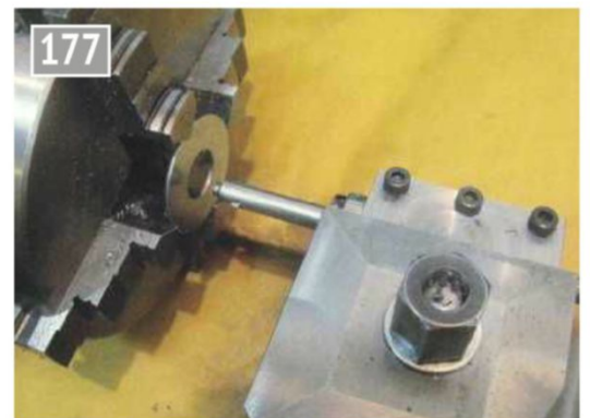
Boring the washer with an 8mm bar.
