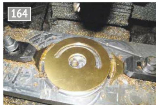
Roughing out the gear blank.
