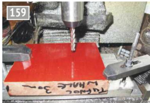
Tufnol billet set on the CNC mill.
