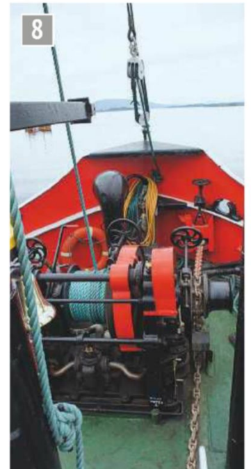
A steam winch hauls up the anchor chain and operates the derrick.
