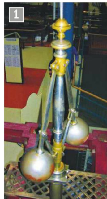
Hardly the handiwork of chimps – yes folks, much of the work on this exquisite governor was created by blacksmiths. Note also the split pins and washers on the pivots...
