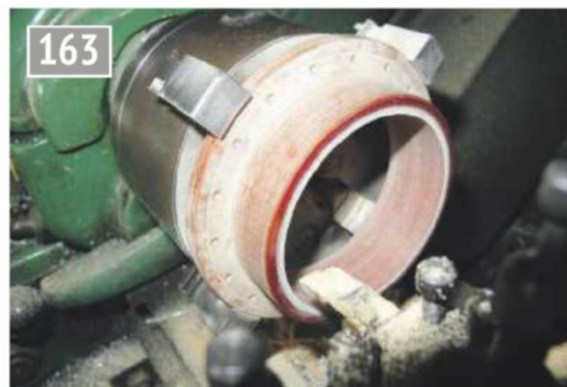
Turning the bore to achieve a close fit to the thrust box.
