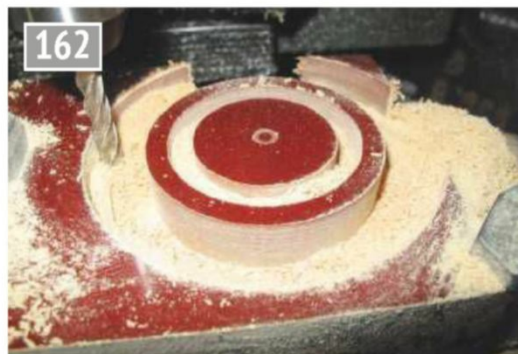
Removing the bulk of the material.
