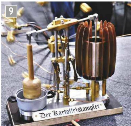
This little potato masher was powered by a hot air engine.
