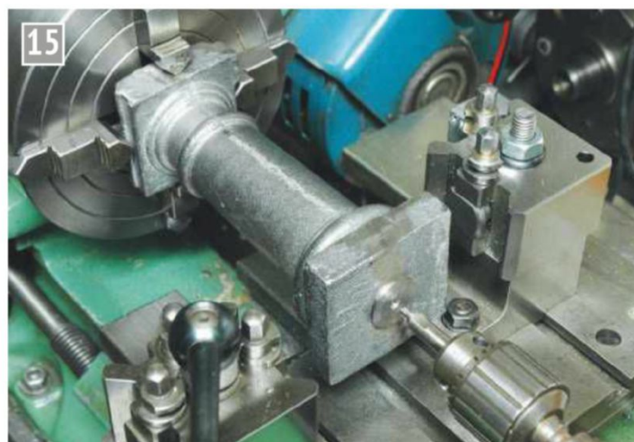
Centring the column.
