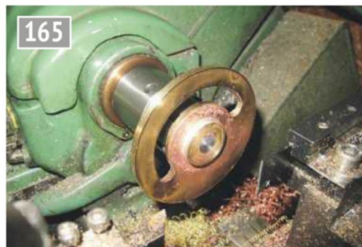
Finish turning the outside diameter.
