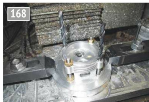
Cylinder head located on the machining fixture.
