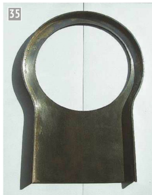
Views of the front plate assembled with the tabs of the flanging strip chamfered and the slots given some clearance so they could be fitted through the curved openings prior to giving each of them a gentle tap with the heel of a hammer to secure them for silver soldering. Cleaning up was quickly done with the bulk of the joint tab area being removed from the outside with the coarse wheel of an off-hand grinder and then the two sections of the joint were filed flush.
