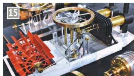
A Stirling engine-powered rear paddle system for a boat.
