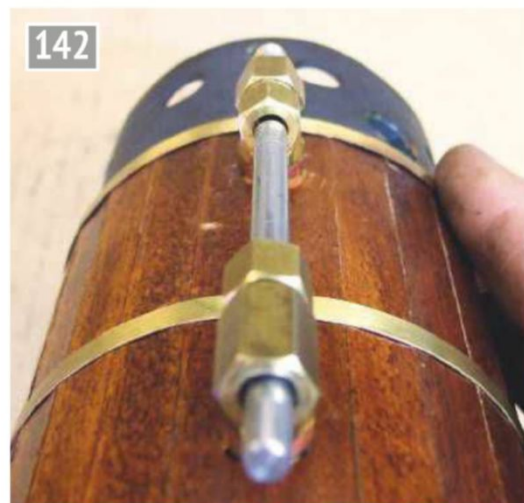
Lining up top fitting with bottom fitting.
