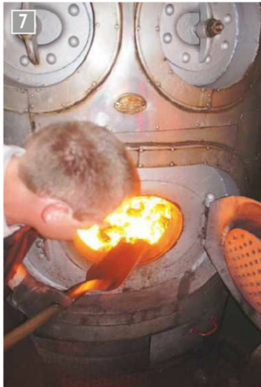
VIC32 burns Ayrshire coal, aiming to keep supplies as local as possible. Unfortunately it can be smoky. Welsh steam coal would burn too hot for the boiler.
