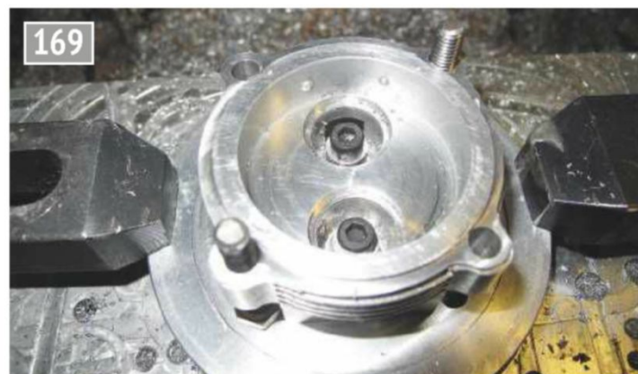
Secondary clamping through the valve stem holes.
