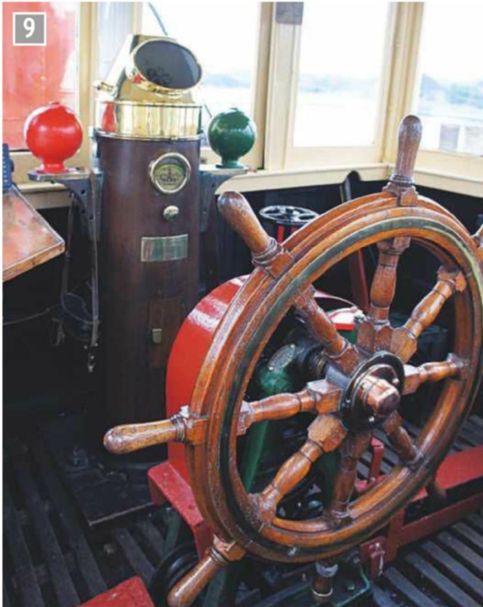
Ship's wheel and compass binnacle. Navigation is now assisted by a marine GPS system.
