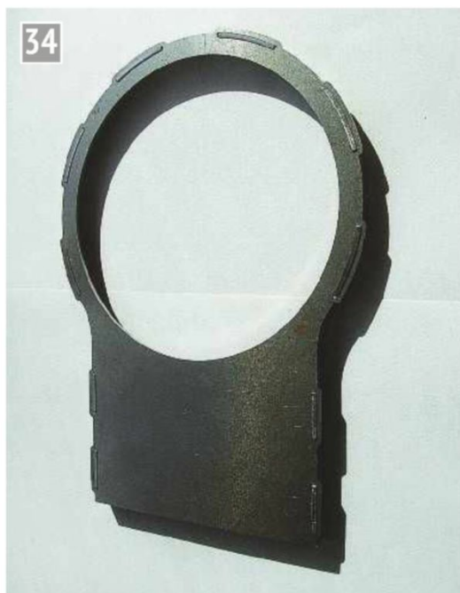
Views of the front plate assembled with the tabs of the flanging strip chamfered and the slots given some clearance so they could be fitted through the curved openings prior to giving each of them a gentle tap with the heel of a hammer to secure them for silver soldering. Cleaning up was quickly done with the bulk of the joint tab area being removed from the outside with the coarse wheel of an off-hand grinder and then the two sections of the joint were filed flush.
