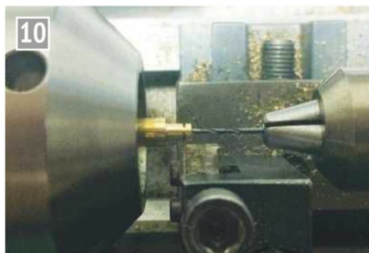
The parting tool rides again - parting off a governor wheel.
