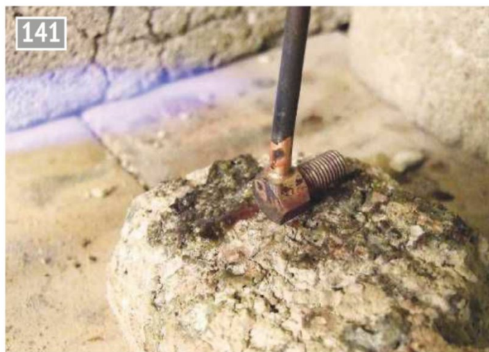
Silver soldering pipe to exhaust cap fitting.
