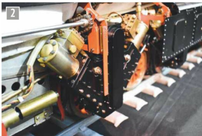
One of the twin Vee double acting cylinders attached to the rear wheel on the right-hand side of the Class 19 locomotive.
