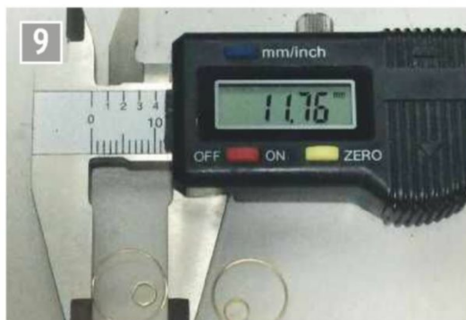
Here's the proof that such thin parts can be parted off with the right tool.
