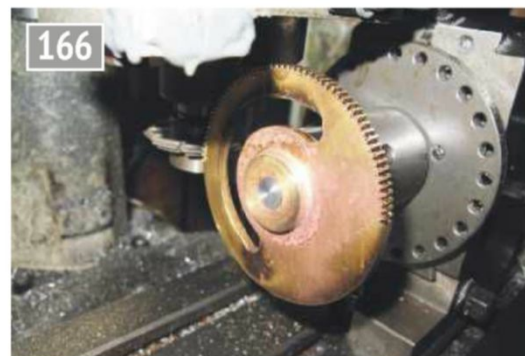
Starting the gear cutting.
