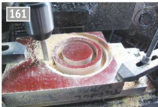
Generating the outside diameter.
