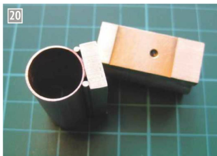
Cylinder soldering finished.
