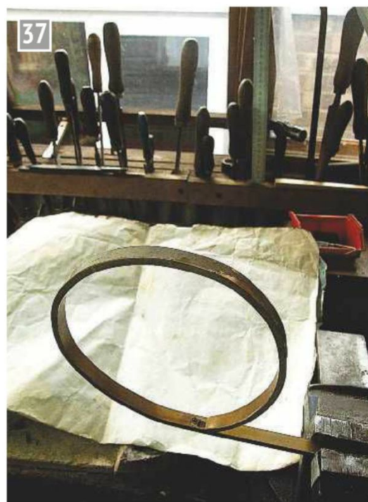
The first stage of forming the brass bar into a circle. It will be found that this heating operation will leave the material slightly soft and able to be locally formed with a vice jaw or a mallet. Afterwards, a joint is made with high temperature silver solder and the ring finally trued to be as near round as possible.
