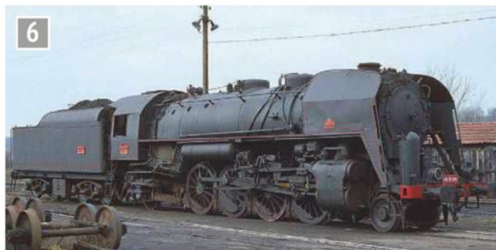
A nearly unbelievable success: the TIA water treatment was employed by the SNCF at its Nice locomotive depot in connection with a fleet of North American-built 141R locomotives, such as the one shown above. The treatment was so successful in reducing boiler maintenance costs that three locomotives, numbers 1156, 1158 and 1159, were able to operate a cumulative 5,500,000 miles with fewer than 900 man hours of maintenance attributable to the boiler with washout intervals - twice that permitted in the U.S. The image above is of 141 R 568 built by the Baldwin Locomotive Works in 1946. Photograph by Dider Duforest on November 11, 1981 (Wikimedia commons).
