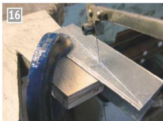
Cutting the rudder out.
