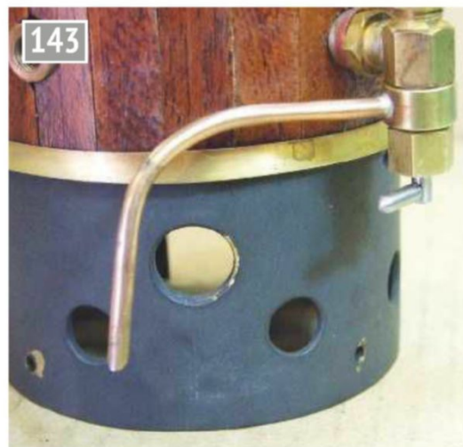
Blow down valve assembled and pipe secured.
