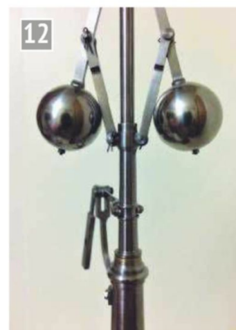
The proof of another pudding: the weeny wheels are juuust visible located in the governor lever's yoke, while the pivots carry the washers and pivots held by split pins.
