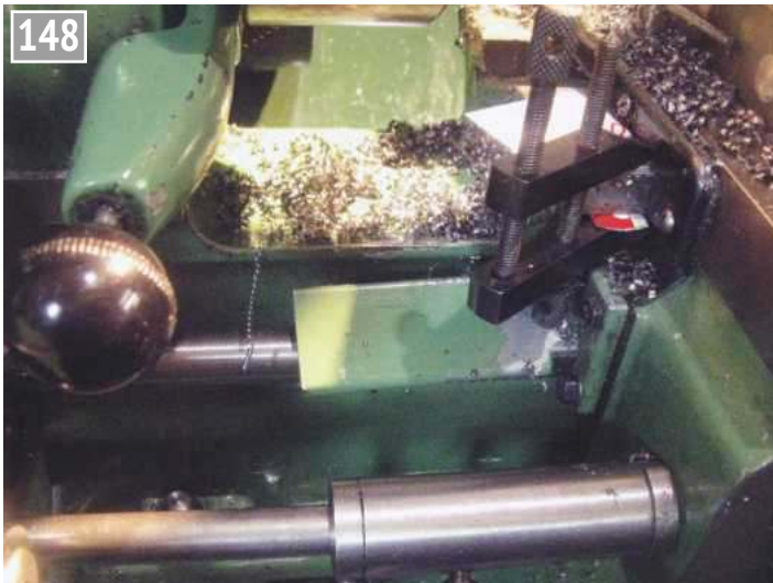
148 Setting a stop on the lathe bed to control the length of the boss.
