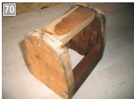
Former for making the firebox wrapper.
