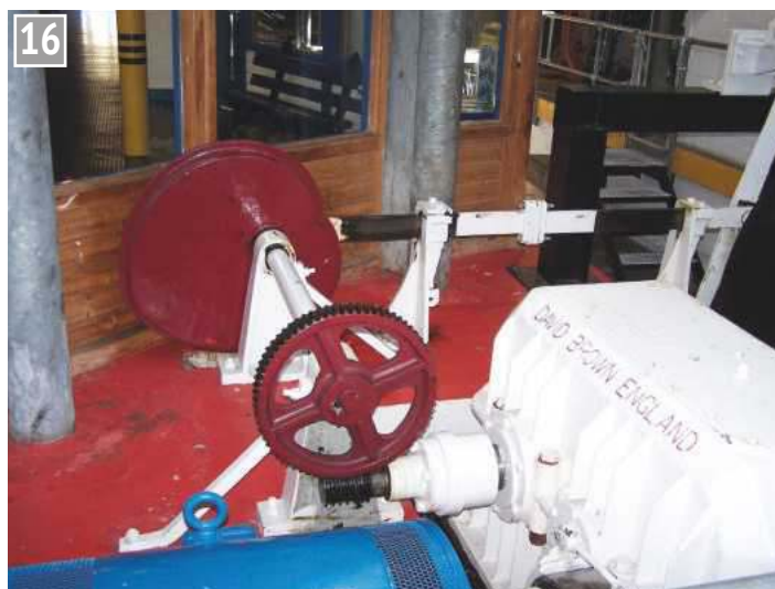
The cam which moves the guide rollers back and forth.
