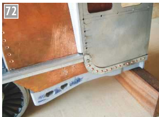
The intersection of cab sides, running boards and firebox outer wrapper.
