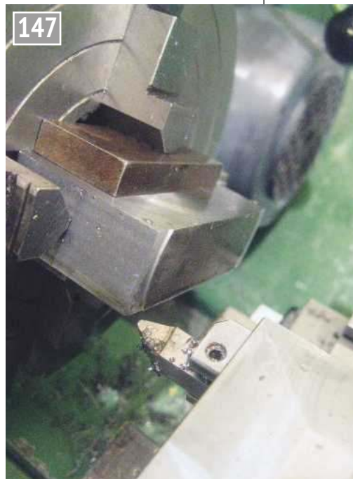
147 Facing the block to size in the four-jaw chuck. Do not use a tipped tool for intermittent cuts of this nature.
