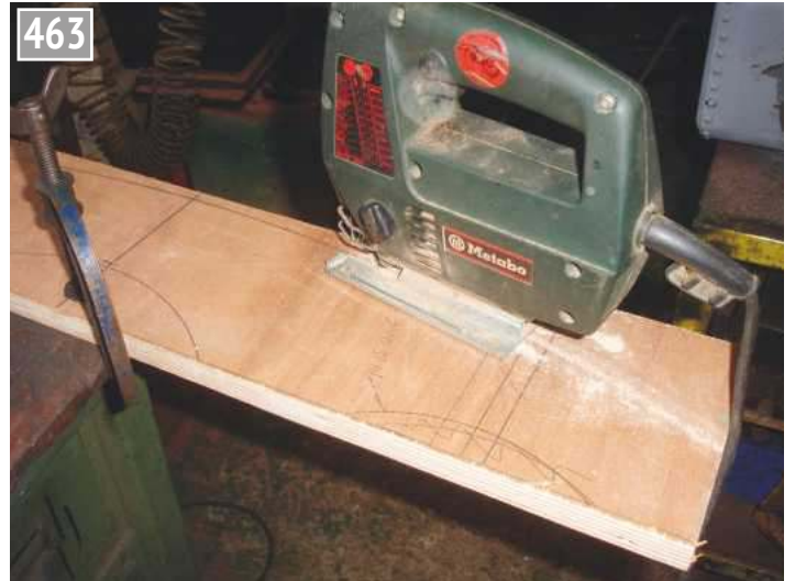
Sawing the canopy support.
