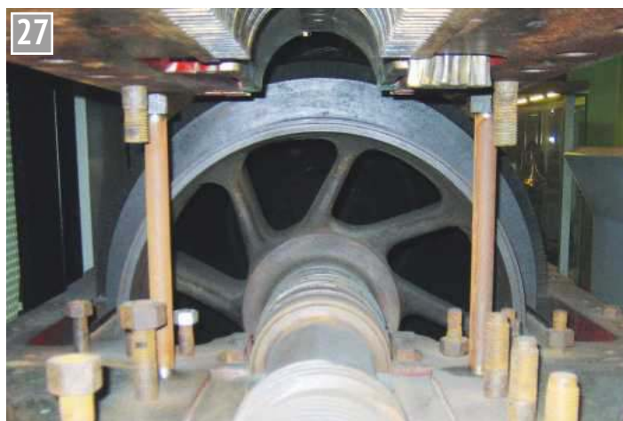
End view of the rotor in a turbine from the T.S.S. King Edward (built 1901 and now in the Glasgow Riverside Museum. Photograph used by courtesy of the museum).
