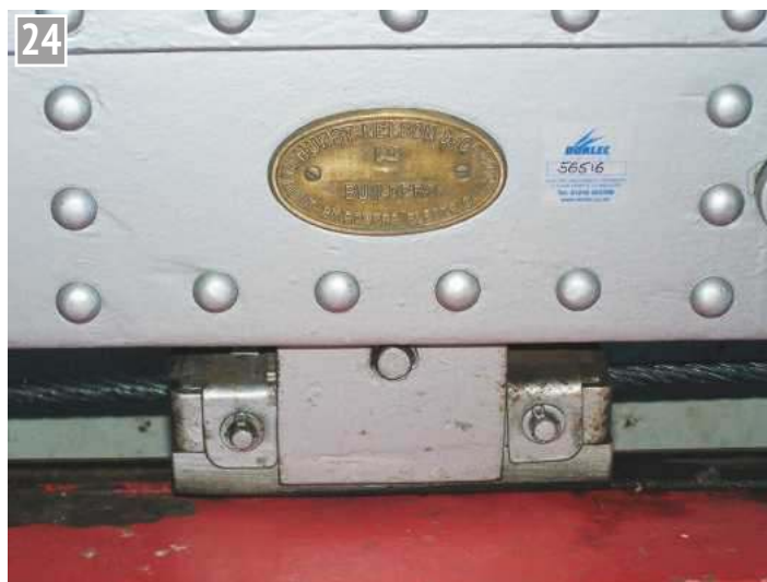
24 The slipper brakes fitted to Cars 6 and 7.
