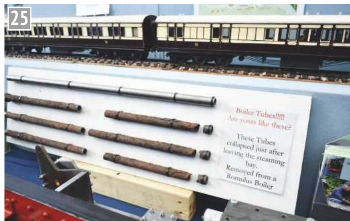
The result of poor boiler management shown on the Hereford SME display.
