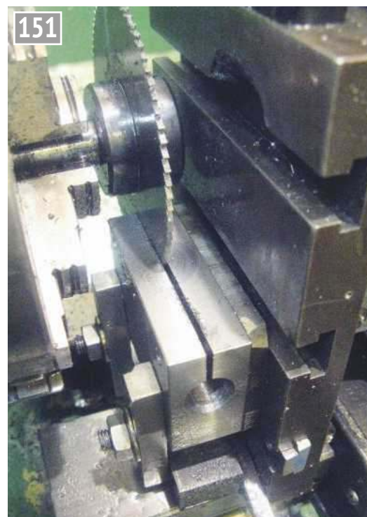
Slitting the block. This could be achieved with a hacksaw but would be untidy. Carefully check for clearance of the fixings. Speed 100rpm.
