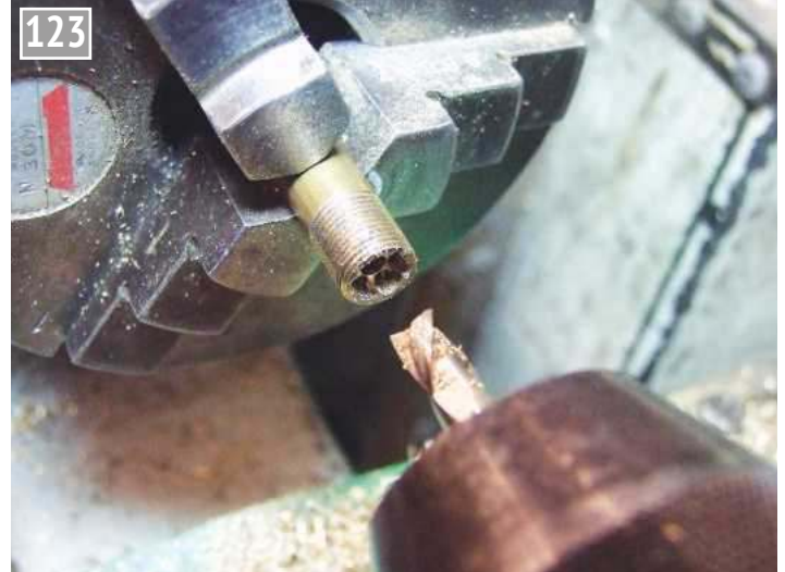
Drilling the spring seat.
