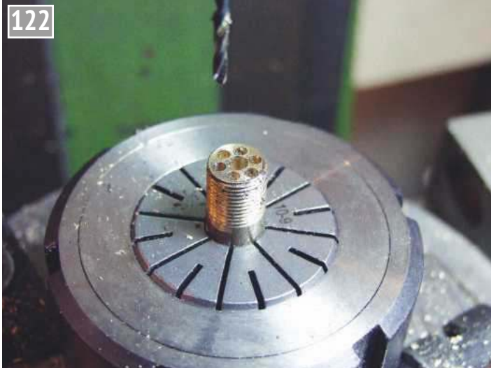
Drilling six vent holes.
