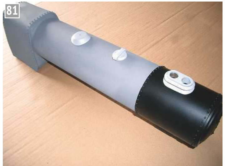
The completed boiler ready for painting.
