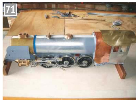
Trial positioning of the firebox wrapper.
