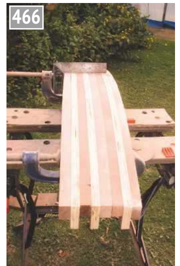
Sanding the stiffeners.
