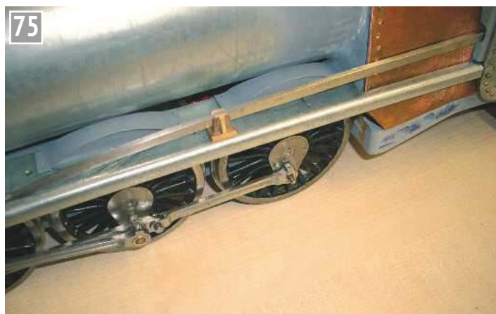
Looking down upon the reach rod support casting.
