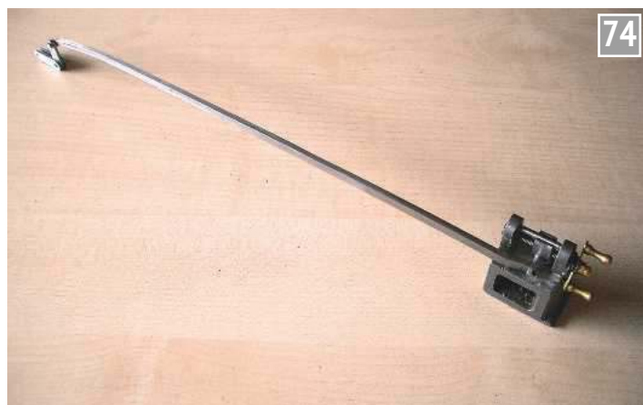
Trial assembly of the reach rod and reversing gear.
