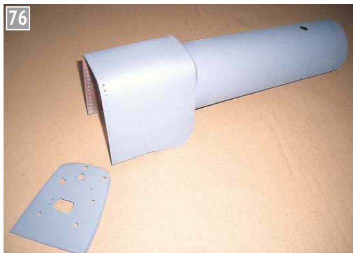
Firebox wrapper and backhead.
