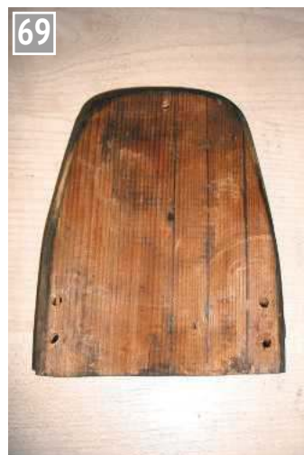
Wooden former for the backhead.
