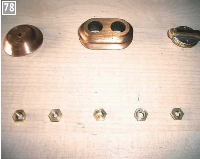
The steam dome and chimney were castings.
