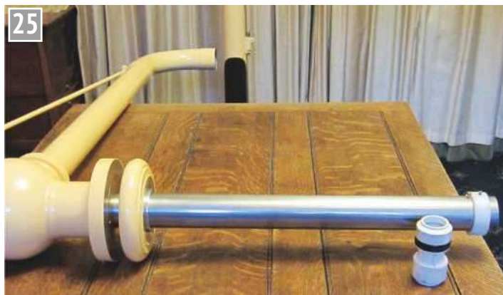
48mm inner tube of pillar with lower bearing and modified Speedfit fitting.
