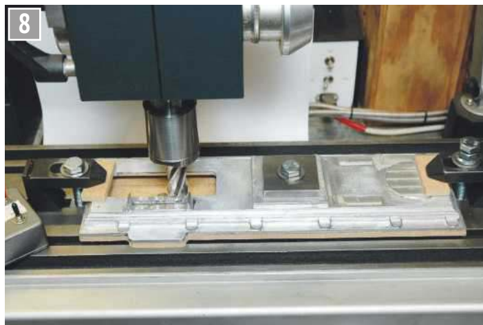
Milling the main bearing face.
