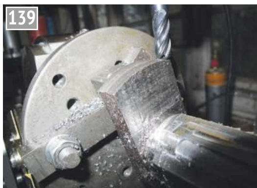
139 Roughing the radial form on the web.
