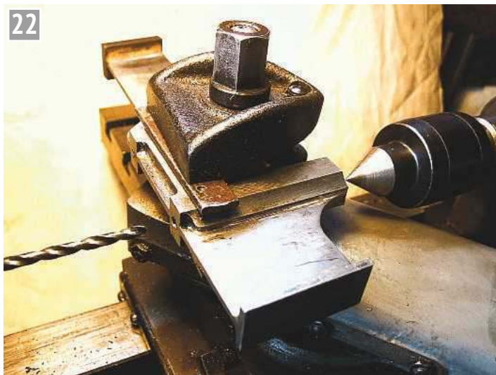
The plate set up on the lathe top slide to drill the long holes through the fabricated joints.
