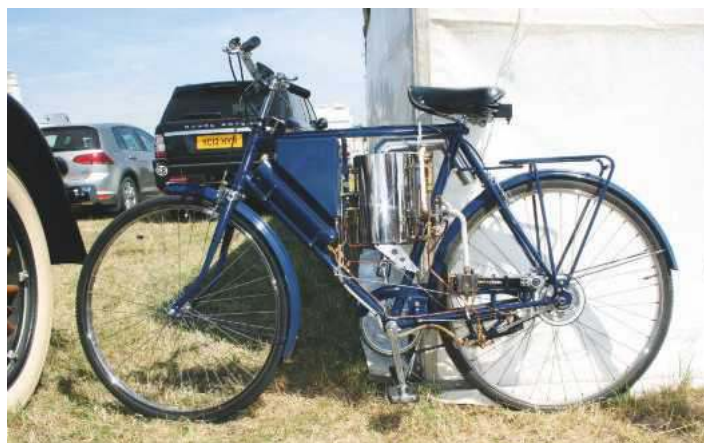
The 'Runscombe Gentleman's Steam Bicycle' was built by Mark Drake. The chrome-lagged cylinder in the middle is the steam generator, to its left the water tank and under that is the fuel tank.
