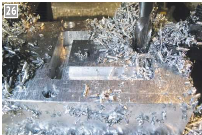
Cutting the motor pulley pocket.
