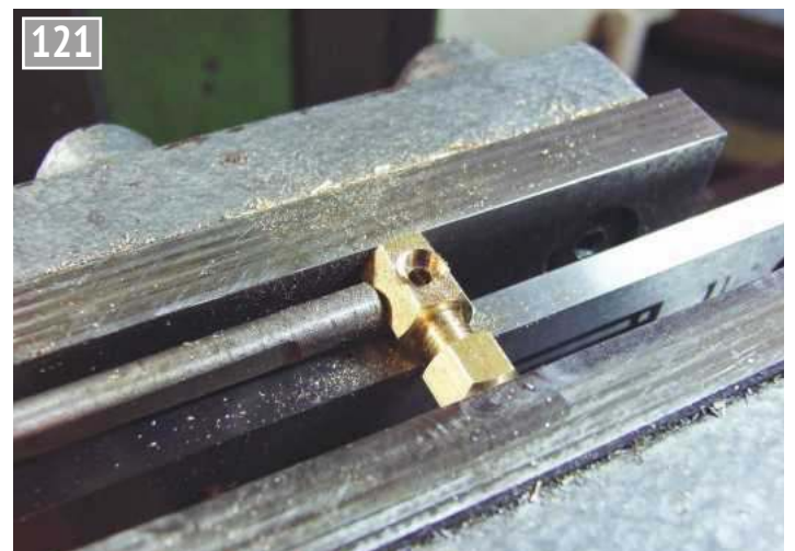
Drilling for mounting stub.
