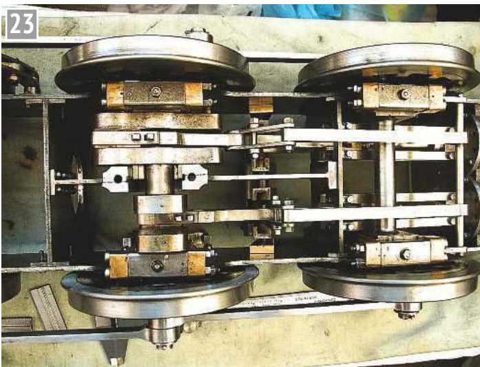
A view from underneath the chassis to show the new assembly in place with slip gauges used to check the clearance between the plate horn cheeks and the centre of the crankshaft. Note that this view also shows the wider anchor links for which thankfully I did not have add an off-set to clear the motion plate. They will have some tube spacers on final assembly.
