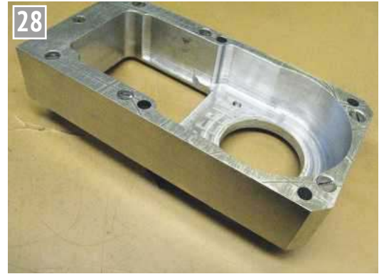
Finished new drive motor carrier.
