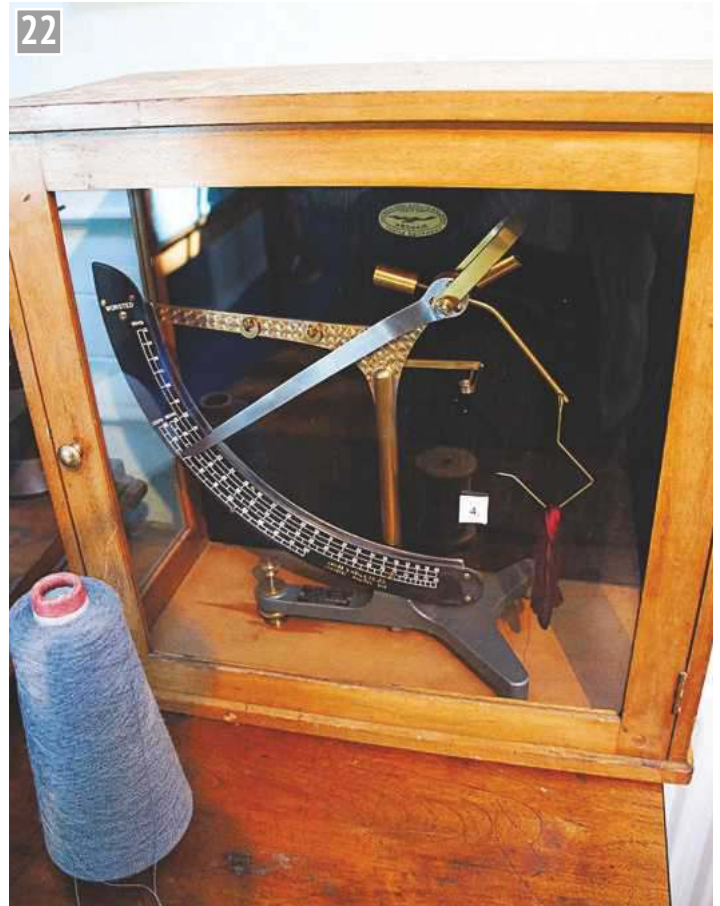
22 Thread tensometer made by James Heal of Halifax. Other textile industries used similar devices to test threads.
