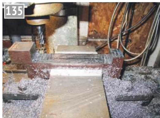
Creating service stock to carry a centre cone.
