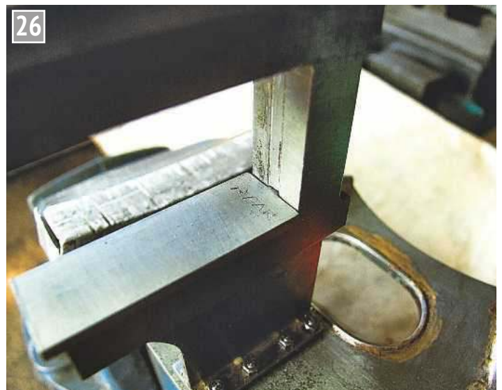
One of the keeps machined to fit in the slot showing the spigot on one end to locate in the frame plate notch. The second view shows a keep in place in its bearing housing.
