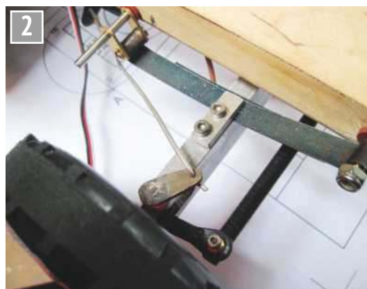
Ackermann steering and control link.
