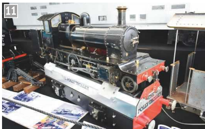
The Polly Trolley for driving 5 inch gauge locomotives on 7 1/4 inch gauge track built by Roy Hollingworth from the Nottingham SME.
