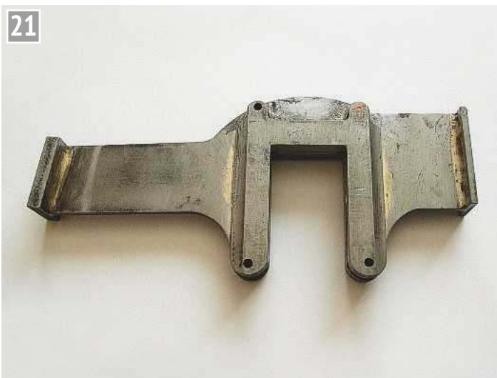
Two views of the new centre plate fabrication; the central slots can just be seen between them but they needed some careful filing in the internal corners to produce a clean channel for the keys.
