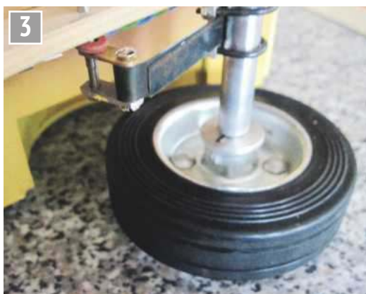
Rear axle, spring and wheel.
