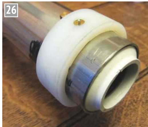
Close up – lower bearing and water fitting connection in place.
