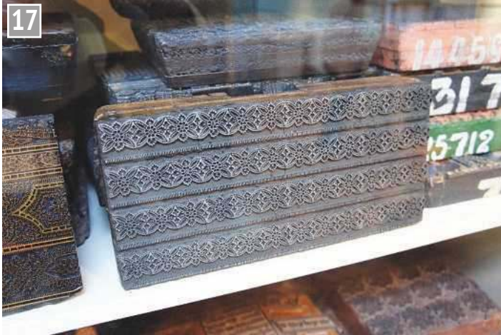
17 Carefully cut blocks used for silk printing by hand. This was highly skilled work.
