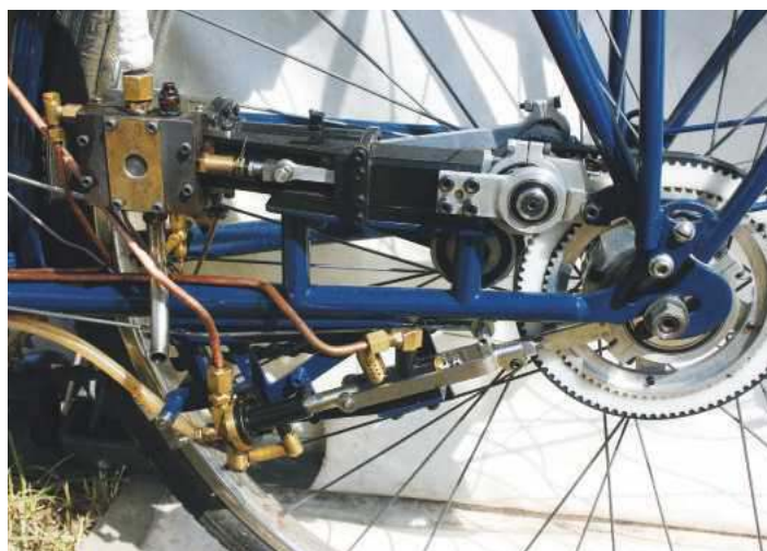
The single cylinder engine drives the back wheel via a 4.33 to 1 ratio toothed belt. Below it is the twin pumps, one delivers compressed air to pressurise the fuel tank to about 30 psi, the other being a variable delivery boiler feed pump.
