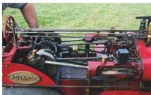
The motion on the Wallis roller, the cylinders are commercially available 7 ¼ inch gauge railway engine castings. While the full size engine has piston valves, the model has slide valves but retains the appearance of piston valves.
