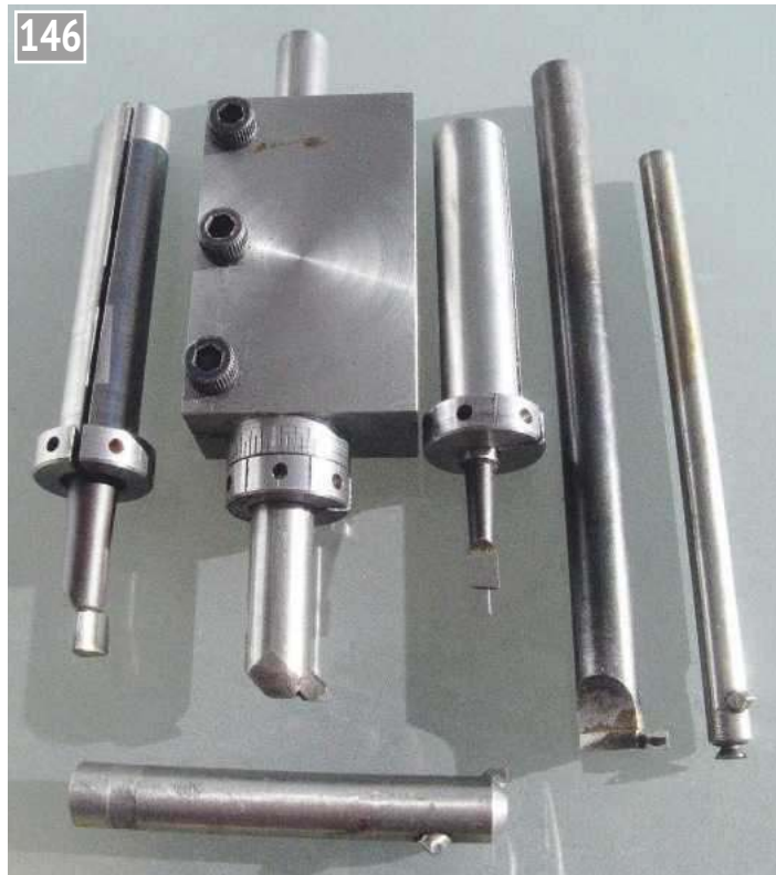
The finished boring tool kit. Bars: 10 mm commercial, angled cutter in a 10mm bar, 6mm commercial (we will make some similar in future), special for a groove at the root of a pocket, 8mm for screw-cutting and a short rigid 10mm with a central push rod to clamp the tool.
