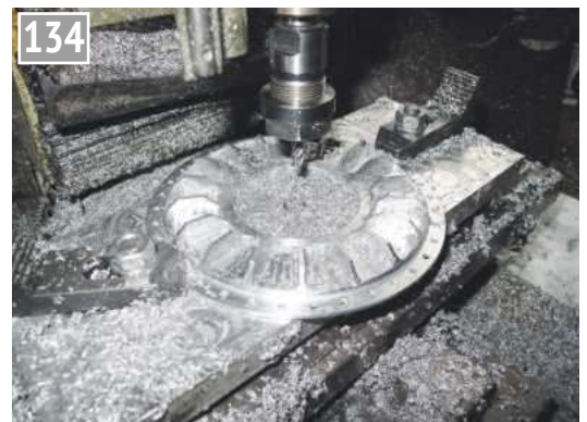
End of program and the finished pocket detail.
