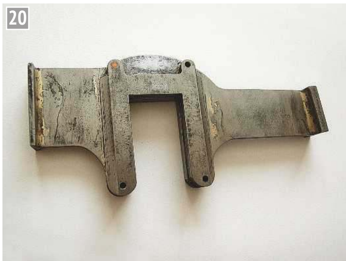
Two views of the new centre plate fabrication; the central slots can just be seen between them but they needed some careful filing in the internal corners to produce a clean channel for the keys.
