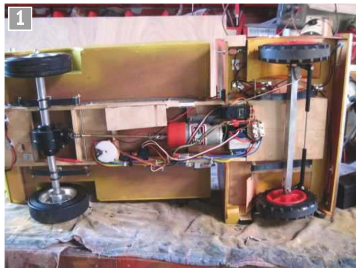
The wooden chassis of the tipper lorry.
