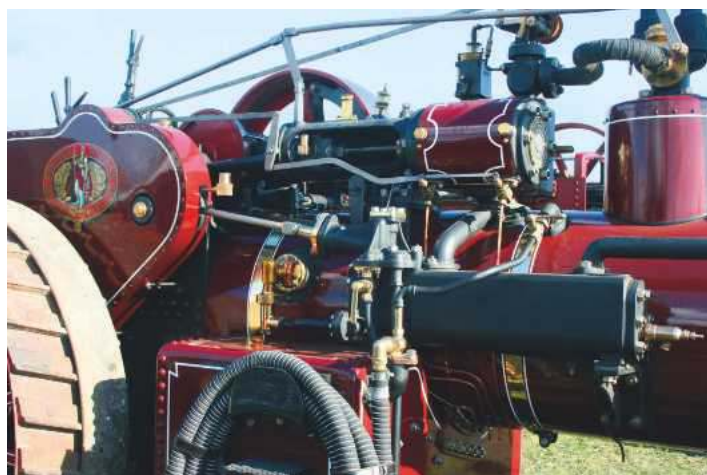
Details of the motion on the Marshall; note the geared down feed water pump and the boiler feed water heater.
