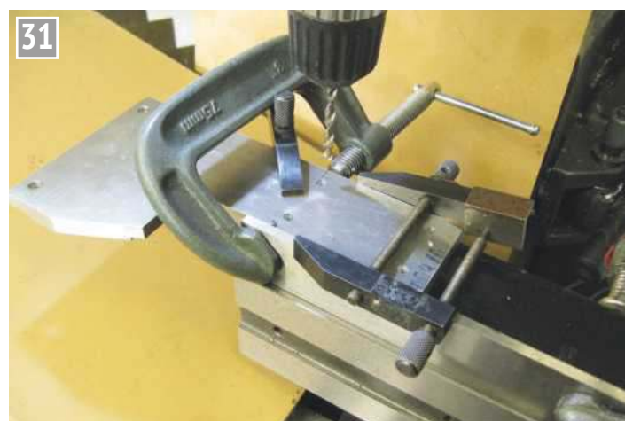
Fitting the Z side plate - note the use of a parallel for alignment.
