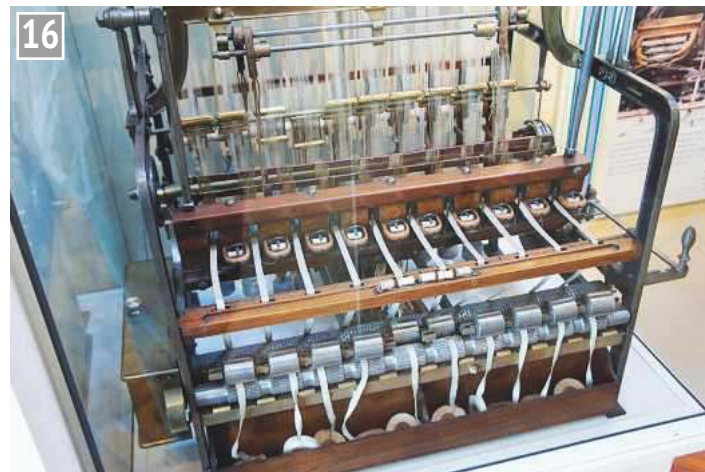
Specialist machine used to weave narrow tapes. It can weave ten at once.
