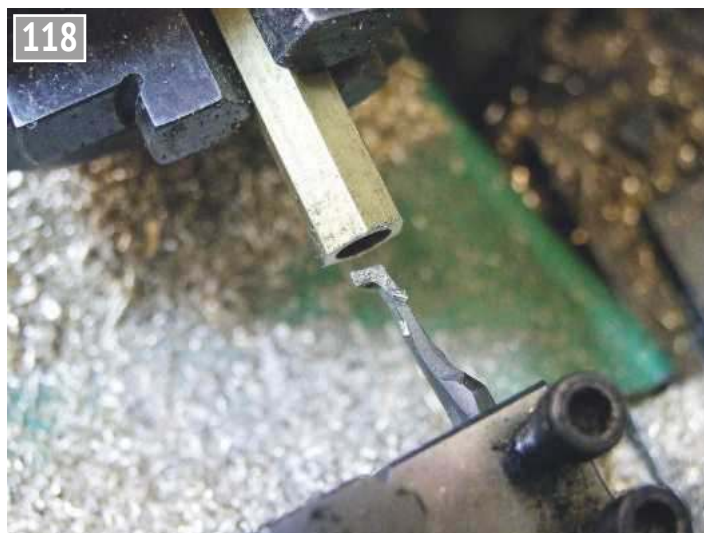
Boring internal recess.
