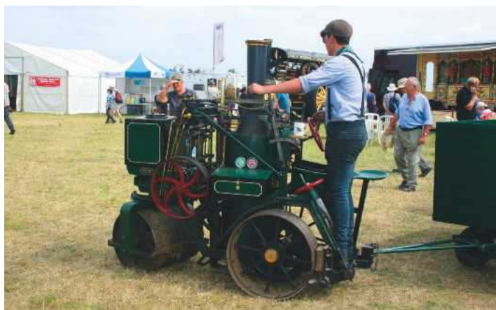
The drive train from the engine mounted ahead of the boiler is via a gear reduction on the other side and then a chain and sprocket to the back axle.
