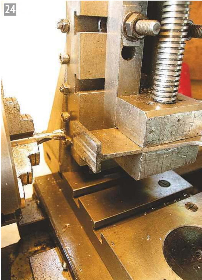
The centre stay was referenced against the lathe chuck face for alignment and the thicker flange was machined down for a 1/8 inch spacer to be added on final assembly.
