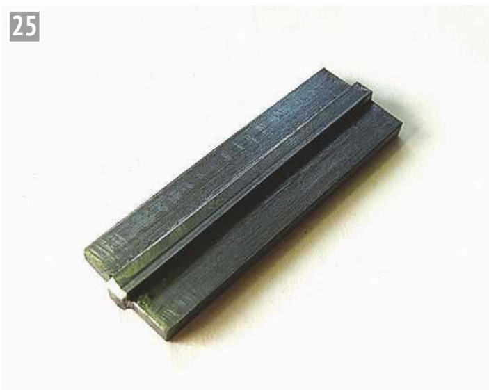
One of the keeps machined to fit in the slot showing the spigot on one end to locate in the frame plate notch. The second view shows a keep in place in its bearing housing.
