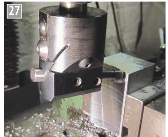
Lock body machining stage 1 (fly cutting).
