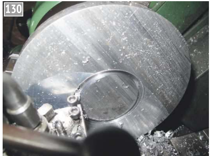
Trepanning the centre bore.
