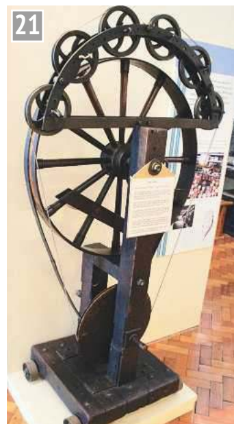
21 Cord twister for making curtain ropes. Machines also make tassels.
