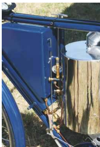
The water gauge on the bicycle; note the circular mirror behind to facilitate reading it while on the move.
