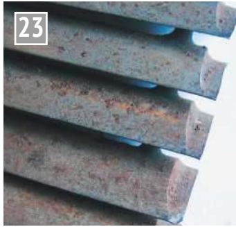
Blades with thinned tips from a Parsons turbine rotor.
