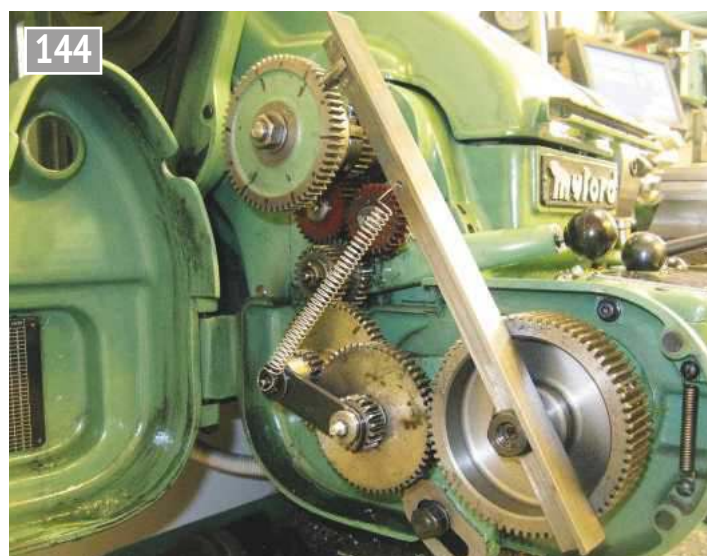
The set up for dividing in the lathe.
