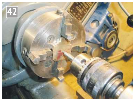
42 Drilling an eccentric strap blank.
