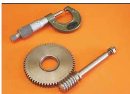
Pete Barker makes worm gears for his Versatile Dividing Head.
