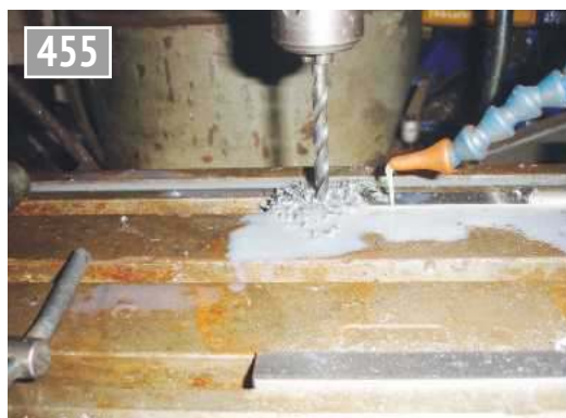
Drilling a canopy support.
