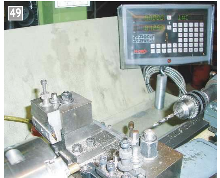
The set-up for machining the side rod bearings.
