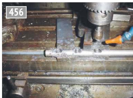
Counterboring a canopy support.
