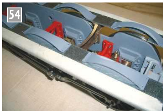
A trial assembly of the splashers.
