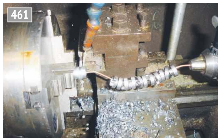
Parting off a set of canopy spacers.
