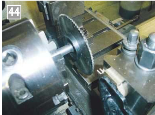
Slitting the eccentric rod end.
