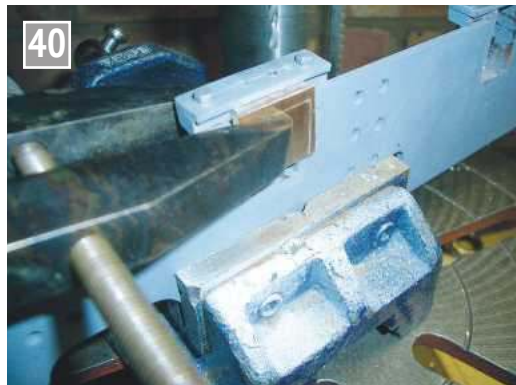
40 Spotting through for the spring rods.
