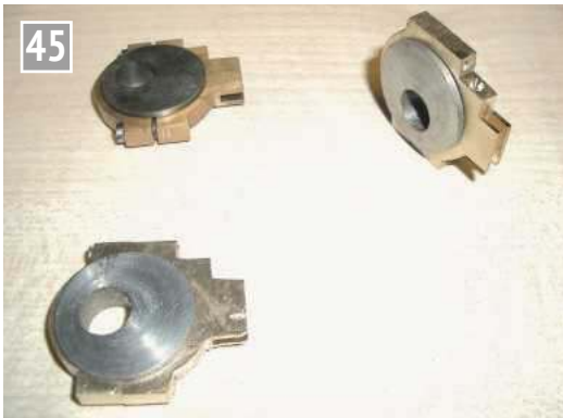
The completed eccentric straps.
