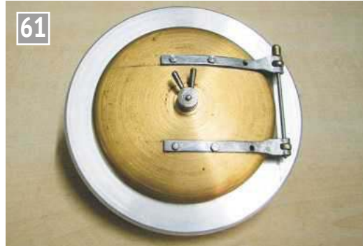
Smokebox ring with cast door and hinges in position.
