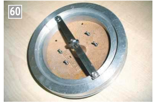
Smokebox ring temporarily assembled.
