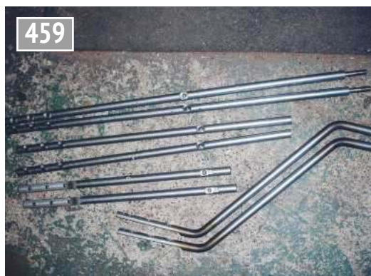
Completed canopy supports.
