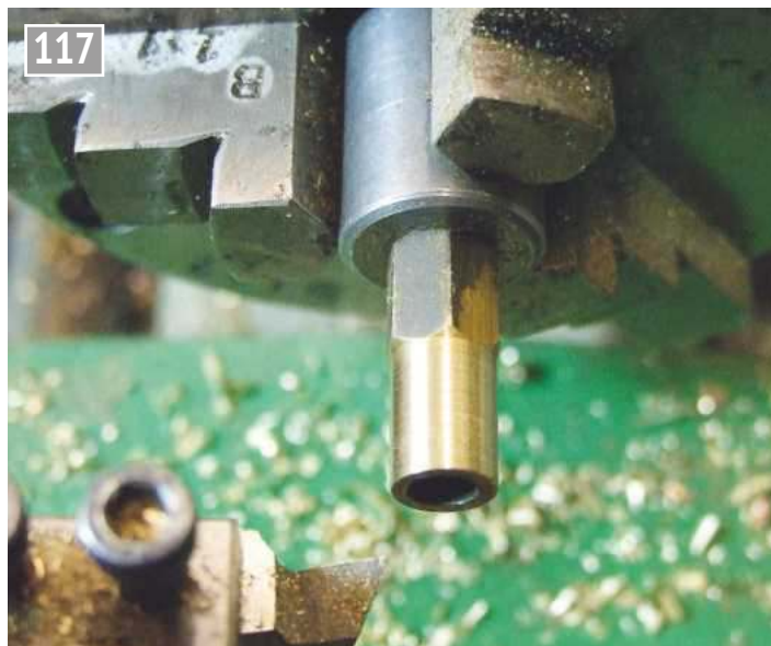
Extension parallel section turned.
