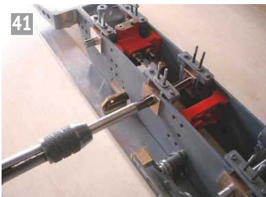
41 Bearings in situ; reaming ready for the centre axle.
