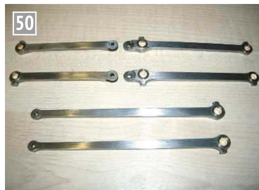
The rods complete with bearings pressed in.
