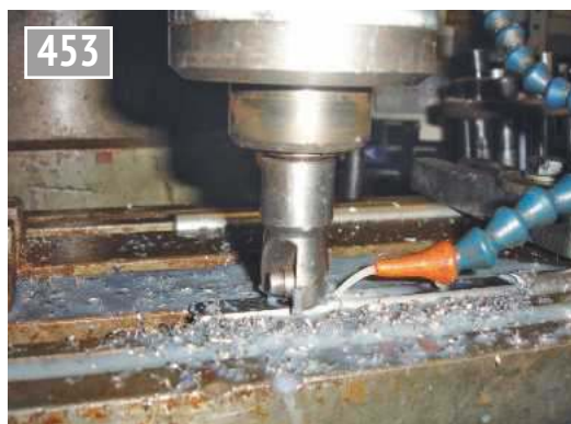
Milling a canopy support.
