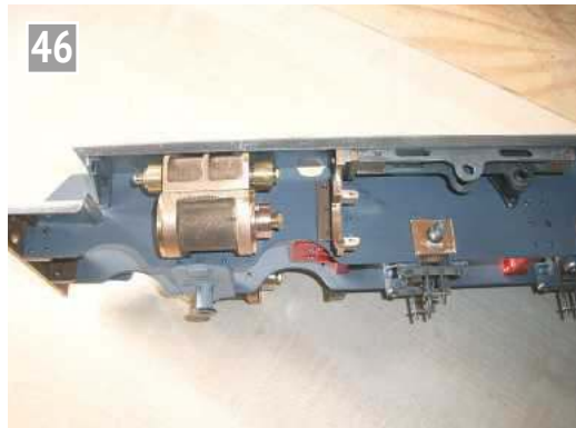
The cylinders fixed in position.
