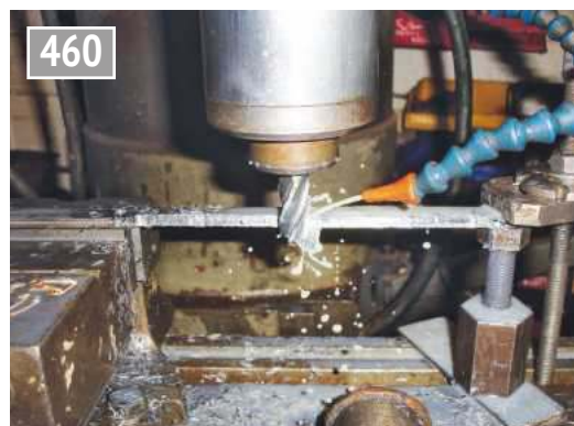
Milling the cross braces.
