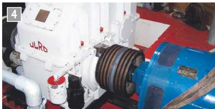
The traction motor and gearbox for the lower section.
