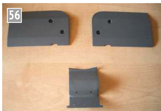
Smoke deflectors in primer.
