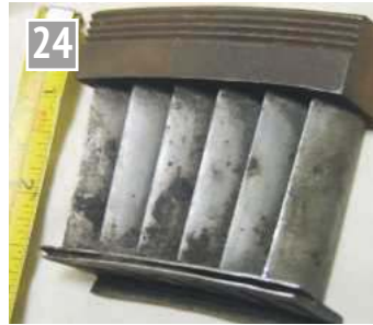
Blades with shroud for end-tightening from a Parsons turbine cylinder (i.e. casing).
