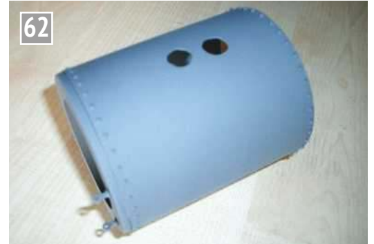
The smokebox, with chimney holes, in primer.
