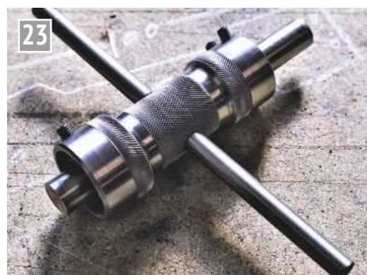
Tom Williams made this double ended die holder as a first attempt at model engineering and toolmaking.
