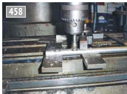
Counterboring another canopy support.
