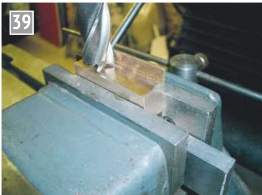
39 Milling the main wheel bearings.
