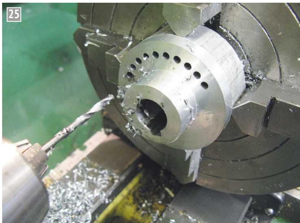
New motor pulley, note clean seating for clocking in the four jaw chuck later.
