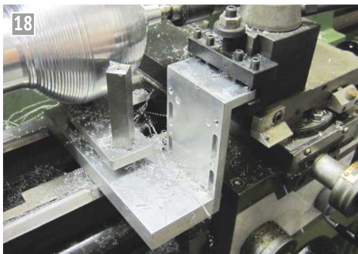
Spherical turning tool in action.
