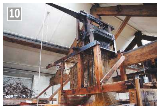
Belt of Jacquard cards. Each card is presented to a cylinder controlled by the yolk mechanism just visible. Needles then insert into card holes to determine which heald to lift, thereby making a pattern.
