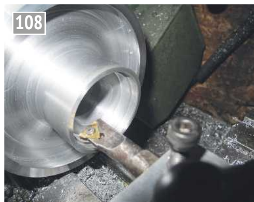
Screw cutting the locking nut thread.
