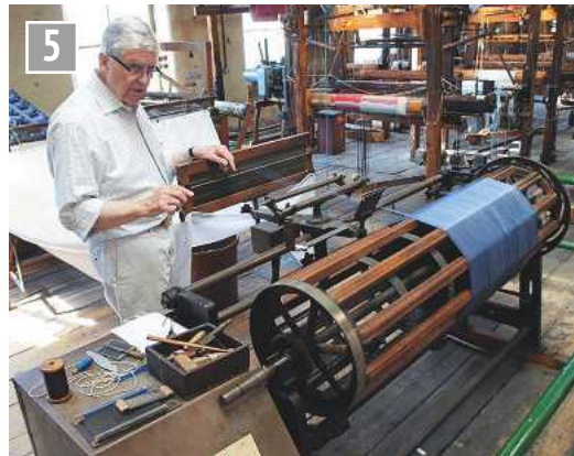
5 Winding silk thread (barely visible) on to the warping beam. Threads are then transferred to the weaver's beam.
