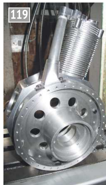
Producing the finished size outlet bore.
