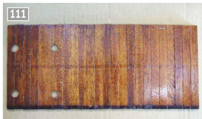
Lagging strips all cut and varnished.
