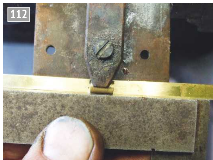
Setting up banding on jig.
