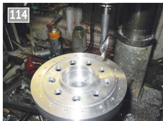
Pilot drilling the thrust box through holes.
