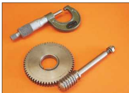
Pete Barker makes worm gears for his Versatile Dividing Head.
