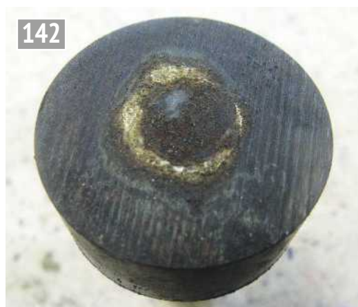
The penetration of silver solder on the face of the body.
