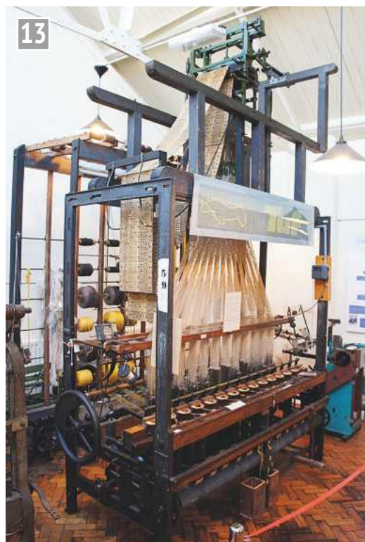
Modern Jacquard looms are power driven. This one was used for weaving several small tapes at once as labels.
