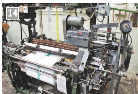
'Jacqualette' controls visible top right on a loom at Queen Street Mill Burnley, used for simpler patterns, in this case lettering. The 'dobby' loom used an even simpler control system with wooden 'cards'.
