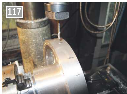
Centring the hole position.
