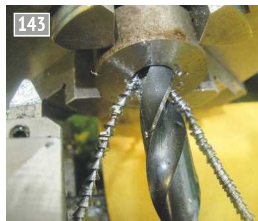
Drilling the 11.5mm hole for fabrication, showing how a sharp drill cuts.
