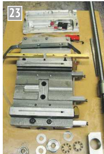
23 Finished saddle components.
