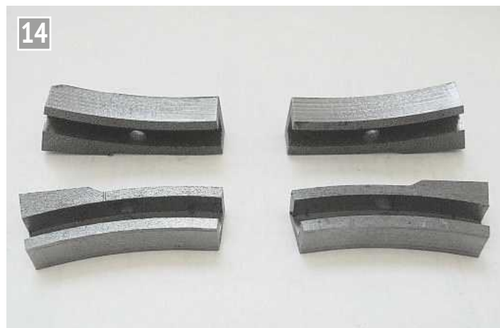
The set of handed slide shaft slides milled in steel with a CNC mill by a kind colleague. They required cleaning-up prior to assembly but the accuracy was superb.
