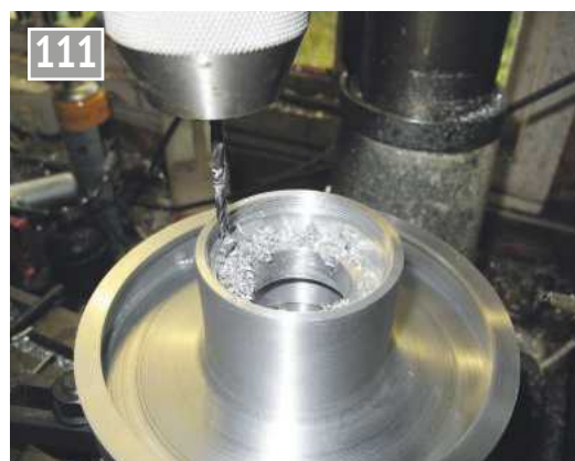
Drilling the first three hole pattern.
