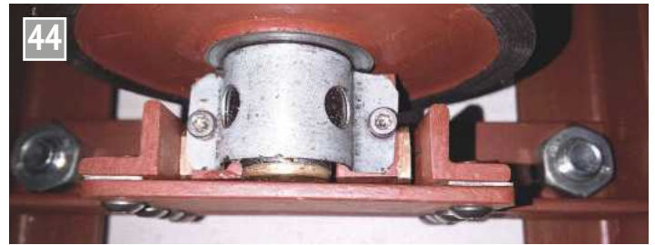
Using shims to restore squareness to the axles.
