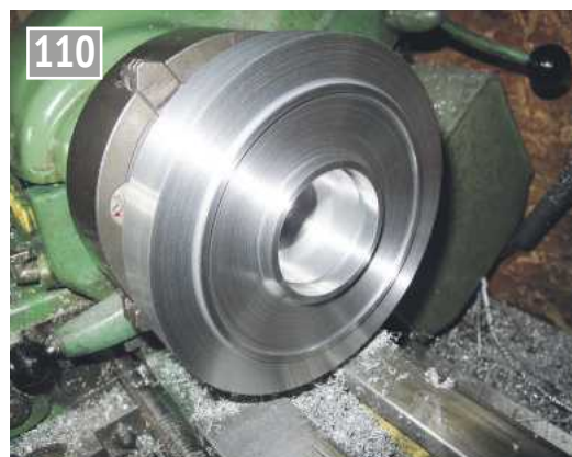
Front face detail finish turned.
