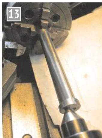
The slide shaft material set up in the lathe to turn the oval section.
