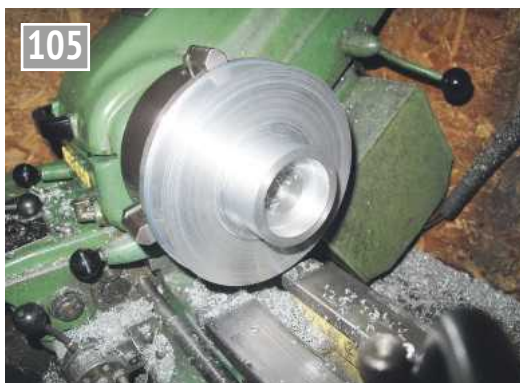
Roughing out the back diameters.
