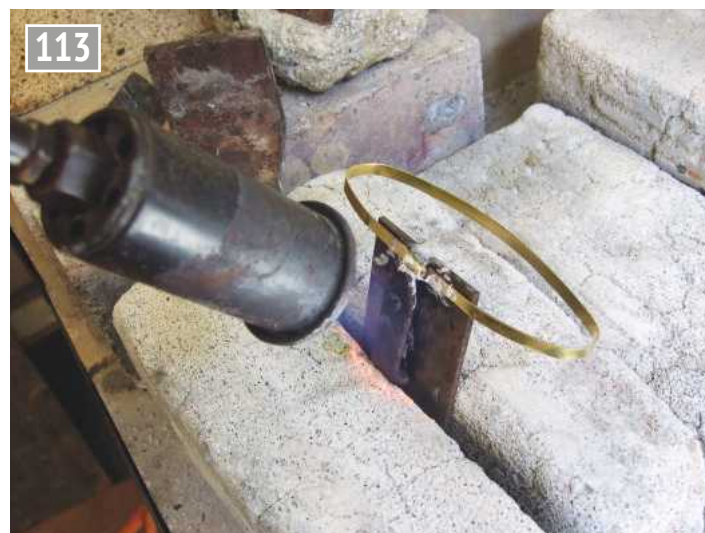
Setup for silver soldering.
