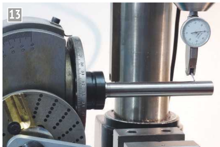
Alignment of dividing head to horizontal position.
