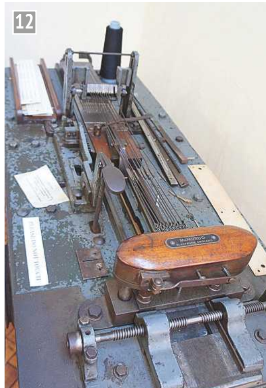
A MacMurdo repeater used to copy or replace damaged cards.
