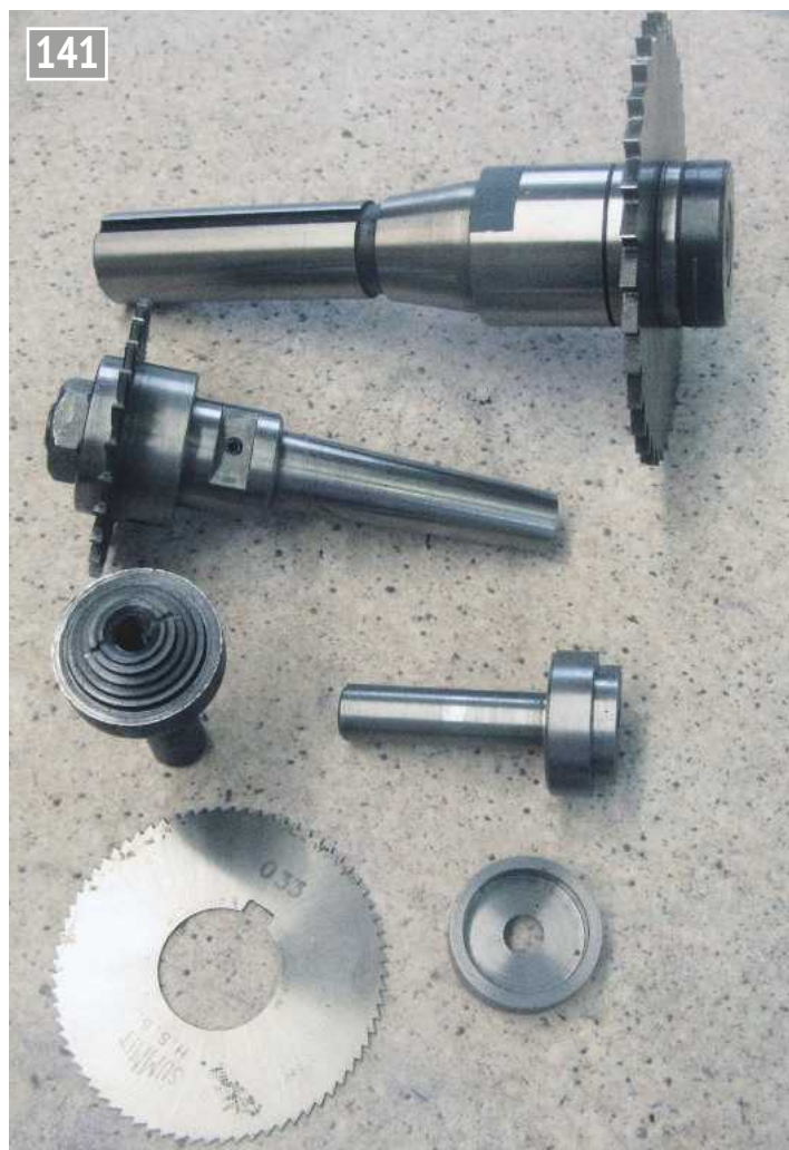
Slitting saw arbors, Morse taper, R8, ours and the failed telescopic type.
