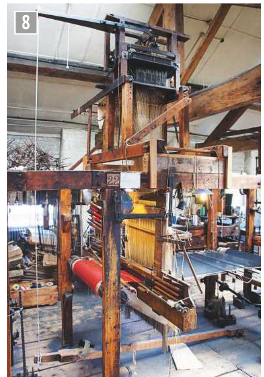
8 Classic hand operated Jacquard loom. The Jacquard mechanism controlling the weave is at the top. Weaver's beam to the right, finished cloth to the left.
