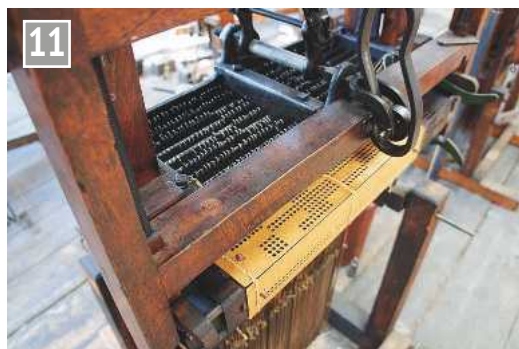
Example of card on cylinder. Needles penetrating the card allow the gripper bar controlled by a treadle to lift the hooks holding healds. Weights visible below hold healds in tension.
