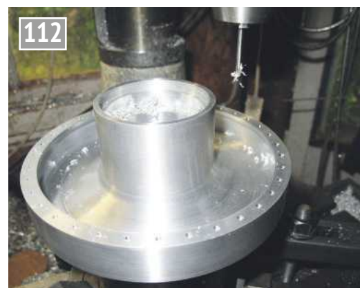
The thrust box cover plate securing holes.
