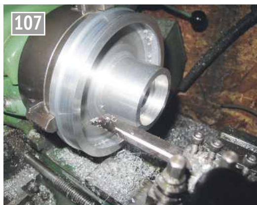
Turning the internal undercut area.
