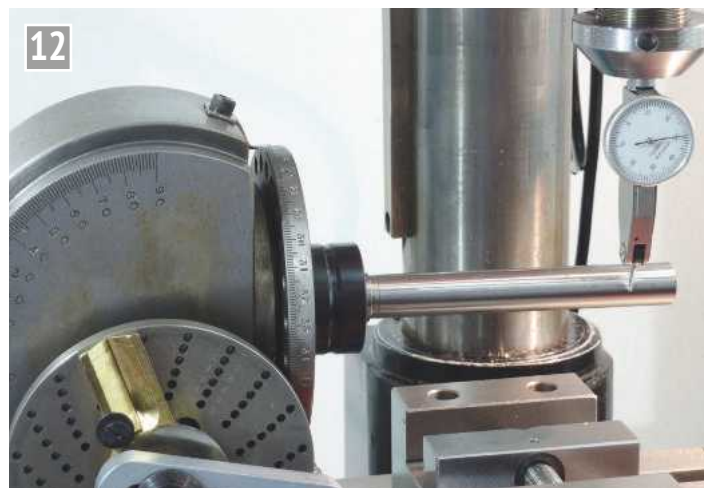
Alignment of dividing head to axis.
