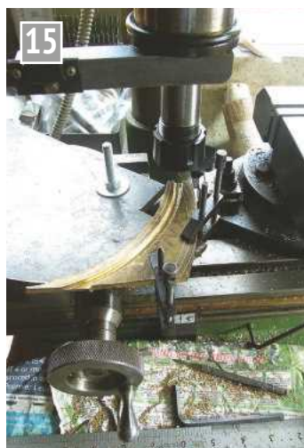
The author using a rotary table with a hefty plate bolted to it to hold some bronze plate for milling the slide slippers. A small radial offset also allowed the four pivot holes to be drilled and reamed.
