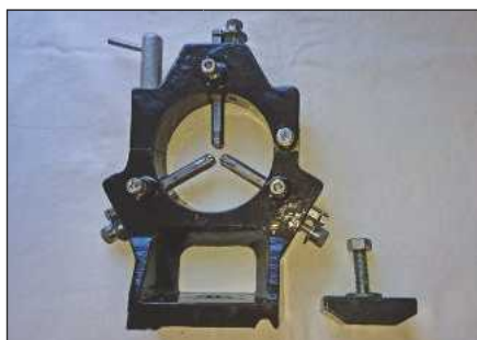
Chris Gill makes a Fixed Steady for a Harrison lathe that can be easily adapted to suit many other machines.
