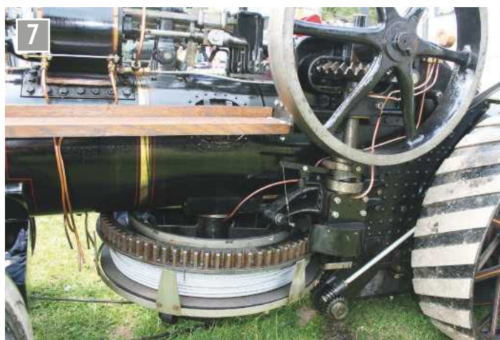
The bevel gear and reduction drive to the winding drum under the boiler.
