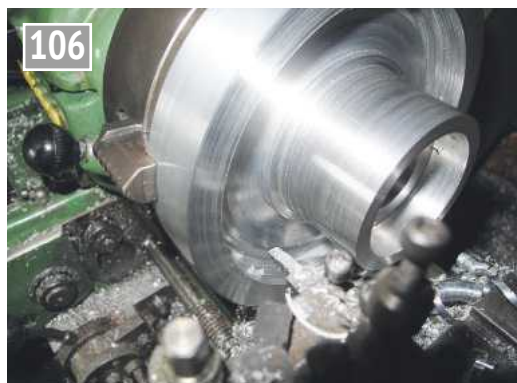
Establishing the transition point with a face grooving tool.
