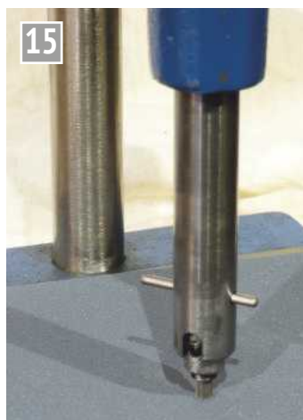
Polishing the cutting face of broach.
