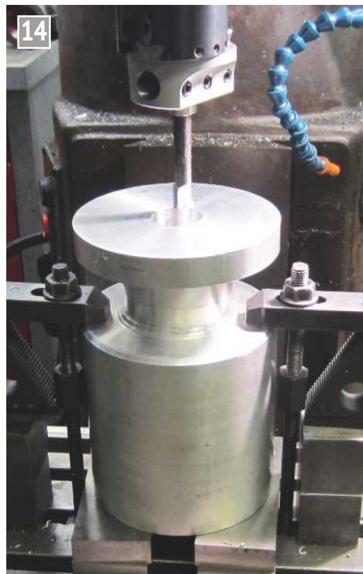
First boring of head spherical component.
