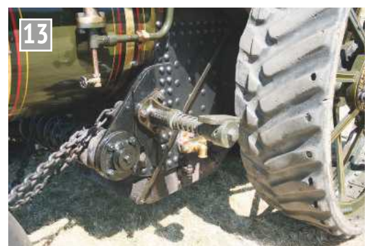
Note the spigots to fit the rear roller scrapers.
