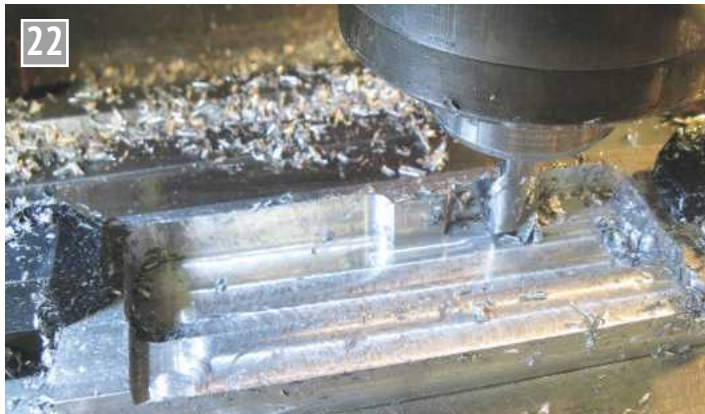
22 Milling the limit switch housing, shortened later in redesign, as only one micro switch is needed.
