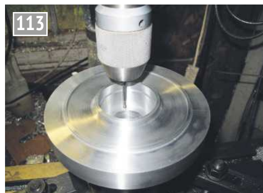
Reversing the thrust box and re-establishing centre position.
