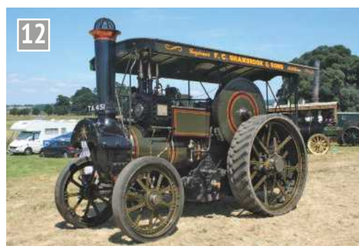
Burrell 3381 built in 1912 as a convertible, being provided with two sets of wheels, one for road rolling and the other for general haulage work.
