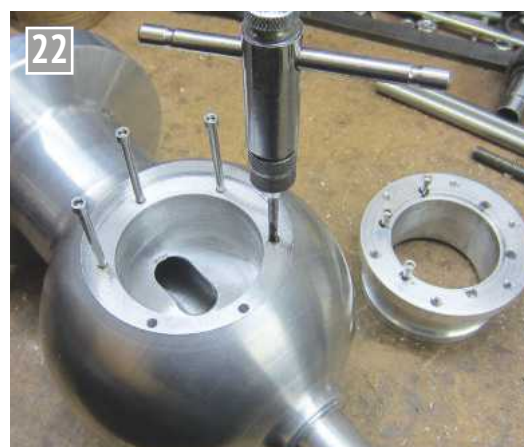
Method securing collar and sphere components.
