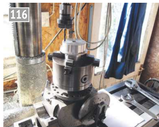
Producing the holding and locating fixture.
