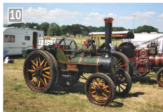
This single cylinder Burrell built from parts from a variety of sources was a great credit to the builder.
