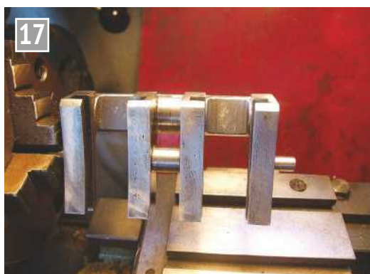
The silver soldered slide shaft assembly being checked on the lathe for concentricity. The extra clearance for the valve gear was started by milling but completed with a file, due to the close proximity of the slides themselves.
