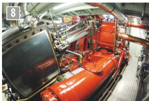
Low pressure side of engine. The horizontal cylinder is a feedwater heater and beyond that is the jet condenser.
