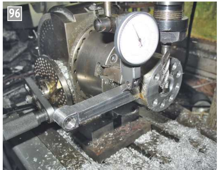
Setting the second roughing operation.
