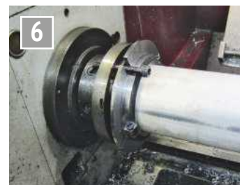
Taper turning between centres - driven clamp plate for workpiece.
