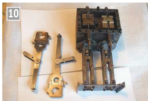
Two views of the connecting rod assemblies with their straps and bearing bronzes added and with the two pairs of taper keys fitted through the straps. The two pairs of jack links have also been added and lined up as described in the text.
