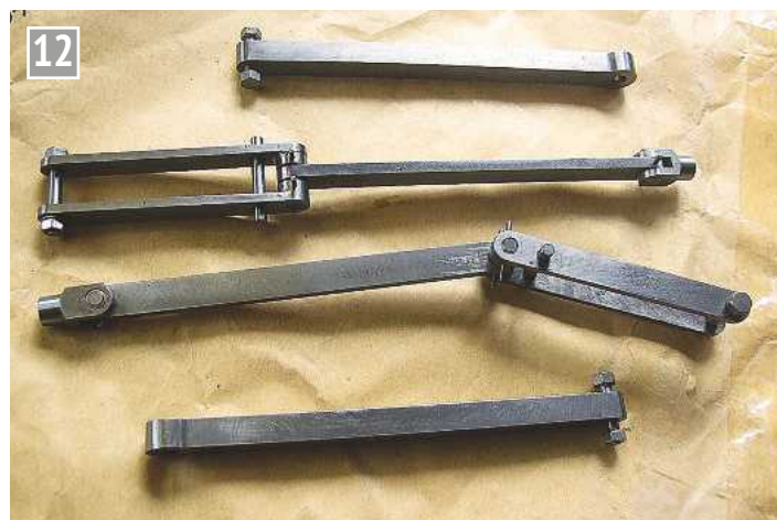
Here are the rest of the valve gear parts which can be identified from the layout diagram. They were laser cut from the most appropriate thicknesses of steel and shaped where necessary then given the usual clean dull finish.
