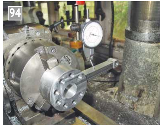
Clocking the angled side of the master rod.
