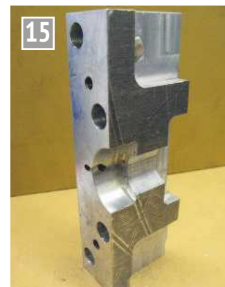
Fig 15 Finished X table end mounting. Complicated! Note: the clearance for the bearing housing is cut later.
