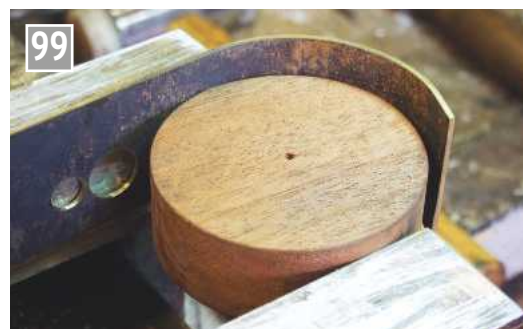
Bending at one end.
