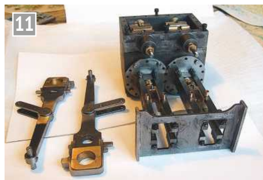
Two views of the connecting rod assemblies with their straps and bearing bronzes added and with the two pairs of taper keys fitted through the straps. The two pairs of jack links have also been added and lined up as described in the text.
