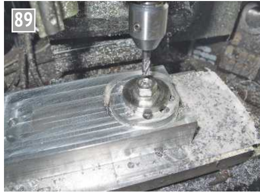
Initial generation of the body.
