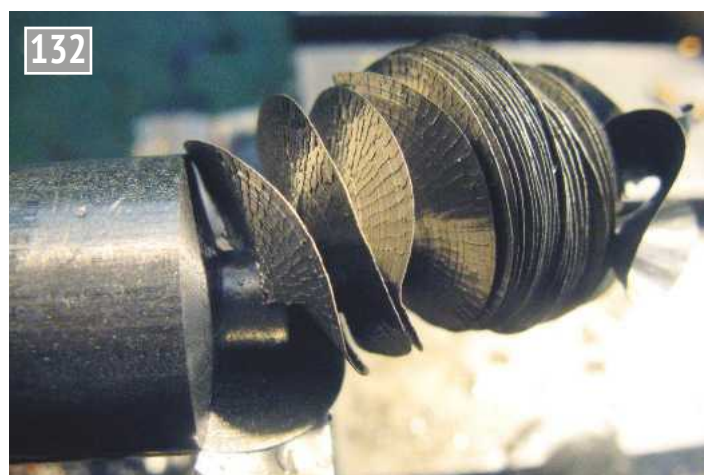
Tool B in action - note the shear planes on work and swarf; tool A shows similar shear patterns.
