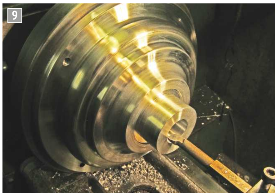
Pillar base boring for water feed pipe.
