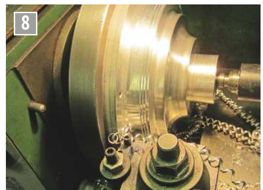
Rough profiling of pillar base.
