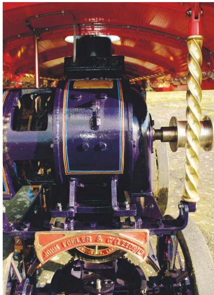
Front view of the dynamo.
