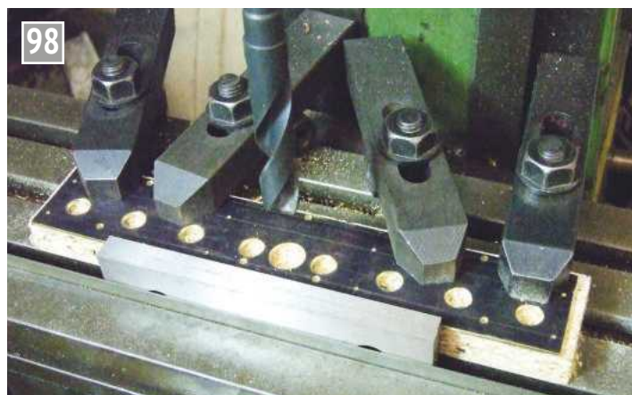
Drilling firebox completed.
