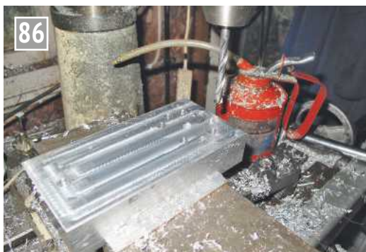
Pilot drilling the pivot positions.
