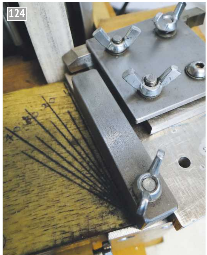
Flip tool bit onto its back edge to grind the side rake 16 degrees and back rake of 8 degrees.
