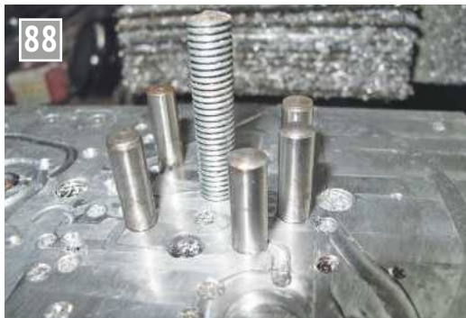
The locating nest of dowel pins.
