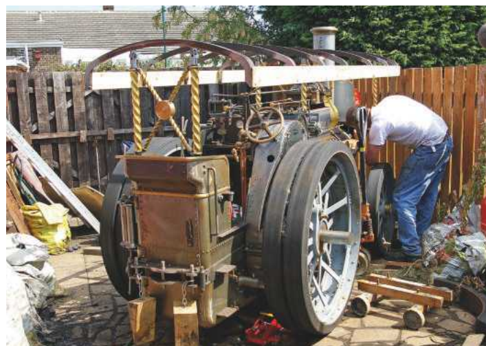
Fowler canopy frame in place (photo Martin Young).
