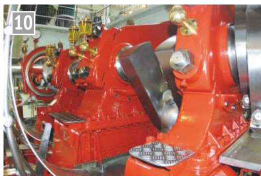
The substantial main bearing housings and the crank.
