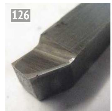
Finished and honed steel roughing tool.
