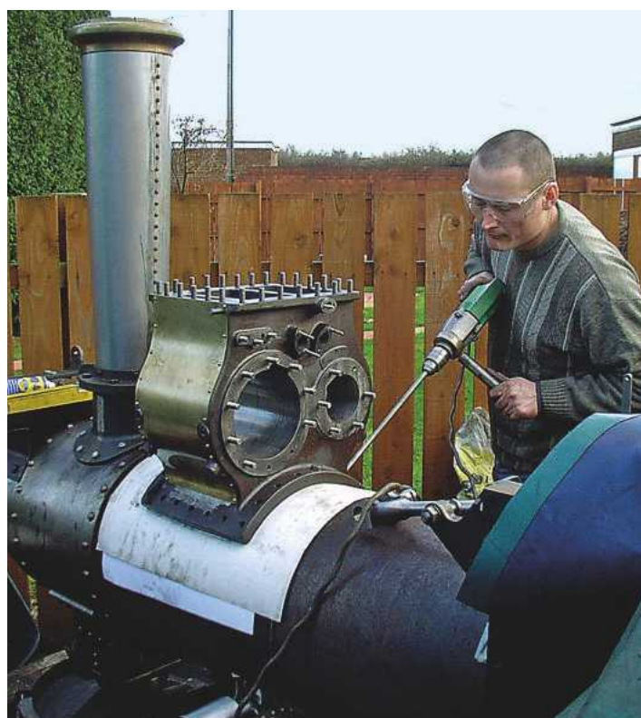
Drilling the boiler for the cylinder block fixing studs (photo Martin Young).
