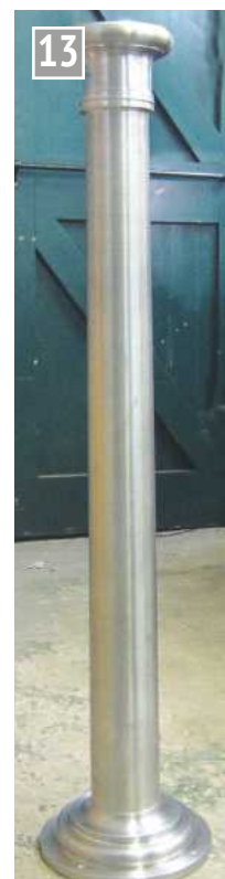
Assembled Water Crane pillar.
