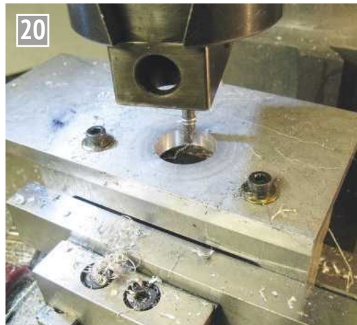
20 Boring the X motor plate and table end for the thrust bearing housing.
