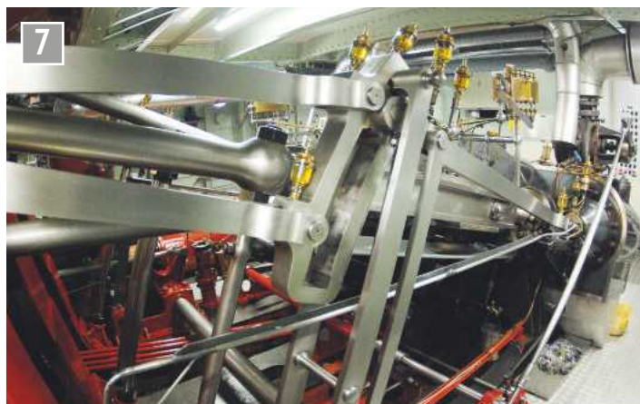
The Stevenson link motion. Since the engine turns slowly, the oilers can go around with the motion.
