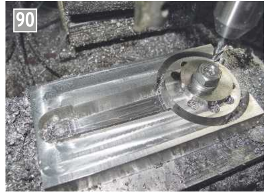
Finish milling the master rod to the depth of its bottom face.
