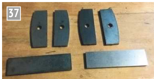
The laser cut parts for the coupling block.
