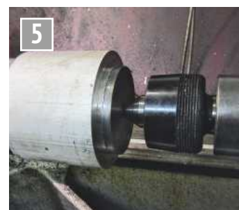
Taper turning - top hat and tailstock revolving centre.
