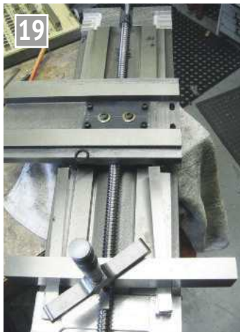
19 Setting X screw heights. Note the plate for X nut carrier bolts.
