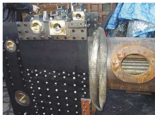
Boiler and firebox (photo Martin Young).
