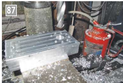
Rough drilling the central bore.
