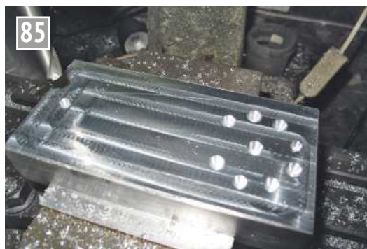
Pitching out the centre positions on the master rod billet.
