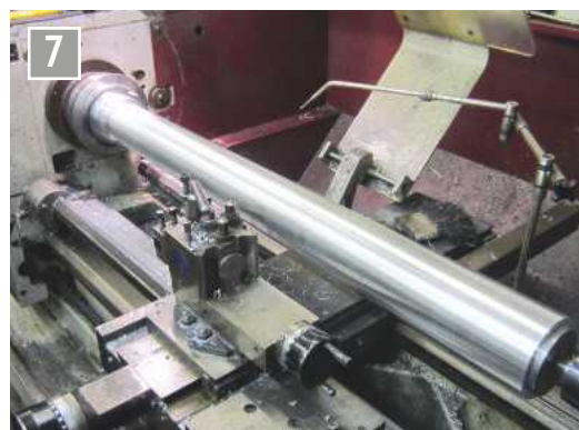
Final turning between centres of column.
