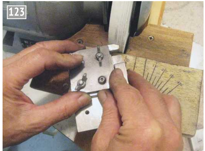
Side clearance at 8 with 16 degree approach angle.
