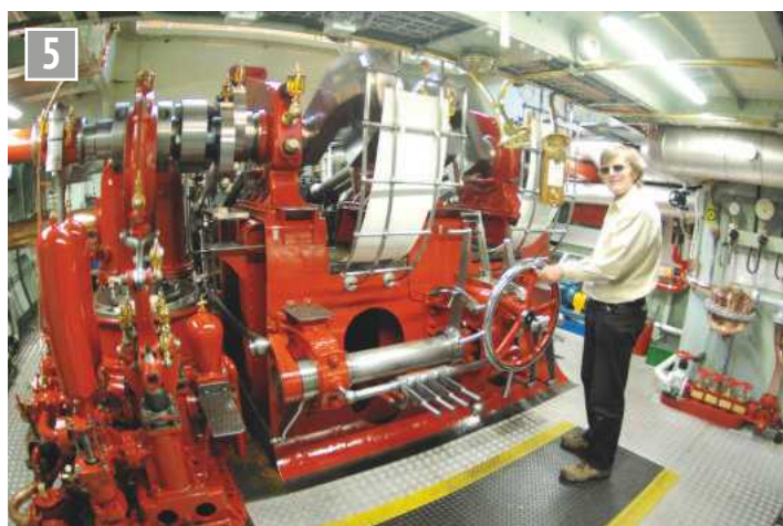
The writer at the controls. The large wheel is the reversing gear. Air and feed pumps to the left.
