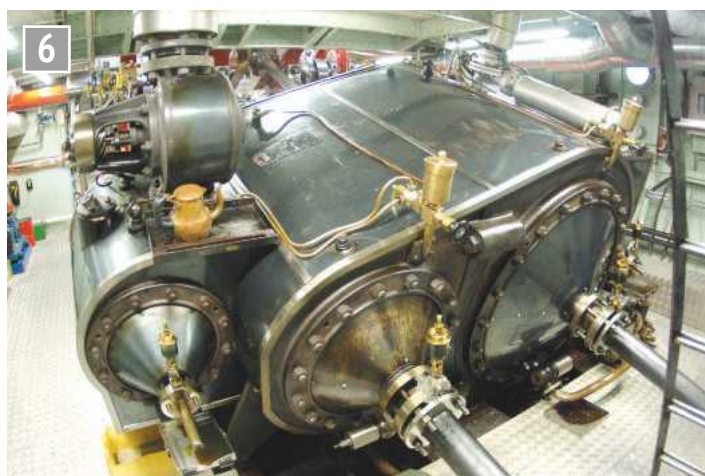
Cylinders clad in Russian Iron. Piston valve on high pressure and slide valve on low pressure.
