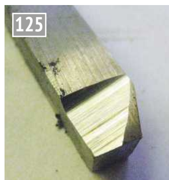
The partly formed top face.
