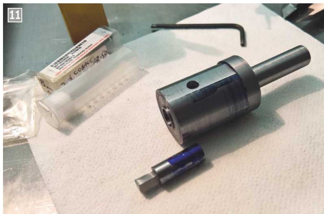
The finished tool and broach.
