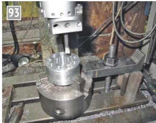
Finishing the through bore.
