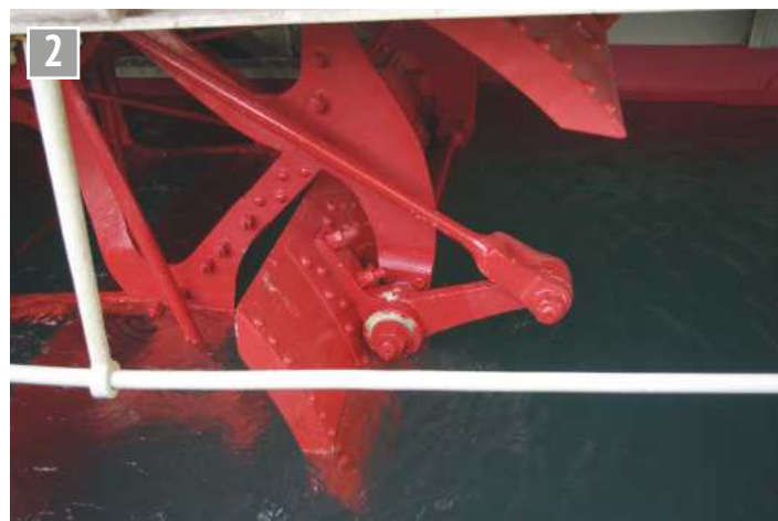
2 Feathering paddle wheel. The engine was turning slowly to warm up.
