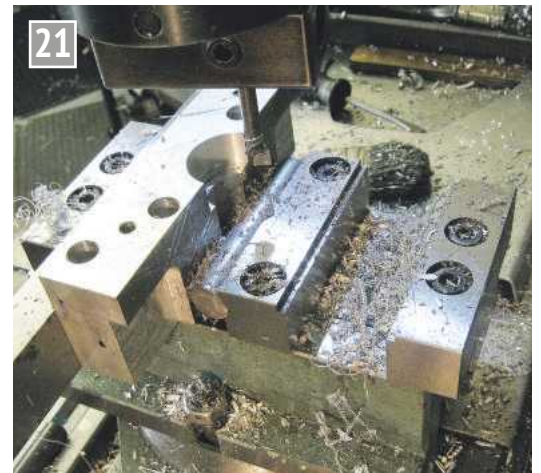
21 Mounting plate removed to add adjustment clearance - increase the bore diameter or move spindle towards the top of the table end.
