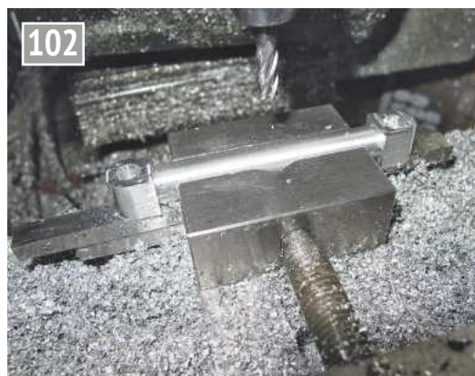
Milling the two ends and bores.
