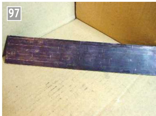
Firebox marked out.
